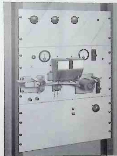
Fig. 12—Photograph of the complete recorder as mounted on a relay rack.
