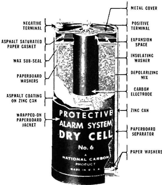
Fig. 30-18. Cross-sectional view of the dry cell.
