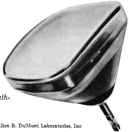
Fig. 43-12. Commercial 21-inch cathode-ray tube.
