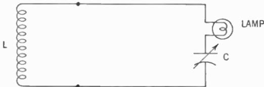
Figure 465. Circuit of the absorption frequency meter.
