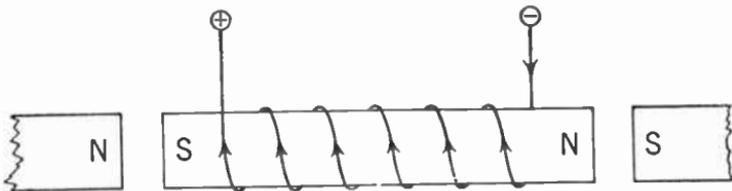
Figure 247. The electromagnet, having rotated a half turn, now comes to rest with unlike poles facing each other.
