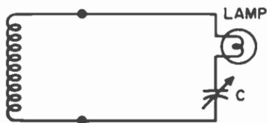
Fig. 40-24. Circuit of the absorption frequency meter.
