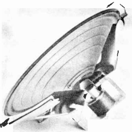
**Fig. 22-6.** *Permanent-magnet dynamic speaker.*
