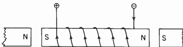
**Fig. 30-22.** The electromagnet, having rotated a half turn, now comes to rest with unlike poles facing each other.
