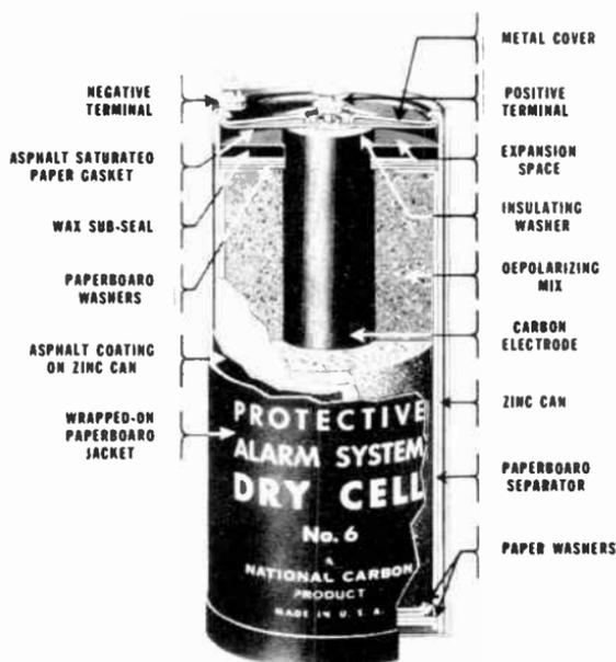
Fig. 29-18. Cross-sectional view of the dry cell. (Courtesy of National Carbon Co., Inc.)
