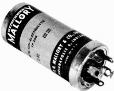
Fig. 18-16. *Electrolytic capacitor.*
