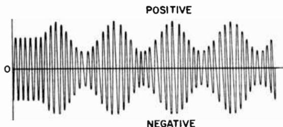
Fig. 9-8. This waveform of alternating current is set flowing in the antenna-ground system when the modulated radio wave shown in Figure 9-7-C passes across the antenna of the receiving set.
