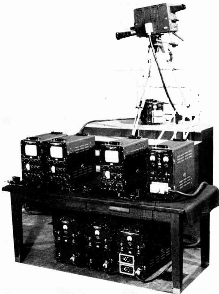
An image orthicon camera chain. The camera is on the upper level. Monitors and control equipment are on the table. The units on the floor are power supplies. (Courtesy of Allen B. Du Mont Laboratories, Inc.)
