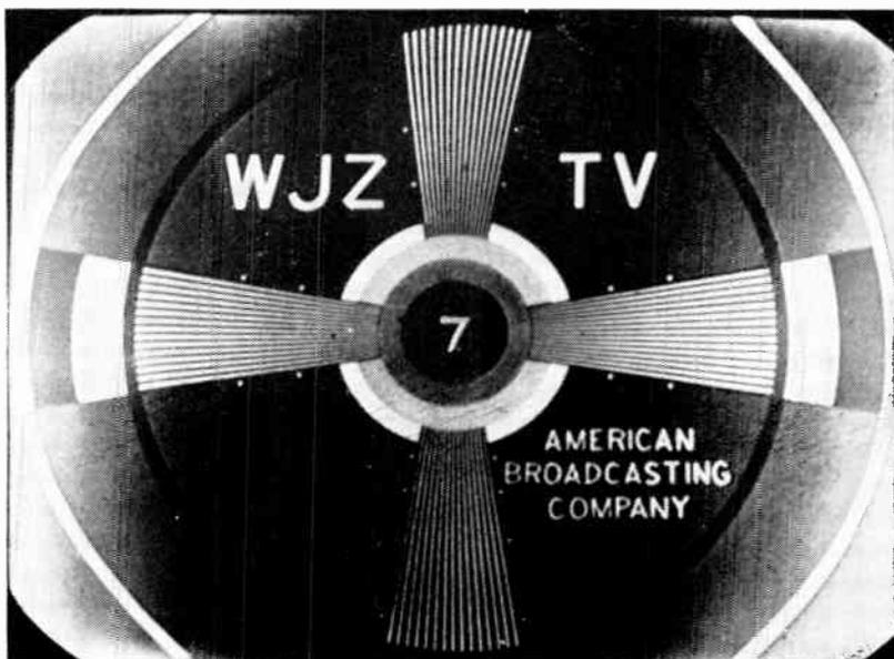
Fig. 6-20f. Actual appearance of the horizontal parabola shade of Fig. 6-20 (b).
