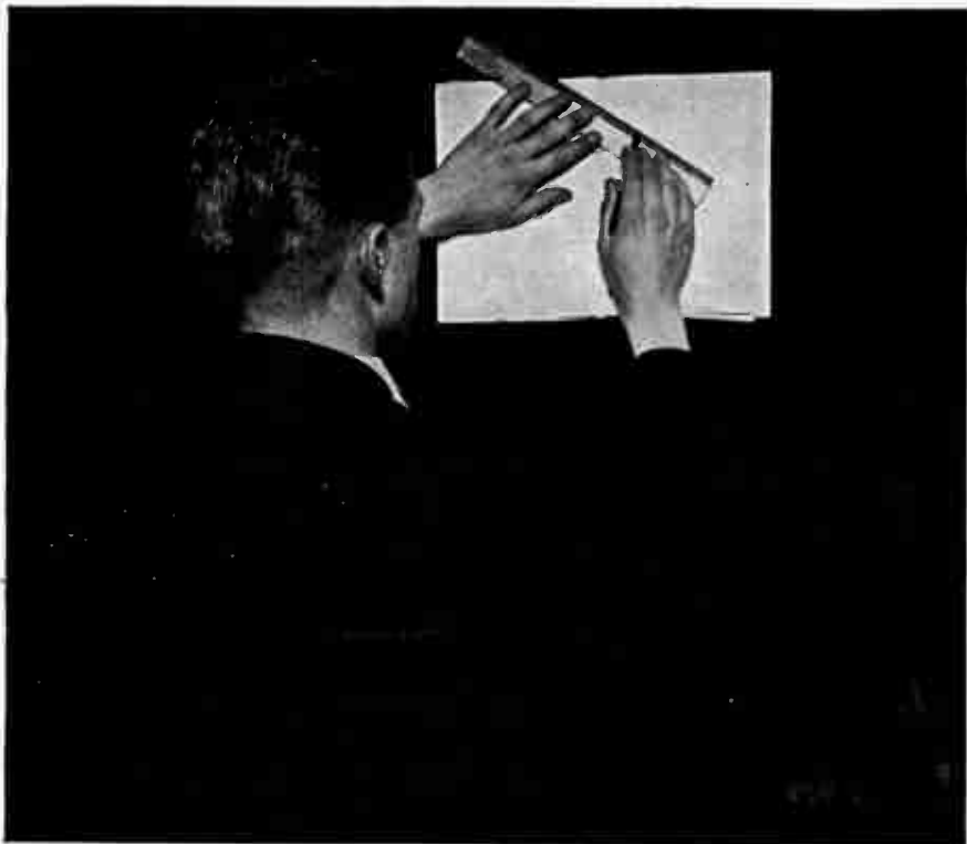
Figure FF: Lay your ruler across the alignment chart, as described in this article—and read off at a glance the answer to your problems in calculations.
