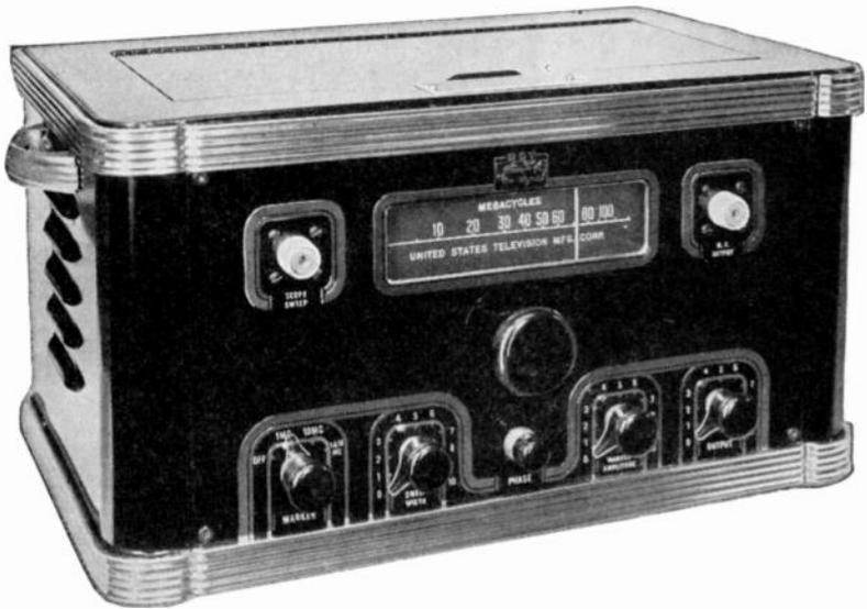
FIG. 11.10. A signal generator covering the F-M and television bands.
