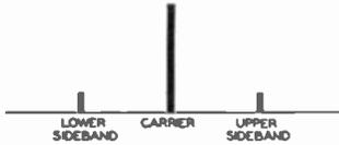
FIG. 16.6. A low value of phase shift produces only two sidebands.
