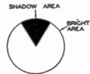
FIG. 8.16C. The eye opening when the grid becomes more positive.
