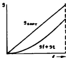
FIG. 9.13.—Approximate variation of input conductance of r.f. stage ( $g_f + g_t$ ) and  $g_{s\text{opt}}$  with frequency.
