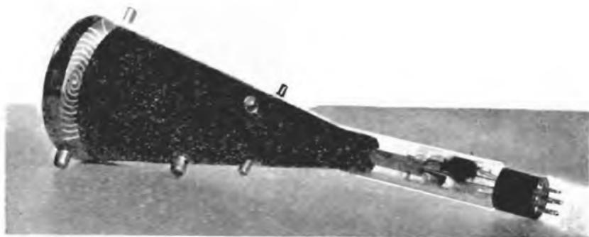
Fig. 7.17.—An R.C.A. cathode ray frequency modulation tube. The target anodes of this tube consist of five complete circles.
