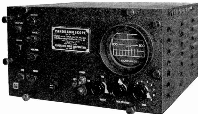
FIG. 10.3.—A typical panoramic monitor for the display of frequency modulation side band spectrum.
