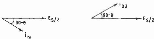
FIG. 8.51.—Showing vector relationships between the two half-secondary voltages and the diode fundamental frequency current components.
