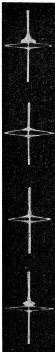
One Circuit Mistuned Round Nose, KQ < 1 Flat Top, KQ = 1 Double Peaked, KQ > 1 Double Peaked, KQ > 1 Fig. 3.16.—Oscillograms showing noise output wave-forms for varying degrees of coupling between circuits. (By courtesy of "Electronics".)
