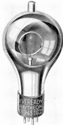
FIGURE 12. Photo-electric cells are used in television, in talking pictures, and in many industrial appliances where an interrupted beam of light opens doors, counts passing objects or sorts objects according to color.
