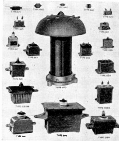
FIGURE 7. A number of condensers made by the Dubilier Condenser Corporation. The mushroom type in the middle is a coupling condenser used in carrier current, wired wireless, systems to permit telephoning over high potential transmission lines. All others condensers except the small ones at the top are used in radio transmitters or generators. The large one at the bottom is used in generating circuits where the voltage is from 3000 to 12000 volts.
