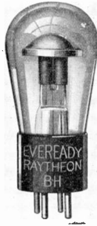
FIGURE 8. Raytheon rectifying tube. This tube rectifies both sides of the a-c. The tube is filled with an inert gas. The rectification depends upon the "point to plane" principle.
