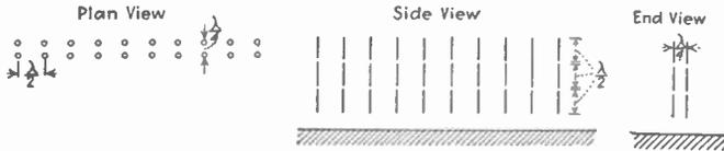
FIG. 229.—Typical antenna array consisting of a stacked broadside array having two curtains to give a unidirectional beam. The spacing between the curtains may be any odd multiple of a quarter wave length.
