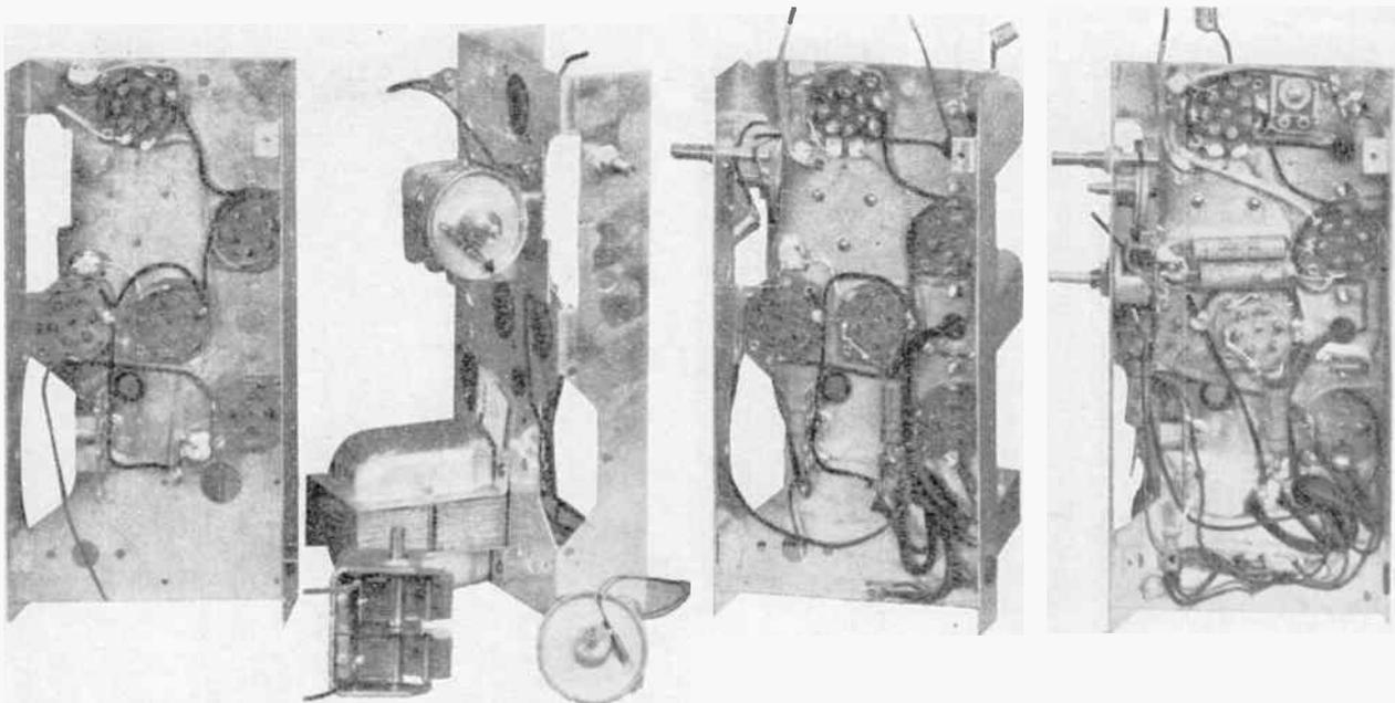
FIG. 178.—Photographs showing successive stages in the assembly of a broadcast receiver. (Courtesy of Giffilan Bros.)
