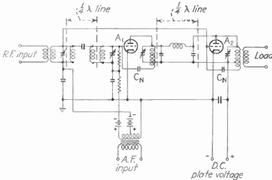
FIG. 122.—Schematic circuit diagram of high-efficiency grid-modulated amplifier.
