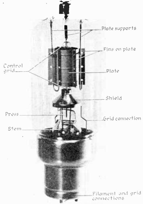
Type HK-354 Triode Tube. (Allowable plate dissipation = 150 watts.)
