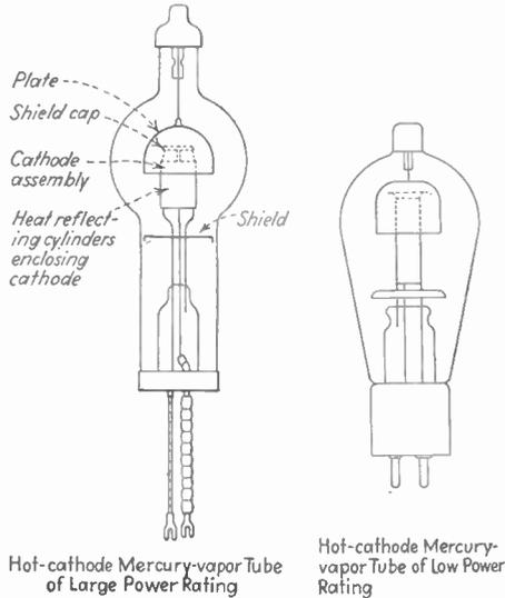
FIG. 149.—Typical hot-cathode mercury-vapor tubes.
