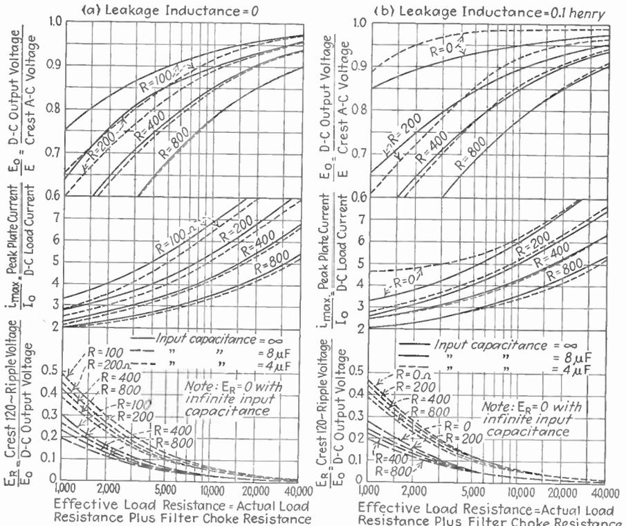
FIG. 156.—Charts giving performance of condenser-input filter systems for 60-cycle power source and full-wave rectifier. In these curves  $R$  is tube resistance plus transformer resistance of one half of secondary with primary shorted, and  $L$  is leakage inductance referred to half secondary with primary shorted.
