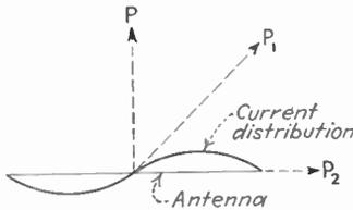
FIG. 219.—Diagram illustrating factors controlling the directional characteristic of an antenna. Note that the radiation does not cancel in the direction  $P_1$  because of the different distances to the two ends of the antenna.
