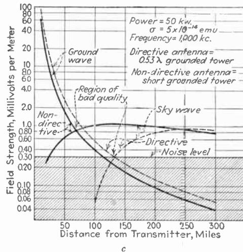
FIG. 202.—Effect of various factors on broadcast coverage. The solid line in each case is for the case illustrated in Fig. 201.
