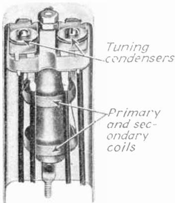
Intermediate-frequency coil assembly.
