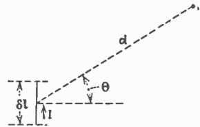
FIG. 210.—Elementary doublet consisting of a length of wire  $\delta l$  carrying a current  $I$ .
