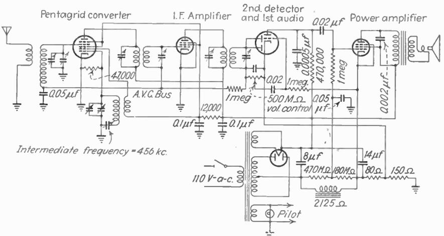
FIG. 173.—Circuit diagram of typical low-priced broadcast receiver.
