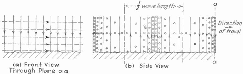
FIG. 1.—Front and side views of a vertically polarized wave. The solid lines represent electrostatic flux, and the dotted lines and circles indicate magnetic flux. This may be considered as an instantaneous view or "snapshot."
