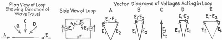
FIG. 246.—Vector diagrams showing how the voltages induced in the two sides of a loop by a passing radio wave combine to give a resultant voltage acting around the loop.
