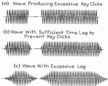
FIG. 166.—Output waves obtained with different keying conditions.
