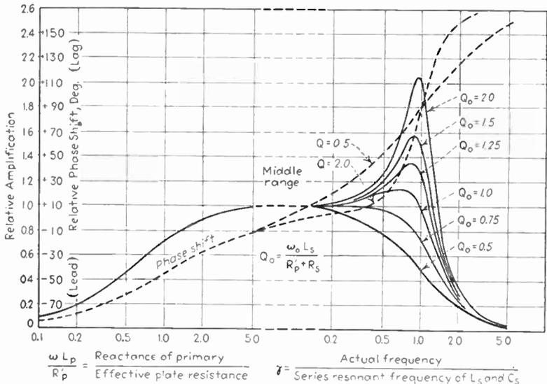
FIG. 63.—Universal amplification curve of transformer-coupled amplifiers.
