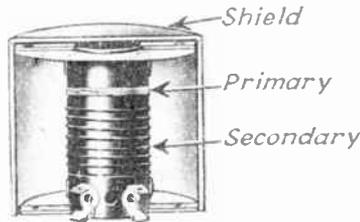
One-band radio-frequency coil assembly.
