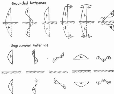
FIG. 215.—Images for common types of antennas.
