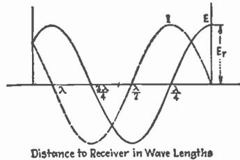
FIG. 29.—Schematic method of representing voltage and current distribution of Fig. 28a. This diagram indicates the  $180^\circ$  phase shift on opposite sides of the minima and is an accurate representation of the conditions existing along the circuit except where the voltage and current are shown going through zero.
