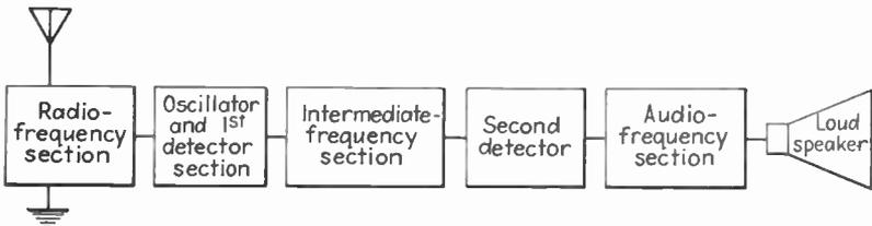
FIG. 172.—Schematic diagram of superheterodyne receiver.
