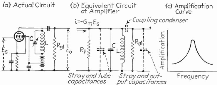
FIG. 68.—Equivalent circuit and amplification curve of a tuned amplifier with direct coupling. The amplification curve has the shape of a resonance curve but with an equivalent  $Q$  less than the actual  $Q$  of the tuned circuit.
