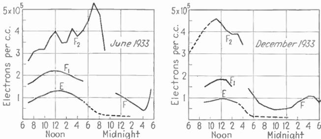
Fig. 190.—Average electron density of the various ionized layers at Washington, D. C., during 1933 (quiet part of sunspot cycle).
