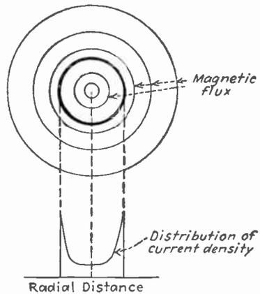
FIG. 9.—Isolated round conductor, showing flux paths and current distribution at radio frequencies. Note that the current density is highest for parts of the conductor encircled by the fewest flux lines.
