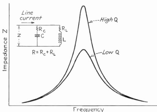
FIG. 19.—Parallel resonant circuit and typical curves of parallel impedance for different values of circuit  $Q$ . Note the similarity to Fig. 17.
