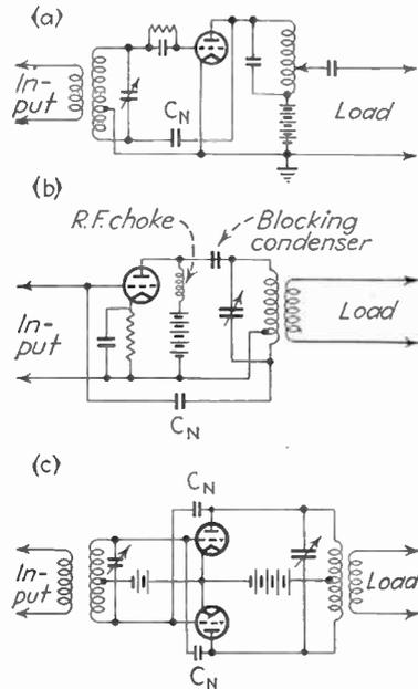
FIG. 95.—Typical circuit arrangements for Class C amplifiers.
