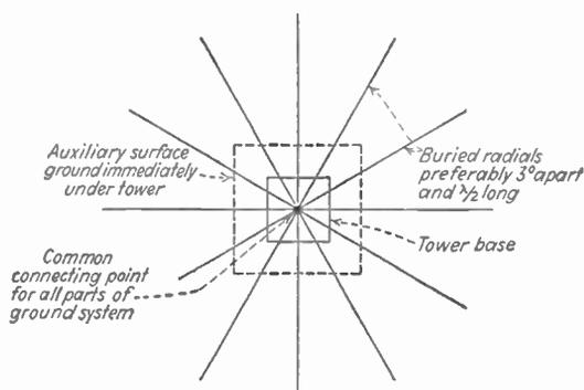
FIG. 243.—Typical ground system for vertical radiator.
