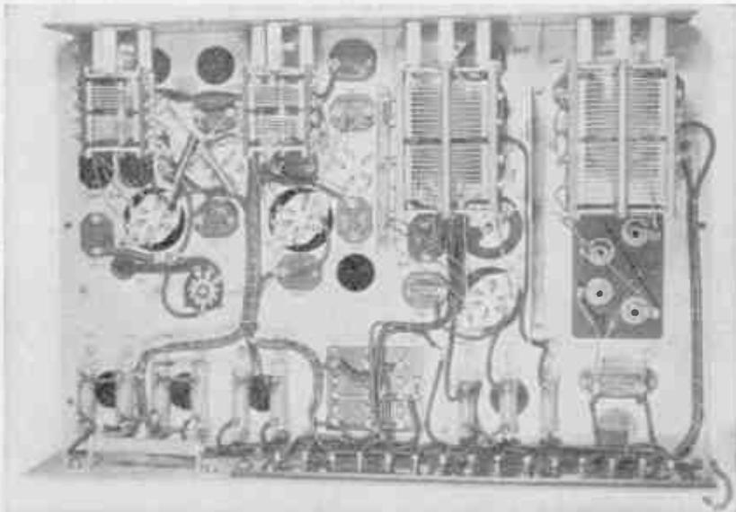
FIG. 164.—Top and bottom views of tray containing crystal oscillator and the three intermediate or buffer stages. Note the plug-in coils and the shields between stages as well as the method of mounting small parts and the cabling of wiring.
