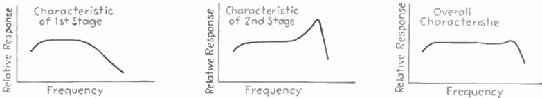
FIG. 79.—Curves illustrating how the deficiencies in the frequency response of one stage of an amplifier may be compensated for by the characteristic of another stage to give a uniform over-all response.
