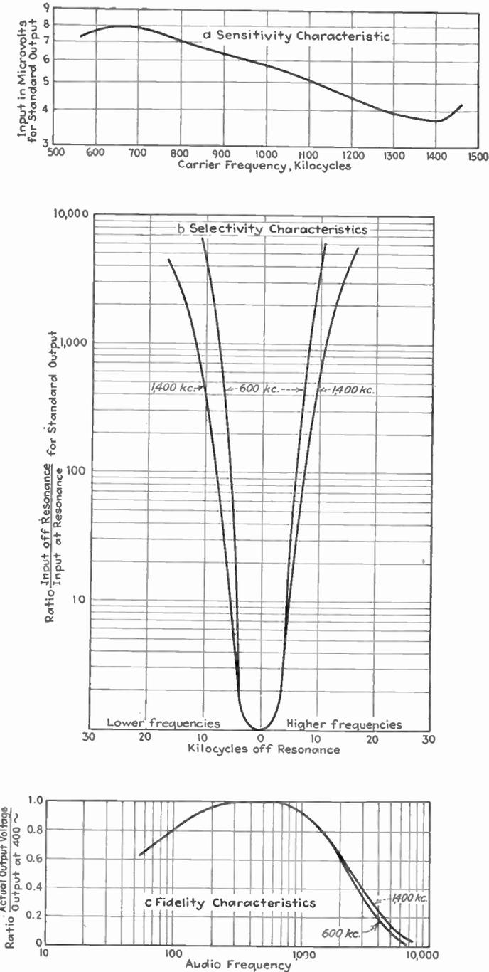
FIG. 170.—Typical sensitivity, selectivity, and fidelity curves of superheterodyne receiver.
