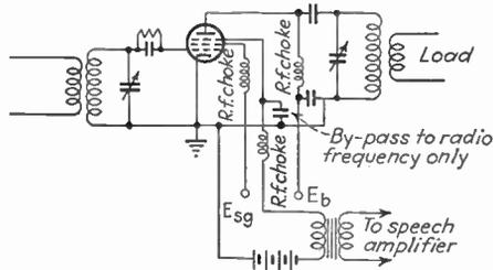
FIG. 123.—Circuit of suppressor-grid-modulated amplifier.
