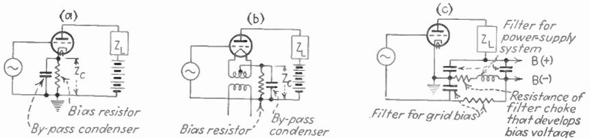
FIG. 148.—Methods of using the plate-supply voltage to make the grid negative with respect to the cathode.
