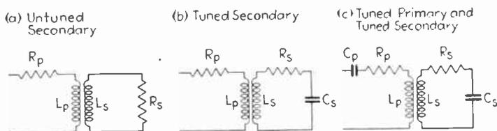
FIG. 21.—Common types of inductively coupled circuits.
