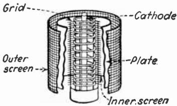
FIG. 48.—Cut-away illustration of a variable- $\mu$  screen-grid tube, showing the variable pitch of the control-grid structure that gives the variable- $\mu$  characteristic.
