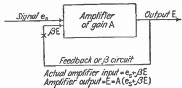
FIG. 76.—Schematic diagram of feedback amplifier.
