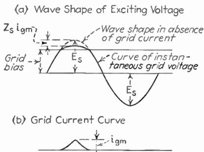
FIG. 86.—Wave shape of exciting voltage when grid is driven positive, showing flattening of the positive peaks resulting from grid current.
