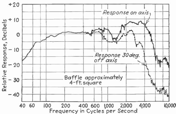
FIG. 268.—Response curve of typical cone dynamic speaker.
