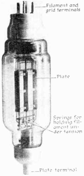
Type 849 Triode Tube. (Allowable plate dissipation = 400 watts)
