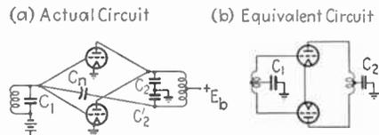
FIG. 113.—Amplifier with parallel tubes showing how the tubes may act in push-pull to produce a high-frequency parasitic oscillation.
