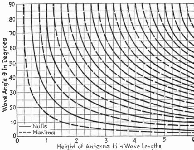
FIG. 217.—Chart showing the vertical angles at which the negative image factor  $\left[ 2 \sin \left( 2\pi \frac{H}{\lambda} \sin \theta \right) \right]$  is maximum and zero. These represent the vertical angles at which the reflections from the ground cause complete reinforcement and complete cancellation, respectively, of the radiation. With a positive image the positions of the nulls and maxima are interchanged.
