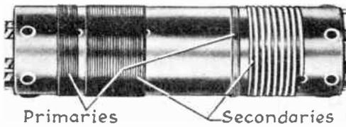
Two band coil assembly (single-layer solenoid)
