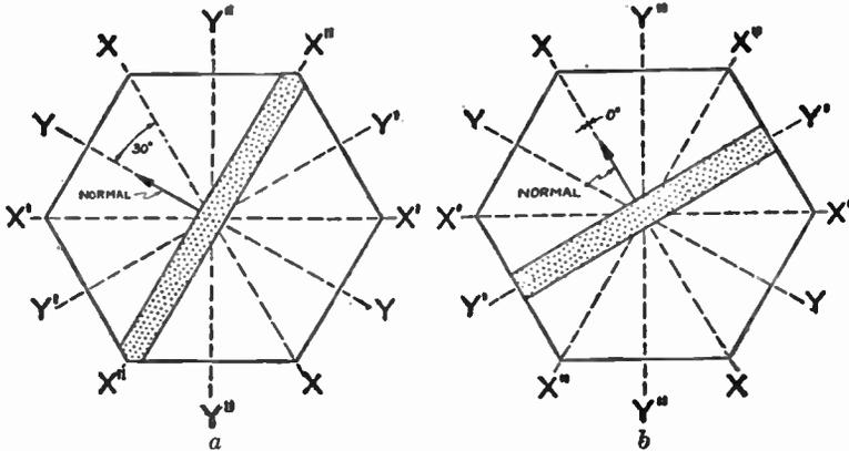
FIG. 106.—Cross sections of the quartz crystal shown in Fig. 105 taken in planes perpendicular to the optical axis  $ZZ$ . The plate at  $a$  is a  $Y$  cut (also called 30-deg. cut), because its face is perpendicular to a  $Y$  (i.e., mechanical) axis, while the plate at  $b$  is an  $X$  cut plate (Curie cut), because its face is perpendicular to an  $X$  (i.e., electric) axis.
