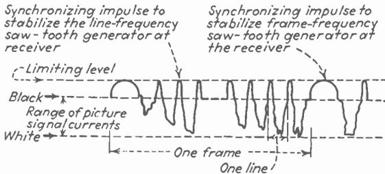
FIG. 259.—Typical television signal showing superimposed synchronizing pulses.
