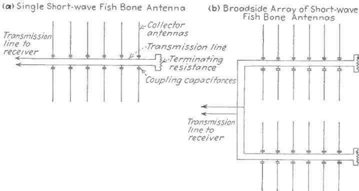
FIG. 227.—Plan view of single fishbone antenna and of an array consisting of two such antennas in broadside.
