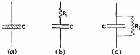
FIG. 4.—Representation of imperfect condenser by a perfect condenser of same capacitance, with series resistance, and by a perfect condenser with shunt resistance.
