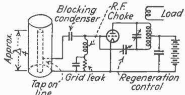
FIG. 104.—Circuit of practical vacuum-tube oscillator employing resonant line to control frequency.
