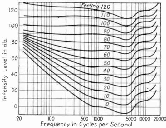
FIG. 265.—Contours giving intensity (*i.e.*, relative sound power) required for equal loudness as a function of frequency, for pure tones. The numbers on the contours give the strength of an equally loud 1000-cycle tone in decibels above the minimum audible 1000-cycle tone.
