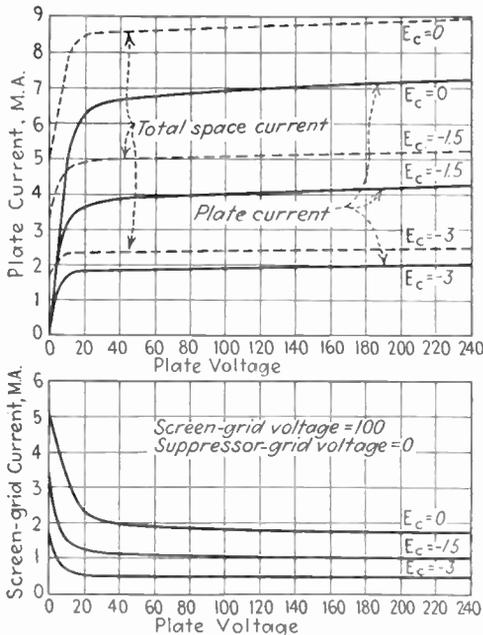
FIG. 40.—Curves showing plate and screen currents and total space current of a pentode as a function of plate voltage for various control-grid potentials. Note that when the plate potential is not too low the plate voltage has relatively little effect on the currents.
