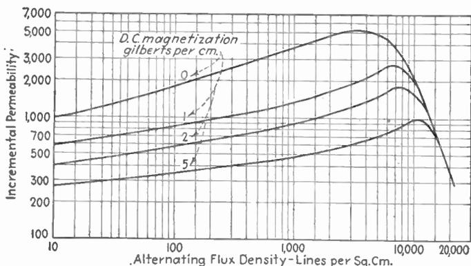
FIG. 7.—Curve giving incremental permeability of typical silicon steel as a function of alternating-current magnetization superimposed upon several values of direct-current magnetization, showing how the inductance decreases with increased direct-current and reduced alternating-current magnetization.
