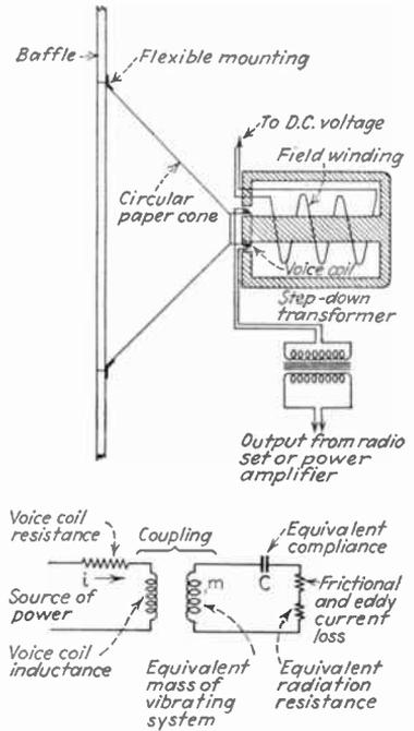
FIG. 267.—Cross section of typical dynamic type of loud-speaker and equivalent electrical circuit of electromechanical system.
