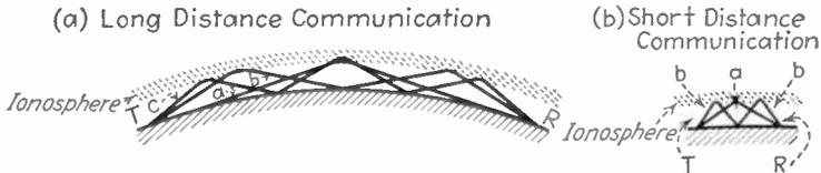
FIG. 204.—Typical wave paths by which energy might travel from transmitter to receiver. For the sake of simplicity only a single ionosphere layer is shown as being effective in determining the paths.
