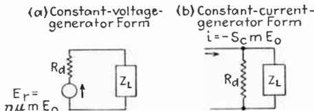
FIG. 136.—Equivalent plate circuits of plate detector. Note the similarity to the equivalent amplifier circuits of Fig. 56.
