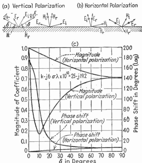
FIG. 198.—Reflection coefficient as a function of angle of incidence together with diagrams illustrating assumed positive polarities for Eq. (116) for the case of a perfect earth. (*E* and *H* denote electrostatic and magnetic flux, respectively, and subscripts *i* and *r* denote incident and reflected components.)
