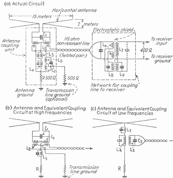
FIG. 244.—All-wave antenna system and equivalent circuits at high and low frequencies.
