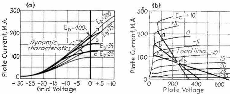
Fig. 87.—Dynamic characteristic of beam tube and resulting output waves for several values of load resistance, together with corresponding load lines. Note that the dynamic characteristics follow the characteristic curves of the tube except when the plate voltage becomes so low that a virtual cathode forms in the tube.
