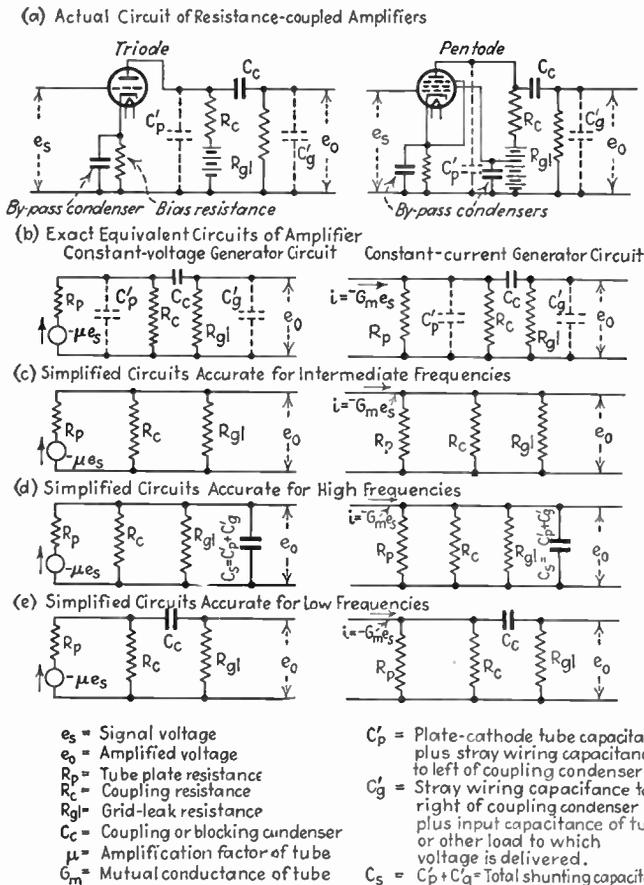
Fig. 57.—Circuits of resistance-coupled amplifiers together with equivalent circuits and simplifications of the equivalent circuits useful in making amplifier calculations. The constant-voltage generator circuit is used with the triode tube, and the constant-current generator form of the equivalent circuit is used for the pentode tube.
