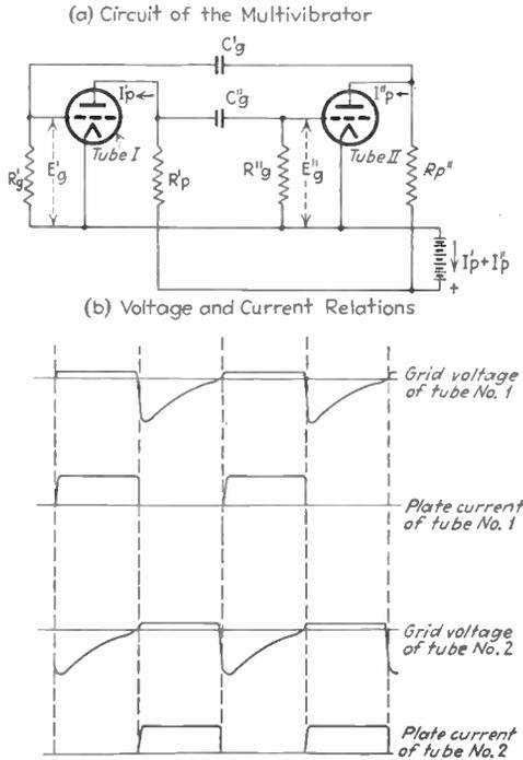
FIG. 116.—Circuit of multivibrator together with oscillograms showing the way in which the instantaneous grid potential and plate currents vary during the cycle of operation.
