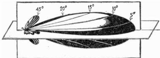
FIG. 230.—Directional characteristic in three-dimensional space of field radiated from a two-curtain broadside array. (From Southworth.)
