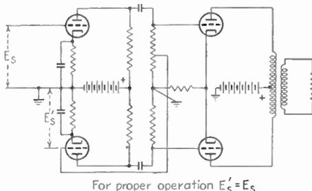
FIG. 92.—Push-pull amplifier excited with the aid of a phase-reversing tube.
