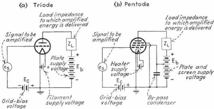
FIG. 54.—Basic circuits of vacuum-tube amplifiers employing triode and pentode tubes.
