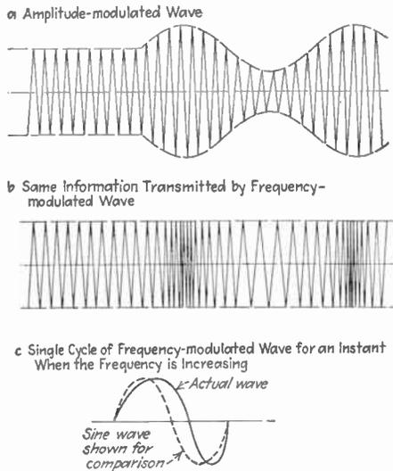
FIG. 129.—Character of waves produced by frequency modulation, together with large-scale reproduction of a single cycle, showing how the wave shapes are not sinusoidal.
