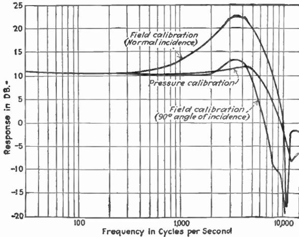
FIG. 277.—Typical pressure and field calibration of a condenser microphone.
