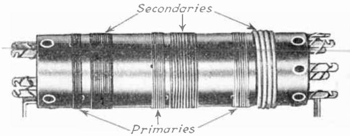
Three-band radio-frequency coil assembly.
