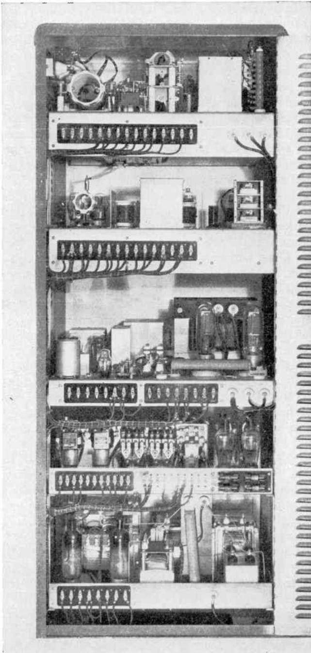
FIG. 163.—Rear view of cabinet of Fig. 162 with back opened showing the metal-shelf and tray construction and how the essential leads of each compartment are brought to a terminal strip.
