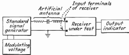
FIG. 171.—Schematic arrangement of equipment for making measurements of receiver performance.
