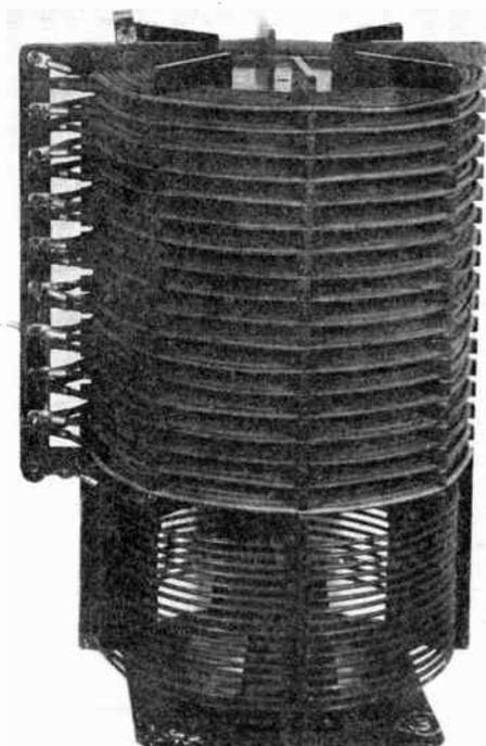
Large inductance for long-wave transmitter (multi-layer litz coil)
