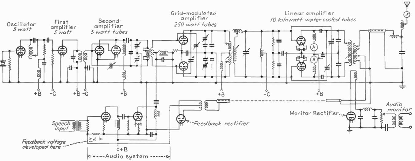
FIG. 169.—Simplified schematic circuit diagram of Western Electric 5-kw broadcast transmitter employing low-level grid modulation.
