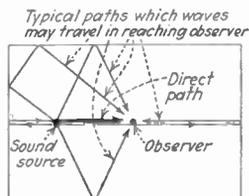
FIG. 266.—Diagram illustrating a few of the many routes that sound produced in a room may travel in reaching a listener.
