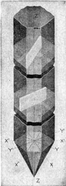
FIG. 105.—Illustration showing the natural quartz crystal and the relation of the electric or  $X$ , the mechanical or  $Y$ , and the optical or  $Z$  axes to the crystal structure. The upper section shows a  $Y$  (or 30-deg.) cut plate while the plate in the center section is  $X$  (or Curie) cut. The third  $Y$  axis,  $Y''Y''$ , is not shown because the perspective of the drawing makes it coincide with the  $ZZ$  axis.
