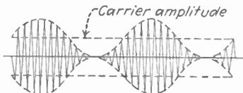
FIG. 3.—Waves having different degrees of simple sine-wave modulation.
