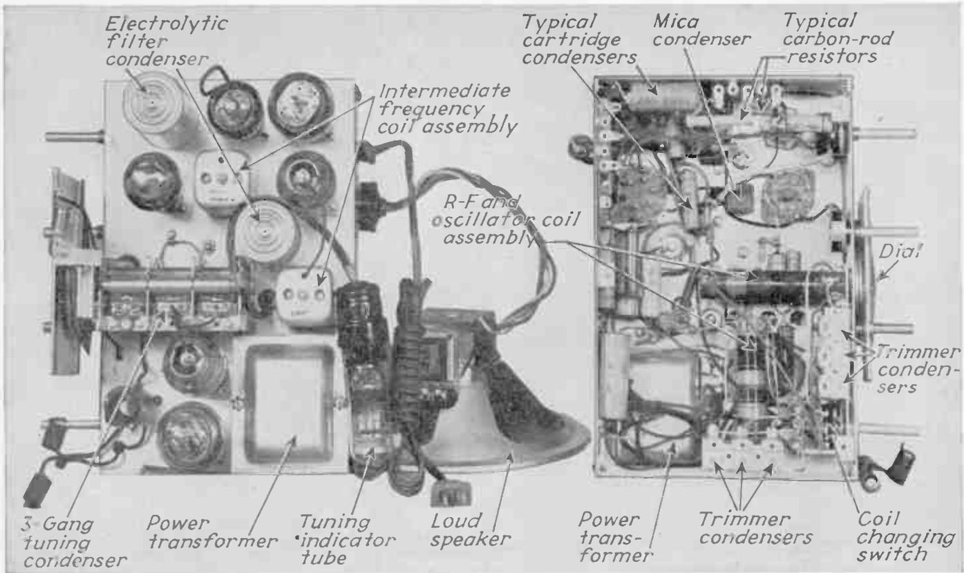
FIG. 179.—Photographs showing views of chassis for receiver of Fig. 174. (Courtesy of Gilfillan Bros.)
