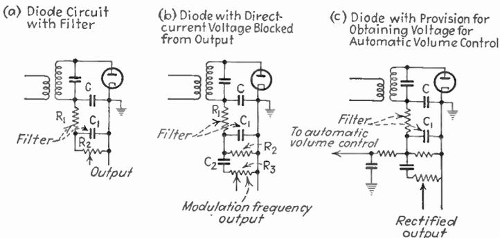
FIG. 132.—Practical diode detector circuits.
