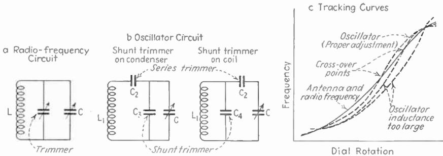
FIG. 181.—Trimmer systems for circuits of superheterodyne radio receiver together with schematic curves showing kind of tracking obtained for typical cases. The solid curve in *c* represents perfect tracking with antenna and radio-frequency circuits, while the dotted curves give the actual tracking obtained under various conditions.
