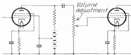
FIG. 78.—Volume-control arrangement normally used in resistance-coupled amplifiers.
