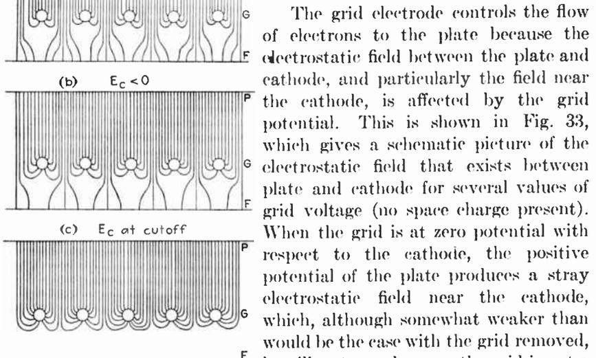
FIG. 33.—Schematic picture of electrostatic field produced between plate and cathode with different grid potentials, showing how the electrostatic field in the vicinity of the cathode can be controlled by the potential of the grid. These curves take into account only those fields produced by the electrode potentials and do not include the field developed by the space charge of electrons which is superimposed upon the fields shown.
