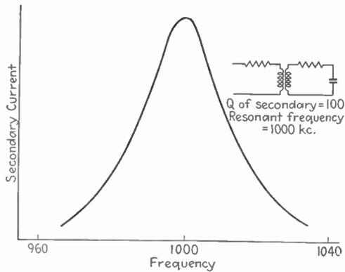
FIG. 22.—Curve of secondary current as a function of frequency for the circuit of Fig. 21b in the typical case where  $R_p \gg \omega L_p$ . This curve has the shape of a resonance curve corresponding to a  $Q$  lower than the actual secondary  $Q$ .
