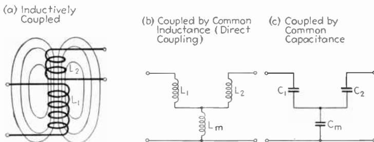
FIG. 8.—Several simple methods of coupling two circuits.
