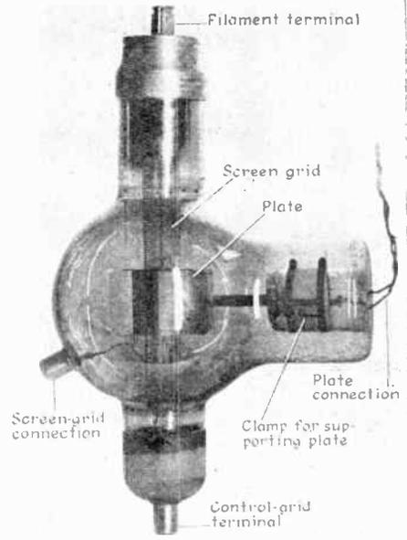
Type 861 Screen-grid Tube. (Allowable plate dissipation = 400 watts.)
