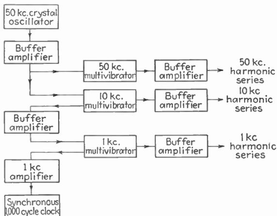
FIG. 278.—Schematic diagram of a primary frequency standard.
