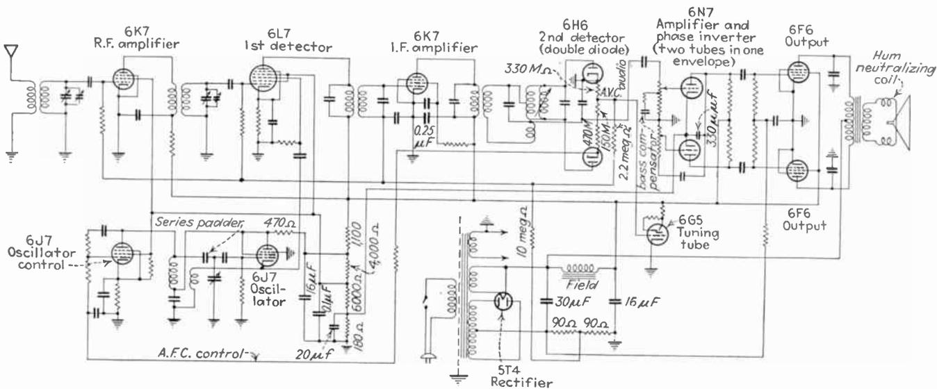
FIG. 175.—Circuit diagram of typical moderately high-priced all-wave broadcast receiver with automatic frequency control.
