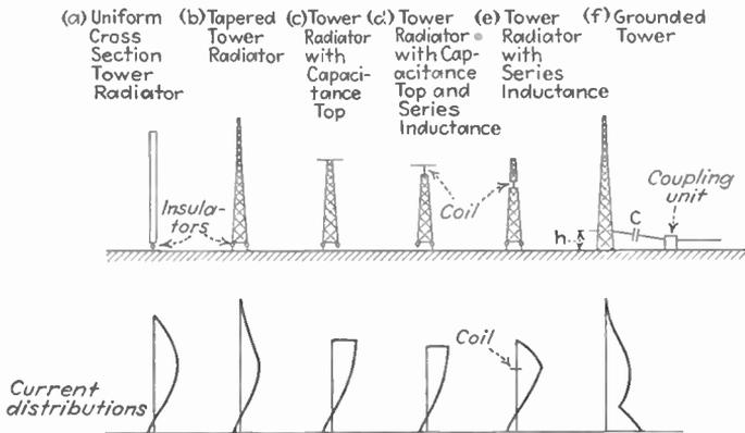
FIG. 242.—Different types of vertical radiators, with current distribution for each.
