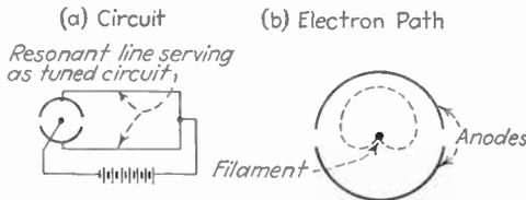
FIG. 115.—Circuit of electron oscillator of split-anode magnetron type together with electron path. The tube is placed in a magnetic field that is approximately axial.
