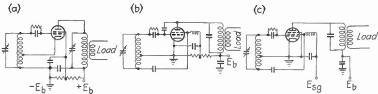
FIG. 103.—Electron-coupled oscillator circuits.
