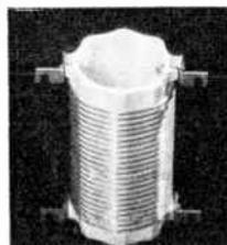
Short-wave coil (solid wire on ceramic form)
