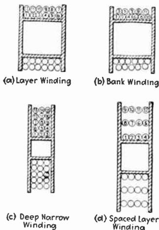
FIG. 14.—Several types of multilayer windings.
