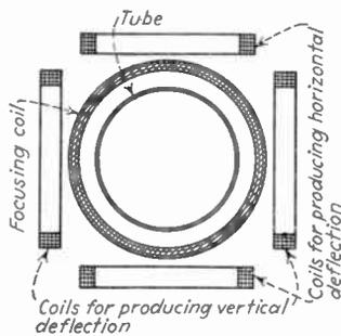
FIG. 255.—Coil system for producing magnetic deflection of electron image and for focusing. The view shown is a cross section through the middle of the tube of Fig. 254 at right angles to the axis.
