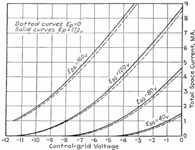
FIG. 43.—Typical curves showing the effect of electrode voltages on the total space current ( $i_p + i_{sg}$ ) of a screen-grid tube. This total current is relatively independent of the plate potential and varies with control- and screen-grid potentials in exactly the same way as the plate current of a triode varies with grid and plate voltages, respectively.
