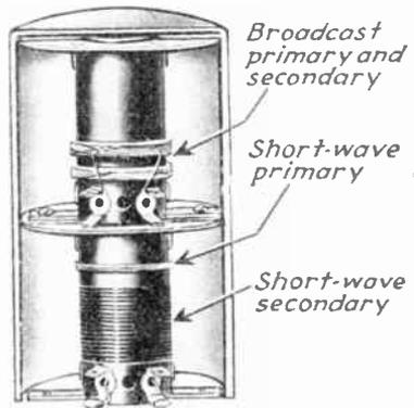
Two-band radio-frequency coil assembly.
