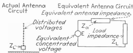
FIG. 213.—Actual receiving antenna with load impedance  $Z_L$  and distributed induced voltages together with equivalent antenna circuit in which the distributed voltages are replaced by a lumped voltage  $E$  and the distributed antenna impedance by an equivalent concentrated impedance  $Z_a$ .
