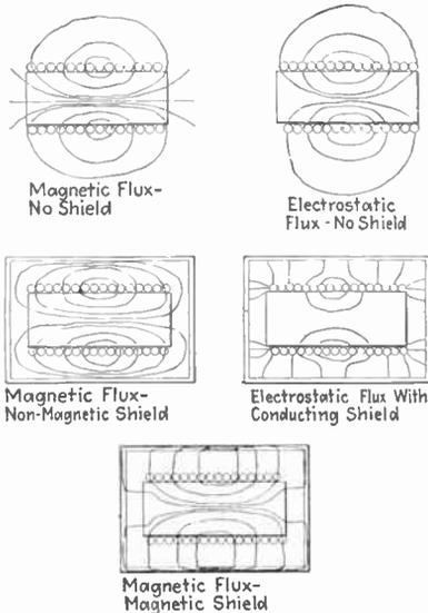
FIG. 16.—Paths of electrostatic and magnetic flux lines about the same coil with and without magnetic and non-magnetic shields.
