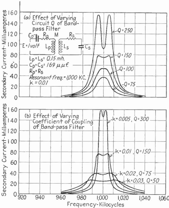
FIG. 24.—Characteristics of band-pass filter, showing (a) effect of circuit  $Q$  on uniformity of response within the pass band and (b) effect of coefficient of coupling upon the width of the pass band and the response within the pass band when the proper circuit  $Q$  is used.
