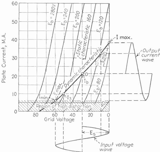
FIG. 82.—Circuits of power amplifier together with dynamic characteristic suitable for Class A operation without driving the grid positive, and resulting input and output waves.
