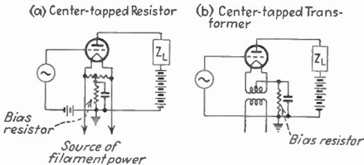
FIG. 147.—Methods of connecting the grid and plate return leads of filament tubes when alternating filament current is used.
