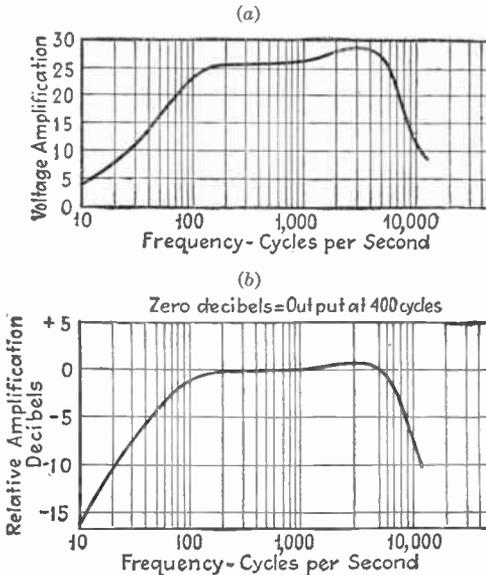
FIG. 80.—Illustration of how relative gain can be expressed in decibels.
