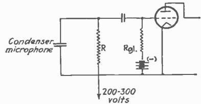
FIG. 276.—Circuit of condenser microphone.
