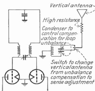
Fig. 248.—Circuit diagram of practical radio compass.
