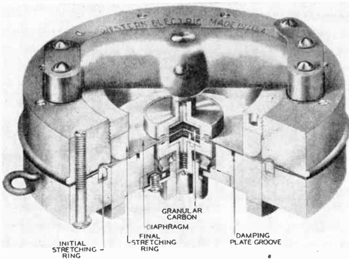
FIG. 274.—Constructional features of high-grade double-button carbon microphone.
