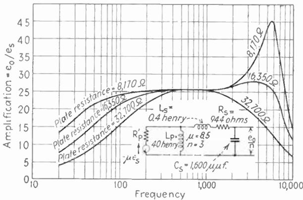
FIG. 64.—Effect of varying the effective plate resistance  $R_p$  in a transformer-coupled amplifier. Note that the best characteristic is obtained when the plate resistance is neither too high nor too low but is rather properly matched to the transformer.
