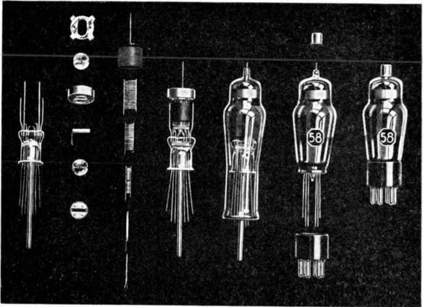
FIG. 51b.—Photographs showing constructional features of small glass-envelope pentode tube, having heater cathode and variable- $\mu$  control grid.
