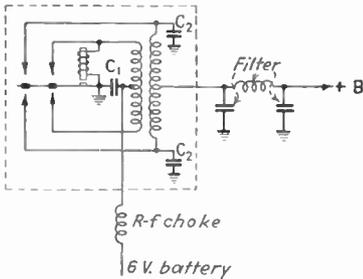
FIG. 157.—Circuit diagram of vibrator power supply.
