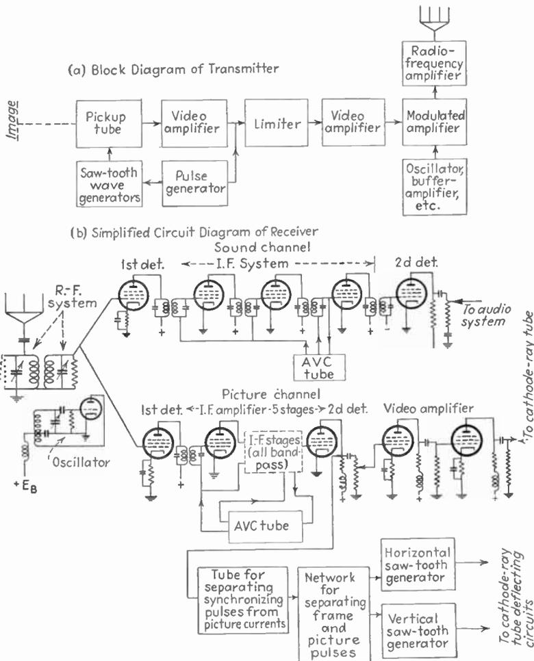
FIG. 262.—Diagram of complete television system.
