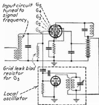
FIG. 140.—Circuit of typical 6L7 mixer tube.
