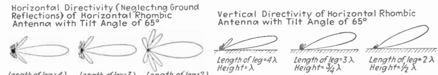
Fig. 235.—Polar diagrams showing directional characteristics of the same horizontal non-resonant rhombic antenna for three different frequencies.
