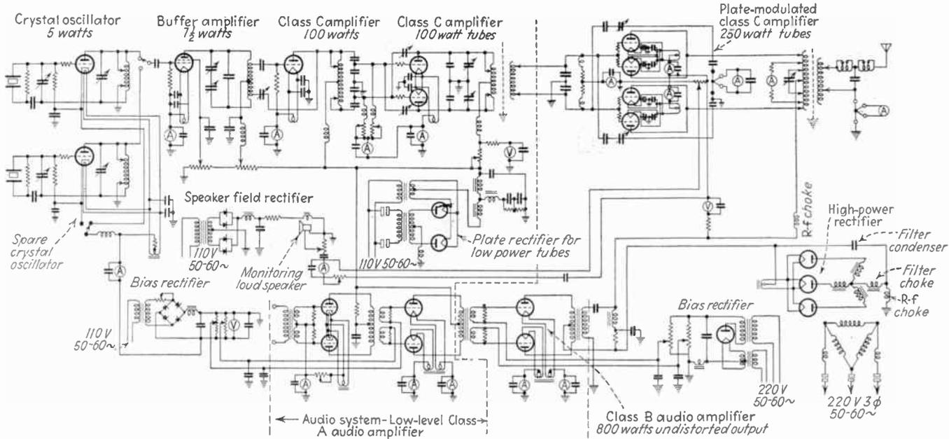
FIG. 167.—Simplified schematic circuit diagram of RCA 1-kw. broadcast transmitter employing high-level modulation.
