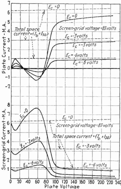
FIG. 44.—Variation of plate and screen-grid currents, and of total space current, with plate voltage (screen-grid voltage constant). It will be noted that changing the control-grid voltage alters the magnitude of the curves without changing their shape (i.e., the control-grid potential affects the total space current but does not alter its division between the plate and screen grid).
