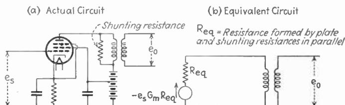
Fig. 65.—Circuit of transformer-coupled amplifier using a pentode tube. The resistance shunted across the primary of the transformer should equal the plate resistance that would be used if the tube were a triode.
