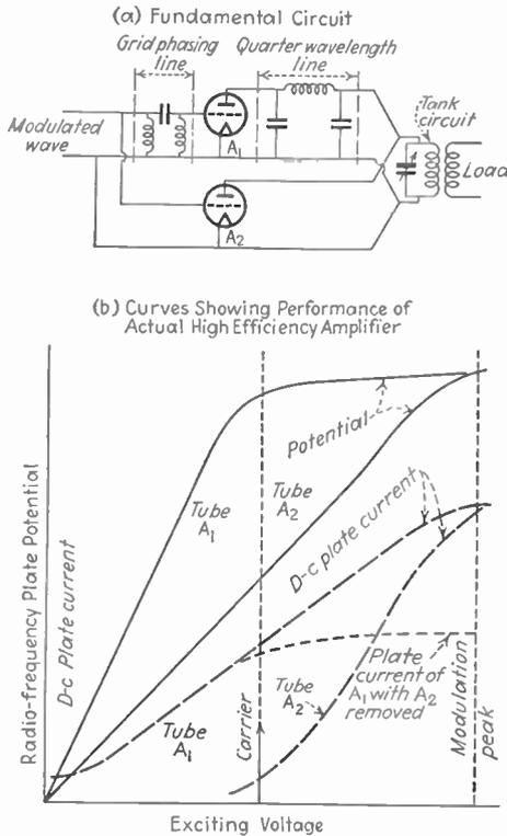
FIG. 99.—Schematic diagram of high-efficiency linear amplifier.
