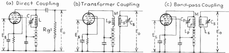
FIG. 67.—Typical tuned-amplifier circuits using pentode tubes.
