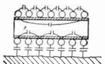
FIG. 13.—Some of the coil capacitances that contribute to the distributed capacitance of a single-layer coil.
