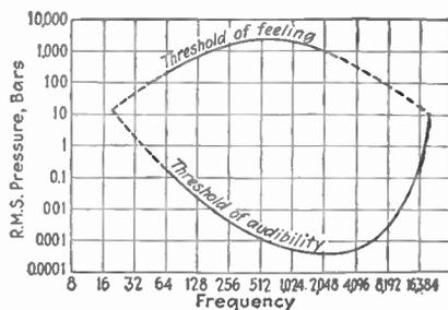
FIG. 264.—Average auditory sensation area of normal ears. The curve marked "Threshold of audibility" represents the weakest audible sound, and the curve "Threshold of feeling" represents the loudest sound that does not produce pain.
