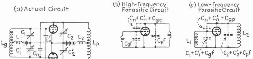
FIG. 112.—Neutralized push-pull amplifier, showing how the tubes can operate in parallel to produce a high-frequency parasitic oscillation and also a low-frequency parasitic oscillation.
