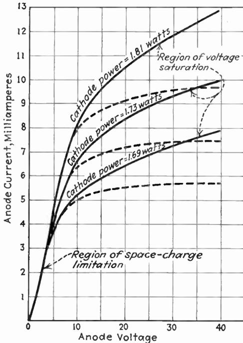
FIG. 31.—Anode current as a function of anode voltage in a two-electrode tube for three cathode temperatures. The solid lines are the characteristics actually obtained using an oxide-coated cathode, whereas the dotted lines show the type of curves given by tungsten and thoriated-tungsten cathodes.
