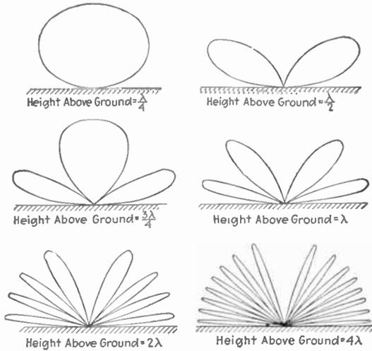
FIG. 216.—Polar diagram of the negative image factor  $\left[ 2 \sin \left( 2\pi \frac{H}{\lambda} \sin \theta \right) \right]$  for various values of  $H/\lambda$ , showing how the height above earth affects the directional characteristic of the antenna.
