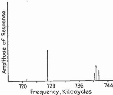
FIG. 109.—Typical frequency spectrum of thin quartz plate showing how several closely spaced resonant frequencies sometimes occur. The length of the vertical lines indicates in a rough way the relative tendency to oscillate at the different resonant frequencies.
