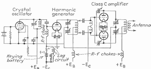
FIG. 160.—Simple short-wave crystal-controlled telegraph transmitter showing keying system provided with time-lag circuit.
