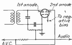
FIG. 176.—Method of obtaining delayed automatic volume control.
