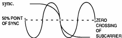
Reference subcarrier is **Positive Going** in Color Field 1 on even lines.
