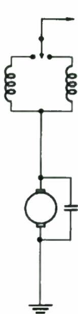
Figure 5-5 a. Location of Capacitor in Series Motor
