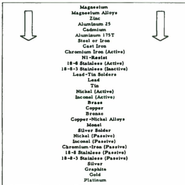
Figure 3-29. Electromotive-Force Series for Selected Metals
