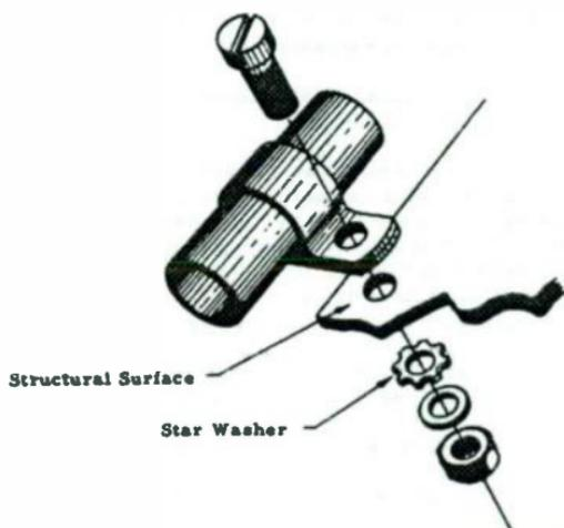
Figure 3-35. Tubing Clamp Bonded to Painted Surface
