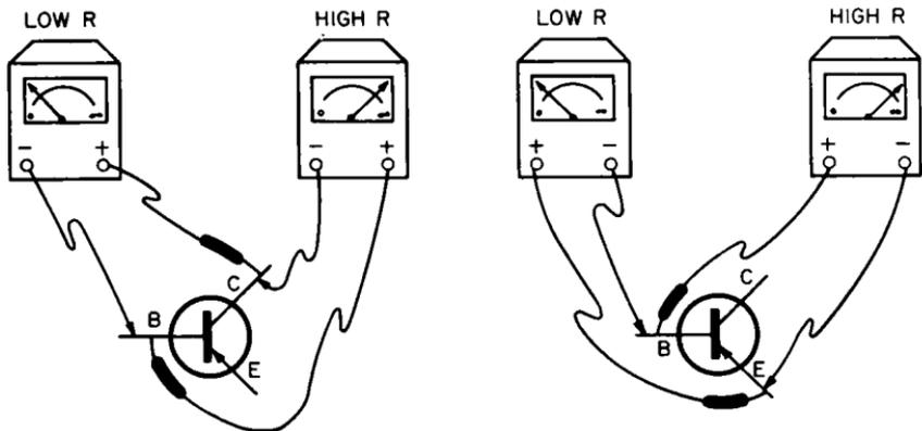
Fig. 10-7. Testing pnp transistors with an ohmmeter. The low resistance should be 50 to 500 ohms. The high resistance should be 50K to 5 megohms. The forward-to-back ratio should be 100:1 or better.
