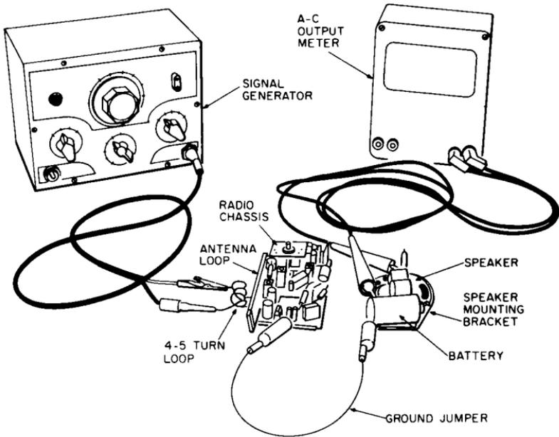
Fig. 5-9. I-F alignment setup for transistor radios. Courtesy Westinghouse.
