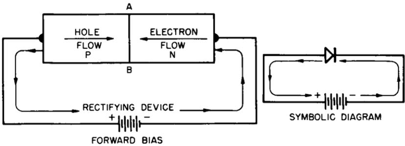
Fig. 1-9. Conduction in a pn junction occurs in one direction only (rectification) by hole movement in the p-type material, and by electron movement in the n-type material. The unit is "forward biased."
