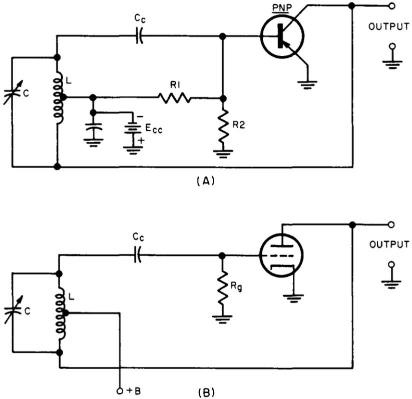
Fig. 6-2. (A) Transistorized Hartley oscillator circuit. (B) Vacuum tube Hartley oscillator circuit.
