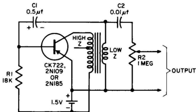
Fig. 10-4. Circuit for a noise-type signal generator using a blocking oscillator circuit.
