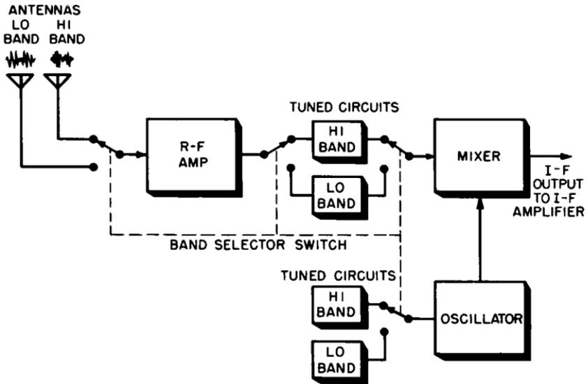
Fig. 2-2. Block diagram of a multiband receiver front end having two bands.
