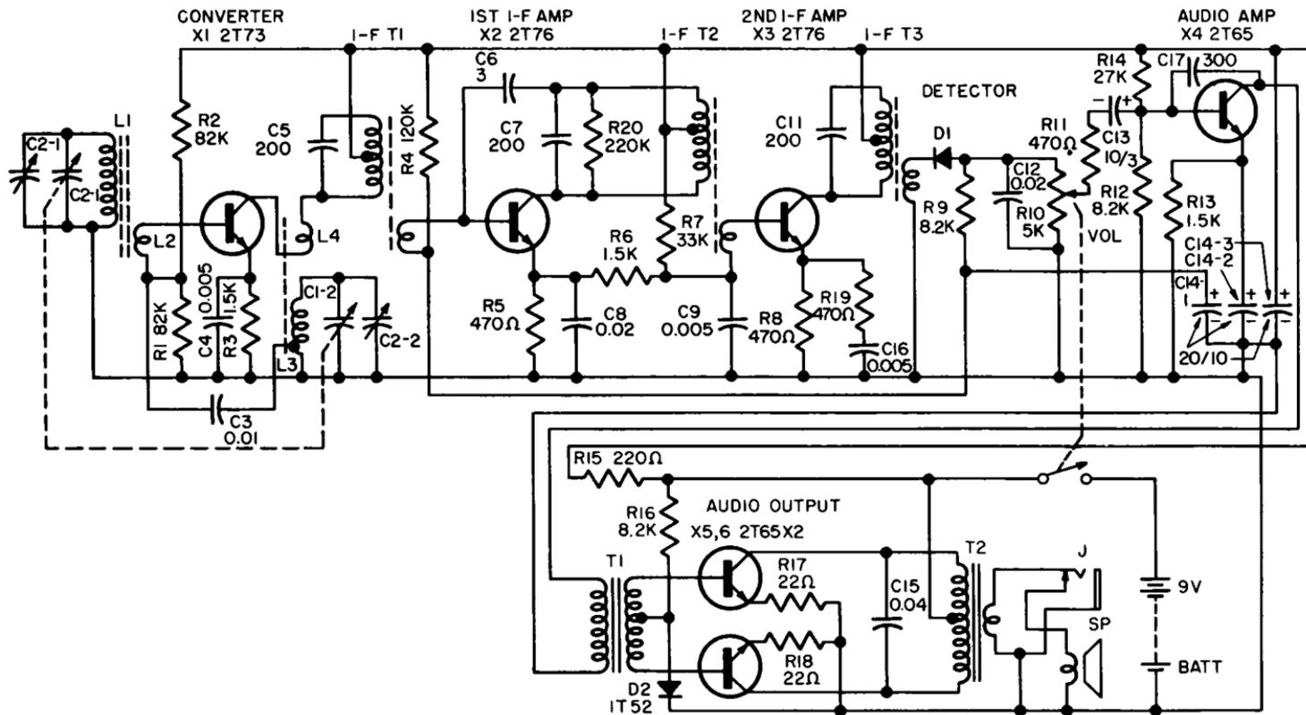
Fig. 8-12. Sony model TR-610 six-transistor portable radio receiver.
