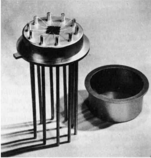
**Fig. 1-25.** IC chip mounted in a TO-type package
