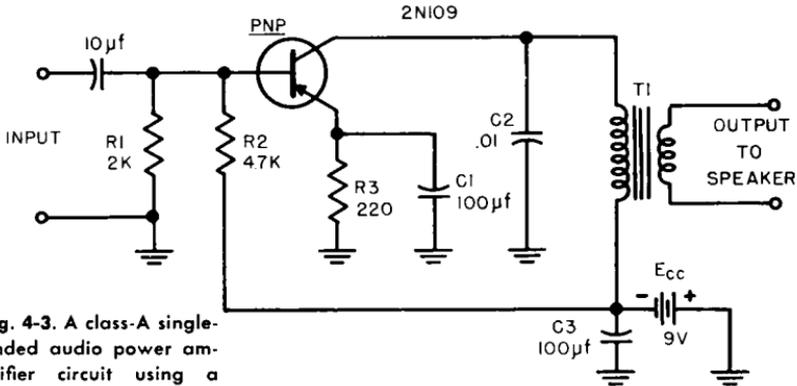
Fig. 4-3. A class-A single-ended audio power amplifier circuit using a 2N109 junction transistor.
