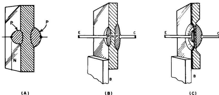
Fig. 1-17. Construction details of alloy-type transistors: (A) standard alloy type, (B) microalloy MAT type, and (C) alloy-diffused MADT type.
