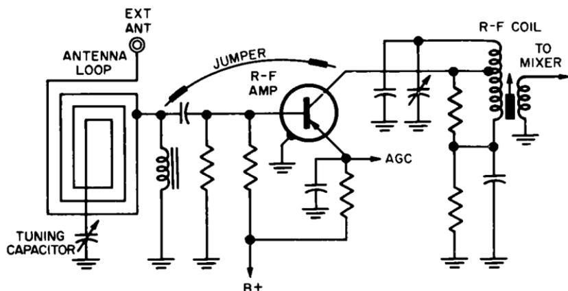
Fig. 5-11. A method of checking for a defective transistor when no exact replacement is available.
