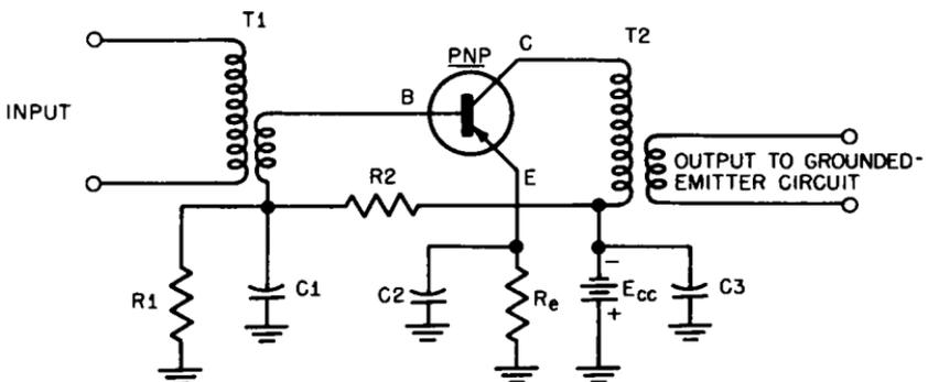
Fig. 3-11. A basic transformer-coupled amplifier.
