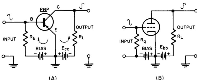
Fig. 3-4. (A) Grounded-emitter transistor amplifier circuit compared to (B) the conventional grounded-cathode vacuum tube amplifier circuit.
