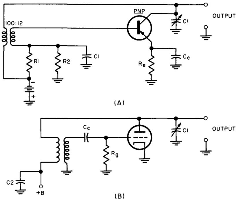
Fig. 6-1. (A) Transistorized Meissner oscillator circuit. (B) Vacuum tube Meissner oscillator circuit.
