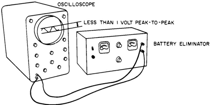
Fig. 9-6. Checking the ripple content of a battery eliminator with an oscilloscope.
