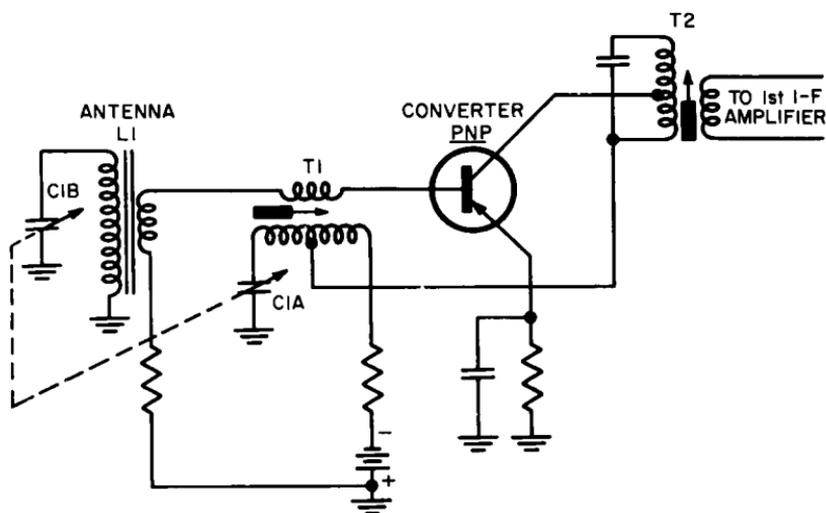
Fig. 6-4. Typical transistorized converter circuit used in many broadcast band portable receivers.
