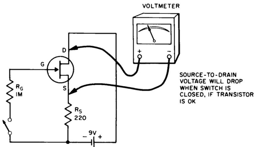
Fig. 10-12. Static test of an N-channel FET (when checking P-channel FET, reverse battery and voltmeter).
