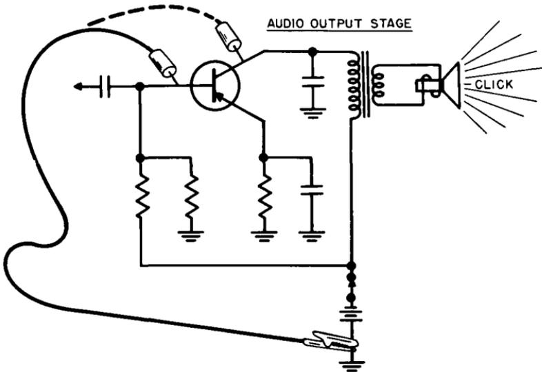
Fig. 4-11. A quick check of the audio driver stage.
