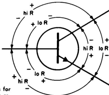
Fig. 10-15. Resistance readings for a power transistor (polarities are reversed for a pnp type).
