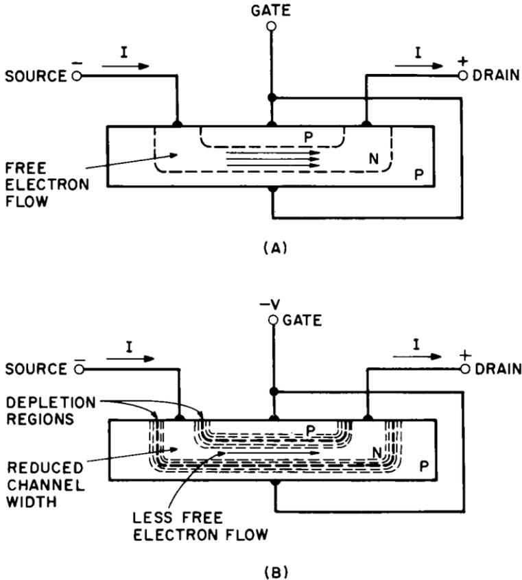
Fig. 1-21. J-FET operation: (A) Source-to-drain current high zero voltage on gate, and (B) source-to-drain current reduced by negative gate voltage, creating depletion regions in channel.
