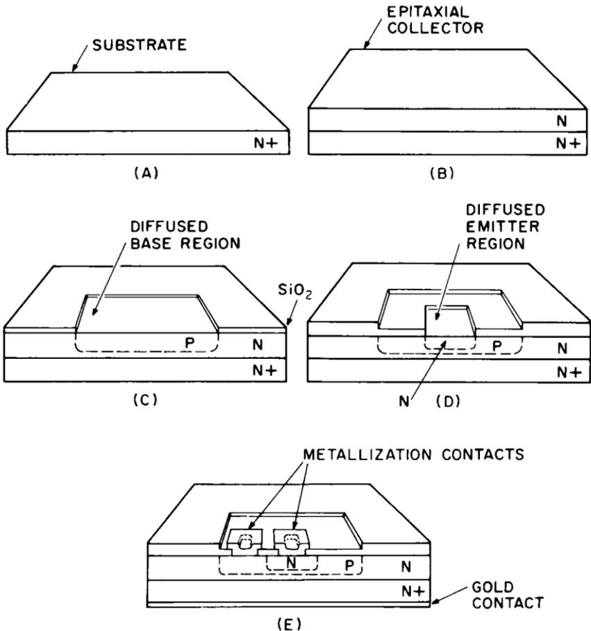
Fig. 1-19. Fabrication of an epitaxial type transmitter.
