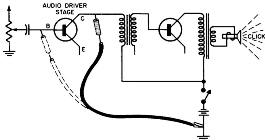
Fig. 3-18. Quick check of audio driver stage.
