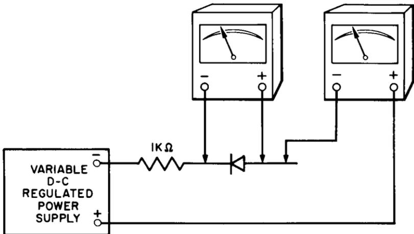
Fig. 10-18. Circuit arrangement for checking zener diodes.
