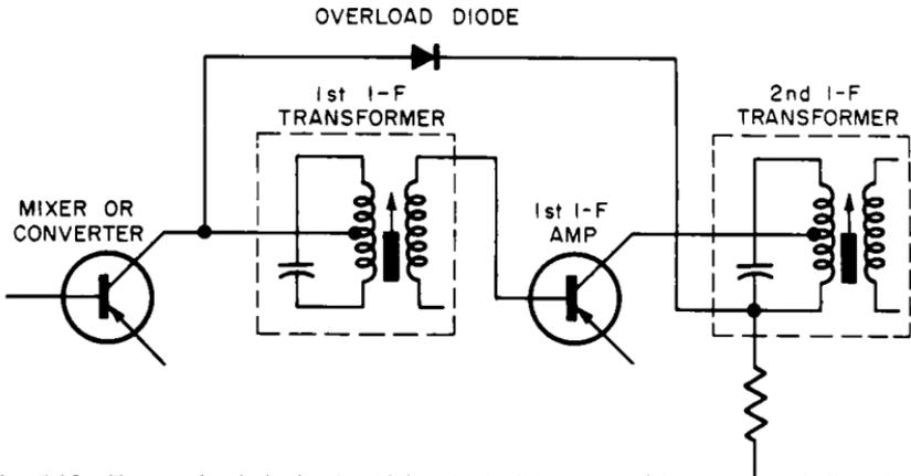
Fig. 7-12. The overload diode should be checked in cases of low gain and distortion (see text).
