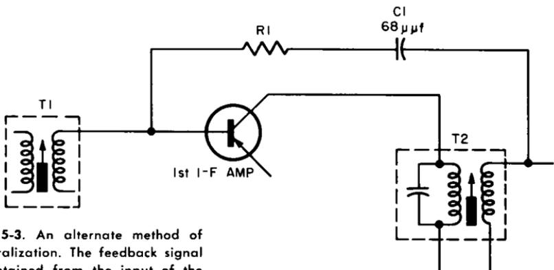
Fig. 5-3. An alternate method of neutralization. The feedback signal is obtained from the input of the following stage.
