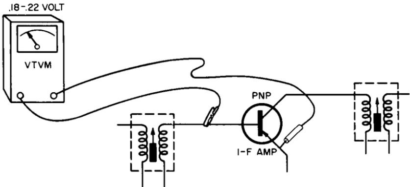
Fig. 5-8. Checking the base-to-emitter bias of an i-f amplifier transistor. For npn transistors, the vtvm leads should be reversed. The voltage in a properly operating circuit will be between 0.18 and 0.22 volt.
