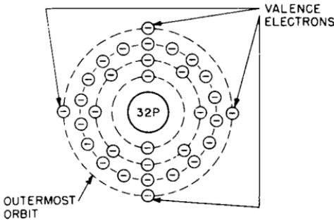
Fig. 1-3. A germanium atom is composed of 13 protons in the nucleus and 13 orbital electrons. Four valence electrons, in the outermost orbit, make this element a semiconductor.
