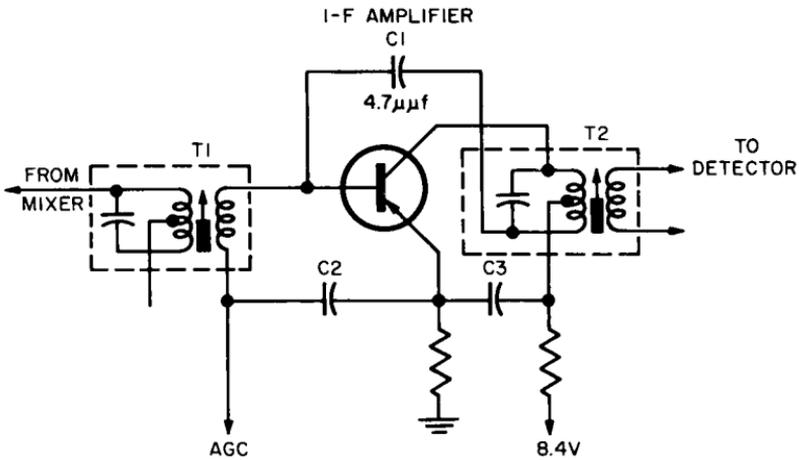
Fig. 5-2. A 455-kc i-f amplifier employing neutralization to increase circuit stability. The i-f transformers are tapped to provide an impedance match and increase the transfer of energy between stages.
