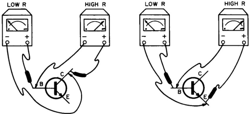
Fig. 10-6. Testing npn transistors with an ohmmeter. The low resistance should be 50 to 500 ohms. The high resistance should be 50K to 5 megohms. The forward-to-back ratio should be 100:1 or better.
