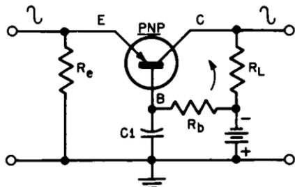
Fig. 3-3. Simplified biasing arrangement for the grounded-base circuit requiring only one battery.
