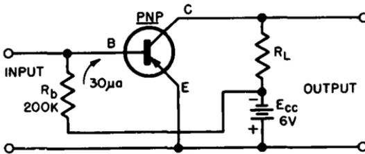
Fig. 3-6. Fixed bias system for developing the proper base bias in a grounded-emitter amplifier circuit.
