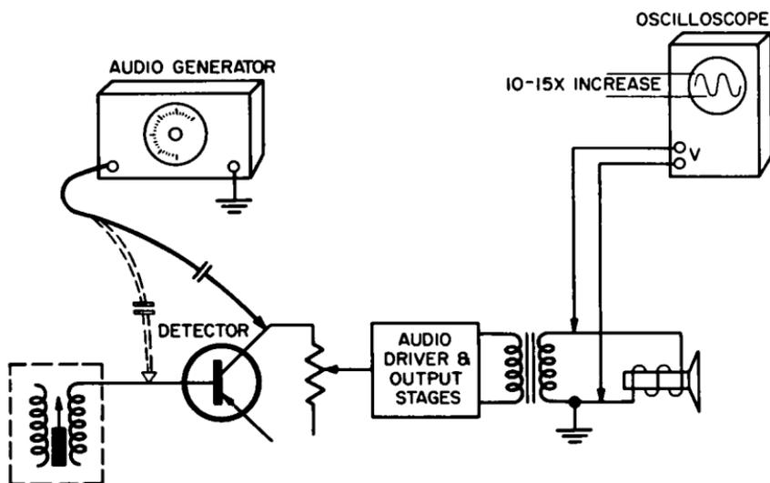
Fig. 7-8. Gain check of a transistor detector circuit. A gain of 10–15X should be measured in a normal circuit.
