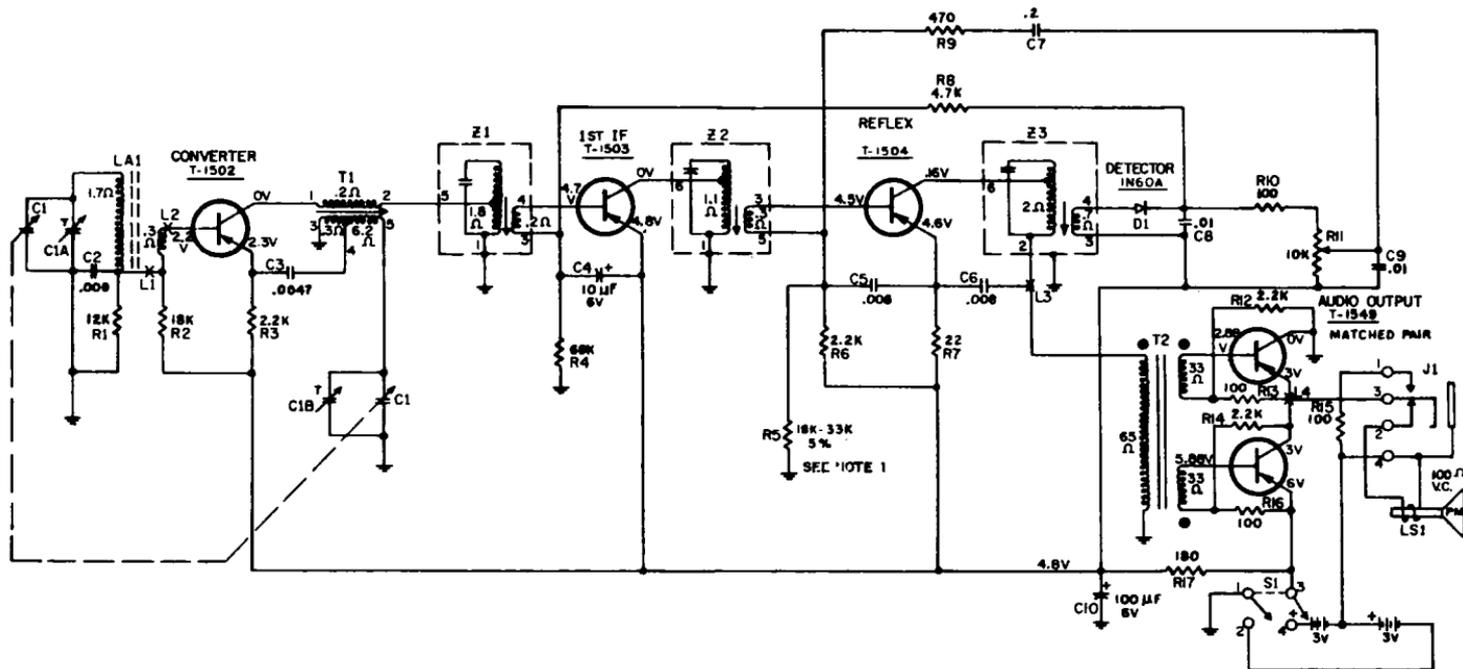
Fig. 8-5. Schematic diagram of the Philco model T-52.
