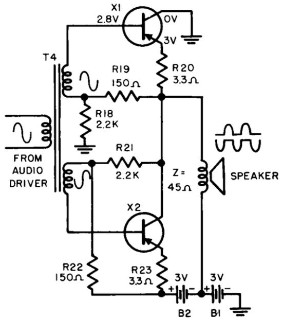
Fig. 4-9. The push-pull transformerless audio power circuit used in many commercial portable radios.
