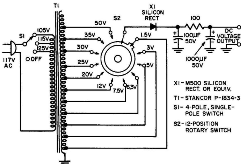
Fig. 11-8. Power supply for servicing transistorized equipment.
