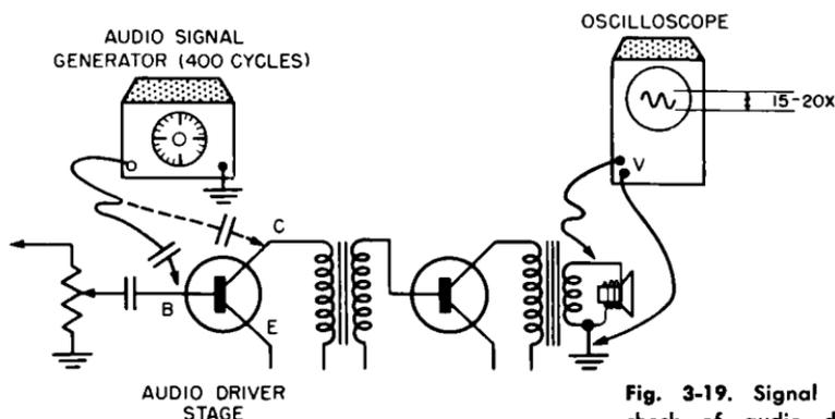
Fig. 3-19. Signal gain check of audio driver stage.
