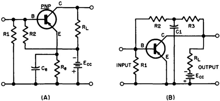
Fig. 3-9. (A) When an emitter resistor  $R_e$  is used to stabilize the circuit, it requires a bypass capacitor  $C_e$  to minimize losses due to degeneration. (B) Another method of bypassing is by splitting the voltage divider ( $R_2 - R_3$ ) and inserting  $C_1$  to bypass a-c variations.
