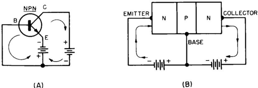
Fig. 1-13. The battery polarities shown here will forward bias the npn transistor, causing current to flow as indicated.
