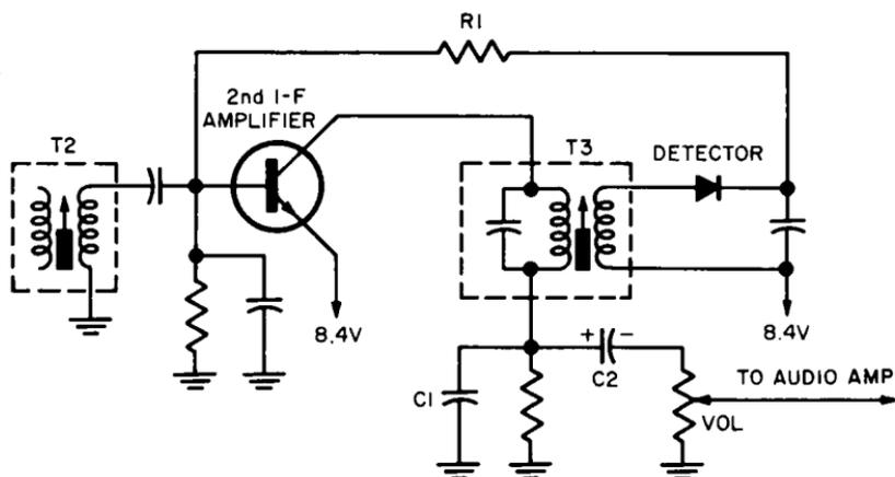
Fig. 5-4. A reflexed i-f audio amplifier. The circuit acts as both i-f and audio amplifier simultaneously with no interaction.
