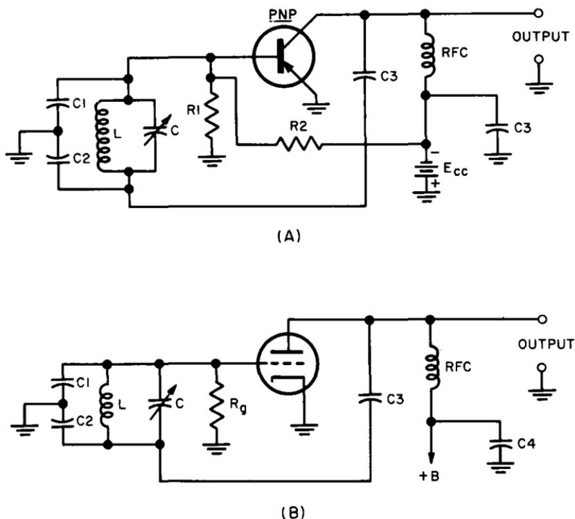
Fig. 6-3. (A) Transistorized Colpitts oscillator circuit. (B) Vacuum tube Colpitts oscillator circuit.
