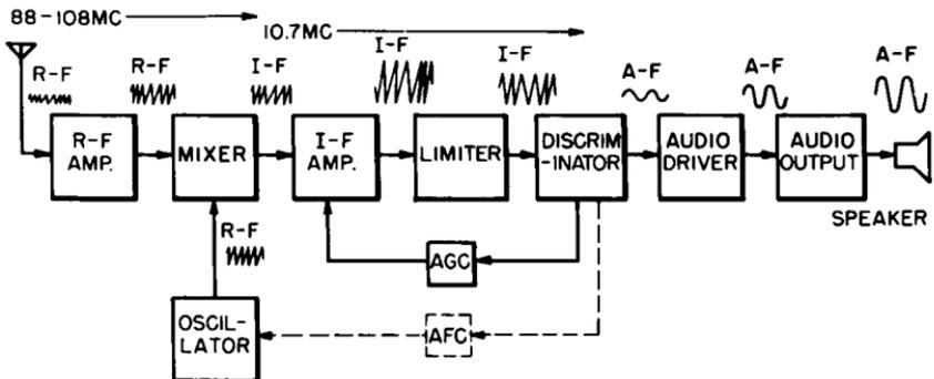
Fig. 2-3. Block diagram of a typical FM receiver (less power supply).
