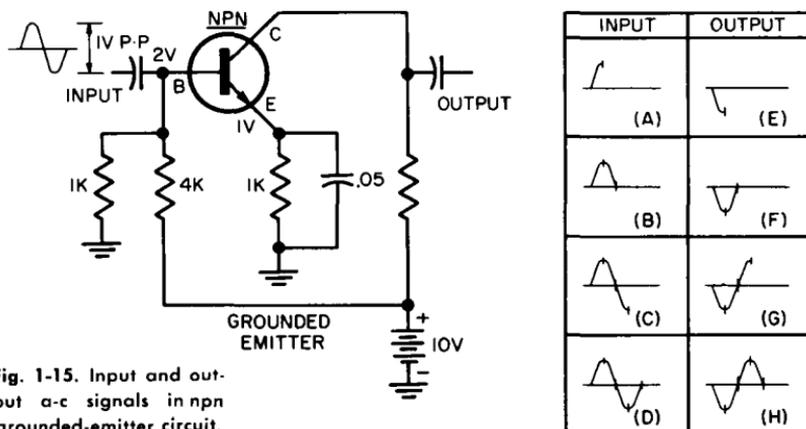
Fig. 1-15. Input and output a-c signals in npn grounded-emitter circuit.
