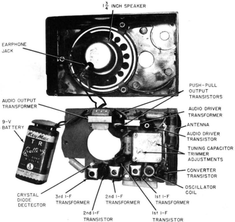
Fig. 8-11. A typical six-transistor Japanese radio chassis removed from its case.
