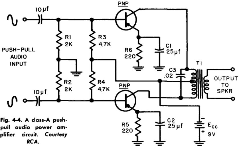
Fig. 4-4. A class-A push-pull audio power amplifier circuit. Courtesy RCA.
