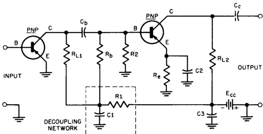
Fig. 3-13. Cascaded R-C coupled amplifiers require decoupling networks to prevent regenerative feedback.
