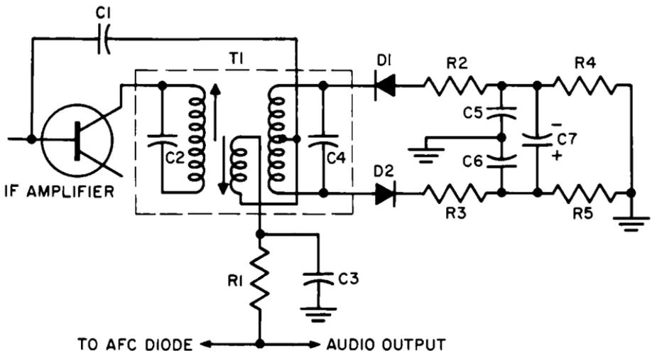
Fig. 7-6. FM ratio detector circuit.
