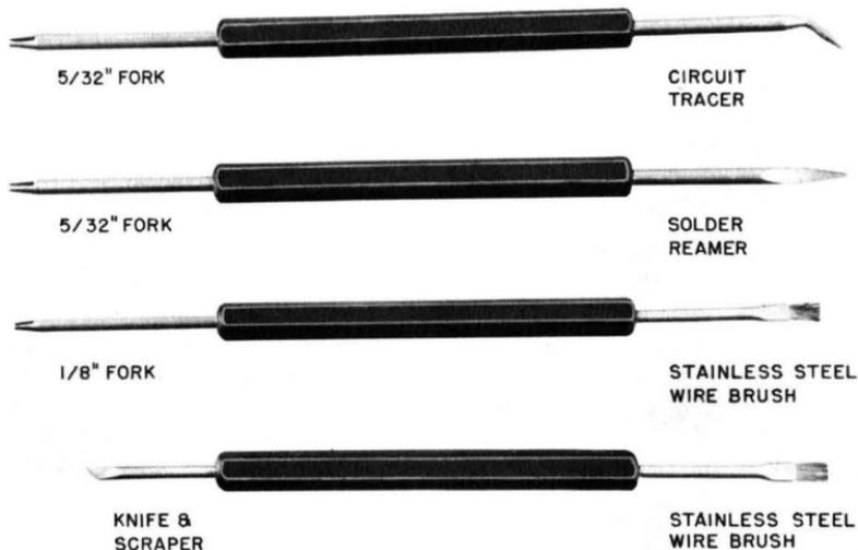
Fig. 11-4. Soldering aids. Courtesy Erikson Tool Co.
