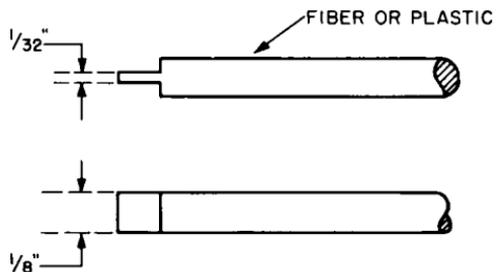
Fig. 5-10. Alignment tool.
