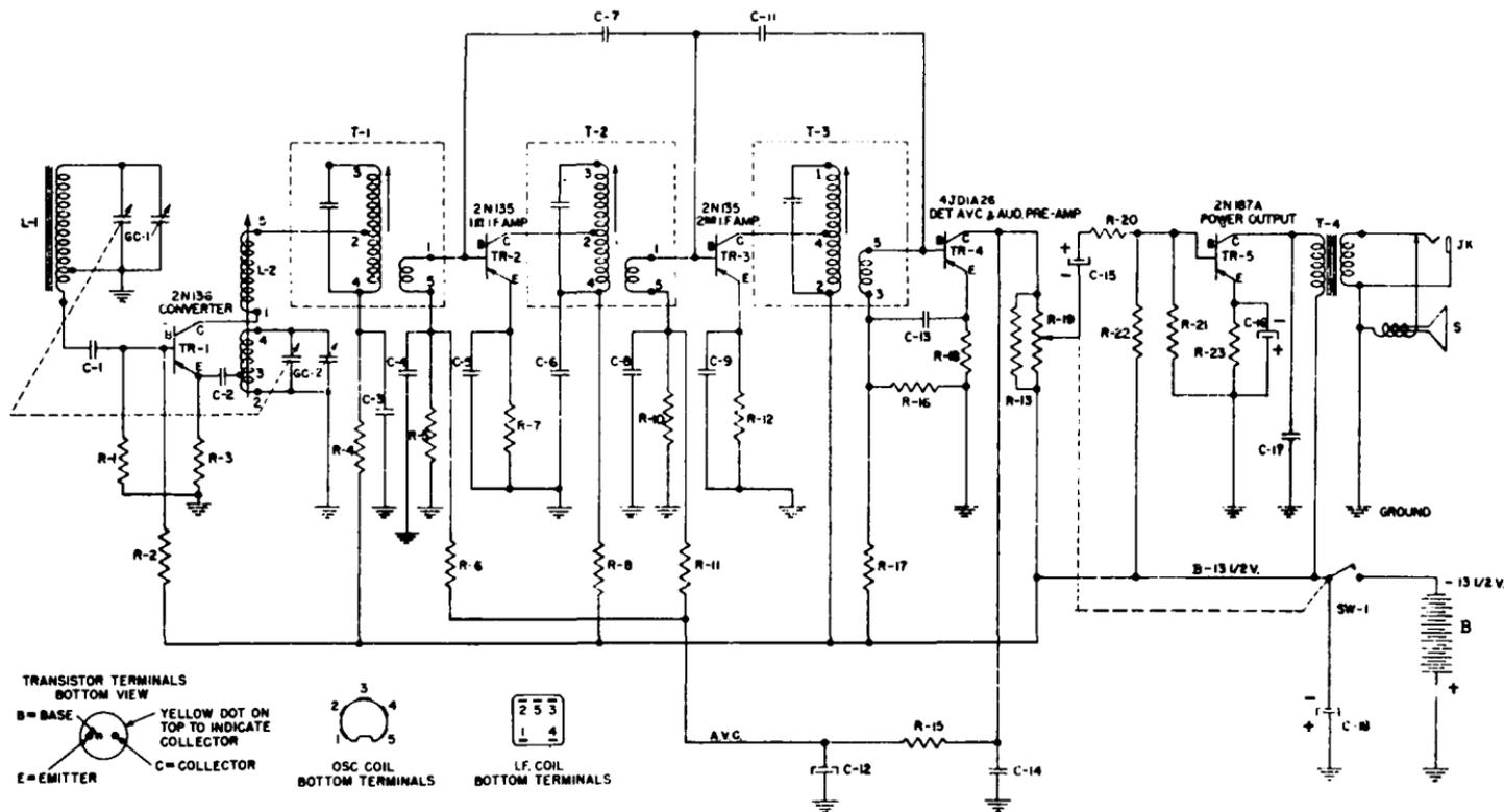
Fig. 8-4. Trav'ler model TR-250A five-transistor AM portable radio receiver. Note the use of a transistor in place of a diode as detector.
