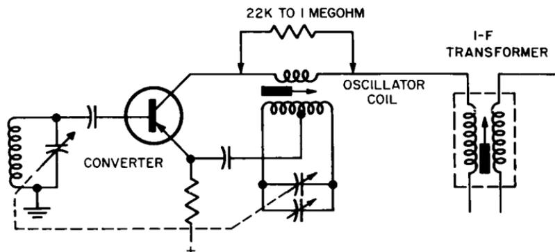
Fig. 6-14. A resistor is placed in shunt with the oscillator coil primary winding to reduce the oscillator voltage where excessive voltage causes whistling.
