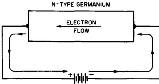
Fig. 1-6. Conduction in n-type germanium is by electron flow from the negative side of the battery to the positive side.
