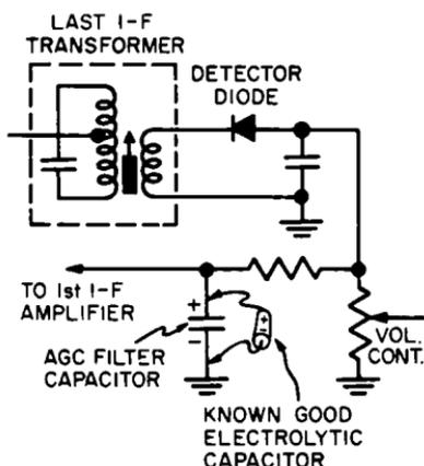
Fig. 7-11. Checking the agc filter capacitor for open condition.
