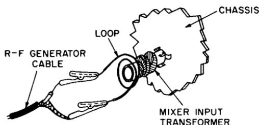
Fig. 6-10. A 2- to 3-loop wire placed across the r-f generator output cable is used to couple the r-f signal to the mixer input transformer.
