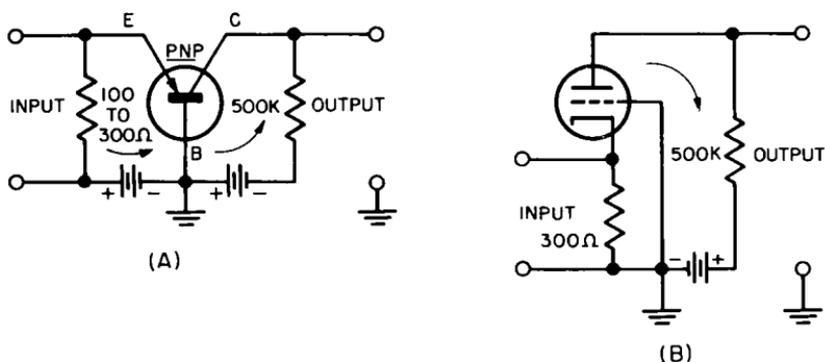
Fig. 3-1. (A) Grounded-base transistor amplifier compared to (B) conventional grounded-grid vacuum tube amplifier.
