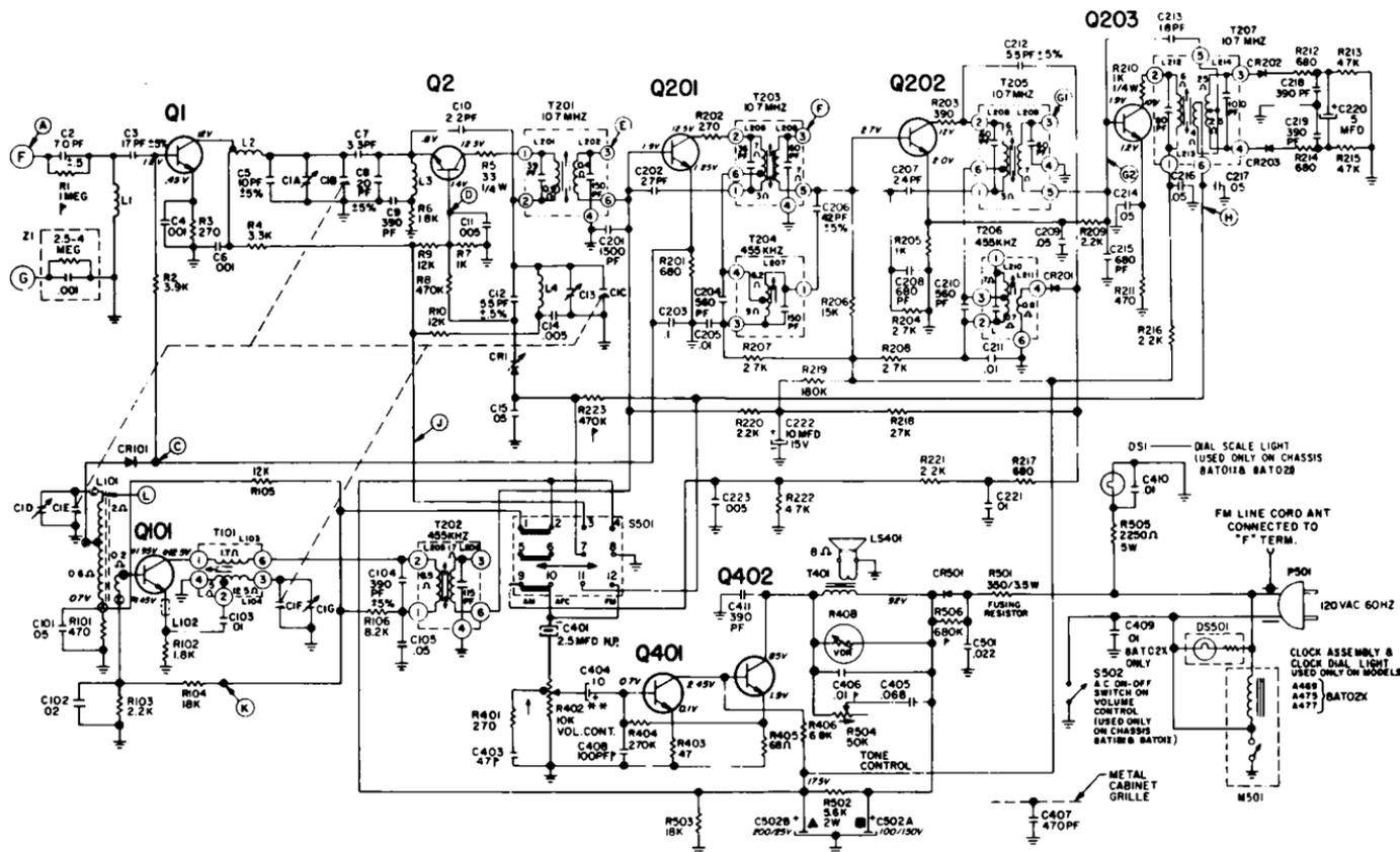
Fig. 8-16. Zenith model A418 AM-FM radio.
