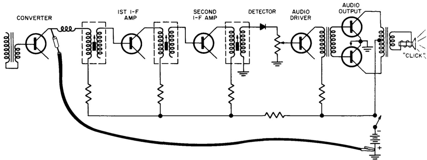
Fig. 10-2. Click test for transistorized radios. When the end of the resistor is momentarily touched to the collector of the converter transistor, a click is heard from the loudspeaker.
