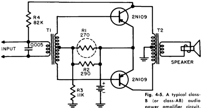
Fig. 4-5. A typical class-B (or class-AB) audio power amplifier circuit.
