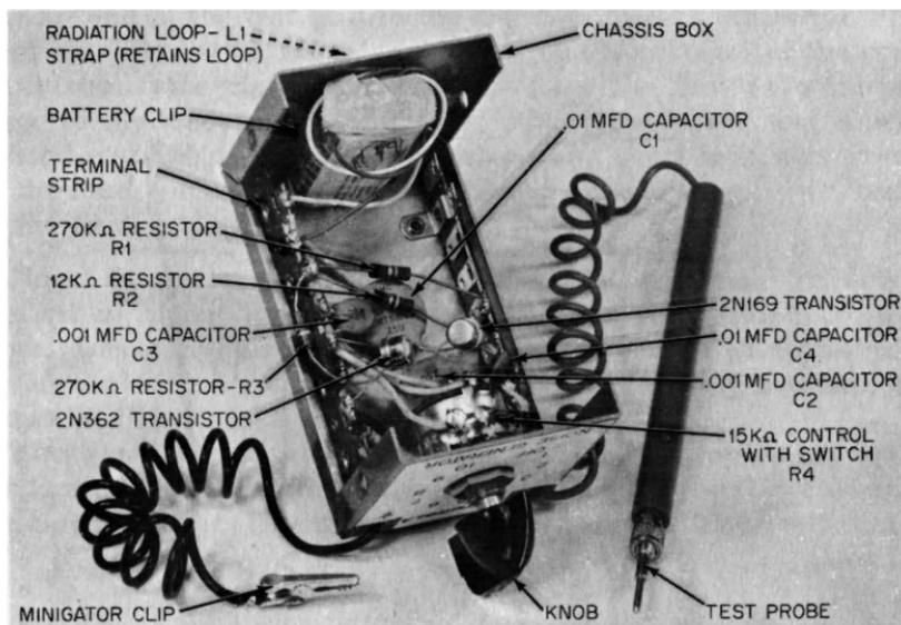
Fig. 10-3. Interior view of a noise generator. Courtesy Motorola.
