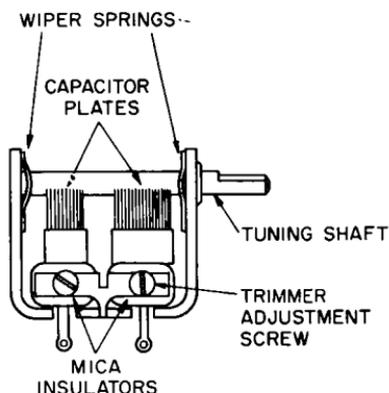
Fig. 6-12. A typical tuning capacitor used in transistorized radios.
