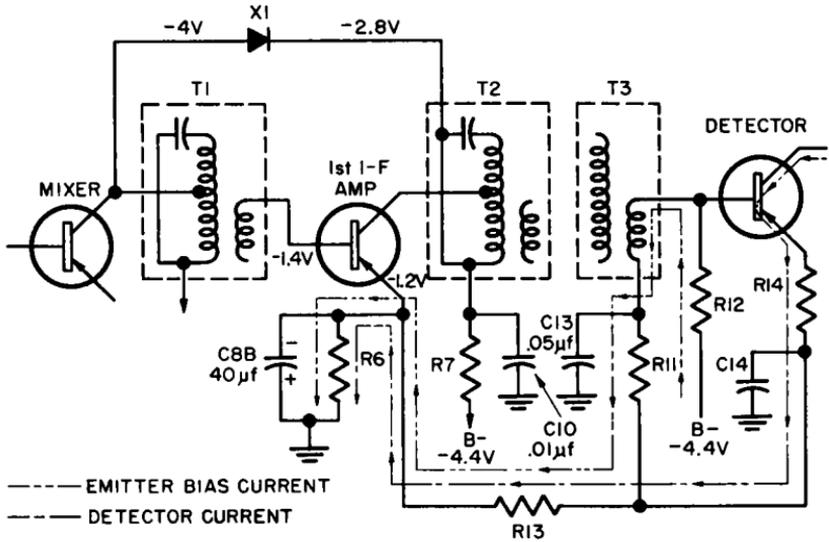
Fig. 7-3. Detector-afc circuit employing an overload diode X1 to prevent distortion on strong signals. The conduction of X1 is controlled by the first i-f amplifier's emitter bias voltage.
