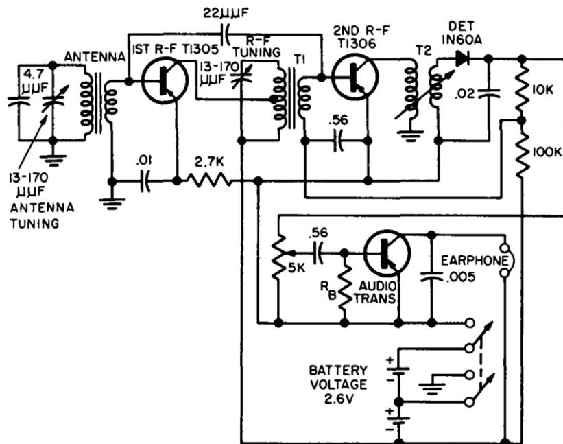
Fig. 8-2. Philco model T-3 three-transistor trf-type portable AM radio receiver.
