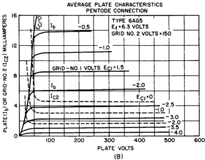
Fig. 3-5. Comparison between the operation characteristic curves for (A) a 2N105 pnp junction transistor and (B) a 6AG5 vacuum tube. Courtesy RCA.
