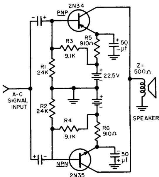
Fig. 4-10. A complementary-symmetry amplifier circuit.
