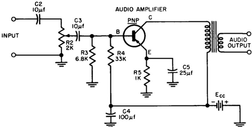
Fig. 3-15. Location of gain control in an R-C coupled amplifier circuit.
