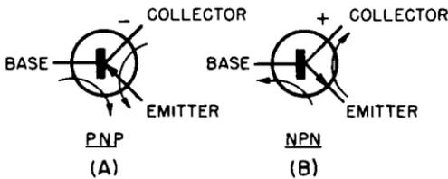
Fig. 1-12. (A) Conduction in a pnp transistor is from base to emitter and from collector to emitter. (B) Conduction in an npn transistor is from emitter to base and from emitter to collector. The arrow in the emitter element is opposite in direction to the electron flow.
