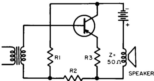
Fig. 4-7. A class-A grounded emitter transformerless power amplifier.
