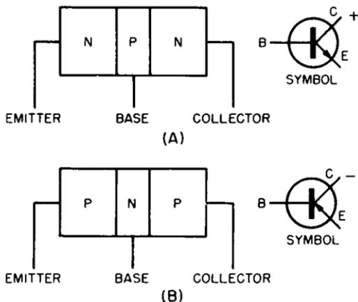
Fig. 1-11. (A) A junction-type npn transistor is constructed by sandwiching a piece of p-type material between two pieces of n-type. Symbol of an npn transistor is shown at the right. (B) A junction-type pnp transistor is constructed by sandwiching a piece of n-type material between two pieces of p-type. Symbol of a pnp transistor is shown at the right.
