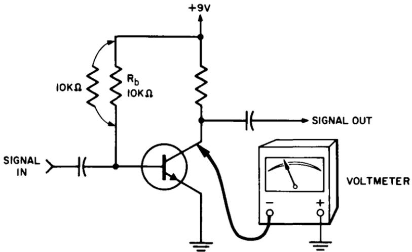
Fig. 10-10. In-circuit transistor testing of self-bias amplifier.
