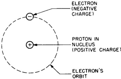
Fig. 1-1. The hydrogen atom is composed of a single proton in the nucleus and one electron orbiting around it. This is the simplest of all atoms.
