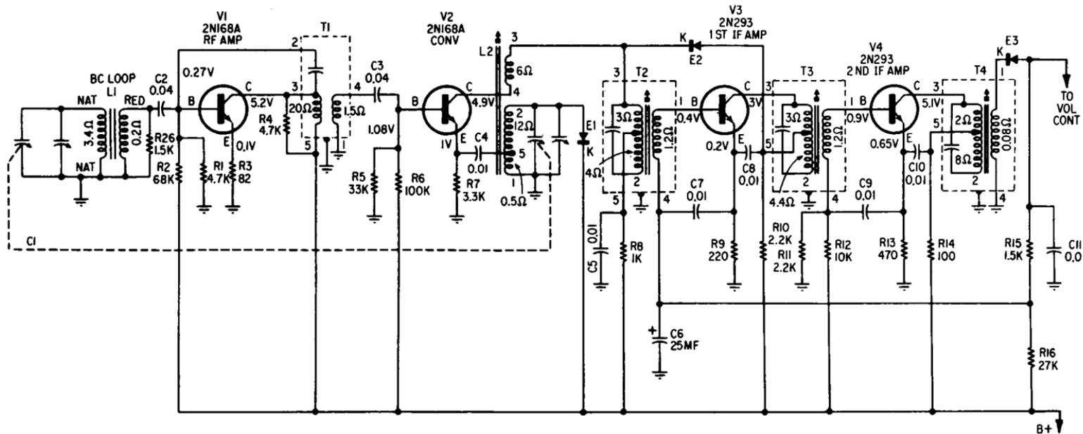
Fig. 8-8. Seven-transistor radio receiver using an r-f amplifier
