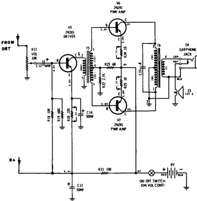
Fig. 8-8. Seven-transistor radio receiver using an r-f amplifier
