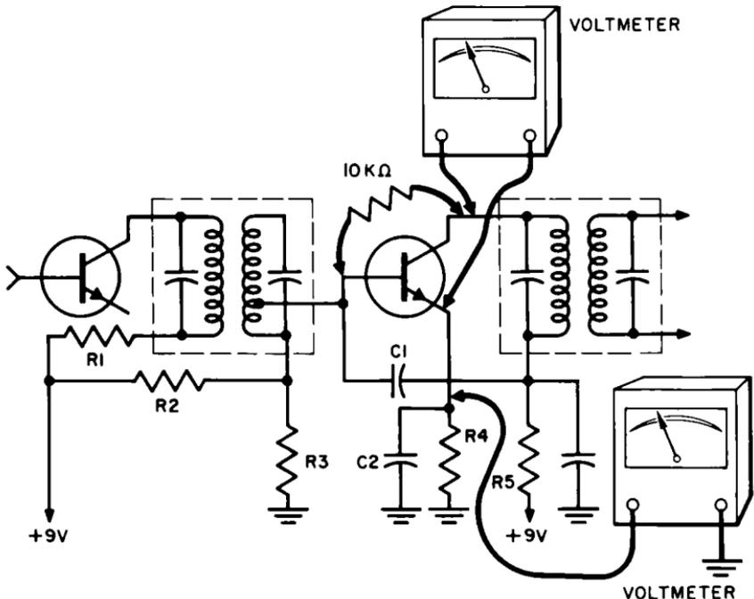
Fig. 10-9. In-circuit transistor testing.
