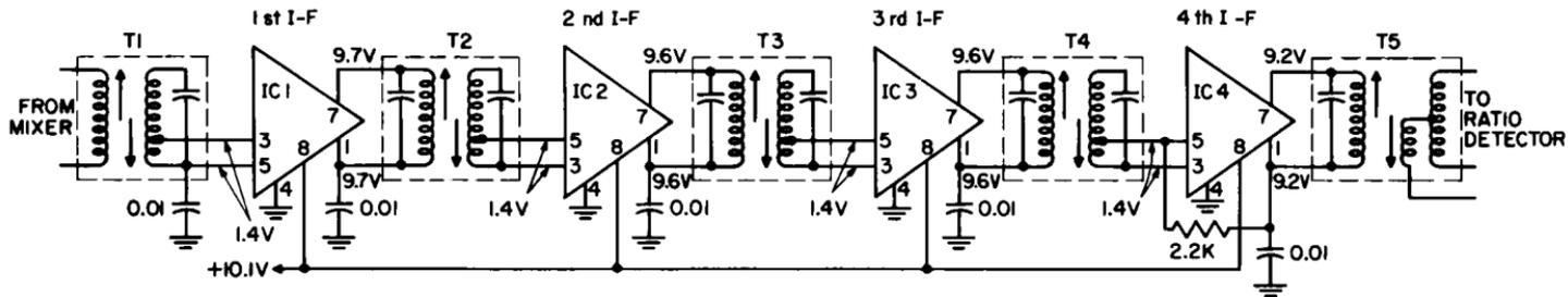
Fig. 10-19. FM i-f amplifier section of AM-FM auto radio (Motorola model FM 108M).
