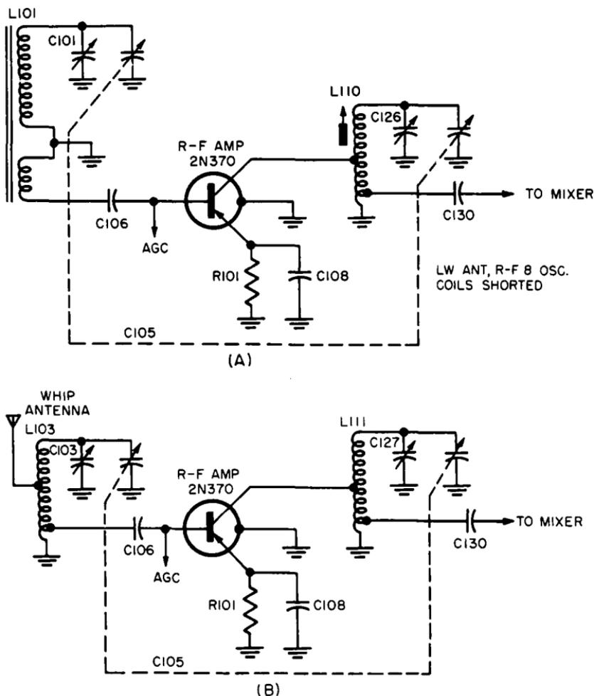
Fig. 8-15. Simplified schematic of Sears Roebuck model 222. (A) R-F amplifier circuit in BC position. (B) R-F amplifier circuit in S1 position (S2 is the same with the exception of tuned circuit changes).
