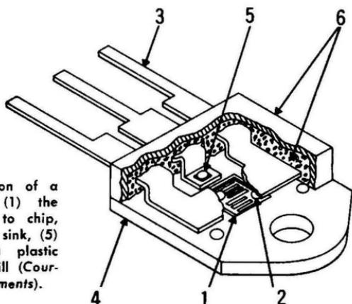
Fig. 4-1. Construction of a power transistor: (1) the chip, (2) contacts to chip, (3) leads, (4) heat sink, (5) collector lead, (6) plastic case with epoxy fill (Courtesy Texas Instruments).
