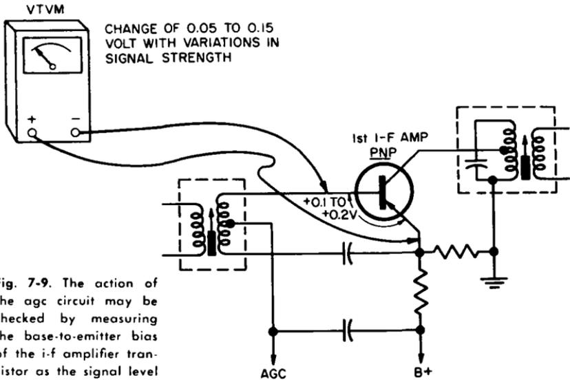
Fig. 7-9. The action of the agc circuit may be checked by measuring the base-to-emitter bias of the i-f amplifier transistor as the signal level is varied.
