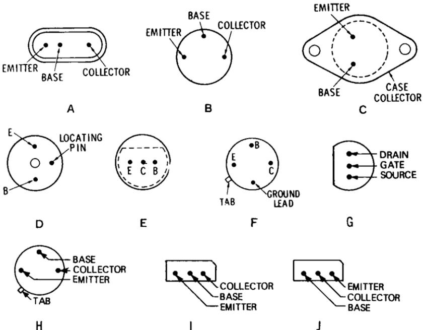
Fig. 10-13. Lead configurations commonly used on transistors.
