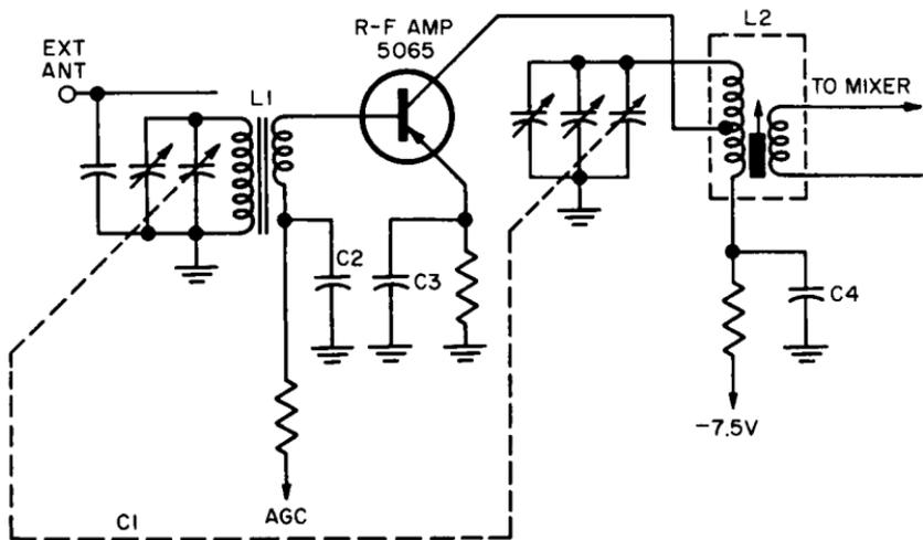
Fig. 5-5. A tuned r-f amplifier using a common-emitter circuit. This amplifier circuit is used to tune the standard broadcast band.
