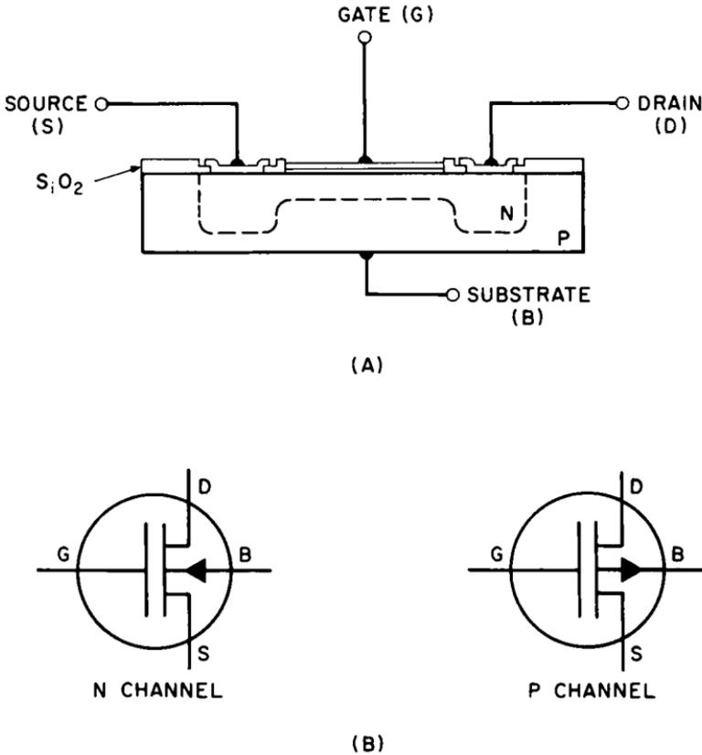
Fig. 1-22. MOS-FET transistor, depletion type: (A) construction, and (B) schematic symbols.
