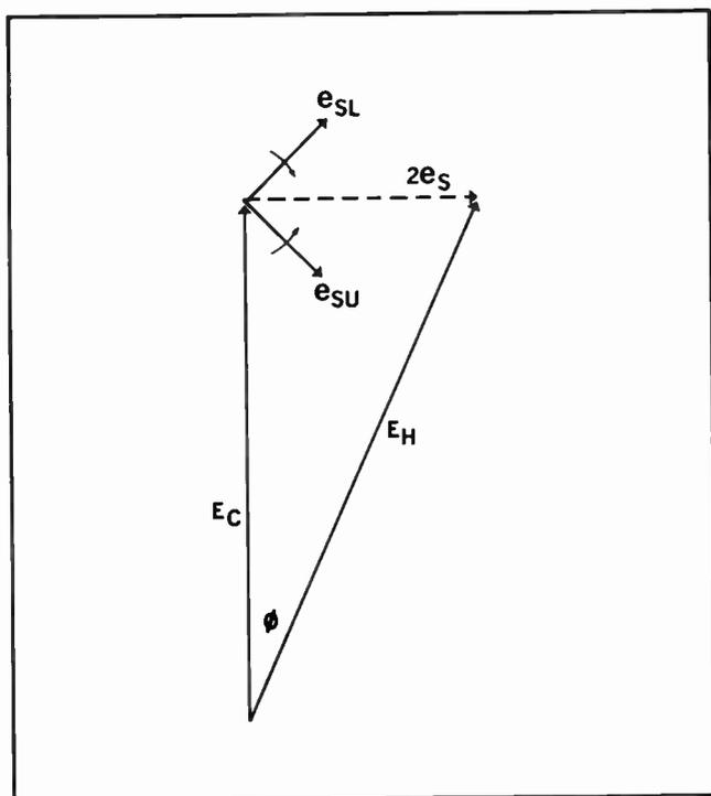
Figure 3-4. Vector representation of phase noise modulation
