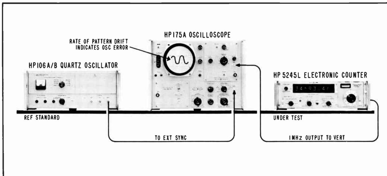
Figure 3-2. Equipment to check a counter's internal oscillator.
