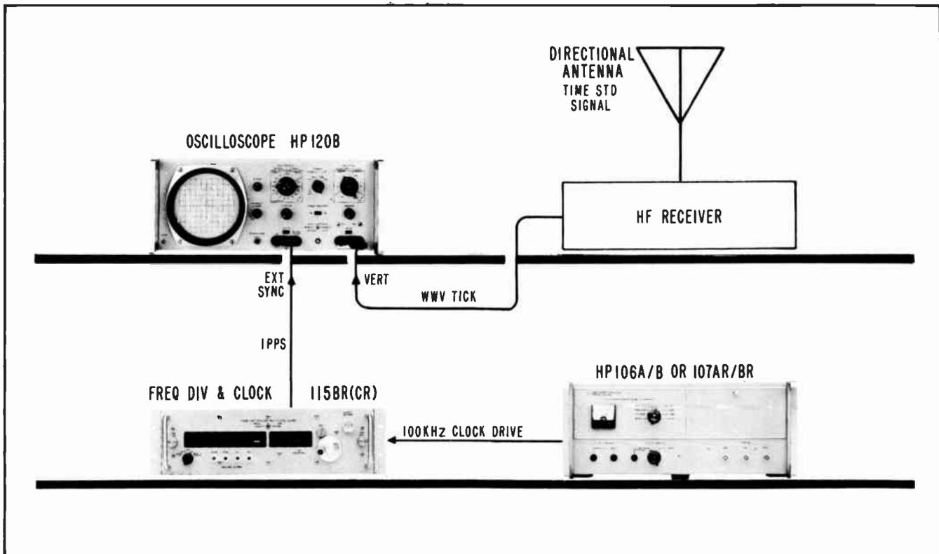
Figure 2-1. Equipment for time comparison with tick phasing adjustment
