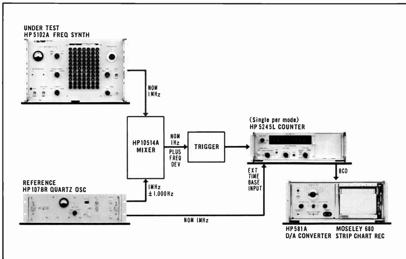
Figure 3-3. Block diagram for frequency comparison measurements.
