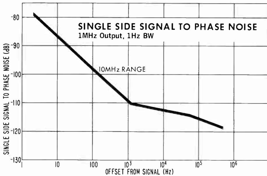
Figure 3-6. 5103A Frequency Synthesizer Phase Noise Plots
