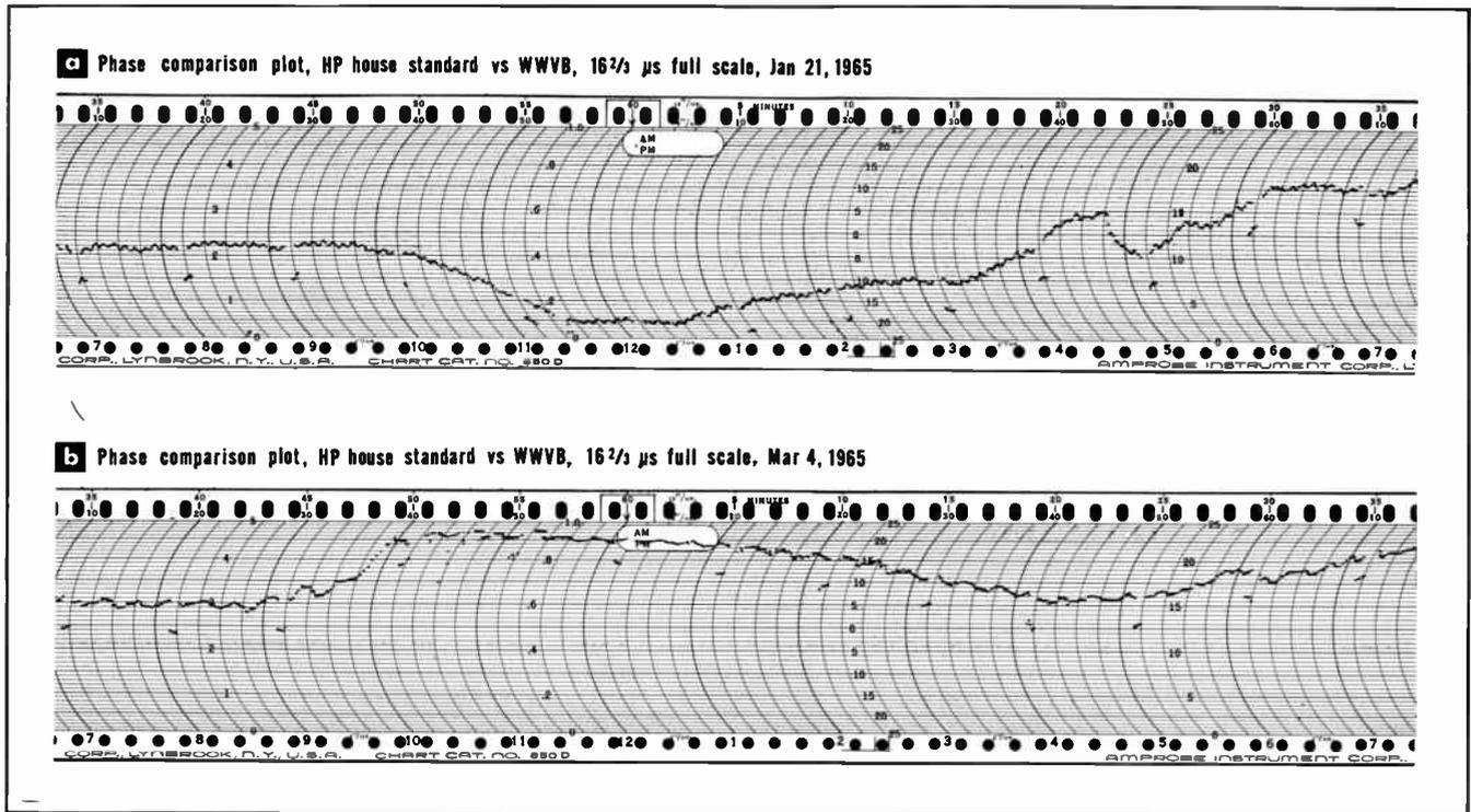
Figure 2-11. Phase comparison recordings showing effects of propagation anomalies
