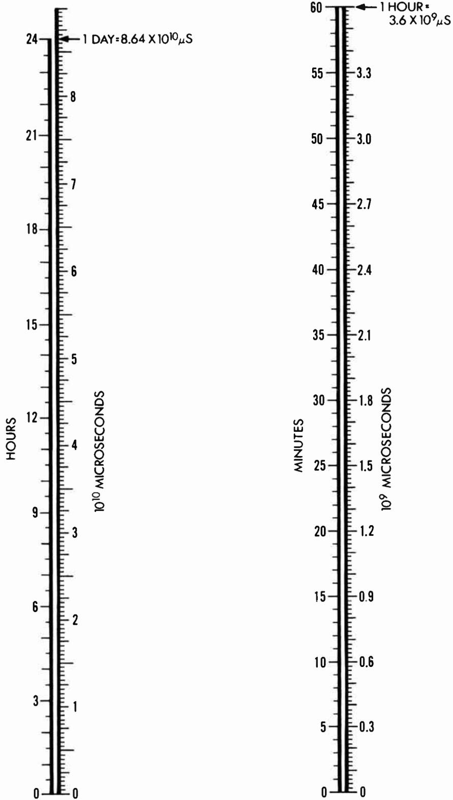
Figure IV-1. Conversion Chart - Hours & Minutes to Microseconds
