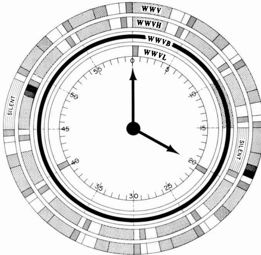
SECONDS PULSES - WWV, WWVH - CONTINUOUS EXCEPT FOR 59<sup>th</sup> SECOND OF EACH MINUTE AND DURING SILENT PERIODS
