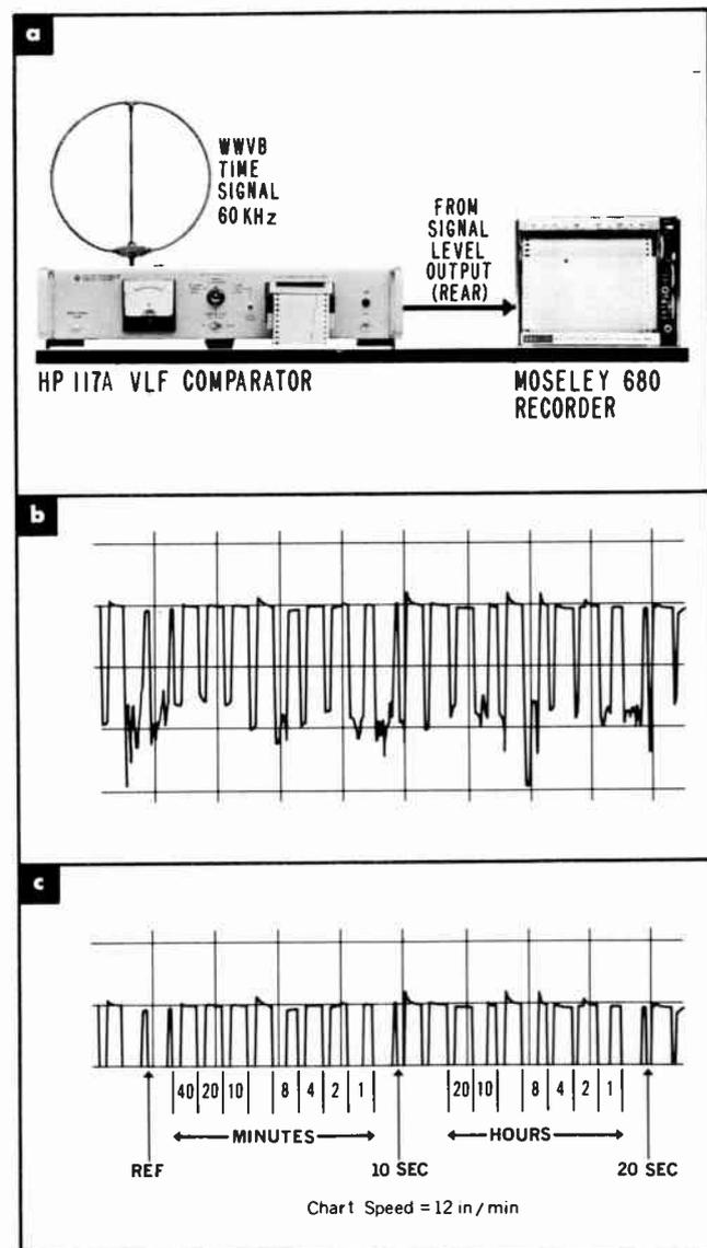
Figure 2-13. Equipment to produce a time record (a), a trace (less than a minute) produced with this equipment (b), and the same trace with a template superimposed to aid in its interpretation (c).
