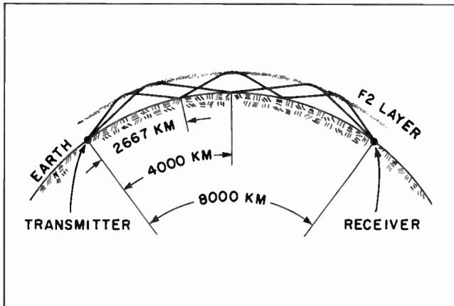
Figure 4-4. Multiple-hop transmission path
