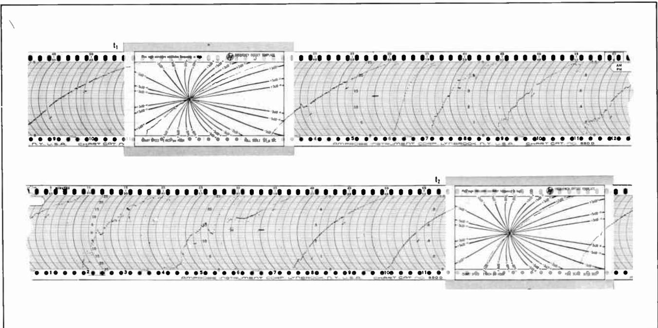
Figure 2-9. Use of template to interpret 117A recording
