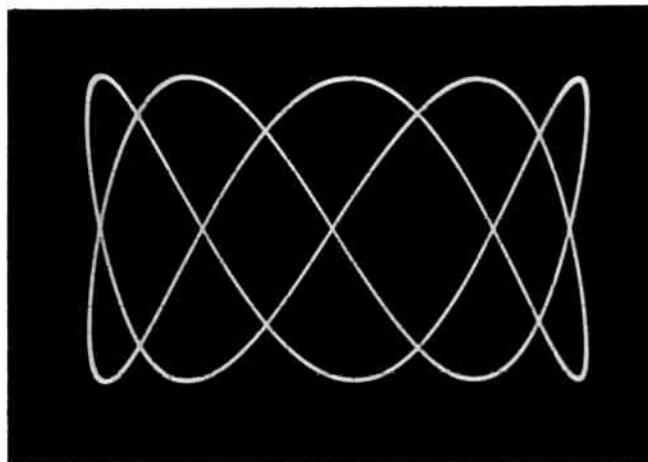
Figure 3-1. Lissajous pattern (frequency ratio 5:2).
