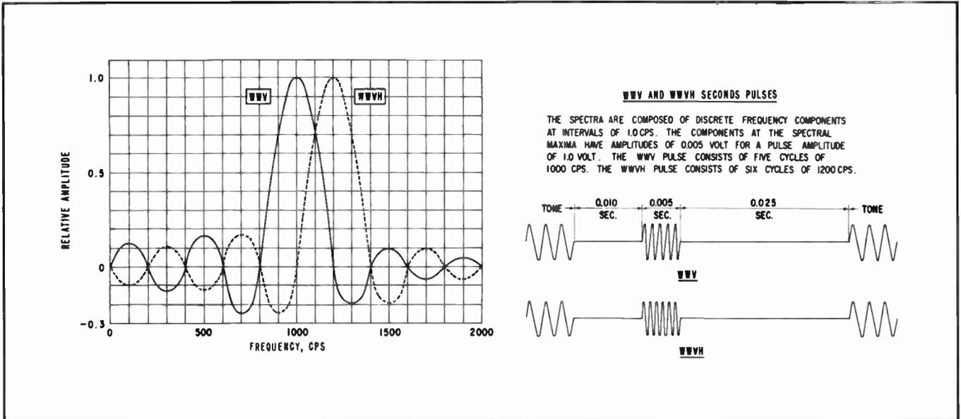
Figure III-2. Sample Characteristics of Time Pulses Broadcast from NBS Stations WWV and WWVH.
