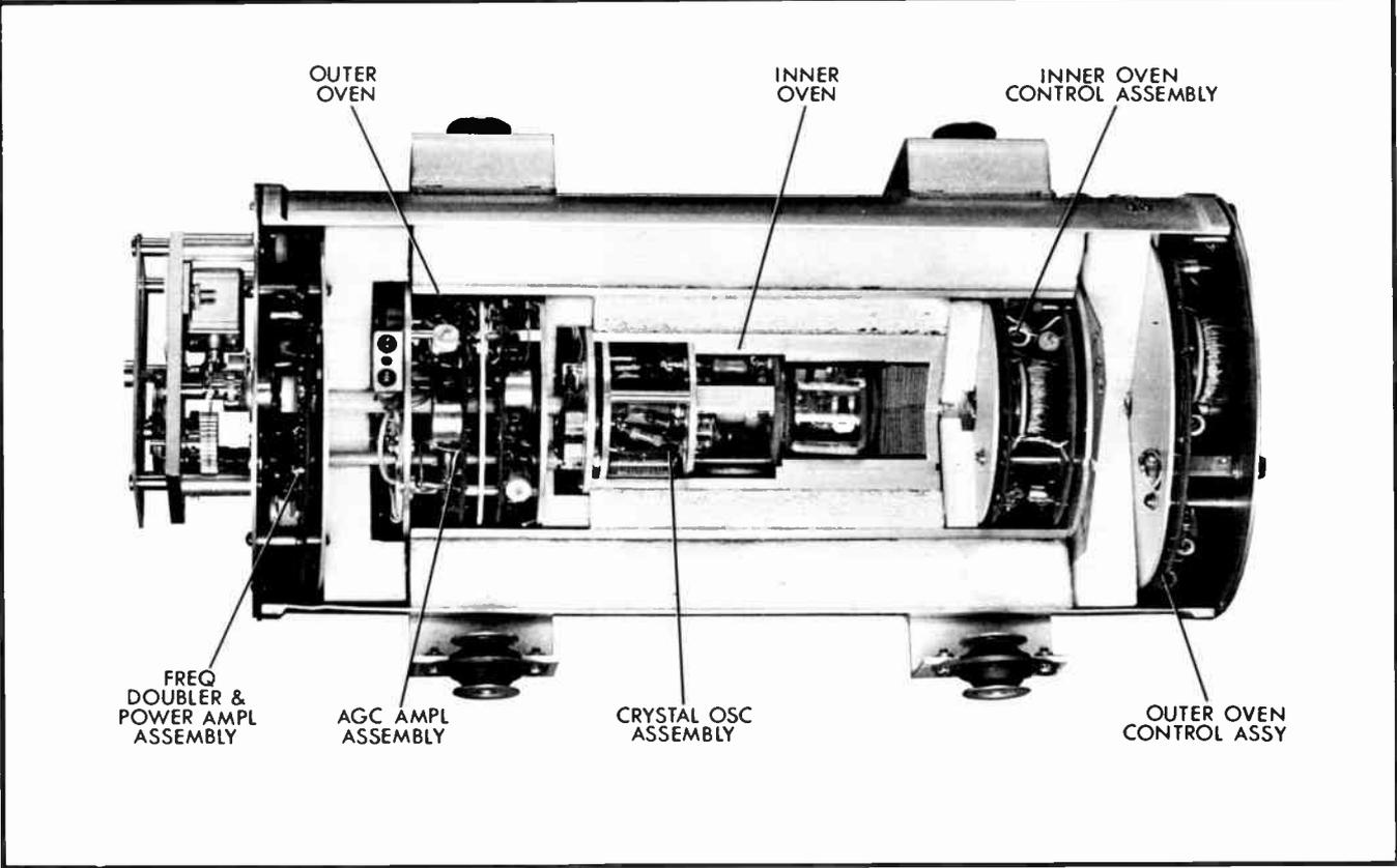
Figure 5-5. Schematic of 106A, B Oscillator and cutaway view of crystal oven assembly
