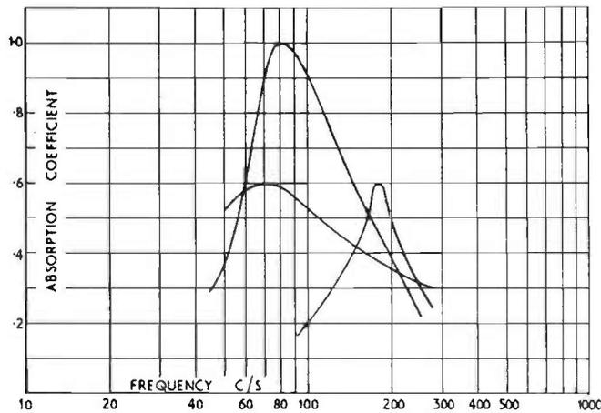
FIG. 17.24. Typical absorption characteristics of resonant absorbers.
