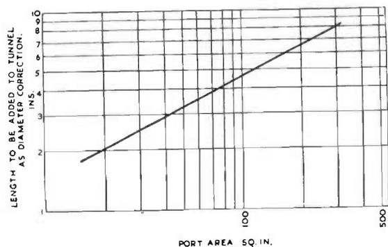
FIG. 16.28. Tunnel correction.
