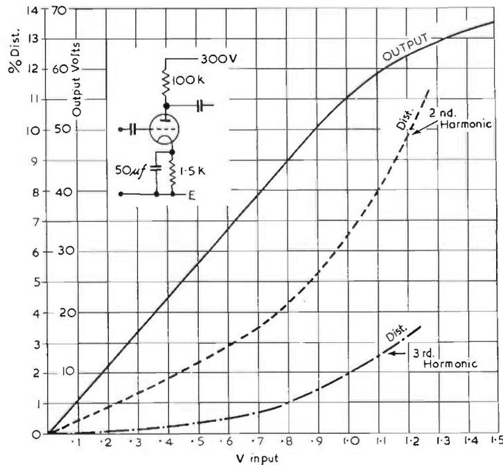
FIG. 9.33. Performance as a straight amplifier of the twin triode used in the phase splitter circuit. (ECC 83)
