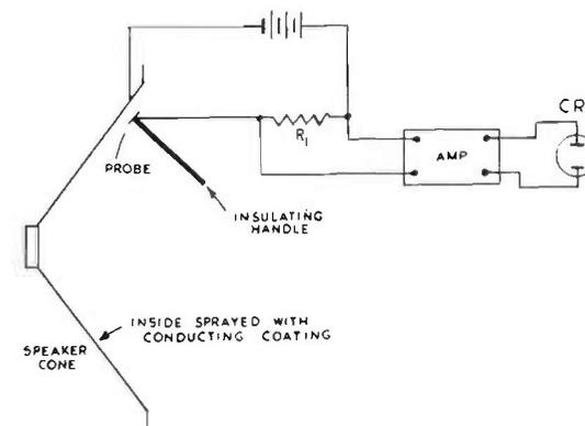
FIG. 16.15. Schematic arrangement for investigating cone motion.
