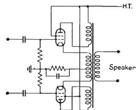
FIG. 10.16. Cathode loaded output stage.
