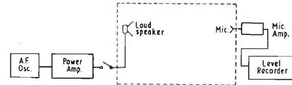
FIG. 17.7. Schematic arrangement for measuring reverberation time.
