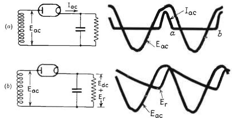
FIG. 14.3(a)-(b). Half wave rectifiers with resistance-capacitance load.
