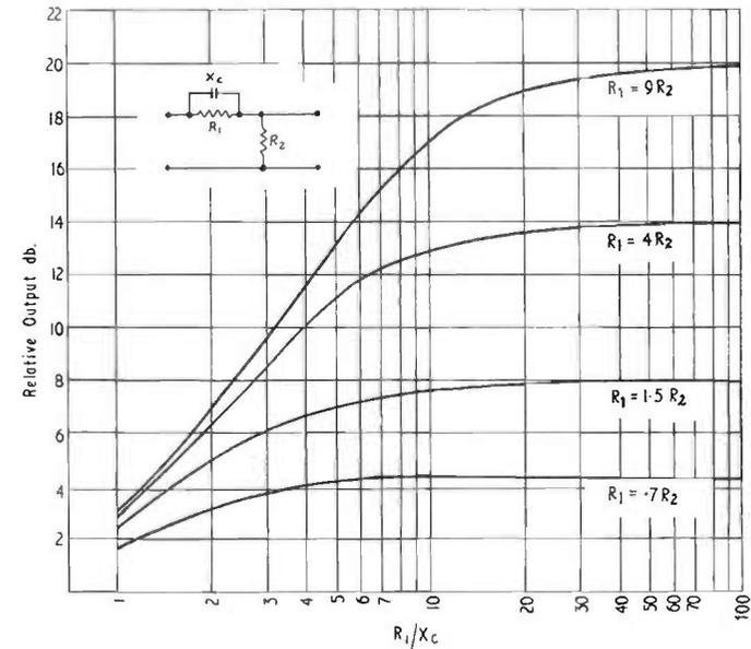
FIG. 13.9. Design curves for top boost circuit.
