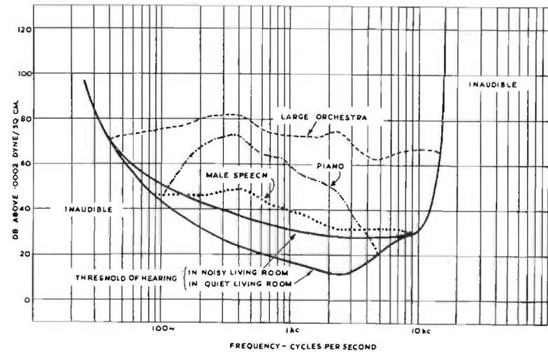
FIG. 3.11. R.M.S. intensity distribution as a function of frequency for large orchestra, piano and male speech. Data from Table 3.2.
