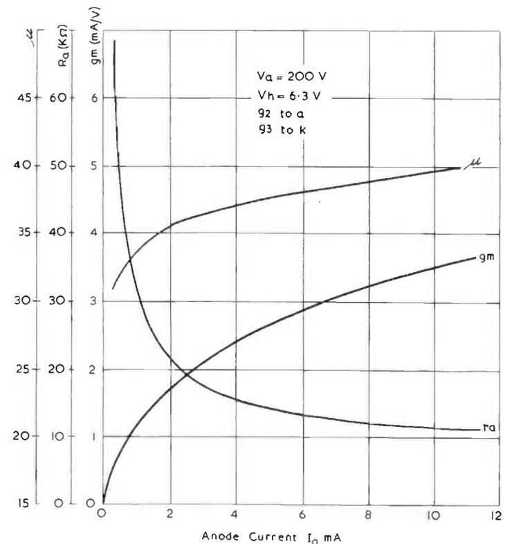
FIG. 9.17(a). Change in triode parameters with anode current.
