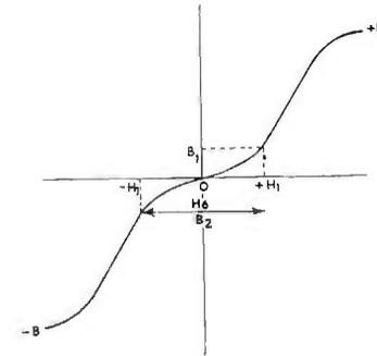
FIG. 8.4. Transfer characteristic without H.F. bias.
