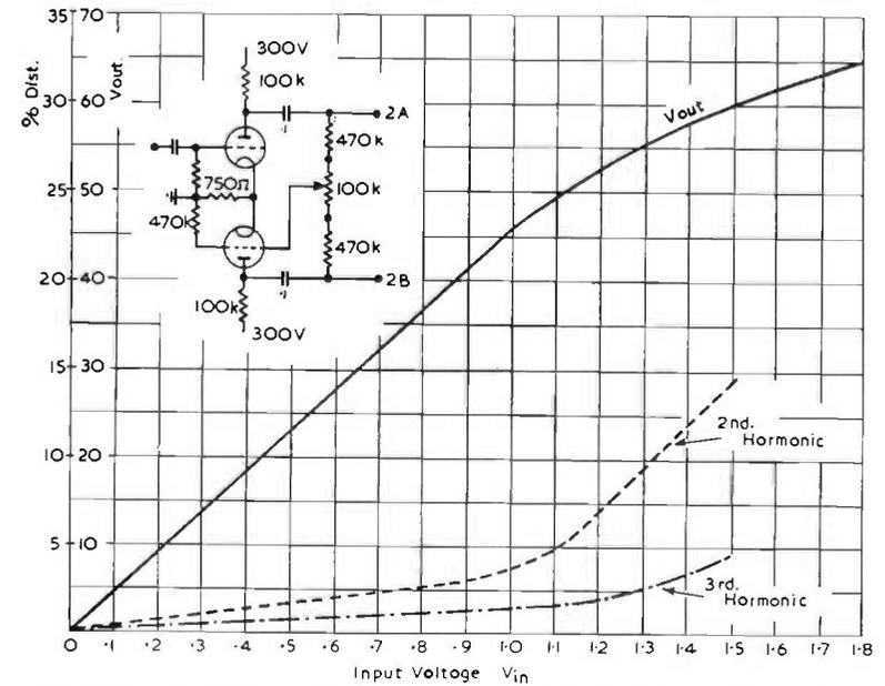
Fig. 9.31. Performance of a twin triode valve as a paraphase phase splitter.
