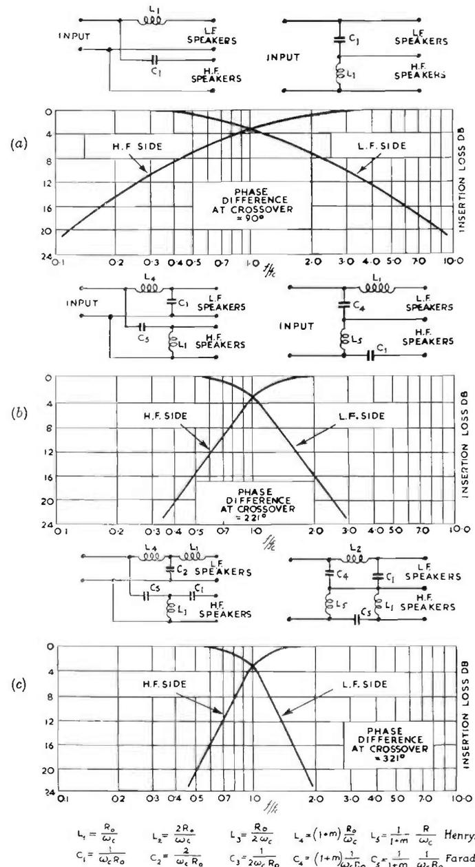
Fig. 15.3(a)-(c). Filter dividing networks design and performance.
