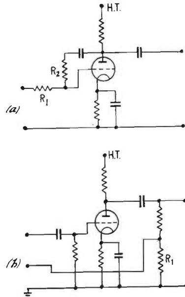
FIG. 13.12(a-b). Single valve feedback tone control circuits.
