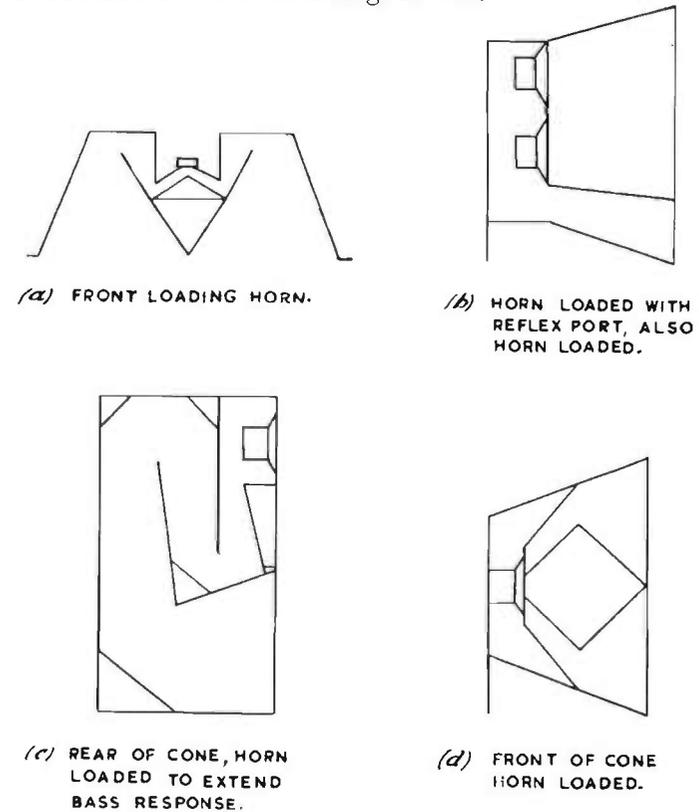
FIG. 16.44. Typical folded horn speakers.
