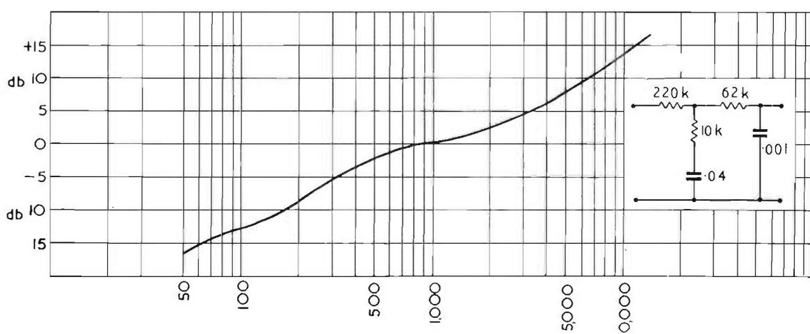
FIG. 7.29(g). The present international standard recording characteristic for 33 and 45 R.P.M. recordings. British Standard "Fine Groove," A.E.S., R.I.A.A. and I.E.C. The RC network shown provides the correction required on replay.
