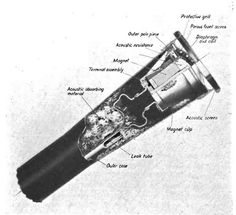
FIG. 5.8(a). S. T. & C. 4037 cutaway view of tubular moving-coil microphone.
