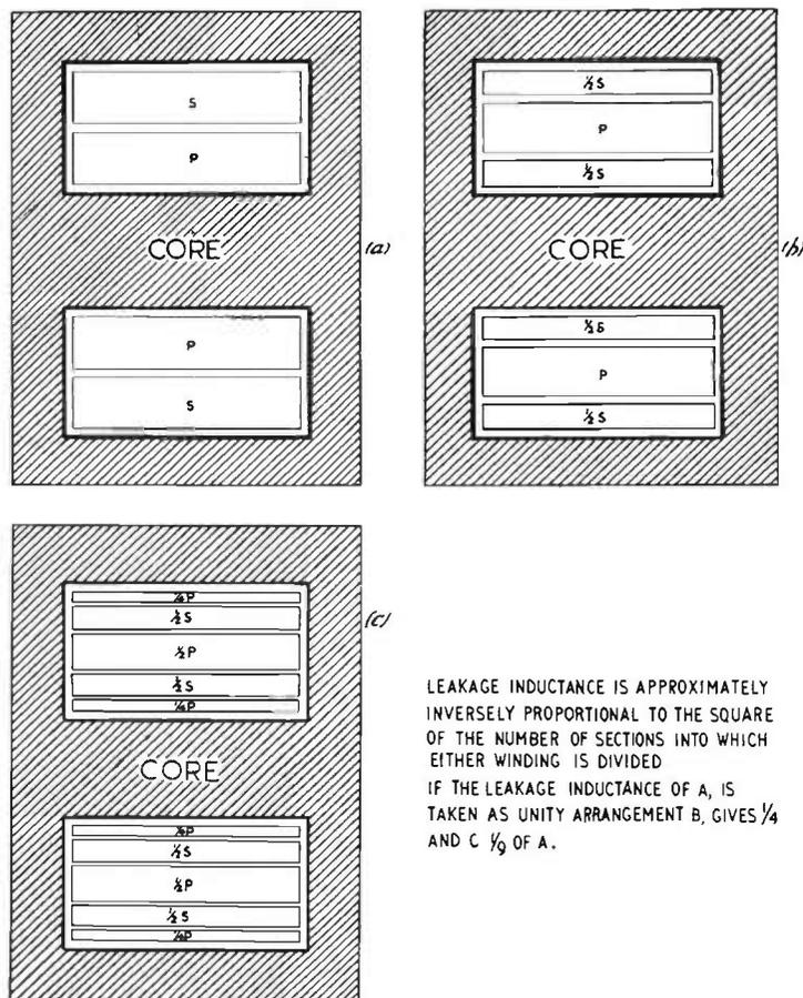
FIG. 11.7. Sectionalized windings to reduce leakage inductance.
