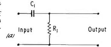
Max. slope  $n \times 6\text{dB/octave}$  where  $n$  = number of meshes. Attenuation at any frequency from Fig. 13.2.
