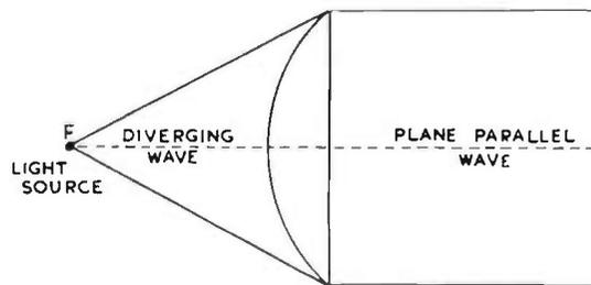
FIG. 16.49(a). Optical plano convex lens.
