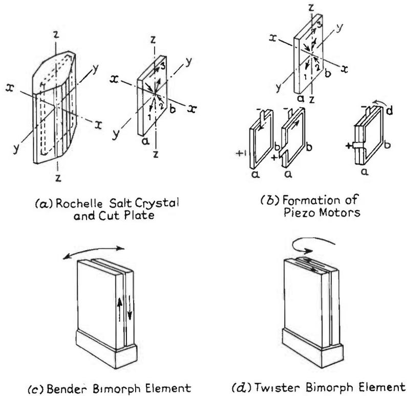
FIG. 5.11(a)-(d). Construction of bimorph unit of Piezo-electric microphone.
