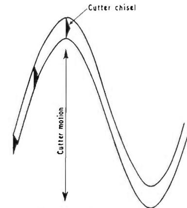
FIG. 7.6. Origin of 'pinch effect'. Cutter chisel constrained to move along the disk radius cuts a groove of variable width having the same width as the cutter only at the peaks of the wave.
