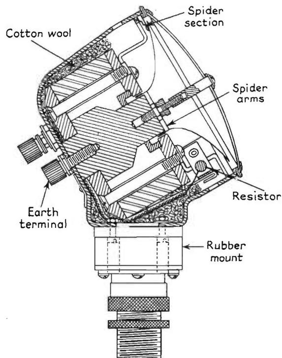
FIG. 5.3. Moving coil microphone (B.T.-H.).
