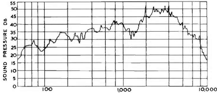
FIG. 16.24. Frequency characteristic of 12-in. loudspeaker in 5-ft. pipe.
