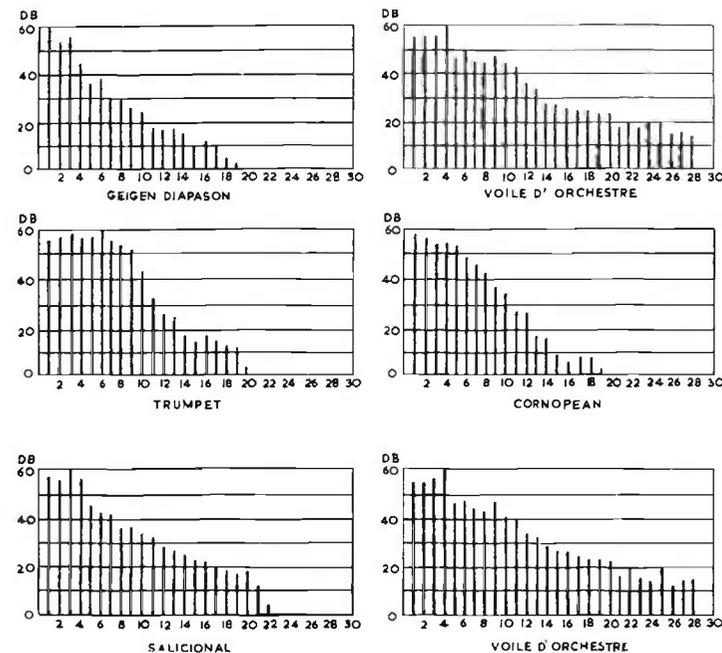
FIG. 1.12. Typical harmonic structure of five 'Instruments' in a modern theatre organ.
