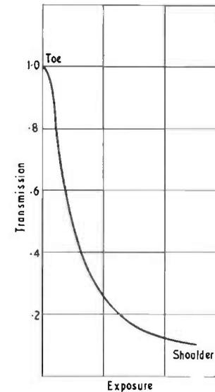
FIG. 18.9 (b). Exposure/transmission relation corresponding to the *H* and *D* curve of (a).  $\gamma = 1.0$ .
