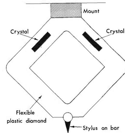
FIG. 7.23. Resolving linkage applied to a piezo-electric pick-up.
