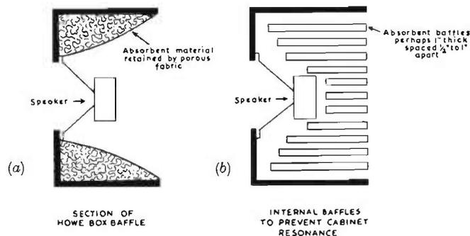
FIG. 16.19. Damping of open backed cabinets.
