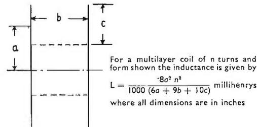
FIG. 15.7. Filter inductance coils.
