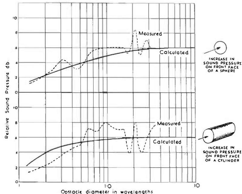
FIG. 5.2. Sound field distortion due to diffraction at an obstacle.
