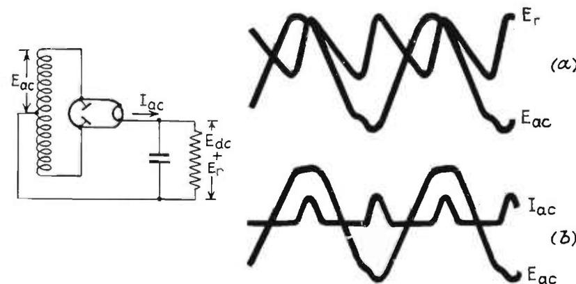
FIG. 14.4(a)-(b). Full wave rectifier circuit.
