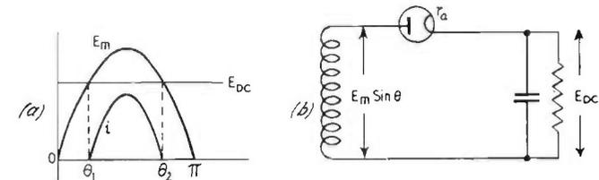
FIG. 14.7. Current pulse and voltage relations in a half wave circuit.
