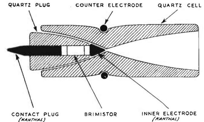
FIG. 16.38. Glow discharge cell used in Ionophone loudspeaker.
