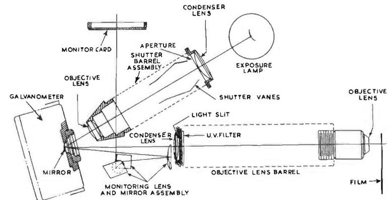
FIG. 18.8. Optical system for RCA variable-width recording.
