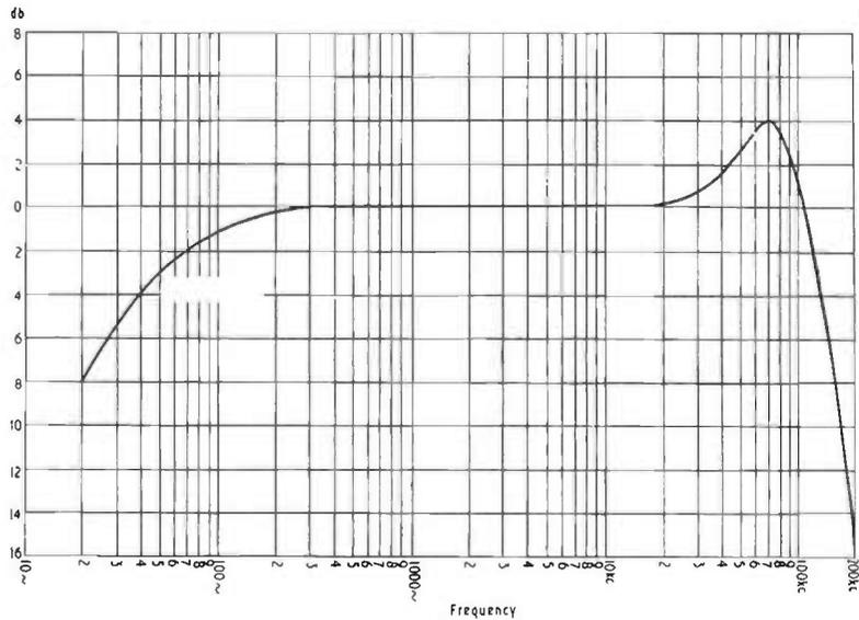
FIG. 11.6. Typical output transformer characteristic indicating resonance at 70 kc/s.
