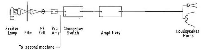
FIG. 18.3. Schematic arrangement of sound film reproducer system.
