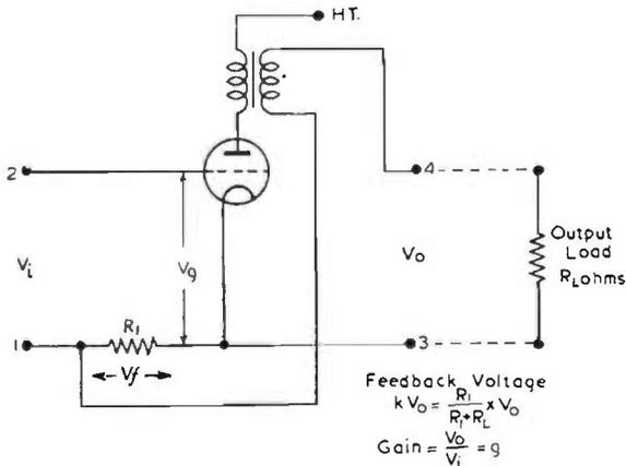
FIG. 12.2. Negative current feedback.
