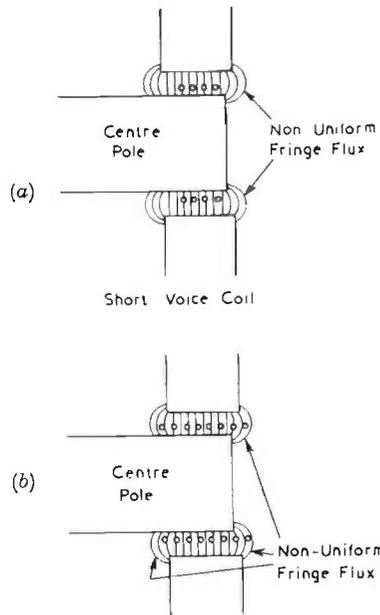
FIG. 16.8. Methods of reducing amplitude distortion due to non-uniform gap density. (a) Short voice call. (b) Long voice call.
