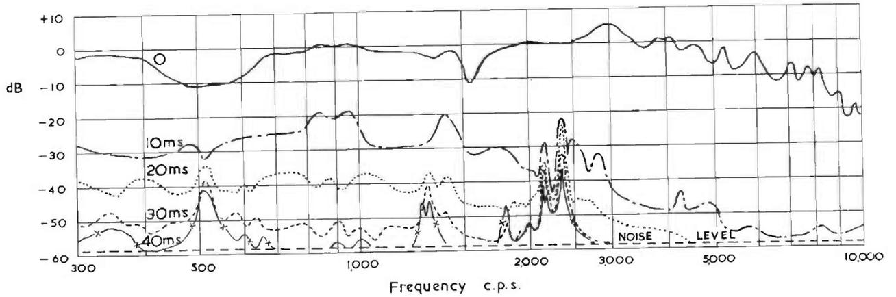
FIG. 16.12. Transient response curves. (b) Speaker No. 2. Produces a 'tunnelled' effect at middle frequencies with dirty top.
