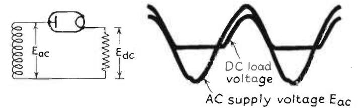
FIG. 14.2. Half wave rectifier circuit with resistance load.
