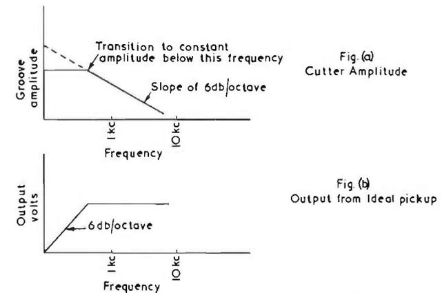
FIG. 7.3. Recording and reproducing characteristics.
