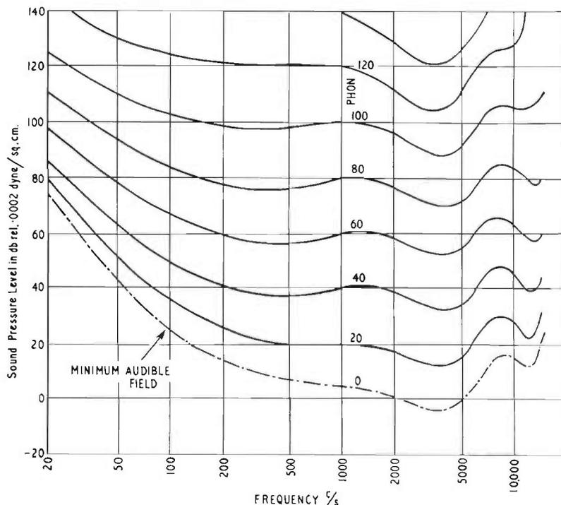
FIG. 3.1(b). Equal loudness contours (Robinson and Dadson, NPL).
