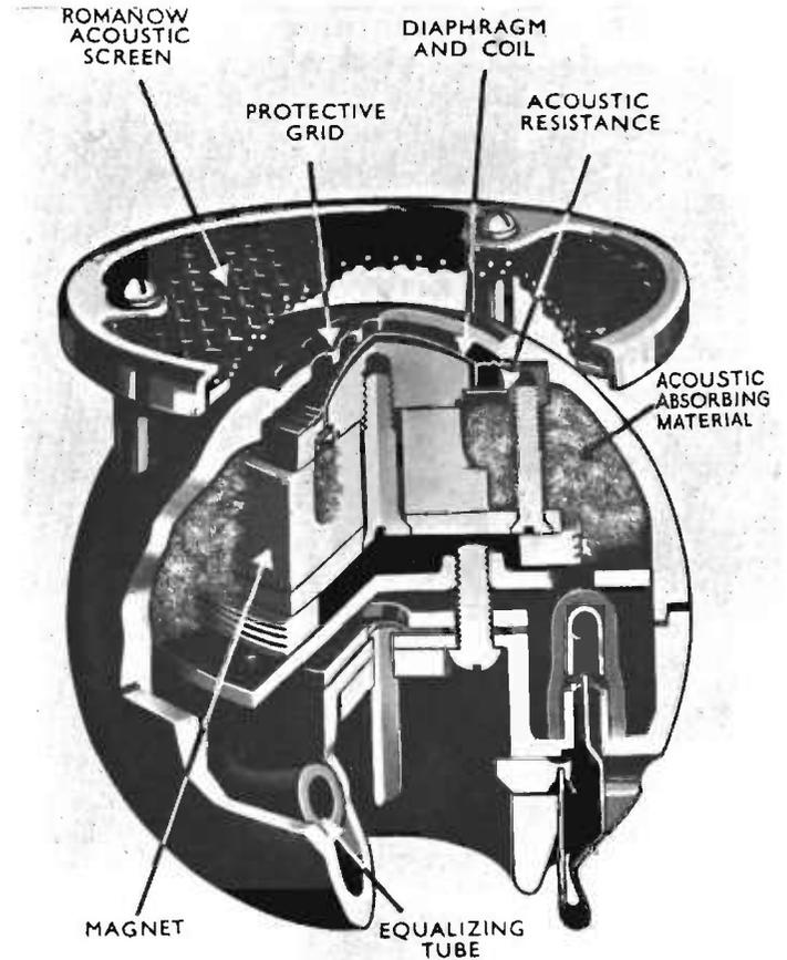
FIG. 5.6. Cutaway view of Type 4021 moving coil microphone.
