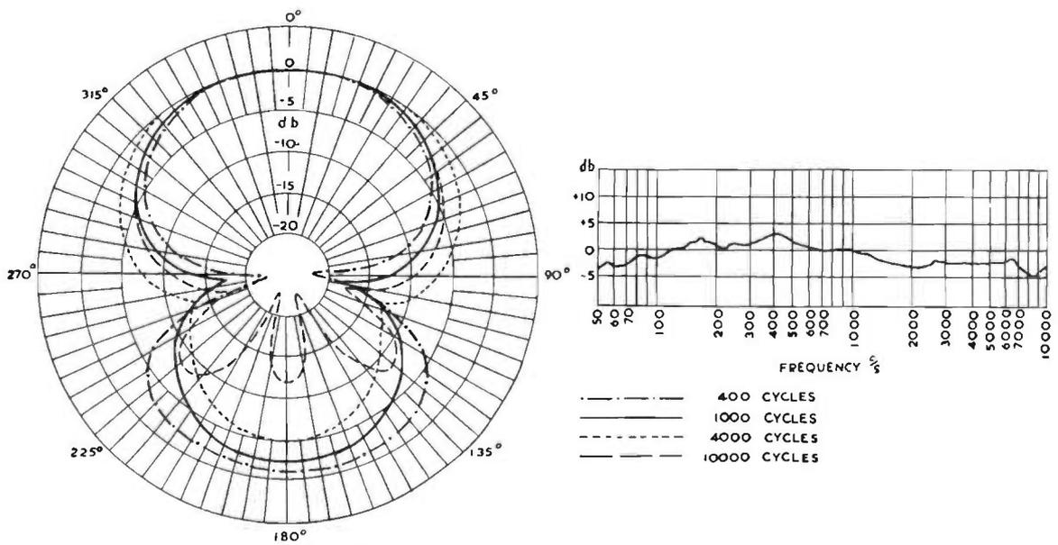
FIG. 5.19(c). Performance characteristics of R.C.A. Varacoustic Microphone Type LMI-6203-C. Velocity position.
