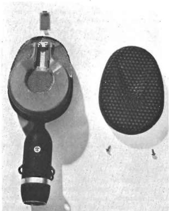
FIG. 5.15(a). View of S.T. & C. Type 4038 ribbon microphone with cover removed.
