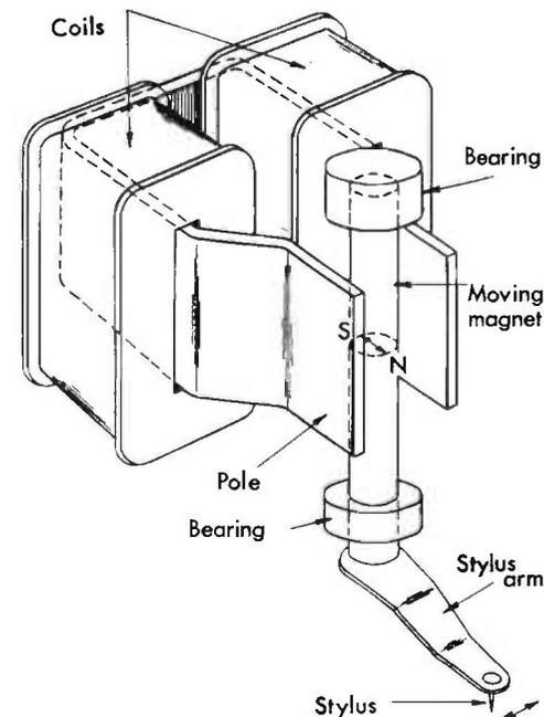
FIG. 7.15(a). Construction of Philips moving magnet pick-up.
