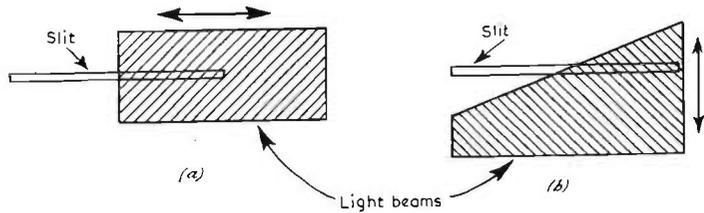
FIG. 18.6. (a) and (b). Two methods of making variable-width sound records.
