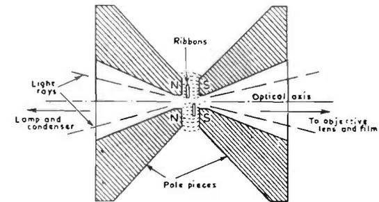
FIG. 18.4. Light-valve ribbon and pole piece arrangement section at right angles to ribbon.
