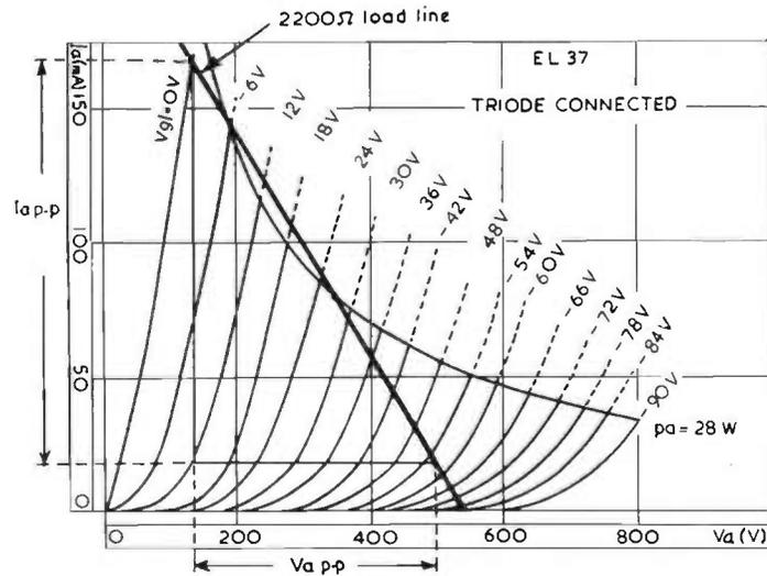
FIG. 10.12. Graphical determination of power per a single valve.
