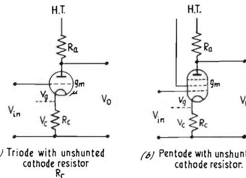
FIG. 9.36. Equivalent circuits with unshunted cathode resistor.
