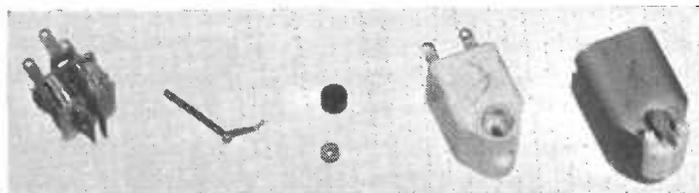
FIG. 7.15(b). Components of the Philips moving magnet pick-up.
