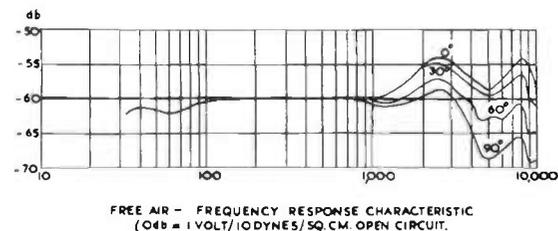
FIG. 5.4. Frequency characteristics of Standard Telephones Type 4017.
