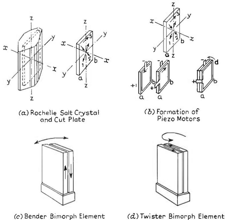
FIG. 7.17(a)-(d). Construction of bimorph assembly.
