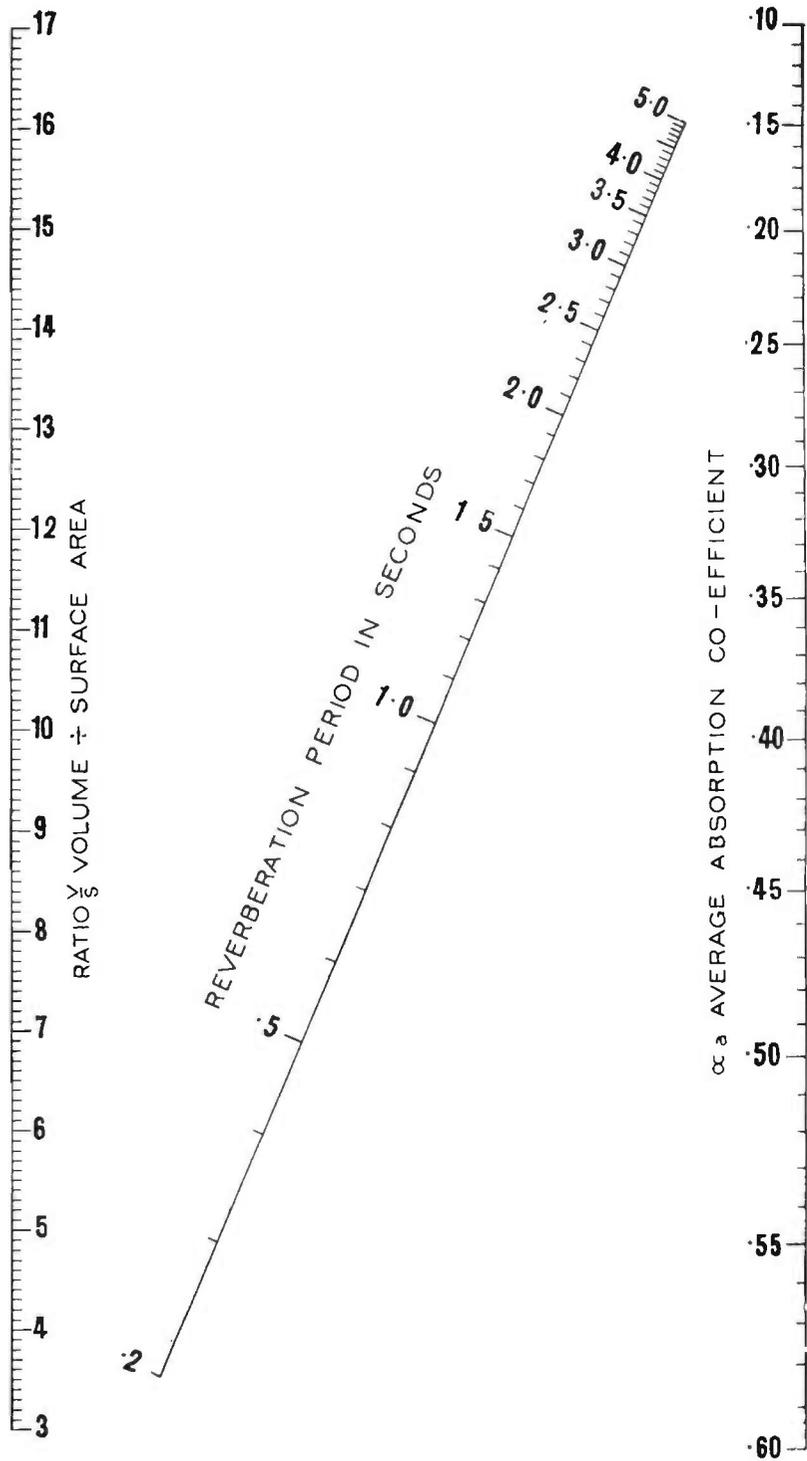
FIG 17.5. Nomogram for determining reverberation period.
