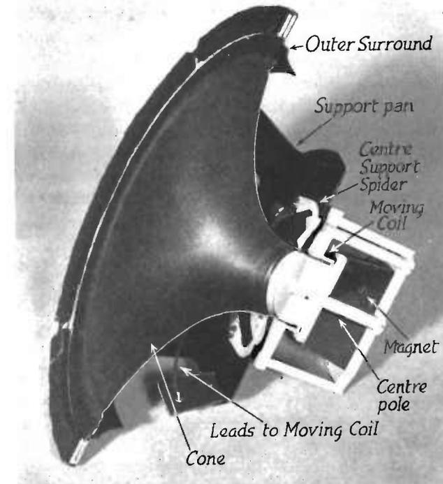
FIG. 16.1. Section through typical moving coil loudspeaker.
