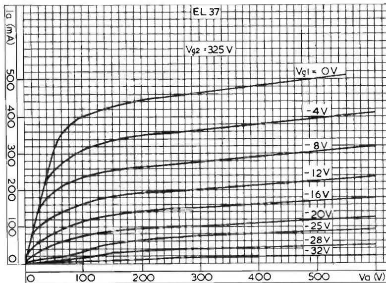
FIG. 10.5.  $I_a/E_a$  characteristics of EL37 as pentode.
