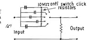
Circuit giving continuous adjustment of bass cut using .001 variable capacitor and feedback to increase effective value of  $R_g$ .
