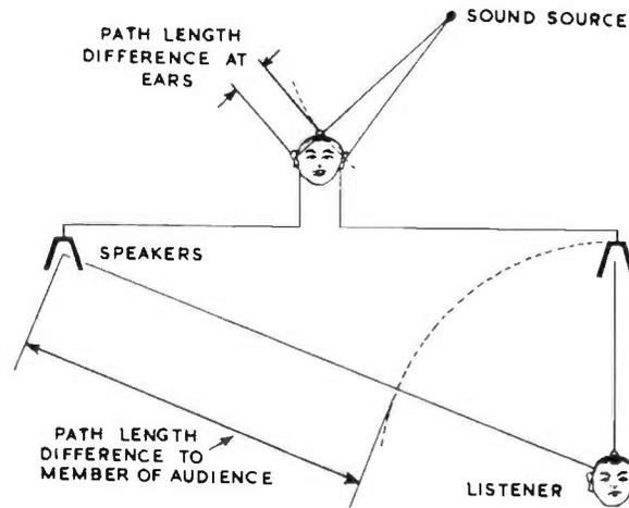
FIG. 19.6. Path length discrepancy using closely spaced microphones and widely spaced speakers.
