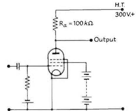
FIG. 9.5(b). Pentode circuit diagram.
