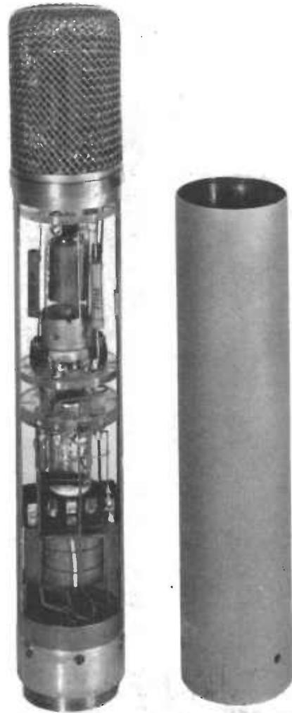
FIG. 5.25. Interior of AKG C12 Microphone, with its associated amplifier.
