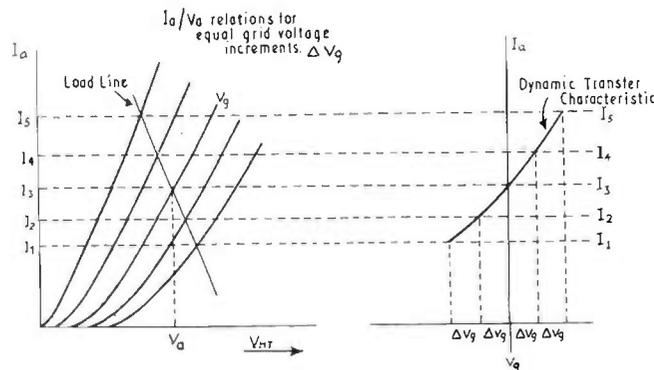
FIG. 9.9. Dynamic transfer characteristic obtained from load line.
