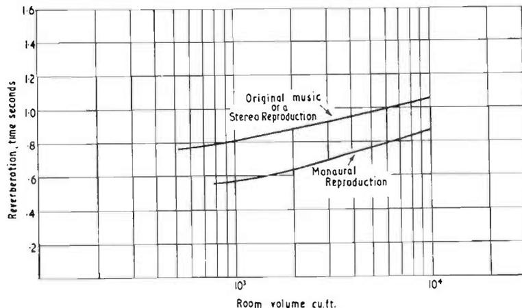
FIG. 17.21. Suggested optimum reverberation times for small rooms.
