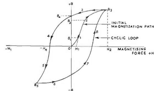
INITIAL MAGNETIZATION PATH AND CYCLIC HYSTERESIS LOOP FOR TYPICAL MAGNETIC MATERIAL.
