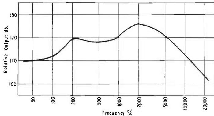
FIG. 1.4. Energy spectrum (octave bands) of metal to metal impact noise.
