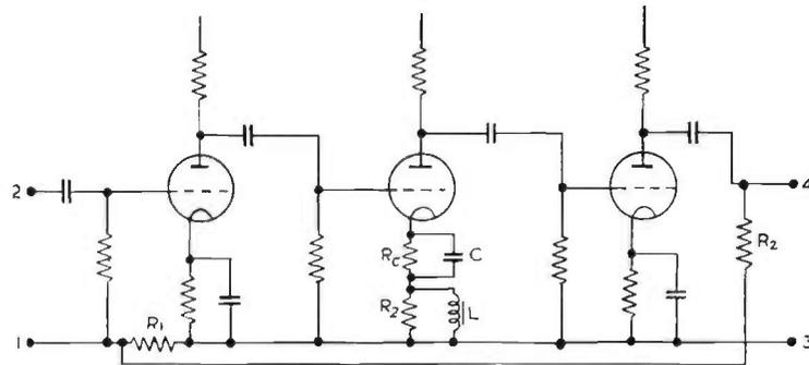
FIG. 12.6. Three-stage feedback circuit.
