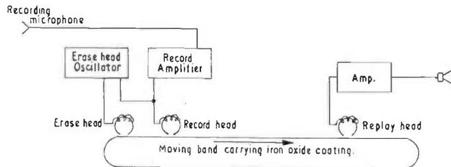
FIG. 8.1. Essential components of a magnetic recording system.
