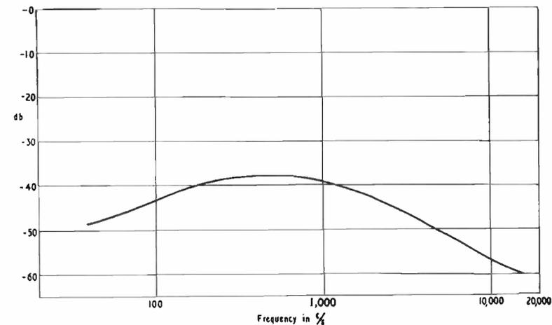
FIG. 18.29. Cross talk data on B.T.H. four track magnetic head.
