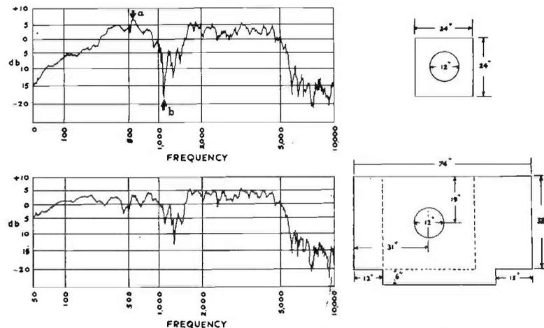
FIG. 16.16. Axial response curves of speaker taken on baffles of different size. Irregularities due to interference are indicated by arrows.
