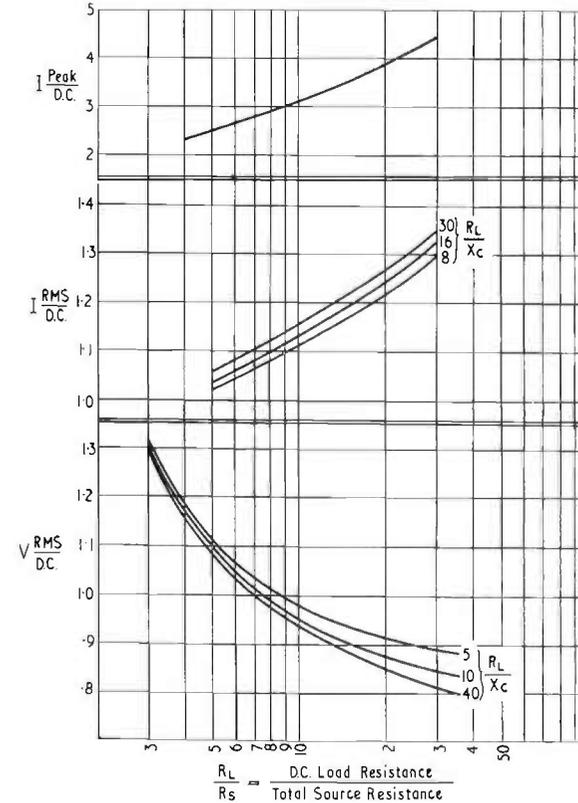
FIG. 14.8. Design relations for full wave rectifier.
