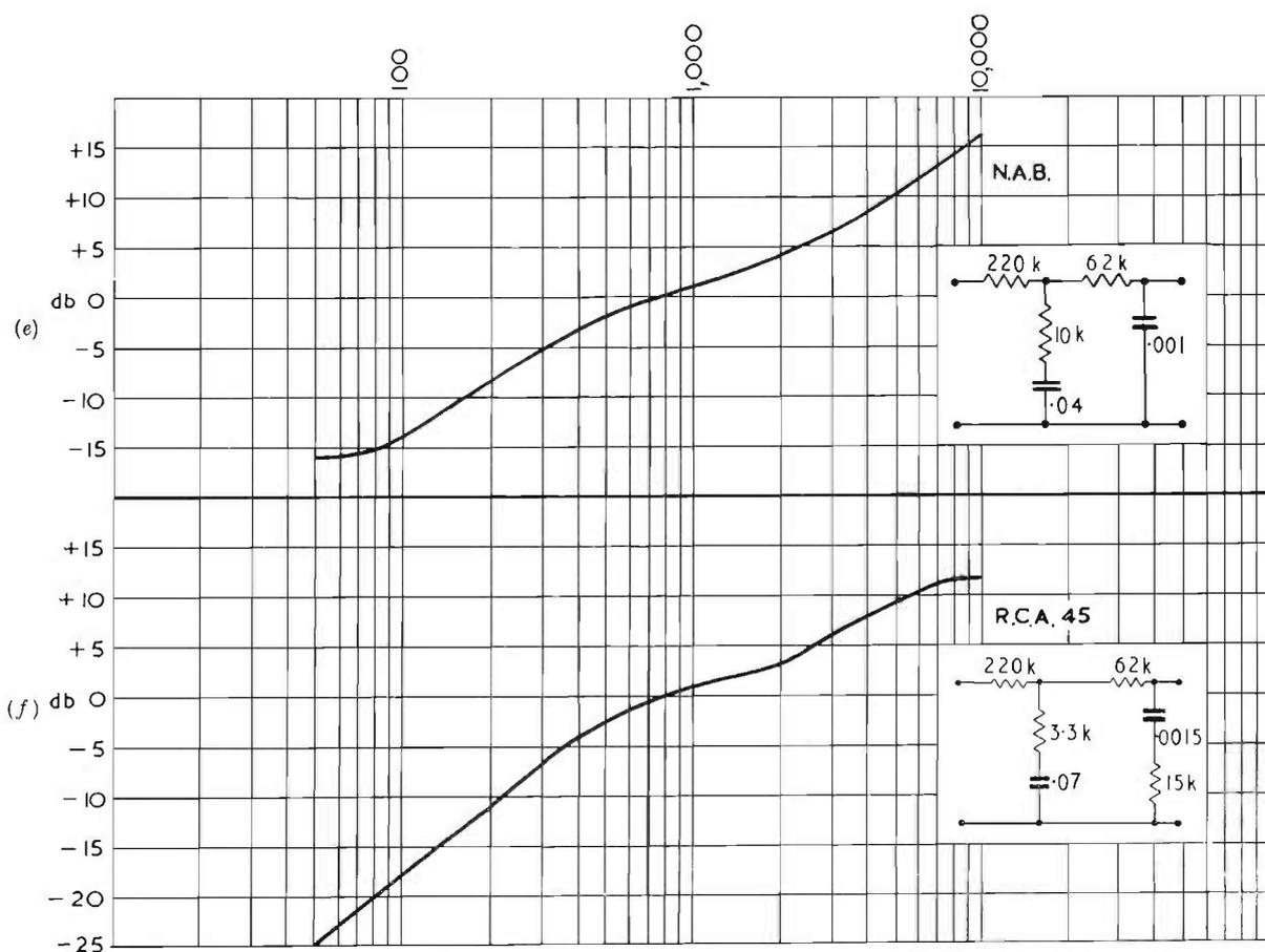
FIG. 7.29(e)-(f). Recording characteristics and correction circuits. (e) N.A.B.; (f) R.C.A. 45.
