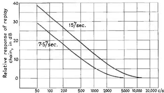
FIG. 8.15. Nominal re-play chain frequency response standardized by C.C.I.R. for tape speeds of 7.5 in./sec. and 15 in./sec.
