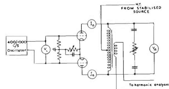
FIG. 10.14. Circuit arrangement used for determining power output of a pair of valves in push-pull.
