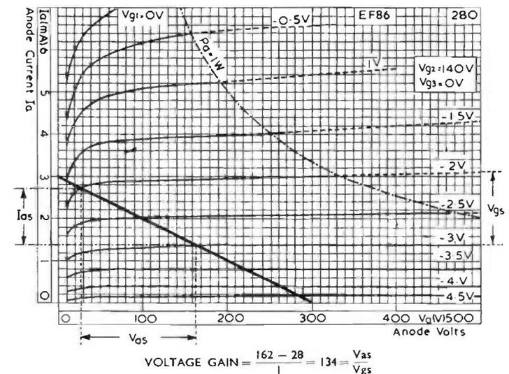
FIG. 9.5(a). Graphical construction for a pentode connected EF 86 as a voltage amplifier in the circuit of Fig. 9.5(b).
