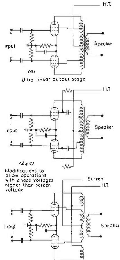
FIG. 10.17. Blumlein ultra-linear output stages.
