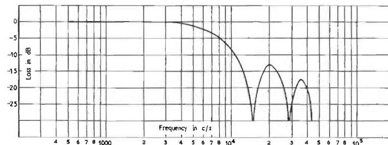
FIG. 8.13. The response is that obtained using heads  $\cdot 09$  in. wide on tape running at  $7\frac{1}{2}$  in./sec. with a head misalignment of 20 minutes. The curve can be used to predict the loss resulting from a greater misalignment by dividing all the frequencies by (misalignment angle in minutes)/20.
