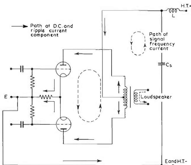
FIG. 10.3. Output valves in push-pull.
