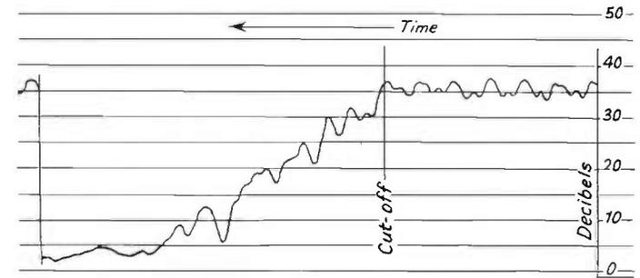
FIG. 17.8. Typical reverberation decay curve.
