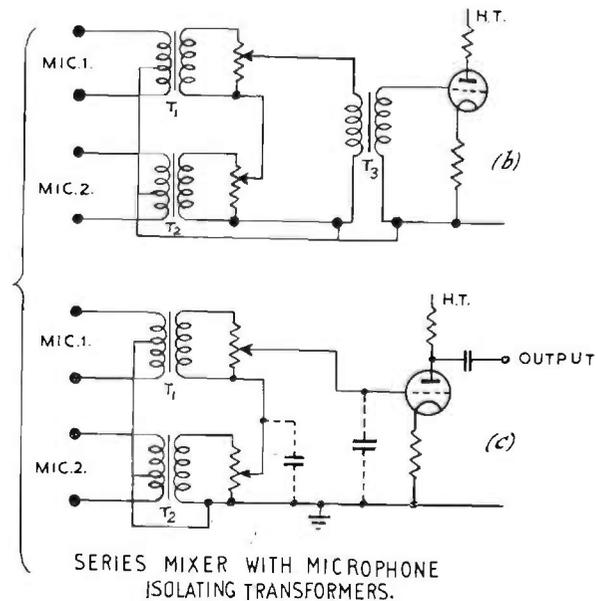
FIG. 6.2(a)-(c). Series mixer circuits.
