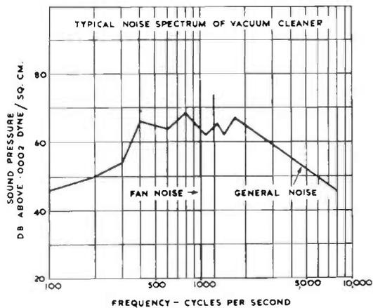
FIG. 1.2. Noise spectrum of vacuum cleaner.
