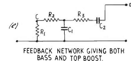
FIG. 13.11 (a-e). Basic feedback tone control circuits.
