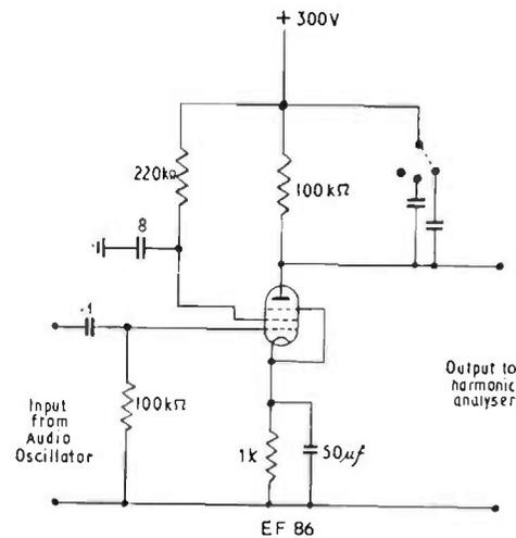
FIG. 9.15(b). Circuit for measurement of distortion due to reactive loading.
