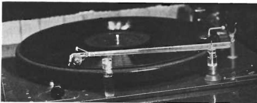
FIG. 7.8. The Watts 'Dust Bug'. A fine nylon brush tracks across the record and removes the dust from the groove immediately in front of the stylus.
