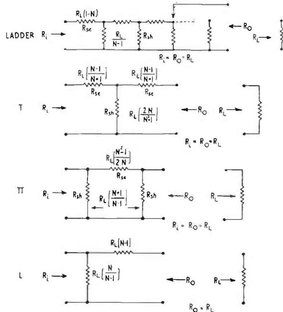
FIG. 6.6. Design data for constant impedance attenuators.
