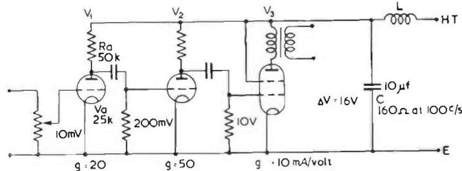
FIG. 9.26(a). Low frequency amplifier.
