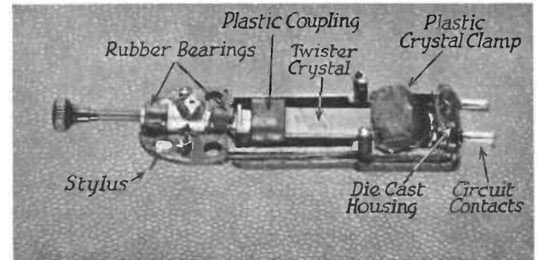
FIG. 7.18. Interior of typical twister bimorph piezo-electric pick-up.
