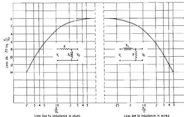
FIG. 11.2. Basic output transformer characteristic.
