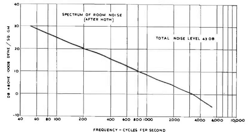
FIG. 1.5. Spectrum of room noise, as recorded by Hoth.
