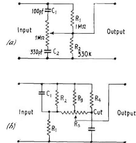
FIG. 13.10. Continuous control of top boost and cut.
