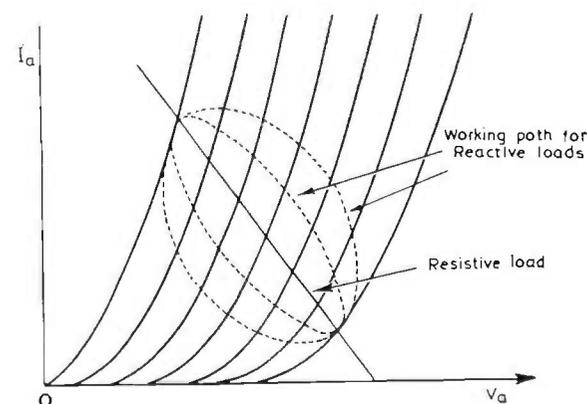
FIG. 9.14. Load line for valve with reactive anode load.
