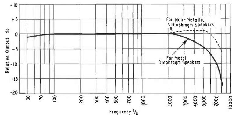
FIG. 18.22. Reproducer frequency characteristic suggested by motion picture research council.
