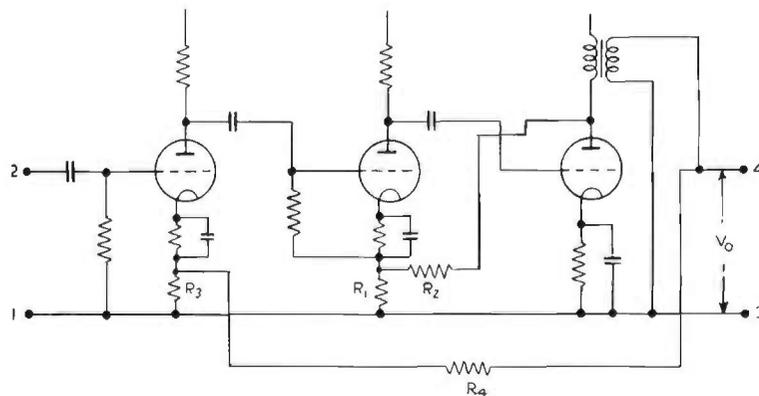
FIG. 12.7. Three-stage multiple loop feedback.
