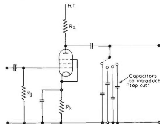
FIG. 9.13. Typical tone control circuit in which the anode load is reactive.
