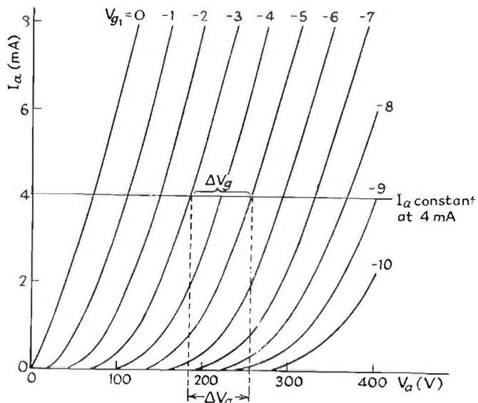
FIG. 9.16(a). Derivation of amplification factor.
