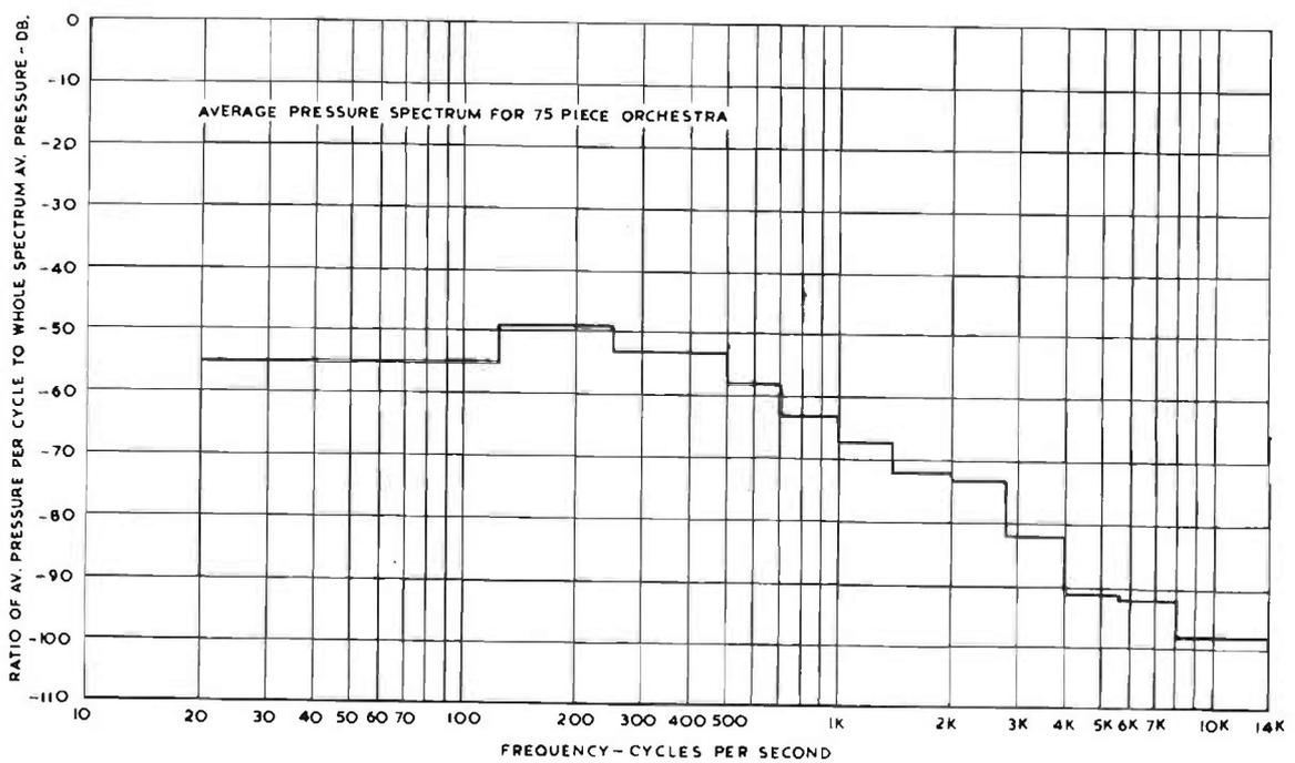
Fig. 1.7(b). Data from tests on 75-piece orchestra ; average pressure spectrum.
