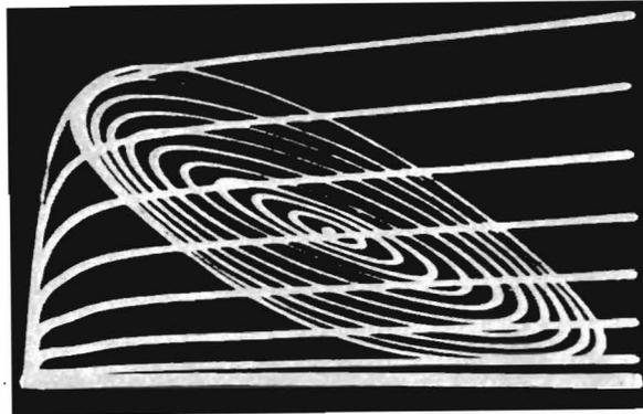
FIG. 10.9. Cathode ray display of  $I_a/E_a$  characteristic with reactive load.
