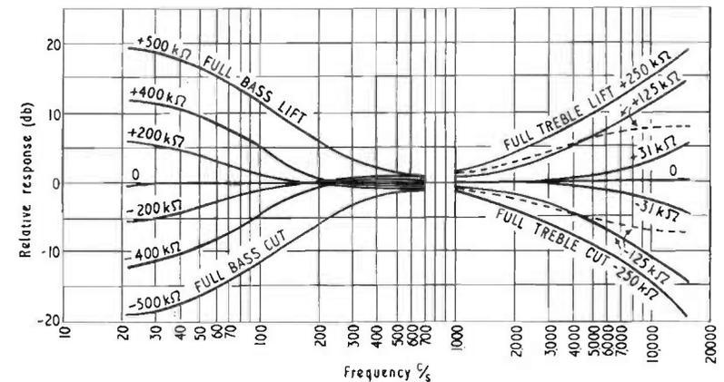
FIG. 13.16. Performance characteristics of Baxandall tone control circuit.
