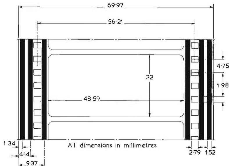
FIG. 18.32. 70 mm. film with six magnetic sound-tracks. Todd A-O film.
