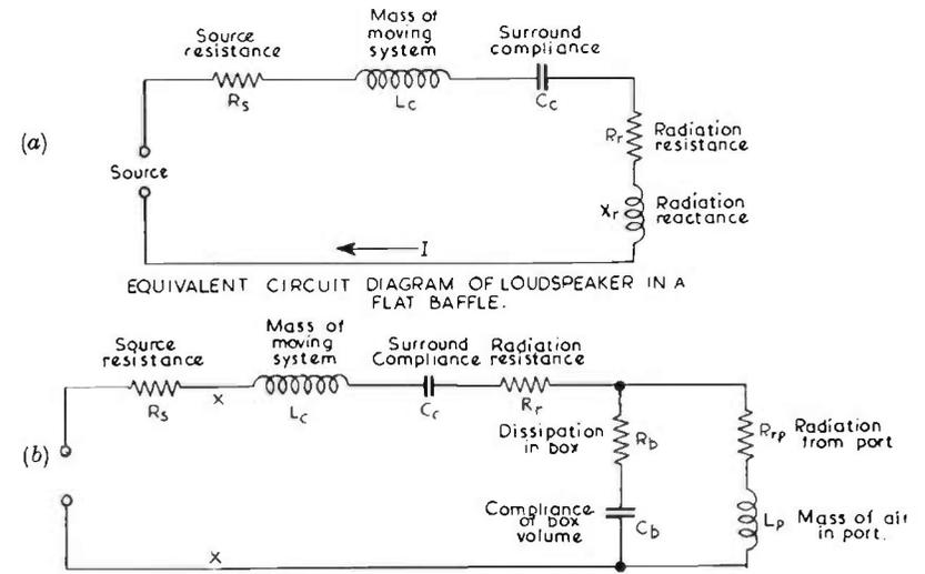
FIG. 16.26. Equivalent circuits for loudspeaker.
