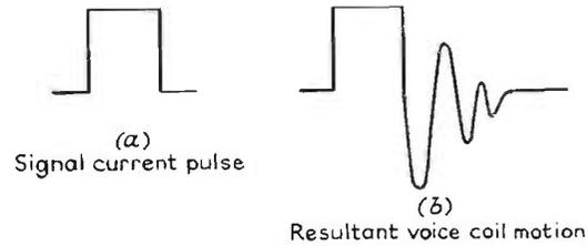
FIG. 16.11(a)-(b). Cone motion.
