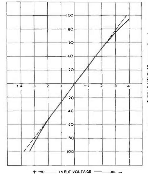
FIG 9.7. Dynamic transfer characteristic obtained from Fig. 9.6(b).
