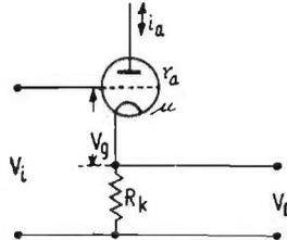
FIG. 9.38. Voltage gain of a cathode follower.
