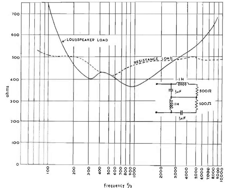
FIG. 15.6. Measured input resistance of a constant resistance dividing network.
