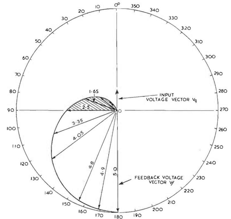
FIG. 12.3. Vector diagram of a two-stage feedback amplifier.
