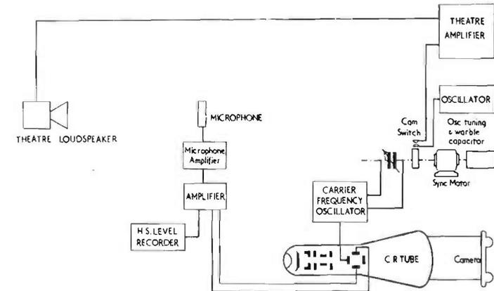
FIG. 17.11. Set up for acoustic survey in auditorium.
