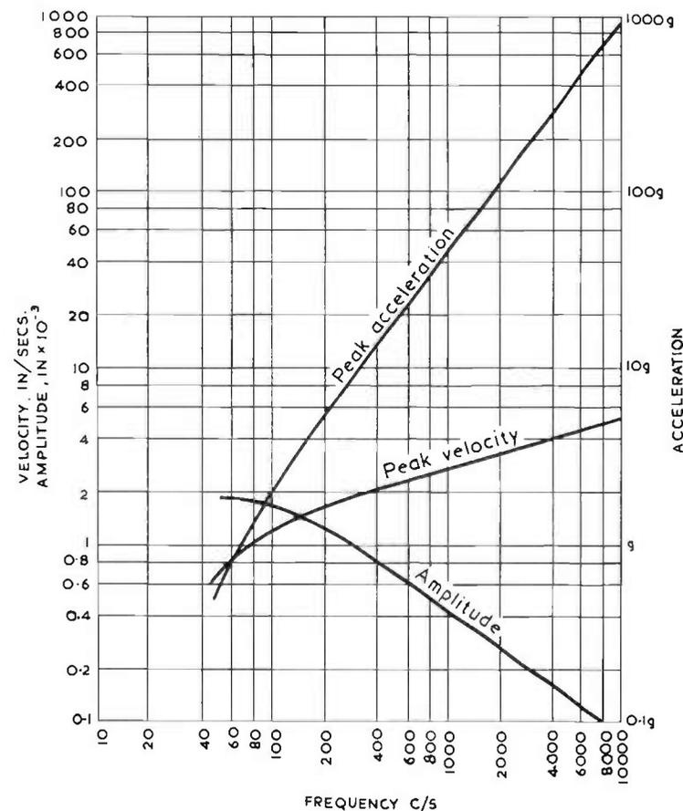
Fig. 7.2. Amplitudes, peak velocities and peak acceleration for maximum level with B.B.C. recording characteristic.
