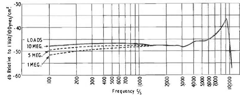
FIG. 5.14. Effect of shunt resistance on Piezo microphone response.
