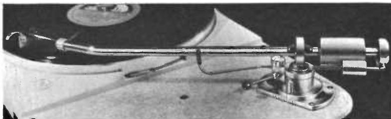
FIG. 7.13. S.M.E. pick-up arm, compensated to give vertical and lateral balance.
