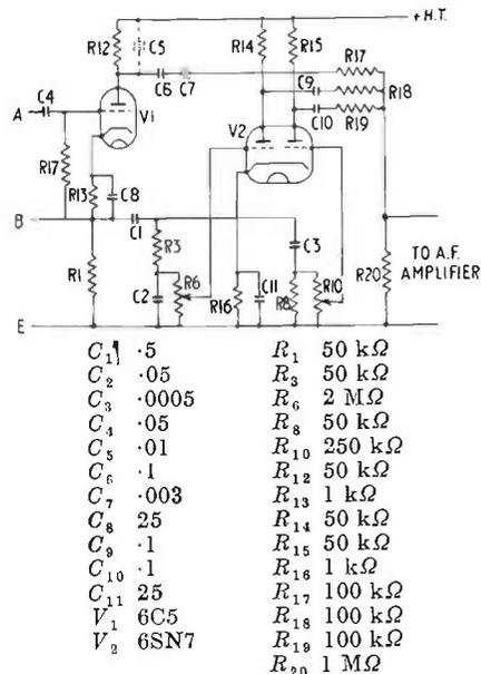
FIG. 13.14. Patchett's tone control circuit.
