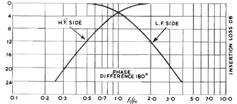
$$L_o = \frac{R_o}{2\pi f_c}, \quad L_1 = \frac{L_o}{\sqrt{2}}, \quad L_2 = \sqrt{2} L_o, \quad C_o = \frac{1}{2\pi f_o R_o}, \quad C_1 = \sqrt{2} C_o, \quad C_2 = \frac{C_o}{\sqrt{2}}$$
