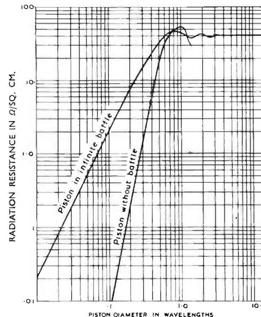
FIG. 16.17. Radiation resistance of piston with and without baffle.
