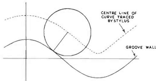
FIG. 7.4. Origin of tracing distortion. When the diameter of the stylus tip is comparable with the groove wavelength, the stylus tip does not follow a sinusoidal path even though the groove modulation is sinusoidal.
