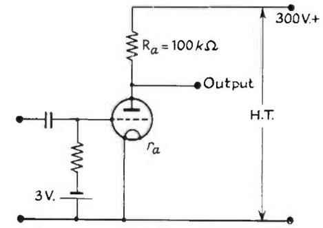
FIG. 9.4(b). Triode circuit diagram.
