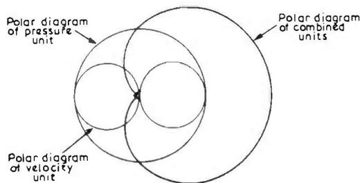
FIG. 5.16. Cardioid polar diagram of pressure and velocity responsive units.
