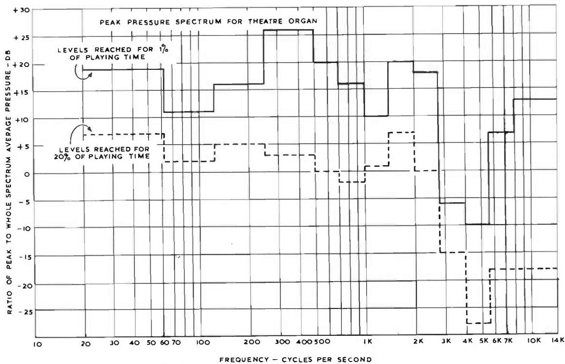
FIG. 1.8(a). Data from tests on two cinema organs ; peak pressure spectrum.
