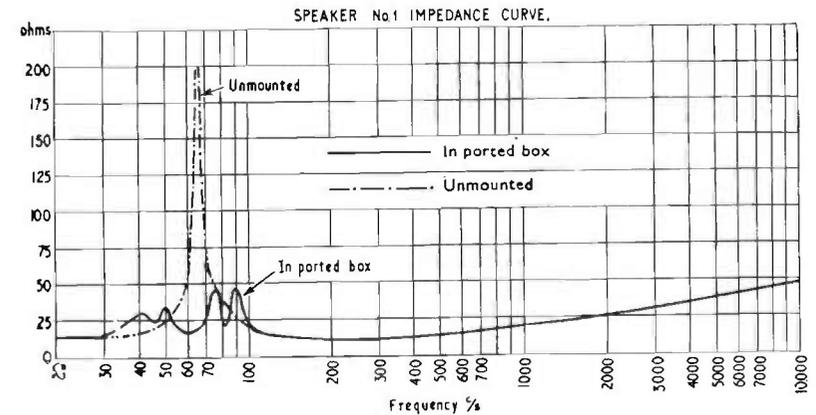
FIG. 16.27. Impedance of 12-in. speaker in free air and in ported cabinet.
