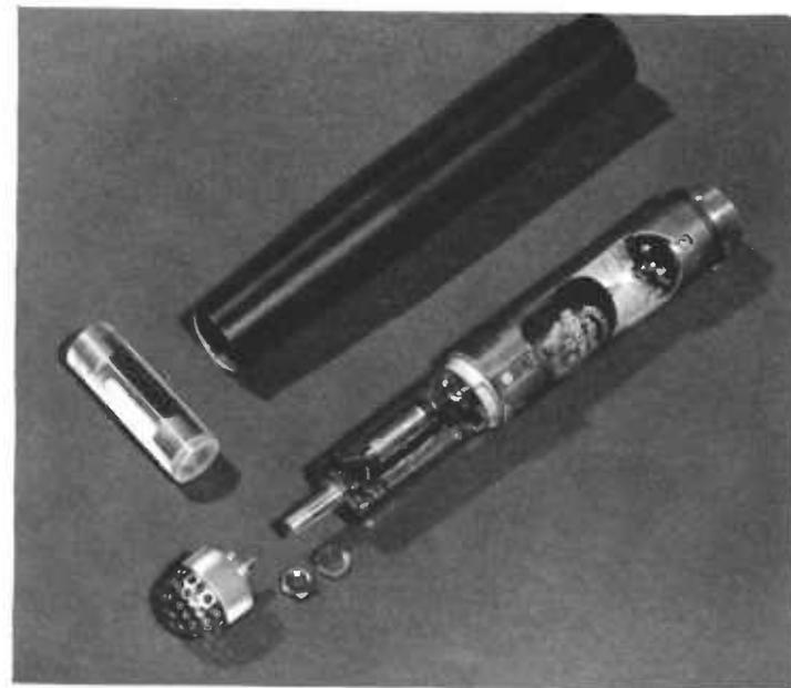
FIG. 5.10. Microphone capsule and head amplifier of Philips capacitor microphone.
