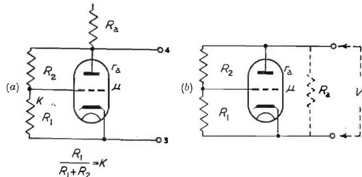
FIG. 12.9 (a) and (b). Equivalent circuits for valve with feedback.
