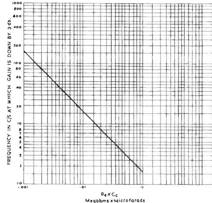
FIG. 9.22. Low frequency attenuation as a function of  $R_e \times C_c$ .
