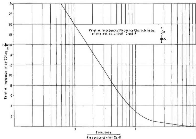
FIG. 13.19. Impedance/frequency characteristic of series circuits.
