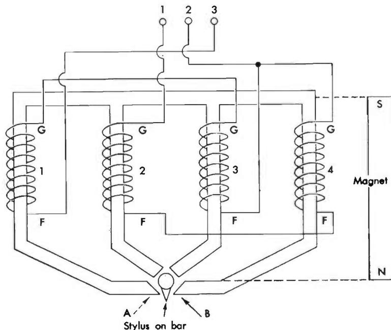
FIG. 7.24. Diagram showing the principle of a variable reluctance stereo pick-up. (Tannoy Ltd.)
