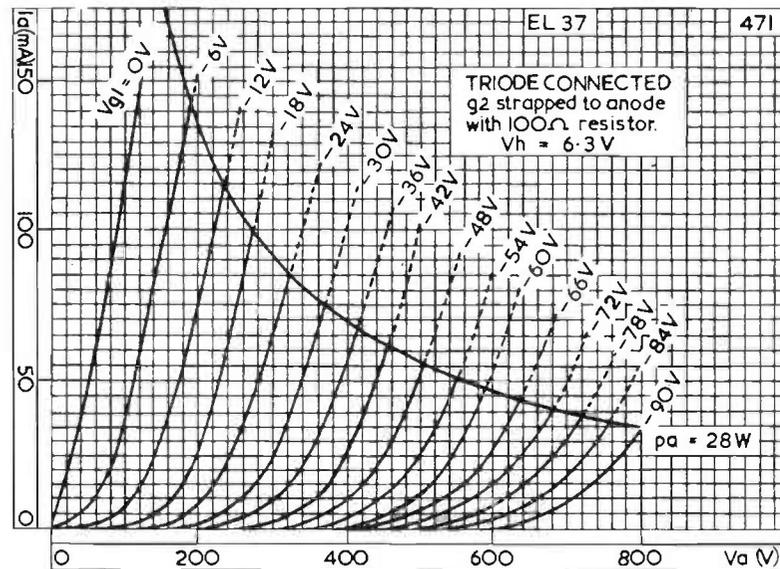
FIG. 10.4.  $I_a/E_a$  characteristics of EL37 as triode.
