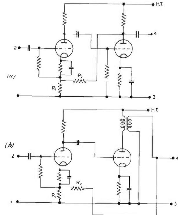
FIG. 12.5. Two-stage feedback circuits.
