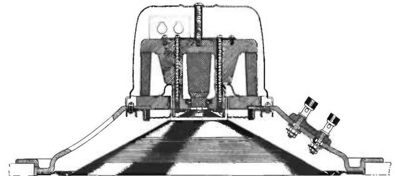
FIG. 16.33. R.C.A. LC-1A coaxial speaker in section.
