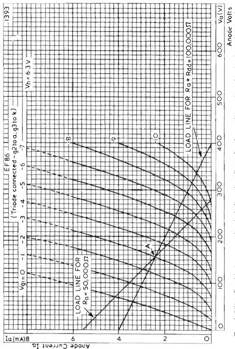
FIG. 9.6(b). Graphical construction including the effect of a decoupling resistor for circuit conditions of Fig. 9.6(a).
