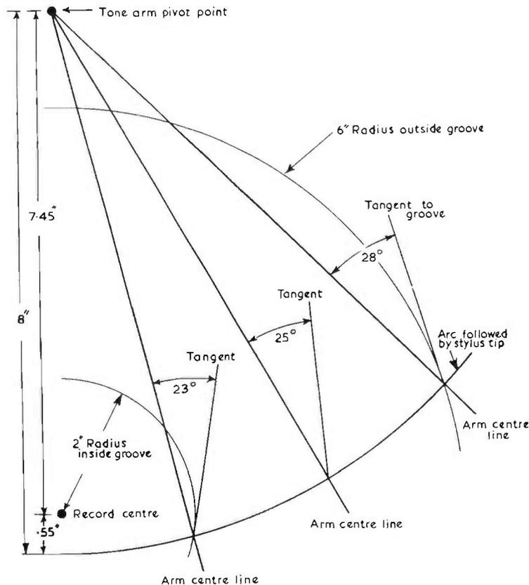
FIG. 7.11. Tone arm tracking diagram showing advantage gained by allowing stylus point to overhang record centre.
