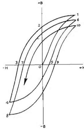
STARTING FROM THE COMPLETELY DEMAGNETISED CONDITION AT O AN ELEMENT REACHES THE FINAL CYCLIC STATE ALONG THE PATH 1-10 THROUGH A SERIES OF INTERMEDIATE HYSTERESIS LOOPS.
