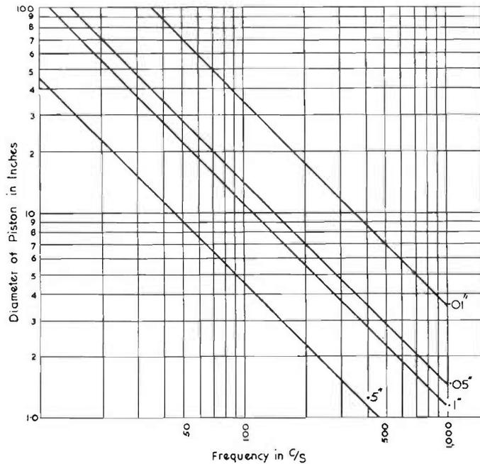
FIG. 16.4. Peak amplitude of vibration required to radiate one acoustic watt from one side of piston.
