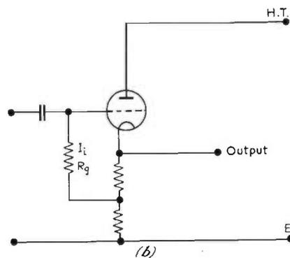
CATHODE LOAD SPLIT TO PROVIDE OPTIMUM BIAS.
