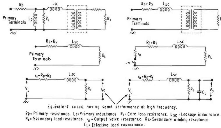
FIG. 11.5. Equivalent circuits for output transformer.
