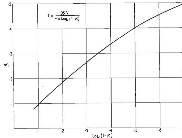
FIG. 17.4. Relation between  $\alpha$  and  $\log_e (1 - \alpha)$  used in the Eyring reverberation equation.
