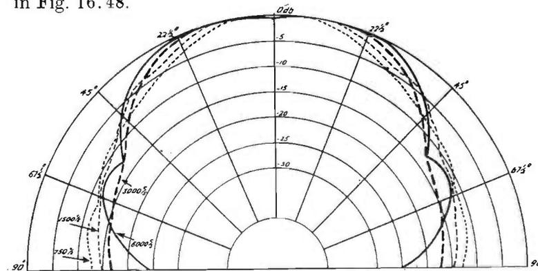
Horn type:— 9 cell. Axis:— Horizontal. Speaker Input:— 2 Watts. Distance: Microphone to Speaker: 12 ft.
