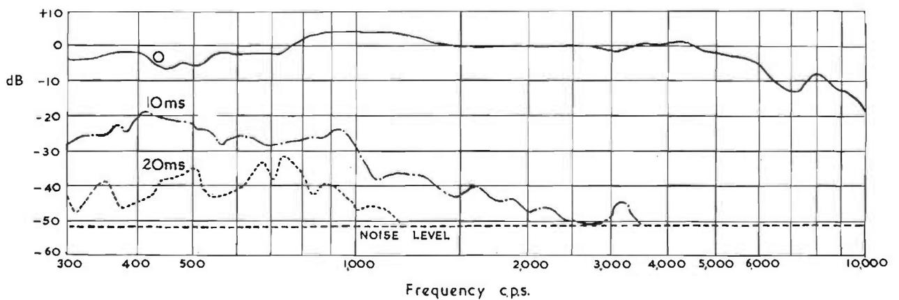
FIG. 16.12. Transient response curves. (c) Speaker No. 3. Less colouration than usual on speech but top response becomes a little irritating after a long period of listening.
