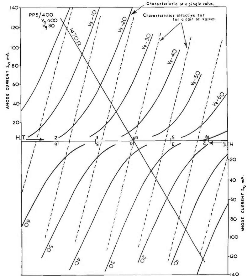
FIG. 10.13. Graphical construction giving composite characteristics of valves in push-pull.
