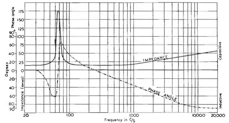
FIG. 16.5. Impedance and phase angle of typical 12 in. direct radiator speaker without baffle.
