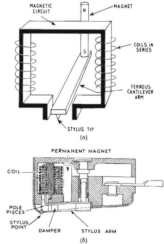
FIG. 7.16. Variable reluctance pick-ups. (a) Principle of operation. (b) Sectional drawing of complete pick-up.
