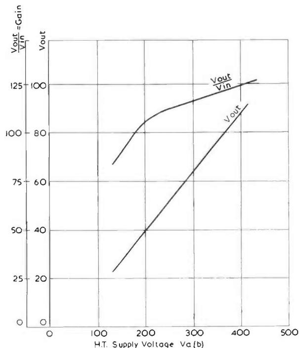
FIG. 9.19. Gain and output voltage change with H.T. voltage for a typical pentode.
