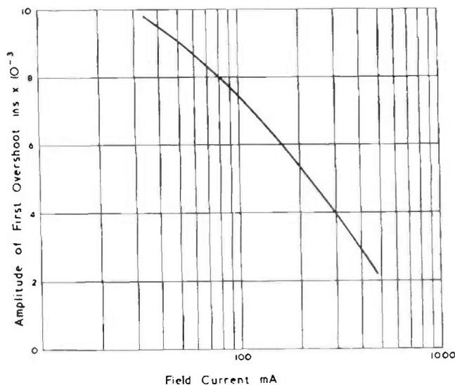
FIG. 16.14. Effect of field current on amplitude of first overshoot of voice coil oscillation.
