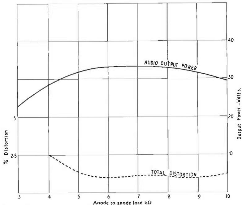
FIG. 10.18. Performance of a pair of EL34 valves in Blumlein ultra-linear circuit.
