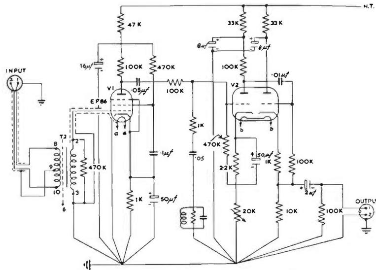
FIG. 18.30. Equalizing pre-amplifier for magnetic sound film reproducer.
