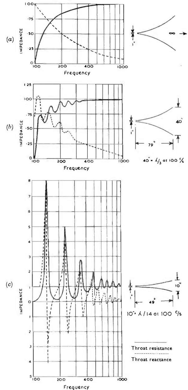
FIG. 16.41(a)-(c). Effect of mouth diameter on throat impedance characteristic. (Ref. 11.)
