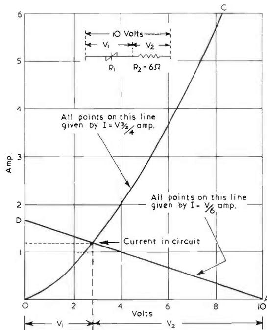
FIG. 9.3. Graphical construction for determination of voltage distribution across a non-linear and linear resistor in series.
