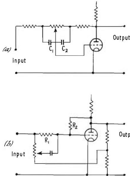
FIG. 13.17(a-b). Basic elements of Baxandall circuit.
