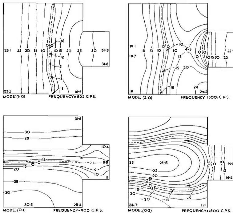
FIG. 17.20. Experimentally determined pressure distribution contours in a model room having a similar shape to the actual room of FIG. 17.19.
