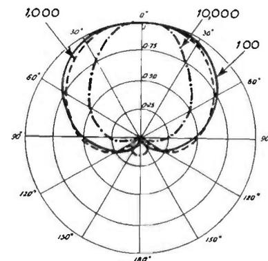
FIG. 5.20. Dynamic Cardioid polar diagram : AKG D20 Microphone.
