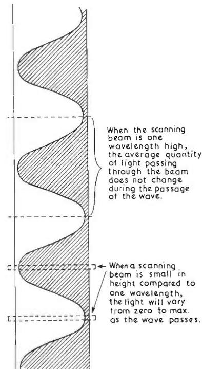
FIG. 18.11. Effect of scanning beam height on reproduction of wave.
