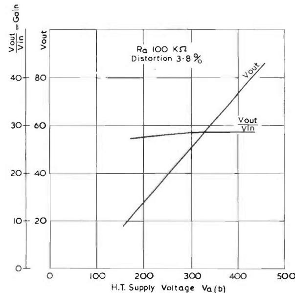
FIG. 9.18. Gain and output voltage change with H.T. voltage for a typical triode.
