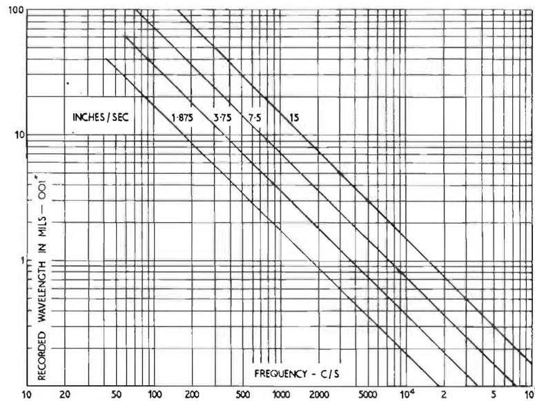
FIG. 8.11. Recorded wavelengths for standard tape speeds.
