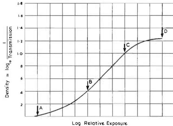
FIG. 18.9 (a). Typical *H* and *D* curve.
