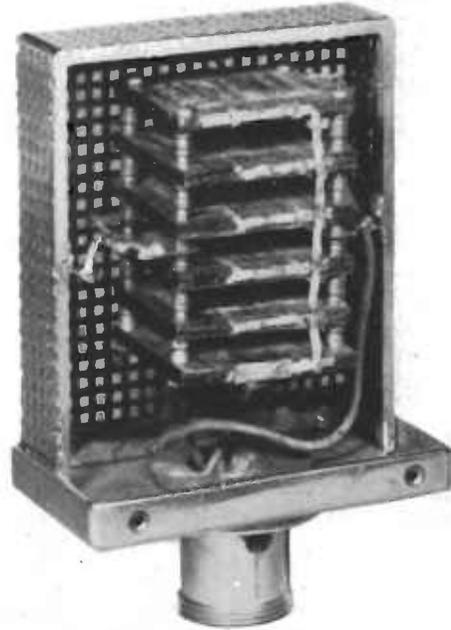
FIG. 5.13. Sound cell assembly.
