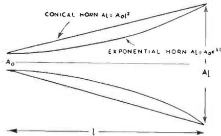
FIG. 16.42. Sections of exponential and conical horns.
