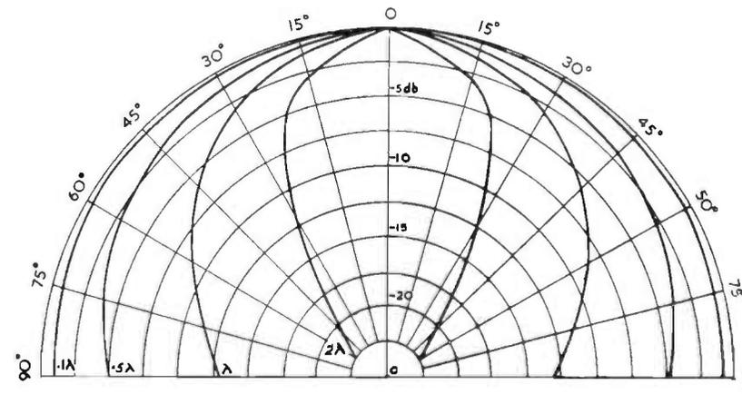
FIG. 16.6. Polar diagram of disk radiator having diameter equal to  $.1\lambda$ ,  $.5\lambda$ ,  $\lambda$  and  $2\lambda$ .
