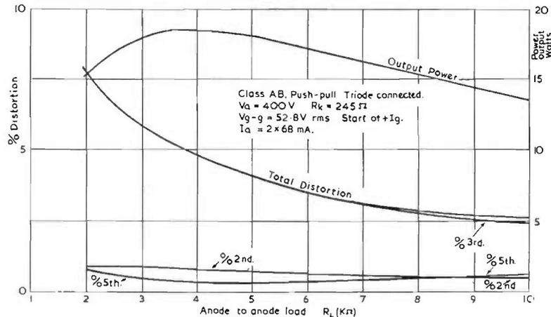
FIG. 10.6. Performance characteristic of EL37 as triode.
