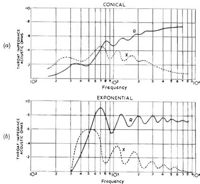
FIG. 16.43. Throat impedance of conical and exponential horns of the same throat and mouth areas. (Ref. 11.)
