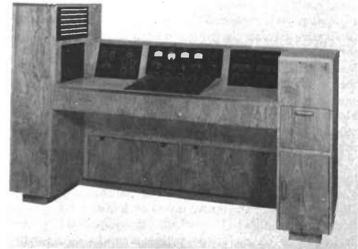
FIG. 6.1. Western Electric mixer console used for sound film recording.
