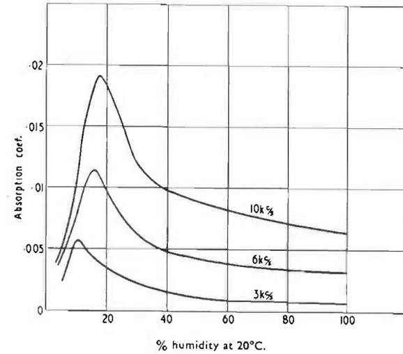
FIG. 17.6. Absorption coefficients for air containing water vapour.
