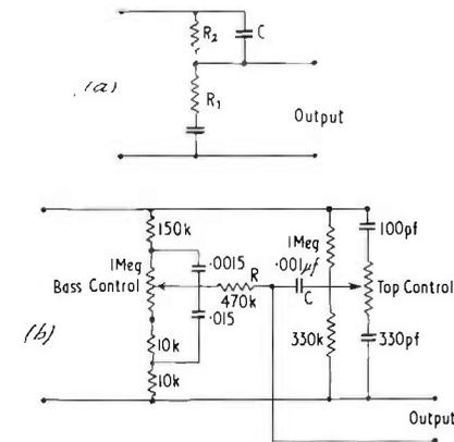
FIG. 13.13(a-b). Combined bass and top control circuits.
