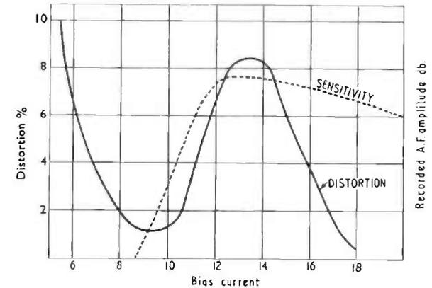
FIG. 8.6. Typical variation of sensitivity and total distortion with bias amplitude.
