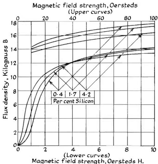
FIG. 11.3.  $B/H$  curve of silicon iron.
