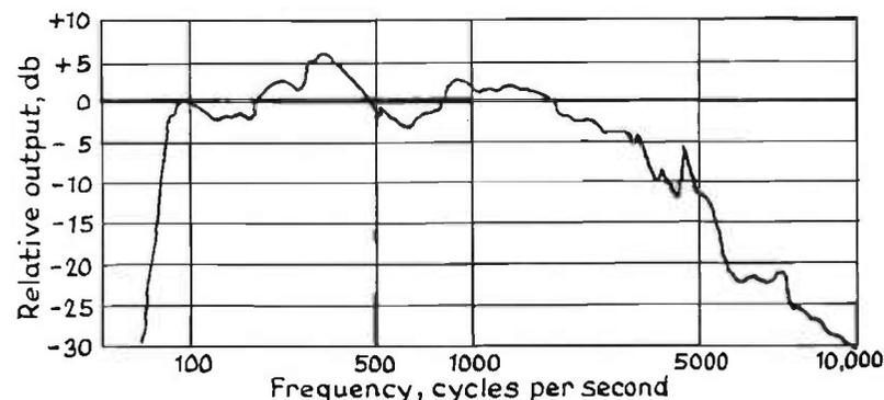
FIG. 4.3. Overall frequency response measured in a leading London cinema.
