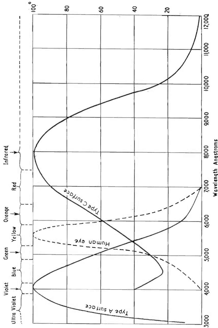
FIG. 18.13. Spectral sensitivity of sound film photo-cells and human eye.
