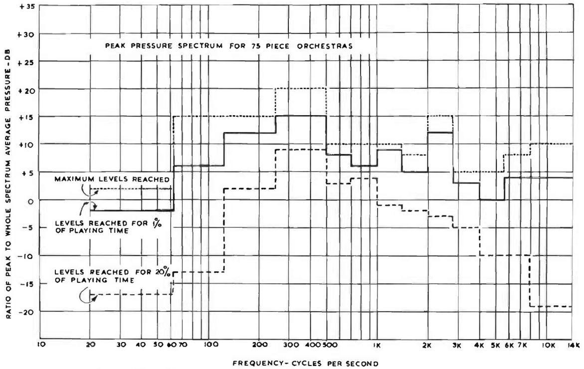
Fig. 1.7(a). Data from tests on 75-piece orchestra ; peak pressure spectrum.
