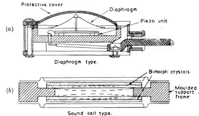
FIG. 5.12. Piezo microphones. (a) Diaphragm type; (b) Sound cell type.
