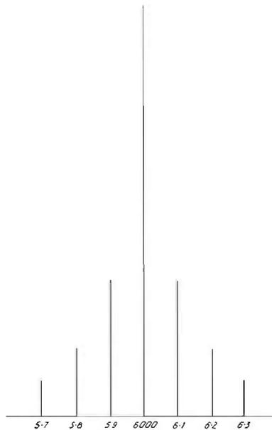
FIG. 16.10. Typical H.F. spectrum resulting from the application of a strong 100 c/s and a weaker 6 kc/s signal.
