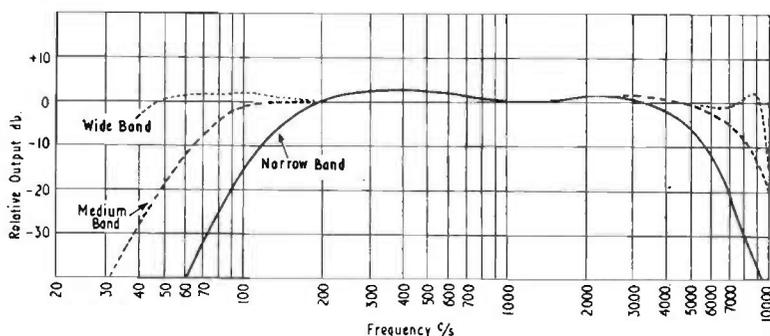
FIG. 4.1. Frequency characteristic of filters used in Chinn and Eisenberg tests.
