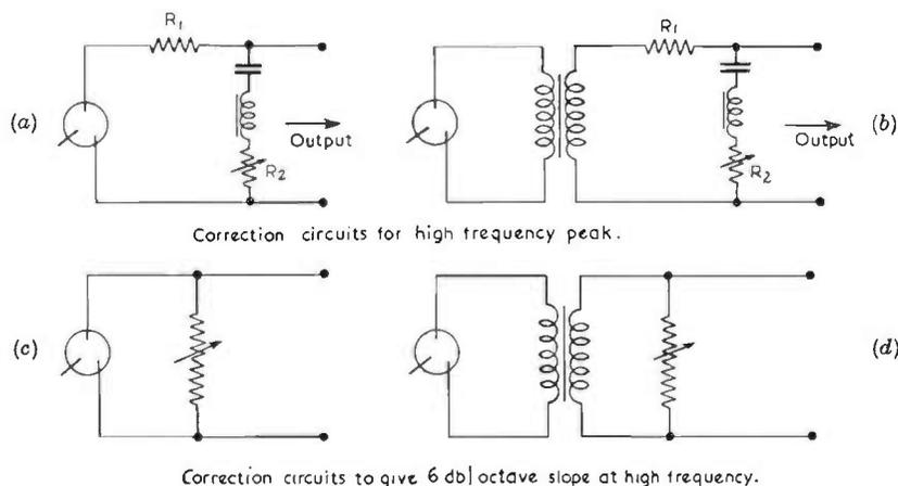
FIG. 7.28(a)-(d). Magnetic pick-up correction circuits.
