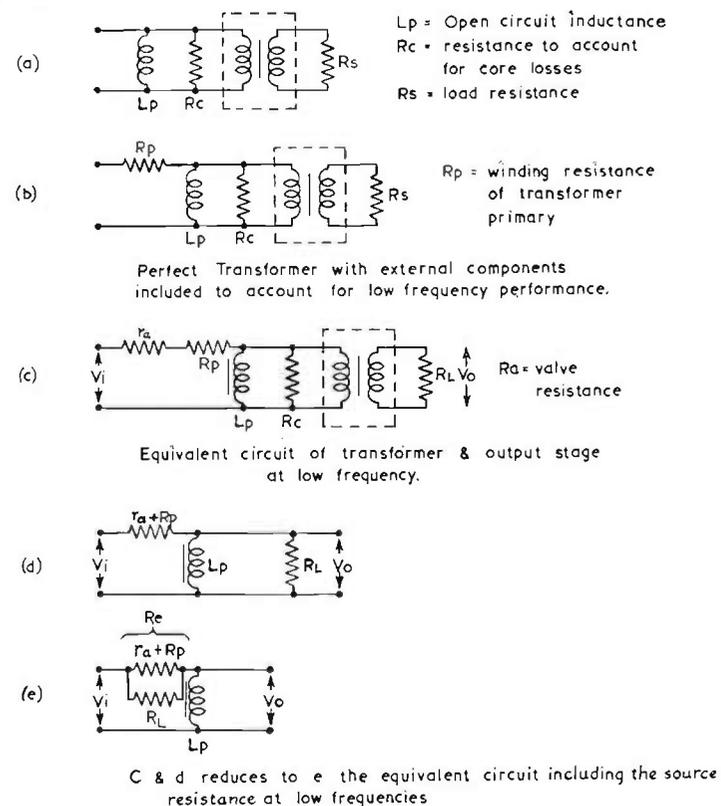
FIG. 11.1. Equivalent circuit of transformer at low frequencies.
