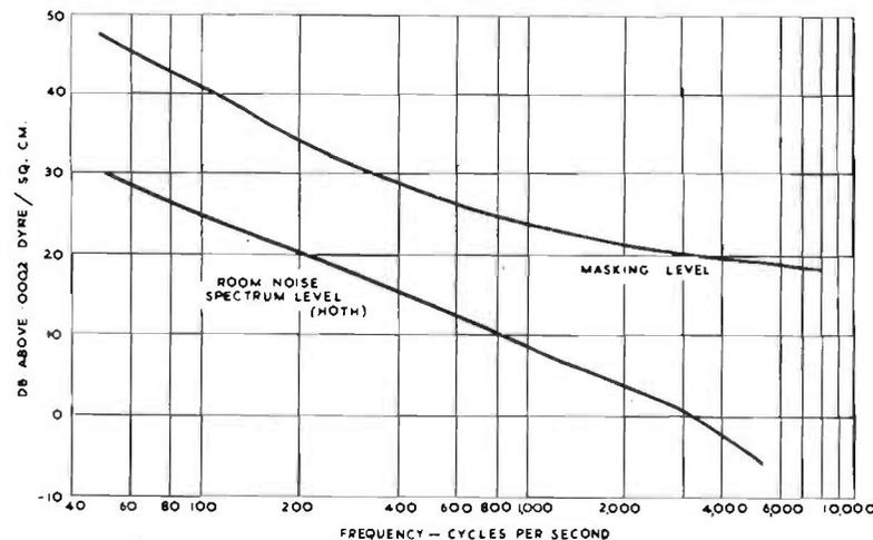
FIG. 3.10. Frequency spectrum of room noise and level to which pure tones must be raised to be audible.
