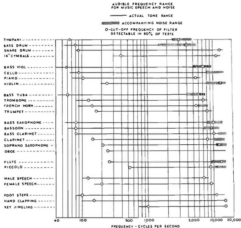
FIG. 3.13. Bar chart showing audible frequency range.
