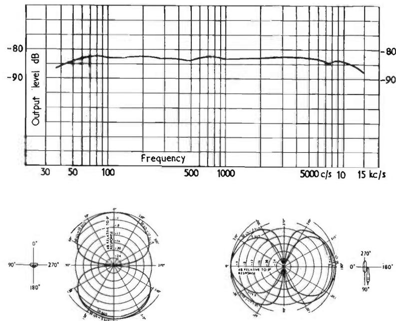
FIG. 5.15(b). Response curves of Type 4038 microphone. (0 dB = 1 volt/dyne/sq. cm.)
