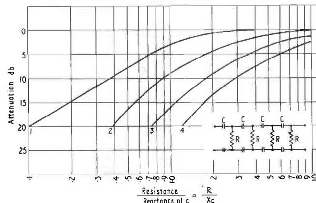
FIG. 13.2. Attenuation of  $n$  series connected meshes.
