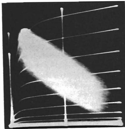
FIG. 10.10. Cathode ray display of  $I_a/E_a$  characteristic on music signal.
