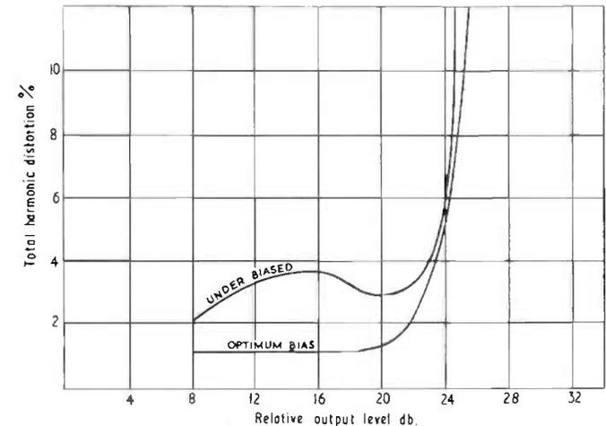
FIG. 8.7. Typical output/distortion relations.
