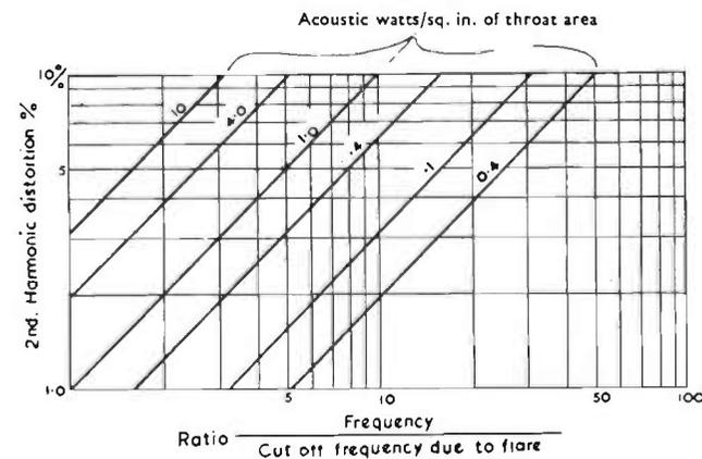
FIG. 16.46. Distortion in horns.
