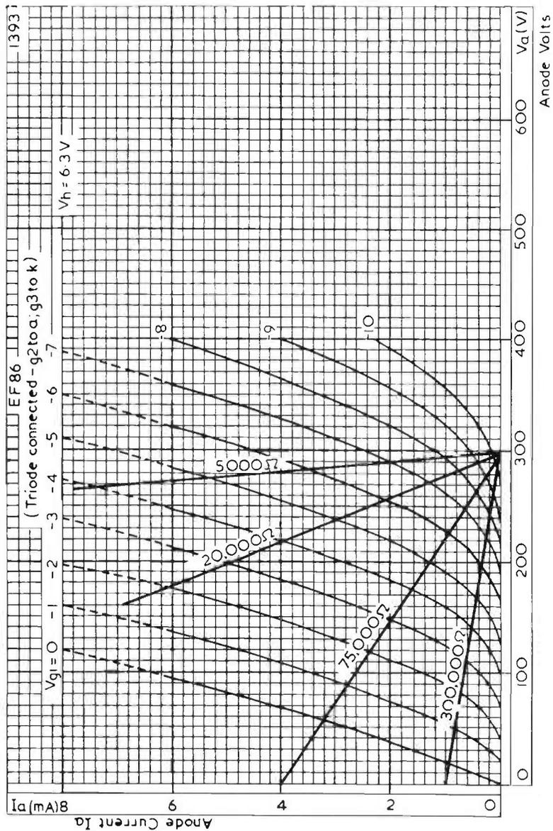
Fig. 9.10. Triode with four load lines.
