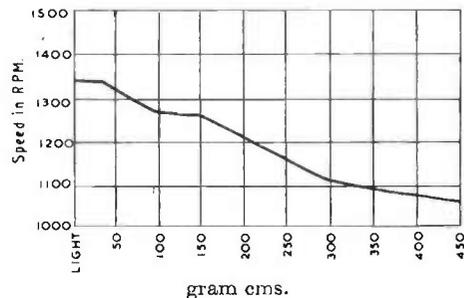
FIG. 7.9. Speed torque curve of a typical induction gramophone motor.
