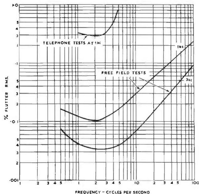
FIG. 3.7(a). Comparison of telephone and free field test results.
