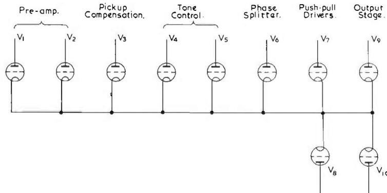
FIG. 9.1. Schematic arrangement of valves in reproducing system.
