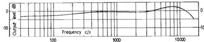
FIG. 7.21. Frequency response of typical piezo-electric pick-up. (Cosmochord Ltd.)
