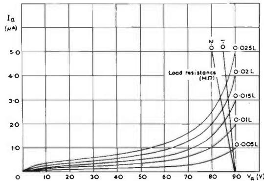
FIG. 18.15. Anode current/incident light for gas-filled cell.
