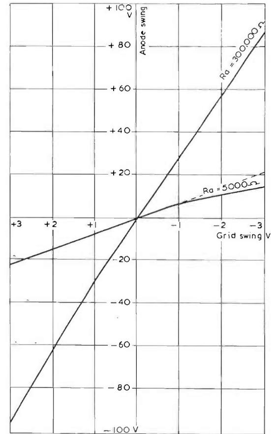
Fig. 9.11. Effect of anode load on dynamic characteristic.
