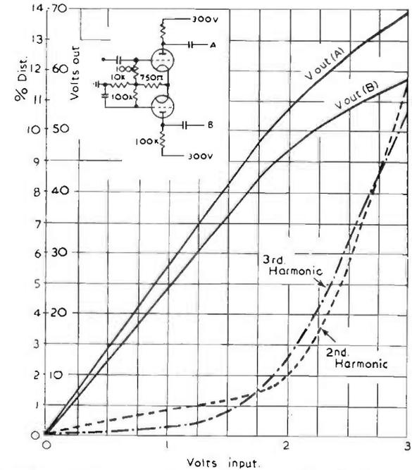
Fig. 9.30. Performance of a twin triode as a Schmitt phase splitter.
