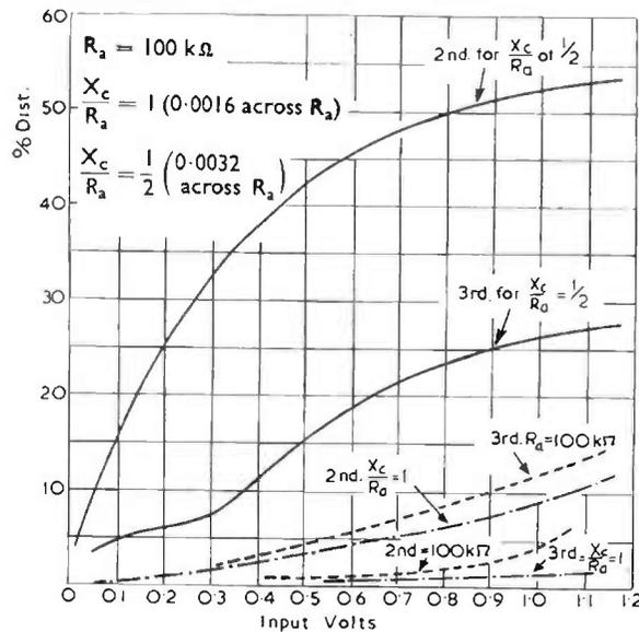
FIG. 9.15(a). Effect of reactive anode load on the distortion of an R.C. coupled stage.
