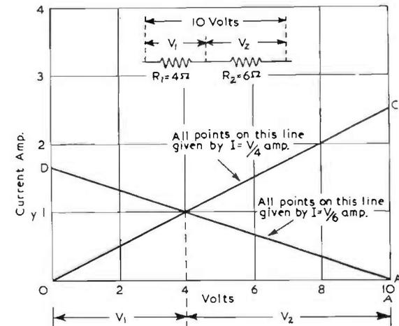
FIG. 9.2. Graphical construction for determining voltage distribution across resistors in series.
