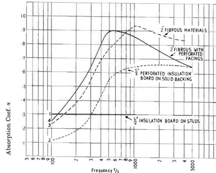
FIG. 17.23. Typical absorption coefficients.
