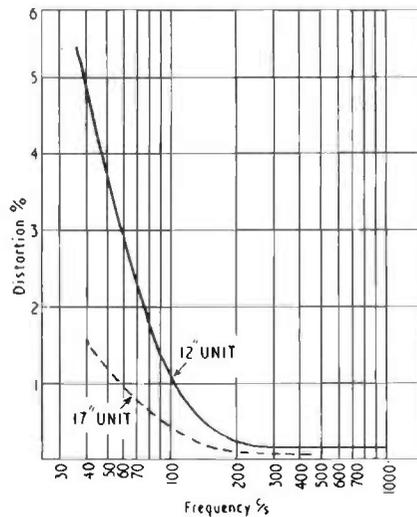
FIG. 16.9. Typical distortion/frequency relation for high quality speakers at 1 watt input.
