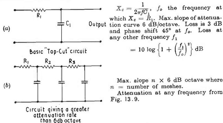
FIG. 13.7 (a-b). Top cut circuits.
