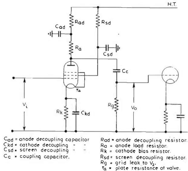
FIG. 9.21. Basic resistance capacitor coupled pentode voltage amplifier stage.
