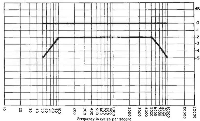
Tolerances on recorded levels and reproducing equipment response  $7\frac{1}{2}$  in/s
