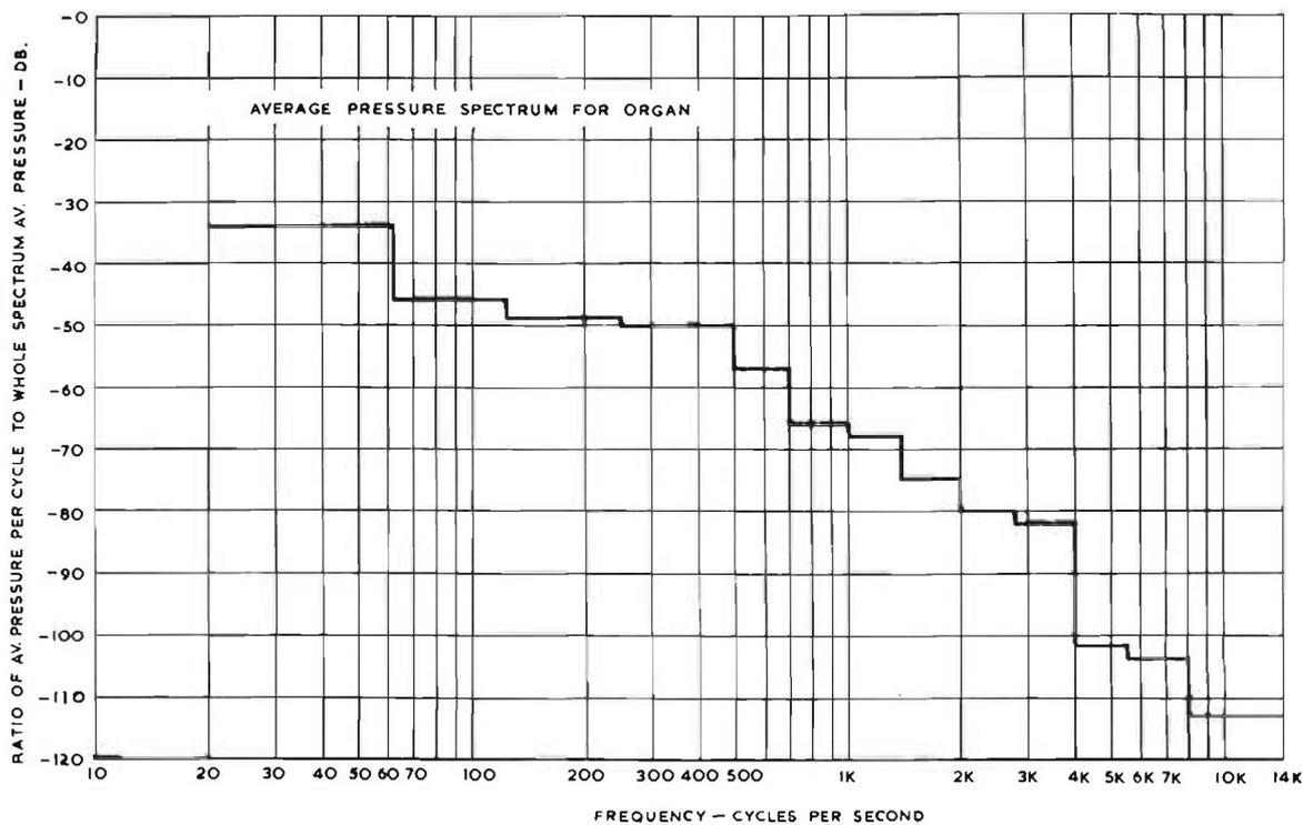
FIG. 1.8(b). Data from tests on two cinema organs ; average pressure spectrum.
