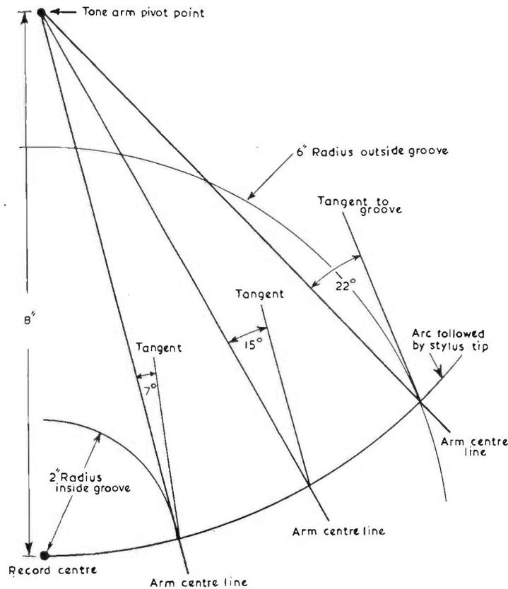
FIG. 7.10. Tone arm tracking diagram. Stylus point passing through centre of record.
