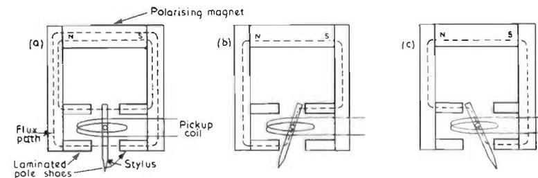
FIG. 7.14. Basic principle of magnetic pick-up.
