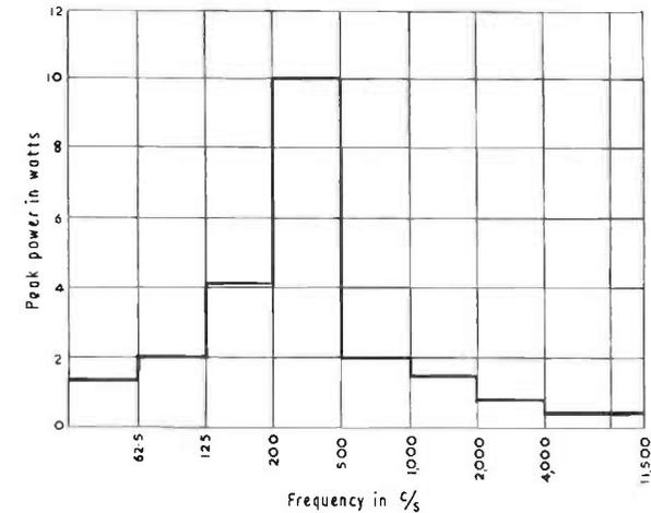
FIG. 15.1. Peak power (watts) in octave bands, based on data by Sivian, Dunn and White.
