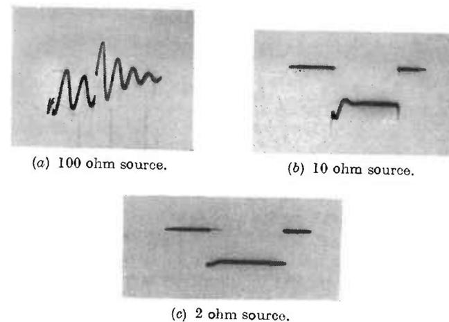
FIG. 16.13. Transient oscillations of loudspeaker voice coil when supplied from an amplifier having the indicated output impedance.
