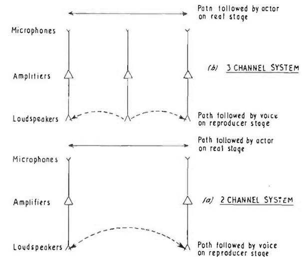
FIG. 19.1. Concave path followed by virtual position of voice in two and three channel stereophonic reproducer systems.
