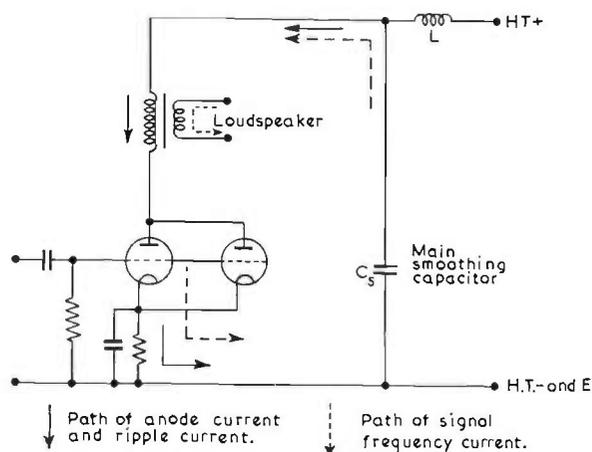
FIG. 10.2. Output valves in parallel.
