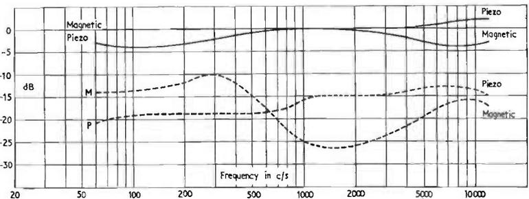
FIG. 7.26. Frequency response and cross-talk of typical magnetic and piezo-electric pick-ups. Cross-talk is shown by the broken line.
