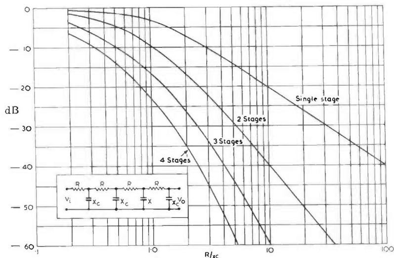
FIG. 9.28. Attenuation due to ladder networks of  $C$  and  $R$ .
