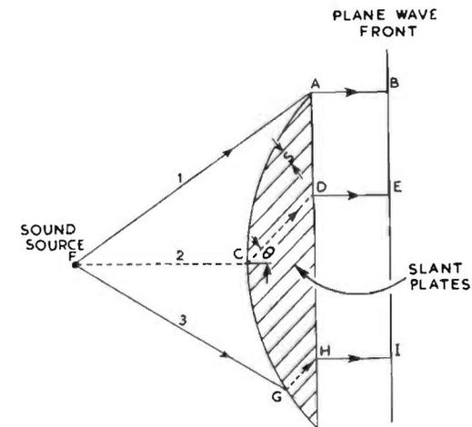
FIG. 16.49(b). Acoustical equivalent.
