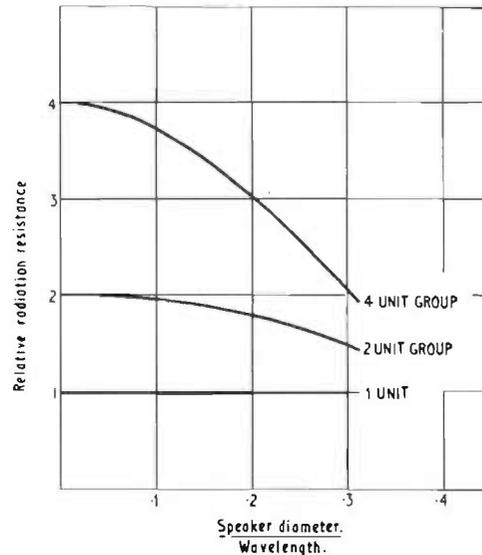
FIG. 16.18. Relative acoustic radiation resistance seen by each speaker of a close spaced group.
