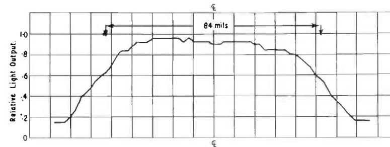
FIG. 18.12. Typical light distribution across scanning slit.
