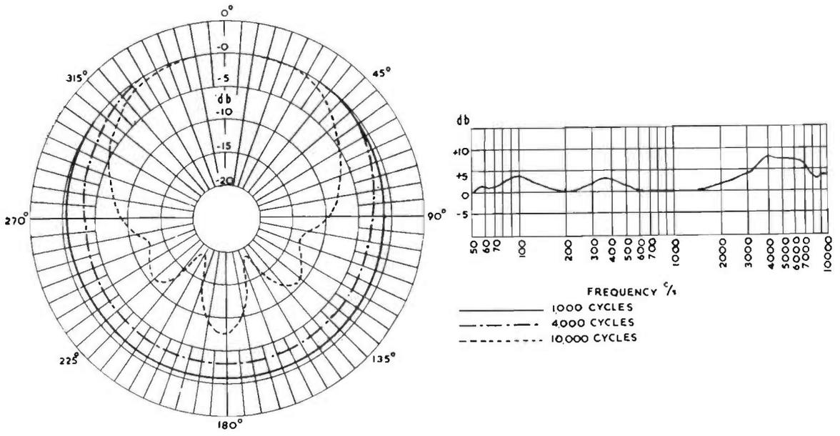
FIG. 5.19(b). Performance characteristics of R.C.A. Varacoustic Microphone Type LMI-6203-C. Pressure position.
