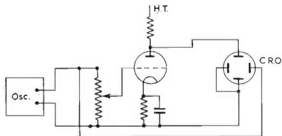
FIG. 9.8. Circuit for display of dynamic characteristic.
