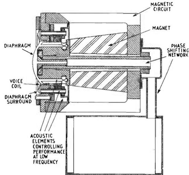
FIG. 5.21. Section of AKG Cardioid Moving Coil Microphone.
