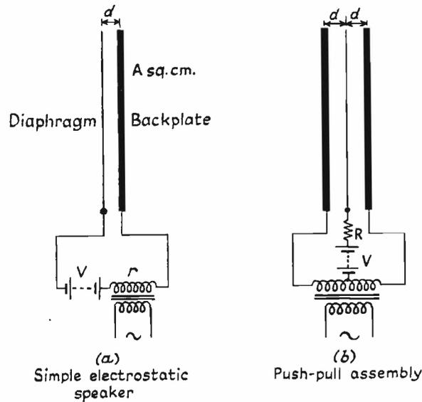
FIG. 16.36. Electrostatic speaker construction. (a) Simple construction. (b) Push-pull assembly.
