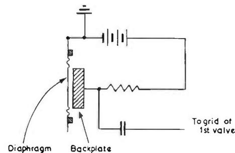
FIG. 5.9. Capacitor microphone coupling circuit.
