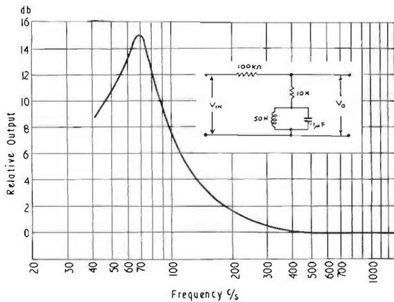
FIG. 13.5. Typical performance of a resonant bass boost circuit.
