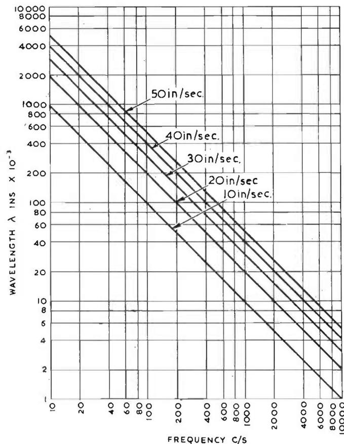
Fig. 7.1. Variation of wavelength with frequency at various cutting speeds.
