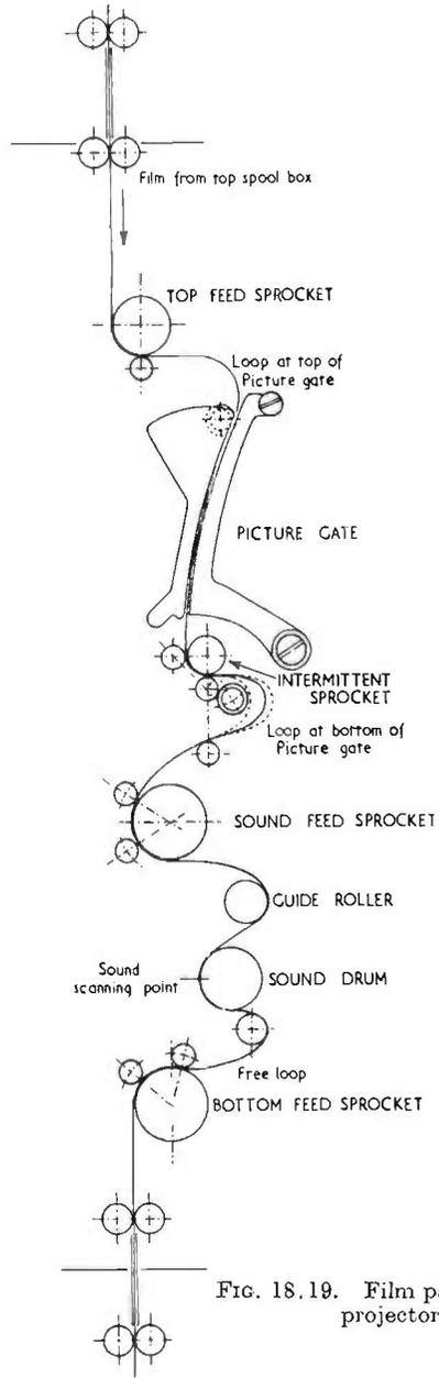
FIG. 18.19. Film path through projector.
