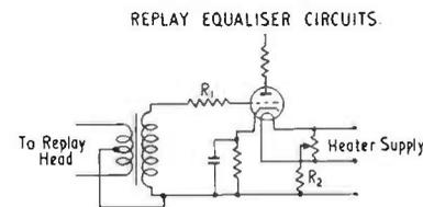
FIG. 8.16. Circuit diagram showing effect of failure of heater cathode insulation of valve.
