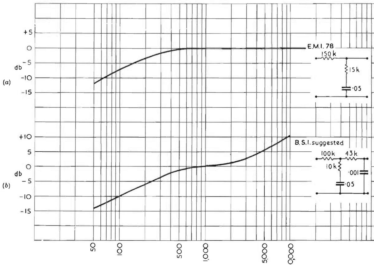
FIG. 7. 29(a)-(b). Recording characteristics and correction circuits. (a) E.M.I. 78 ; (b) B.S.I. 78.
