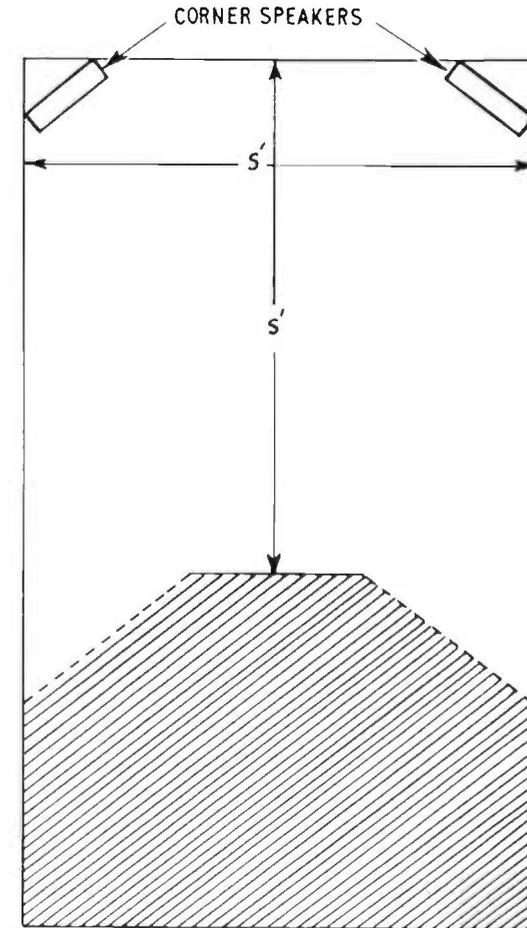
FIG. 19.7. Useable floor area using a two-channel stereophonic system.
