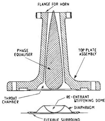
FIG. 16.45. Section of H.F. loudspeaker diaphragm and throat assembly.
