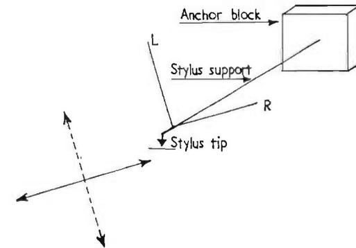
FIG. 7.22. Diagram of two-arm resolver.
