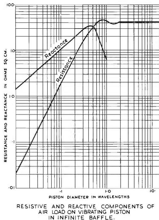
FIG. 16.2. Resistive and reactive components of air on vibrating piston in infinite baffle.
