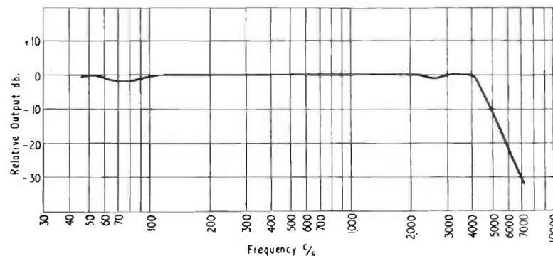
FIG. 4.2. Frequency characteristic of acoustic filters used in Olson's tests.
