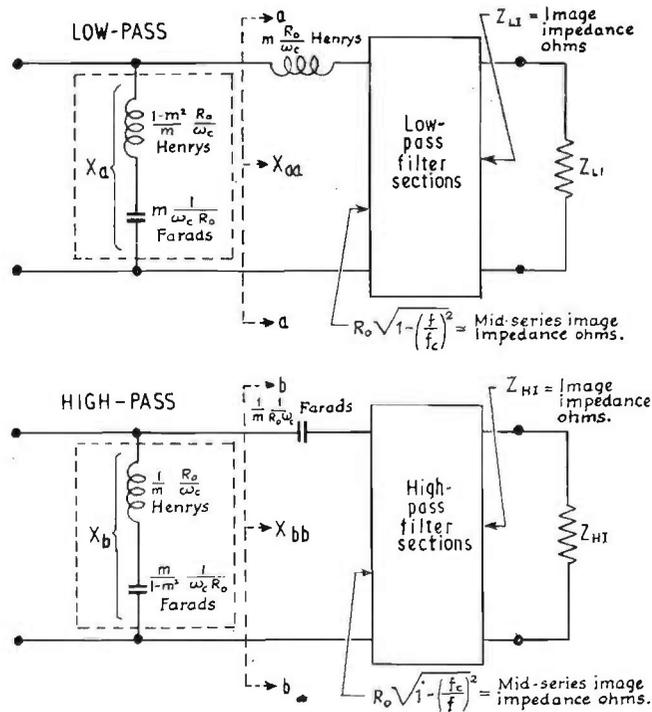
Fig. 15.2. Formation of filter type dividing networks.
