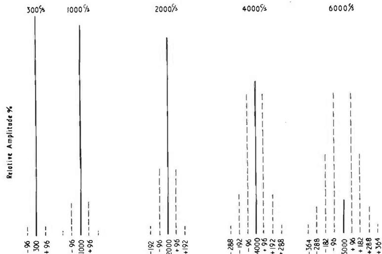
FIG. 18.18. Approximate distribution of sideband frequencies due to sprocket ripple for five recorded frequencies.
