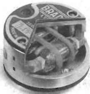
FIG. 8. 8. Cut-away view of re-play head. (Bradmatic)
