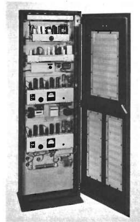
FIG. 18.20. Amplifier construction—Rack open—Units shut. (R.C.A.)
