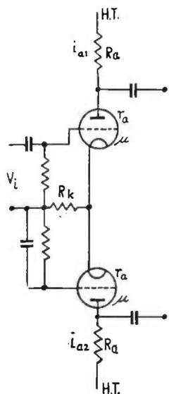
FIG. 9.40. Cathode-coupled phase-splitter.
