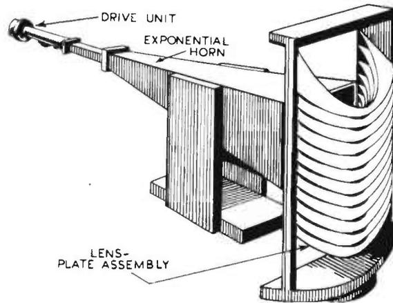
FIG. 16.50. Slant plate acoustic lens.
