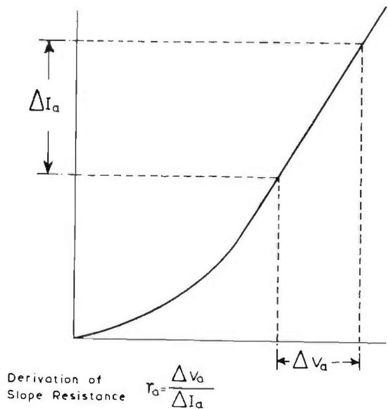
FIG. 9.16(b). Derivation of slope resistance.
