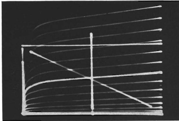
FIG. 10.8. Cathode ray display of  $I_a/E_a$  characteristic with resistive load.
