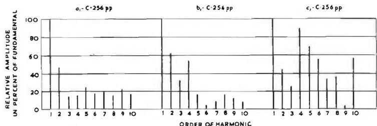
FIG. 1.11. Harmonic analysis of 256 cps note played on piano at three different loudness levels.
