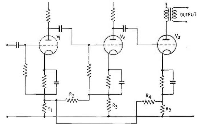
FIG. 12.8. Combination of positive and negative feedback.
