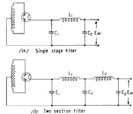
FIG. 14.6. Ripple filter circuits. (a) Single stage. (b) Two section.
