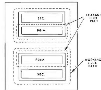
FIG. 11.4. Flux leakage diagram.
