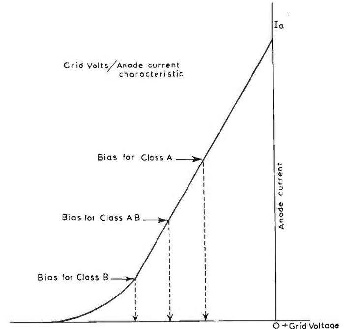
FIG. 10.1. Relative bias values for Class A, B, and AB operation.
