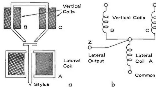
FIG. 7.25. (a) Diagram of Decca stereo pick-up; (b) internal connexions.
