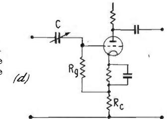
FIG. 13.1 (a-d). Bass cut circuits.
