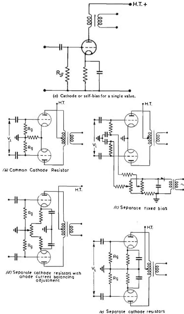
FIG. 10.15. Methods of biasing the output stage.
