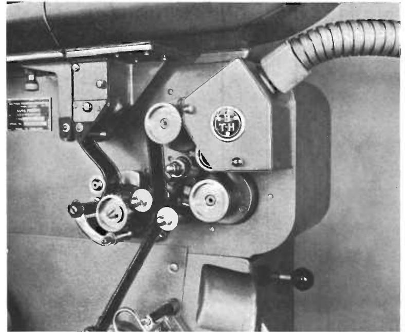
FIG. 18.27. CinemaScope magnetic reproducer head. (B.T.-H.)
