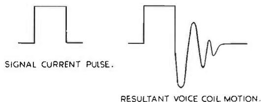
FIG. 10.11. Square pulse and cone motion.
