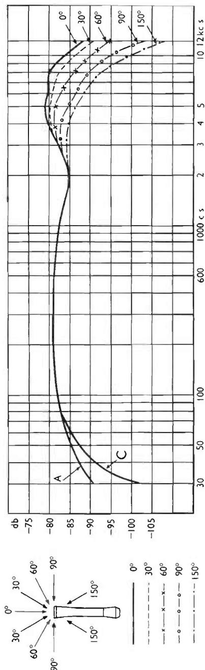
FIG. 5.8(b). Response curve of S.T.C. 4037 microphone (0 dB = 1 volt/dyne/sq. cm.)
