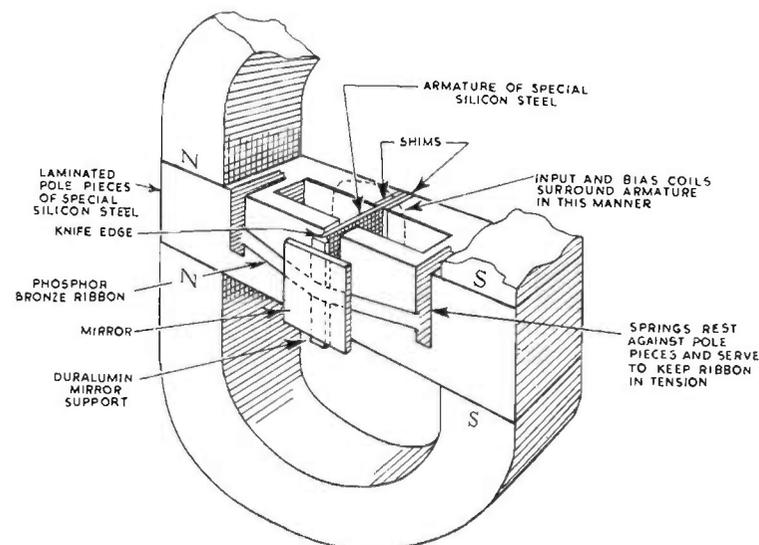
FIG. 18.5. General construction of RCA photophone magnetic galvanometer.
