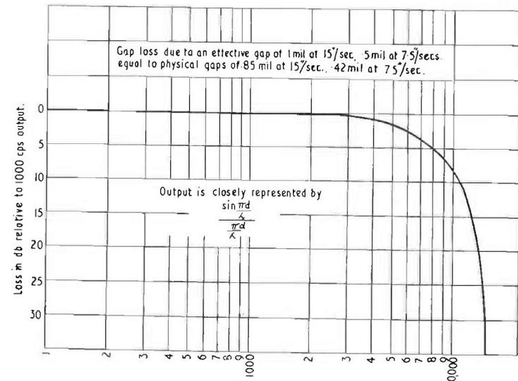
FIG. 8.12. Frequency characteristic due to gap loss only.
