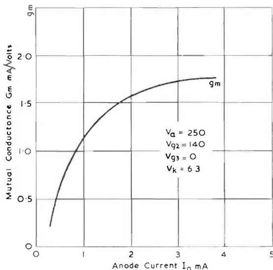
FIG. 9.17(b). Change in  $g_m$  for a typical pentode.
