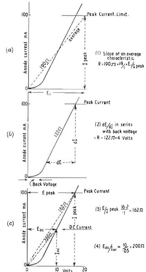
FIG. 14.9(a)-(c). Interpretations of rectifier valve resistance.
