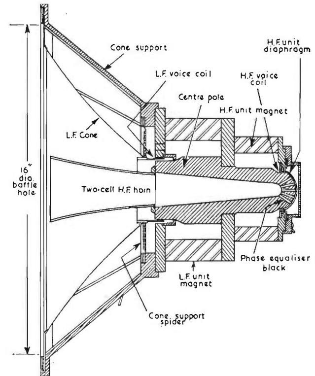
FIG. 16.34. B.T.-H. coaxial speaker. Type 213 H.
