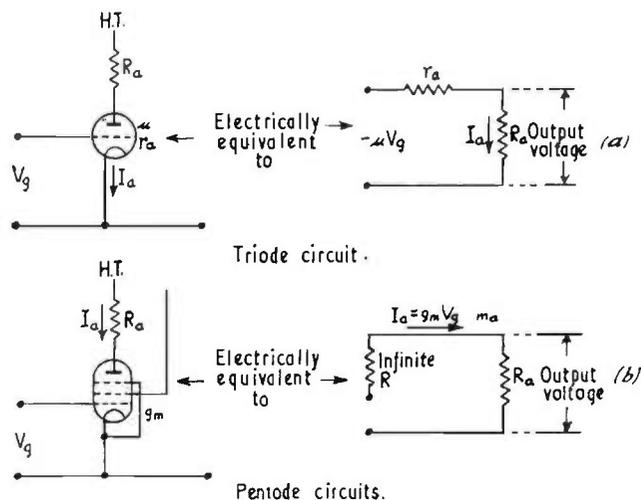
FIG. 9.35. Equivalent circuits.
