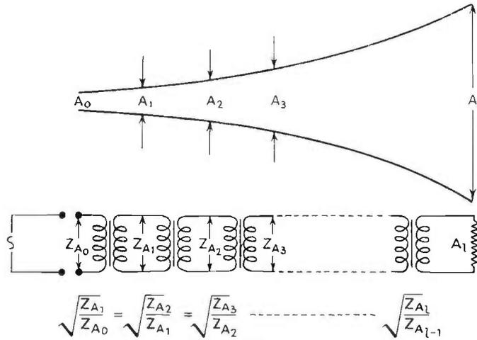
FIG. 16.40. Electrical analogue of exponential horn.
