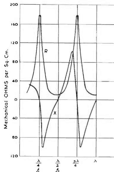
FIG. 16.22. Driving point impedance of a tube terminated in 10 ohms resistance.
