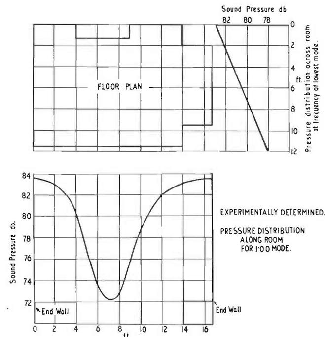
FIG. 17.19. Experimentally determined sound level distribution in a typical living room at lowest mode frequency 1.0.0.
