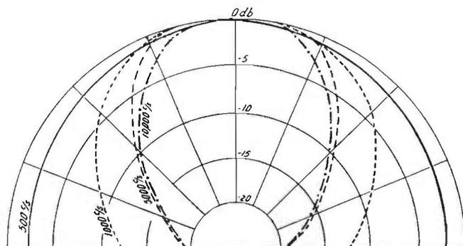
FIG. 16.7. Polar diagram of a high quality 12 in. speaker.
