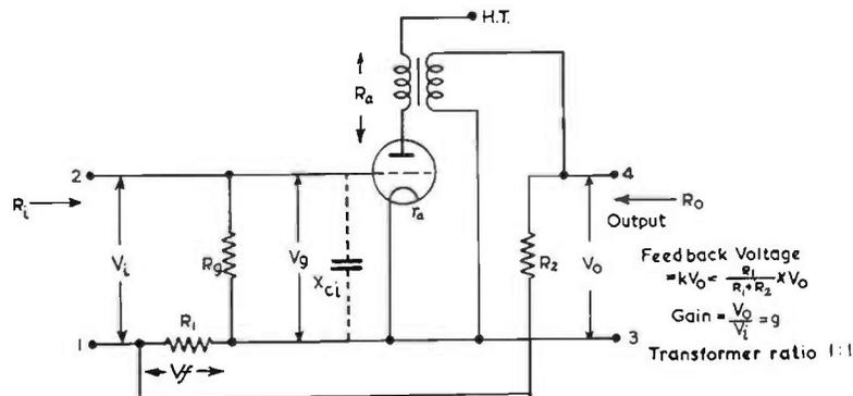
FIG. 12.1. Negative voltage feedback.
