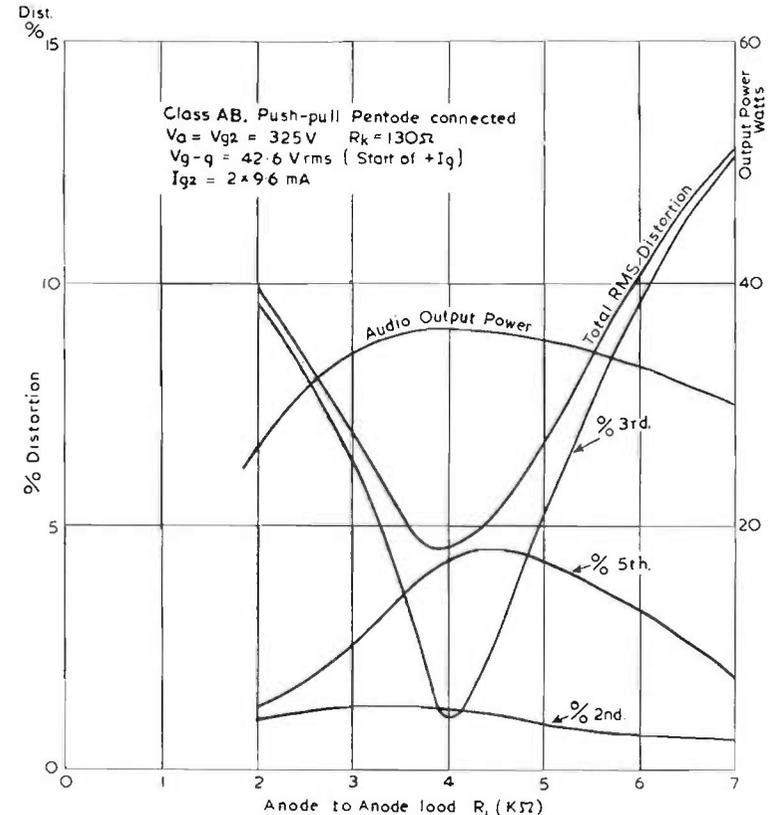
FIG. 10.7. Performance characteristic of EL37 as pentode.
