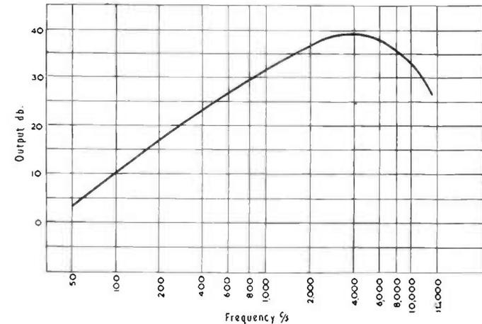
FIG. 8.10. Typical frequency response characteristic obtained from magnetic tape.
