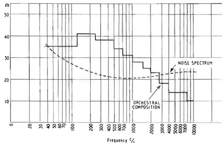
FIG. 7.7. Comparison of the frequency spectrum of surface noise and a typical orchestral composition. (Relative levels are arbitrary.)
