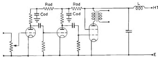
FIG. 9.26(b). Low frequency amplifier with decoupling.
