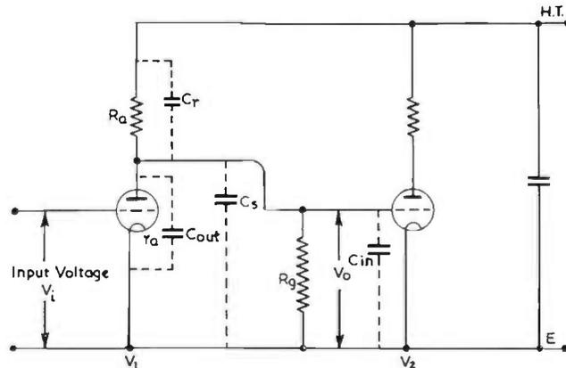
FIG. 9.23. R.C. stage showing important capacitances in H.F. range.
