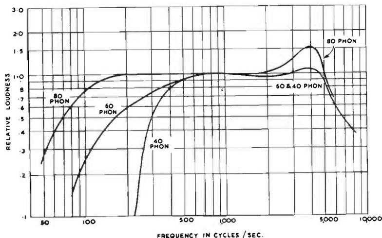
FIG. 3.6. Frequency characteristic of the ear as a function of loudness level.
