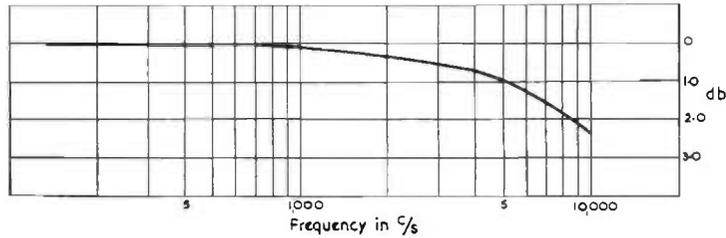
FIG. 18.14. Frequency characteristic of gas-filled photo cell.
