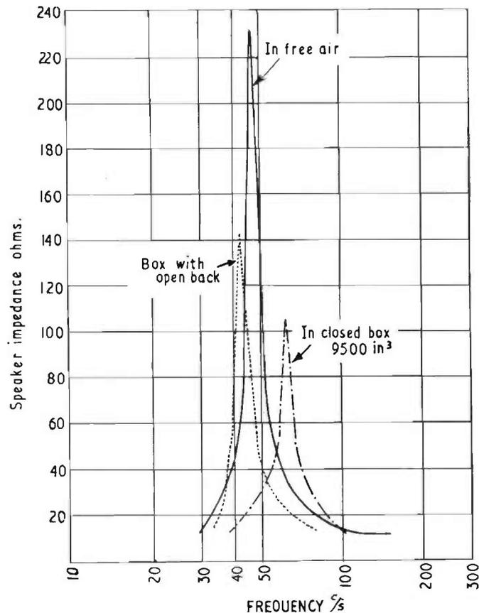
FIG. 16.20. Impedance of 12-in. speaker in free air and enclosure.
