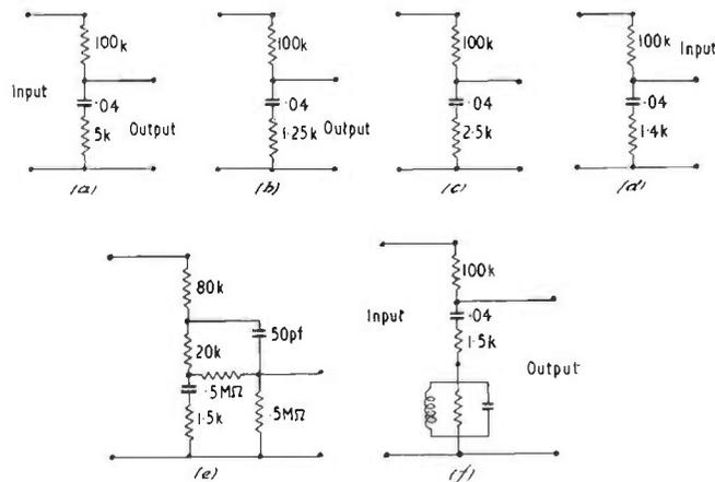
FIG. 8.14. Replay equalizer circuits.
