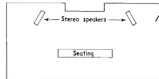
FIG. 19.8. Speaker placement resulting in poor stereo effect.
