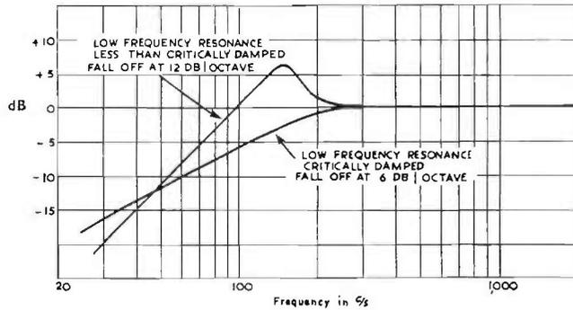
FIG. 16.3. Effect of damping of low frequency resonance on acoustic output of a cone loudspeaker.
