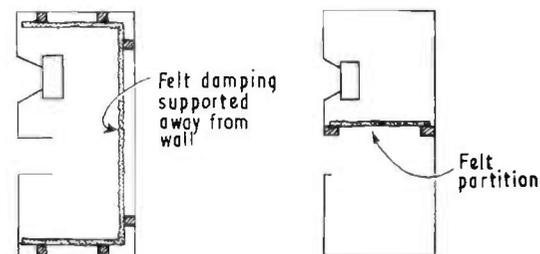
FIG. 16.30. Suggested methods of adding damping material to ported cabinet.
