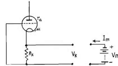
FIG. 9.39. Output impedance of a cathode follower.
