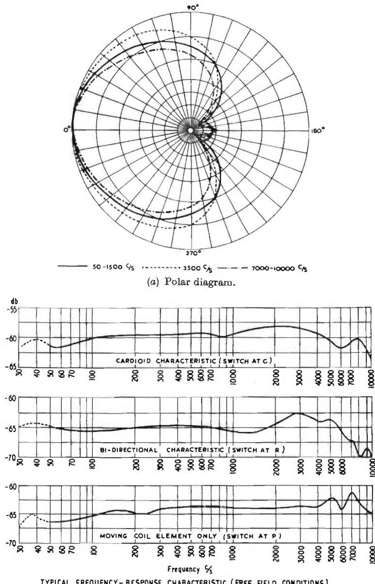
FIG. 5.18. Performance characteristics of Cardioid Microphone. S.T. & C. Type 4033.
