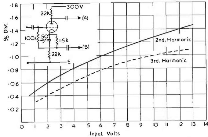
FIG. 9.32. Performance of a twin triode valve as an anode/cathode loaded phase splitter.
