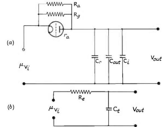
FIG. 9.24. Equivalent circuits of R.C. stage at H.F. range ; (a) is equivalent to (b) when  $C_i = \text{sum of } C_r, C_{out} \text{ and } C_a$ .  $R_e = \text{parallel continuation of } R_a, R_g, \text{ and } r_a$ .
