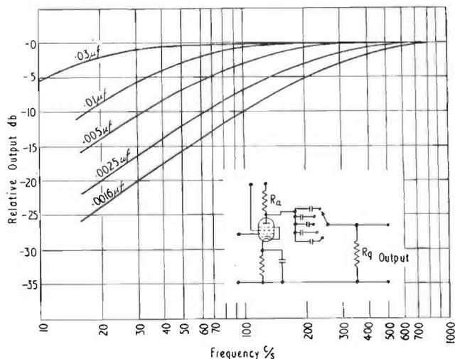
FIG. 13.1 (e). Basic cut characteristics produced by indicated values of coupling capacitor and  $R_a + R_g = 330 \text{ k}\Omega$ .
