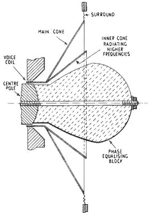
FIG. 16.53. Section of Lowther twin cone speaker.
