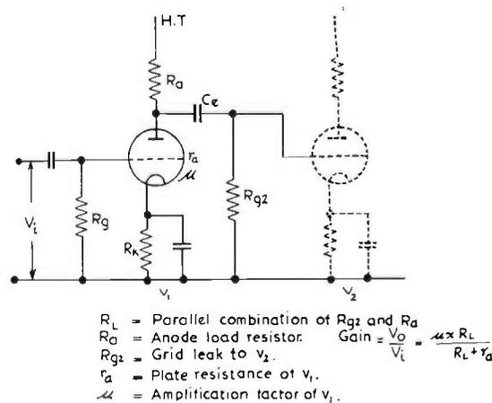
FIG. 9.20. Basic triode voltage amplifier stage
