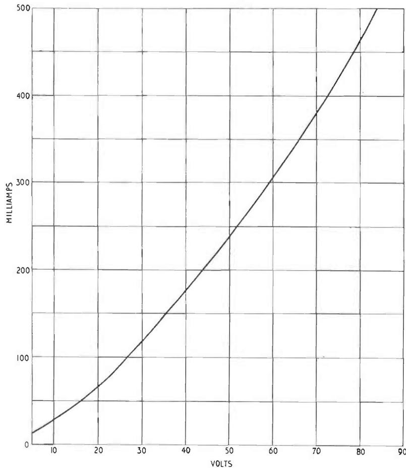
FIG. 14.1. Typical  $I_a/V_a$  relation for thermionic rectifiers.
