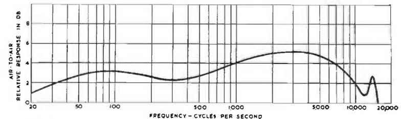
FIG. 3.12. Frequency characteristics of sound reproducer system used for subjective evaluation of the frequency spectrum of orchestral instruments.
