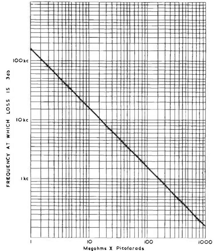
FIG. 9.25. H.F. loss as a function of  $R_e$  and  $C_t$ .
