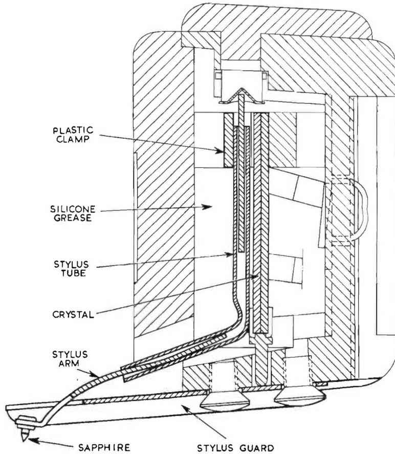
FIG. 7.19. Cosmocord GP39 pick-up shown in section.
