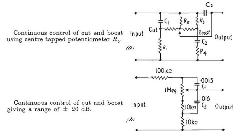
FIG. 13.6 (a-b). Continuous control of bass boost or attenuation.
