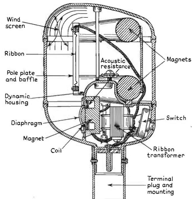
FIG. 5.17. Western Electric Cardioid Microphone, Type 639A. British Equivalent S.T. & C. Type 4033.
