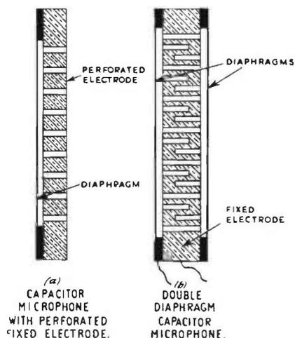
FIG. 5.23. Capacitor microphones.
