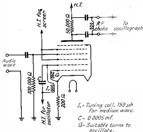
FIG. 104.—OCTODE MODULATION.
