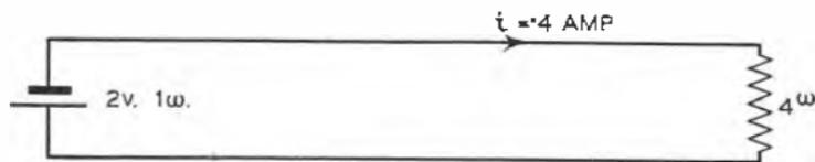
FIG. 23.—FINDING THE INTERNAL RESISTANCE IN THE BATTERY.
