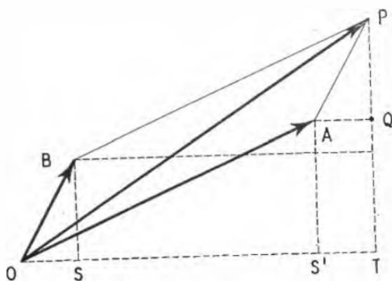
FIG. 65.—ADDITION OF SINE CURVES BY VECTORS.
