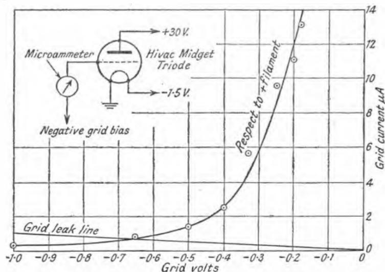
FIG. 107.—CURVE FOR A DIODE.
