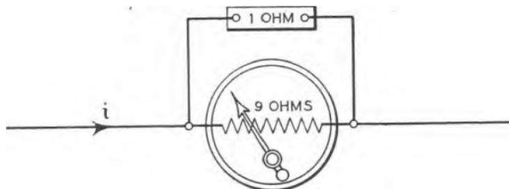
FIG. 16.—AMMETER SHUNTED WITH LOW RESISTANCE.
