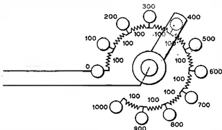
FIG. 19.—A DIAL TYPE OF VARIABLE RESISTANCE.
