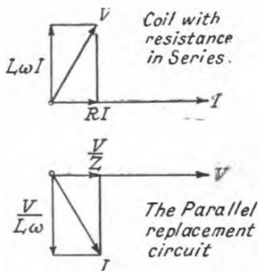
FIG. 75.—VECTOR DIAGRAMS FOR COIL AND ITS REPLACEMENT.
