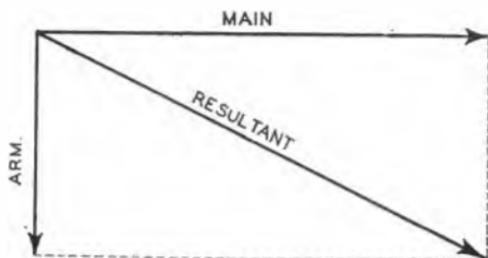
FIG. 58.—DISTORTION DUE TO ARMATURE REACTION FLUX.
