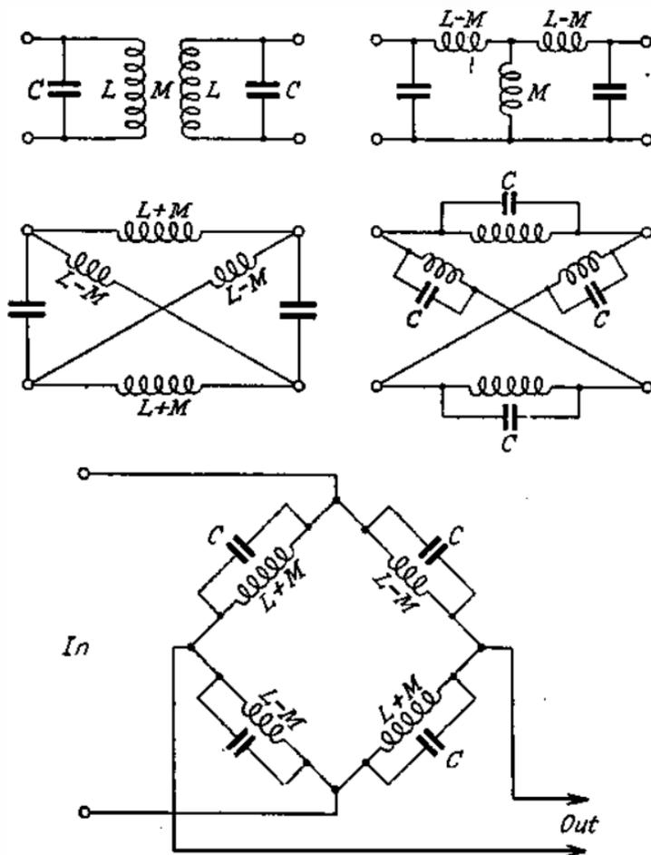
FIG. 130.—CIRCUIT EQUIVALENTS OF TUNED TRANSFORMER.
