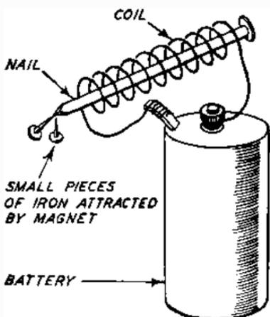
FIG. 3.—A NAIL AS AN ELECTRO-MAGNET.
