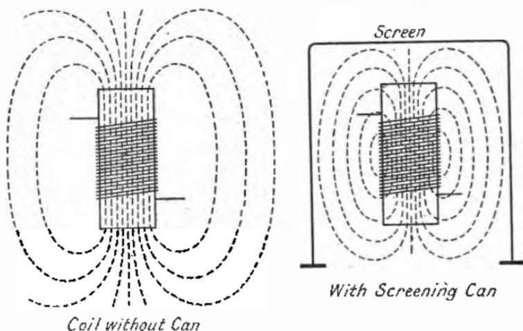
FIG. 163.—EFFECT OF SCREENING IN MAGNETIC FIELD.
