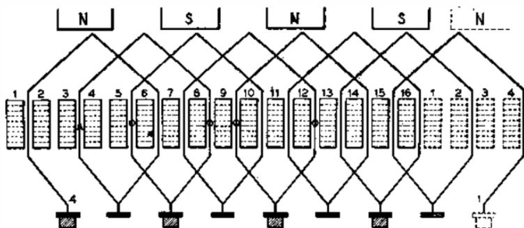
FIG. 44.—A FOUR-POLE LAP ARMATURE WINDING.
