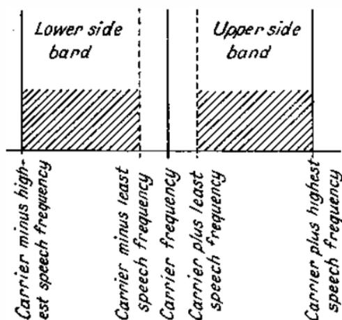
FIG. 98.—THE SIDE BANDS OF A MODULATED WAVE.
