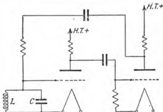
FIG. 182.—DOUBLE VALVE OSCILLATOR.
