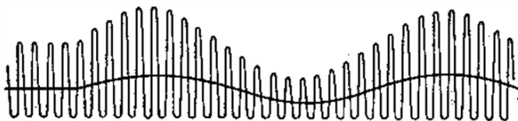
FIG. 105.—ONE-DIRECTION CURRENT PULSES PRODUCED BY MODULATOR CARRIER.
