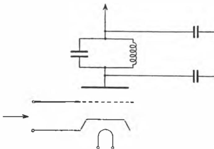
FIG. 191.—CIRCUIT FOR FREQUENCY DOUBLING.
