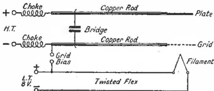
FIG. 190.—OSCILLATOR FOR 2 TO 3 METRES.
