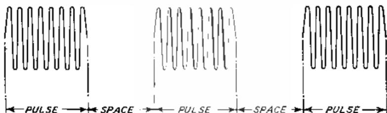
FIG. 99.—PULSE-TIME MODULATION. DURING MODULATION THE SPACING CHANGES.
