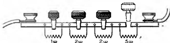
FIG. 20.—PLUG TYPE VARIABLE RESISTANCE.
