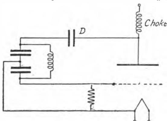
FIG. 93.—COLPITTS OSCILLATOR (SHUNT FED).
