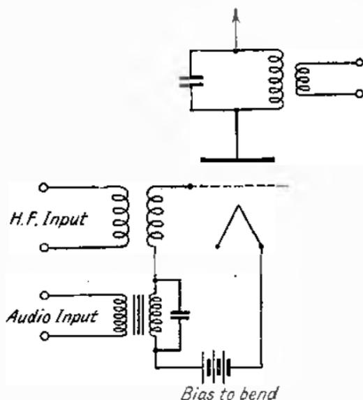
FIG. 101.—ANODE BEND MODULATION.
