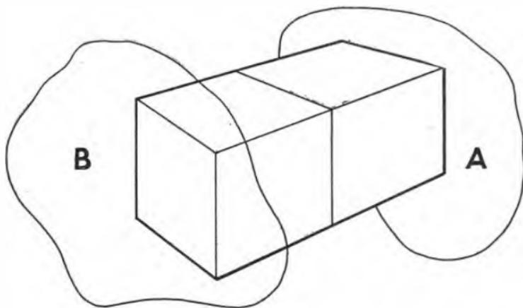
FIG. 22.—CONDUCTOR MADE OF TWO CUBES IN SERIES.
