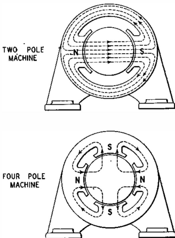
FIG. 43.—THE FLUX PATHS IN TWO AND FOUR-POLE MACHINES.
