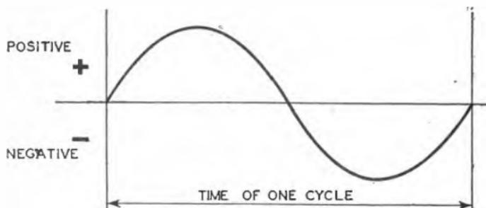
FIG. 27.—CURVE OF AN ALTERNATING CURRENT.
