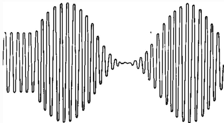
FIG. 125A.—COMPLETELY MODULATED WAVE.
