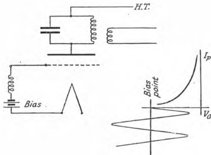
FIG. 122.—CLASS C AMPLIFICATION.
