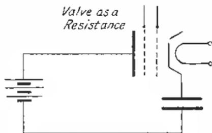
FIG. 135.—TIME BASE CIRCUIT SIMPLIFIED.
