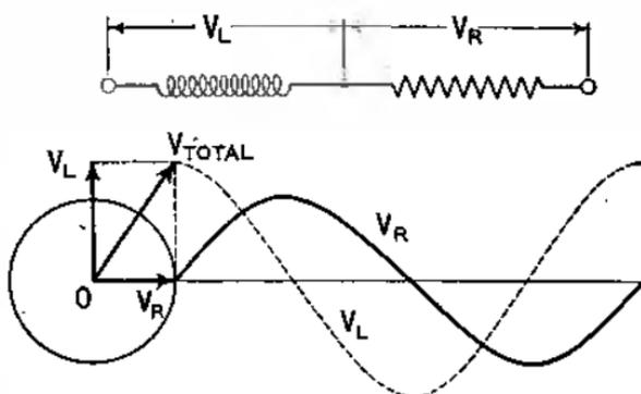
FIG. 64.—CURRENT AND VOLTAGES IN AN INDUCTIVE CIRCUIT.
