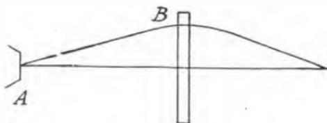
This is done in modern oscillographs in a most ingenious manner. A cylinder is placed as a circus hoop through which the electrons must pass. It has a negative bias which can be varied. The action is shown in Fig. 131.
