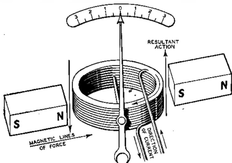
FIG. 9.—CONSTRUCTION OF MOVING COIL AMMETER.
