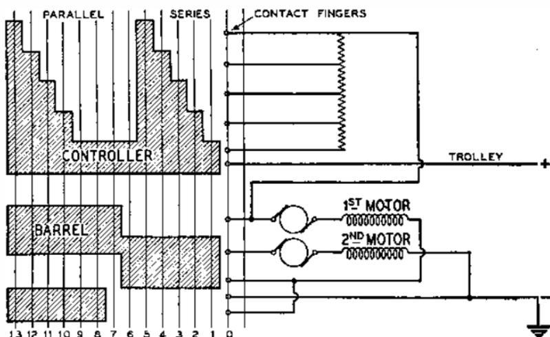
FIG. 56.—CONTROL DIAGRAM OF TRAMCAR WITH TWO MOTORS.
