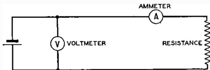
FIG. 15.—THE CONNECTIONS OF A VOLTMETER.
