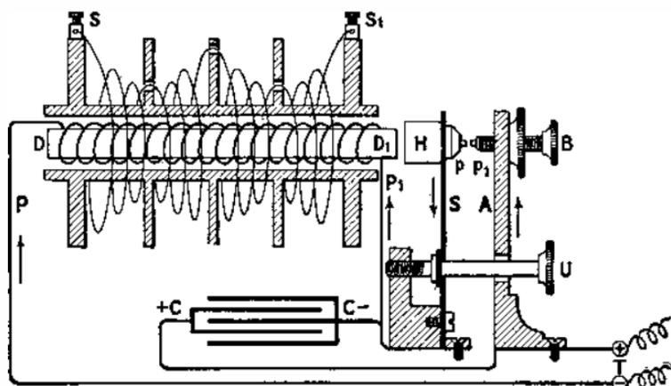
FIG. 28.—THE CONSTRUCTION OF AN INDUCTION COIL.
