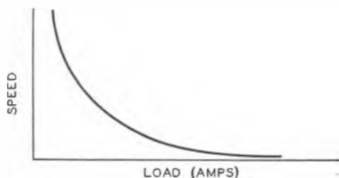
FIG. 55.—SPEED-LOAD CURVE OF A SERIES WOUND MOTOR.
