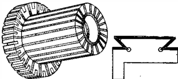
FIG. 38.—A COMMUTATOR.
