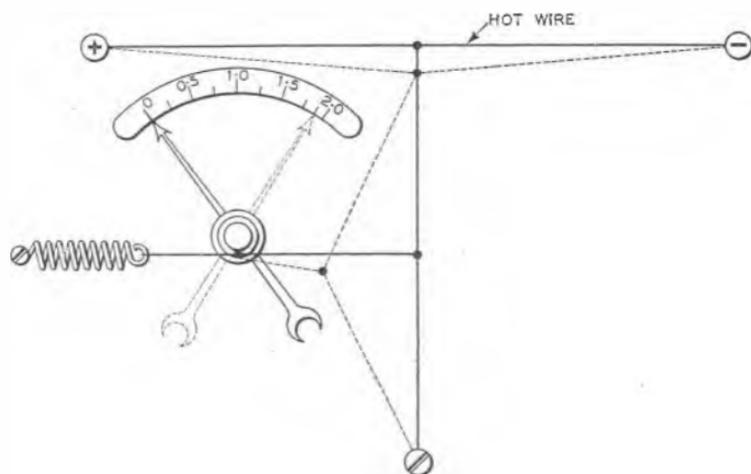
FIG. 7.—HOT WIRE AMMETER.
