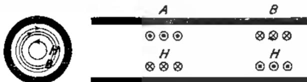
FIG. 173.—THE ELECTRIC AND MAGNETIC FLUXES IN AN ELECTRIC WIRE IN A ROUND GUIDE.
