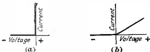
FIG. 106.—IDEAL DETECTOR CHARACTERISTICS.
