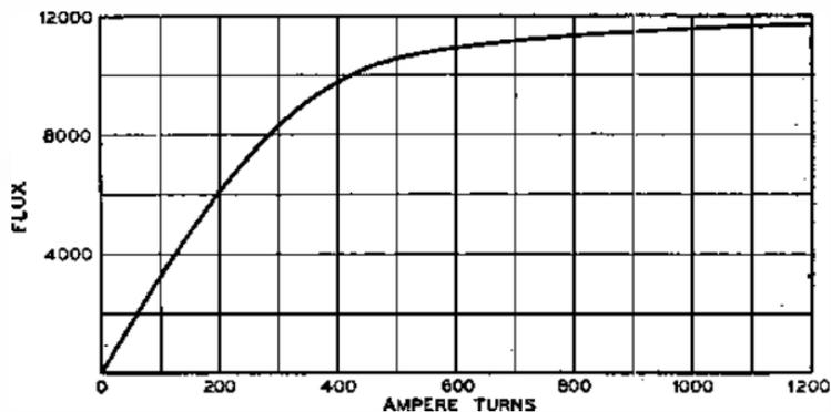
FIG. 51.—FLUX CURVE IN TELEPHONE RELAY.
