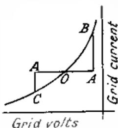
FIG. 109.—ONE CYCLE OF I.F. CURRENT SHOWING DIFFERENTIAL EFFECT IN LEAKY GRID DETECTION.
