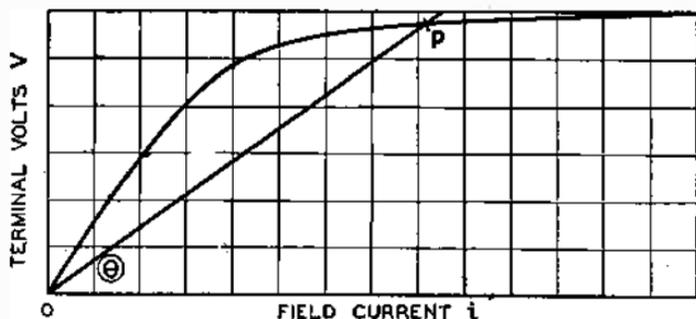
FIG. 52.—THE EQUILIBRIUM VOLTAGE OF A SHUNT WOUND DYNAMO.
