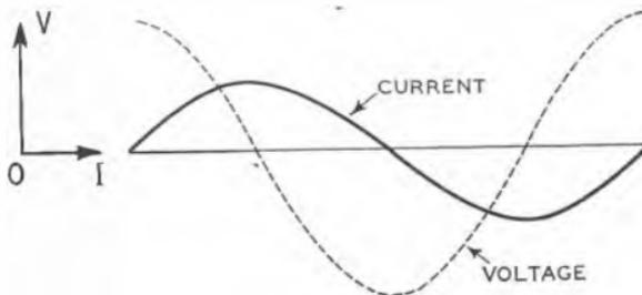
FIG. 63.—CURRENT AND VOLTAGE ON A PURE INDUCTANCE.
