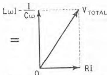
FIG. 68.—VOLTAGE LEADING OR LAGGING.
