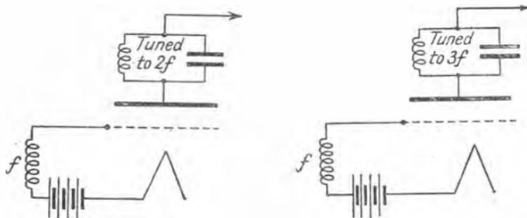
FIG. 145.—FREQUENCY DOUBLER. FIG. 146.—FREQUENCY TREBLER.
