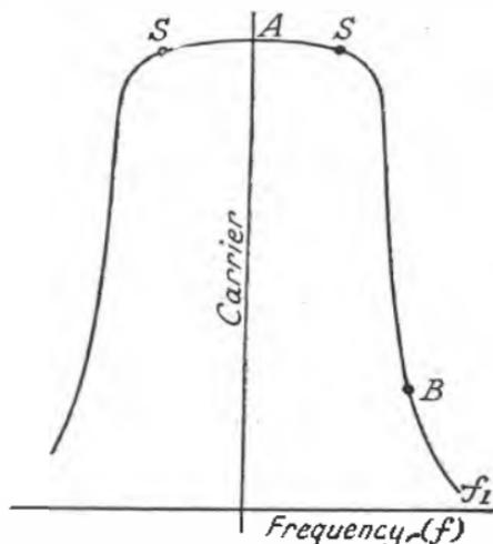
FIG. 129B.—RESONANCE CURVE OF BAND PASS FILTER.
