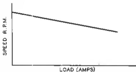
FIG. 54.—SPEED-LOAD CURVE OF A SHUNT WOUND MOTOR.
