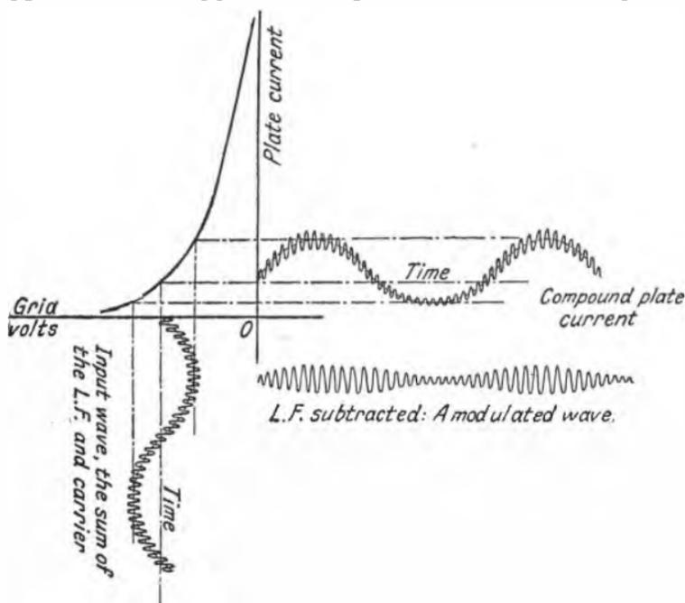
FIG. 102 — SHOWING THE DISTORTION OF L.F. WAVE WITH PRODUCTION OF PRONOUNCED RIPPLE.
