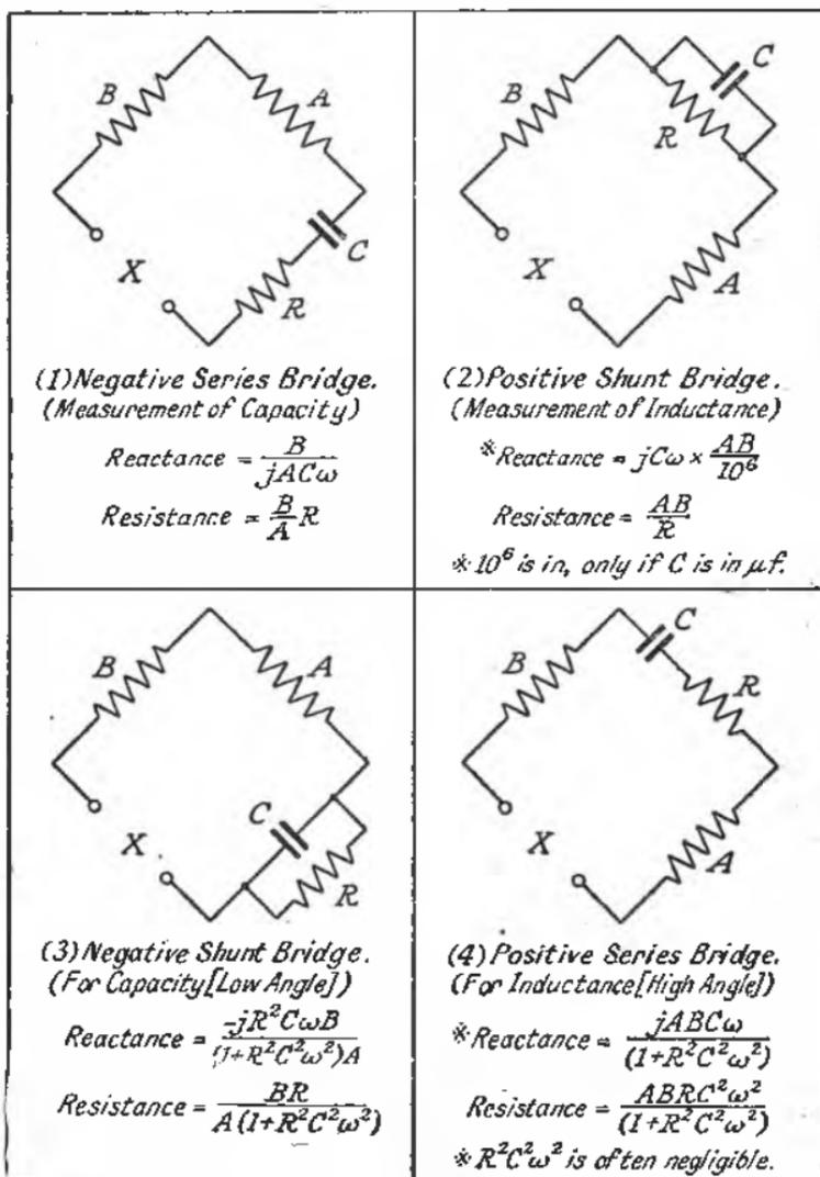
FIG. 149.—FOUR BRIDGES USING CAPACITY STANDARD.
