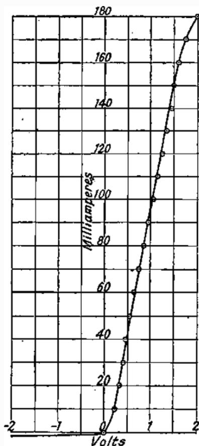
FIG. 79.—TEST ON A CRYSTAL.
