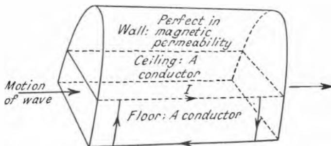
FIG. 70.—RADIO WAVE TRAVELLING DIRECTIONALLY IN SPACE.
