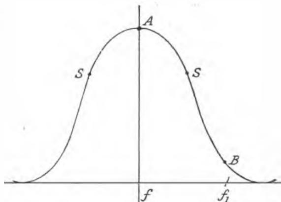
FIG. 129A.—SELECTING A WEAK STATION OVER A STRONG STATION.
