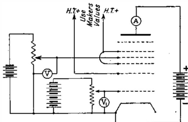
FIG. 180.—CIRCUIT FOR TAKING OCTODE CHARACTERISTICS.
