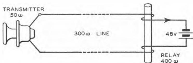
FIG. 12.—IMPULSE RELAY IN CIRCUIT WITH TELEPHONE TRANSMITTER.
