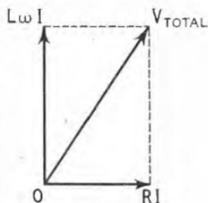
FIG. 66.—VOLTAGES IN AN INDUCTIVE CIRCUIT.
