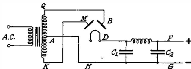
FIG. 165.—RECTIFYING AND SMOOTHING FROM A.C. MAINS.
