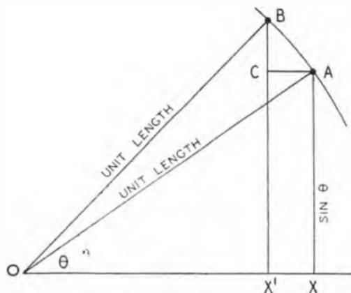
FIG. 61.—THE SLOPE OF A SINE CURVE.
