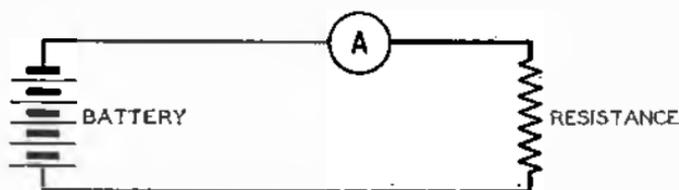
FIG. 14.—THE CONNECTIONS OF AN AMMETER.
