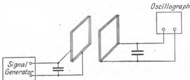
FIG. 184.—COMPONENTS OF TUNED TRANSFORMER BAND PASS FILTER.
