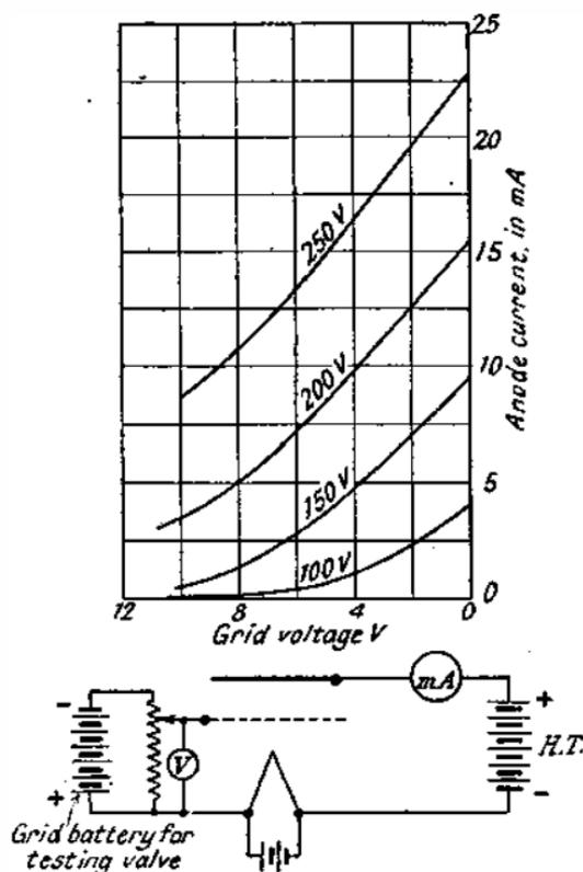
FIG. 81.—CURVES FOR TRIODE VALVE.
