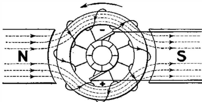
FIG. 37.—THE GRAMME RING ARMATURE.
