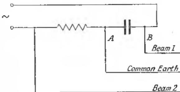
FIG. 179.—VECTOR ADDITION OF VOLTAGES.
