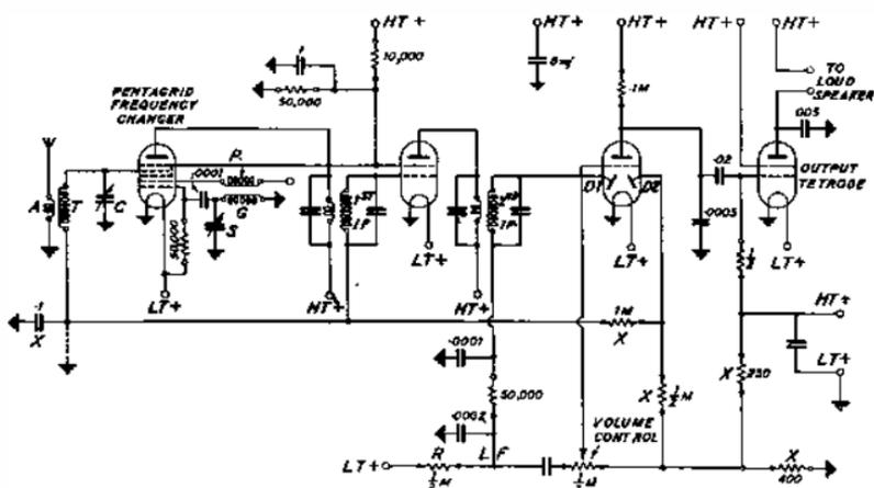
FIG. 166.—THEORETICAL DIAGRAM OF A BATTERY TYPE SUPER-HETERODYNE RECEIVER.
