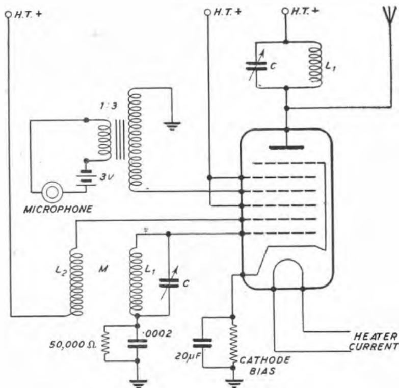
FIG. 197.—WIRING DIAGRAM OF SIMPLE BROADCAST TRANSMITTER.
