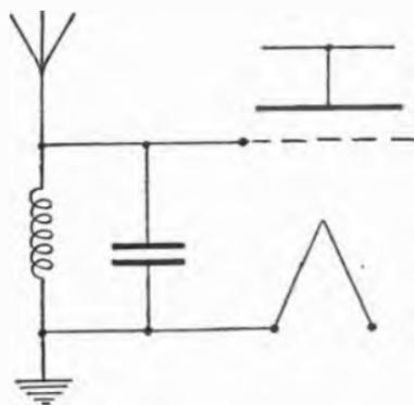
FIG. 77.—PARALLEL RESONANCE IN A RECEIVER CIRCUIT.
