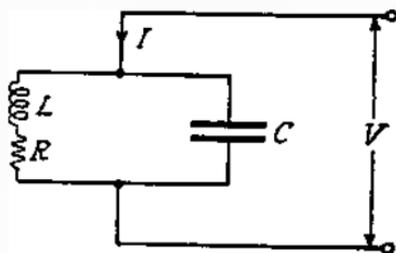
FIG. 73.—A COIL AND CONDENSER IN PARALLEL.
