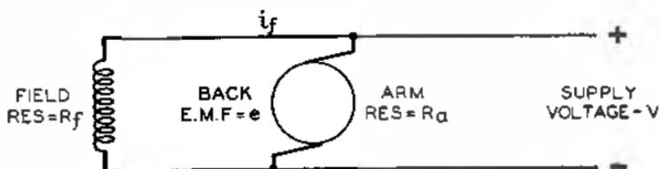
FIG. 53.—THE E.M.F.'S IN A SHUNT MOTOR.
