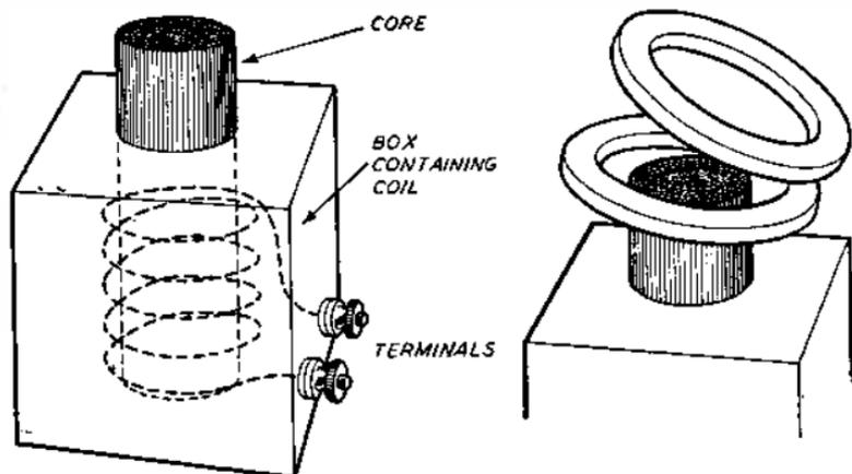
FIG. 196.—EXPERIMENT FOR DEMONSTRATING EDDY CURRENTS.
