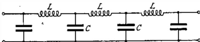
FIG. 136.—THE LOW PASS FILTER.
