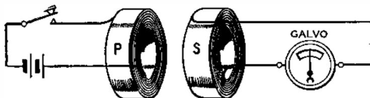
FIG. 26.—CURRENT INDUCED BY ONE COIL IN ANOTHER.
