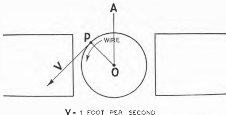
FIG. 34.—THE DIRECTION OF MOTION OF A WIRE ON AN ARMATURE.
