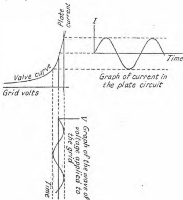
FIG. 113.—THE VALVE AS AN AMPLIFIER.
