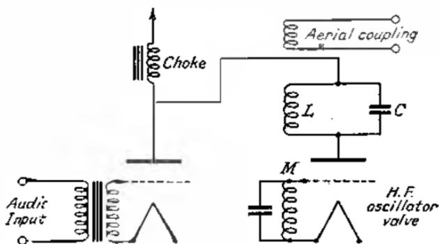
FIG. 103.—CHOKE MODULATION CIRCUIT.
