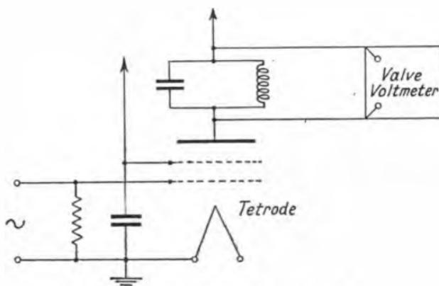
FIG. 186.—PARALLEL RESONANCE.
