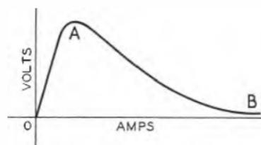
FIG. 176.—GRAPH OF SUBSTANCE HAVING "DYNAMIC" NEGATIVE RESISTANCE.
