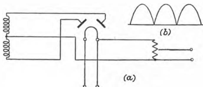
FIG. 192.—FULL WAVE RECTIFIER.
