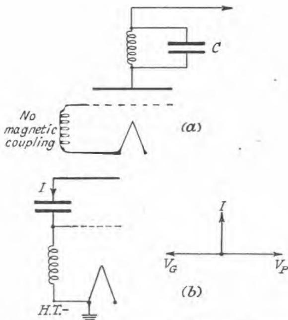
FIG. 94. OSCILLATOR ELECTRODE CAPACITY COUPLING
