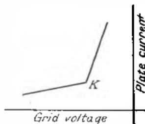
FIG. 111.—ANODE BEND DETECTOR CURVE.
