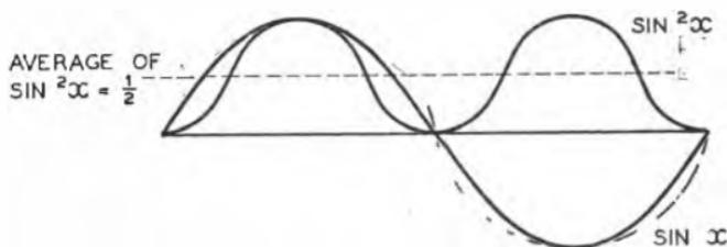
FIG. 62.—THE SQUARE OF A SINE CURVE.
