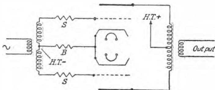
FIG. 117.—PUSH PULL AMPLIFICATION.
