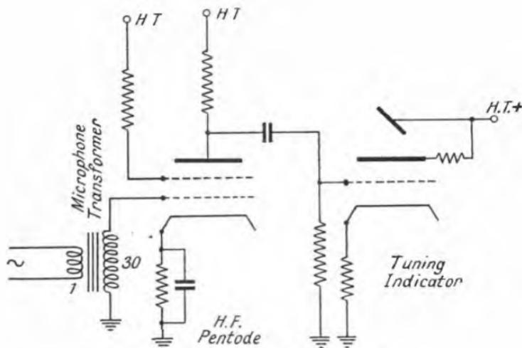
FIG. 152.—A BRIDGE DETECTOR.
