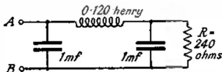
FIG. 137.—A FILTER SECTION.
