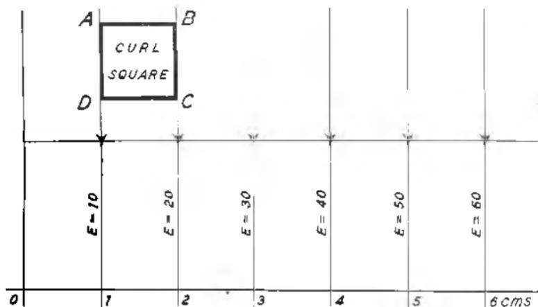
FIG. 167.—A NON-UNIFORM FIELD OF ELECTRIC FORCE
