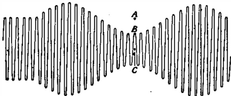
FIG. 125B.—A COMMON MODULATED WAVE.
