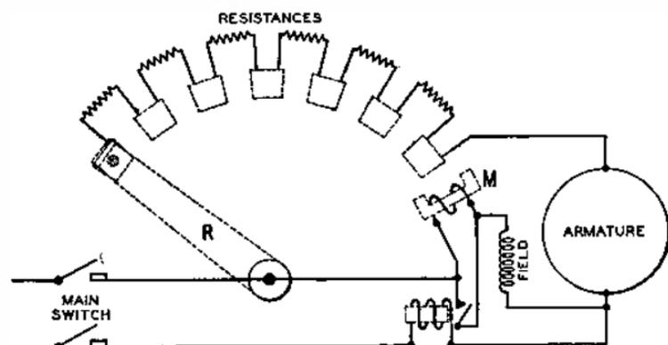
FIG. 59.—SHUNT MOTOR STARTER.
