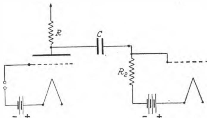
FIG. 116.—RESISTANCE CAPACITY COUPLING.
