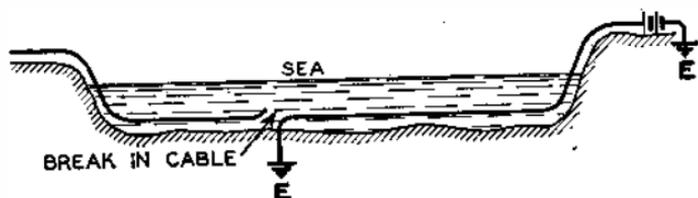
FIG. 17.—A SUBMARINE CABLE WITH A FAULT.
