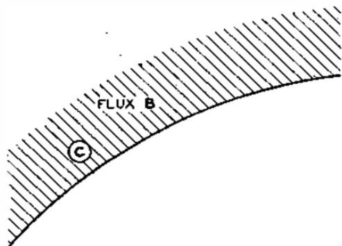
FIG. 49.—CONDUCTOR IN A FLUX.
