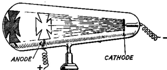
FIG. 1.—ELECTRONS FLOWING IN A VACUUM.
