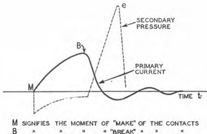
FIG. 30.—CURRENT AND VOLTAGE IN AN INDUCTION COIL.
