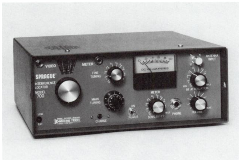
Fig. 10 Model 700 portable interference locator covers broadcast band through tv channel 13. Receiver is battery equipped and has video output terminal so photograph of interference can be made with auxillary oscilloscope.
