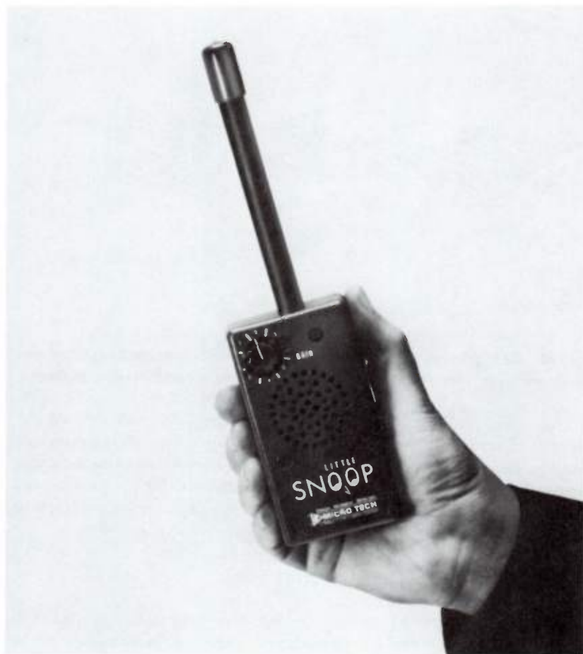
Fig. 13 Hand held RFI “snooper” picks up RFI and aids in locating noise source. It is designed to be used in vicinity of high voltage lines.
