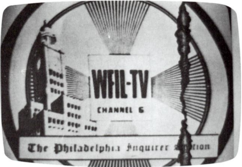
Fig. 15 Transistor oscillation in tv receiver produces vertical line on the screen. Problem can be eliminated by circuit modification performed by a serviceman.
