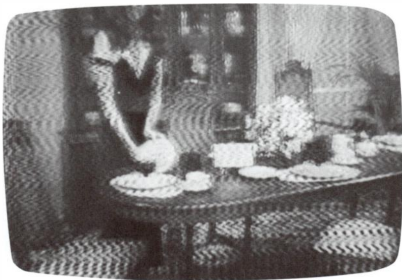
Fig. 7 "Herringbone weave" pattern on tv screen is caused by interference from nearby fm broadcast station. This interference is limited to older sets and may be cured by addition of fm trap filter in the antenna circuit.
