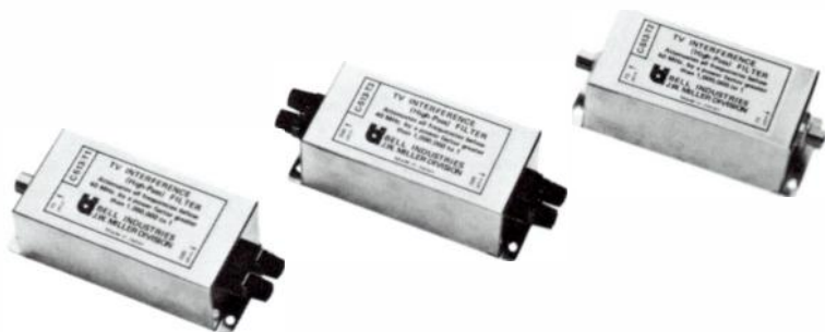
Fig. 12 Representative high-pass filters that will help to protect the tv receiver against overload from strong signals. Filter should be mounted as close to the input terminals of the tv tuner as possible. These filters are made by the J.W. Miller division of Bell Industries. Filters made by Drake, Barker and Williamson and other manufacturers are also available.
