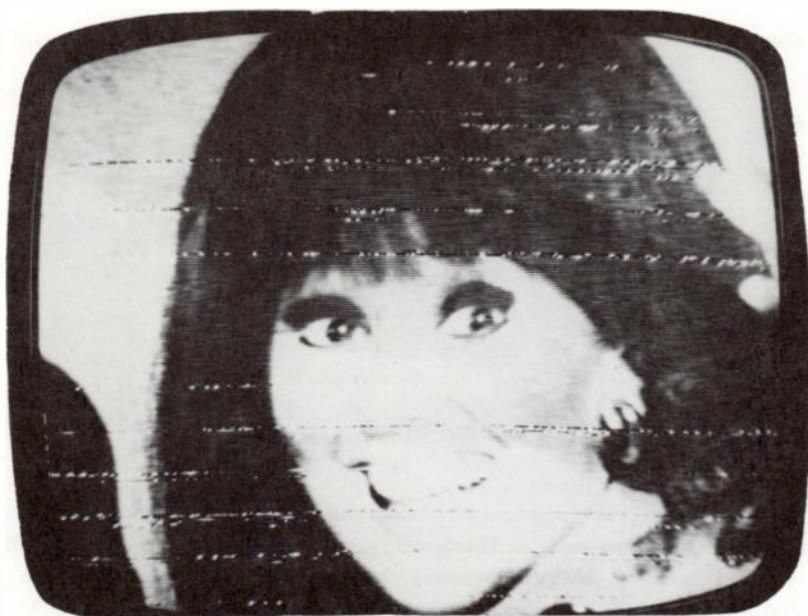
Fig. 5 (above) Spark discharge creates "shot lines" on TV screen and shows up as sharp pulses on oscilloscope pattern (below). This interference pattern is often caused by passing autos and trucks.
