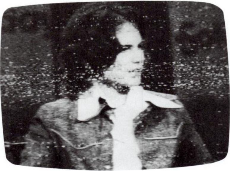
Fig. 2 Horizontal, white "shot lines" on tv screen and the staccato buzz in the radio receiver offer clues to spark discharge interference.
