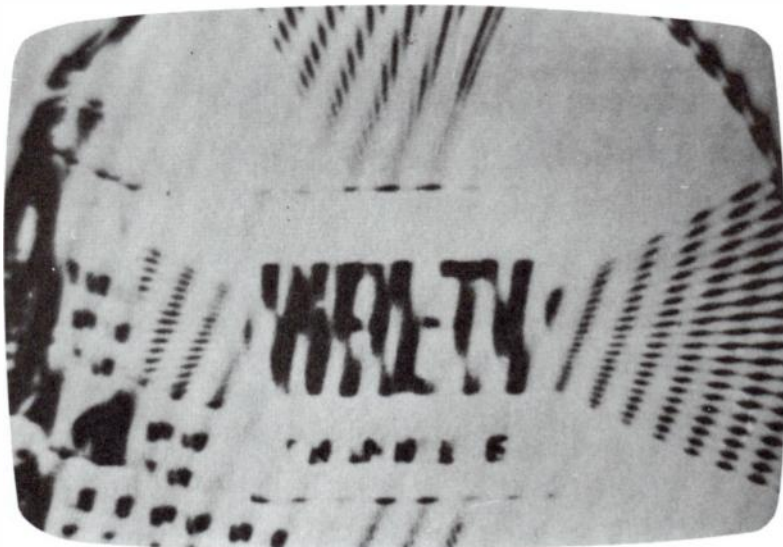
Fig. 8 Picture interference caused by local oscillator of a nearby fm receiver. Interference comes and goes as listener changes stations. Fm trap or antenna stub on the fm receiver will help cure the problem.
