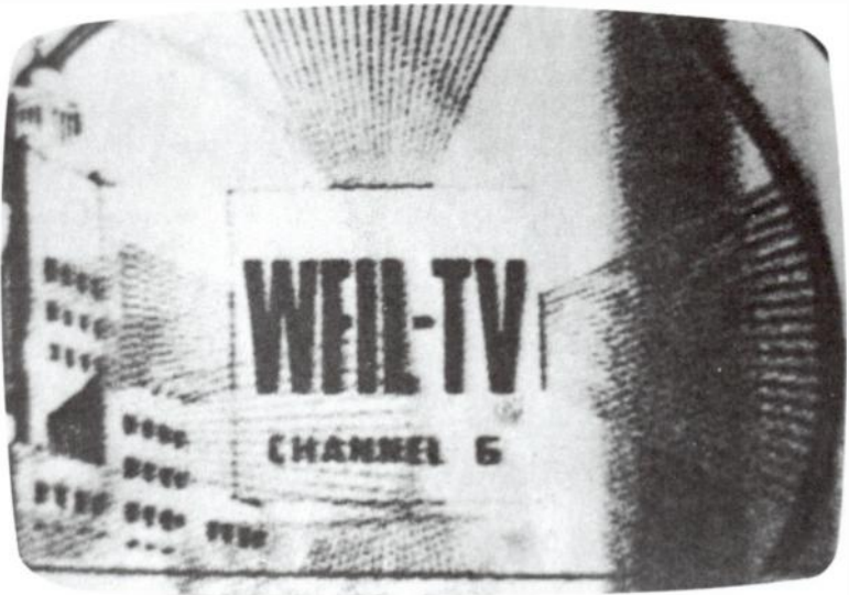
Fig. 4 Cross modulation effect from adjacent-channel strong signal results in unwanted picture seen along with desired channel picture.
