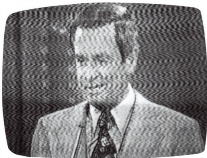
Fig. 14 The interference pattern created by internal circuits of the receiver. Elimination requires replacement of defective component in the retrace circuit by a competent serviceman.
