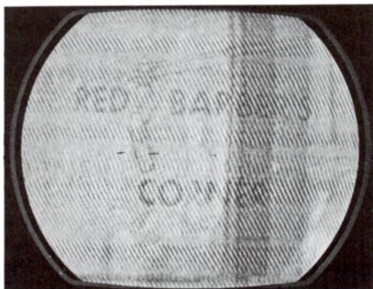
Fig. 6 Adjacent channel interference is common when signals from two different cities are received near midpoint between them. New Jersey viewers receive this interference from transmitters in New York and Philadelphia.
