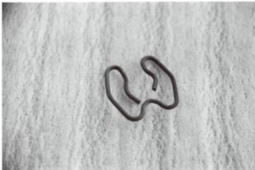
Fig. 14 (top) RIV clip is made of stainless steel and locks around the hardware in a bell insulator. Fig. 15 (bottom) Improved stainless steel RIV clip corrects and eliminates RFI when properly installed.
