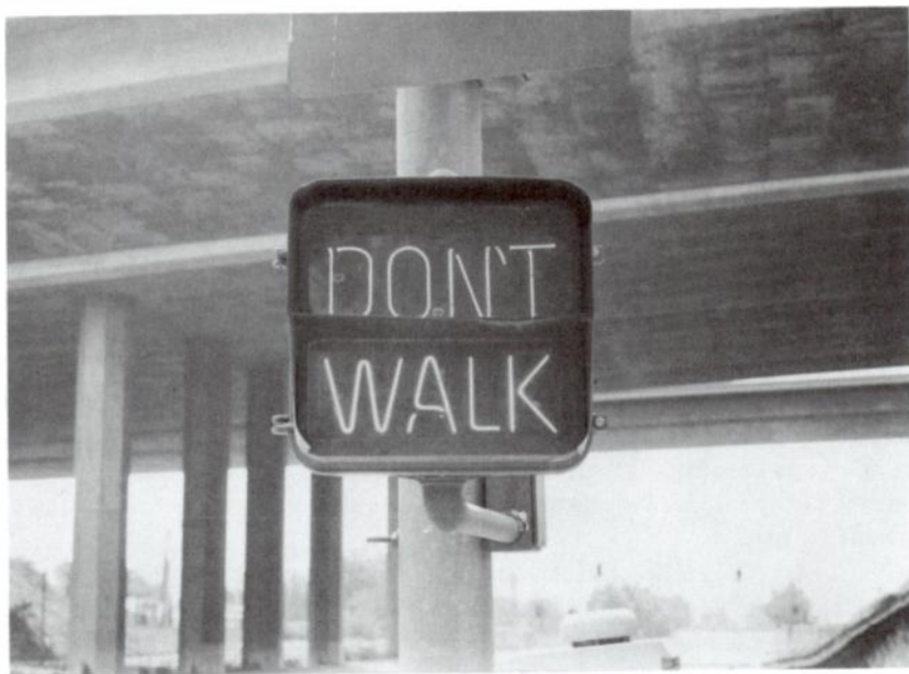
Fig. 9 Modern neon sign has built-in RFI suppression circuits. Older signs create severe interference and a sign company should be contacted for repair or maintenance of the offending device. Rf filters are available, but they should be installed by one familiar with the operation of the sign.
