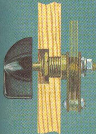
HOW THE CAPACITOR IS MOUNTED THROUGH THE BOARD
