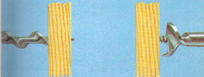
With a  $\frac{3}{8}$ " bit, drill from the marked side until the point of the bit just appears on the other side. (Do not drill right through)
