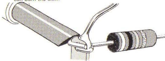
4) *Lightly push the end of the solder onto the joint and allow the solder to flow freely over the whole joint. DO NOT apply the solder to the bit, the heat of the joint should do the melting.*
