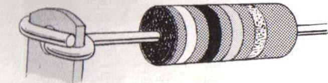
2) *Join the wire to the tag to make a firm joint that will not move*
