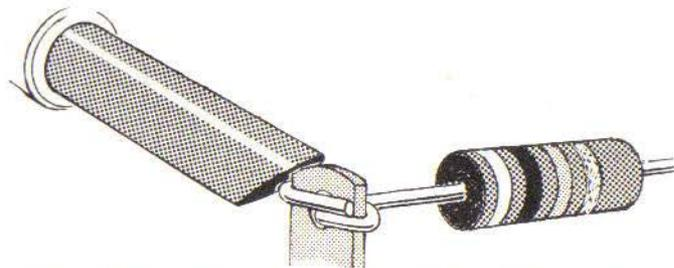
3) *Put the hot bit of the iron firmly upon the joint and allow a few seconds for the joint to heat up. Take care. The soldering iron bit and metal shaft can burn the skin!*
