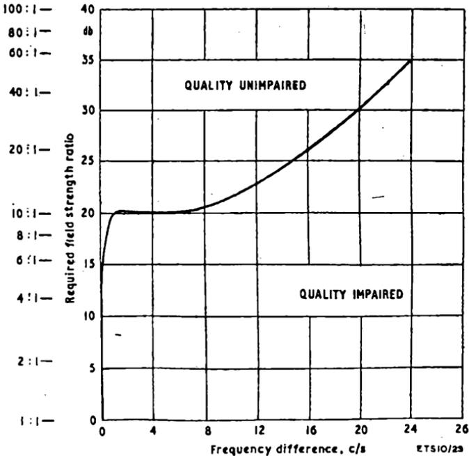
Fig. 14. Relationship between the frequency difference of two signals and the ratio of their field strengths required for good reception
