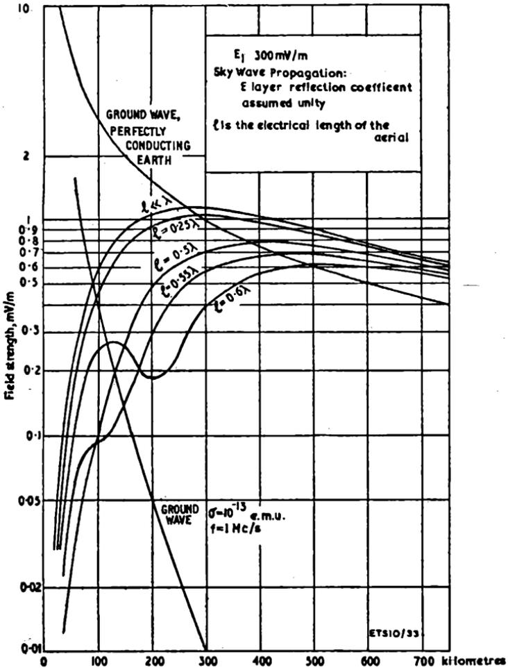
Fig. 21. Sky-wave field strengths plotted against distance for various heights of aerial average value of 0.25, the intersection shows the range where the strengths of the received signals have a ground-wave : sky-wave average ratio of 4 : 1. This range is usually accepted as the fade-free range of the transmission. In the example shown a transmission would have the following range:
