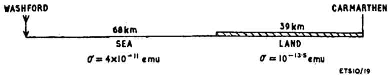
Fig. 12. Mixed-path propagation example. Washford to Carmarthen
