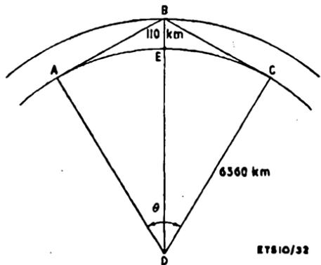
Fig. 22. Diagram showing path of reflected signal for maximum range via E-region reflection
