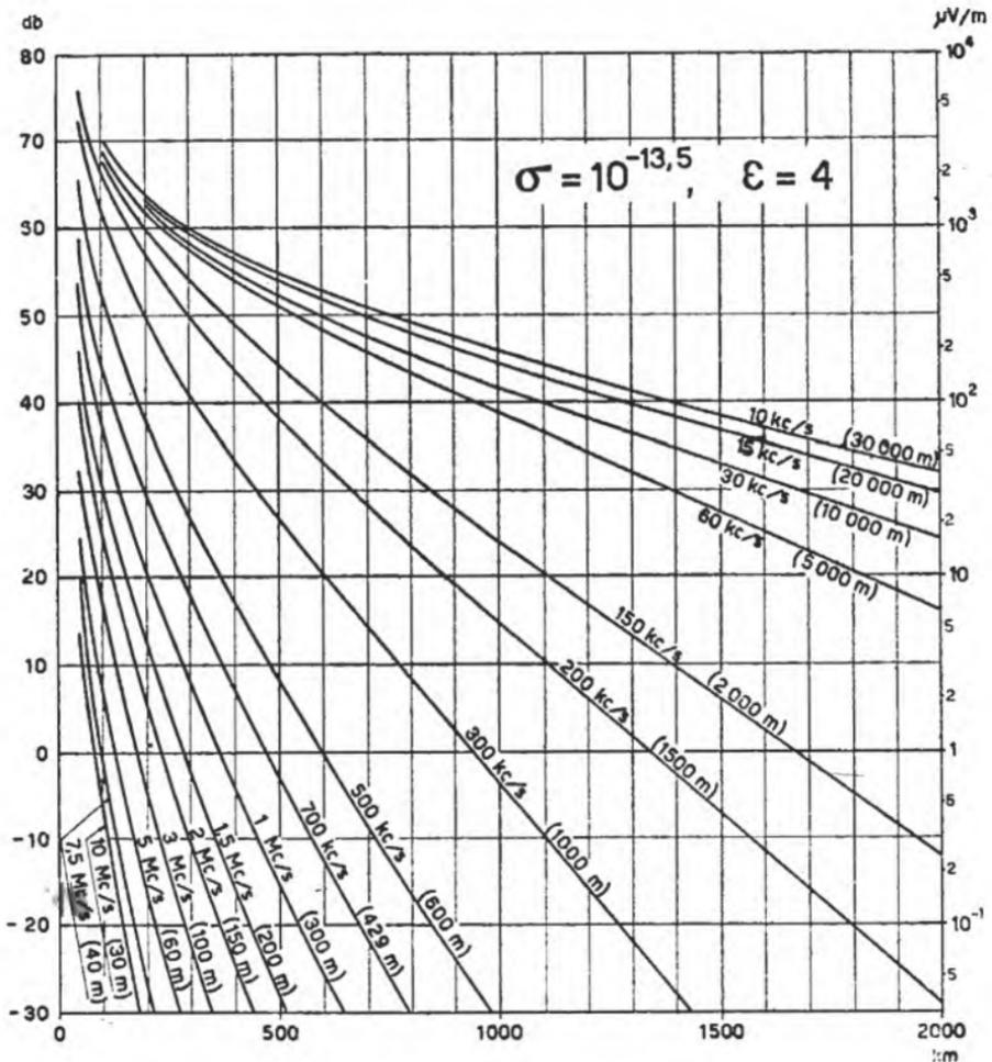
Fig. 9. Propagation over land of moderate conductivity (conductivity  $\sigma = 10^{-13.5}$  e.m.u., dielectric constant  $\epsilon = 4$  e.s.u.) over long distances.  $E_1 = 300$  mV/m
