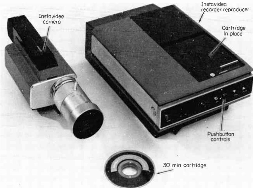
Fig. 12-20 Ampex Instavideo system. (Ampex Corporation.)
