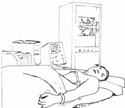
A complete EKG system can be seen here. Note the electrodes picking up the heart potentials which are then amplified and fed to the storage system and visual readout devices.
