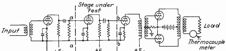
FIG. 102.—Arrangement for testing performance of single stage of multistage amplifier.
