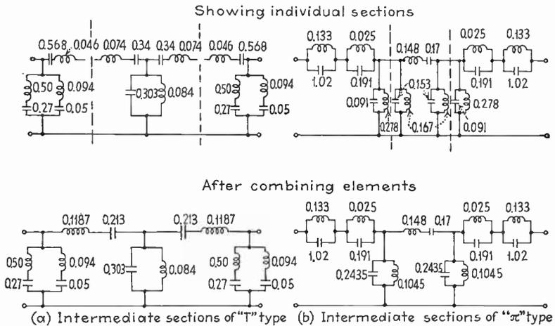
Fig. 197.—Example of a band-pass filter having cut-off frequencies of 500 and 2000 cycles, one intermediate section, and proportioned to operate with a load resistance of 700 ohms.
