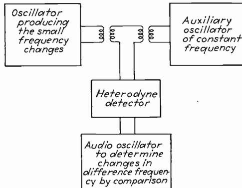
FIG. 82.—Schematic diagram illustrating how small change in frequency may be accurately measured.
