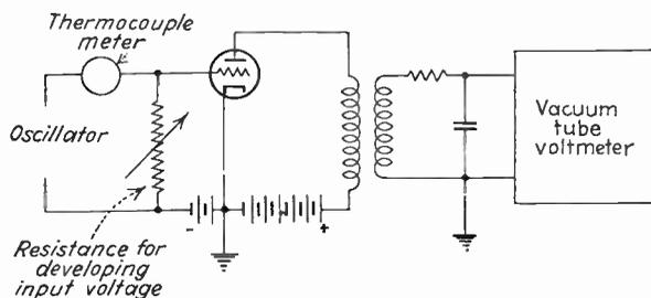
FIG. 206.—Measurement of the characteristics of tuned amplifiers.
