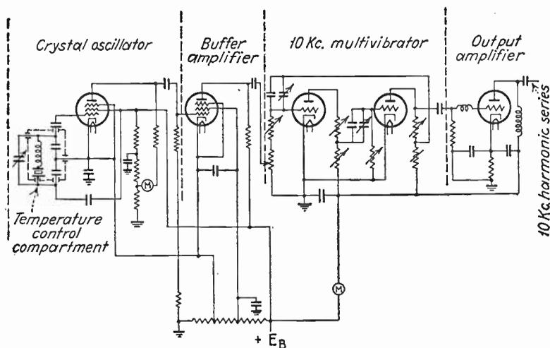
Fig. 73.—Schematic circuit diagram of secondary frequency standard.
