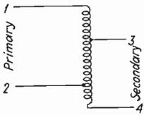
Fig. 37.—Auto-transformer coupling.
