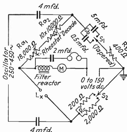
FIG. 39.—Hay bridge arranged to measure incremental inductance.
