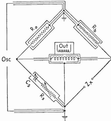
FIG. 56.—Typical completely shielded radio-frequency bridge.
