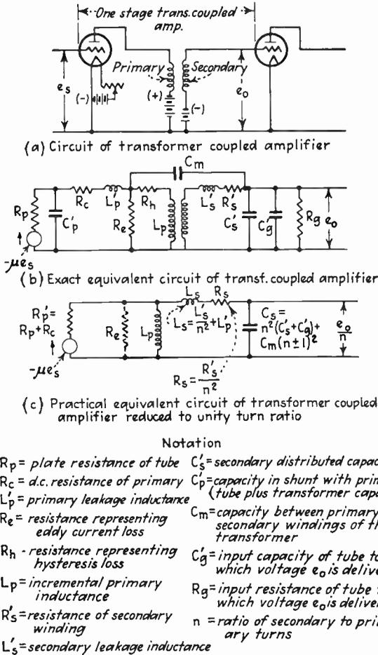
FIG. 112.—Actual circuit of a transformer-coupled amplifier, together with exact and approximate equivalent circuits.
