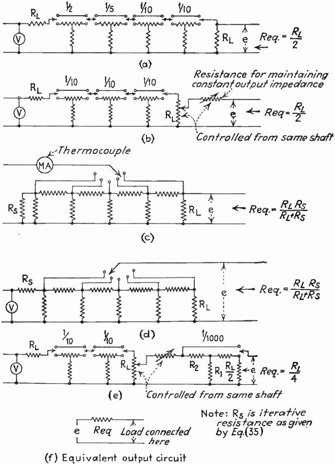
FIG. 104.—Attenuator systems for producing known audio-frequency voltages.
