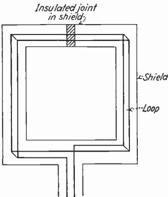
FIG. 139.—Electrostatically shielded loop antenna.
