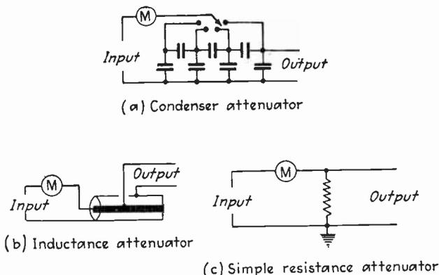
FIG. 123.—Miscellaneous types of attenuators.
