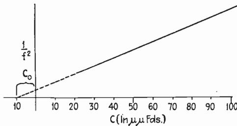
FIG. 48.—Plot of  $1/f^2$ , where  $f$  is the resulting resonant frequency, as a function of external tuning capacity. The value of negative capacity  $C_0$  at which the extrapolated line intercepts the capacity axis is the distributed capacity of the coil, and the slope of the line is a measure of the coil inductance.
