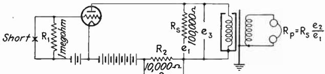
(b) Complete Circuit for Measuring Plate Resistance
