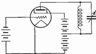
FIG. 150.—Circuit of simple dynatron oscillator.
