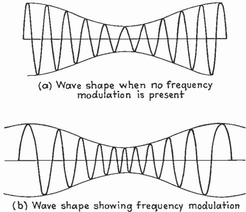
FIG. 132.—Beat notes obtained when carrier has (a) no frequency modulation, and (b) considerable frequency modulation.
