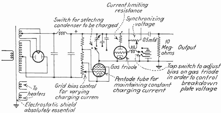
FIG. 170.—Saw-tooth oscillator circuit operating from 60-cycle power.
