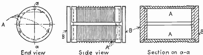
FIG. 66.—A coil having zero temperature coefficient of inductance. The material *A* controlling the expansion in an axial direction has a different coefficient of expansion from the material *B* controlling the coefficient of expansion in a radial direction, and the two can be so related that the resultant coefficient for inductance is zero.
