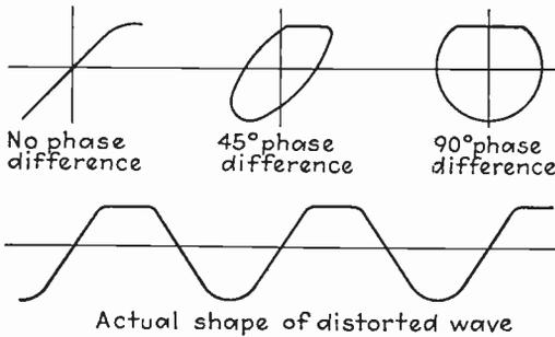
FIG. 173.—Typical patterns produced by cathode-ray tube when a sinusoidal deflecting force acts along the horizontal axis and a distorted sinusoidal force of the same frequency acts along the vertical axis, together with oscillograms of distorted wave plotted on a linear time axis.
