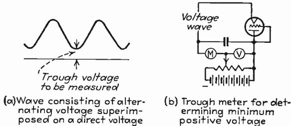
Fig. 19.—Trough meter for reading trough of a pulsating positive wave. Note that the battery polarity has been reversed from that in Fig. 18c.
