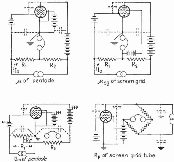
FIG. 96.—Methods of applying the bridge circuits of Fig. 95 to the determination of pentode and screen-grid tube coefficients.
