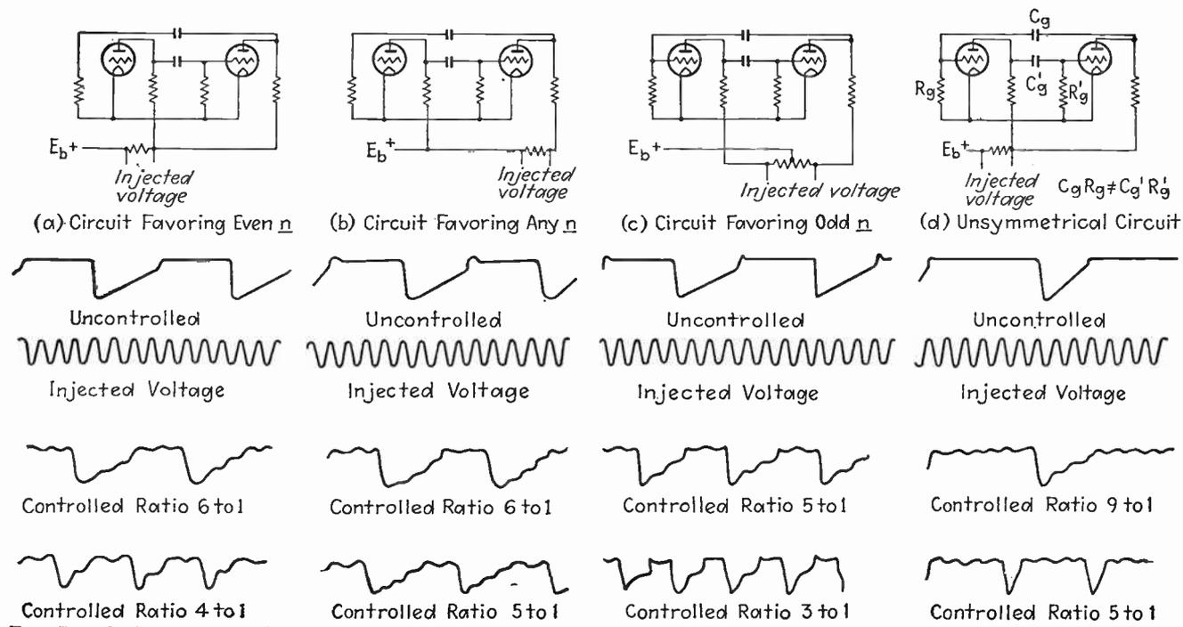
FIG. 79.—Oscillograms showing the mechanism whereby an injected voltage is able to control the frequency of the multivibrator oscillations.
