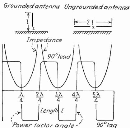
FIG. 144.—Antenna impedance and power-factor angle as a function of antenna length in wave lengths.
