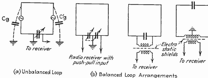
Fig. 138.—Unbalanced and balanced loop arrangements.
