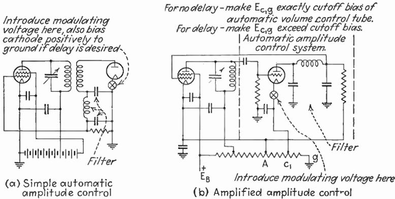
FIG. 151.—Dynatron oscillators provided with automatic amplitude control.
