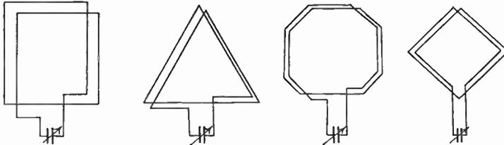
FIG. 135.—Examples of typical loop antennas.
