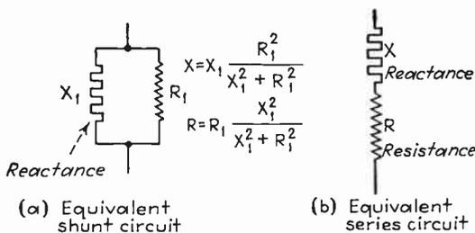
FIG. 47.—Methods of representing the impedance of a radio-frequency choke coil.
