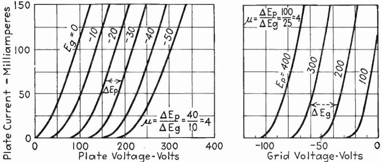
FIG. 90.—Evaluation of triode amplification factor using small but finite increments obtained from curves of tube characteristics. In each case one increment is the potential difference between adjacent curves while the other increment is scaled off as shown.
