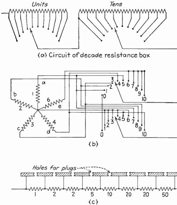
FIG. 60.—Switching arrangements for resistance boxes.
