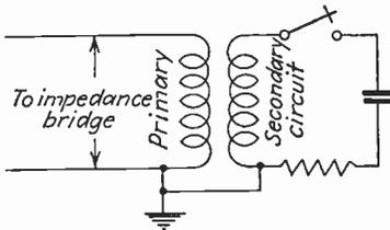
FIG. 200.—Circuit for measuring coupled impedance.
