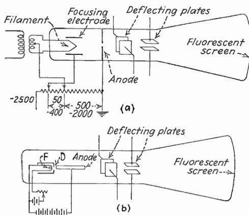
FIG. 161.—Medium- and low-voltage gas-filled type cathode-ray tubes.
