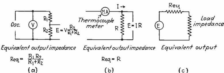
FIG. 103.—Simple methods of producing known voltages, together with equivalent output circuit for calculating reduction in voltage produced by a load.
