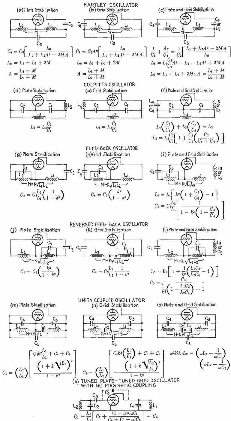
FIG. 155.—Circuits and circuit proportions that will make the generated frequency independent of the tube constants, provided the Q of the resonant circuit is very high (theoretically infinite).
