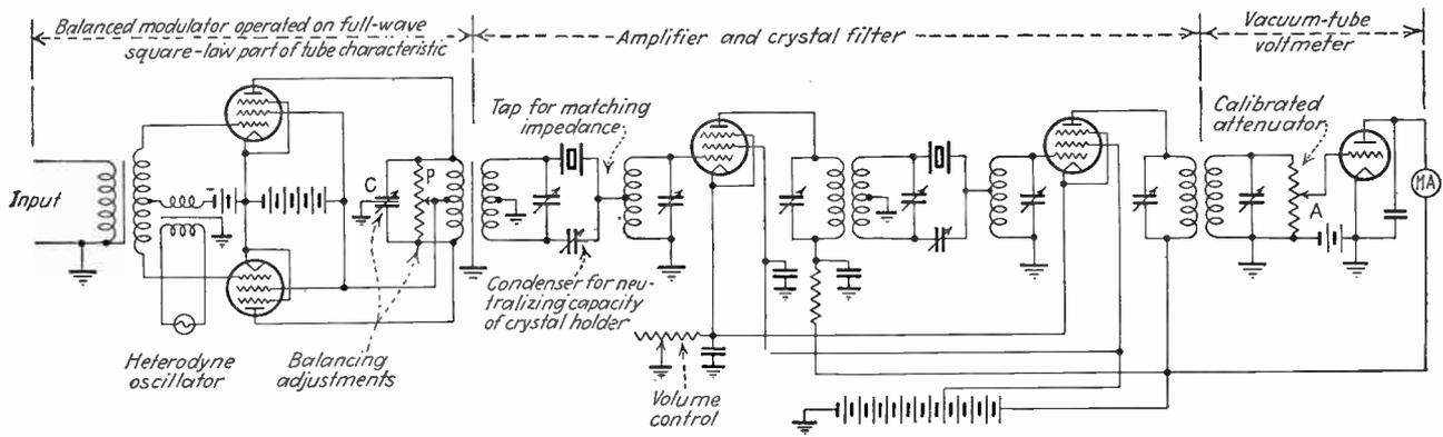
FIG. 87.—Circuit diagram of typical heterodyne type of wave analyzer.
