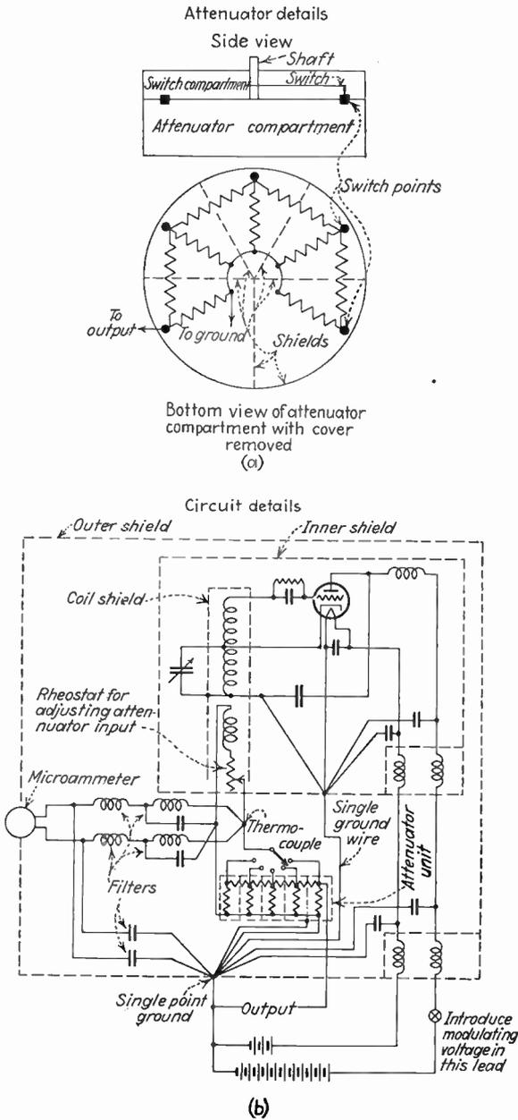
FIG. 120.—Signal generator of the resistance attenuator type.
