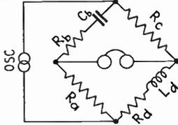
$$L_d = \frac{R_a R_c C_b}{1 + (R_b \omega C_b)^2}$$
