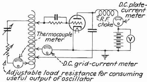
FIG. 209.—Circuit for studying vacuum-tube oscillator.
