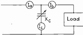
FIG. 23.—Three-ammeter shunt-reactance method of measuring power.
