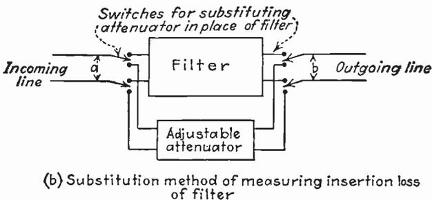
Fig. 107.—Typical circuit arrangements for measuring power gain and loss by the substitution method.
