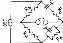
$$\omega^2 = \frac{1}{R_d R_c C_d C_c} \text{ and } \frac{C_d}{C_c} = \frac{R_b}{R_a} \frac{R_c}{R_d}$$
