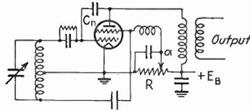
(a) Neutralized electron-coupled oscillator
