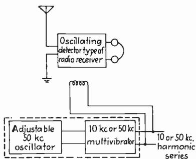
FIG. 75.—Schematic diagram of equipment for utilizing the Bureau of Standards 5000-kc standard-frequency transmissions. The multivibrator is provided with a switch that will change its fundamental frequency from 10 to 50 kc.
