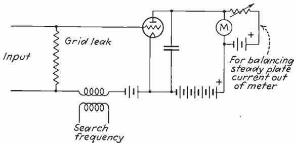
FIG. 85.—Vacuum-tube voltmeter method of analyzing wave forms. If desired, a shielded input transformer may be used to couple the wave being measured to the vacuum-tube voltmeter.
