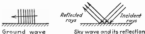
FIG. 141.—Character of ground wave, showing forward tilt of wave front, and also the reflection at the earth's surface of a sky wave. In the latter case the actual field is the resultant of the incident and reflected waves.
