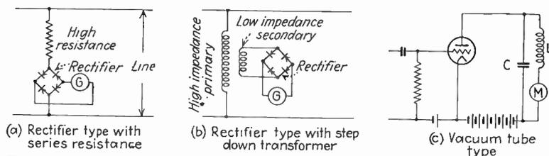
FIG. 26.—Various types of volume-level indicators for monitoring power level in voice-frequency circuits.
