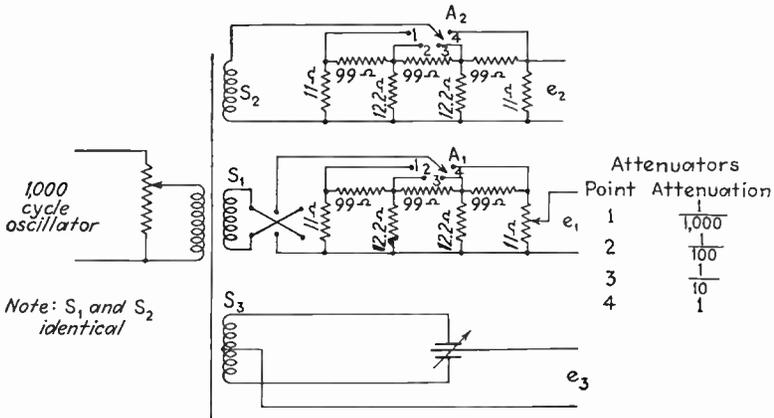
(a) Circuit for Production of Voltages  $e_1$ ,  $e_2$ , and  $e_3$
