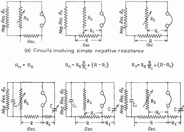
Fig. 53.—Bridge circuits for measuring negative resistance.
