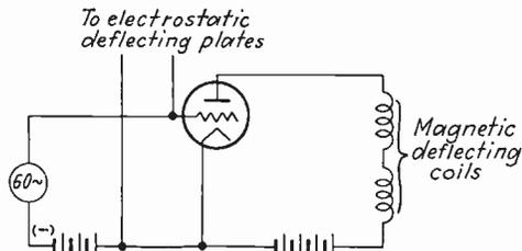
FIG. 180.—Circuit arrangement for obtaining  $E_g - I_p$  curve of triode with a cathode-ray tube.
