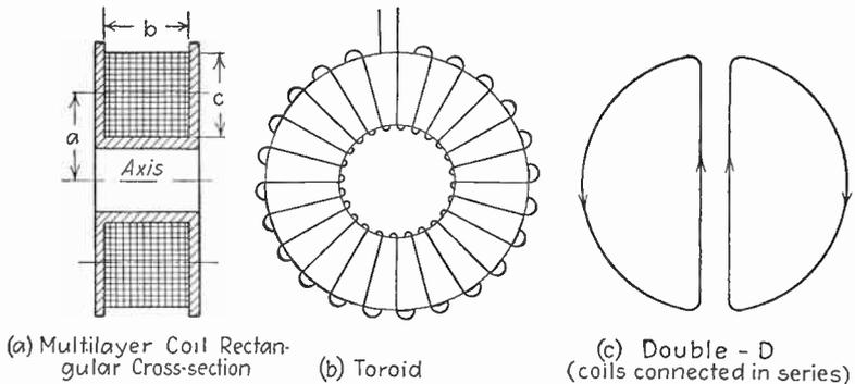
FIG. 65.—Methods used to wind inductance standards for audio frequencies.
