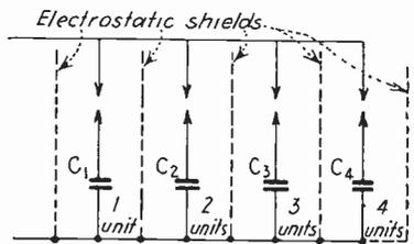
FIG. 70.—Switching arrangement for decade condenser. This requires a four-gang 11-position switch so wired up that the necessary condensers are connected across the circuit for the various switch positions. The electrostatic shields shown are necessary if the upper sides of the condensers and the associated wiring are not spaced so as to have negligible direct capacities to introduce errors.
