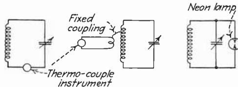
FIG. 74.—Methods of indicating when a wavemeter is tuned to resonance with the frequency being measured.
