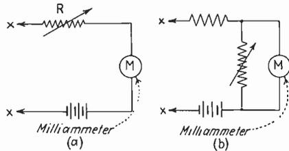
FIG. 31.—Ohmmeters used in servicing communication equipment.
