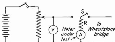
FIG. 3.—Convenient circuit arrangement for calibrating an ammeter or milliammeter  $A$  using a standard voltmeter  $V$ .
