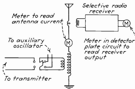
FIG. 89.—Diagram illustrating the measurement of harmonics in the antenna circuit by the substitution method.
