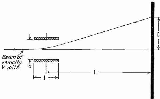
FIG. 162.—Deflection of electron beam by electrostatic fields.
