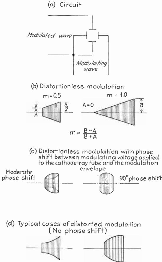
FIG. 178.—Circuit arrangement for observing modulation, together with typical resulting patterns.
