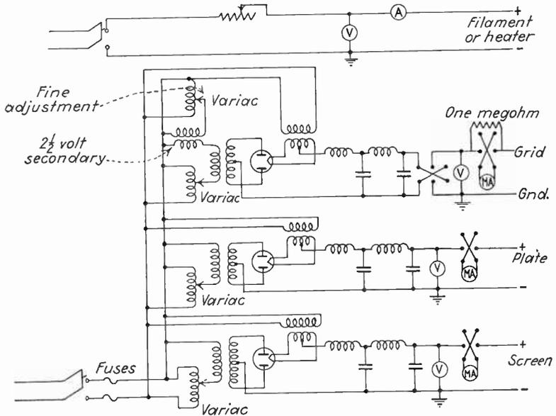
Note:- Each voltage and current instrument provided with a series of multipliers or shunts controlled by a tap switch
