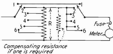
FIG. 5.—Multiplying network for rectifier milliammeter that follows a common scale for different ranges. The two switches shown are operated from a common shaft.
