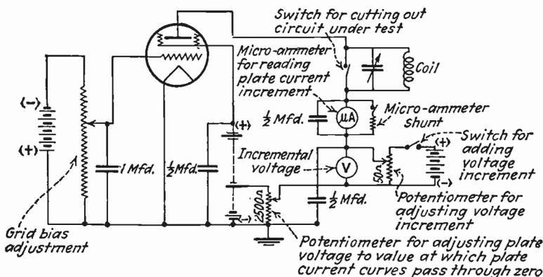
FIG. 52.—Circuit connections for measuring the parallel-resonant impedance of a tuned circuit by the resistance-neutralization method, including means for measuring the negative resistance by the incremental method.
