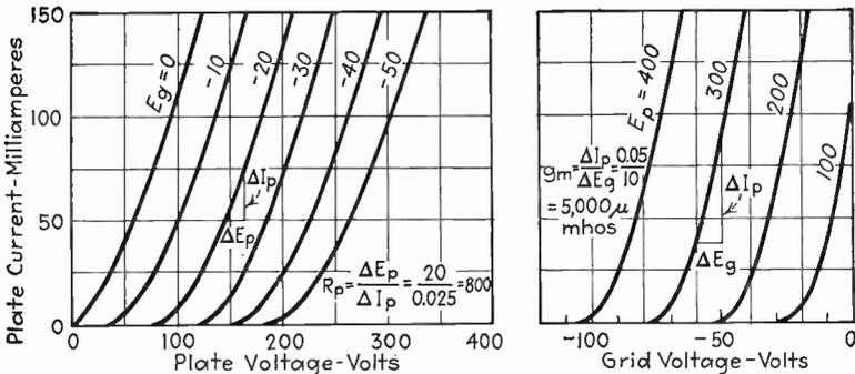
FIG. 91.—Evaluation of triode plate resistance from curves of tube characteristics. Plate resistance is by definition the reciprocal of the slope of the  $E_p - I_p$  curve for constant grid bias  $E_g$ .
