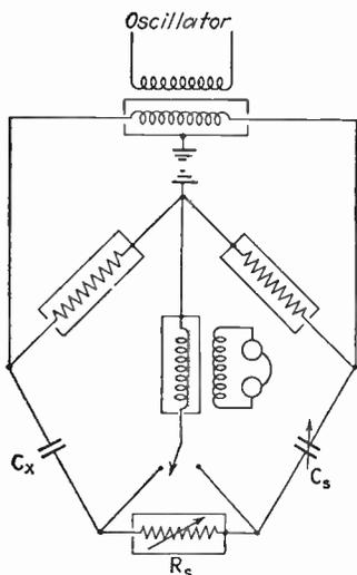
FIG. 42.—Shielded capacity bridge. The entire bridge is inclosed in a copper-lined box that serves as the ground.
