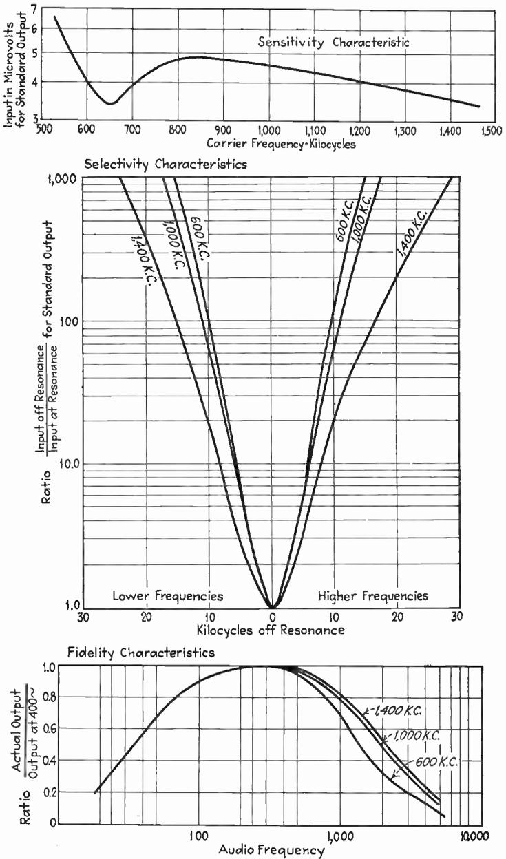
Fig. 115.—Sensitivity, selectivity, and fidelity characteristics of a broadcast receiver having manual volume control.
