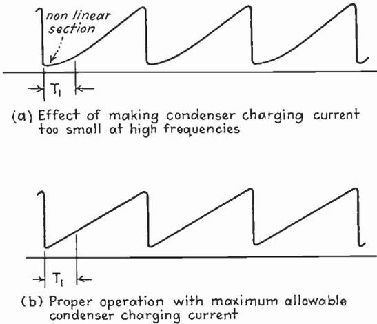
FIG. 169.—Effect of different condenser charging currents when generating high-frequency oscillations. A small charging current makes the wave curved during the deionization period  $T_1$ , thereby reducing the useful (*i.e.*, linear) part of the oscillation.
