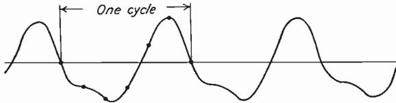
FIG. 84.—Arbitrary curve with six equally spaced ordinates. A six-point schedule will give a curve that will pass through the six selected points, and this calculated curve will or will not coincide with the actual curve between selected points according to whether or not the actual curve contains coefficients not evaluated by the six-point schedule.
