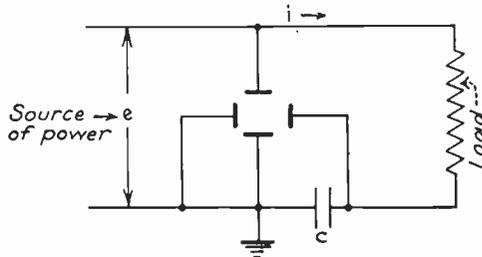
FIG. 174.—Cathode-ray tube connected to measure power dissipated in a load. The area of the pattern traced by the luminous spot is proportional to power, provided the losses in the condenser *C* are negligible.
