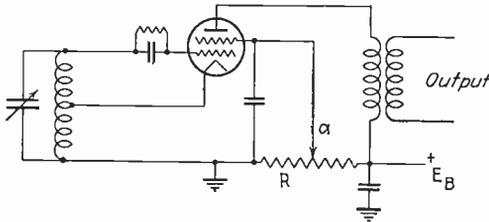
FIG. 153.—Typical electron-coupled oscillator circuit with grounded screen grid. The frequency can be made independent of plate voltage by connecting the screen-grid tap  $\alpha$  to proper point on the voltage-dividing resistance  $R$ .
