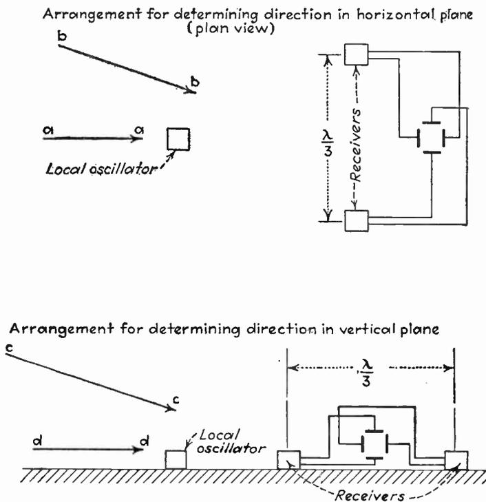
FIG. 184.—Method of using cathode-ray tube to determine direction of arrival of radio waves.
