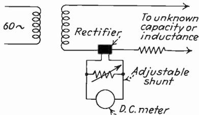
FIG. 46.—Simple type of capacity and inductance meter used in service work.
