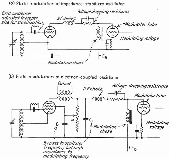
FIG. 156.—Plate modulation of electron-coupled and impedance-stabilized oscillators.
