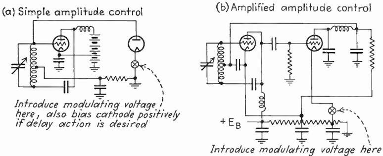
FIG. 152.—Conventional Hartley oscillator with automatic amplitude control.
