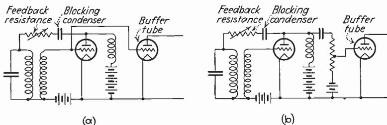
FIG. 148.—Methods of coupling a buffer tube to a resistance-stabilized oscillator.
