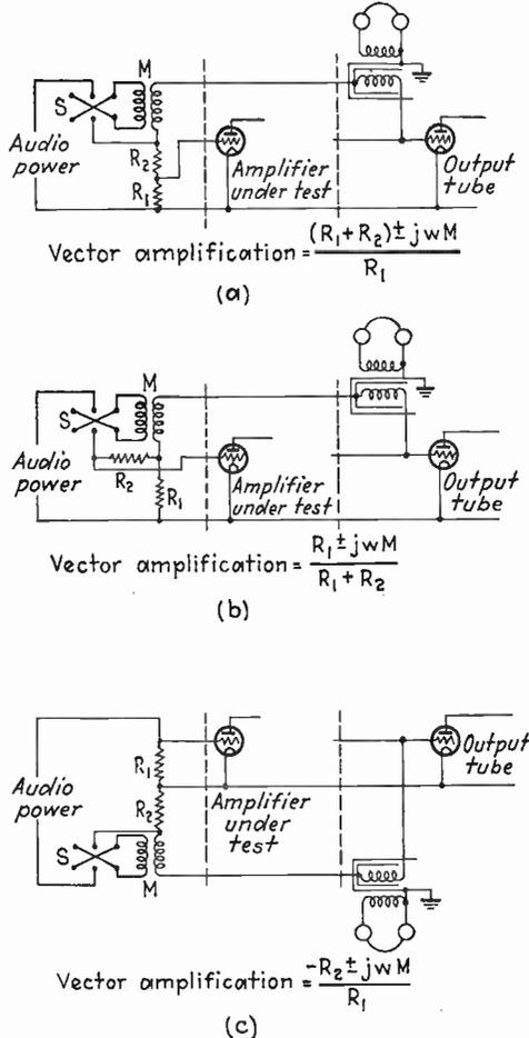
FIG. 105.—Circuits for determining phase shift in audio-frequency amplifiers. output as a function of frequency with respect to some arbitrary power. Thus if the output voltage varies with frequency as
