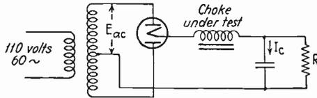
FIG. 40.—Circuit for approximate measurement of incremental inductance at high alternating flux densities.
