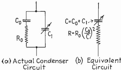
FIG. 69.—Actual and equivalent circuits of condenser with losses.
