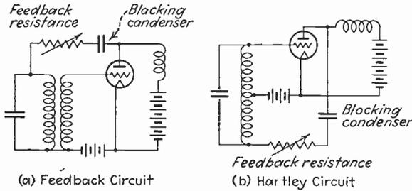
FIG. 147.—Typical oscillator circuits provided with resistance stabilization.
