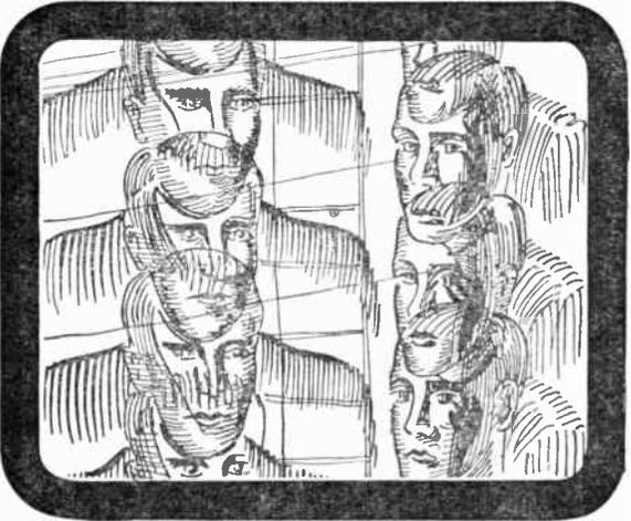
Fig. 110.—A sketch giving an impression of the effect obtained when the frame time base is slightly out of adjustment. This effect is impossible to photograph and difficult to draw accurately.
