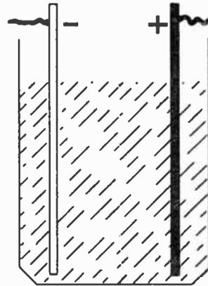
Fig. 23.—A simple cell consisting of a zinc plate (-) and a copper plate (+) partly immersed in a weak solution of sulphuric acid and water.
