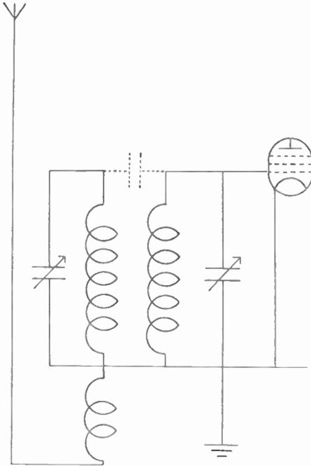
Fig. 113.—Aerial coupling which relies on over coupling between the two tuned circuits to obtain bandpass characteristics.
