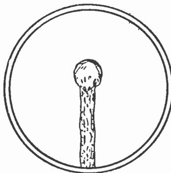
Fig. 37.—Sketch showing the appearance of a filament or heater that has been fused due to the application of excessive voltage. (Much enlarged.)
