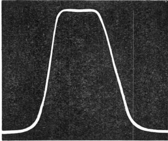
Fig. 130.—The combined high- and intermediate-frequency response-curve of a modern superheterodyne.
