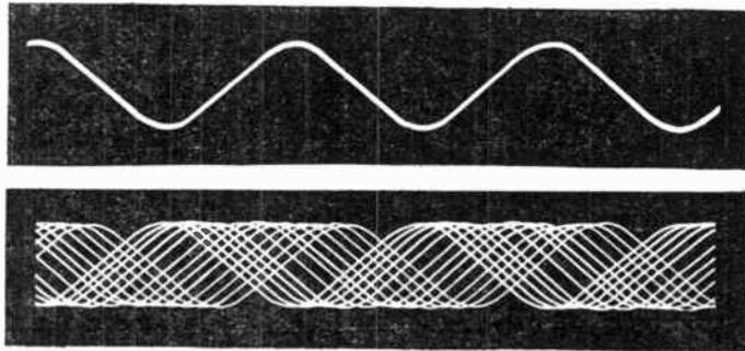
Fig. 16 (*top*).—A simple waveform, and Fig. 17 (*below*) an attempt to show the effect produced when the waveform being examined is not a multiple or sub-multiple of the time-base frequency. The effect thus produced will appear in a photograph like the complicated trace shown above, but with many types of tubes it will appear to the eye as though a single or perhaps a double trace is moving across the screen.
