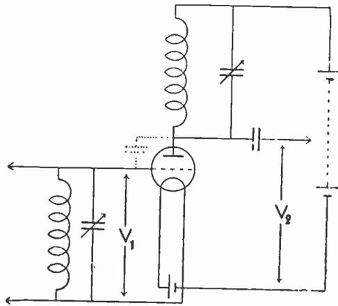
Fig. 86.—A skeleton circuit using a tuned circuit as input and output.
