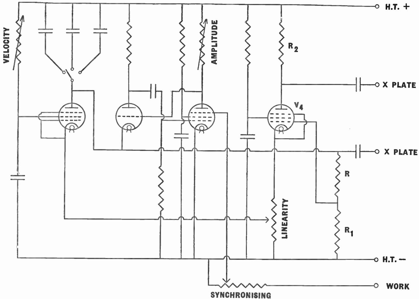
Fig. 20.—Complete circuit of a time base using high-vacuum valves, with an additional valve to give a balanced output and correct linearity.
