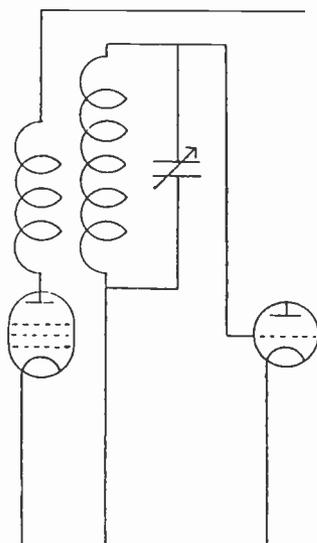
Fig. 117.—Tuned inter-valve transformer coupling.
