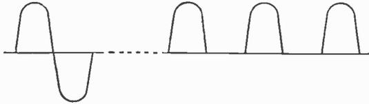
Fig. 76.—(Left) An alternating current waveform, and (Right) after rectification.
