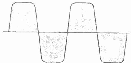
Fig. 57.—A waveform where the mean and peak values are nearly equal ; note the large tinted area.
