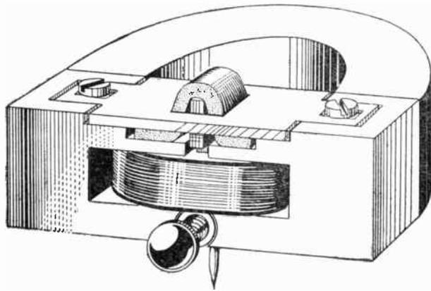
Fig. 21.—Movement of a simple gramophone pick-up shown to illustrate the principle (cover removed).
