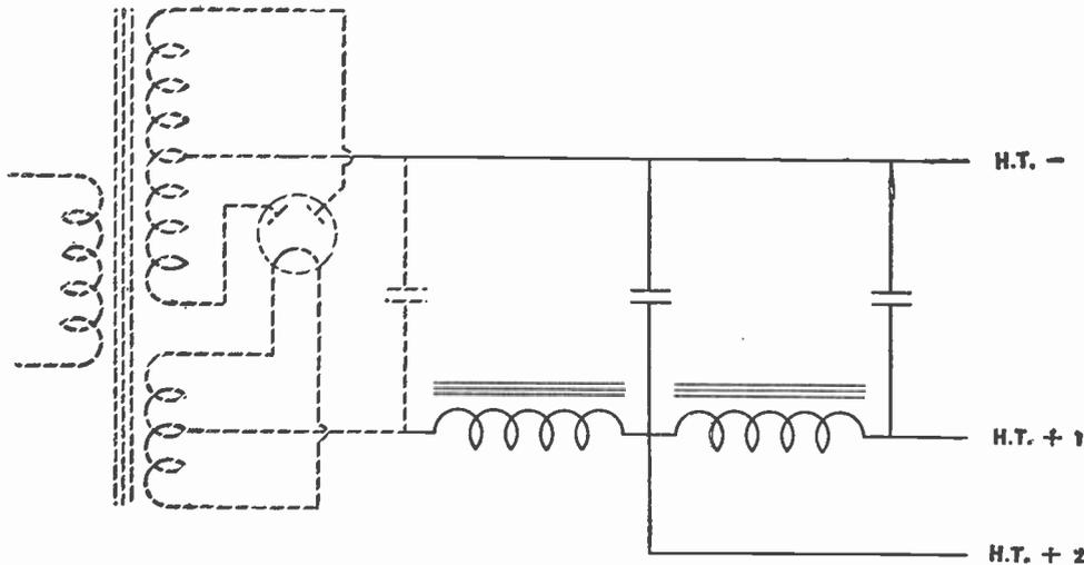
Fig. 14.—Two-stage mains filter arranged to give additional smoothing to the earlier stages of the receiver.
