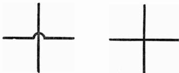
Fig. 80.—(left) Wires crossing, (right) a junction.
