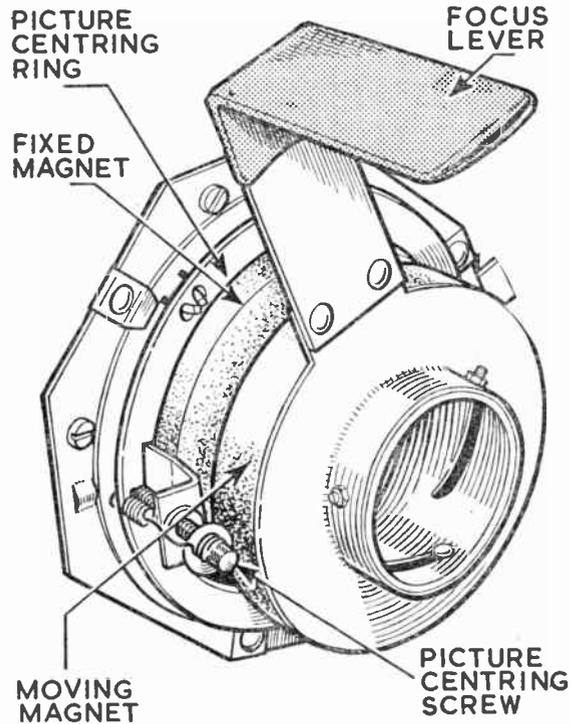
Fig. 74.—A ring magnet focusing assembly with picture shift plate and "screw" type focus lever.
