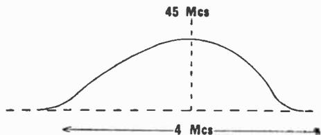
Fig. 101.—The type of response-curve to be expected from a vision receiver.
