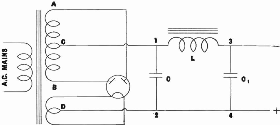
Fig. 2.—Basic circuit using a full-wave valve rectifier.
