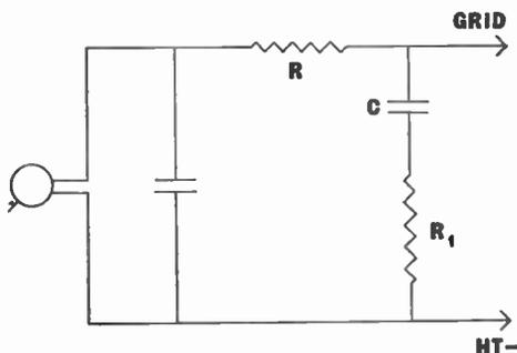
Fig. 26.—A bass-lift circuit for a 600-ohm pick-up; the parallel condenser may be  $.004 \mu\text{F.}$ ,  $R$ , 50,000 ohms,  $C$ ,  $.03 \mu\text{F.}$ , and  $R_1$  15,000 ohms.
