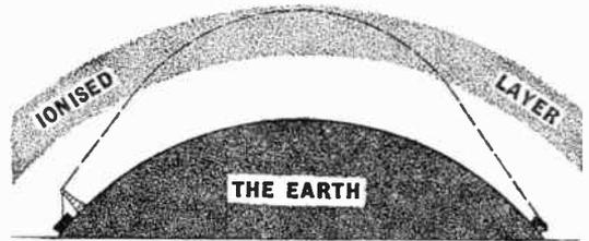
Fig. 15.—The sky wave propagated by the transmitter (left) is bent by an ionised layer many miles above the earth's surface and returns earthwards to impinge on the receiving aerial (right).
