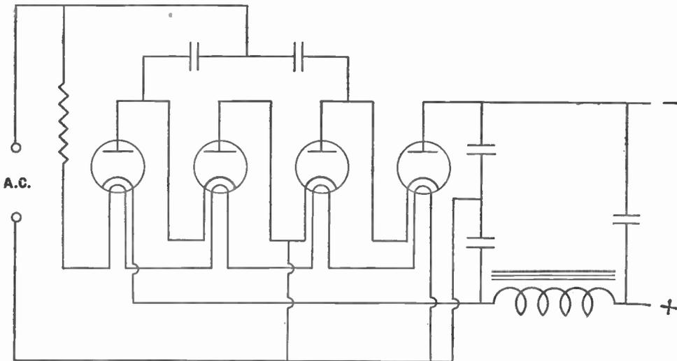
Fig. 13.—Voltage-quadrupling circuit arranged for direct connection to alternating-current supply.
