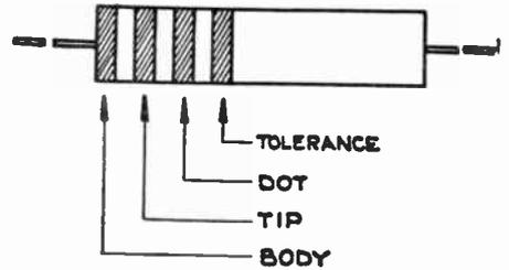
Fig. 84b.—The new modified colour code used for resistances with axial leads.
