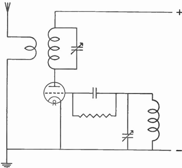
Fig. 49.—A simple oscillator loosely coupled to a single wire aerial.
