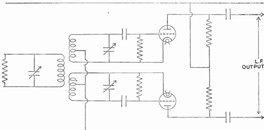
Fig. 206.—An interesting circuit which combines the functions of limiter and frequency-amplitude converter; using the super-regenerative principle this arrangement has very high stage gain.
