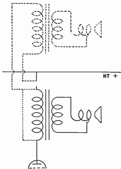
Fig. 29.—This diagram shows (dotted) the temporary connection of a loudspeaker as a means of checking the original speaker.
