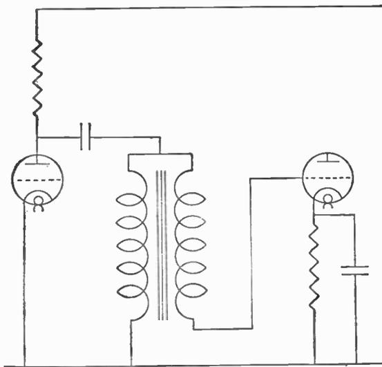
Fig. 152.—The circuit shown at Fig. 151 rearranged to give increased gain.
