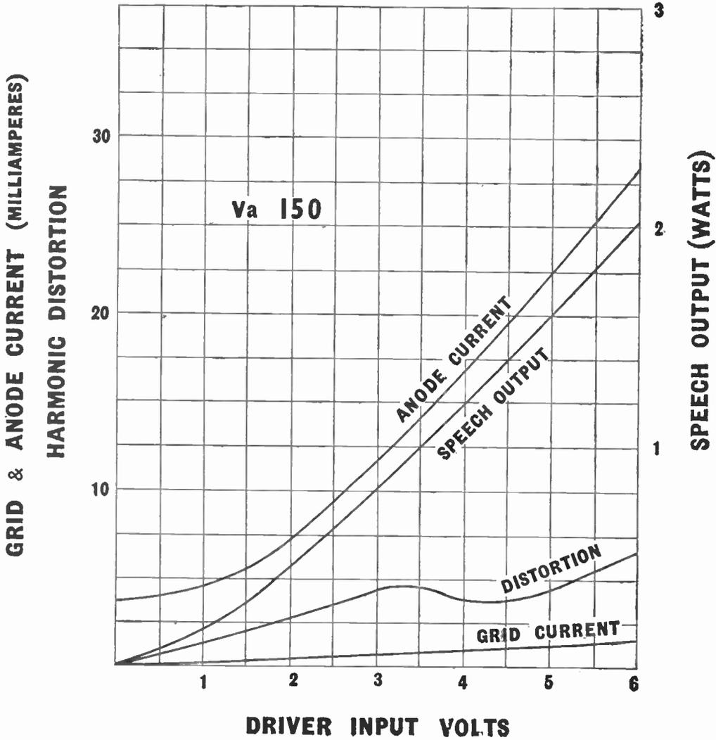
Fig. 168.—Performance curves of a Class B output stage. The curves show the combined performance of driver and output valves.
