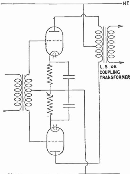
The simplest method of phase splitting, using an input transformer with centre-tapped secondary. Separate bias resistances are shown, but a common bias resistance can be used if desired.
