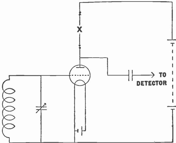
Fig. 104.—Basic circuit of a high-frequency amplifier using a triode valve.
