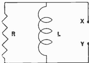
Fig. 61.—Resistance and inductance in parallel.
