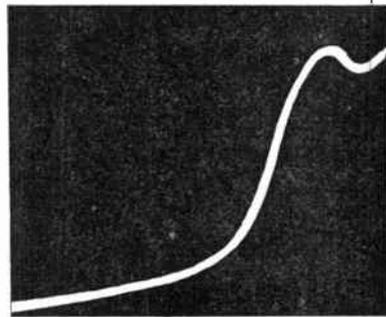
Fig. 47.—In this illustration the shape of the response-curve is probably correct but out of centre, due to the coils being adjusted to a few kilocycles off the correct frequency.
