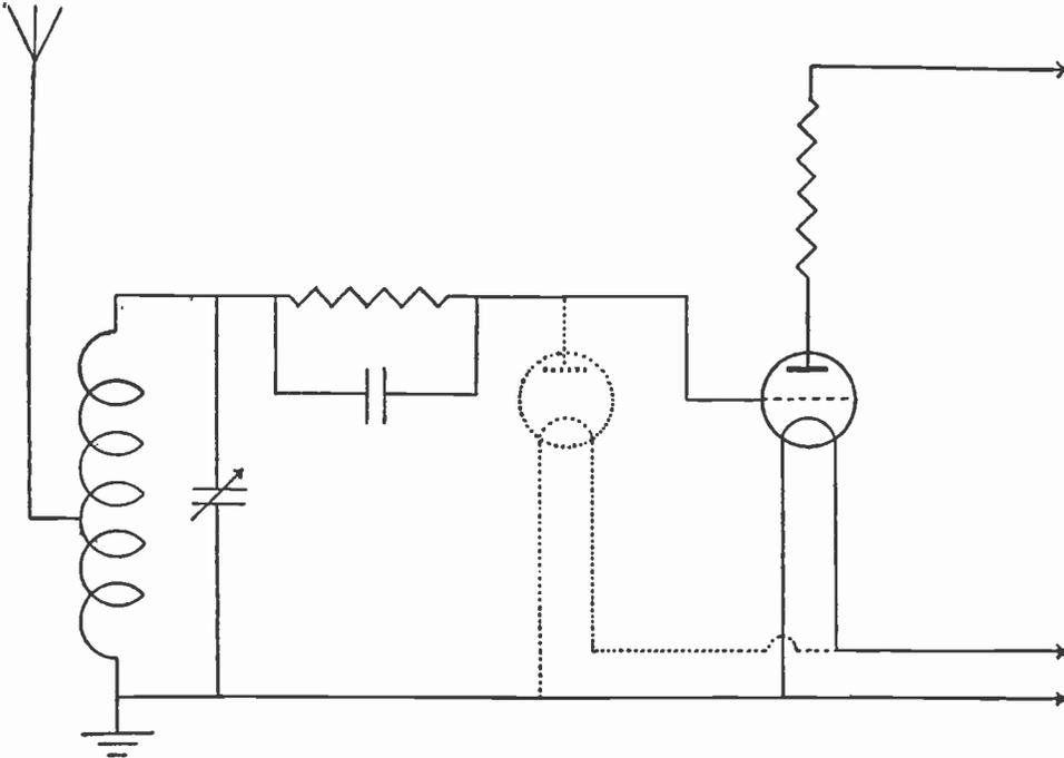
Fig. 97.—This circuit illustrates the function of a leaky grid detector.
