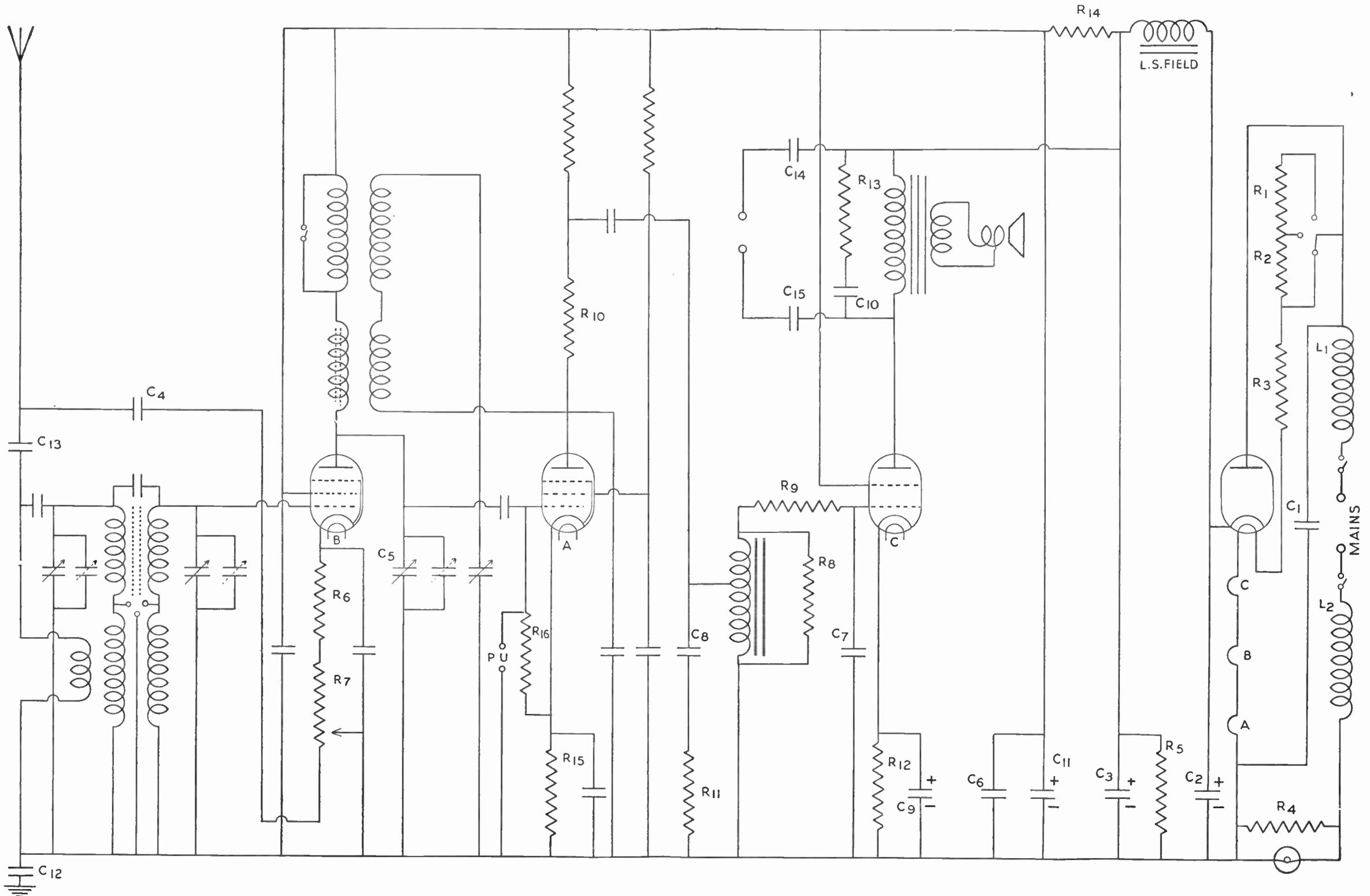
Circuit diagram of a three-valve (plus rectifier) A.C./D.C. receiver.
