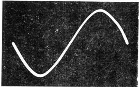
Fig. 55.—An oscillogram of a sine wave ; the illustration shows one complete cycle.
