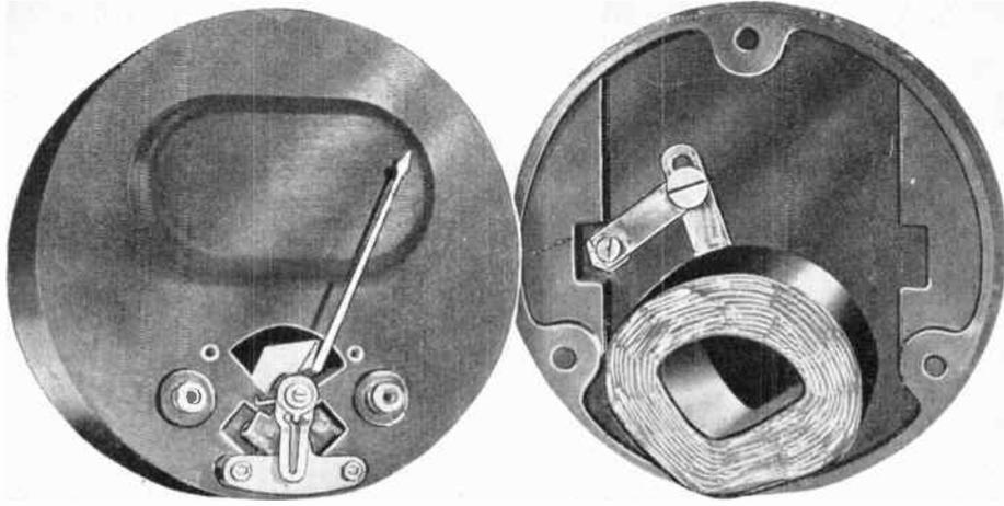
A typical moving-iron meter. (*Left*) Front of instrument, showing mechanism. (*Right*) Front view of rear portion, showing deflecting coil.
