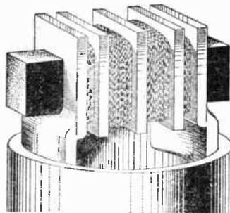
Fig. 69.—An example of a dust-iron-cored coil. The former is moulded from a special synthetic material having very low dielectric loss. The secondary has an inductance of  $185 \mu\text{H}$  with a high-frequency resistance of  $4.7 \Omega$  at 1,000 kilocycles.
