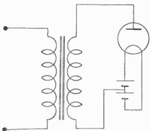
Fig. 75.—A simple circuit to illustrate the uni-directional properties of a diode.
