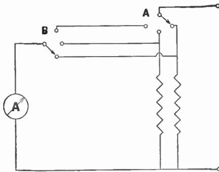
Fig. 8.—The correct method of switching shunts; the switch A is not included in the actual shunt circuit, being outside the point of connection between meter and shunt. The switch B is in series with the meter, which has relatively high resistance, and not in series with the shunts, which have relatively low resistance. The switches must be ganged.
