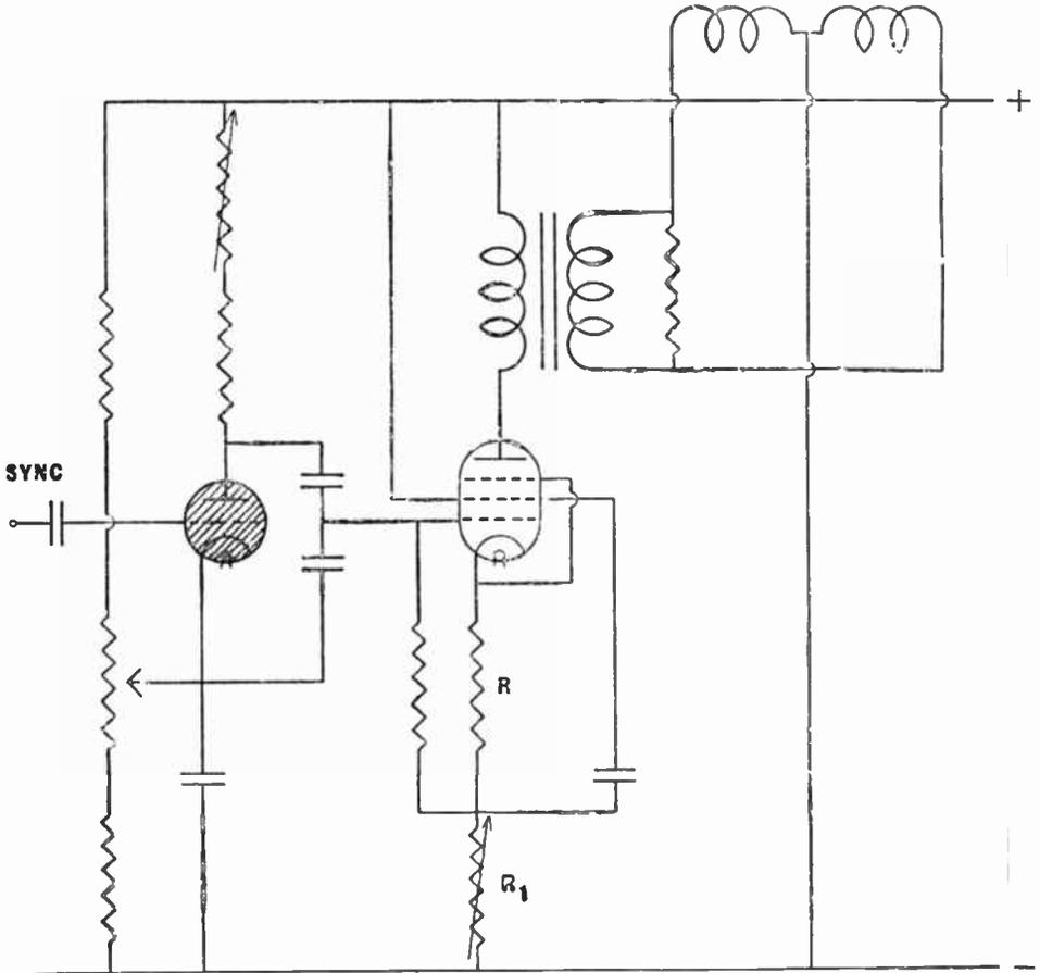
Fig. 93.—Another arrangement somewhat similar to Fig. 91, but employing the principle of cathode feed-back which is described in the text.
