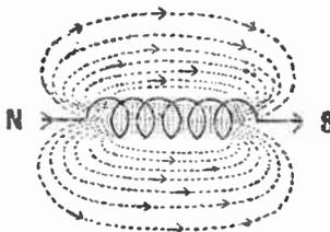
Fig. 40.—The field around a coil through which a current is flowing. The larger arrows indicate direction of conventional current.
