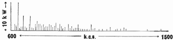
Fig. 128.—The number and power of European broadcasting stations working in 1928. Height of lines represent power, and position in the horizontal direction shows frequency.
