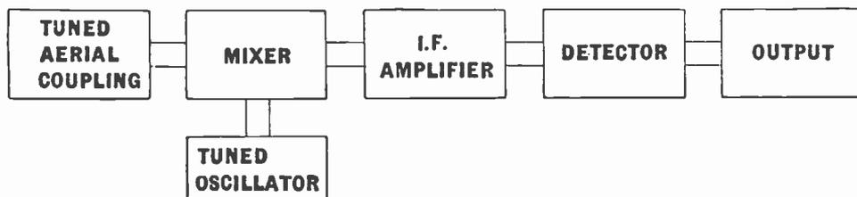
Fig. 118.—A block diagram showing the various sections of a superheterodyne receiver.
