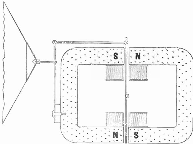
Fig. 170.—Section of a balanced armature loudspeaker.
