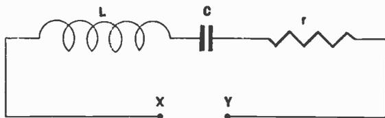
Fig. 64.—Inductance and capacity in series: the high-frequency resistance of the complete circuit is symbolised by a series resistance.
