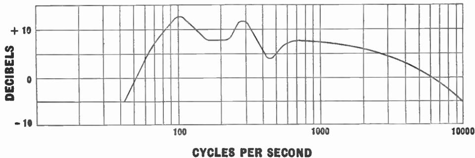
Fig. 27.—A purely imaginary response-curve, showing frequency distortion in the form of peaks and troughs as well as attenuation at both ends of the audio scale.
