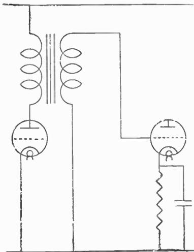
Fig. 149.—Transformer coupling with indirectly heated mains valves.
