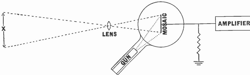
Fig. 96.—A diagrammatic illustration of the Iconoscope applied to television transmission.
