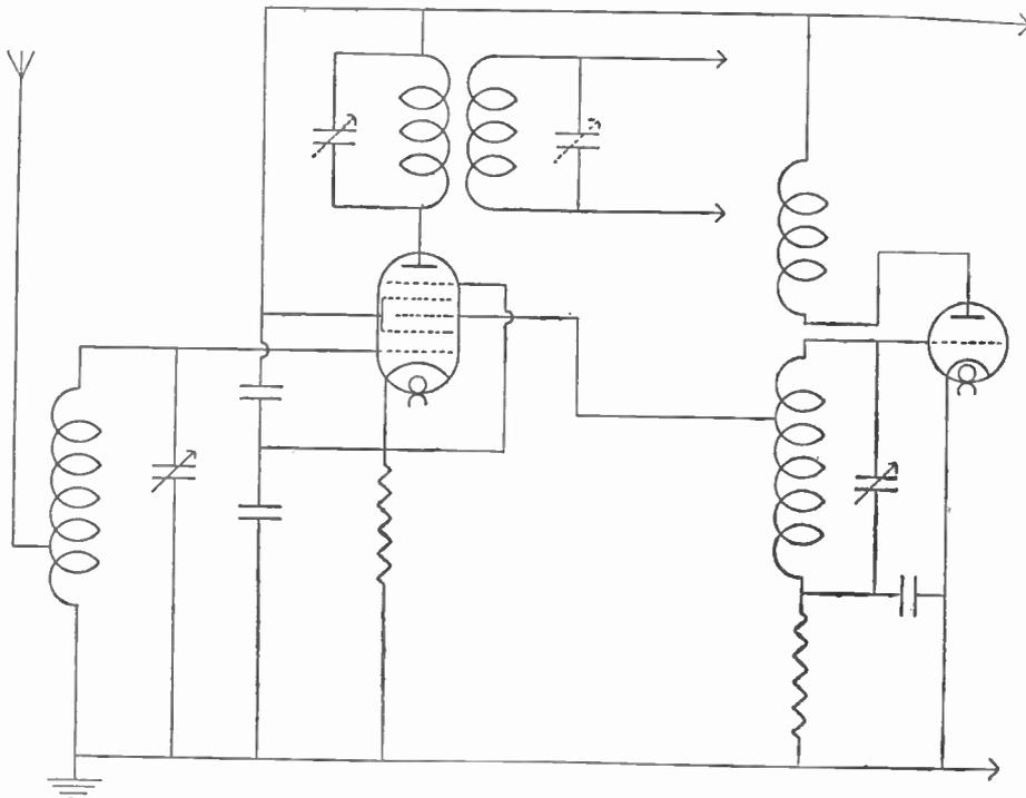
Fig. 123.—Basic circuit of a heptode mixer-valve with separate triode oscillator.
