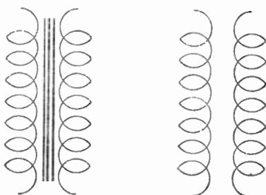
Fig. 46.—Left: the conventional symbol for an iron-core transformer. Right: the symbol for an air-core transformer.
