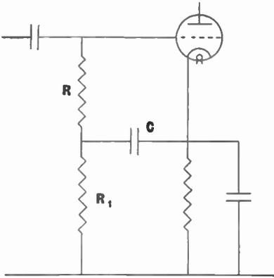
Fig. 18.—Grid decoupling.
