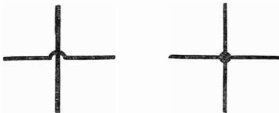
Fig. 81.—A slightly modified convention: (left) wires crossing, (right) a junction.
