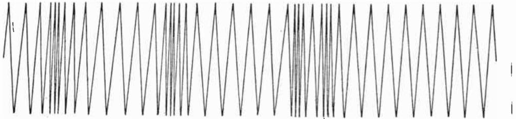
Fig. 200.—A diagrammatic representation of frequency modulation. (For ease in drawing and general clarity straight lines have been used instead of curved lines of sinusoidal character.)
