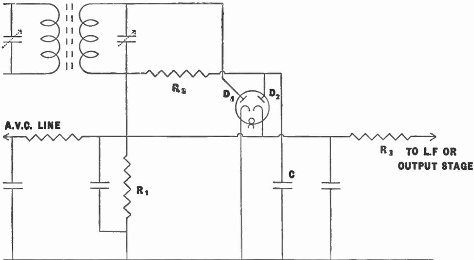
Fig. 40.—Typical static-suppression circuit.
