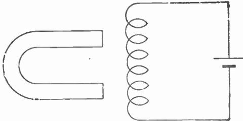
Fig. 43.—The energised coil and permanent magnet will attract or repel each other according to their relative polarity.
