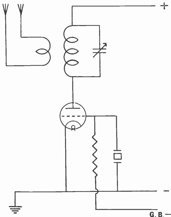
Fig. 54.—The basic arrangement of a crystal-controlled oscillator.
