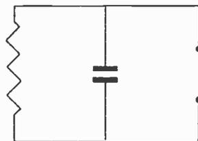
Fig. 62.—Resistance and capacity in parallel.
