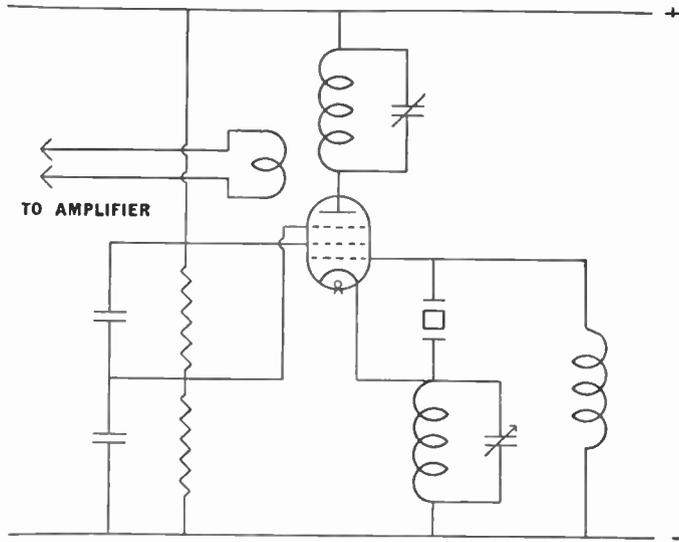
Fig. 64.—A pentode valve arranged as a combined oscillator and harmonic generator.
