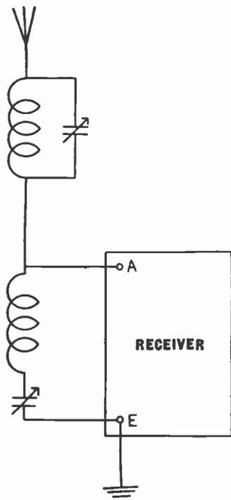
Fig. 50.—This illustration shows a rejector connected in the aerial lead aided by an acceptor circuit connected between the aerial and earth terminals of the receiver.
