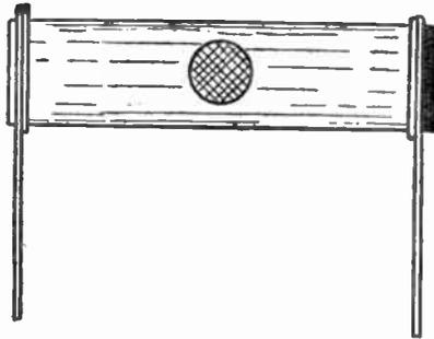
Fig. 84a.—The body colour denotes the first digit. The colour of the tip the second digit, and the colour of the spot the number of noughts.
