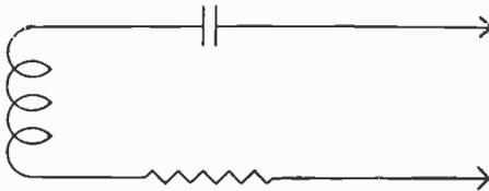
Fig. 86.—A standard dummy aerial circuit. The values are  $25\ \Omega$ ,  $20\ \mu\text{H}$ , and  $200\ \mu\mu\text{F}$ .
