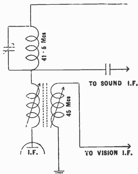
Fig. 100.—The separating stage of a combined vision and sound receiver.
