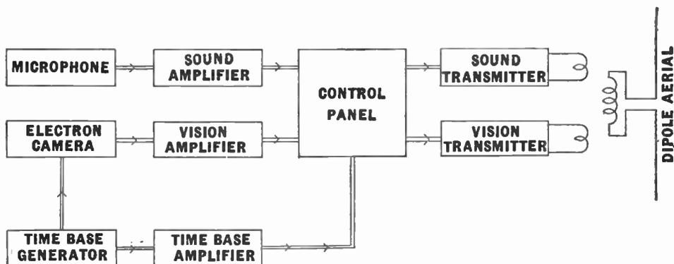
Fig. 97.—Diagram showing the various sections of a television transmitter. Only the essential units are included in this diagram.
