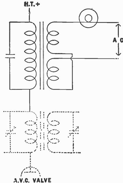
Fig. 181.—Circuit of the diminishing light indicator. A special transformer is necessary, as described in the text.
