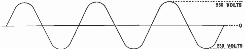
Fig. 32.—An A.C. voltage waveform with a peak value of 250 volts.
