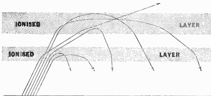
Fig. 16.—This illustration shows the variation in the behaviour of radio waves due to difference in frequency and also the effect of ionised layers of different density.
