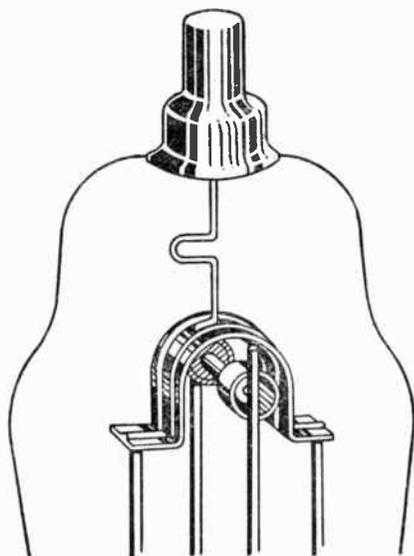
Fig. 103.—A typical high-voltage rectifier.
