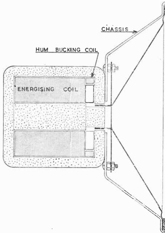
Fig. 174.—Section of an energised loudspeaker with hum bucking coil.
