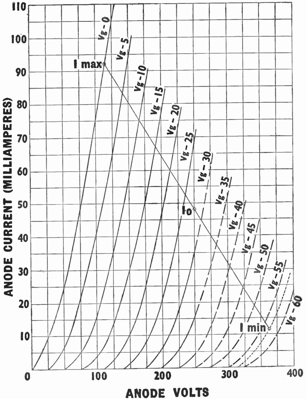
Fig. 166.—Anode-volt/anode-current curves of a directly heated output triode. The dotted curve is drawn in to show the position of  $V_g - 57$ , which is double the operating voltage of 28.5 volts.
