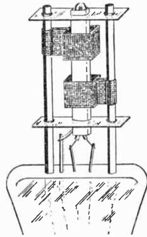
Fig. 176.—The electrode assembly of an indirectly heated double diode valve.
