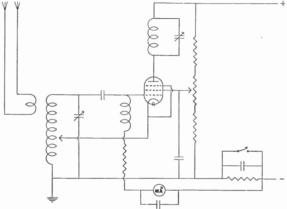
Fig. 53.—An example of the so-called electron-coupled oscillator; note that keying is accomplished by means of a biasing resistance in the high-tension negative lead.
