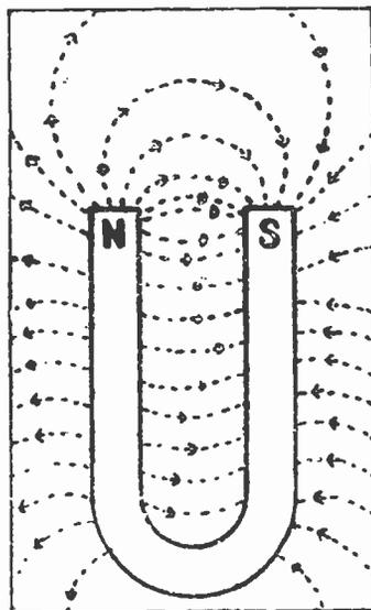
Fig. 36.—The field of a permanent magnet determined by means of iron filings placed on a sheet of glass.
