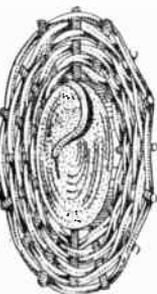
Fig. 87.—A typical basket coil.
