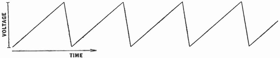
Fig. 11.—Waveform of a perfect time-base generator. This relationship between time and voltage is known as a saw-toothed waveform; the voltage rises from zero to maximum following a truly linear law and then returns to zero very rapidly.
