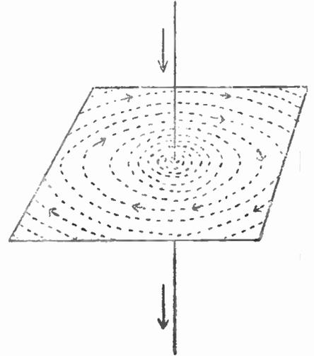
Fig. 37.—The field caused by conventional current; the conductor is passed through a sheet of paper on which iron filings are sprinkled.
