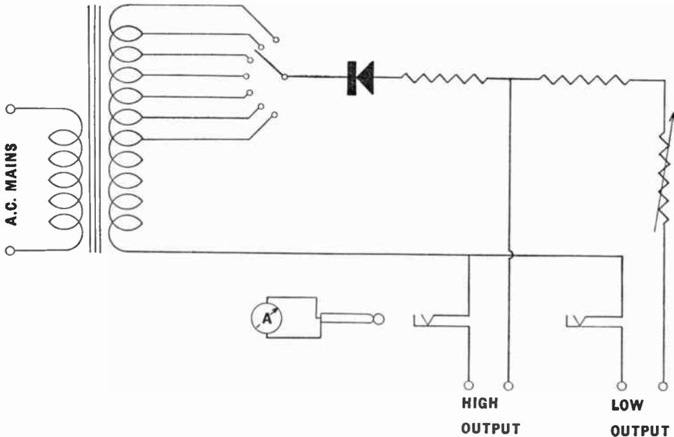
Fig. 75.—A more elaborate accumulator charger, allowing a group of large cells and a group of small cells to be charged simultaneously. The arrangement shown has a disadvantage that the current flowing through one circuit will vary the current flowing through the other, although any error can be corrected by means of the transformer tappings and variable resistance.
