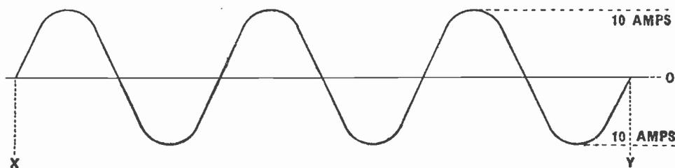
Fig. 31.—An alternating current waveform which has a peak value of 10 amps.
