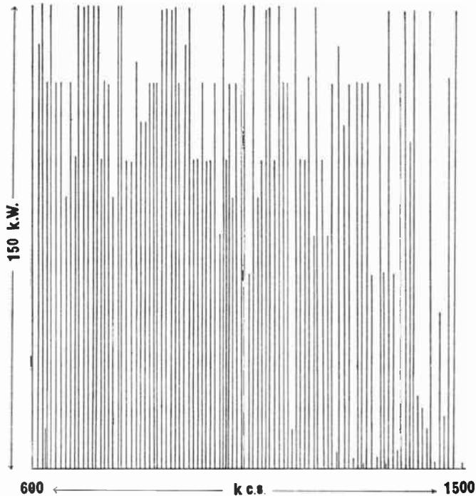
Fig. 129.—This diagram was prepared in exactly the same way as Fig. 128, but shows the situation to-day; a few stations actually are powered at 300 and even 500 kW and some have been omitted as they are too close to be drawn as separate lines, one line may represent as many as a dozen stations all working on the same wavelength.
