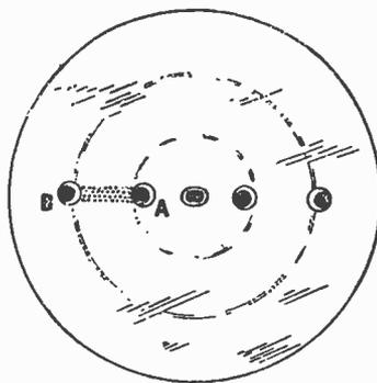
Fig. 34.—Top view of a mains triode, showing the ends of the electrode supports located in holes of a mica locking disc. This sketch illustrates a cause of hot leak, as described in the text.
