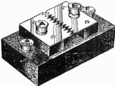
Fig. 91.—A simple form of lightning arrester.
