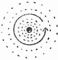
Fig. 38.—This diagram shows the direction of the magnetic field when the conventional current is travelling along the conductor towards the reader.
