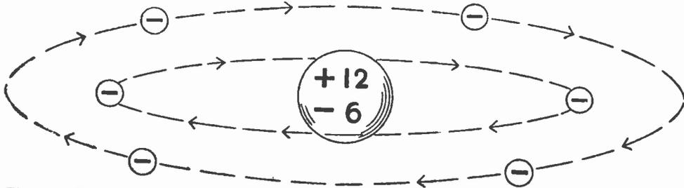
Fig. 22.—The carbon atom has six free electrons revolving on two orbits round the nucleus which is made up of twelve protons and six electrons and has, therefore, a positive charge equal to six protons.
