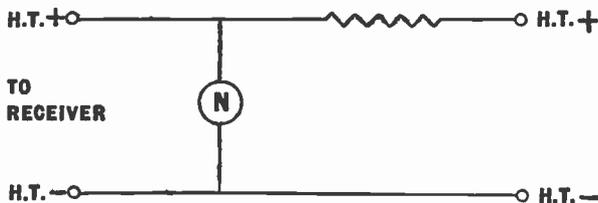
Fig. 15.—Basic circuit of a neon voltage stabiliser.
