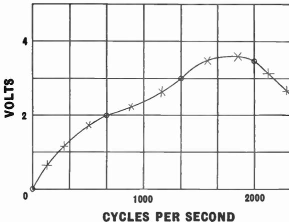
Fig. 79.—A graph showing the danger of insufficient points. Additional points might show that Fig. 78 is incorrect and should be as shown here.
