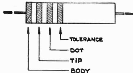
The modified colour code used for resistances with axial leads.
