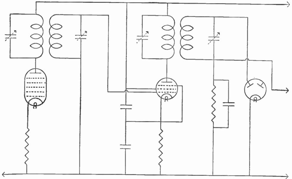
Fig. 132.—A complete circuit of an intermediate-frequency amplifier. The dotted arrows indicate that the associated condensers are of the variable pre-set type. The resistance shown on the right forms the diode load.
