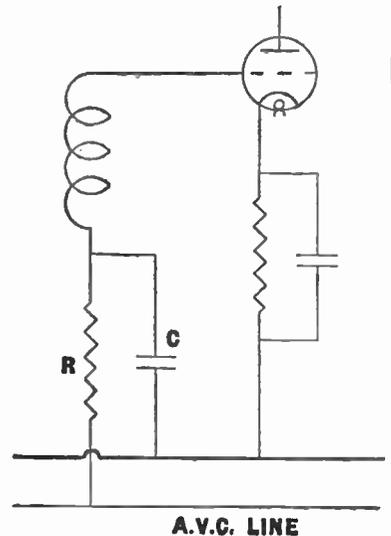
Fig. 17.—Arrangement for decoupling a grid circuit from the common impedance of the A.V.C.
