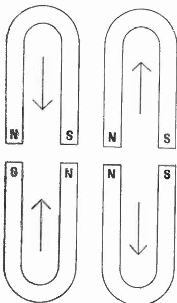
Fig. 34.—When permanent magnets are placed with unlike poles opposite they attract each other.
