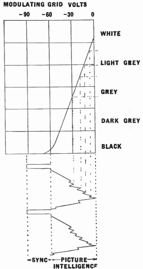
Fig. 84.—The television signal applied to the modulating grid of a typical cathode-ray tube.
