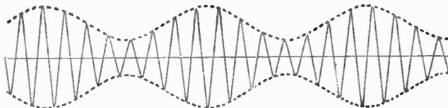
Fig. 12.—The modulated carrier wave showing both carrier and sound frequencies (amplified modulation system).
