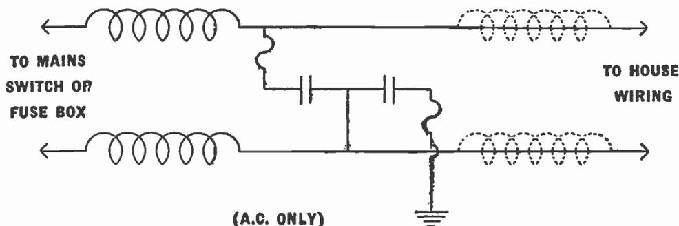
Fig. 60.—A more elaborate suppressor circuit for use on A.C. mains employing either two or four high-frequency chokes.
