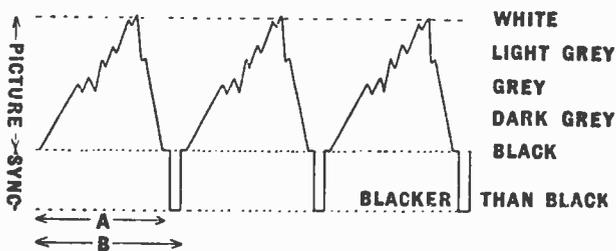
Fig. 82.—Modulation waveform of the television signal.
