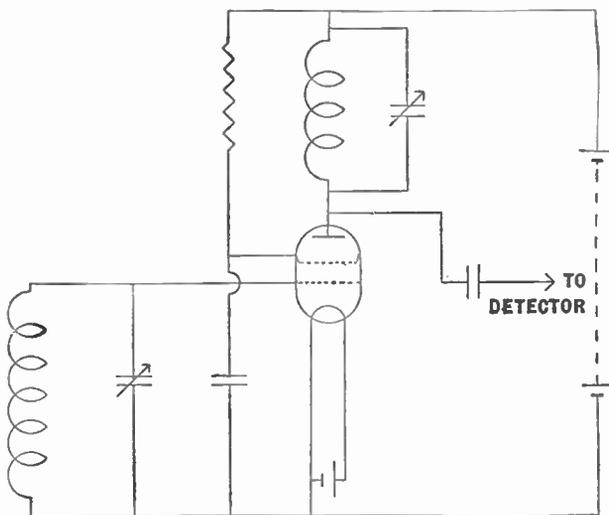
Fig. 106.—Basic circuit of a high-frequency amplifier using a screened-grid tetrode.
