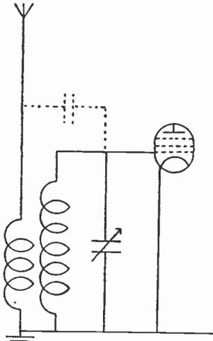
Fig. 111.—Aerial transformer coupling.
