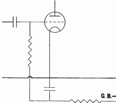
Fig. 19.—Grid-bias decoupling.
