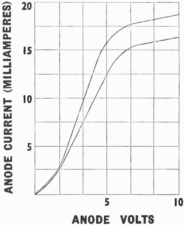
Fig. 74.—The characteristic curve of a diode valve showing the effect of filament temperature. The upper curve was taken with a potential difference of 4 volts across the filament, and the lower curve with 3.5 volts across the filament.
