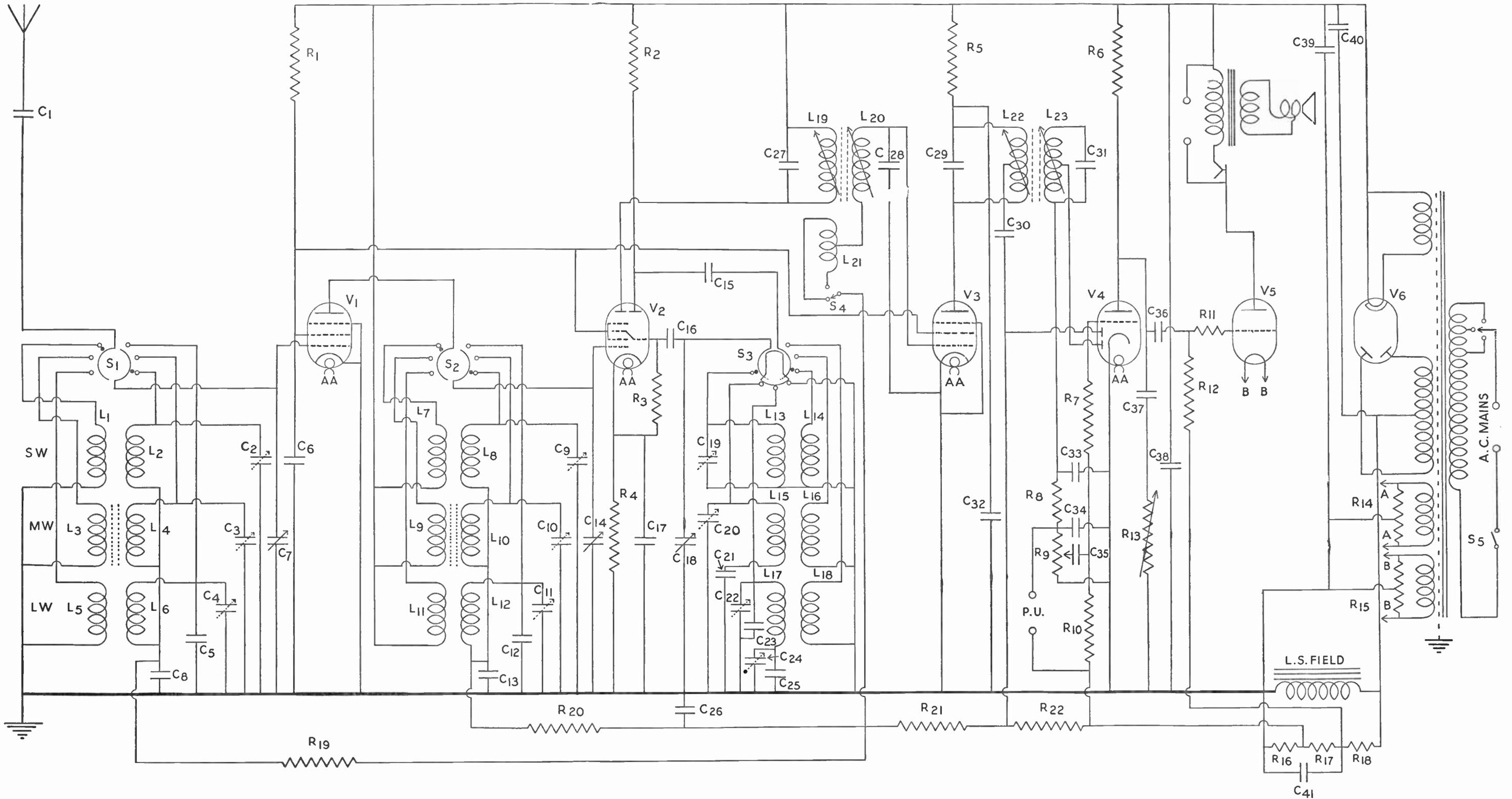
Circuit diagram of a five-valve (plus rectifier) A.C. superheterodyne receiver.
