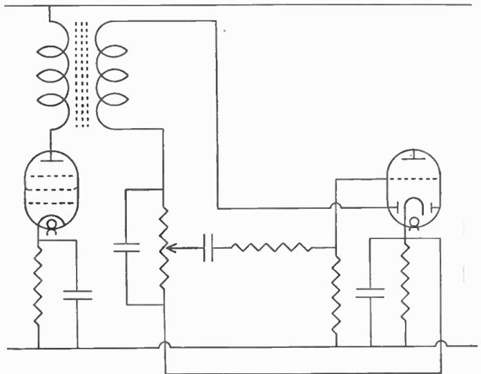
Fig. 154.—A double diode triode used as detector and low-frequency amplifier in a superheterodyne.
