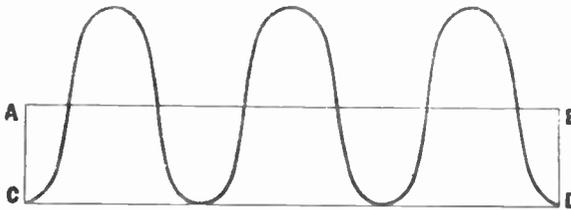
Fig. 54.—This diagram shows how the expression root mean square is derived.
