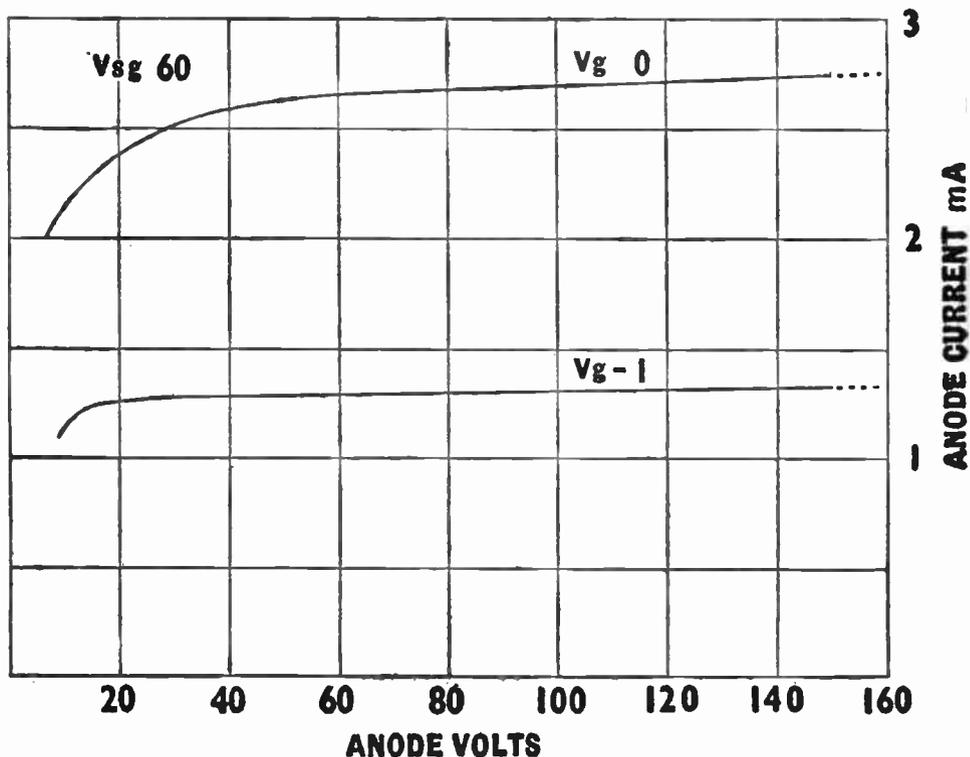
Fig. 108.—Characteristic curve of a screened-grid pentode. Note the increased linearity due to the suppression of secondary emission.
