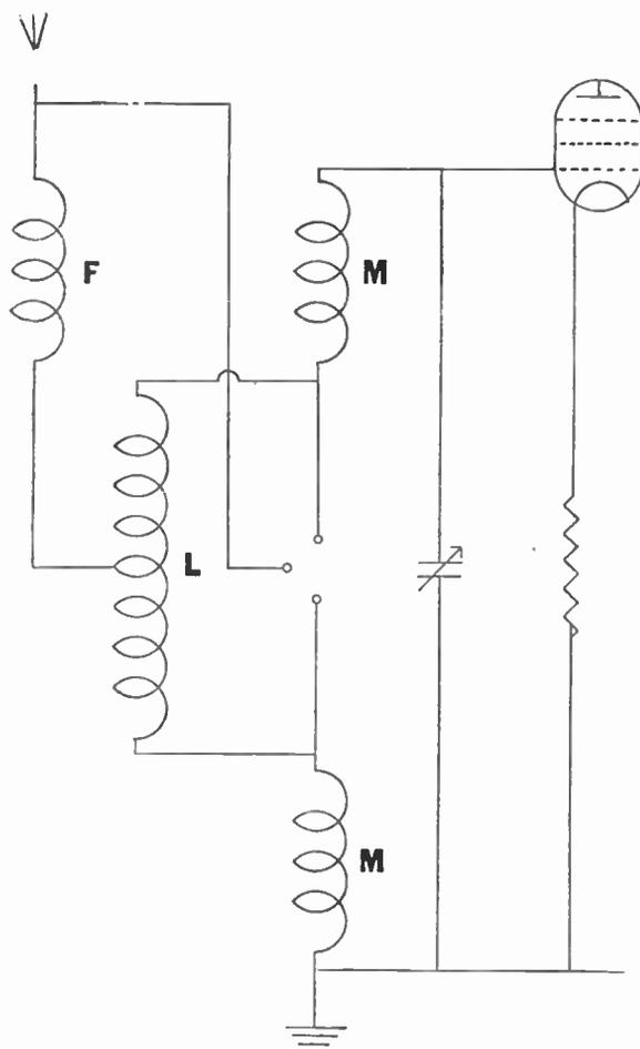
Fig. 145.—Wave-change and filter switched by means of a simple three-point switch.
