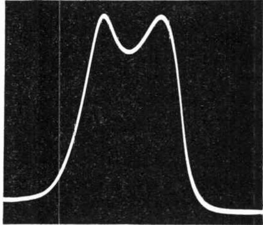
Fig. 134.—The intermediate-frequency response-curve using two tuned intermediate-frequency transformers slightly over-coupled.
