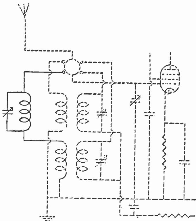
Fig. 49.—A rejector circuit placed in series with the long-wave winding so that it is automatically switched out of circuit on the medium waveband.
