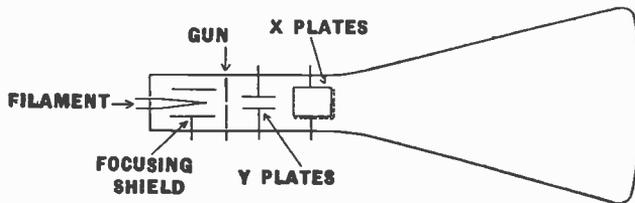
Fig. 13.—Symbolic representation of a gas-focused cathode-ray tube. Unfortunately there is no precise standardisation, but that shown above is typical.
