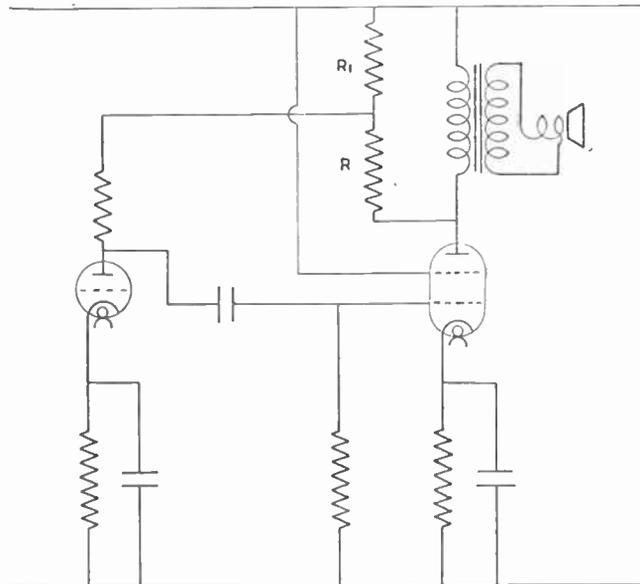
Fig. 163.—A satisfactory method of applying negative voltage feed-back to a tetrode or pentode output valve.
