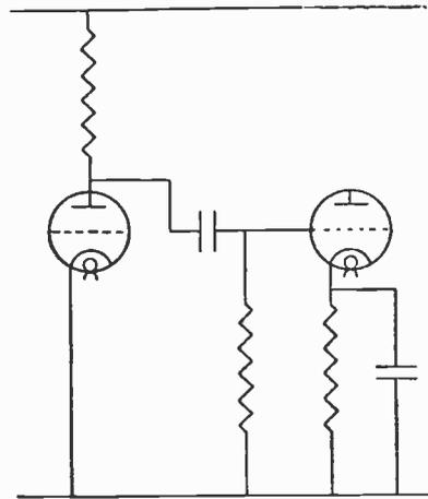
Fig. 148.—Resistance-capacity coupling.
