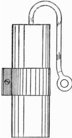
Fig. 43.—A condenser of the type specially designed for motor-car ignition interference suppression.
