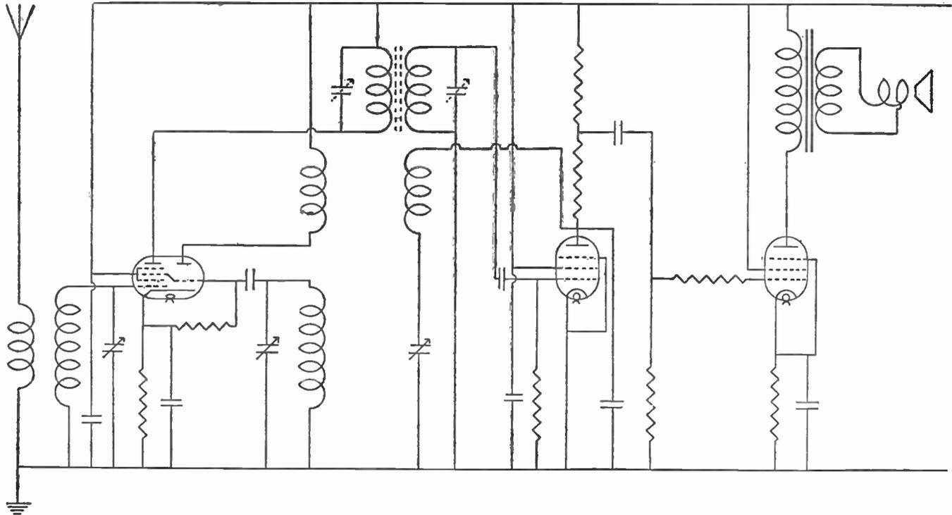
Fig. 30.—An alternative way of arranging a three-valve superheterodyne receiver. Note that no intermediate-frequency stage is used. Circuits of this type are used in midget receivers.
