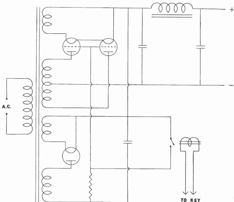
Fig. 65.—The use of grid-controlled rectifiers for keying a transmitter.
