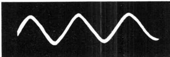
Fig. 4.—Oscilloscope showing mains ripple appearing across the points 1 and 2 in the circuit arrangement shown at Fig. 2.
