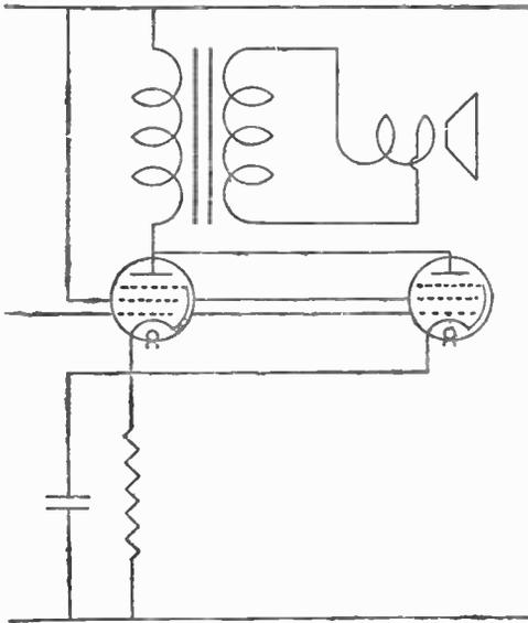
Fig. 160.—Output valves in parallel.
