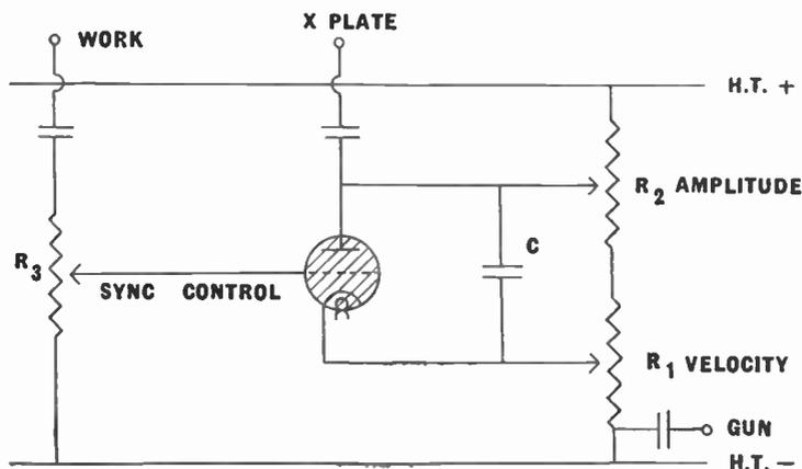
Fig. 18.—A simple time base using a gas-discharge triode. Although non-linear, it is nevertheless useful for certain types of work, and has the advantage of synchronising control. The valve symbol is shaded to indicate that a gas-filled valve is represented.
