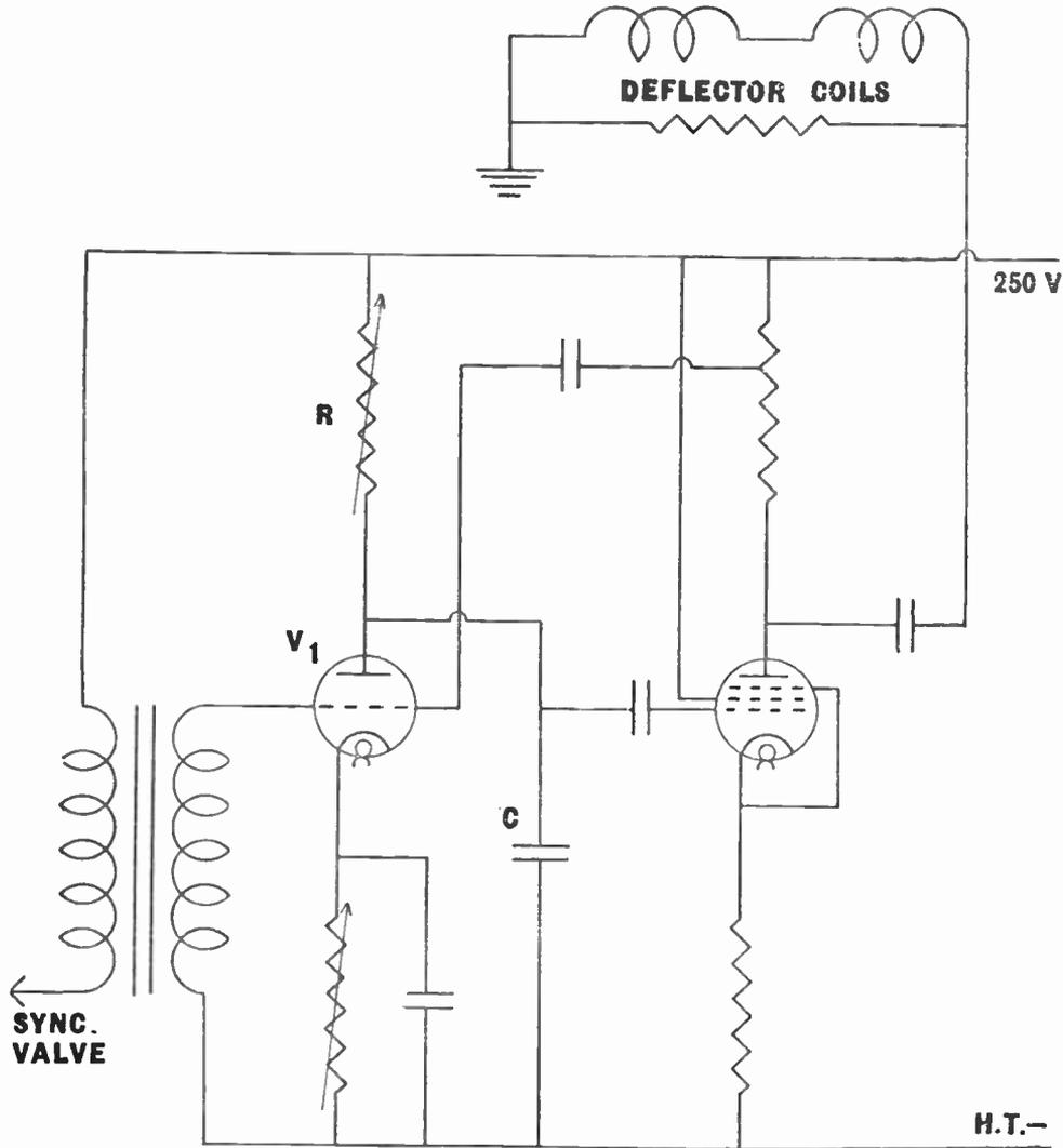
Fig. 90.—A skeleton circuit of a time base suitable for magnetic deflection.
