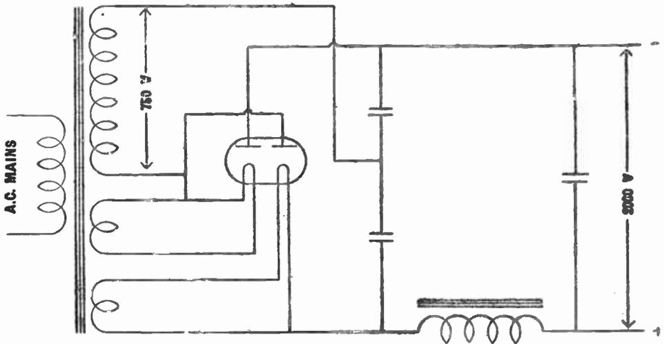
Fig. 11.—Voltage doubler circuit employing valve rectification; note that the filaments must be led out separately and not connected together inside the valve.
