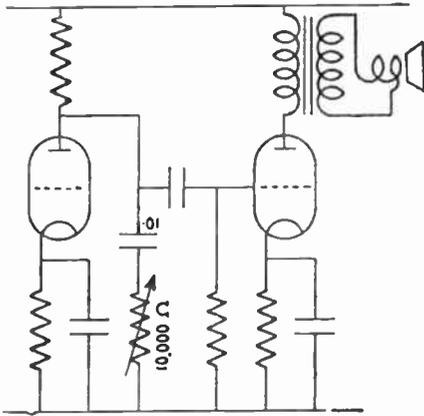
The conventional variable tone-control circuit for cutting the higher frequencies.
