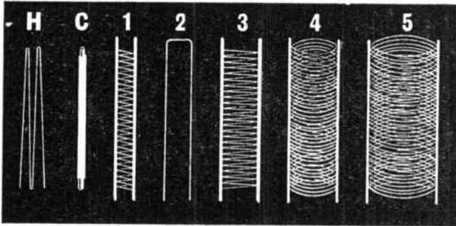
Fig. 121.—The electrodes of a pentagrid valve. The anode is not shown, since it may readily be seen at Fig. 120. Those shown are, from left to right: heater, cathode, oscillator grid, oscillator anode (phantom grid), inner screening grid, signal grid, and outer screening grid.
