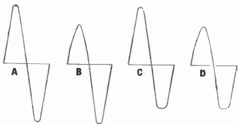
Fig. 83.—(A) A normal undistorted A.C. waveform. (B) The effect of underbiasing. (C) The effect of overbiasing, and (D) Overloading.
