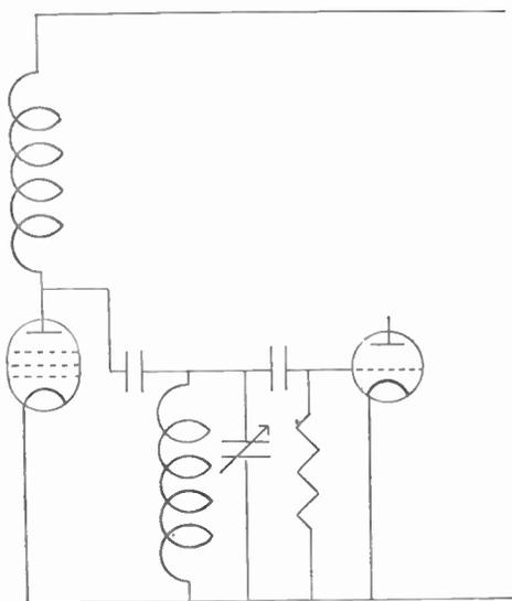
Fig. 116.—Tuned grid intervalve coupling.
