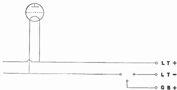
Fig. 146.—A three-point switch arranged to break the filament and grid-bias battery circuits simultaneously.
