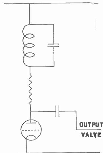
Fig. 27.—A top-lift circuit using an inductance tuned by a condenser as part of the anode load. Typical values are  $.006 \mu\text{F.}$  and  $.1$  henry and 3,000 ohms.
