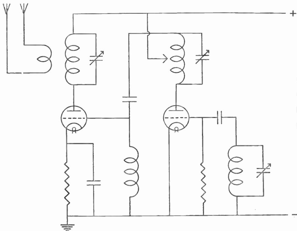
Fig. 58.—A high-frequency amplifying stage with an improved type of coupling which is explained in the text.
