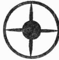
Fig. 185.—Appearance of the "magic eye" under conditions of maximum signal.
