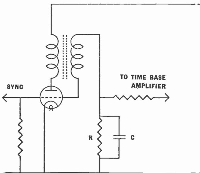
Fig. 94.—The basic circuit of the squegger time base.
