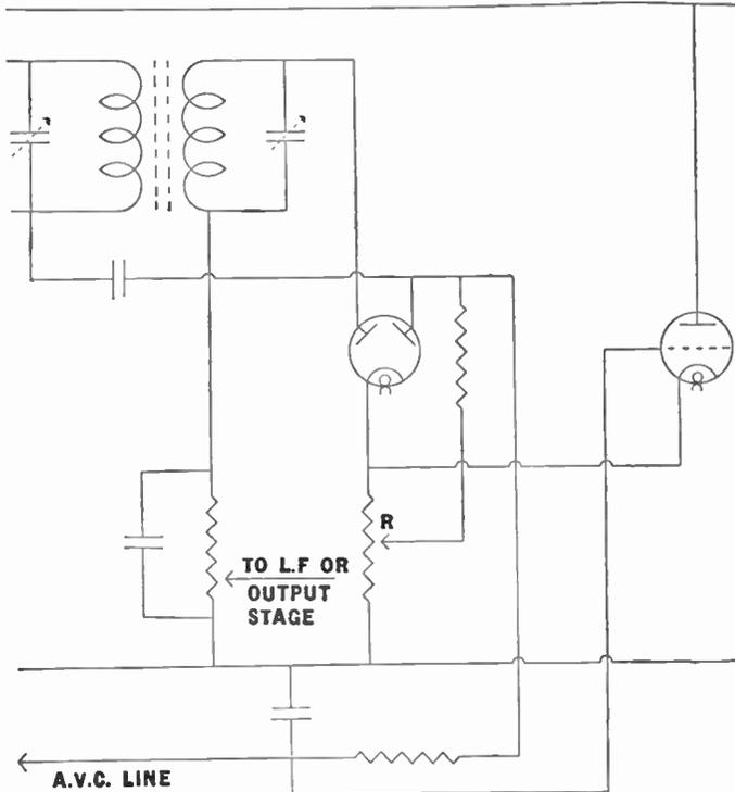
Fig. 195.—A simple inter-station noise-suppressor circuit using a triode valve for muting.
