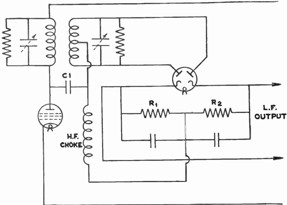
Fig. 205.—The phase detector frequency-amplitude converter.
