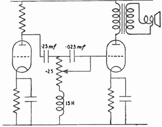
A variable tone-control circuit for cutting the lower frequencies.
