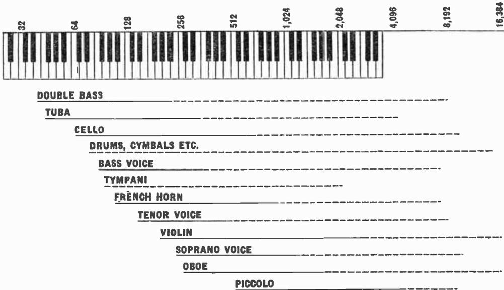
Fig. 10.—The frequency range of various instruments is shown above. The solid lines represent the fundamental notes, while the broken lines show the harmonic range necessary for true reproduction; the tympani and drums have no range of notes, but a wide frequency band is covered by harmonics, rattling noises, etc. The total scale is shown in cycles per second and extends two octaves and two notes above a full-scale piano.
