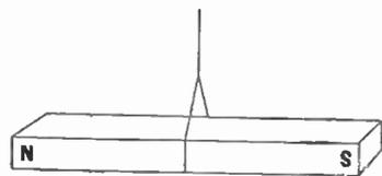
Fig. 33.—If a magnet is freely suspended, it will come to rest on a line due north and south. That end which points to the north is termed the north pole.
