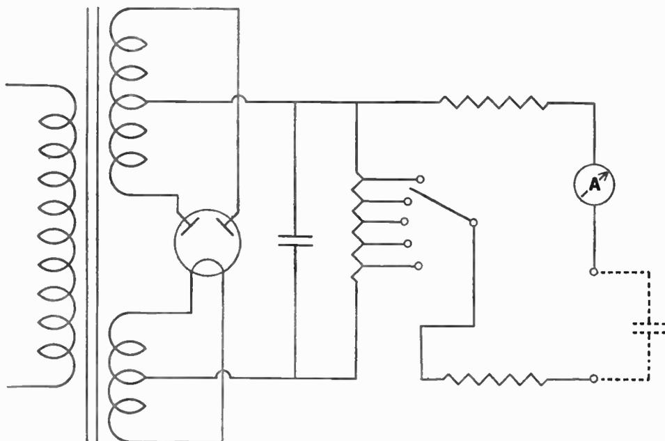
Fig. 53.—An arrangement for testing condensers for leakage which has the advantage over usual methods that the full working voltage may be applied. A tapped resistance permits the selection of a suitable voltage consistent with the type of condenser under test. A tapped resistance is used in preference to a potentiometer, to dispense with a voltmeter.
