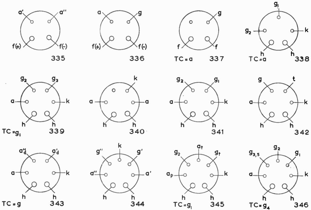
Note.—All connections are as viewed from underside of valve bases.
