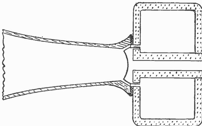
Fig. 175.—Section of a horn-type moving-coil loudspeaker; the shape of the horn usually follows an exponential law. Note the concave diaphragm.
