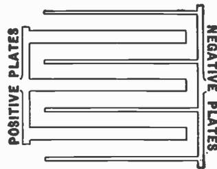
Fig. 25.—The arrangement of a seven-plate accumulator.
