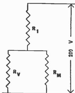
Fig. 23.—Symbolic rearrangement of Fig. 22, when  $R_v$  represents the resistance through the valve and  $R_m$  the resistance of the meter.
