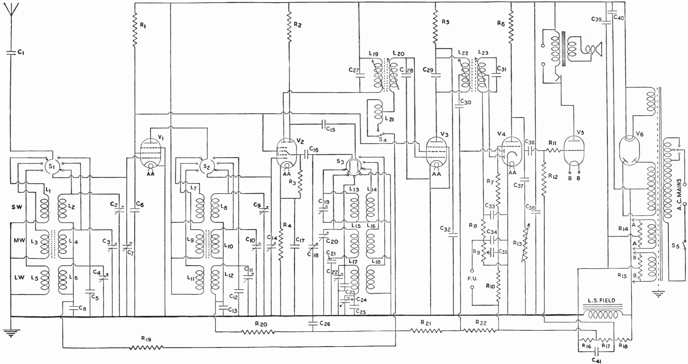
Circuit diagram of a five-valve A.C. superheterodyne receiver.
