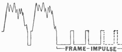
Fig. 87.—Frame impulse terminating a scanning field which ends with a complete line.
