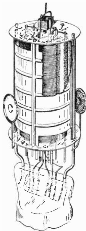
Fig. 120.—The electrode assembly of a typical pentagrid valve. The external appearance of the octode is similar.
