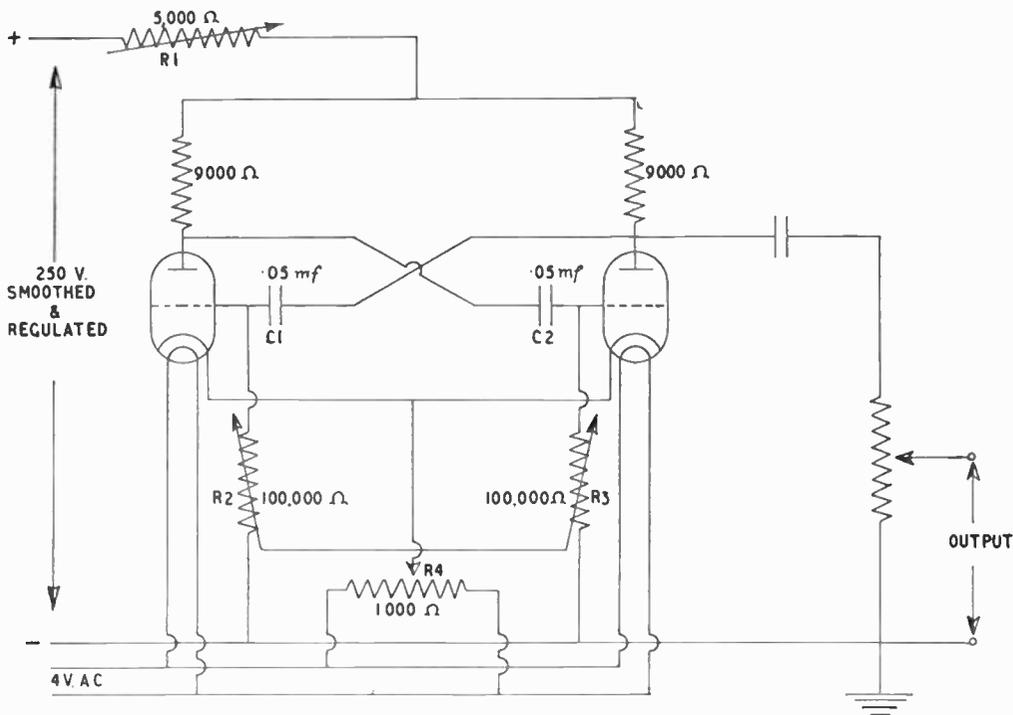
This improved form of multi-vibrator has the advantages of wide frequency range and extreme simplicity; the multi-vibrator unfortunately, however, has a bad waveform, although with this particular arrangement some improvement can be made by careful adjustment of R1. The ganged variable resistances R2, R3 control the output frequency, R4 allows a small voltage at mains frequency to be used to lock the oscillator frequency at any desired multiple of the mains frequency.
