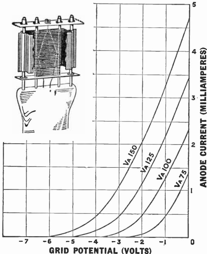
Fig. 80.—Characteristic curves of a typical triode valve. The valve from which they were taken is illustrated in the inset.
