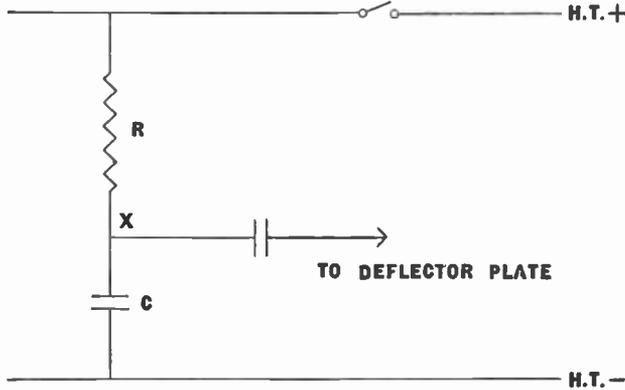
Fig. 77.—Diagram illustrating the principle of a time base.
