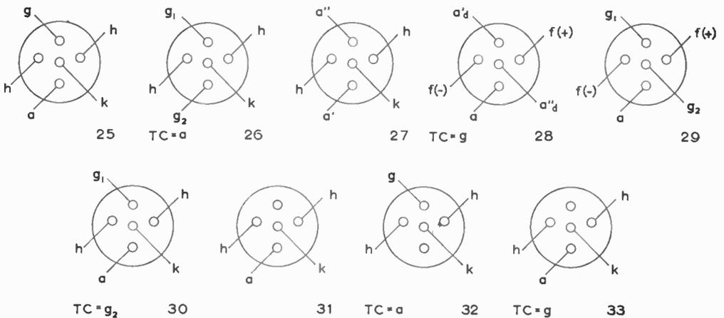
Note.—All connections are as viewed from underside of valve bases.
