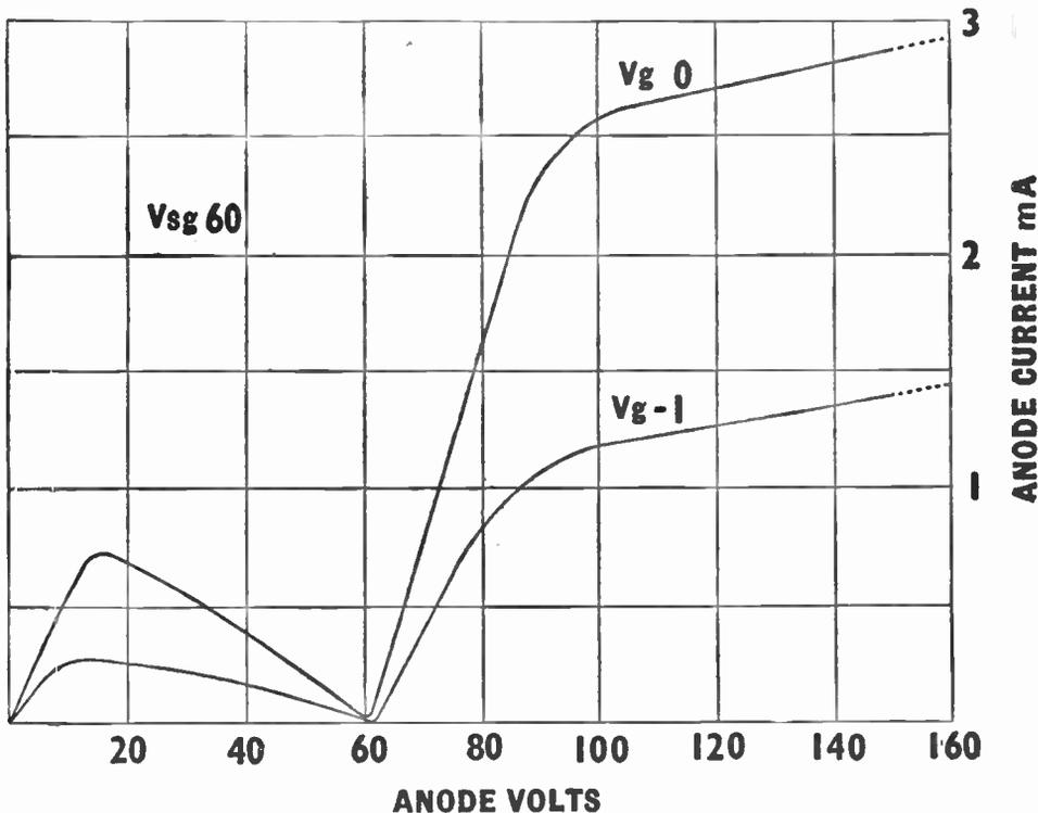
Fig. 107.—Characteristic curve of a screened-grid tetrode. Note that the straight portion (105–150 volts) is restricted by the negative resistance kink.
