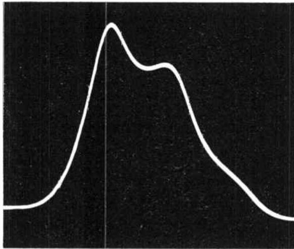
Fig. 135.—A response-curve taken from the same intermediate-frequency amplifier as that used for taking Fig. 134, but with the secondary of the first transformer slightly mis-tuned.
