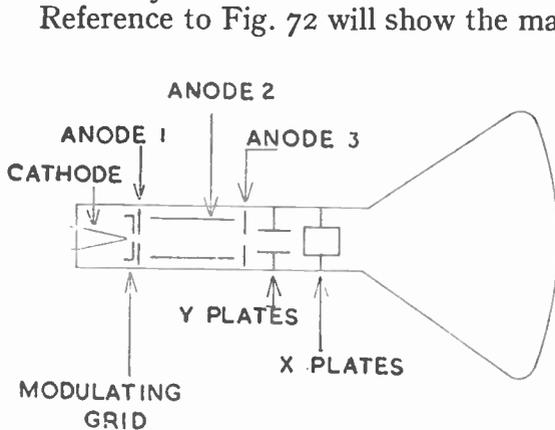
Fig. 72.—Symbolic representation of an electrostatically focused and deflected cathode-ray tube.
