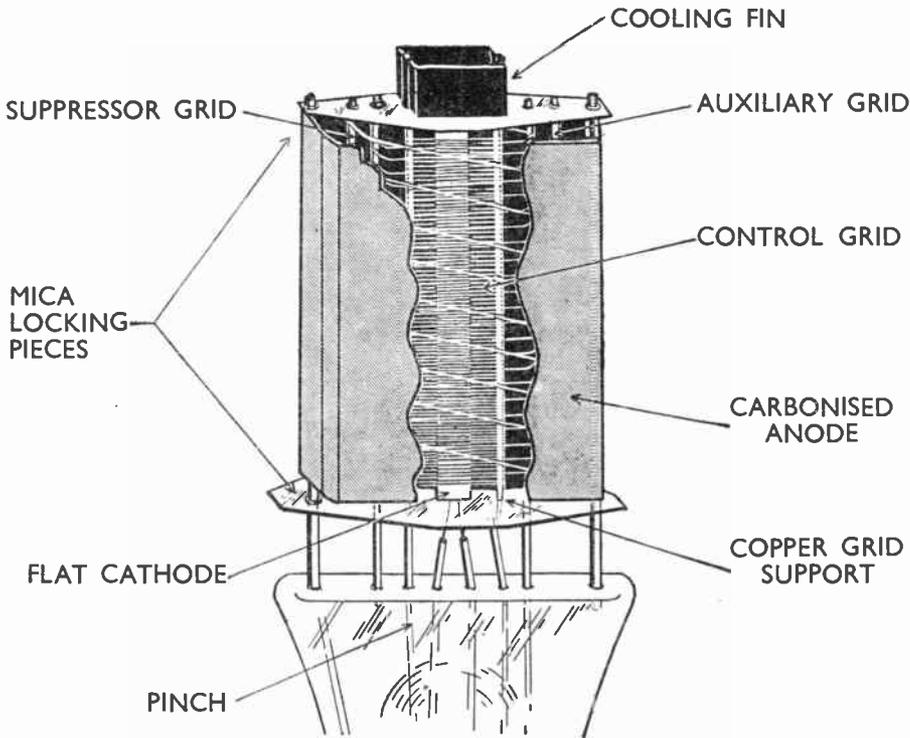
Fig. 165.—A high-slope output pentode rated to dissipate 20 watts.
