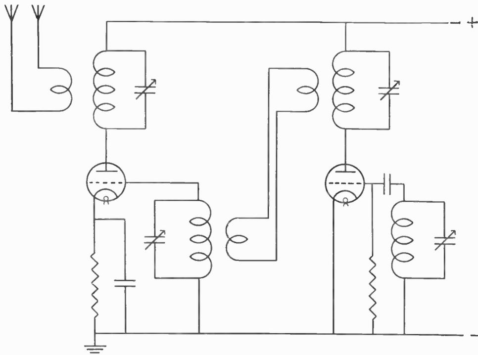
Fig. 59.—This illustration shows the use of link coupling between the oscillator and high-frequency amplifier.
