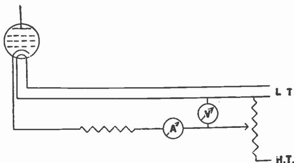
Fig. 35.—An arrangement for testing insulation between heater and cathode of a mains valve. When testing A.C. types the potential difference between the two electrodes should not normally exceed about 10 volts, but when testing universal types the potential difference may be relatively high. (See text.) This circuit could be incorporated with that shown at Fig. 31 or Fig. 33, but is shown separately for clearness.
