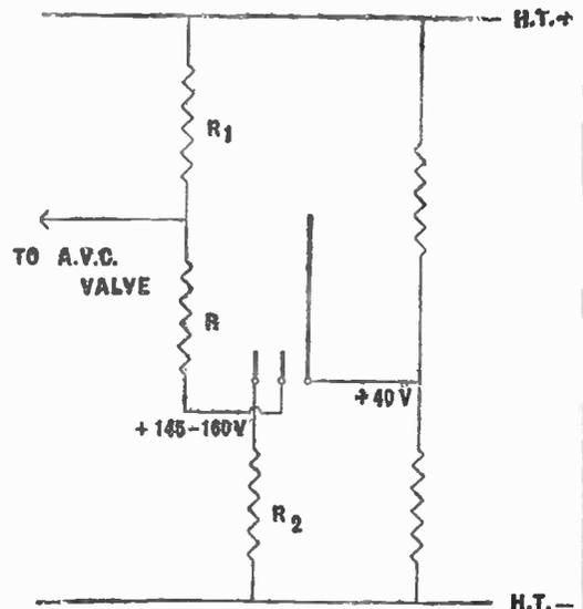
Fig. 183.—Basic circuit of the neon tuning indicator
