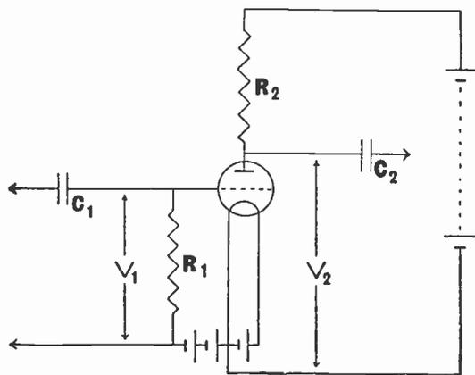
Fig. 85.—A skeleton diagram to illustrate the principles of voltage amplification.
