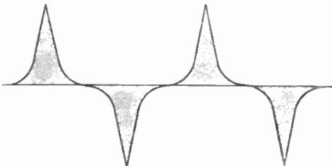
Fig. 56.—A waveform which has a low mean value ; note the comparatively small tinted area. This illustration, like Fig. 57, has been drawn to accentuate the explanation in the text ; the shape is rather improbable.
