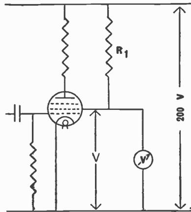
Fig. 22.—The error introduced by connecting a voltmeter in this circuit is described in the text.
