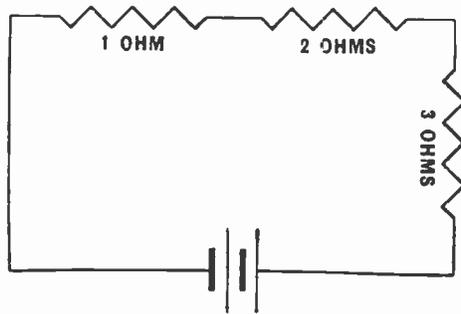
Fig. 29.—A circuit comprising three resistances in series.
