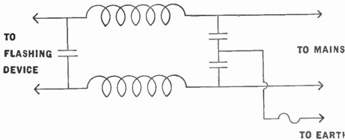
Fig. 65.—A filter circuit for use with a heavy-duty make-and-break device.
