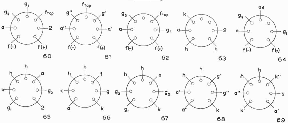
Note.—All connections are as viewed from underside of valve bases.
