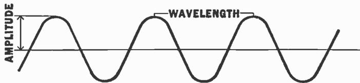
Fig. 1.—A wavetrain or series of waves showing how wavelength and amplitude are measured.
