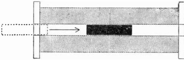
Fig. 41.—Section of a coil showing the position taken up by an iron rod due to action of the magnetic field.
