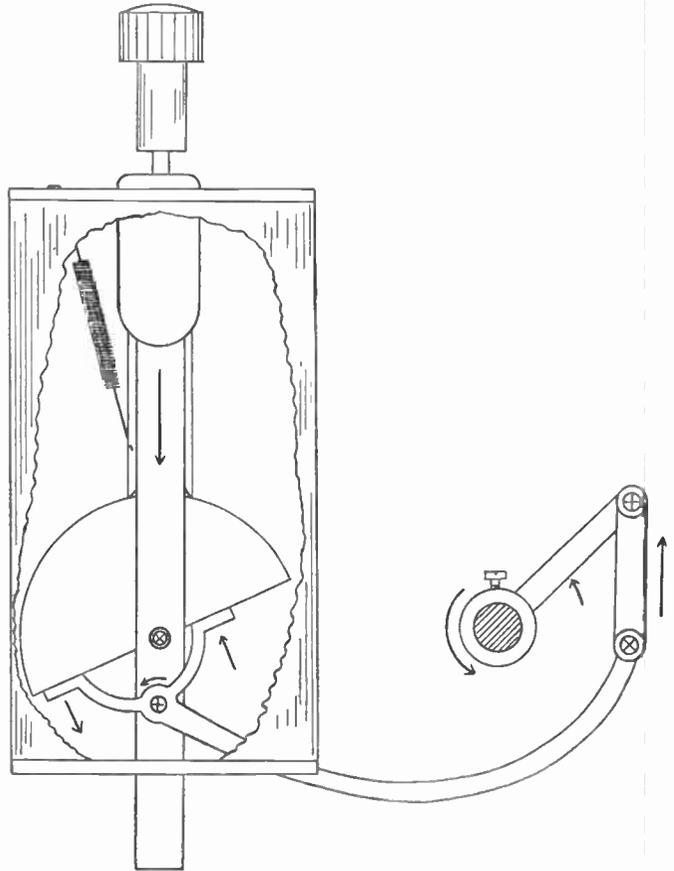
Fig. 197.—A diagrammatic drawing showing the operation of a push-button unit.
