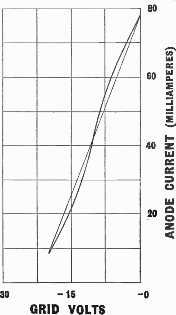
Fig. 156.—Dynamic curve of a pentode output valve; the curve deviates on both sides of the imaginary straight line, indicating the presence of third harmonic distortion.
