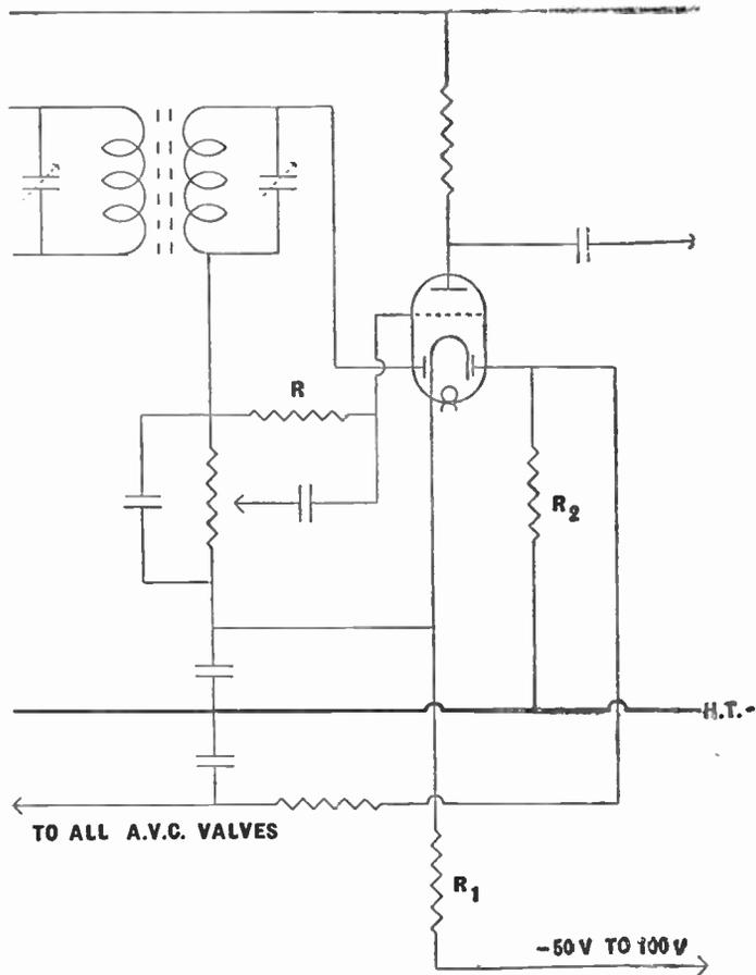
Fig. 180.—Basic circuit for delayed and amplified automatic volume control.
