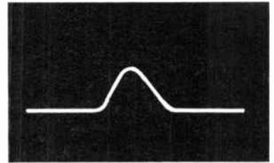
Fig. 40.—By adjustment of the intermediate frequency amplifier the first trace is obtained.
