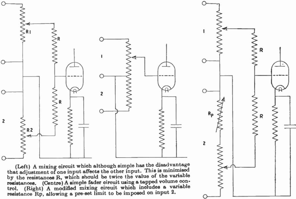
(Left) A mixing circuit which although simple has the disadvantage that adjustment of one input affects the other input. This is minimised by the resistances R, which should be twice the value of the variable resistances. (Centre) A simple fader circuit using a tapped volume control. (Right) A modified mixing circuit which includes a variable resistance  $R_p$ , allowing a pre-set limit to be imposed on input 2.
