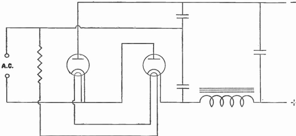
Fig. 12.—Voltage-doubling circuit arranged for direct connection to alternating-current supply.
