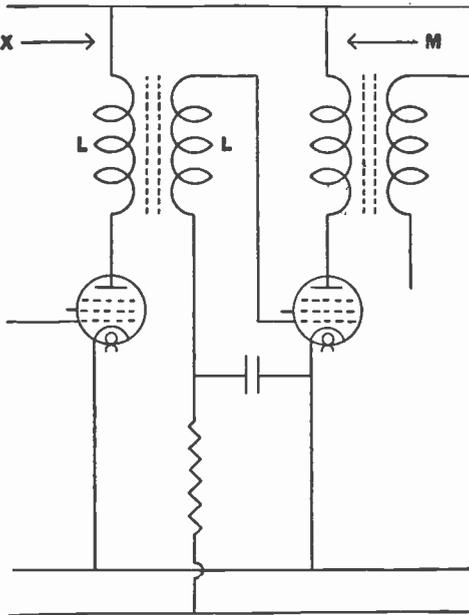
Fig. 55.—Skeleton circuit, showing an indirect method of measuring for leakage between the coils LL. A suitable milliammeter is inserted at the point marked M, and the high-tension feed is broken at the point marked X.
