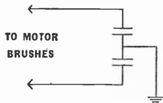
Fig. 61.—A simple suppressor circuit suitable for a small D.C. motor.
