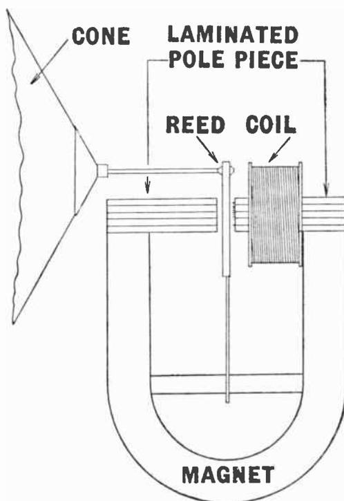
Fig. 169.—A reed-type loudspeaker; some examples have a coil on both pole pieces
