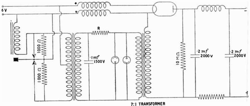
An interesting vibrator power pack used by the author for the E.H.T. supply of a portable oscillograph which worked from a 6-volt car battery. The author has used a similar circuit to obtain the E.H.T. supply for a television receiver converted for use on D.C. mains. H.F. chokes marked \* should be inter-wound; R should be adjusted so that the neon stabiliser tubes just glow. The 10MΩ resistance must be made up of several resistances in series, e.g. five resistances of 2MΩ each.
