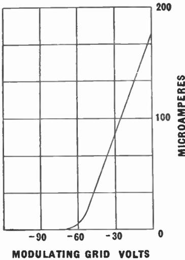
Fig. 83.—Modulating-grid-volts/beam-current curve of a typical cathode-ray tube.
