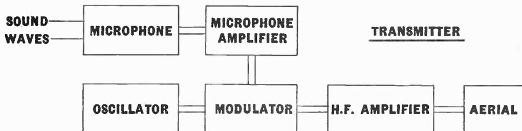
Fig 11.—A "block diagram" of the broadcasting chain showing the links. This diagram and accompanying text is based on the standard A.M. broad-
