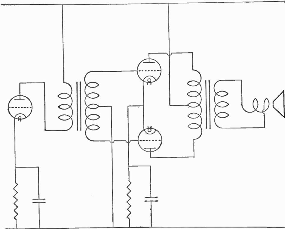
Fig. 161.—Basic circuit of a push-pull output stage using indirectly heated valves.
