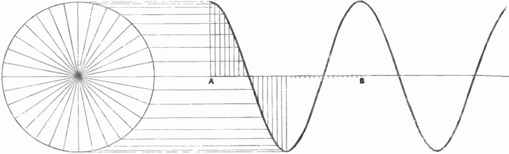
Fig. 58.—The relationship between a sine wave and a circle can readily be seen from this illustration in conjunction with the text.
