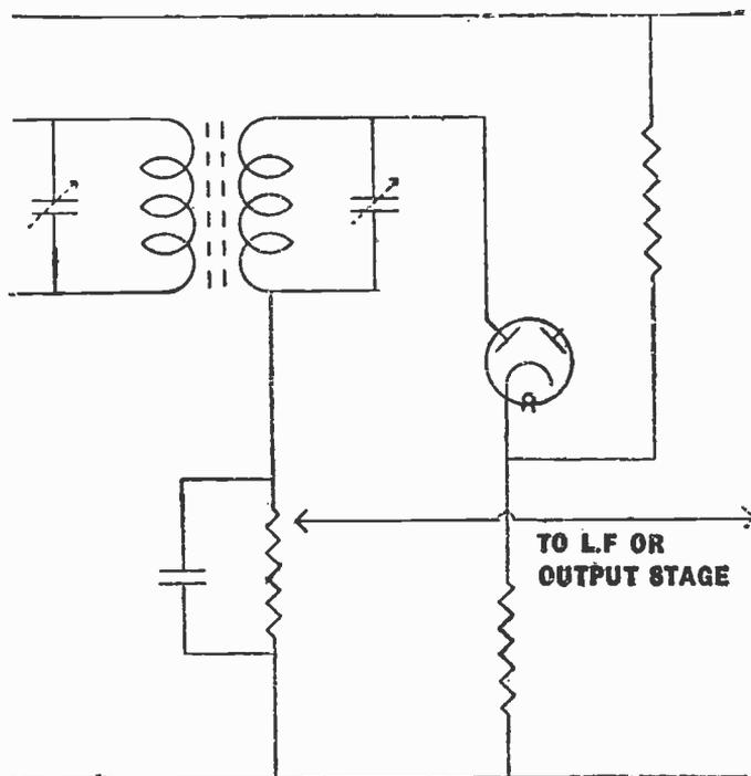
Fig. 192.—A very simple form of inter-station noise suppression achieved by placing a negative bias on the detector anode.
