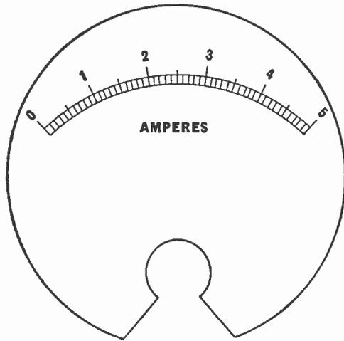
Fig. 2.—Scale of a moving-coil instrument. Note the linear division of the scale.
