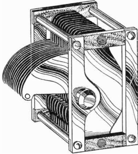
Fig. 48.—A simple variable condenser.
