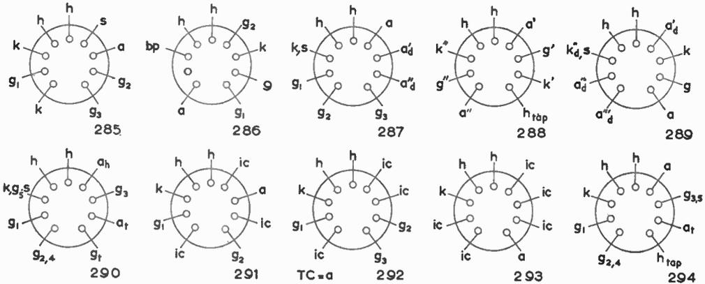
Note.—All connections are as viewed from underside of valve bases.
