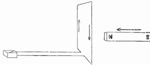
Fig. 42.—A current will be induced in a conductor if a magnet is moved in its vicinity. Small arrows show direction of conventional current when the north pole is moved towards the conductor.
