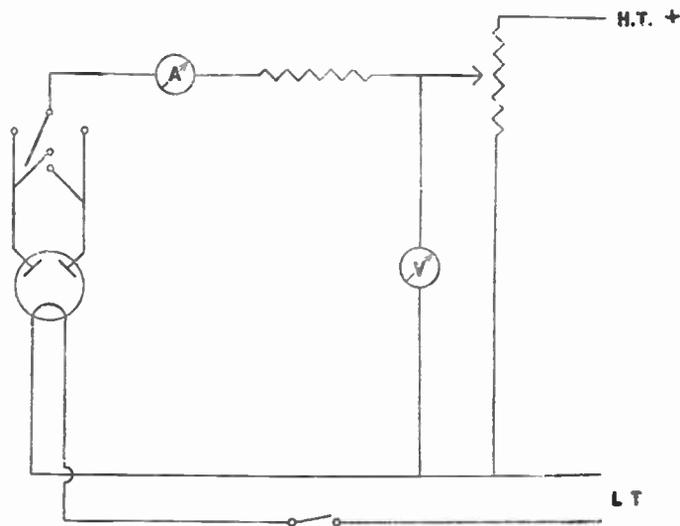
Fig. 32.—Circuit arrangement for measuring emission of a rectifier or diode valve. The switch permits emission to be measured for either or both sections. By opening the single-pole switch relatively high potential may be connected between anodes and filament to test for leak. This circuit could be incorporated with that shown at Fig. 31 or Fig. 33, but is shown separately for clearness.
