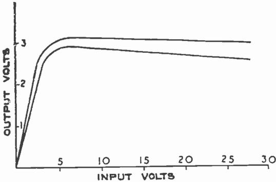
Fig. 203.—Action of the limiter valve; typical input-voltage, output-voltage curves.
