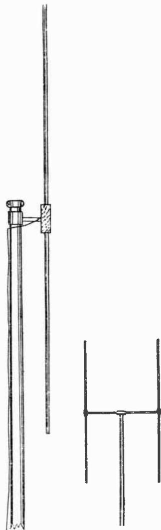
Fig. 104. — (Left) A typical dipole. The feeder should be led away at right angles for a distance of at least 12 inches; dipole aerial must be horizontal for receiving certain B.B.C. transmitters. (Right) Dipole aerial with reflector.
