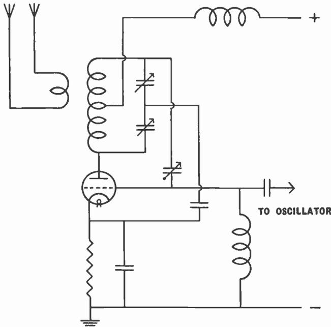
Fig. 62.—An improved arrangement for anode-circuit neutralisation.
