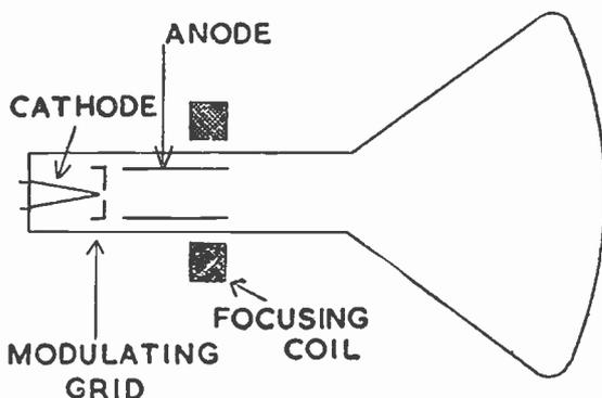
Fig. 73.—Symbolic representation of a magnetically focused and deflected cathode-ray tube. The shaded area can represent either coil or magnet.
