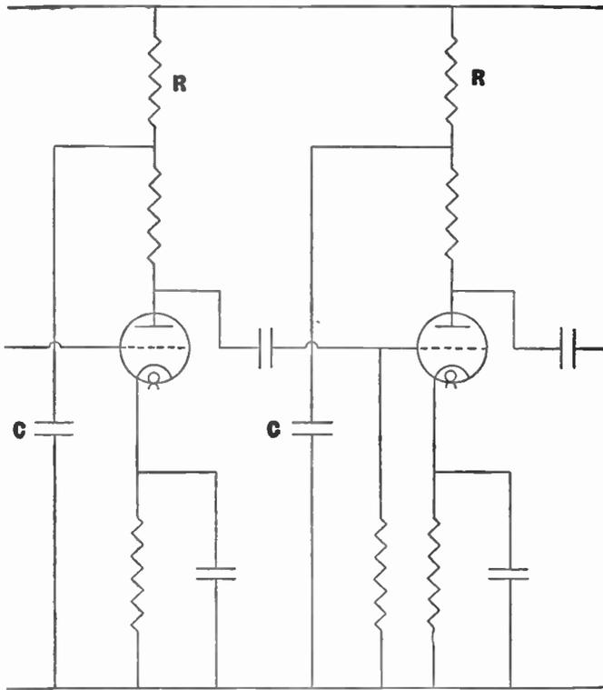
Fig. 16.—Two stages with anode decoupling, which is effected by means of resistances and condensers.
