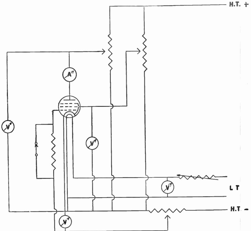
Fig. 31.—A circuit permitting the characteristics of any valve to be measured, providing the meters used have adequate ranges. In addition, a number of faults can be detected, as described in the text. This may be taken as the basic circuit of a valve test-board, but the complete circuit is greatly complicated by the diversity of valve types and the non-standardisation of their pin connections.
