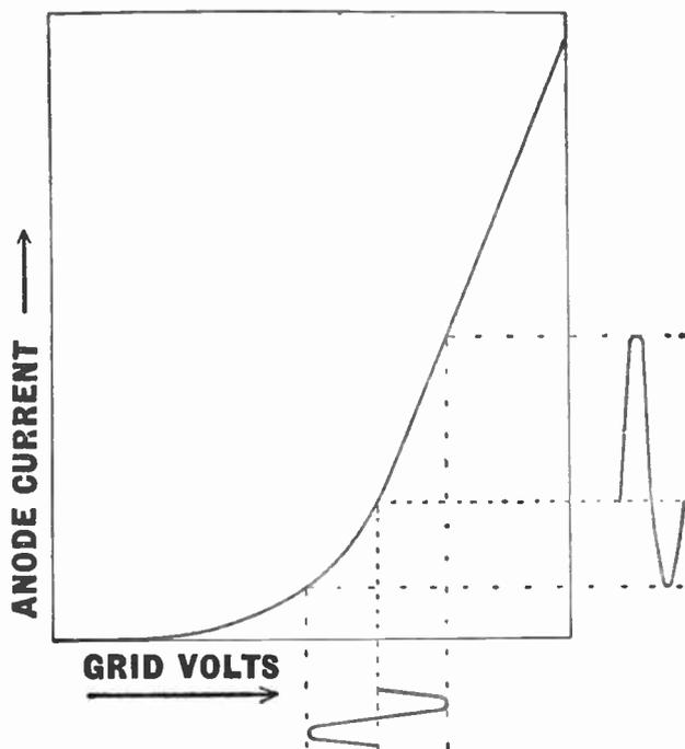
Fig. 82.—Showing an alternating voltage input and resulting alternating current output when valve is overbiased.
