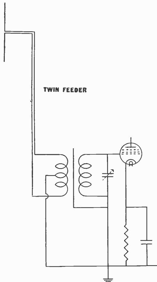
Fig. 107.—The aerial circuit arranged for use with twin feeder.
