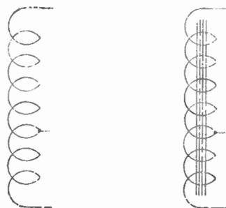
Fig. 47.—Right: the conventional symbol for an iron-core auto-transformer. Left: the symbol for an air-core auto-transformer.
