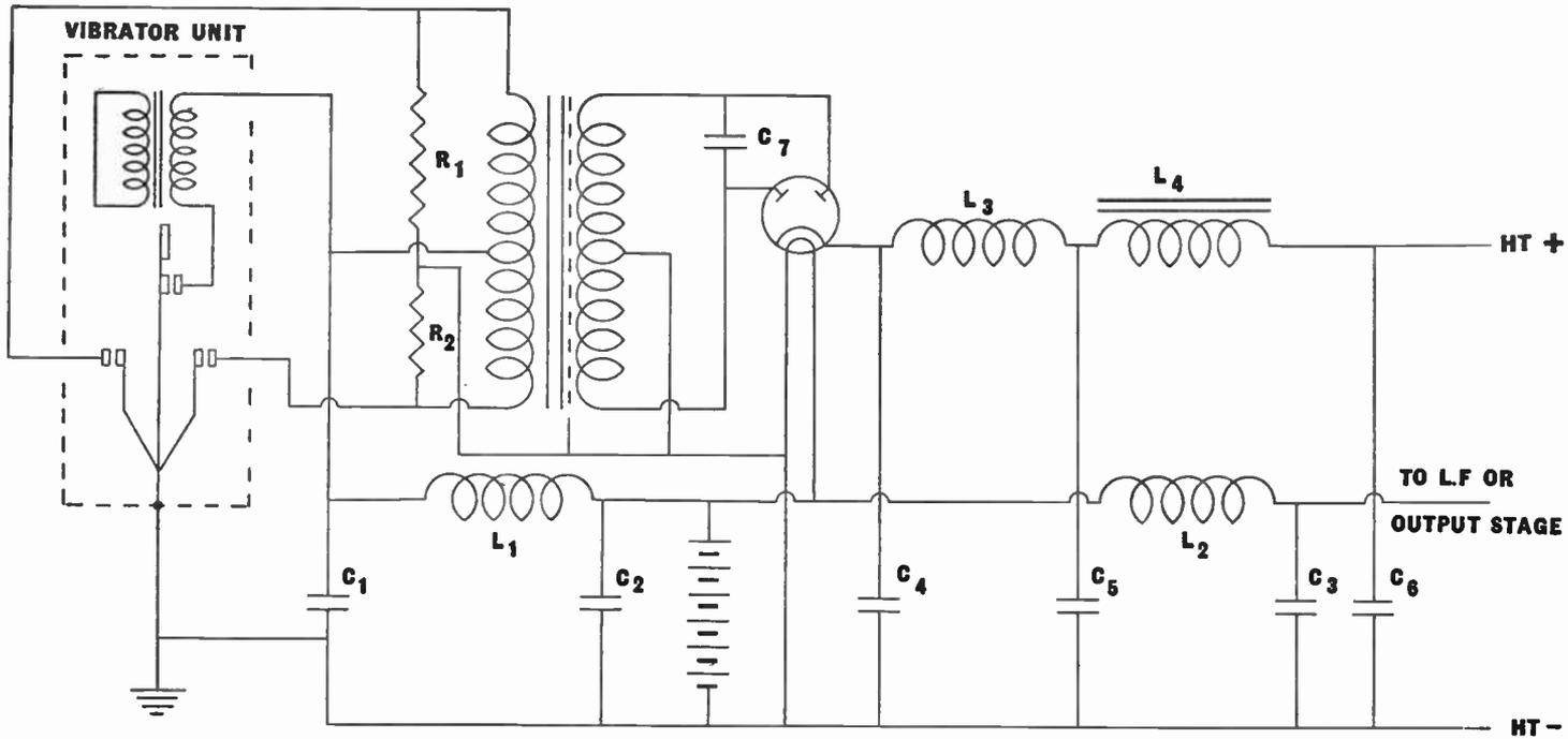
Fig. 41.—A simple car-radio power unit.
