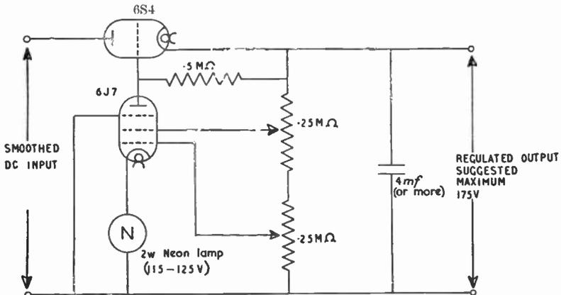
A valve voltage regulator circuit suitable for laboratory use which gives a remarkably constant output voltage; the maximum current output is about 25 m.a. but two or more S64 valves may be used in parallel as desired to increase output. In exacting conditions where the output voltage must be independent of ambient temperature, the neon lamp must be replaced by some source of D.C. bias such as the 24-volt accumulator.
