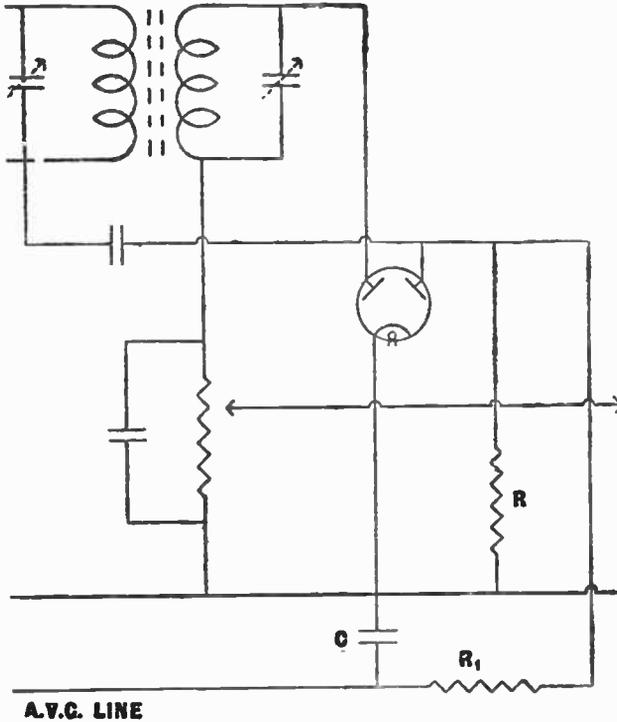
Fig. 191.—A modified automatic volume control circuit where the diode is fed from the primary of the intermediate-frequency transformer to minimise sideband shriek.
