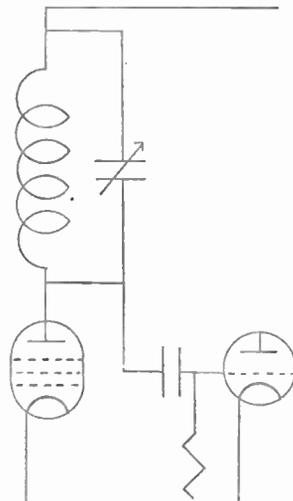
Fig. 115.—Tuned anode intervalve coupling.
