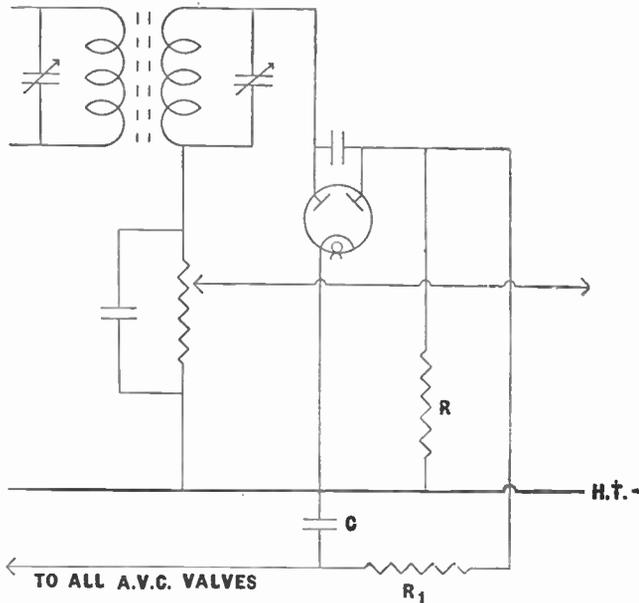
Fig. 177.—The circuit arrangement for simple automatic volume control. The H.T.—(earth) line is emphasised to indicate that the leads shown below it are negative in respect to H.T.—
