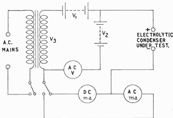
This electrolytic-test set will give leakage current and approximate capacity under working conditions. With switch in position shown, leakage current may be read directly from D.C. milliammeter; V1 should equal D.C. working-voltage of condenser (V2 must exactly equal V1).
