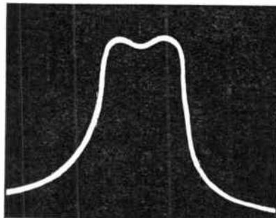
Fig. 45.—Alignment of the intermediate-frequency amplifier duly completed, the response-curve being as flat as possible and also as high as possible.
