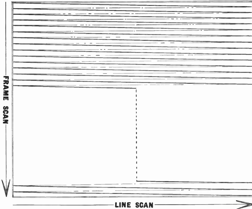
Fig. 76.—A sequential, or continuous raster; the thick lines represent the line scan, and the thin lines the fly-back.
