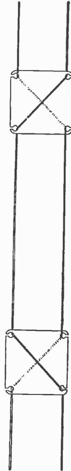
Fig. 38.—Enlarged view showing a section of a transposed feeder. Note the special insulators employed.
