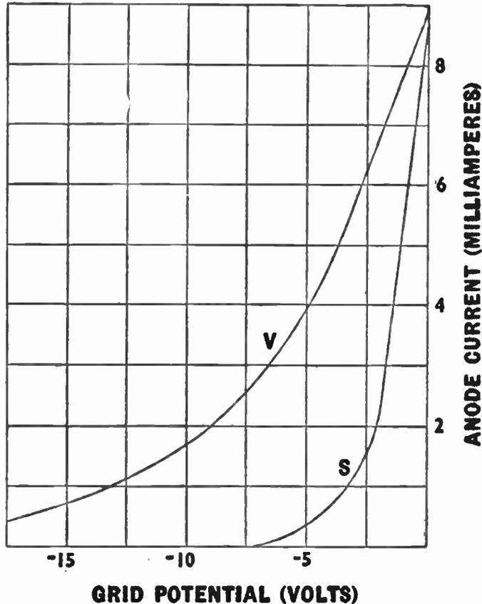
Fig. 109.—Comparison between a variable-mu valve and a "straight" valve.
