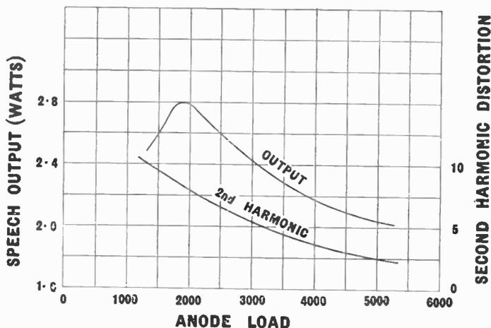
Fig. 157.—This illustration shows the speech output and second harmonic distortion plotted against anode load. The valve used for these curves was a triode having an anode dissipation of 12 watts.
