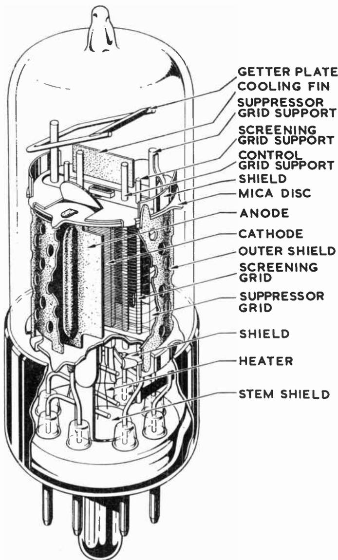
Fig. 105.—The construction of a modern valve; the example shown is a Mazda 6F1 screened pentode.
