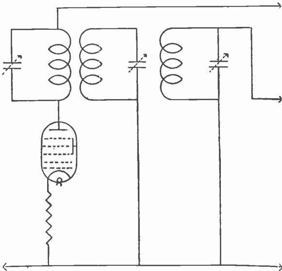
Fig. 136.—A triple-tuned circuit intermediate-frequency coupling.
