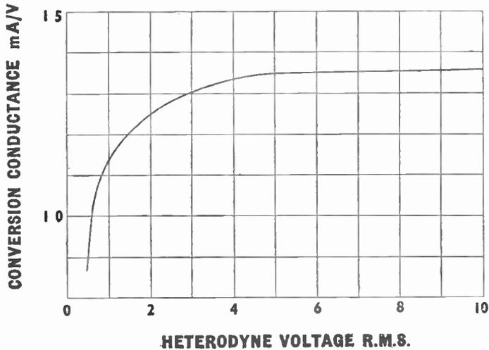
Fig. 127.—Curve showing the effect of heterodyne voltage (oscillator output) on the conversion conductance of the frequency-changing stage. The actual valve used to plot this curve was an indirectly heated triode hexode.
