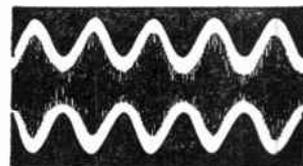
Fig. 88.—A drawing from an oscillogram of an amplitude modulated carrier wave. The individual cycles of the carrier have become merged owing to the small space between them.
