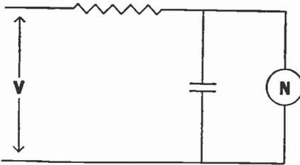
Fig. 3.—Basic circuit for measuring capacity with the aid of a neon lamp.
