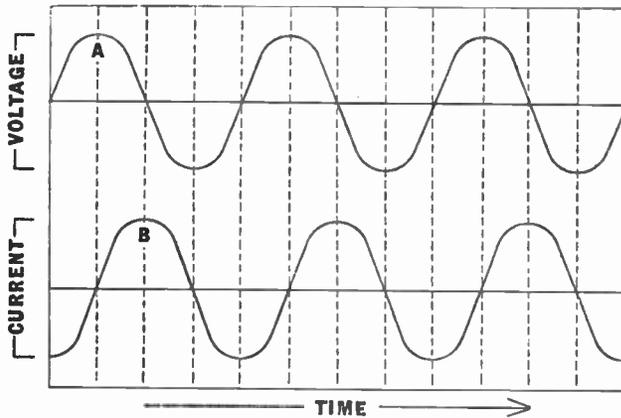
Fig. 52.—Each vertical division represents  $90^\circ$ , i.e.  $\frac{1}{4}$  cycle. This illustration shows the  $90^\circ$  current lag in a purely inductive circuit. As time is depicted as moving from left to right the current reaches its maximum at B after the voltage reaches its maximum at A.
