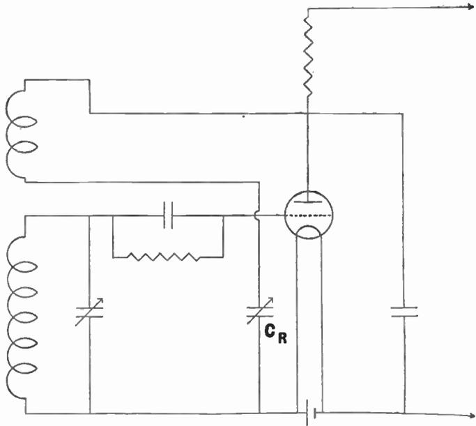
Fig. 103.—Detector circuit showing capacity-controlled magnetic reaction. A high-frequency choke is desirable between the anode resistance and reaction coil but is seldom used in practice.
