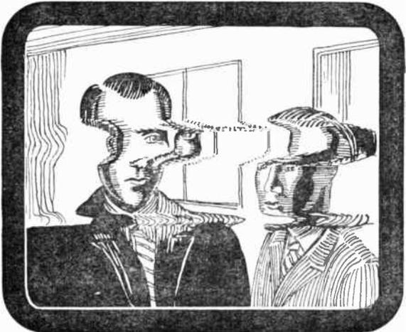
Fig. 111.—Another drawing which gives an idea of the effect resulting from an unstable line time base. Single lines or isolated groups of lines slip out of synchronism, with the result that a portion of the picture moves to the right, as shown.
