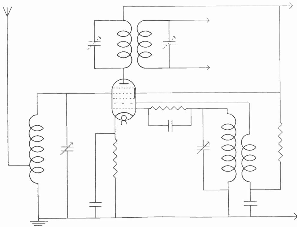
Fig. 122.—The basic circuit of a pentagrid frequency changer. Like all circuits in this chapter it is a skeleton circuit, and lacks certain necessary refinements.
