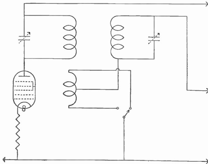
Fig. 131.—A method of obtaining two band widths.
