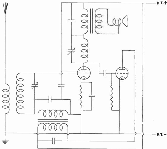
Fig. 95.—A typical reflex circuit.
