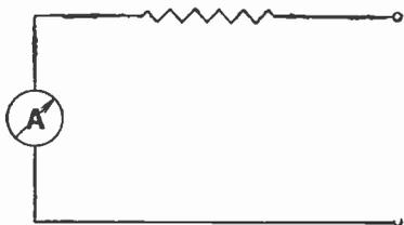
Fig. 6.—A series resistance to increase the range of a voltmeter or to enable voltage to be read with a milliammeter.
