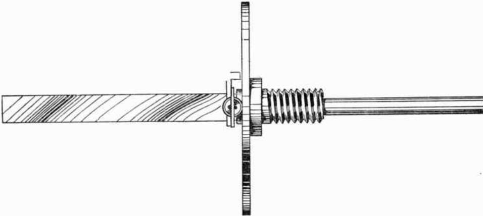
Fig. 143.—The control spindle and locating plate; the switch wafers are threaded on the flat "blade." Illustration three-quarters full size.
