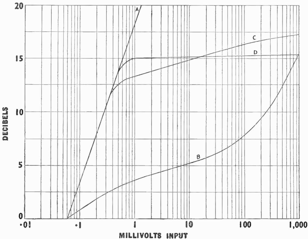
Fig. 178.—Performance curves of various automatic volume control systems.
