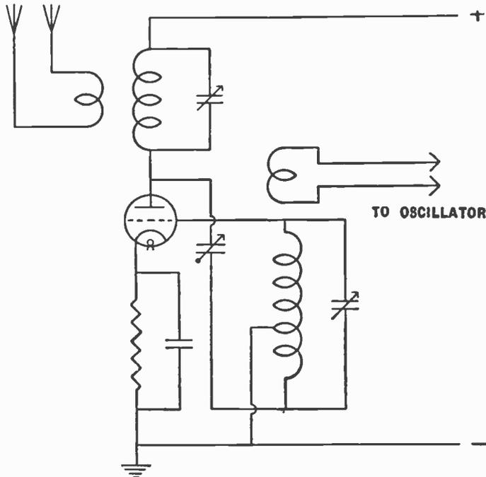
Fig. 61.—A typical high-frequency amplifier employing grid neutralisation.
