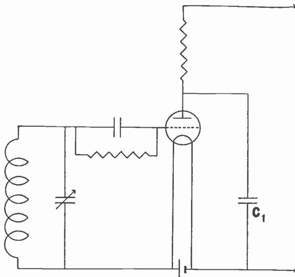
Fig. 101.—Amplitude modulation detector circuit showing the connection of a bypass condenser.
