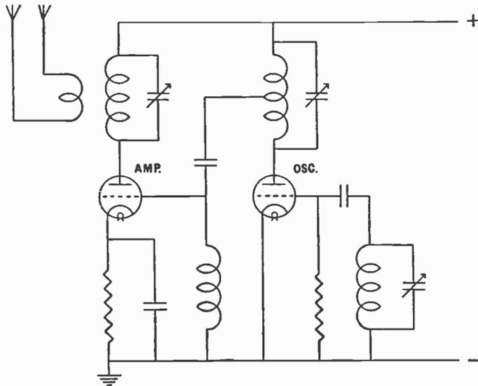
Fig. 57.—A straightforward high-frequency amplifying stage.
