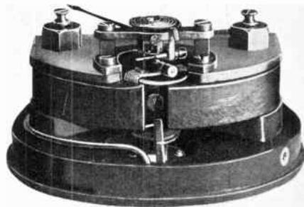
(*Above*) A typical moving-coil meter, showing the location of the moving coil between the poles of the circular permanent magnet.
