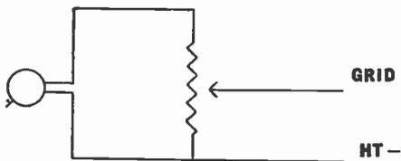
Fig. 24.—The normal connections for gramophone pick-up and volume control.
