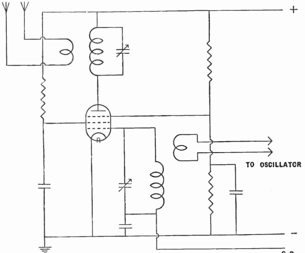
Fig. 60.—A high-frequency pentode as amplifier. It is desirable but not essential to apply a small positive bias to the suppressor grid.
