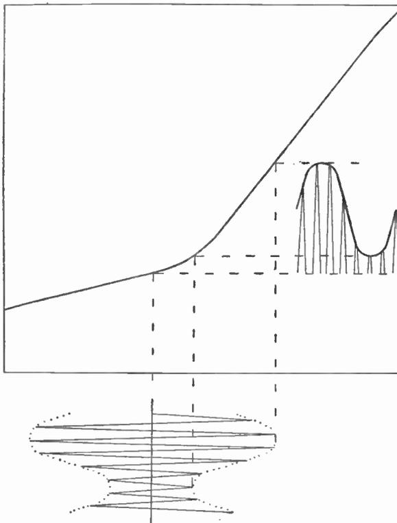
Fig. 93.—The same curve as at Fig. 91, showing the application of an amplitude modulated carrier and resulting audio-frequency waveform. The values of voltage and current are omitted in the interest of clarity, but may be obtained by reference to Fig. 91. The comparatively small audio waveform resulting from the negative half-cycle of the modulated carrier is omitted for the same reason.
