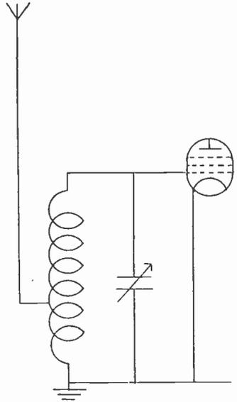
Fig. 110.—Auto-transformer aerial coupling.
