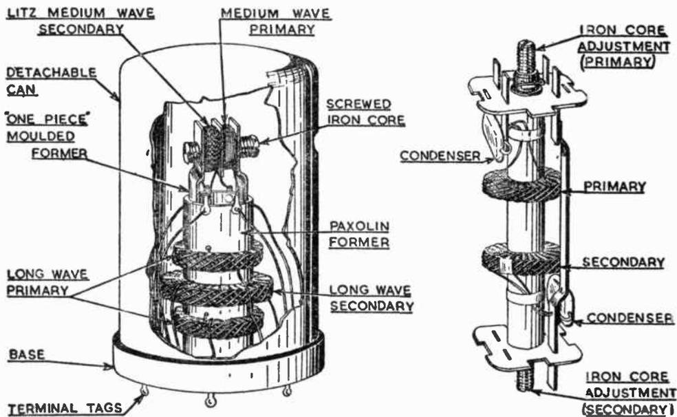
FIG. 138.—Typical coil assemblies. (Top) A compact oscillator coil unit. (Bottom, left) An older type 2 waveband H.F. transformer. (Bottom right) Modern I.F. transformer with screening can removed.
