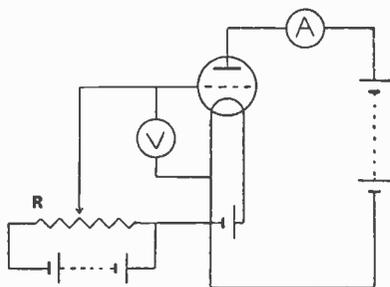
Fig. 79.—This circuit permits grid-volt characteristics to be plotted.
