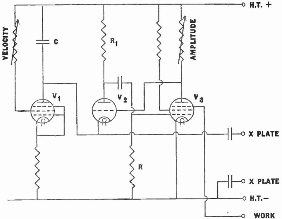
Fig. 19.—Basic circuit of a time base using high-vacuum valves. In acknowledgment of the engineer who introduced it, the circuit is often referred to as the Puckle time base.
