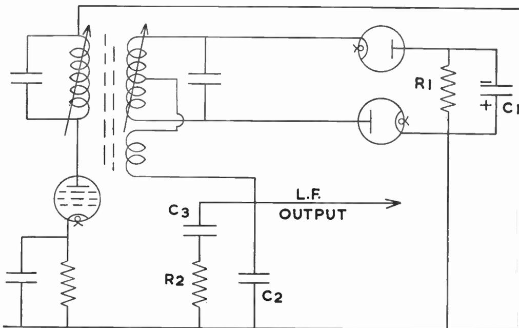
Fig. 204.—The ratio detector.
