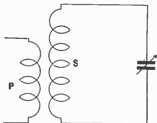
Fig. 70.—A tuned high-frequency transformer.
