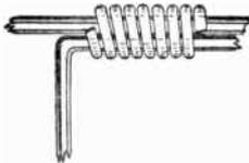
Fig. 72.—A connector used to facilitate soldering a joint between two wires.
