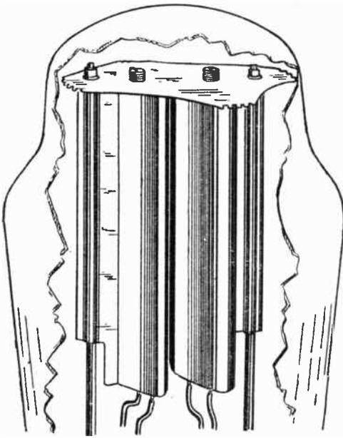
Fig. 1.—A full-wave rectifying valve.
