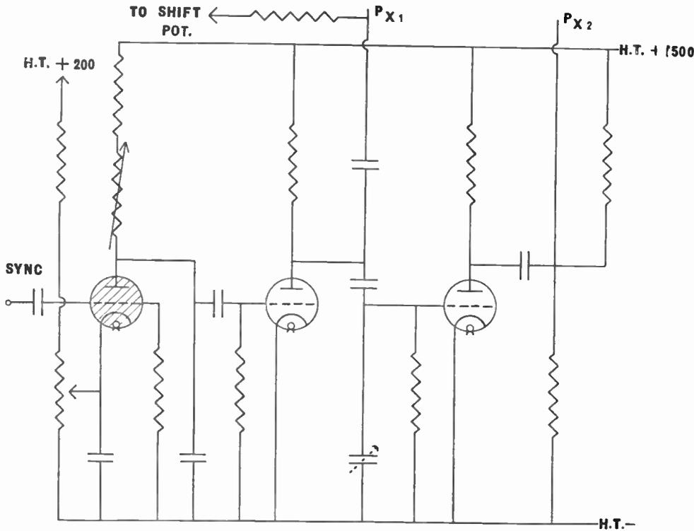
Fig. 95.—A relatively elaborate gas-discharge valve time base arranged for use with an electrostatically deflected cathode-ray tube. By using a separate push-pull amplifier, the initial sweep can be very small, thus allowing a high degree of linearity to be obtained.
