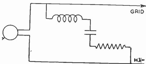
Fig. 25.—A typical top cut or scratch-filter circuit.
