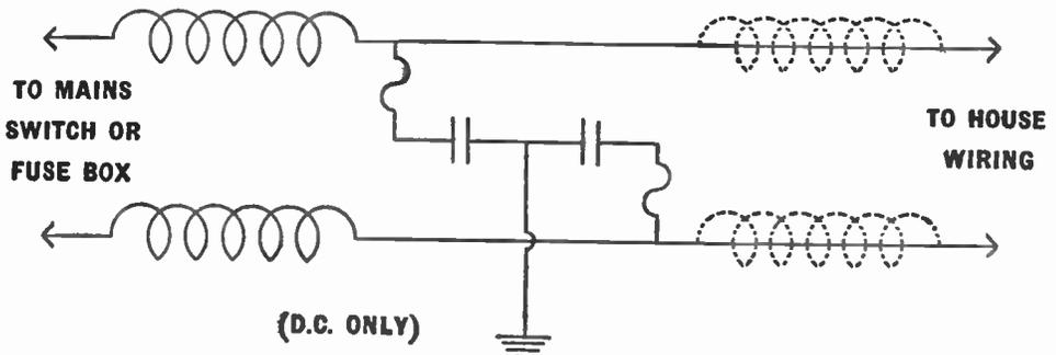
Fig. 59 —A more elaborate suppressor circuit for use on D.C. mains employing either two or four high-frequency chokes.
