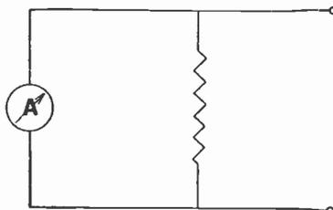
Fig. 5.—A simple shunt to increase the range of an ammeter or milliammeter.
