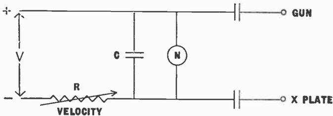
Fig. 14.—A neon-lamp time base. The illustration above shows the circuit of the simplest possible form of time base.
