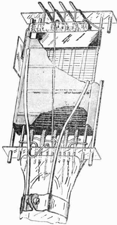
Fig. 164.—A typical directly heated output triode.
