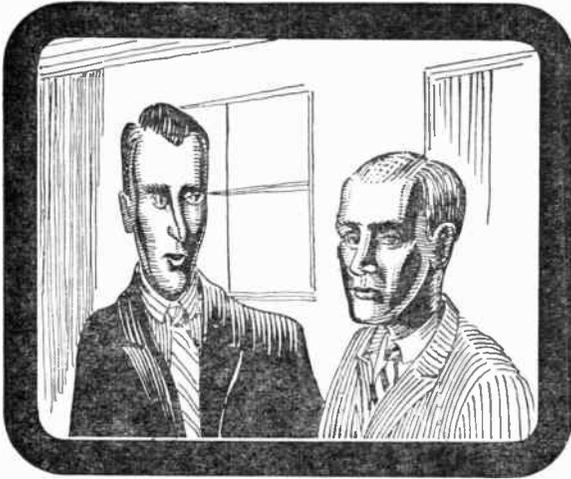
Fig. 109.—A drawing to illustrate the effect of bad line linearity. It will be observed that while the right-hand side of the picture is fairly normal, the left-hand side is progressively cramped.
