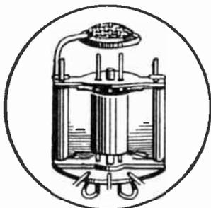
Fig. 93.—Electrode assembly of a "peanut" valve. The illustration is twice full size and the outer circle shows the proportionate size of a sixpenny piece.
