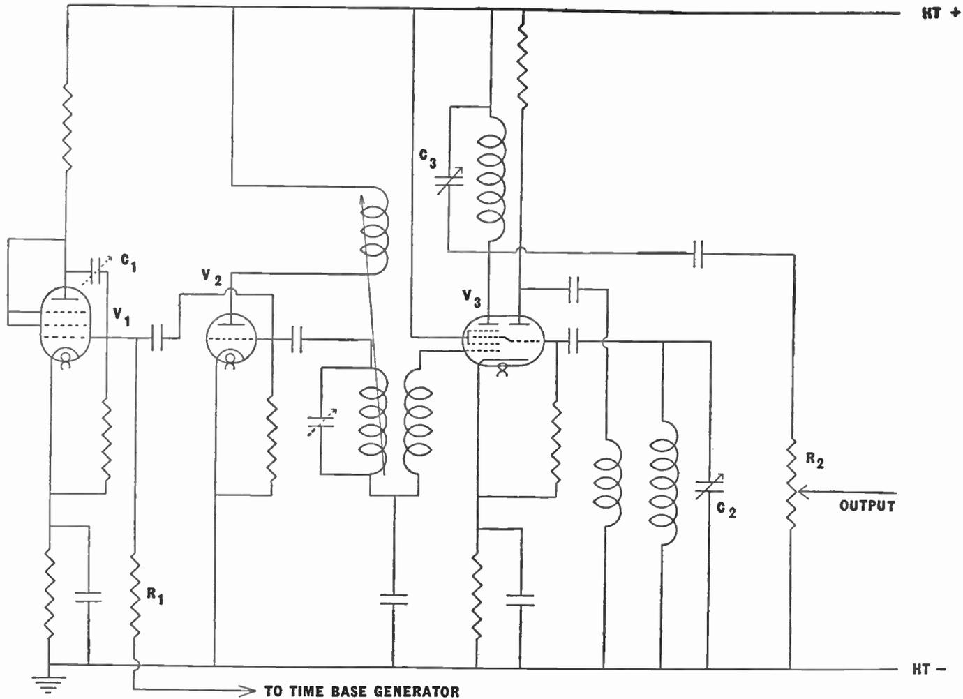
Fig. 10.— Basic circuit of a frequency-modulated oscillator suitable for use with an oscillograph for receiver alignment
