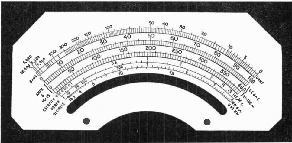
Fig. 4.—Scale of a typical multi-purpose moving-coil instrument.
