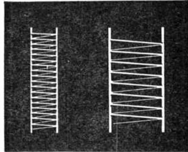
Fig. 84.—Sketch showing two grids taken from normal triode valves. Note the wide difference in mesh and width.
