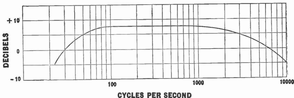
Fig. 26.—A response-curve where frequency distortion takes the form of attenuation at both ends of the audio scale.
