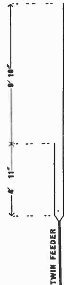
Fig. 108.—A dipole aerial with matching stub.
