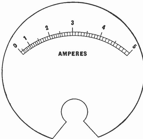
Fig. 1.—Scale of a typical moving-iron meter. Note particularly the non-linear division of the scale.
