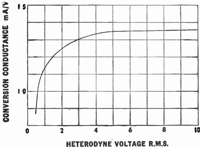
Fig. 48.—A curve showing the relationship between the heterodyne voltage and conversion conductance of a typical frequency changer.
