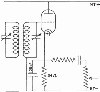
The infinite impedance detector. The volume control is usually about .5 megohm; the unmarked resistance is intended as a filter and is usually about 10,000 ohms; a suitable value for the blocking condenser is .1 mf.
