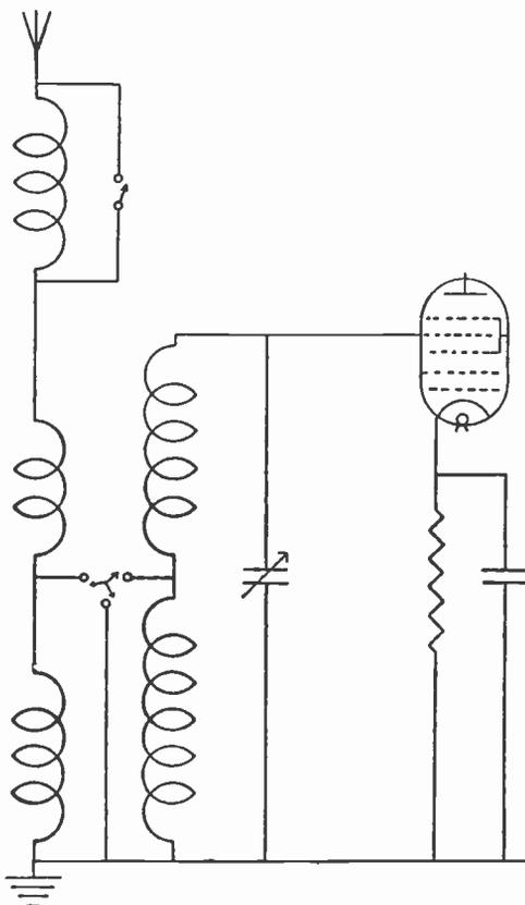
Fig. 137.—Input coupling using a choke in the aerial lead to suppress whistles on the long waveband.
