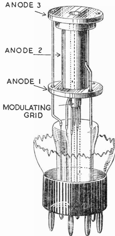
Fig. 69.—Electrode assembly of a typical magnetically focused and deflected cathode-ray tube. The heater and cathode are placed vertically in the centre of the modulating grid.
