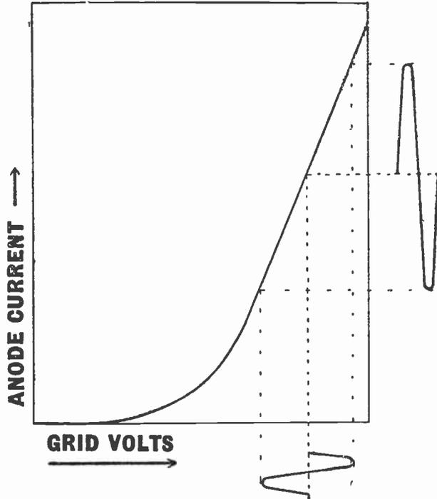
Fig. 81.—Showing an alternating voltage input and resulting alternating current output when valve is correctly biased.
