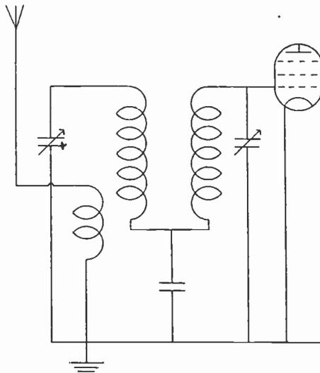
Fig. 112.—Capacity-coupled bandpass aerial coupling.
