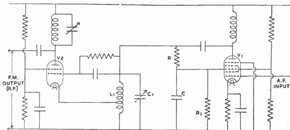
Fig. 207.—A typical reactance modulator circuit coupled to a simple oscillator.
