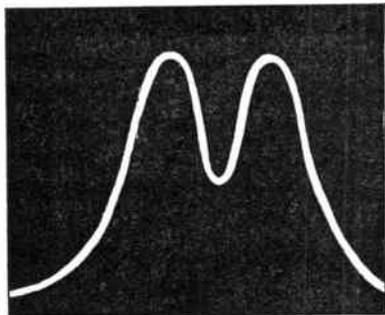
Fig. 46.—Incorrect adjustment. The response-curve is too wide, resulting in a very pronounced double hump.
