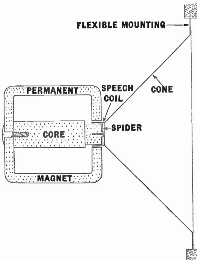
Fig. 171.—Simplified section of a permanent-magnet moving-coil loudspeaker ; the chassis has been omitted for simplicity but may be seen in Fig. 174.
