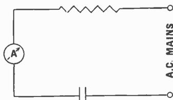
Fig. 54.—A method of determining the approximate capacity of a condenser. This arrangement must not be used for electrolytic types.
