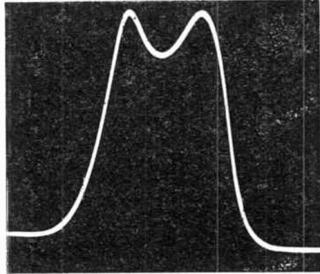
Fig. 71.—An oscillogram showing the frequency response of a bandpass filter.
