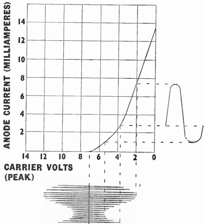
Fig. 98.—The principle of anode-bend detection.
