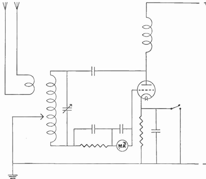
Fig. 52.—A modified oscillator using the Hartley principle.
