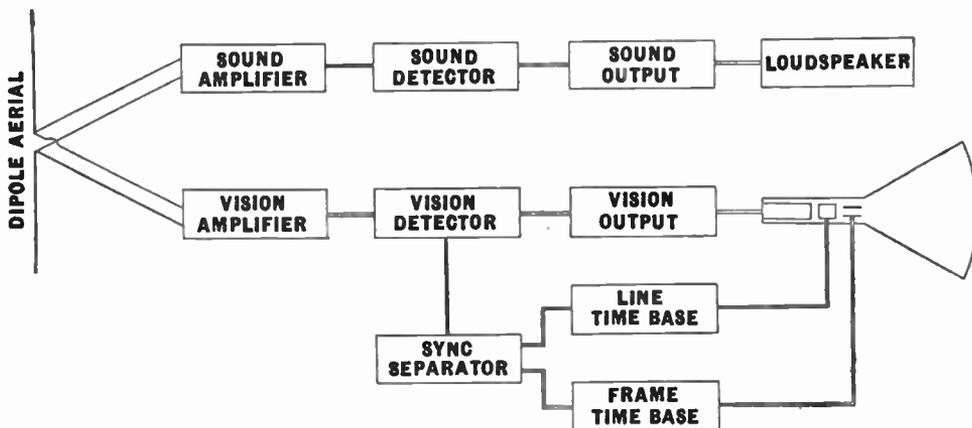
Fig. 98.—Diagram showing the various sections of a simple television receiver.
