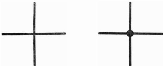
Fig. 82.—An entirely different convention: (left) wires crossing, (right) a junction.
