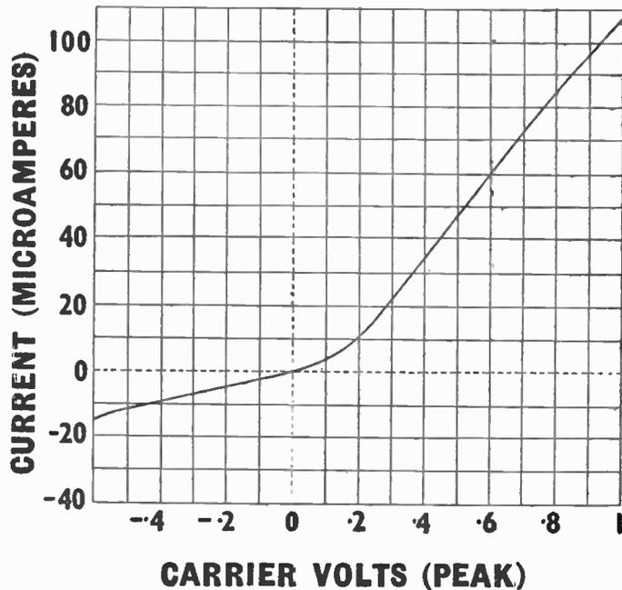
Fig. 91.—Characteristic curve of a crystal detector, showing the relationship between voltage and current.
