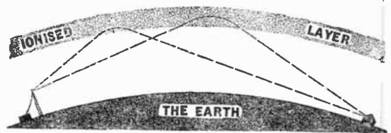
Fig. 18.—Variations in the density of an ionized layer sometimes cause two sky waves to impinge on the receiving aerial, resulting in particularly bad and erratic fading.
