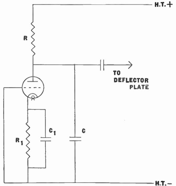
Fig. 78.—Diagram of an elementary time base, to illustrate the text.
