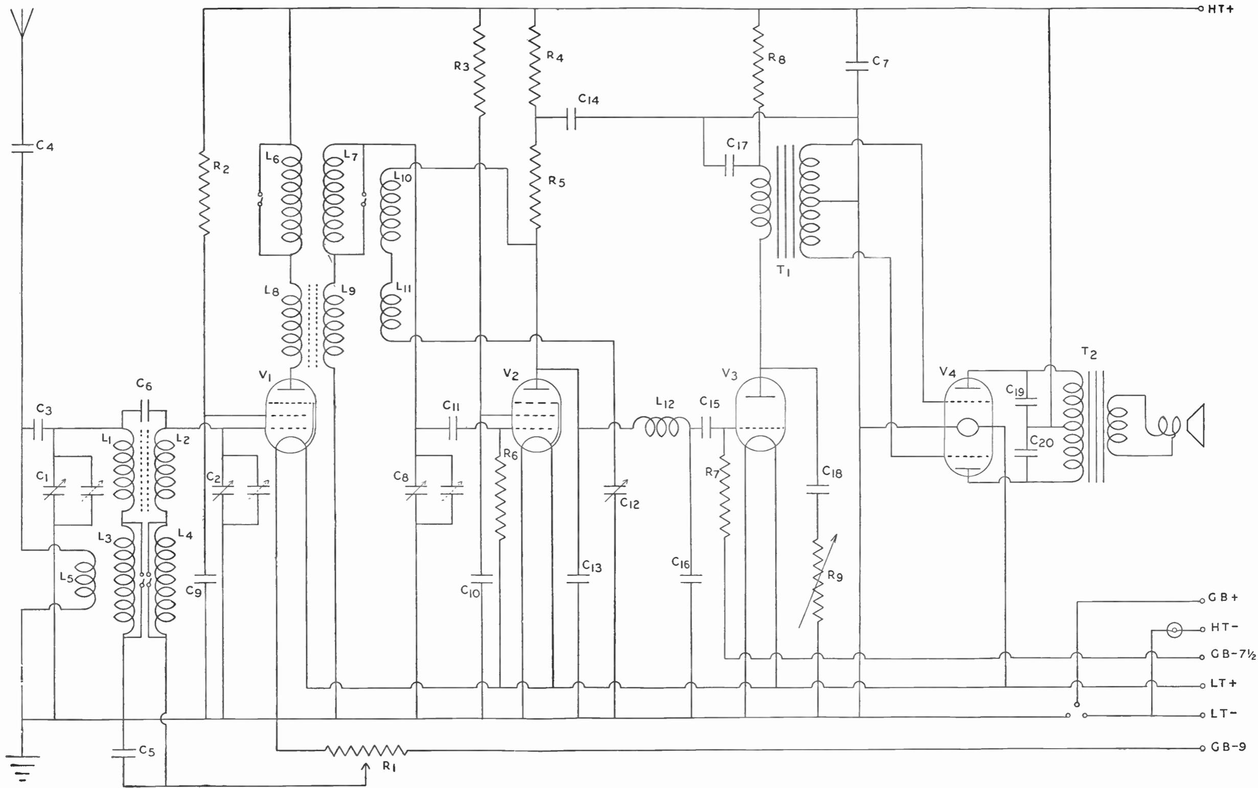
Circuit diagram of a four-valve battery receiver with a class B output. This type of receiver is popular in export markets.
