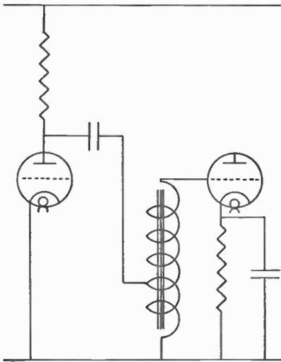
Fig. 153.—Resistance-fed auto-transformer coupling.
