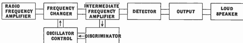
Fig. 199.—Block diagram of a superheterodyne with automatic-frequency control.
