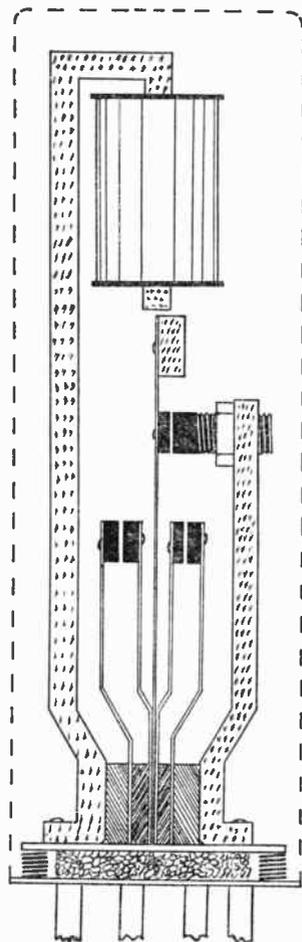
Fig. 42.—A simple vibrator. It will be noted that the whole assembly is mounted on springs which are mechanically damped by an inset of sponge rubber.
