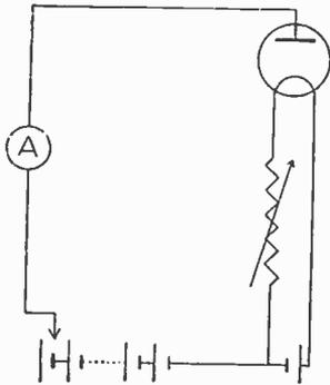
Fig. 73.—A diode valve arranged for plotting its characteristic curve.
