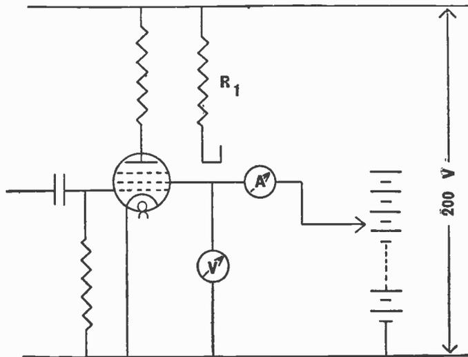
Fig. 24.—Circuit illustrating a suggested method of measuring the screen voltage in the circuit at Fig. 22.
