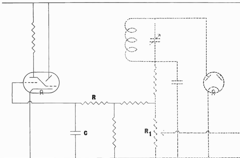
Fig. 190.—The complete circuit suggested for the "magic eye" fed from the anode of a diode detector.
