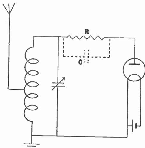
Fig. 94.—A simple circuit showing a diode as amplitude modulation detector.
