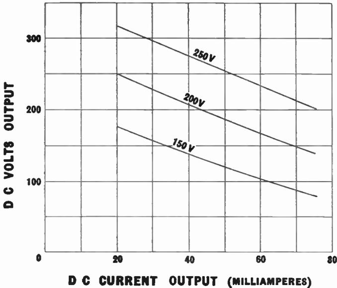
Fig. 3.—Performance curves for full-wave rectifier.
