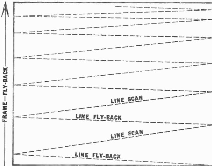
Fig. 86.—The frame fly-back following a scanning field which terminates in a complete line.
