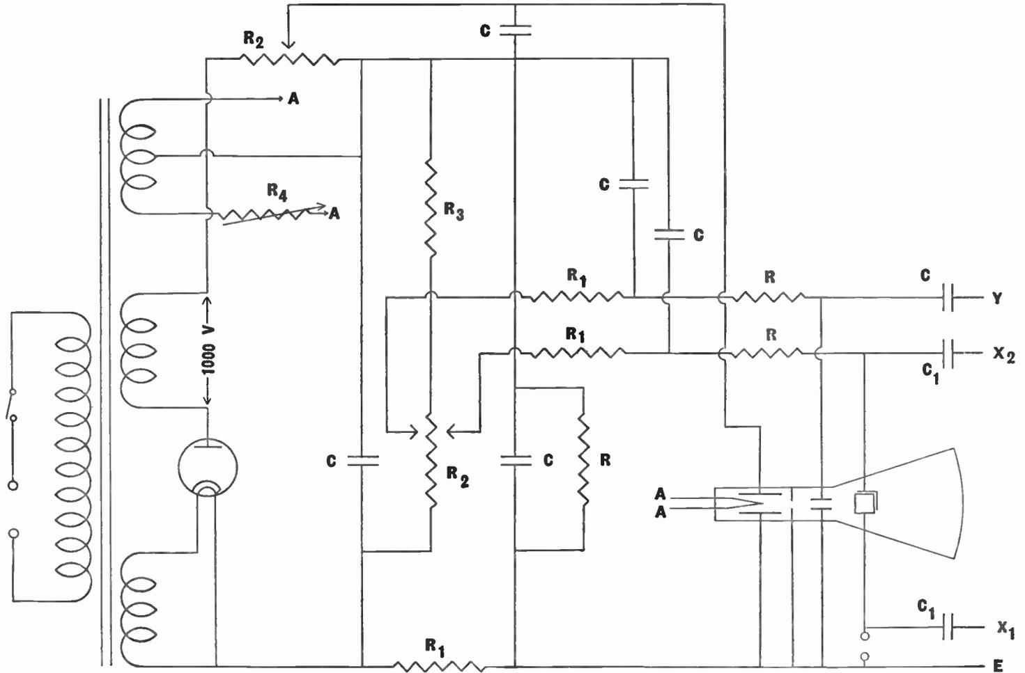
Fig. 21.—Circuit of a simple but useful oscillograph built by the author, using a gas-focused cathode-ray tube. The values are subject to some variation to suit different makes of tube.
