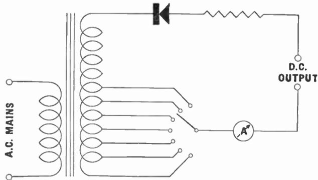
Fig. 74.—A simple accumulator charger using a metal rectifier.
