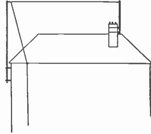
Fig. 33.—An L aerial mounted above the roof to give increased effective height.
