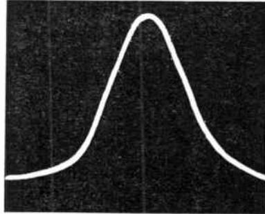
Fig. 43.—The intermediate-frequency amplifier for peak maximum response. It is important that the peak is in the centre of the screen.
