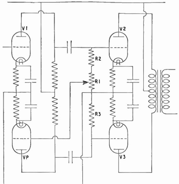
A very useful phase-splitting arrangement which offers a simple means of achieving balance.  $R1 + R2$  should equal  $R3$ ,  $R1$  being just large enough to give the required input to the paraphase valve  $Vp$ . This valve makes no contribution to the stage gain of the amplifier.
