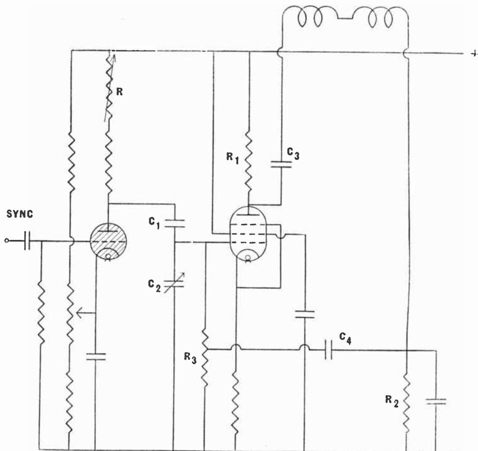
Fig. 92.—An improved arrangement of Fig. 91, employing a form of negative feed-back to correct linearity.
