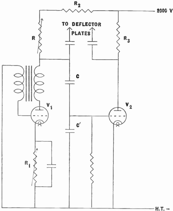
Fig. 80.—Circuit shown at Fig. 79, with an additional valve to obtain linearity. It should be noted that  $R$  and  $R_2$  together form the charging resistance.
