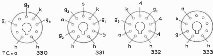
Note.—All connections are as viewed from underside of valve bases.
