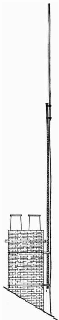
Fig. 35.—A vertical aerial mounted on a mast to increase the height.
