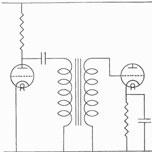
Fig. 151.—Resistance-fed transformer coupling.
