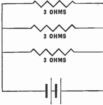
Fig. 30.—Three resistances in parallel.
