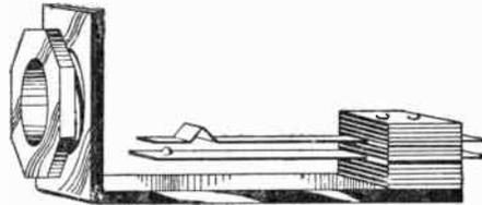
Fig. 90.—A typical example of a single-circuit jack.
