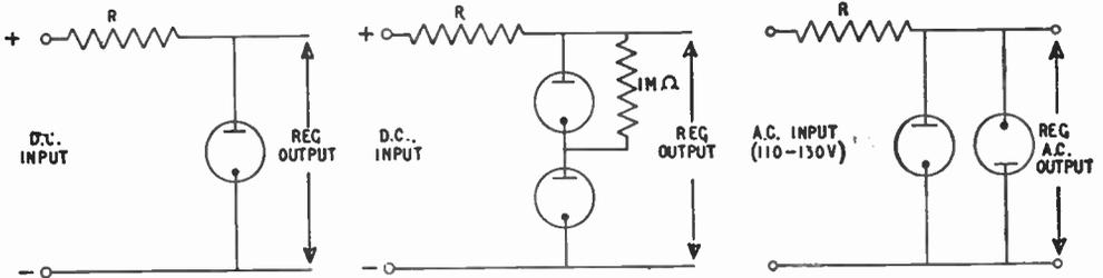
(Left) A simple circuit giving a sensibly constant voltage output irrespective of the current drawn within stated limits. Stabiliser tubes are made by various manufacturers, who publish curves from which the value of  $R$  may be determined. The controlled output voltage is usually 120/130 volts. (Right) In this arrangement two tubes are used to double the voltage output.
