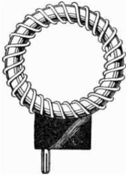
Fig. 96.—A toroidal coil.
