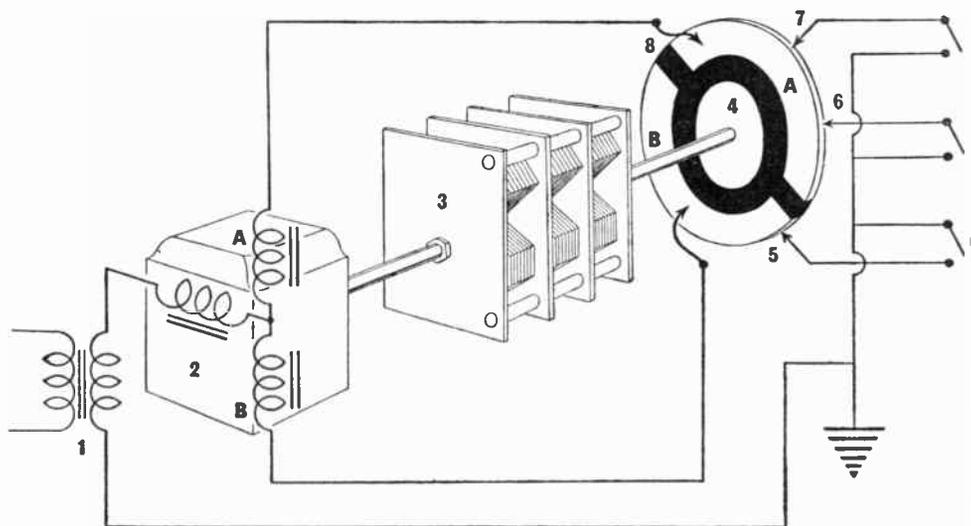
Fig. 198.—A composite illustration showing the principle of motor tuning using the direct-homing method.
