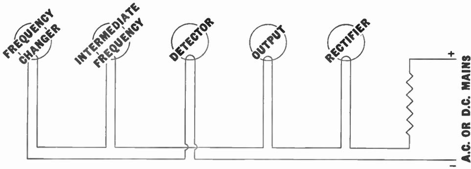
Fig. 9.—Suggested sequence for connecting heaters in a universal receiver.
