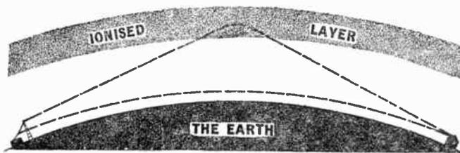
Fig. 17.—Under certain conditions both ground and sky wave will impinge on a receiving aerial and cause the phenomenon known as fading.
