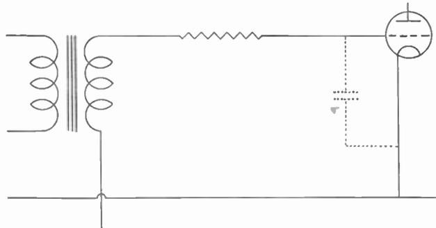
Fig. 20.—Circuit to illustrate the function of a grid stopper.
