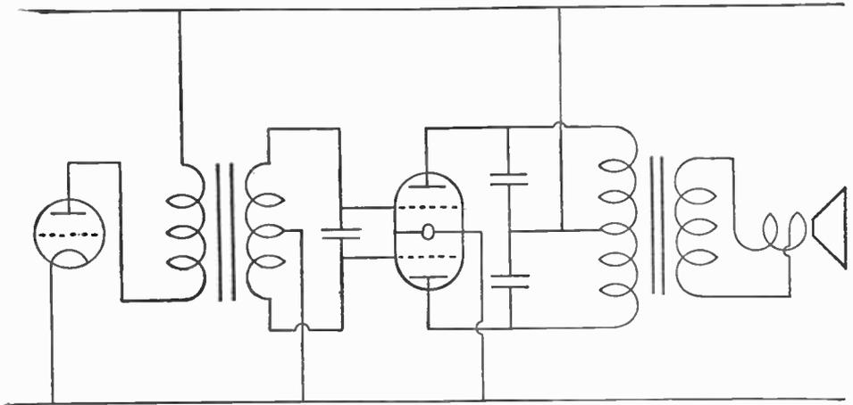
Fig. 162.—Basic circuit of a Class B output stage; special reference is made in the text to the condenser connected between the grids of the Class B valve.
