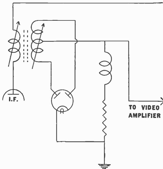
Fig. 99.—A typical vision detector.
