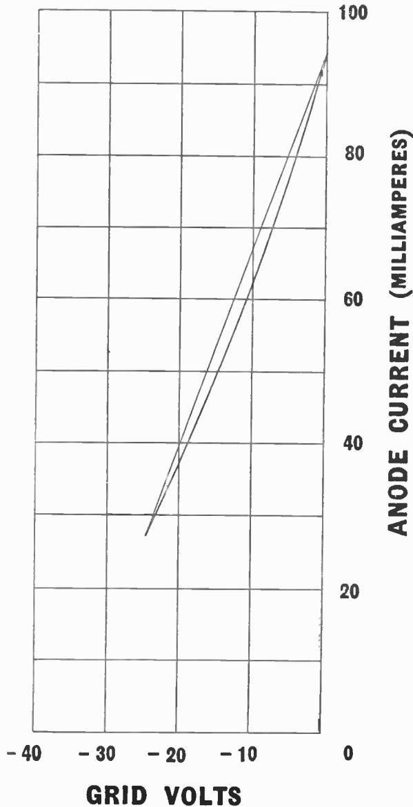
Fig. 155.—Dynamic curve of a triode output valve. Since this curve is taken from the valve under working conditions, it is limited to the portion actually operated by the input voltage. The straight line shows the theoretical condition of zero distortion.
