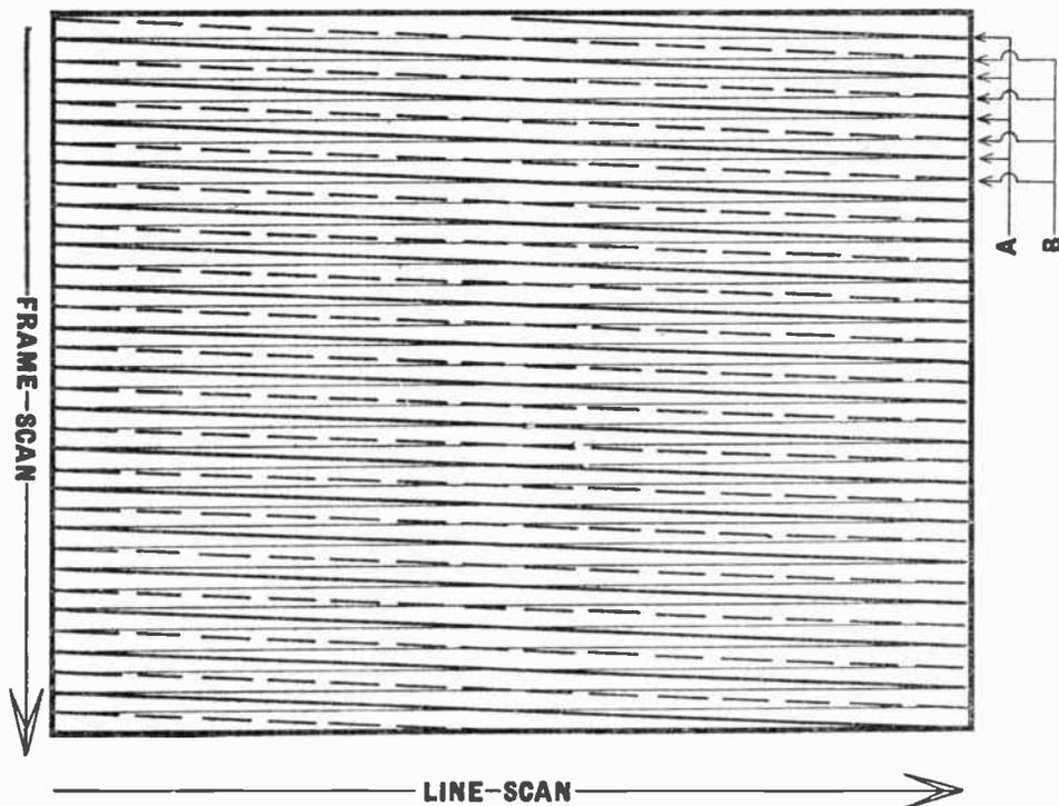
Fig. 85.—Two scanning fields, comprising lines marked A and B, which together form a complete interlaced raster.
