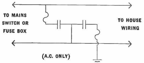
Fig. 58.—A simple suppressor circuit for use on A.C. mains.
