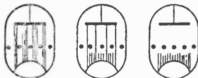
Fig. 78.—A purely imaginary sketch, showing the influence of the grid on the electron stream. (Left) Indicates no grid bias; (middle) shows the effect of moderate grid bias, while (right) shows that excessive grid bias will completely stop the flow of electrons to the anode.
