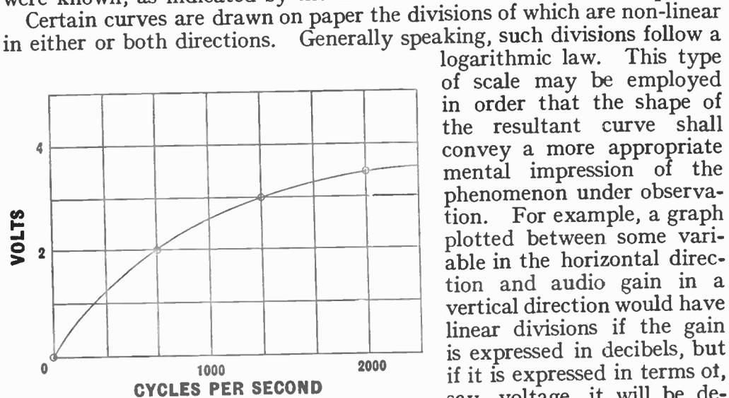
Fig. 78.—Second step in preparing a graph—joining up the points. It is essential that the number of points be adequate for the type of work.
