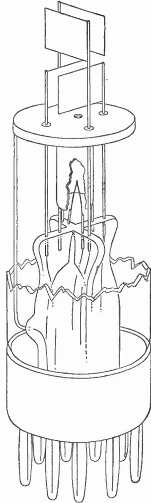
Fig. 12.—The electrode assembly of a typical gas-focused cathode-ray tube. The focusing shield is cut away to show the cathode, the circular aperture can be clearly seen in the dish-shaped gun. Note also the two pairs of deflector plates.
