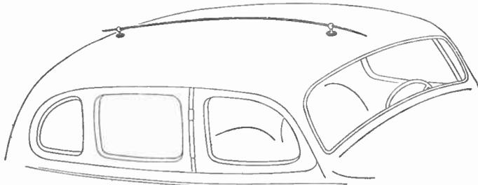
Fig. 44.—A roof aerial of the single-rod type.
