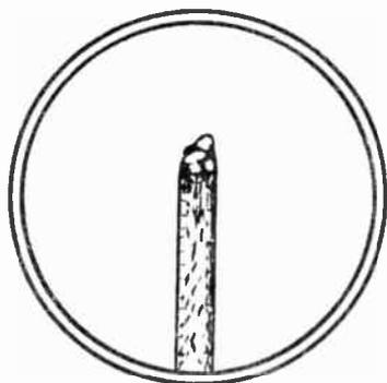
Fig. 36.—Sketch showing the appearance of a broken filament or heater (much enlarged).
