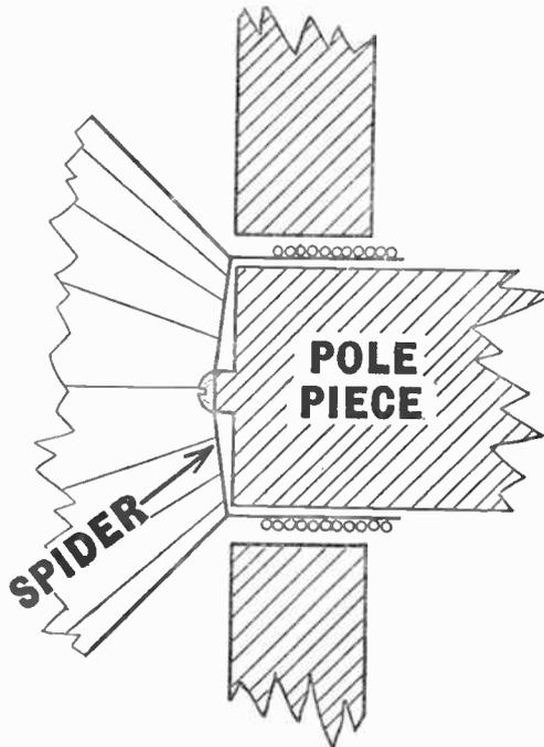
Fig. 51.—This illustration shows how a bent spider will cause the speech-coil to rest out of alignment with the magnet.
