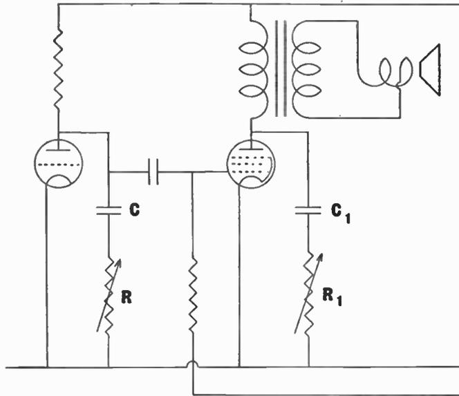
Fig. 159.—Alternative positions for variable tone control;  $R$  and  $C$  is preferable to  $R_1$  and  $C_1$ .
