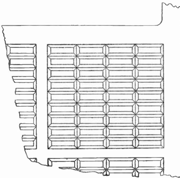
Fig. 24.—A corner of a typical accumulator plate showing the grid formation before it has been filled with lead paste.
