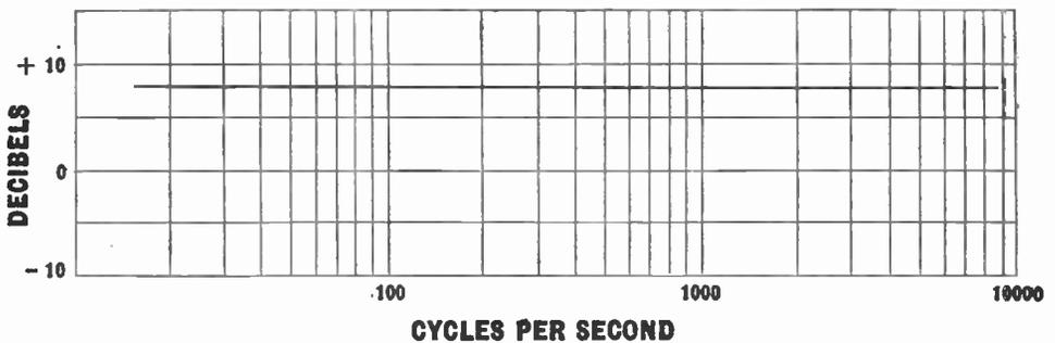
Fig. 25.—A theoretically perfect response-curve; frequency distortion is entirely absent.
