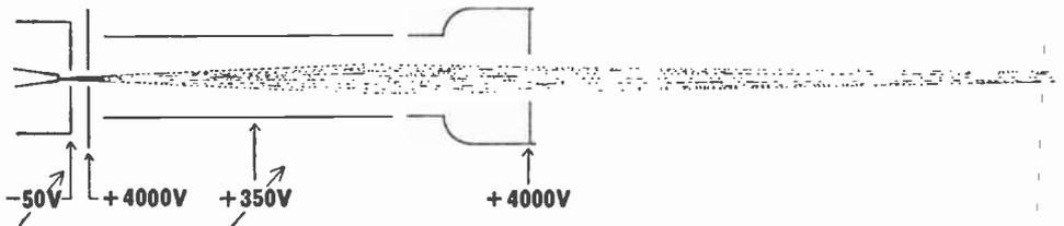
Fig. 70.—An impression of the focusing of an electron beam due to the varying fields of the anodes.
