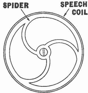
Fig. 172.—A typical "spider."
