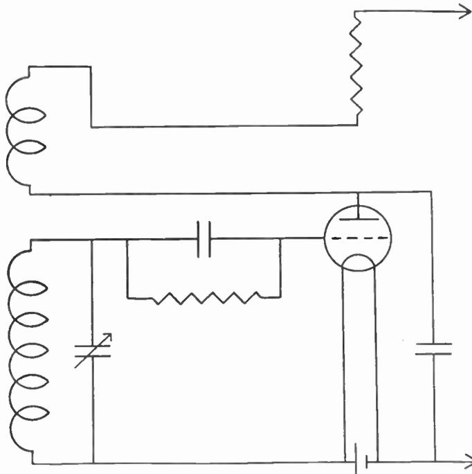
Fig. 102.—A typical amplitude detector circuit with magnetic reaction. The degree of reaction is varied by the coupling between the reaction and grid coils.
