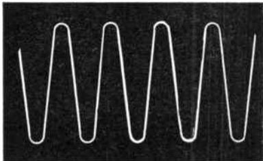
Fig. 41.—If the oscillator is fitted with low-frequency modulation, this can be used in the preliminary stage, as it makes the first sign of deflection much more apparent and appears as shown above.
