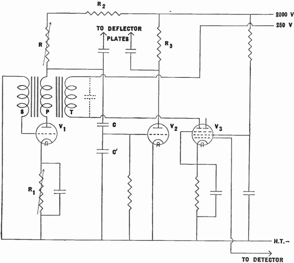
Fig. 81.—A complete time base for either line or frame, with synchronising separator valve.
