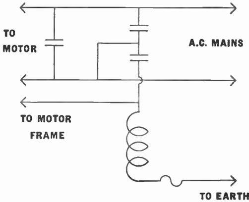
Fig. 63.—A suppressor circuit suitable for use with a repulsion-type motor. It is also useful for use on D.C. motors, in which case connection is made to the brushes.
