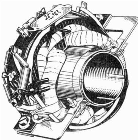
Fig. 75.—A typical deflector coil assembly, note that it carries small components.
