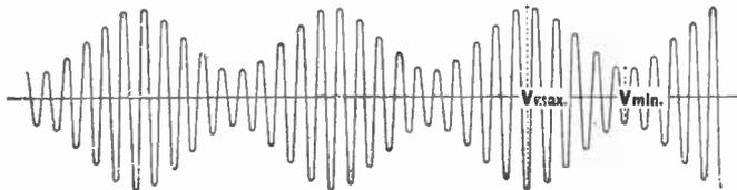
Fig. 87.—An amplitude modulated carrier. Each peak is offset by a trough, with the result that the mean amplitude is zero.
