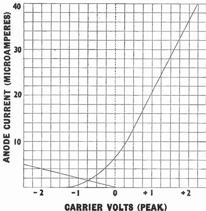
Fig. 95.—Emission curve of a diode.
