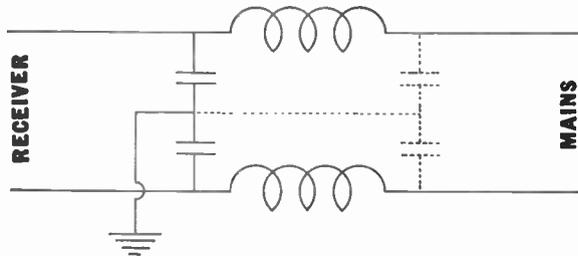
Fig. 10.—A simple mains filter. The dotted section indicates alternative or additional connections.
