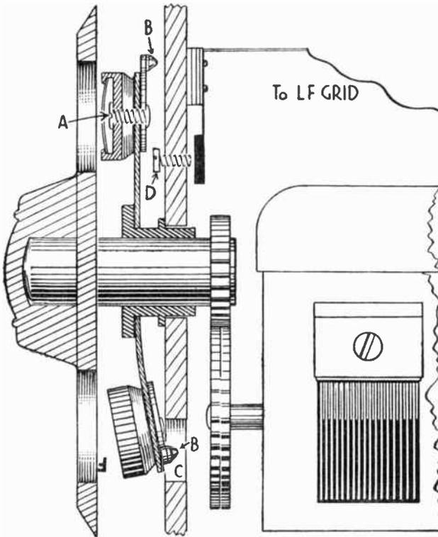
Fig. 196.—Semi-section of the teledial automatic tuning system. Note that the pegs on the perimeter of the buttons do not touch the back-plate until depressed.
