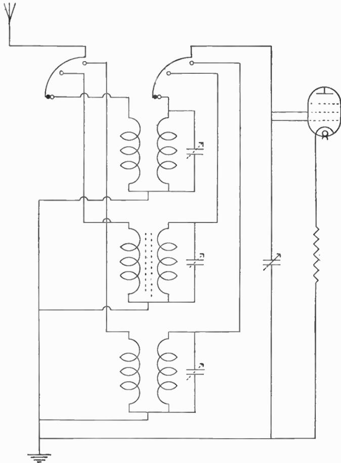
Fig. 147.—Three-band aerial circuit switched by means of a two-pole, three-way wafer switch.
