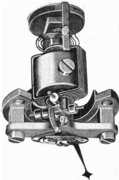
(*Left*) An enlarged view of the moving mechanism shown right. This photograph shows clearly the moving coil, the two hair-springs and balance-weights. It should be understood that the heavy top assembly, the structure inside the coil and the base are stationary. This photograph is about twice natural size.
