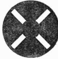
Fig. 184.—Appearance of the "magic eye" under conditions of no signal.
