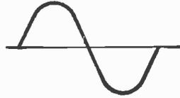
Fig. 2.—One complete cycle; a series of cycles form a wavetrain such as that shown at Fig. 1.
