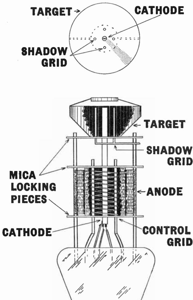
Fig. 186 (*Lower drawing*).—A broadside view of the "magic eye," with target and anode cut away to show the shadow grid and control grid respectively.
