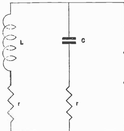
Fig. 67.—A symbolic representation of a parallel-tuned circuit.
