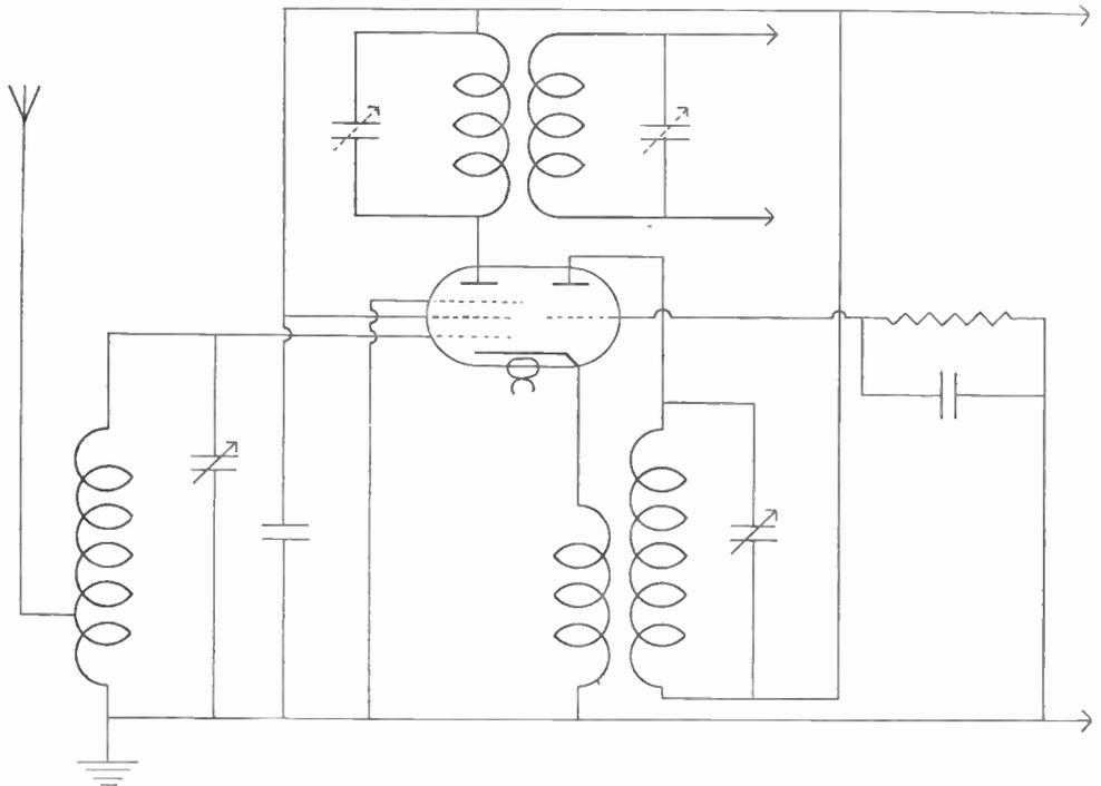
Fig. 126.—Basic circuit of a triode pentode frequency changer. That shown is an indirectly heated valve. Considerable modification is necessary when using a battery type.
