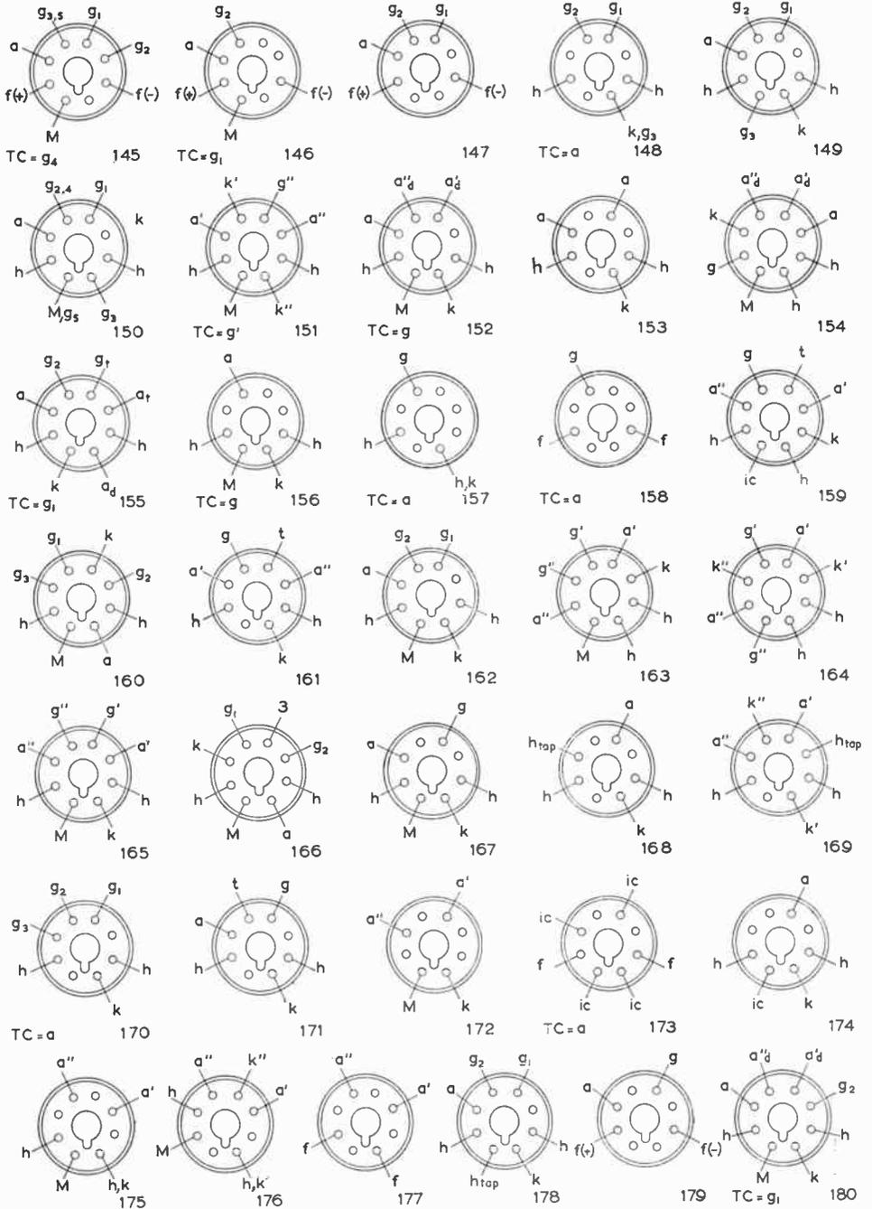
*Note.*—All connections are as viewed from underside of valve bases.
