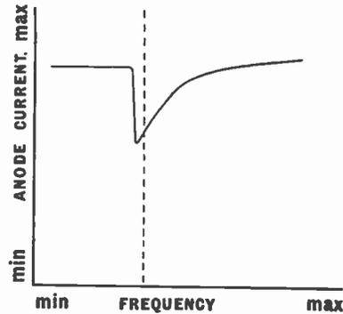
Fig. 55.—The relationship between frequency and anode current of a normal oscillator.
