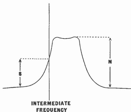
Fig. 30.—An exaggerated drawing, showing the decrease of signal to noise ratio resulting from misalignment. N represents the response to noise and S the response to the signal.
