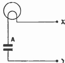
Fig. 53.—A lamp in series with a condenser. In suitable circumstances the lamp will light if an A.C. potential is applied across XY.
