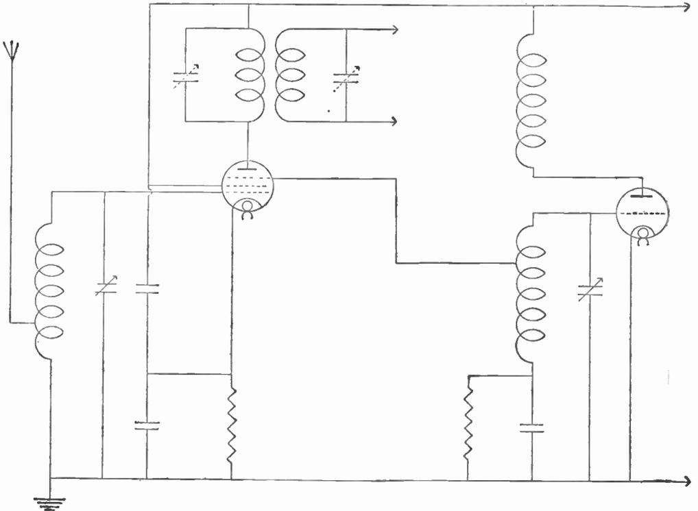
Fig. 119.—Basic circuit showing the use of an ordinary triode and pentode valve to form a frequency-changing stage. This circuit is not recommended, but is included to illustrate the text.
