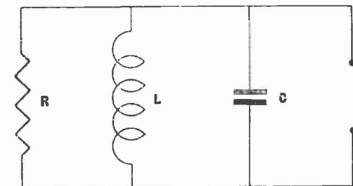
Fig. 68.—In this diagram  $L$  and  $C$  represent pure inductance and capacity and  $R$  symbolises the dynamic resistance.
