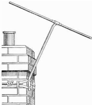
Fig. 208.—A Simple dipole for V.H.F. reception.
