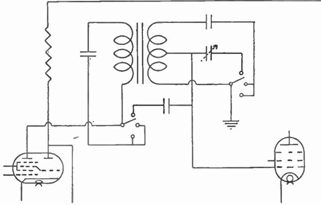
Fig. 31.—A special type of intermediate-frequency coupling, giving alternative intermediate frequencies.
