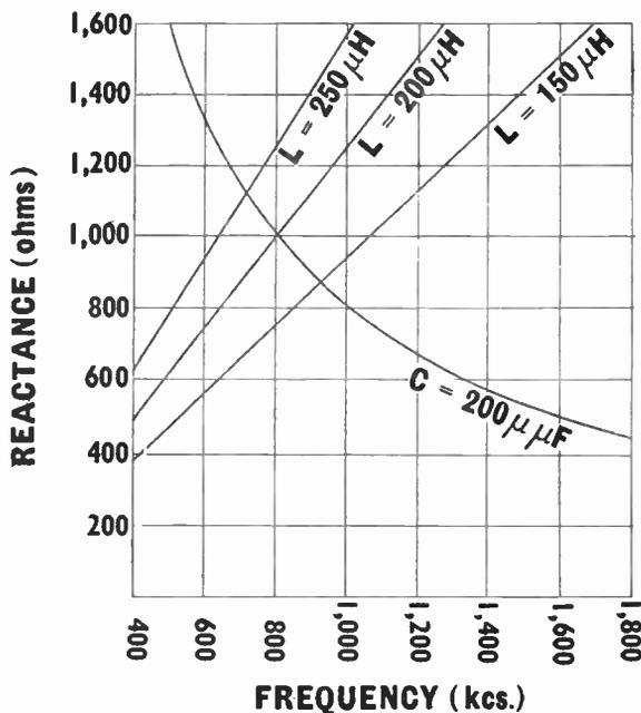
Fig. 65.—The reactance over a range of frequencies of three values of inductance and one value of capacity can be read from this graph.
