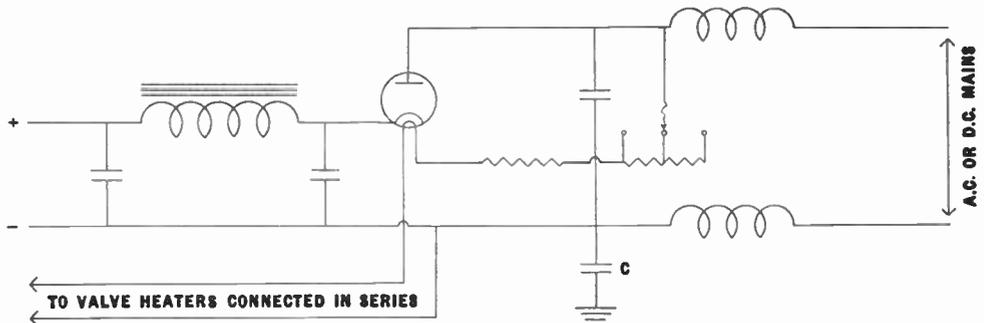
Fig. 8.—Basic circuit of a universal receiver mains pack; the tapped resistance permits adjustment to suit various mains voltages. It will be noted that the rectifier must be of the indirectly heated type.
