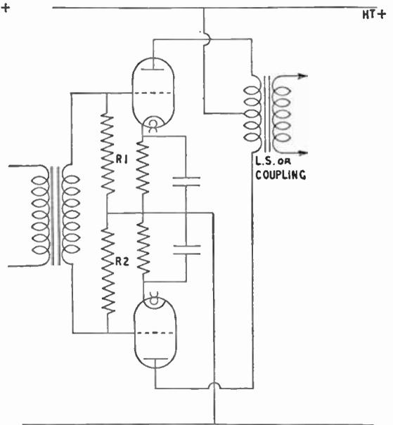
A variation of the circuit (left) sometimes advocated when a centre-tapped transformer is not available; it is a bad arrangement, since the value of  $R1 + R2$  divided by the square of the transformer ratio appears as a reflected load in the anode circuit of the preceding valve.
