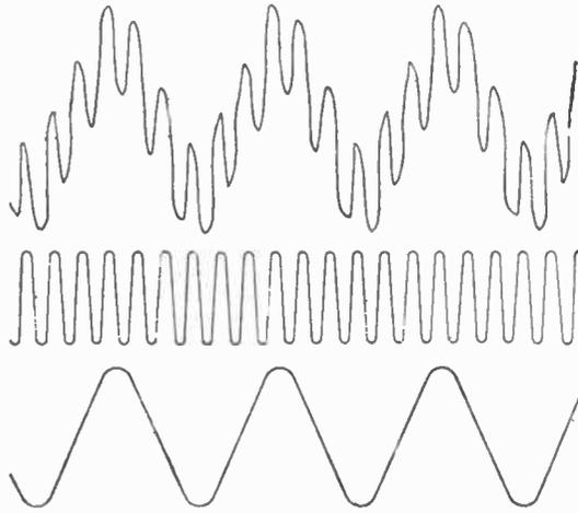
Fig. 9.—The top waveform is simply the lower two waveforms combined and illustrates that highly complicated waveforms, such as those shown at Figs. 3-8, are made up of two or more simple waves.
