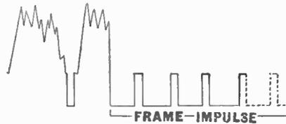
Fig. 88.—Frame impulse terminating a scanning field which ends with a half-line.
