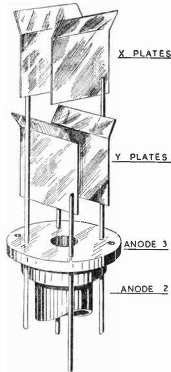
Fig. 71.—The arrangement of deflector plates in a typical electrostatic cathode-ray tube.
