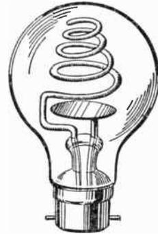
Fig. 92. — A type of neon lamp that is equally adaptable for simple time bases or domestic purposes.
