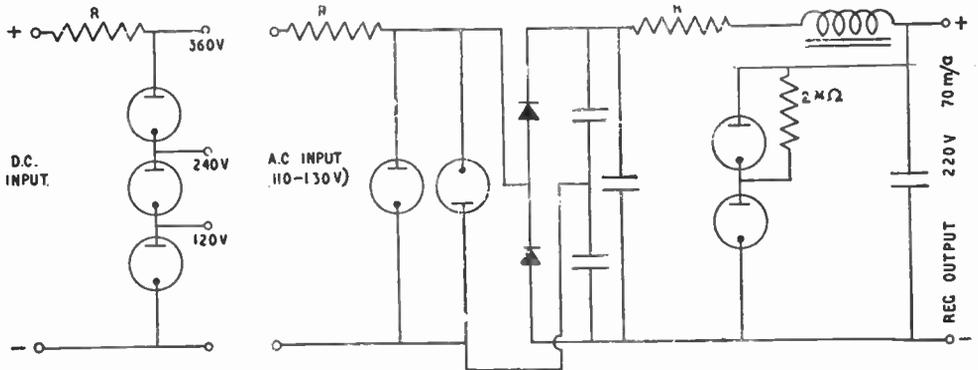
Stabiliser tubes arranged as a voltage divider. This circuit is only suitable where current drawn from the 120-V and 240-V tapplings does not exceed about 2mA each.
