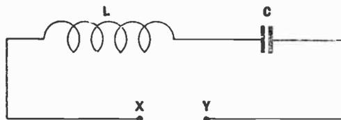
Fig. 63.—Inductance and capacity in series.
