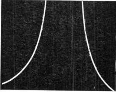
Fig. 42.—When the trimmers are brought more nearly to the correct positions deflection will usually be so large that only a portion is visible. The input is then reduced so that the complete trace is visible as shown in Fig. 43.
