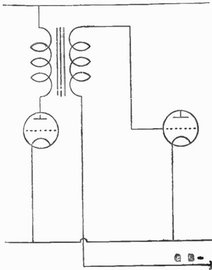
Fig. 150.—Transformer coupling for directly heated battery valves using battery grid bias.
