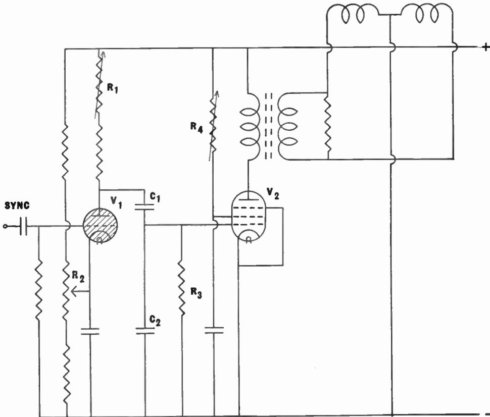
Fig. 91.—A simple circuit using a gas discharge valve and arranged for use with a magnetically deflected cathode-ray tube.
