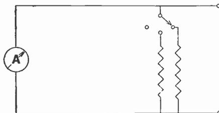
Fig. 7.—The *incorrect* method of switching shunts; the resistance of the switch is in the actual shunt circuit and may introduce considerable error.
