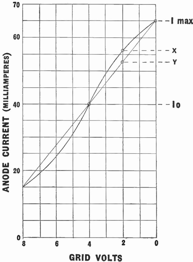
Fig. 167.—The text describes how the third harmonic distortion can be calculated from data obtained from the above drawing.
