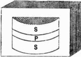
Fig. 45.—A simple transformer; the primary is between the split secondary winding.
