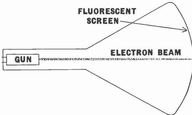
Fig. 68.—A sketch illustrating the fundamental principles of a cathode-ray tube.
