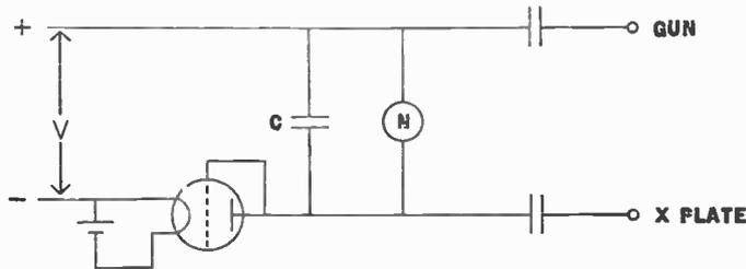
Fig. 15.—An improved form of time base in which a saturated diode is used to improve linearity.
