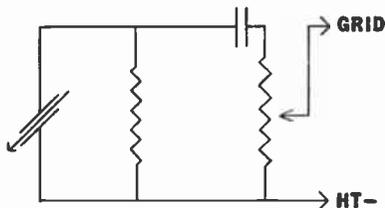
Fig. 22.—A circuit to isolate a crystal pick-up. This illustration shows the conventional symbol for this type of pick-up.
