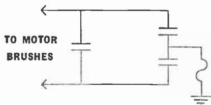
Fig. 62.—A slightly improved suppressor circuit for use with a small D.C. motor.
