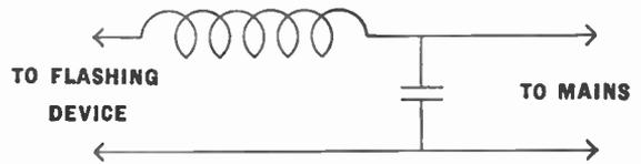
Fig. 64.—A simple circuit for suppressing a make-and-break device. Also suitable for suppressing an electric bell.
