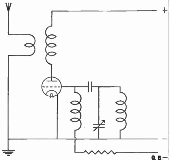
Fig. 50.—A modified oscillator circuit allowing grid bias to be obtained from a D.C. source.
