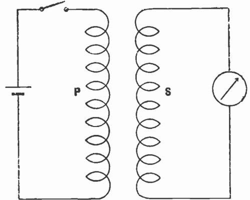
Fig. 44.—When the switch is closed or opened a current will flow in coil "s."
