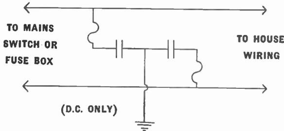
Fig. 57.—A simple suppressor circuit for use on D.C. mains; the fuses shown in this and other diagrams in this chapter are optional.
