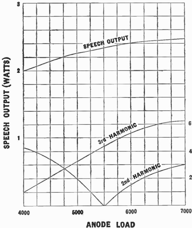
Fig. 158.—Curves showing the relationship between anode load and speech output, second harmonic distortion and third harmonic distortion. The valve used was a pentode having an anode dissipation of 8 watts.
