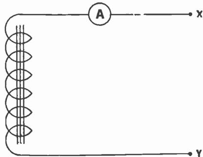
Fig. 51.—This illustration shows diagrammatically an iron-cored coil in series with an ammeter.
