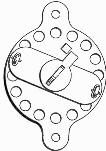
Fig. 144.—The locating plate of a wafer-switch assembly.
