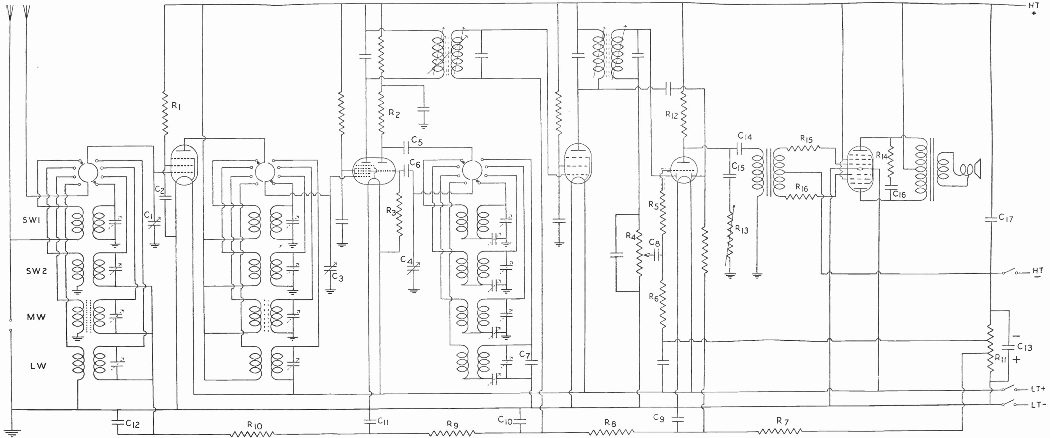
Circuit diagram of a four-band battery receiver with quiescent push-pull pentode output. In common with all circuits in this chapter, this diagram is intended purely to illustrate various points made in the accompanying text.
