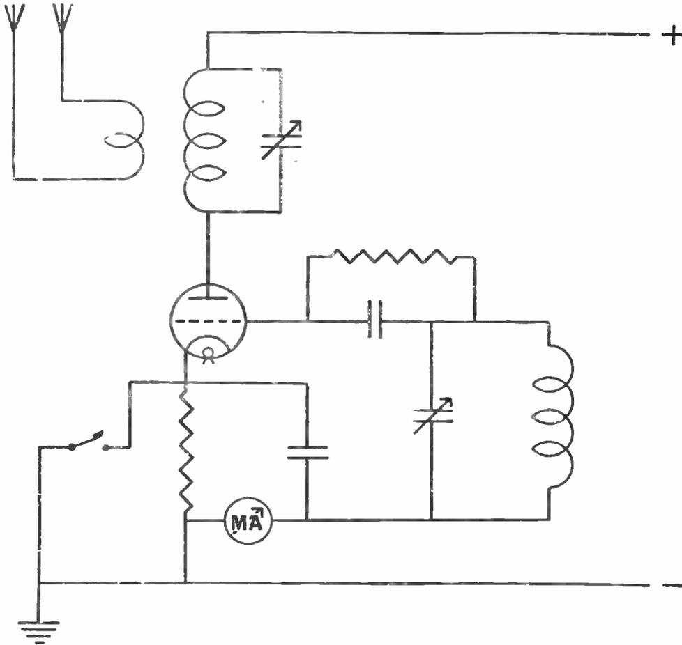
Fig. 51.—A very simple, but nevertheless complete, transmitter. The method of keying is not recommended for practical purposes.
