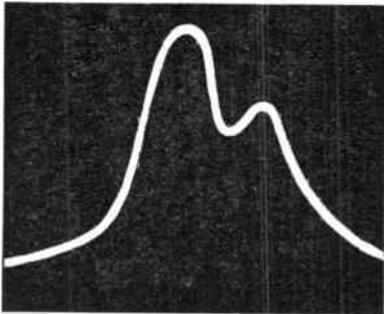
Fig. 44.—By suitable adjustment of the trimmers an effort is made to flatten the top of the response-curve. (Operation not yet complete.)
