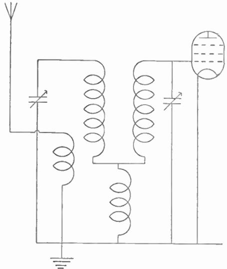
Fig. 114.—Inductively coupled bandpass aerial coupling.
