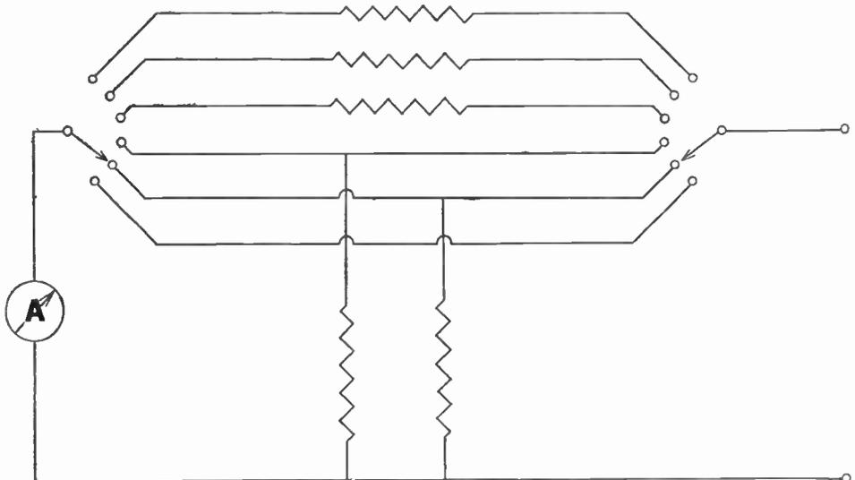
Fig. 9.—An arrangement by which a single meter measuring from 0–1 milliampère and having an internal resistance of 45 ohms may be used for three current ranges and three voltage ranges. It is essential for the switches to be ganged.
