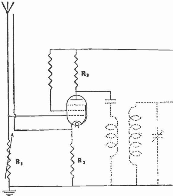
Fig. 39.—The circuit arrangement of a local interference suppressor, which utilises the phase-reversing properties of a valve.
