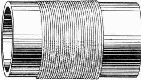
Fig. 139.—A typical single-layer coil.
