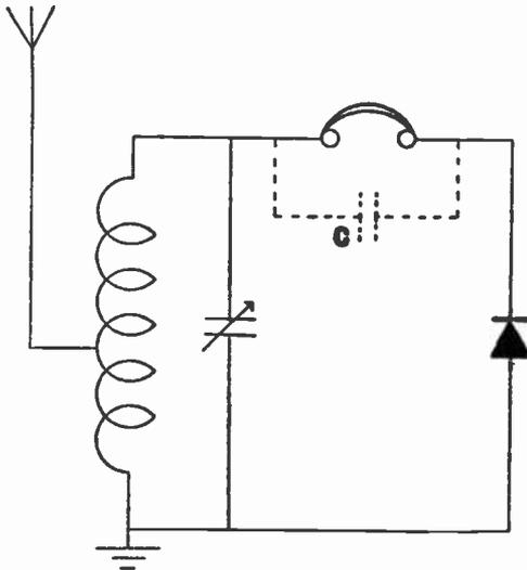
Fig. 92.—The circuit of a simple crystal detector.
