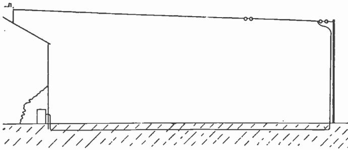
Fig. 56.—An anti-static aerial erected remote from the house.
