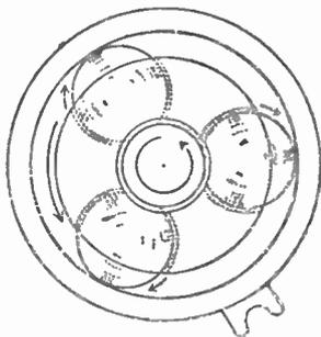
Fig. 28.—A diagrammatic illustration of a planetary gear. The arrows show the relative direction of rotation of the three main units; the outer ring is stationary.
