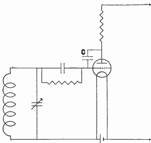
Fig. 99.—A simple detector circuit to emphasise the capacity between anode and grid of a triode valve.
