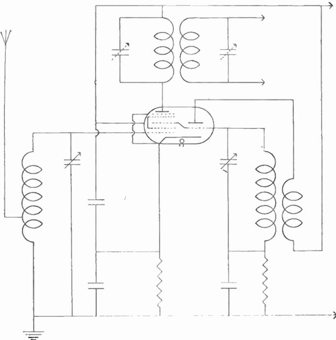
Fig. 125.—A basic circuit using a triode heptode for frequency changing.
