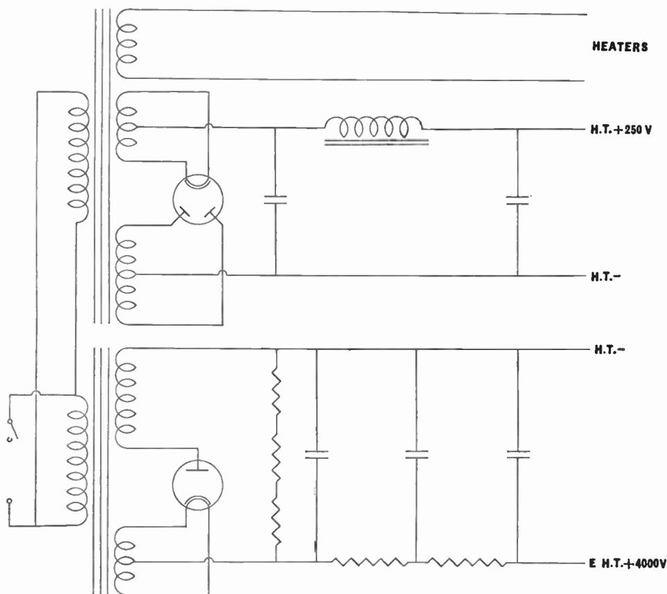
Fig. 102.—Circuit of a power pack for supplying a vision receiver.
