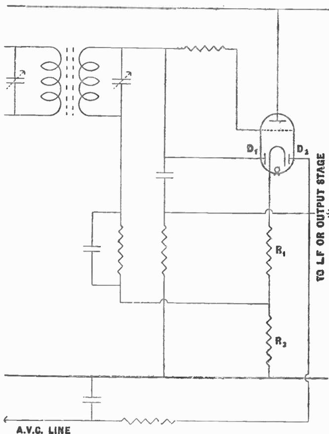
Fig. 193.—An improved Q.A.V.C. circuit. Note particularly that the valve performs the function of detection, noise suppression, and automatic control. The triode section does not amplify.
