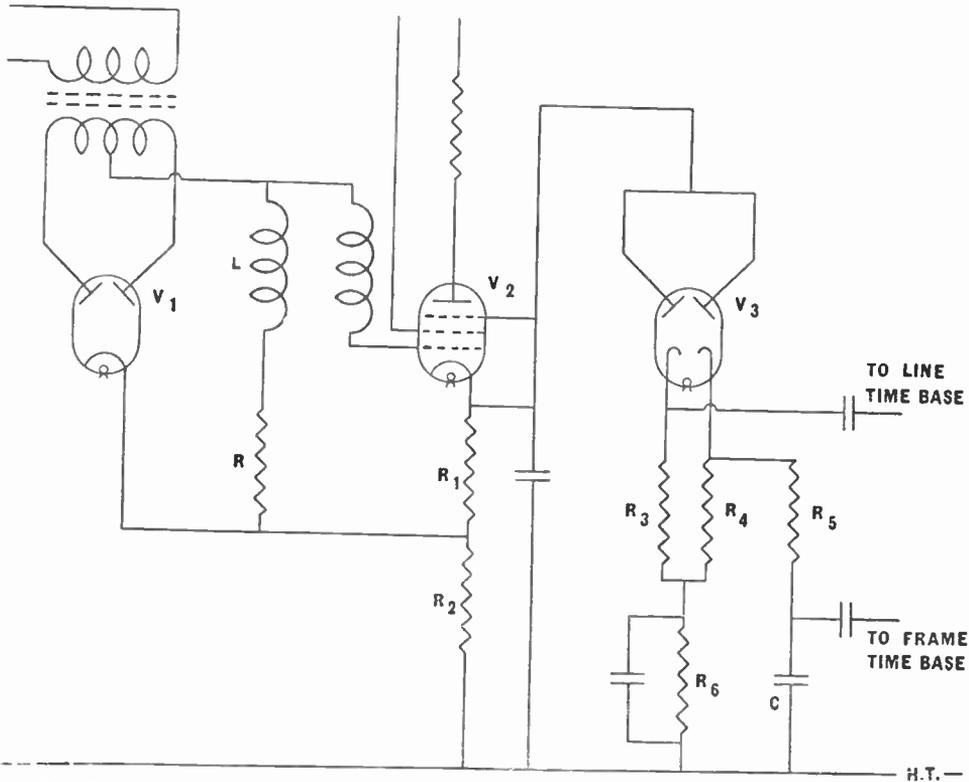
Fig. 89.—Circuit arrangement for using a double diode valve for synchronism separation.
