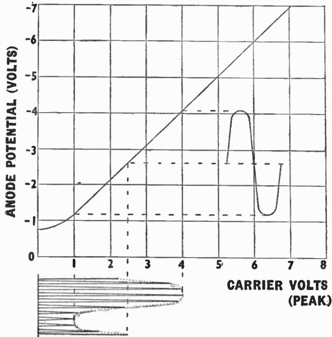
Fig. 96.—Detection curve of a diode. Note that the negative half of the amplitude modulated carrier is omitted.
