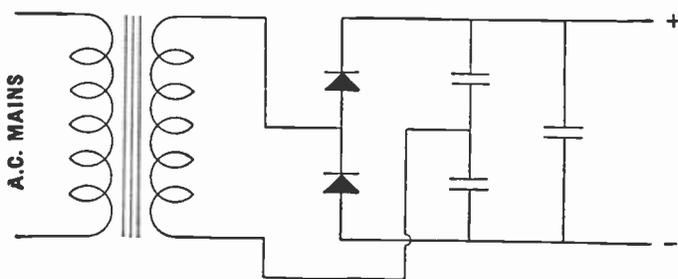
Fig. 7.—Basic circuit of metal rectifiers arranged for voltage doubling.
