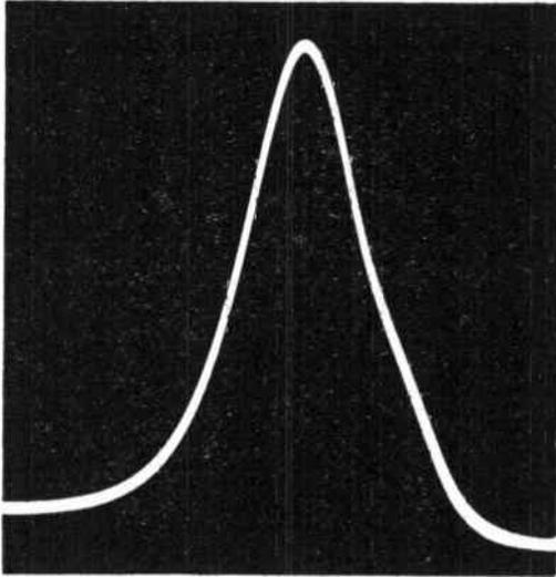
Fig. 133.—The response-curve of an over-coupled bandpass intermediate-frequency transformer. To obtain this illustration the secondaries were so badly mis-tuned that the bandpass characteristics have been lost.
