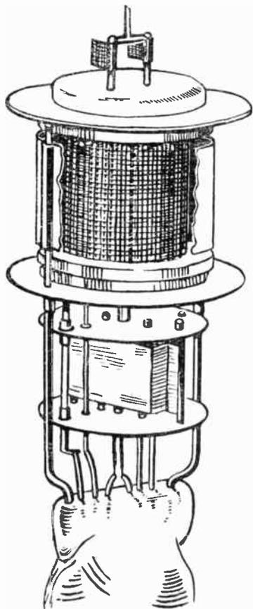
Fig. 124.—The electrode assembly of a typical triode heptode; the lower section is the triode, while the upper section is the heptode, with anode partly cut away to show the outer screening grid.
