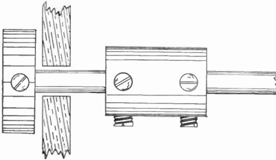
Fig. 67.—A spindle coupling; this device has special significance when the control is on the side of the cabinet.
