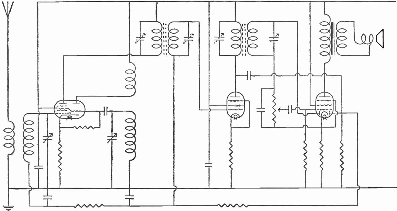
Fig. 29.—Skeleton circuit showing a possible arrangement of a three-valve midget superheterodyne receiver. The power pack is omitted, as it is perfectly conventional.
