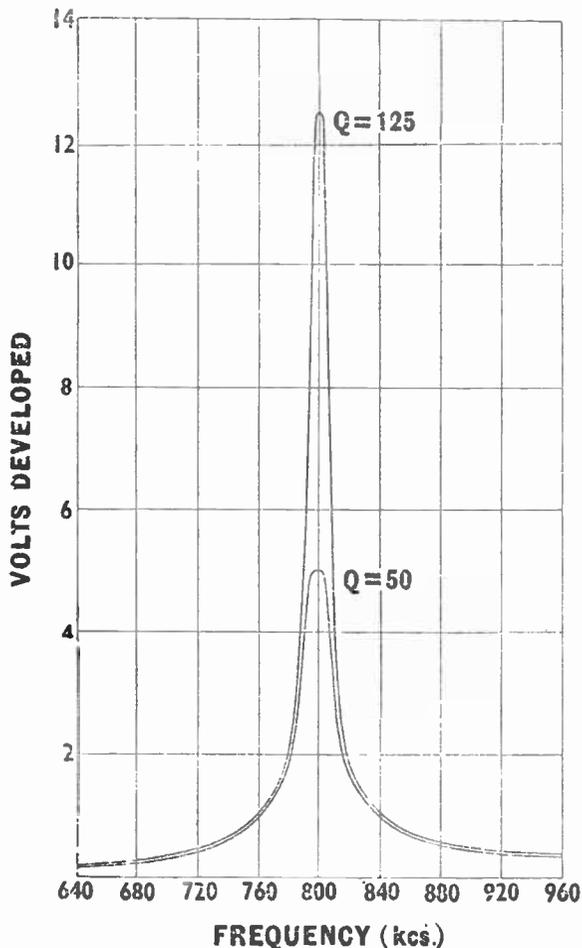
Fig. 66.—The response curve of two inductances having a magnification of 50 and 125 respectively.
