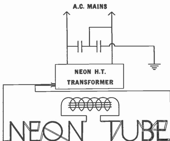
Fig. 66.—Suppressors fitted to the high- and low-tension circuits of a neon sign.
