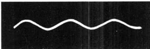
Fig. 5.—Oscilloscope showing mains ripple appearing at points 3 and 4 when  $C_1$  has a capacity of  $2 \mu\text{F}$ .
