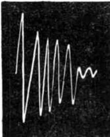
Fig. 19.—An atmospheric recorded by the cathode-ray oscillograph.
