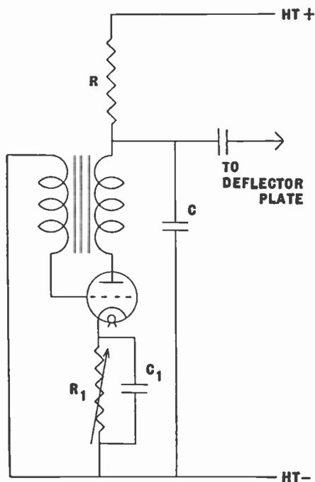
Fig. 79.—The circuit shown at Fig. 78, modified to speed up the discharge.
