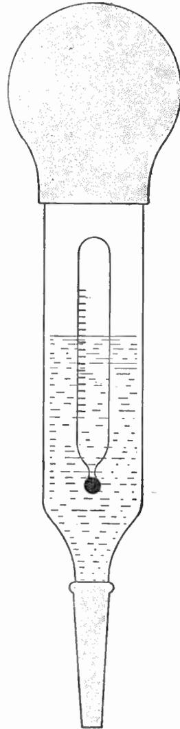
Fig. 73.—A hydrometer with acid drawn in, permitting its specific gravity to be read from the scale on the float.
