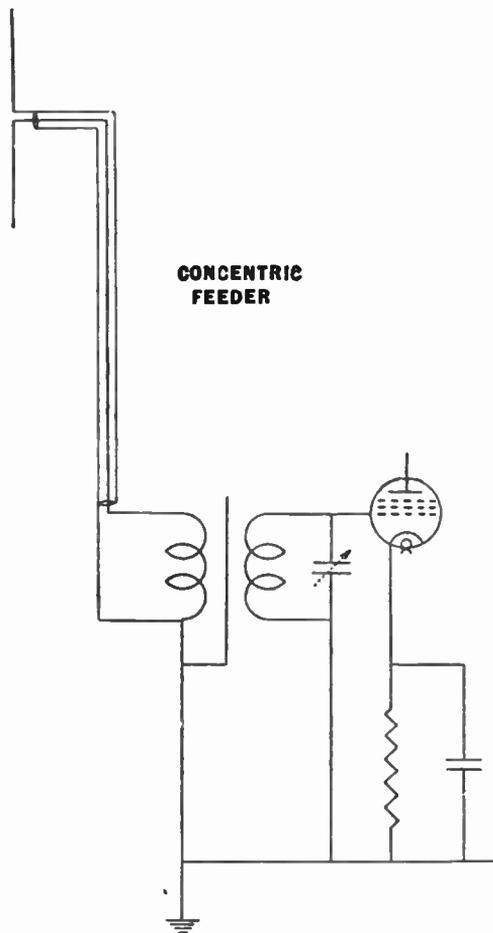
Fig. 106.—The aerial circuit arranged for use with concentric feeder.
