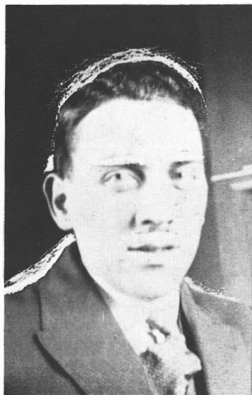
FIG. 149.—If the receiver gives undue high-frequency response, the image will be accompanied by white patches surrounding the dark sections, somewhat after the manner shown in this illustration.
