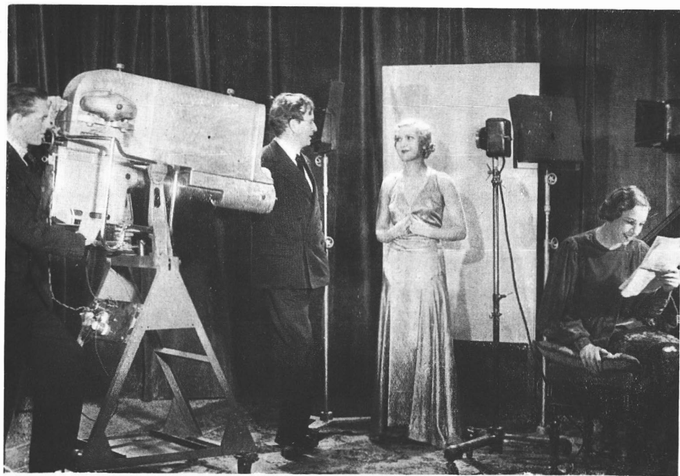
FIG. 128. — A photograph of a spotlight television transmission being carried out. On the left may be seen a portable transmitter.
