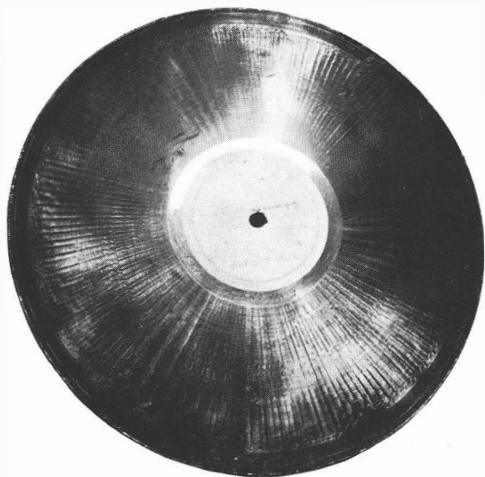
FIG. 85.—An actual phonovision disc record. When “played” on the appropriate apparatus, instead of song or music being heard, the movements of an artist can be watched in the vision apparatus.
