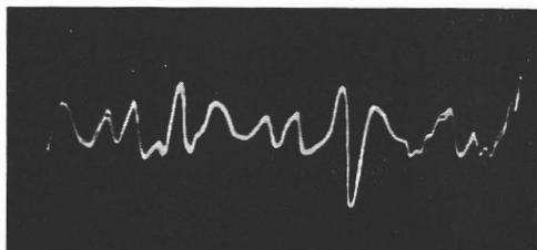
FIG. 81 ( left ).—An A.C. ellipse. Note that the spot has travelled many times round its orbit, hence the woolly line. Stop, f/6.3 ; exposure \frac{1}{2} sec.
