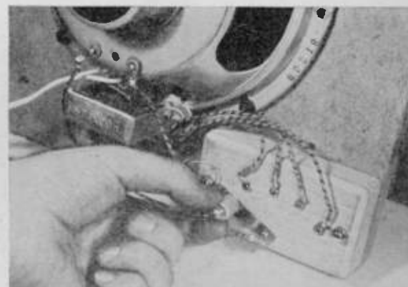
8. Filter chokes may be improvised from either filament or output transformers. One winding isn't used; it can even be open or shorted.
