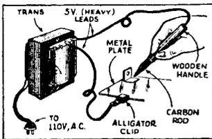
FIG. 4—Set-up of the electric-arc apparatus for soldering.
