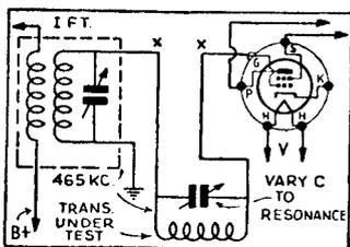
FIG. 13—Determining inductance of I.F. transformers.
