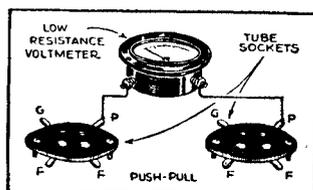
FIG. 3—Illustrating procedure for matching push-pull tubes.
