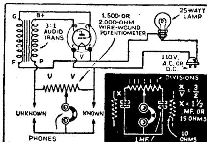
FIG. 22A—Simplified A.C. Bridge unit. B, method of calculation at lower right.
