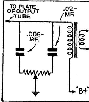
FIG. 4—A novel tone-control circuit.
