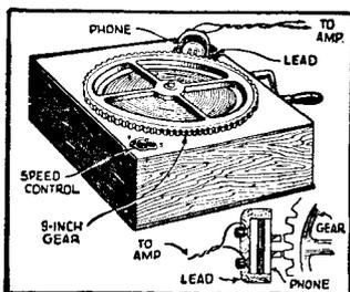
FIG. 1—Calibrated A.F. Alternator.
