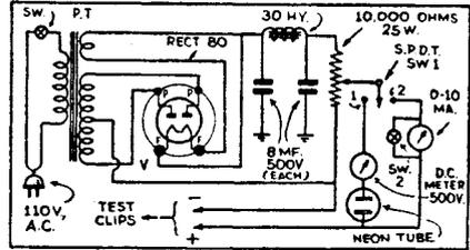
FIG. 5—A Neon-Tube condenser tester.
