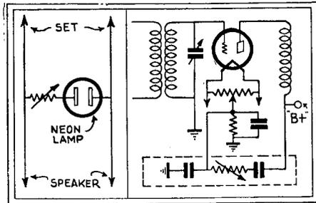
FIG. 11, left—Circuit of the static reducer.
