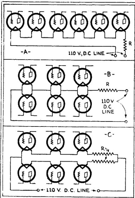
FIG. 4—"DC"-tube filament connections. Circuit A consumes little filament current, but "B" potential is low; that of B, results in high "A" current and "B" potential, and; C, a safer arrangement.
