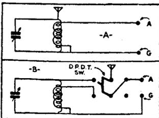
FIG. 19—Increasing sensitivity of midgets.
