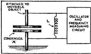
FIG. 8—Ultra-Micrometer head.
