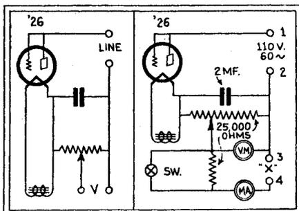
FIG. 26A, left—Theoretical circuit of the resistance calculator.
