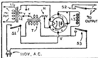
FIG. 27—A V-T. type time-delay relay circuit which is variable from 10 to 60 seconds.
