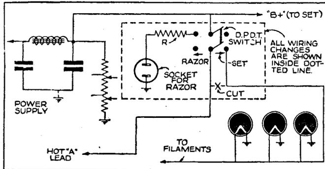
of the correct value to reduce the voltage delivered by the power supply to approximately 110 volts when the razor is running. This value must be found by experimentation.
