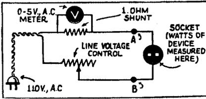
FIG. 6—Circuit of a simple wattmeter.
