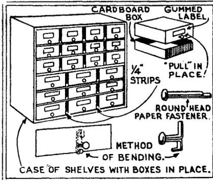
FIG. 2—The cabinet here shown provides a place for everything; yet it is made of paper boxes, etc., which would otherwise be thrown away. Small wooden strips serve instead of partitions, as shown.
