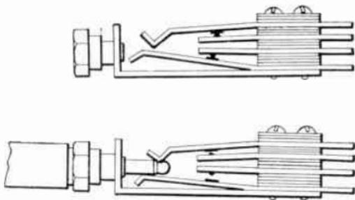
FIG. 90.—Typical jack for vacuum tube plate circuit.
