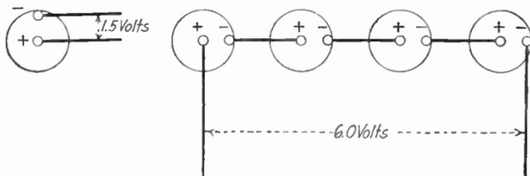
FIG. 66.—Dry cells connected in series.
