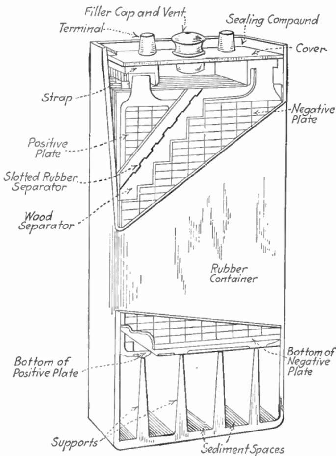
FIG. 68.—Typical lead-plate storage battery.
