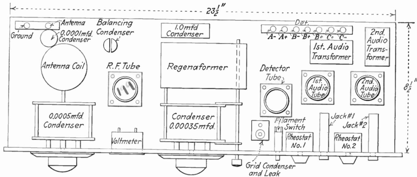
FIG. 177.—Base-board lay-out for Browning-Drake receiver.
