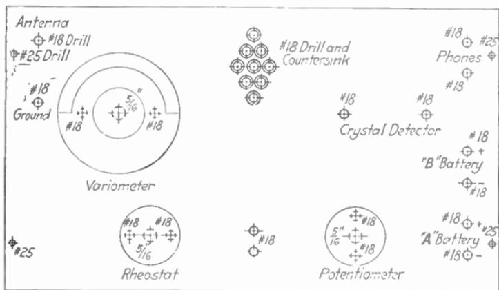
FIG. 159.—Drilling templet for single-tube reflex receiving set.
