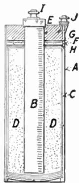
FIG. 64.—Construction of ordinary dry cells.
