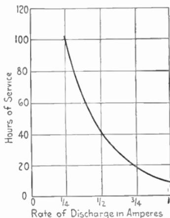
FIG. 65.—Curve of discharge of dry cell.
