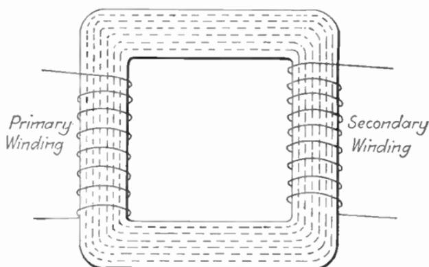
FIG. 26.—Simple transformer.
