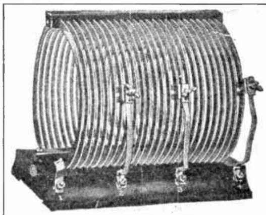
FIG. 130.—Oscillation transformer.
