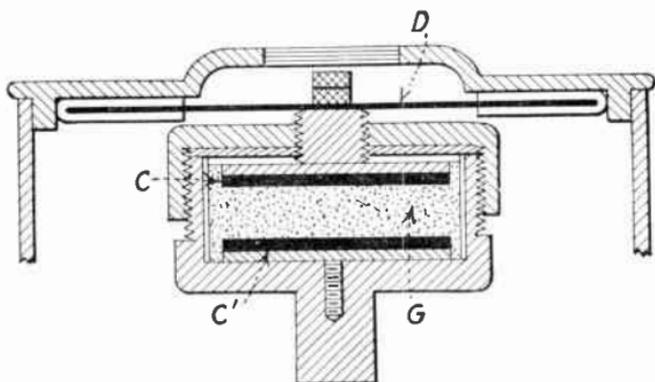
FIG. 137.—Low-capacity microphone for transmitter.
