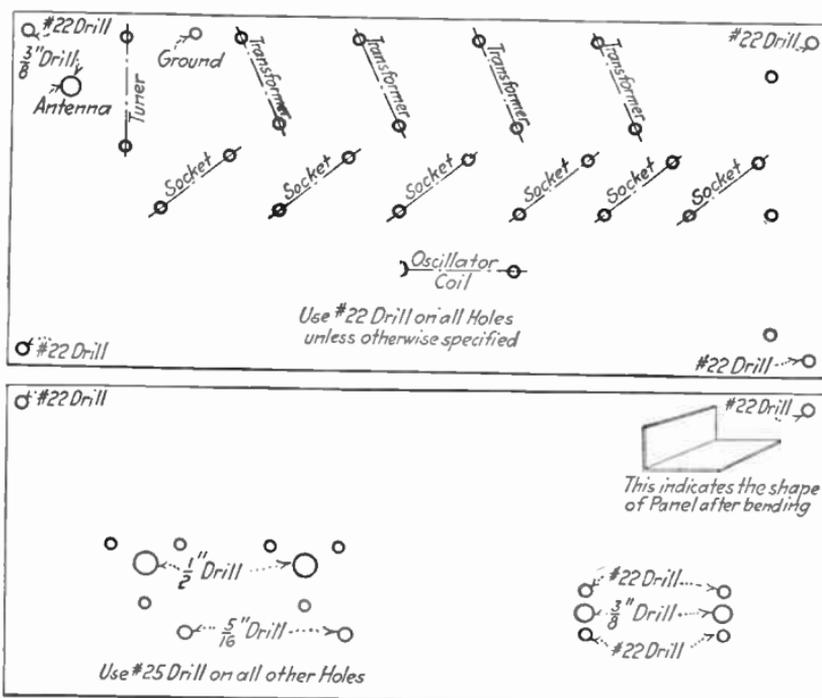
FIG. 165.—Drilling templet for six-tube super-heterodyne receiving set.
