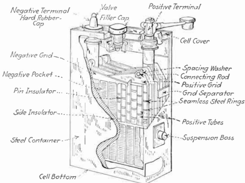
FIG. 69.—Typical nickel-iron storage battery.
