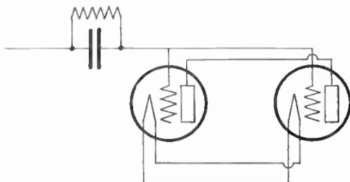
FIG. 125.—Parallel connections of vacuum tubes.
