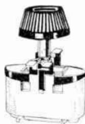
Fig. 57.—Typical resistance rheostat.
