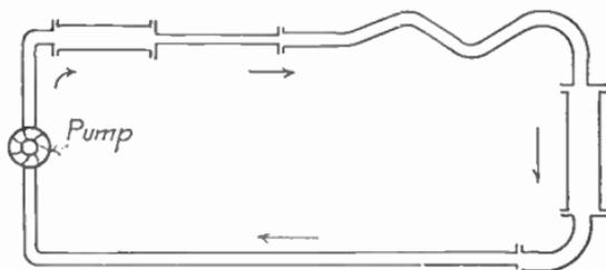
FIG. 21.—Pipes connected in series.
