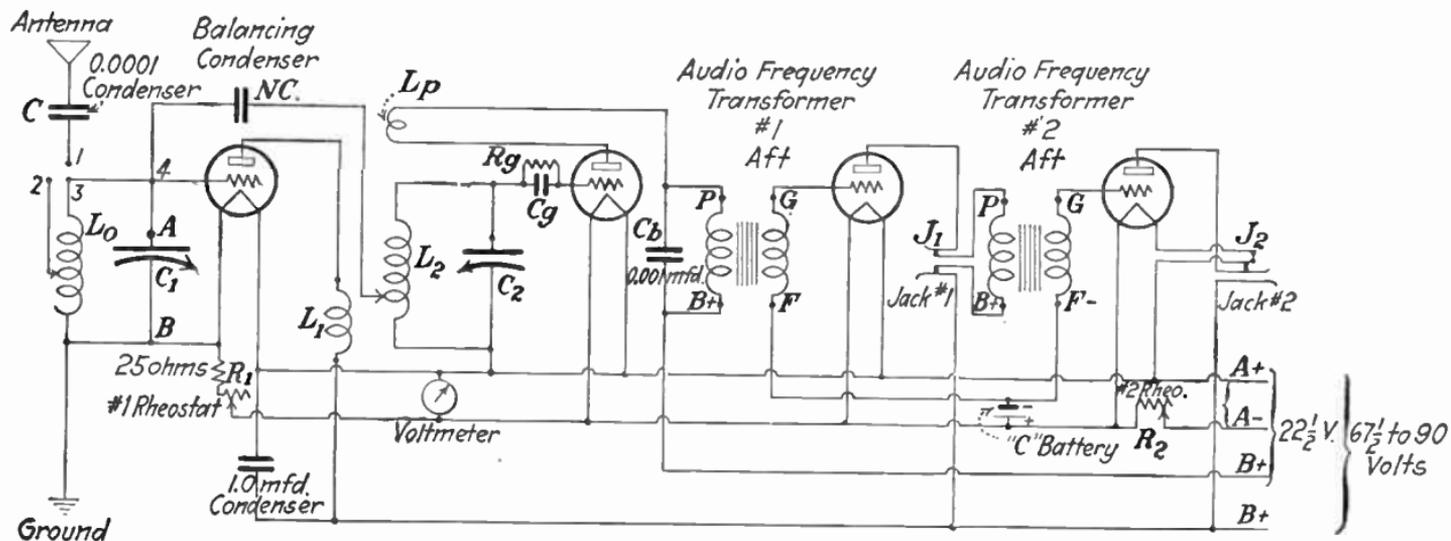
FIG. 175.—Browning-Drake circuit diagram.
