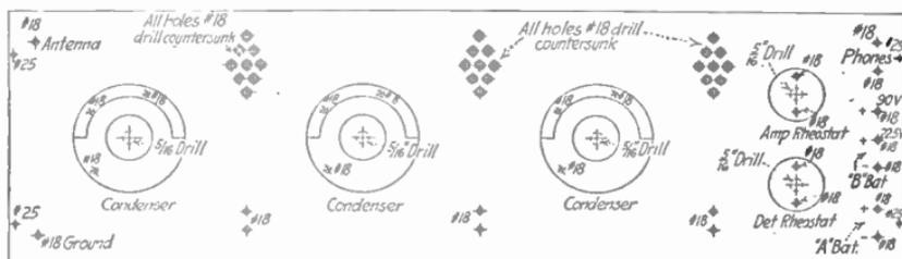
FIG. 163.—Drilling templet for three-tube neutrodyne receiver.
