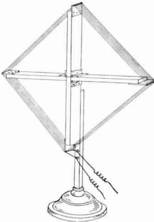
FIG. 148.—Small radio loop.
