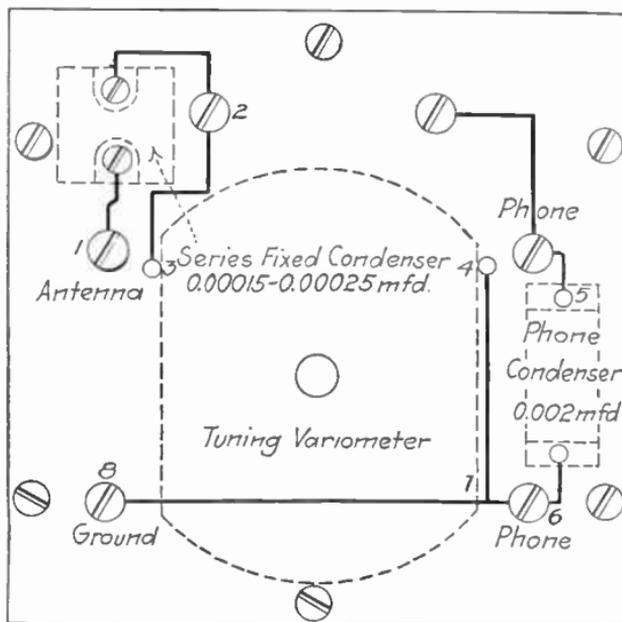
FIG. 152.—Wiring diagram for crystal receiving set.
