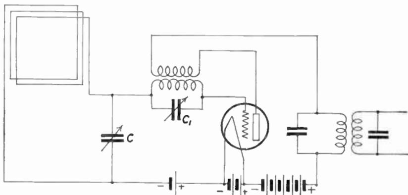
FIG. 114a.—Self-heterodyne detector.
