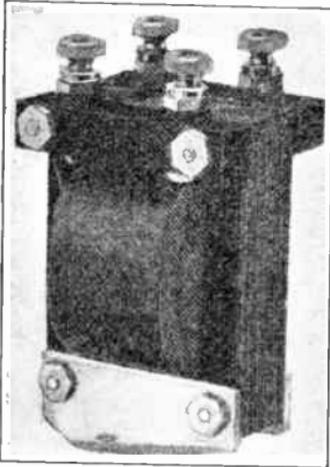
FIG. 78.—Audio-frequency transformer with iron core.
