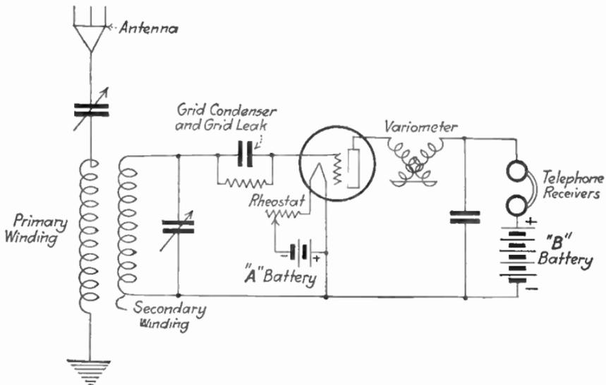
FIG. 59.—Regeneration with tuned plate circuit.
