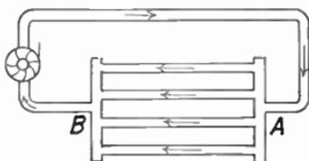
FIG. 22.—Pipes connected in parallel.
