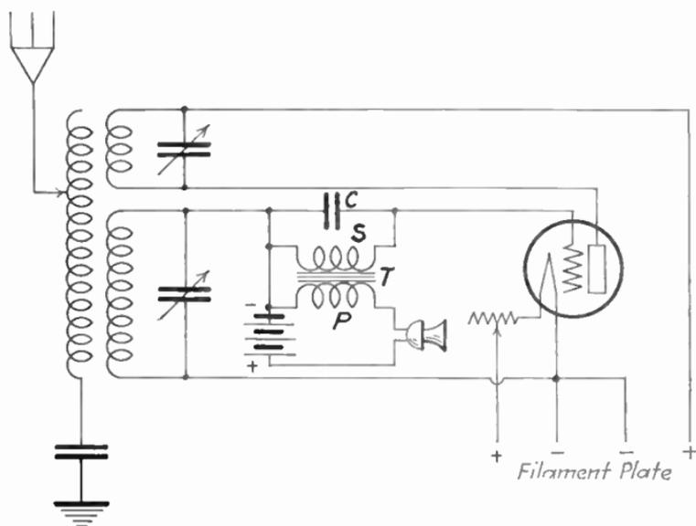
FIG. 127.—Microphone in grid circuit.
