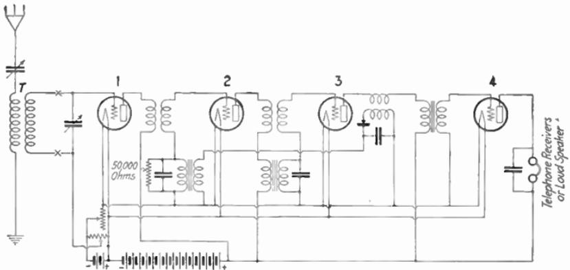
FIG. 109.—Four-tube Acme reflex circuit.
