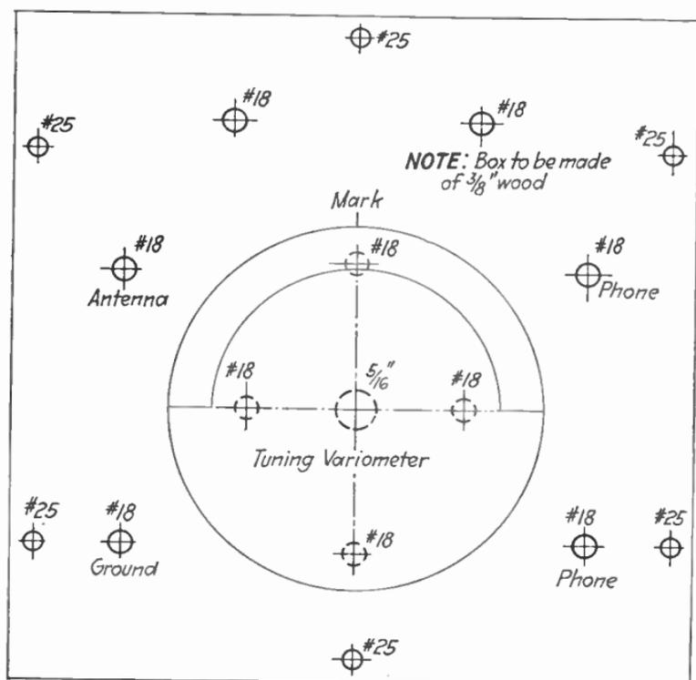
FIG. 151.—Drilling templet for crystal detector receiving set.
