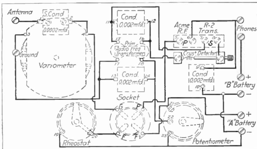
FIG. 160.—Wiring diagram for single-tube reflex receiving set.
