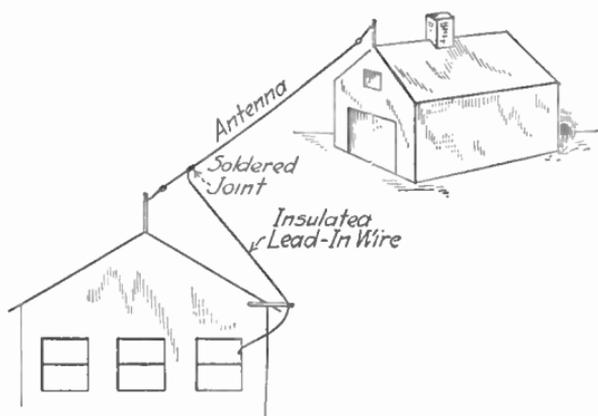
FIG. 3.—Simple outside antenna.
