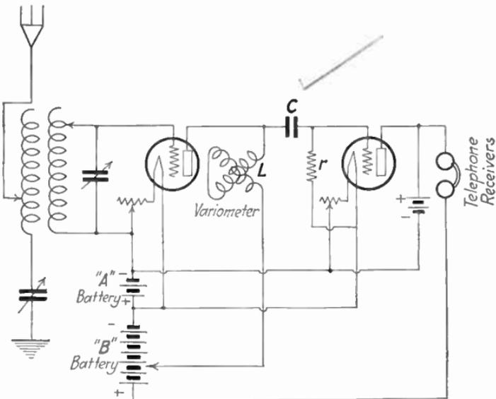
Fig. 94.—Radio-frequency amplification with plate variometer.
