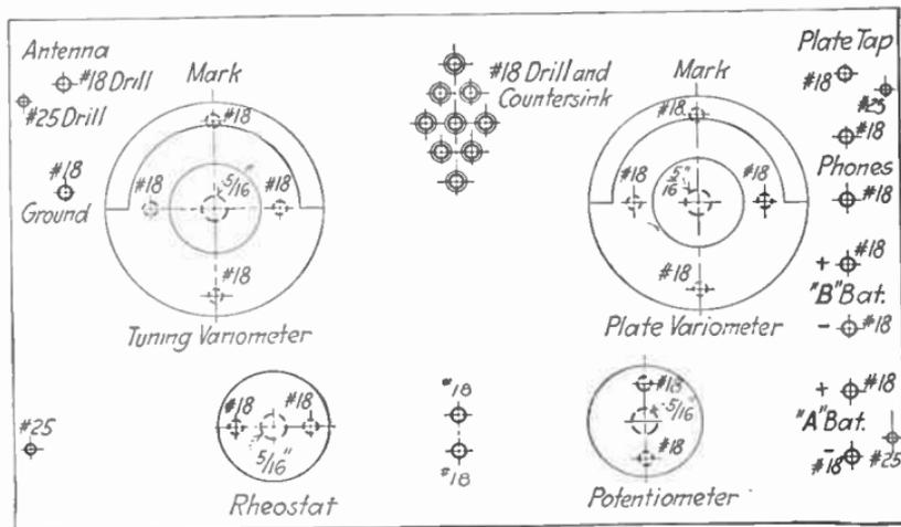
FIG. 153.—Drilling templet for single-tube receiving set.
