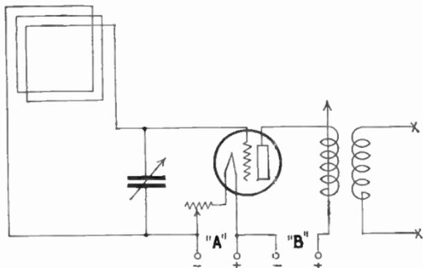
Fig. 110.—Tuned radio-frequency circuit.
