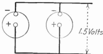
FIG. 67.—Dry cells connected in parallel.
