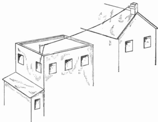
FIG. 7.—Typical outside antenna.
