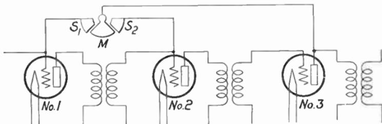
FIG. 103.—Capacity for regeneration control.
