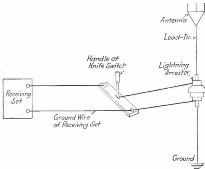
FIG. 17.—Combined knife-switch and lightning arrester.
