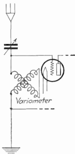
FIG. 95.—Radio-frequency amplification with single circuit tuner.
