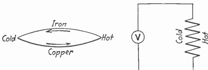
FIG. 180.—Thermo-electric battery.
