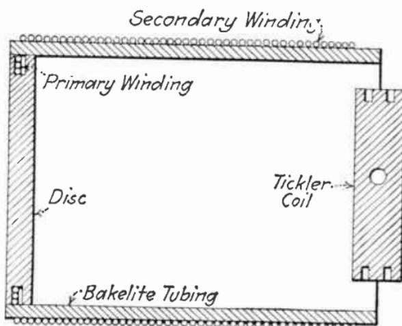
FIG. 173.—Simple "slot" transformer winding.
