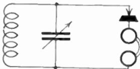
FIG. 142.—Radio wave meter.
