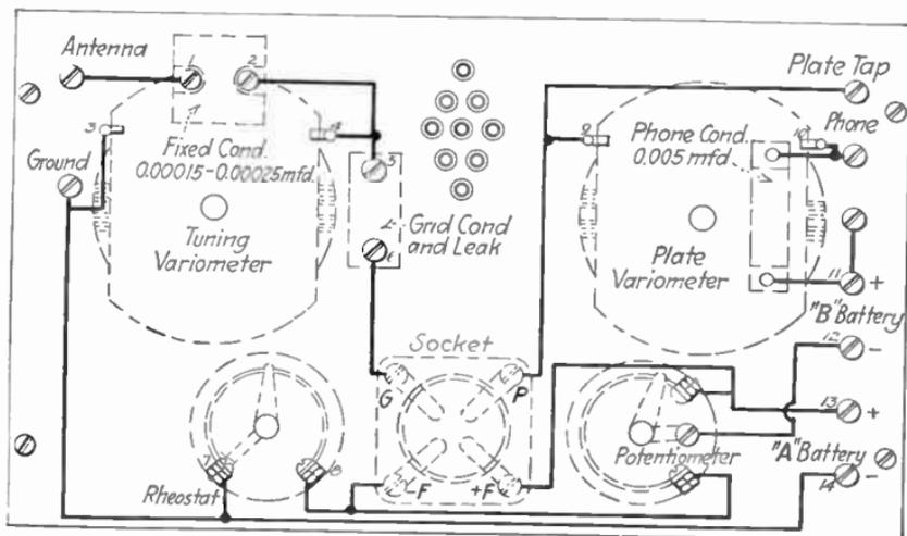
FIG. 154.—Wiring diagram for single-tube receiving set.
