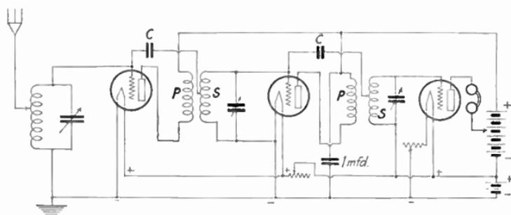
FIG. 100.—Reversed capacity for regeneration control.
