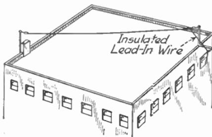
FIG. 8.—Typical outside antenna.
