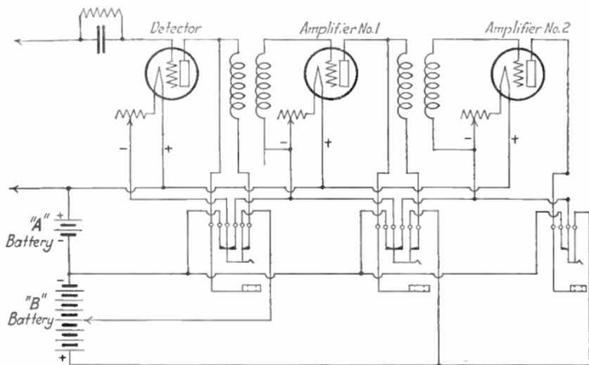
FIG. 89.—Five-and-three spring jacks for vacuum tube filament circuit.
