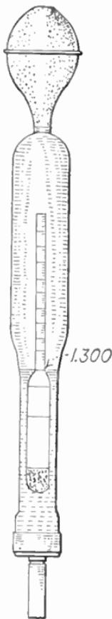
Fig. 70.—Hydrometer for testing storage batteries.
