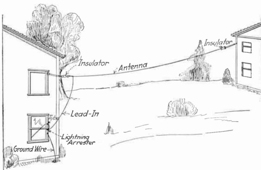
FIG. 9.—Typical outside antenna.
