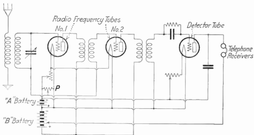
FIG. 96.—Grid-potentiometer for regeneration control.
