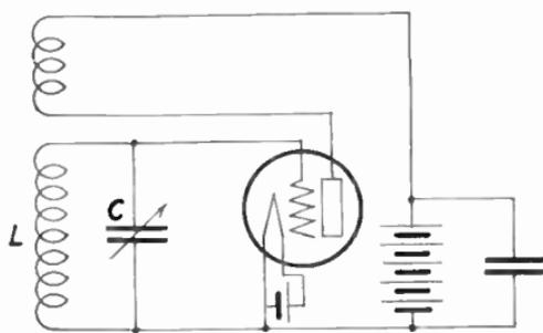
FIG. 122.—Control of tube oscillator.
