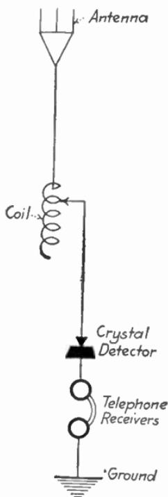
FIG. 43.—Inductance coil in antenna circuit for tuning.
