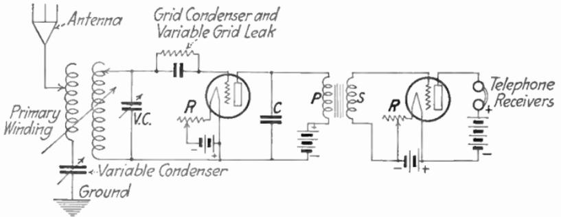
FIG. 77.—Audio-frequency amplification by transformer coupling.
