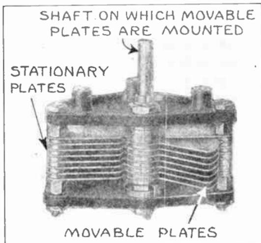
FIG. 28.—Commercial type of condenser.
