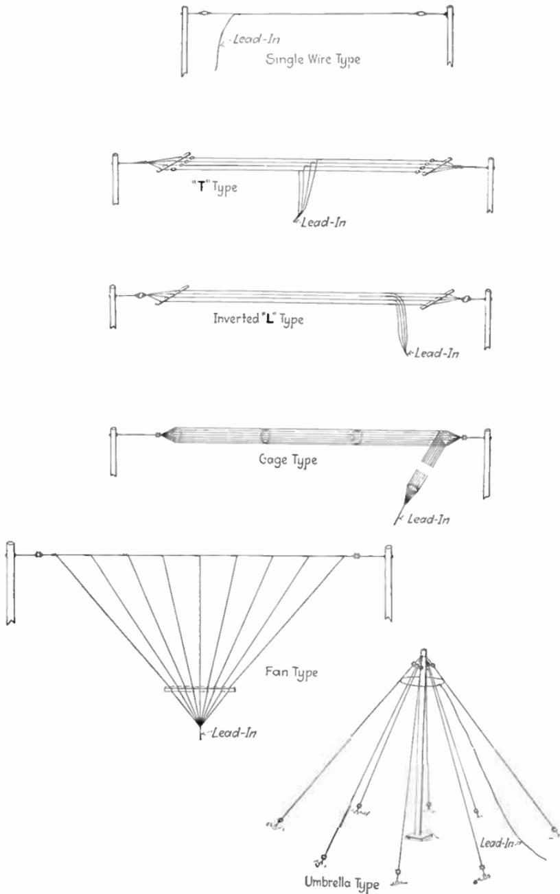
FIG. 18.—Forms of transmitting antennas.
