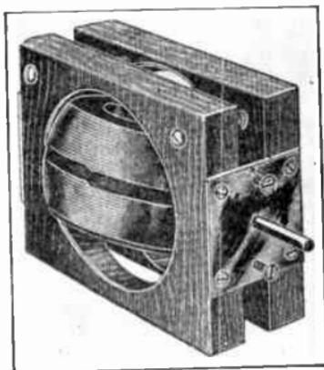
FIG. 41.—Variable type of inductance coils.
