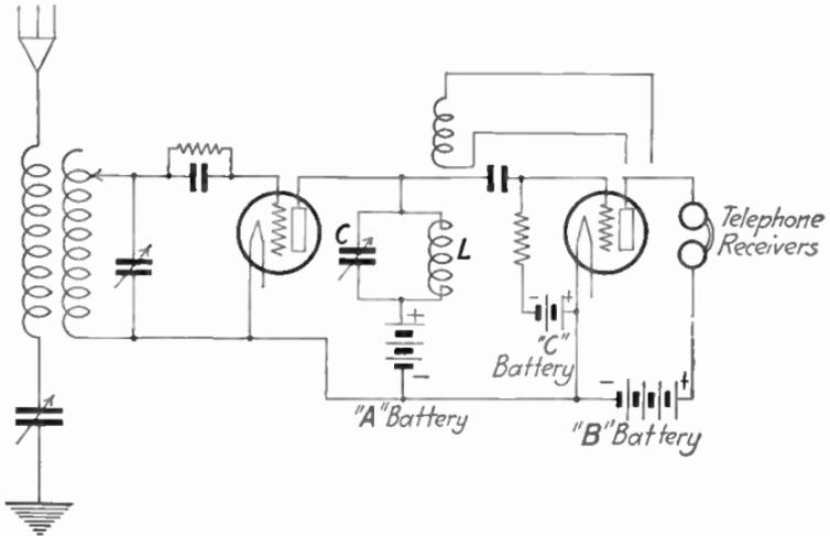
Fig. 93.—Radio-frequency amplification by inductance coupling.
