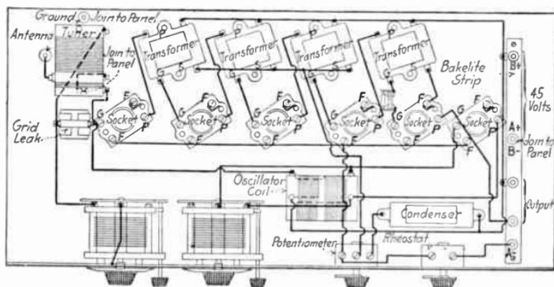
FIG. 166.—Wiring diagram for six-tube super-heterodyne receiving set.
