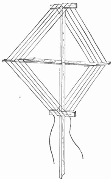
FIG. 13.—Typical radio loop.
