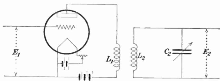
FIG. 172.—Radio-frequency transformer circuit.
