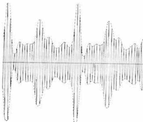
FIG. 32.—Carrier radio wave modulated by sound waves.
