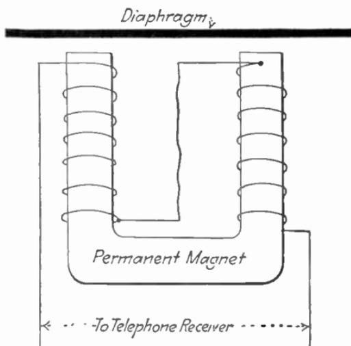
FIG. 82.—Diagram of loud speaker (sound distributor type).
