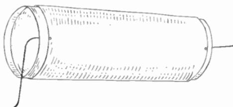
FIG. 38.—Fixed type of inductance coil.
