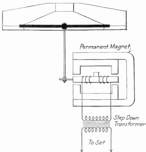
FIG. 85.—Loud speaker (balanced armature type).
