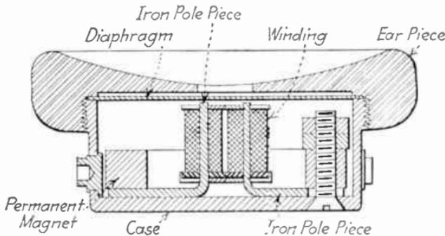
FIG. 30.—Typical telephone receiver.
