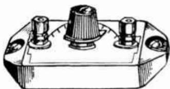
FIG. 54.—Combined grid leak and grid condenser.
