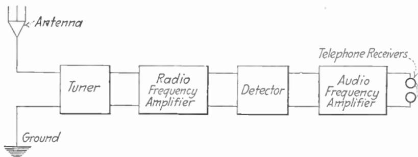
FIG. 76.—Position of amplifiers in radio receiving sets.
