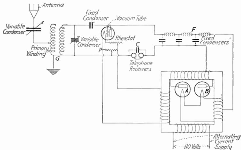
FIG. 73.—Potentiometer connections for alternating current.
