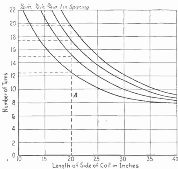
FIG. 149.—Drawing for construction of radio loop.
