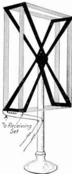
FIG. 12.—Typical radio loop.
