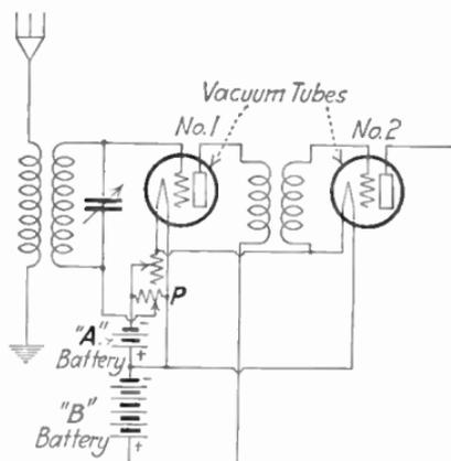
FIG. 97.—Grid-potentiometer for regeneration control.
