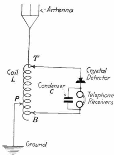
FIG. 44.—Crystal detector in secondary circuit.
