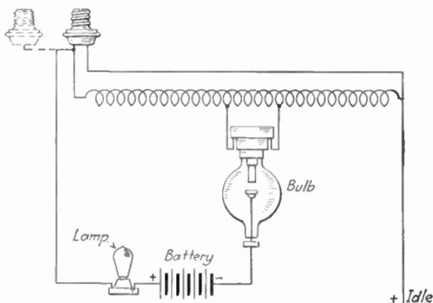
FIG. 72.—Vacuum tube rectifier for charging "B" batteries.
