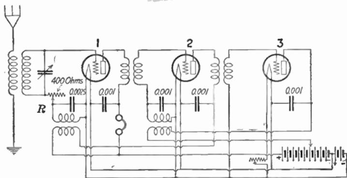
Fig. 111.—Grimes inverse duplex circuit (reflex).
