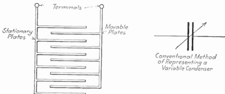
FIG. 27.—Diagram of a simple condenser.
