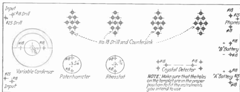
FIG. 161.—Drilling templet for four-tube reflex receiving set.
