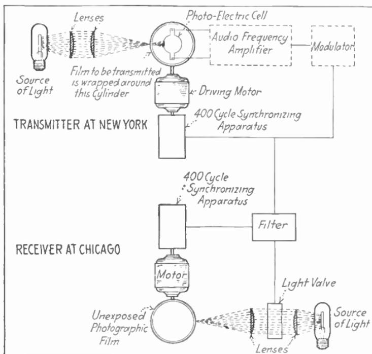
FIG. 181.—Photographic apparatus for radio transmission.
