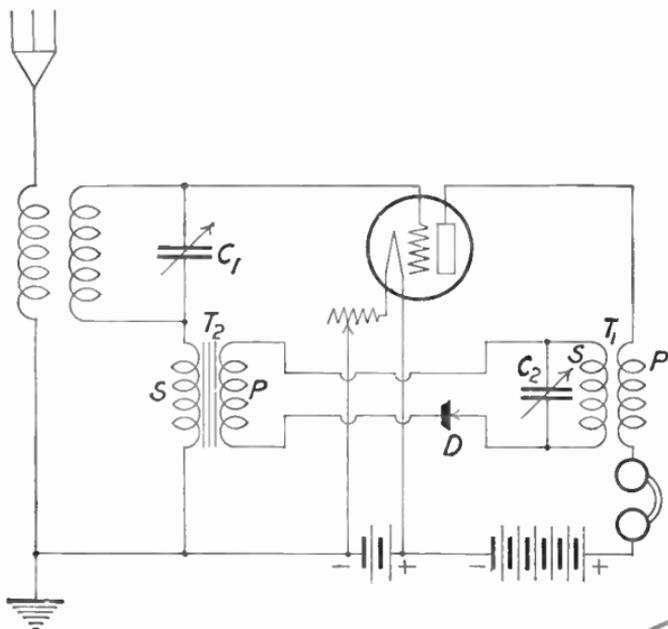
FIG. 107.—Harkness reflex circuit.
