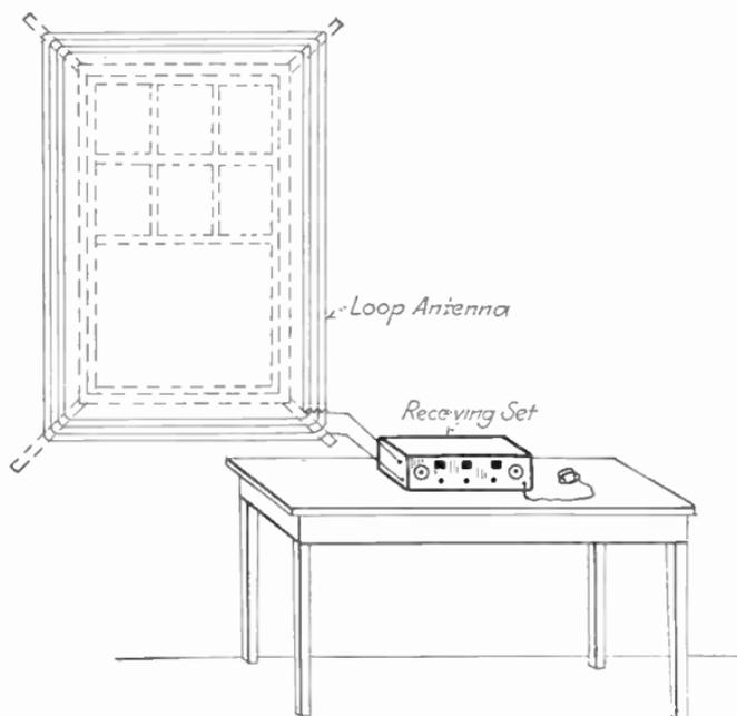
FIG. 15.—Typical radio loop around a window.
