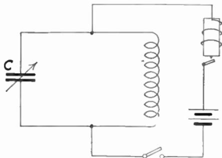
FIG. 143.—Radio wave meter with interrupter and battery.
