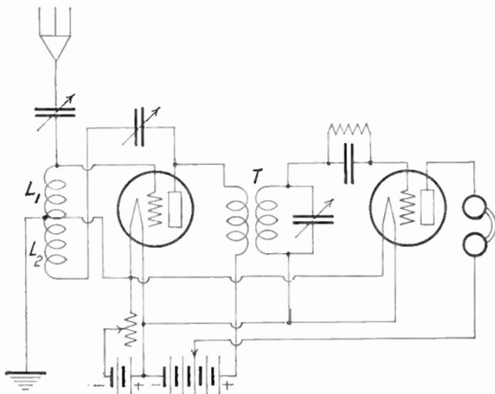
FIG. 102.—Inductance coupling for regeneration control.
