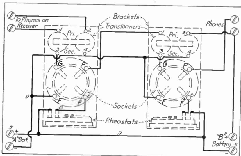
FIG. 156.—Wiring diagram for two-stage audio-frequency amplifier.
