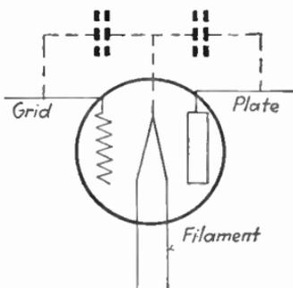
FIG. 60.—Capacity effect in vacuum tube.
