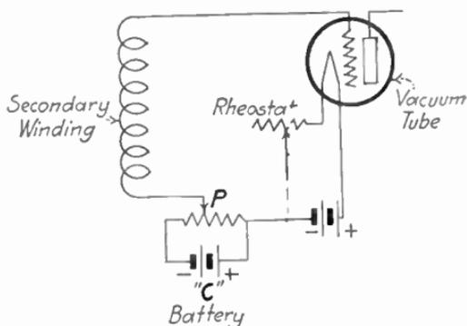
FIG. 53.—Combined use of potentiometer and "C" battery.
