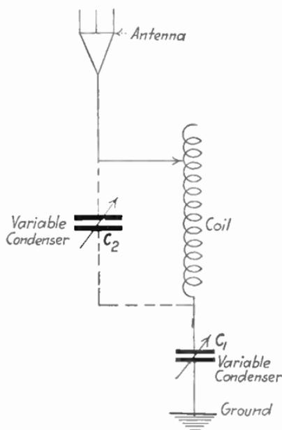
FIG. 46.—Variable antenna condensers for tuning.
