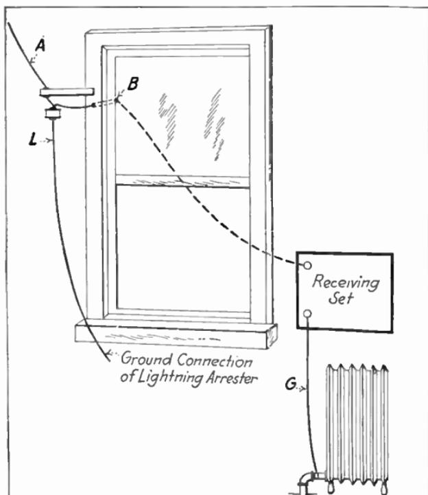
FIG. 16.—Method of attachment of lightning arrester.
