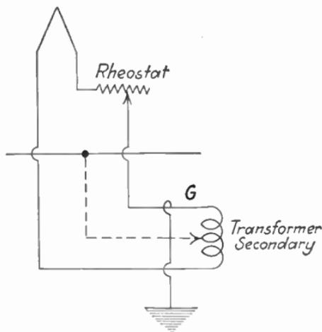
FIG. 74.—Transformer connections for alternating current.
