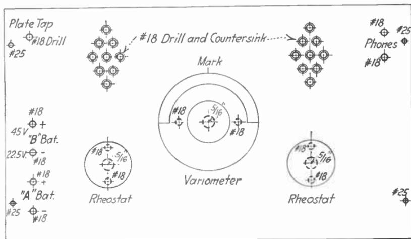
FIG. 157.—Drilling templet for two-stage radio-frequency amplifier.
