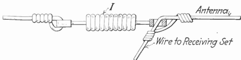
FIG. 10.—Extension antenna used as lead-in wire.
