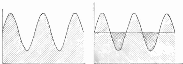
FIG. 121.—Alternating current super-imposed upon direct current.
