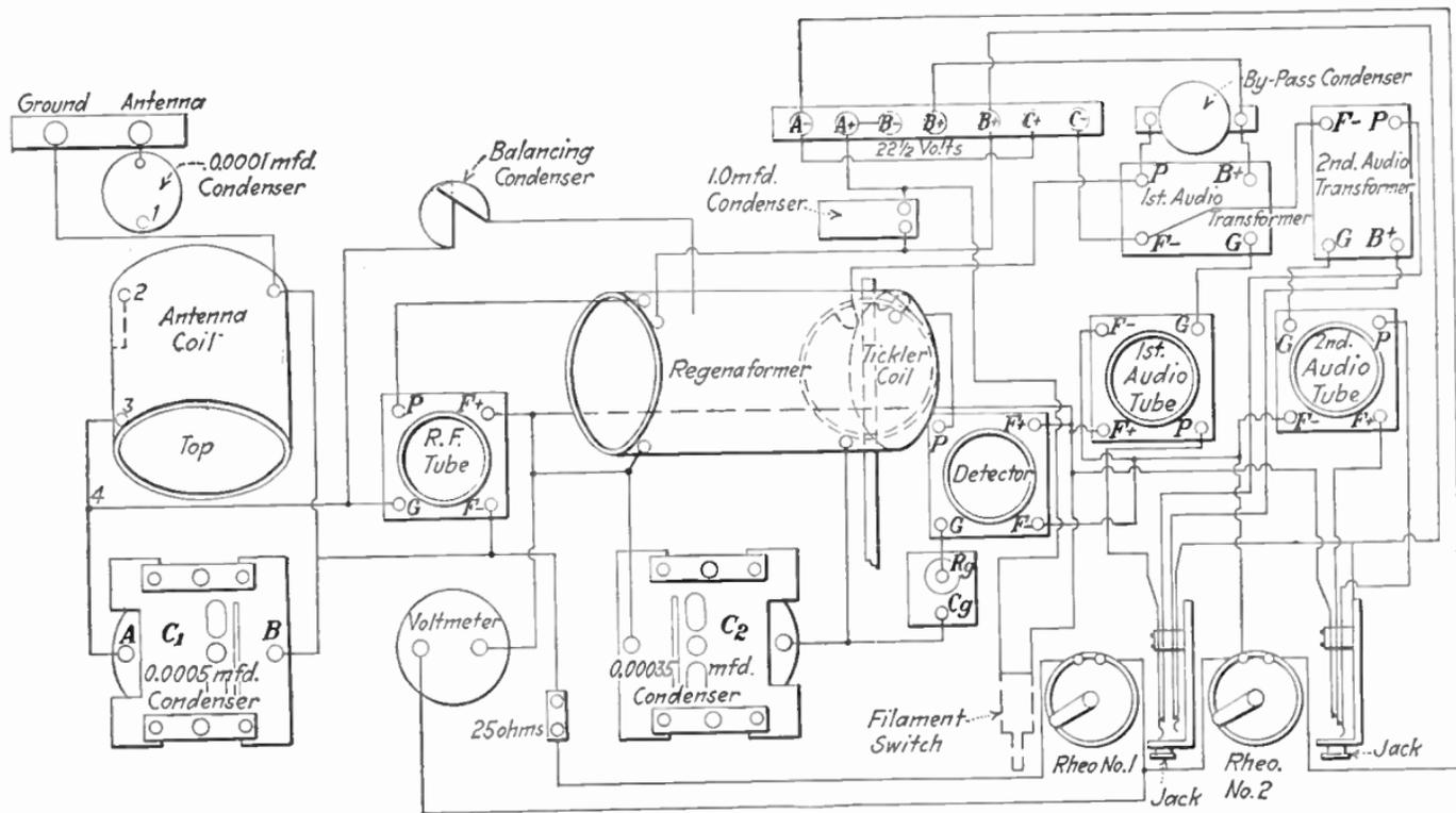
FIG. 178.—Wiring diagram for Browning-Drake receiver.
