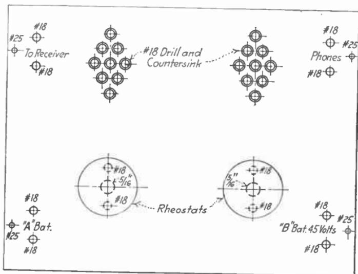
FIG. 155.—Drilling templet for two-stage audio-frequency amplifier.
