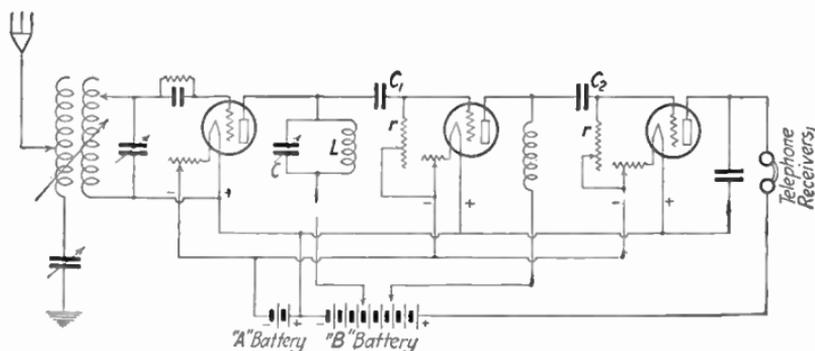
FIG. 81.—Audio-frequency amplification by inductance coupling.
