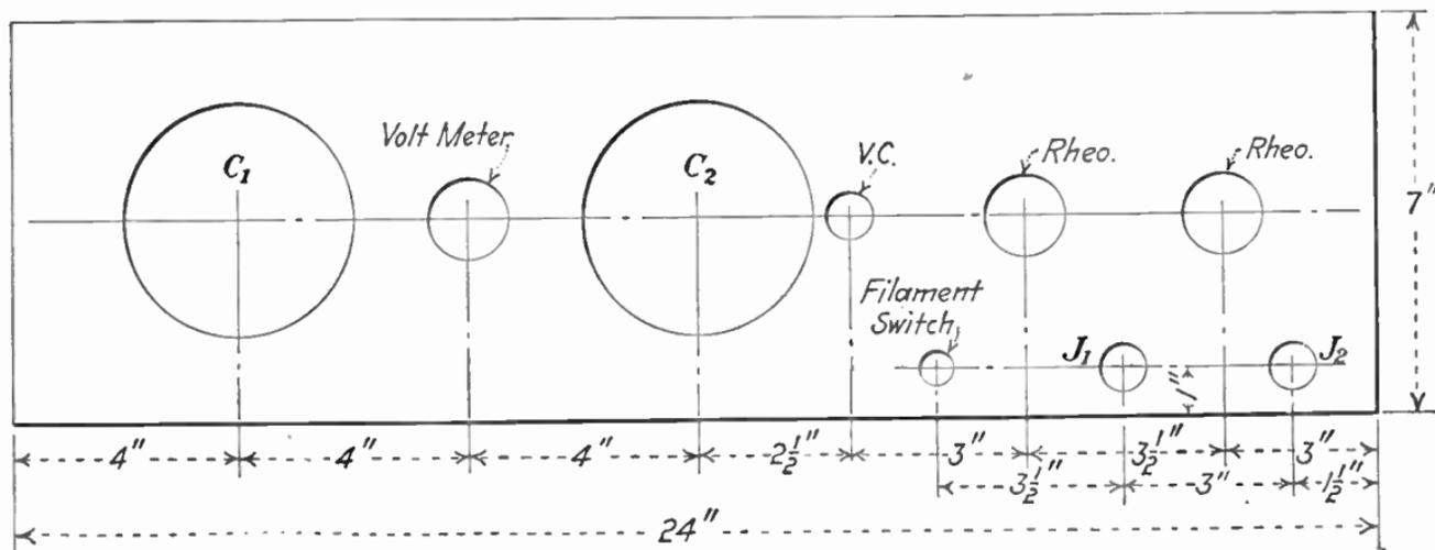
FIG. 176.—Panel lay-out for Browning-Drake receiver.
