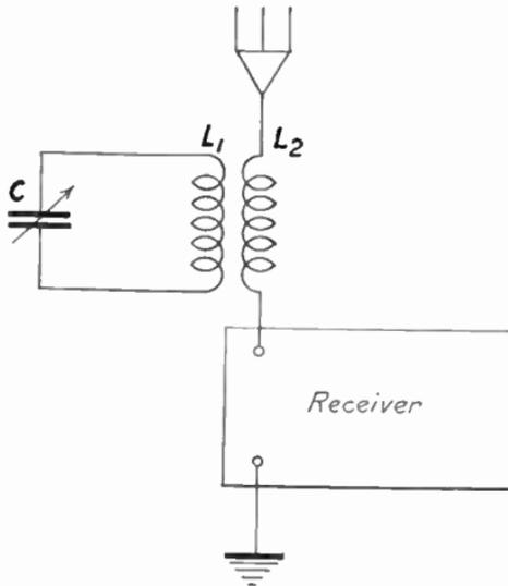
FIG. 141.—Radio wave trap.
