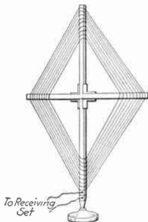
FIG. 14.—Typical radio loop.
