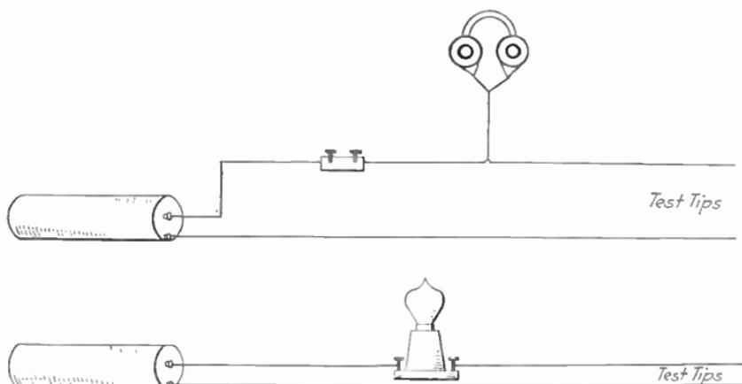
FIG. 150.—Practical radio testing outfit.
