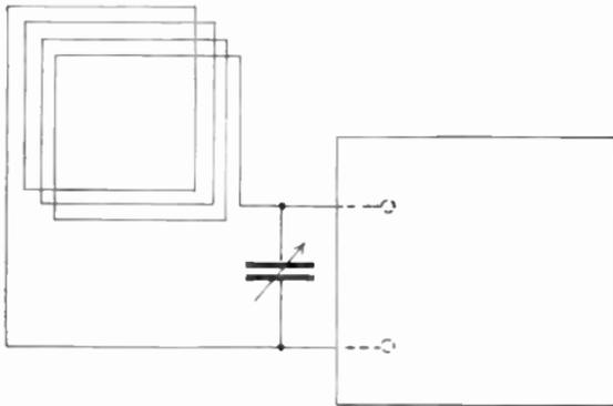
FIG. 147.—Radio loop and condenser to replace tuner.
