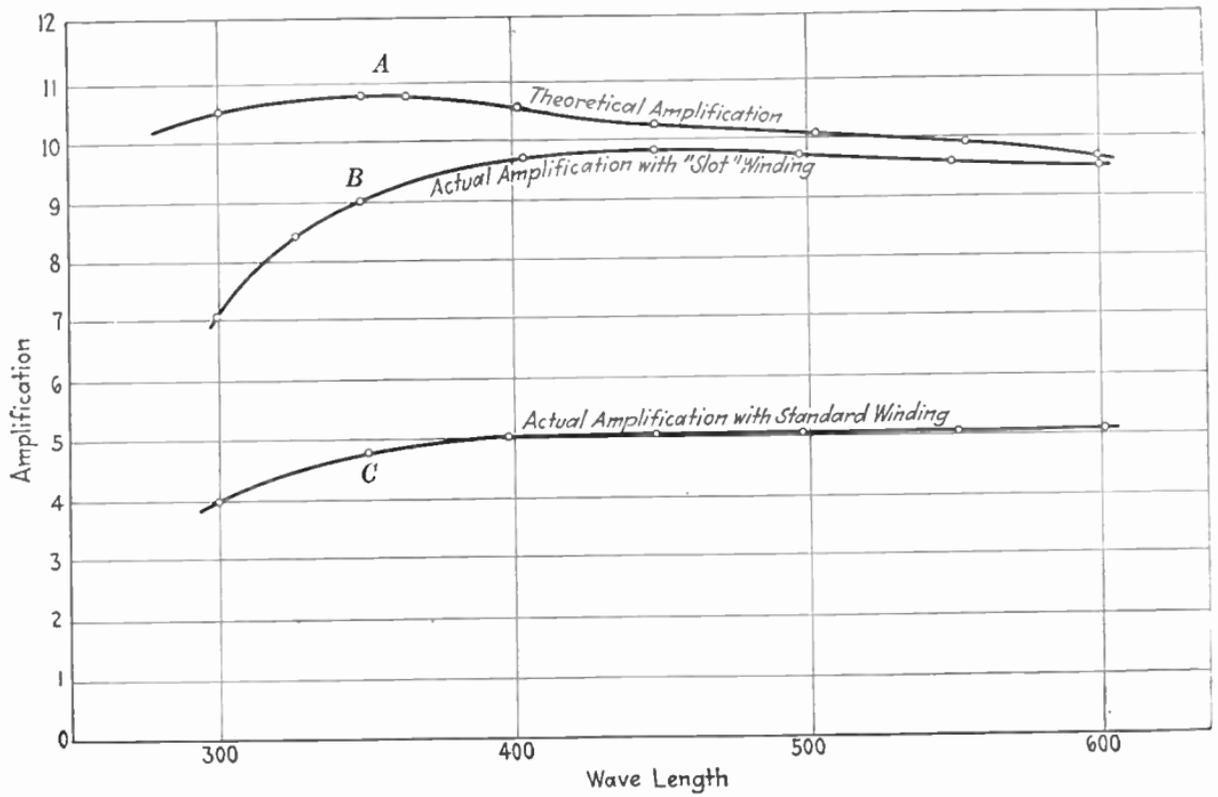
FIG. 174.—Theoretical and actual transformer amplification.
