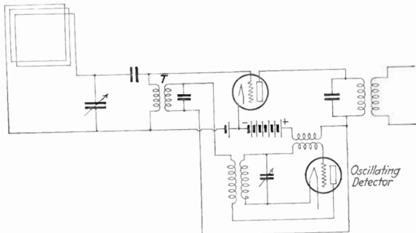
FIG. 114b.—Super-heterodyne circuit with reflex arrangement.
