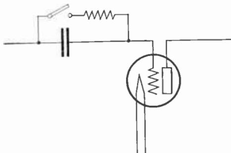
FIG. 123.—Telegraph key in grid circuit.
