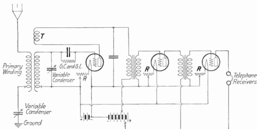
FIG. 79.—Tickler coil for regeneration with audio-frequency amplification.
