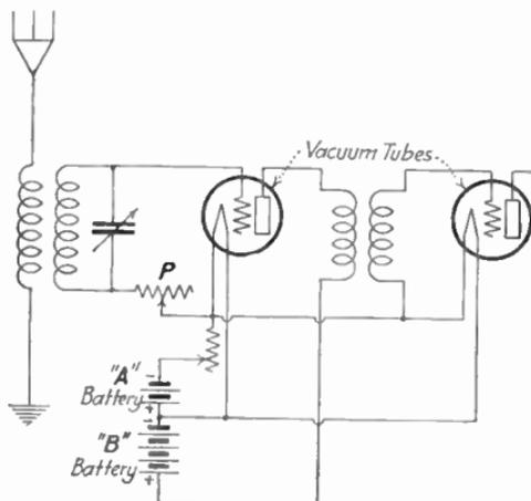
FIG. 98.—Grid-potentiometer for regeneration control.
