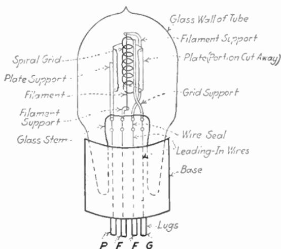
FIG. 47.—Typical vacuum tube.
