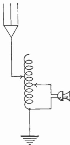
FIG. 126.—Microphone in antenna circuit.
