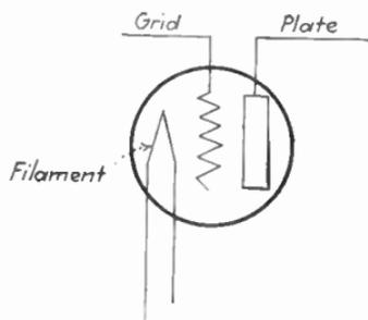
FIG. 48.—Conventional representation of vacuum tube.
