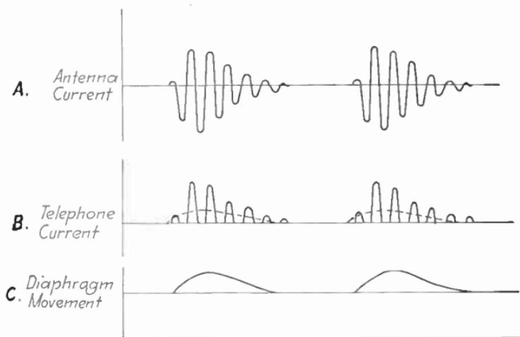
FIG. 31.—Action of crystal detector on radio currents.
