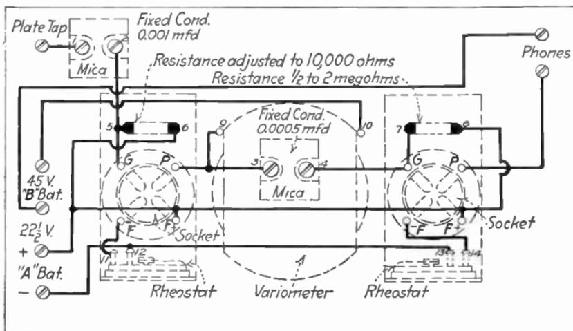
Fig. 158.—Wiring diagram for two-stage radio-frequency amplifier.
