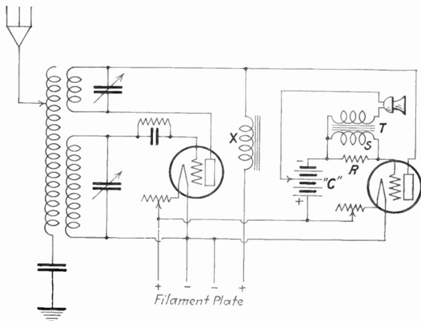
FIG. 128.—Heising system (modulator tube).
