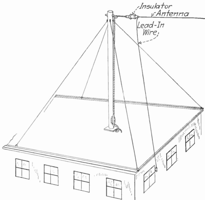
FIG. 11.—Substantial pole for attachment of antenna.
