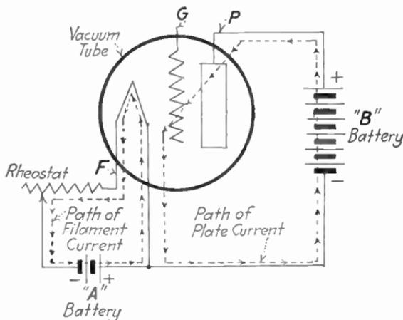
FIG. 50.—Plate and filament currents in vacuum tube.
