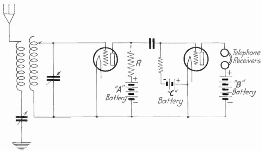
FIG. 92.—Radio-frequency amplification by resistance coupling.
