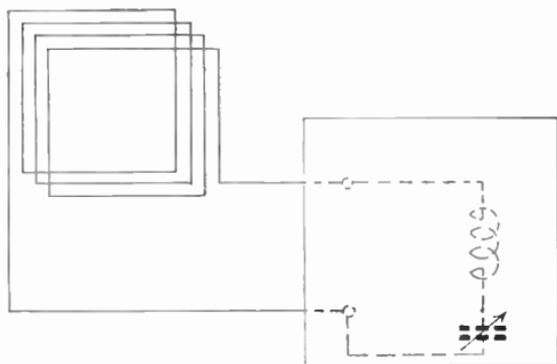
FIG. 145.—Typical method of connecting radio loop to receiving set.
