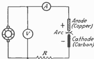
FIG. 136.—Fundamental arc circuit.
