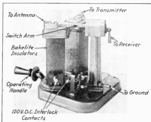
FIG. 146.—Send-ground-receive switch.
