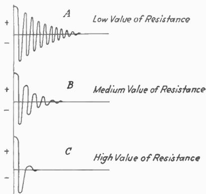
FIG. 79.—Types of damped waves.
