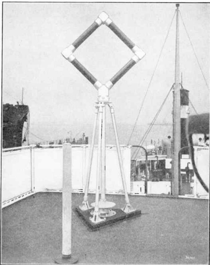
FIG. 214.—R.C.A. radio compass loop.
