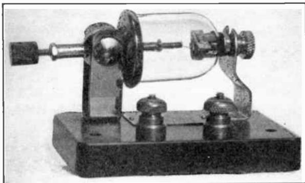
FIG. 110.—Typical crystal detector.
