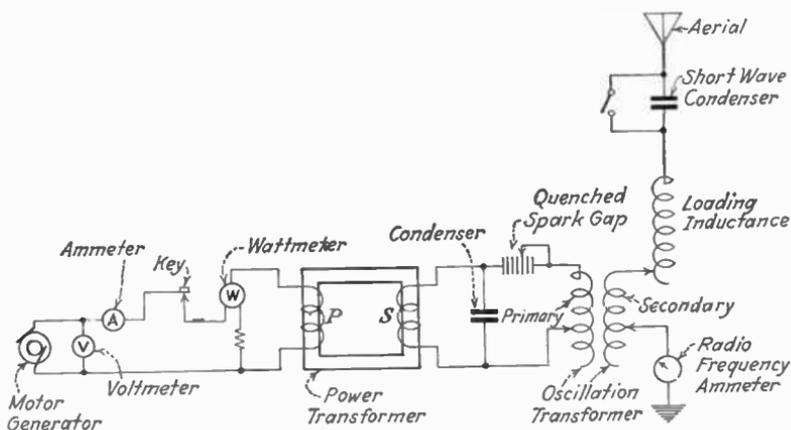
FIG. 87.—Elementary transmitter.
