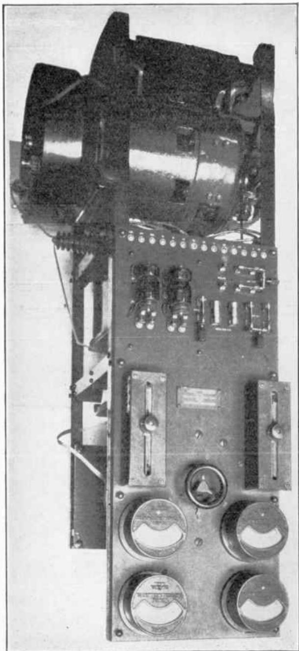
Fig. 189—Independent spark transmitter
