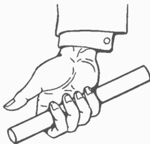
Fig. 16.—Right-hand rule for field direction.
