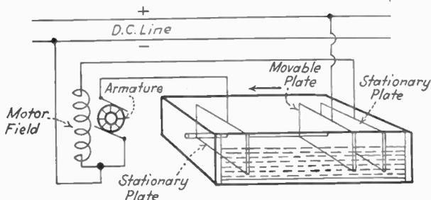
FIG. 34.—Salt-water rheostat.
