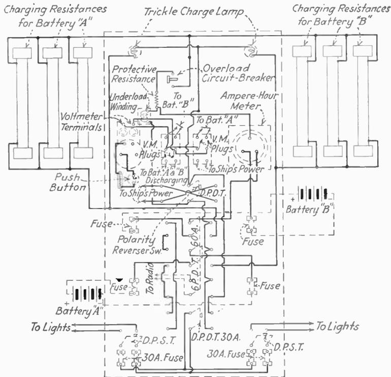
FIG. 67.—Electric storage-battery charging panel (rear-view wiring diagram).
