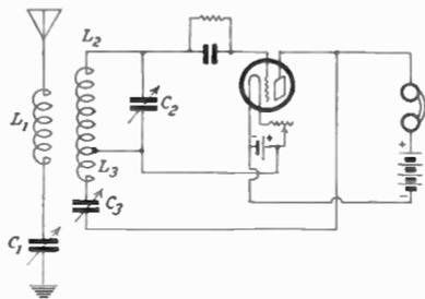
FIG. 128.—Regenerative circuit (capacitive feed-back method).
