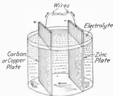
FIG. 36.—The simple primary wet cell.
