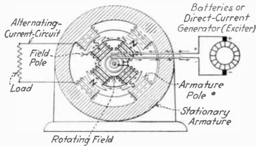
FIG. 22.—Rotating field-type alternator.
