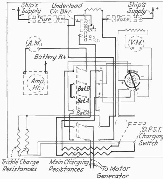
FIG. 60.—Navy standard charging panel (complete).
