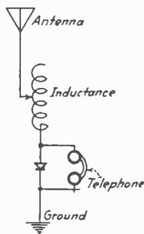
FIG. 105.—Simplest tuned receiving circuit.
