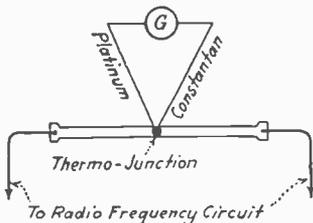
FIG. 59.—Principle of thermoammeter.
