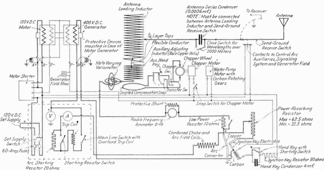
FIG. 154.—Wiring diagram model X 2-kw. Federal Arc ignition key system.
