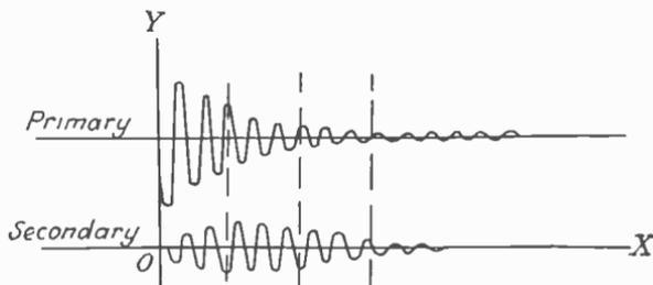
FIG. 94.—Comparative damping of coupled circuits.
