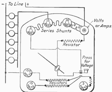
FIG. 53.—Diagram of Weston direct-current voltammeter, model 280.
