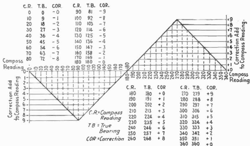
FIG. 210.—Correction curve.
