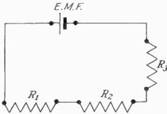
FIG. 11.—A series circuit with three resistances.
