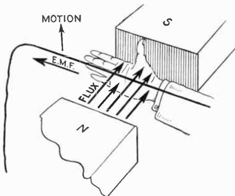
FIG. 17b.—Right-hand rule for direction of e.m.f.
