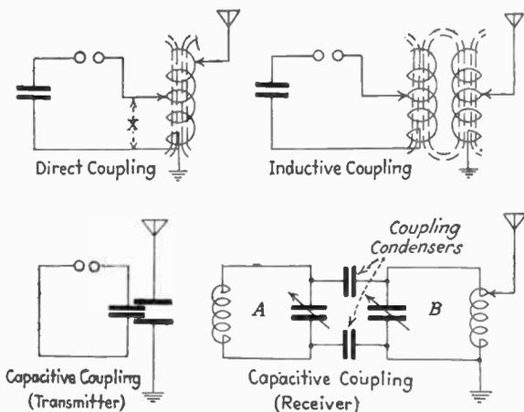
FIG. 89.—Methods of coupling the transmitter.
