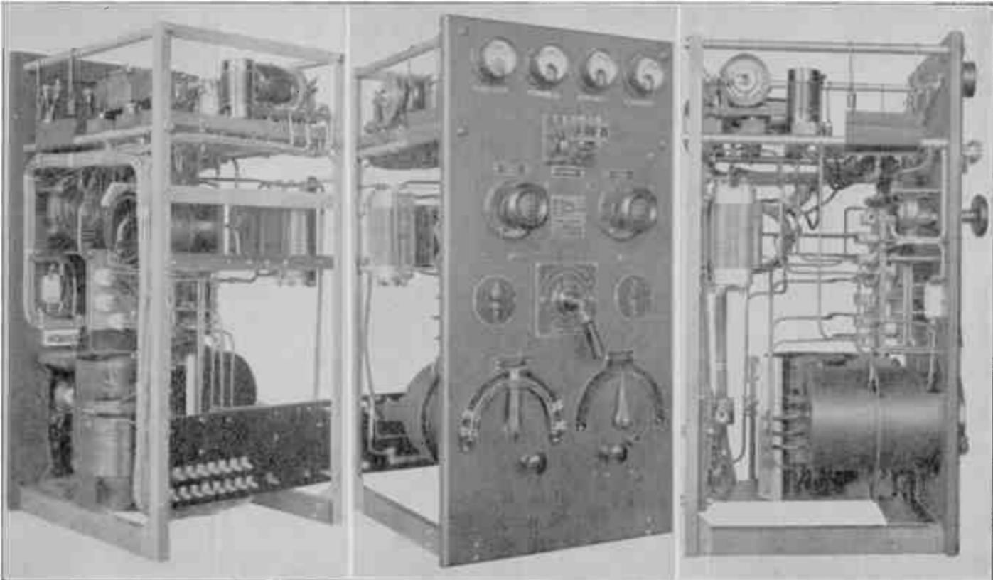
FIG. 162 *a, b, c*.—Rear, front and side views of R.C.A. 200 watt transmitter ET3627A.
