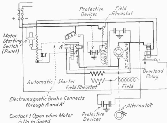
FIG. 35.—Automatic motor starter.
