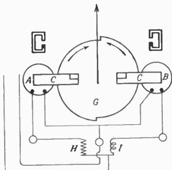
FIG. 56.—Principle of frequency meter.
