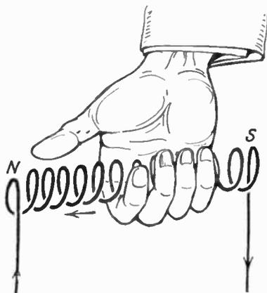
FIG. 17a.—Right-hand rule for polarity of solenoid.
