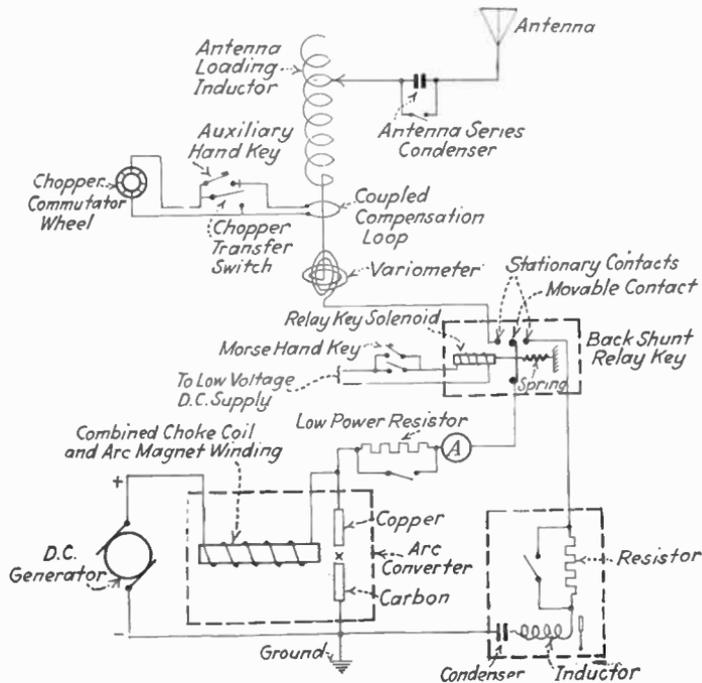
FIG. 138.—“Back-shunt” signaling system.
