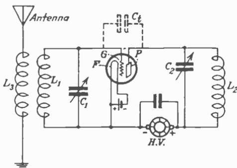
FIG. 134.—Tuned-plate and tuned grid-circuit.
