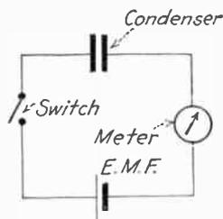
FIG. 74.—Meter connection for showing displacement current.
