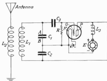
FIG. 135.—Colpitts circuit.
