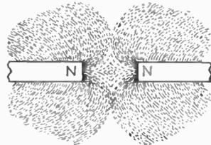
FIG. 2*b*.—Magnetic repulsion between two like poles.
