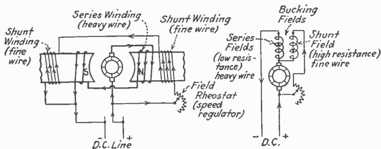
FIG. 31.—A differentially wound compound motor.
