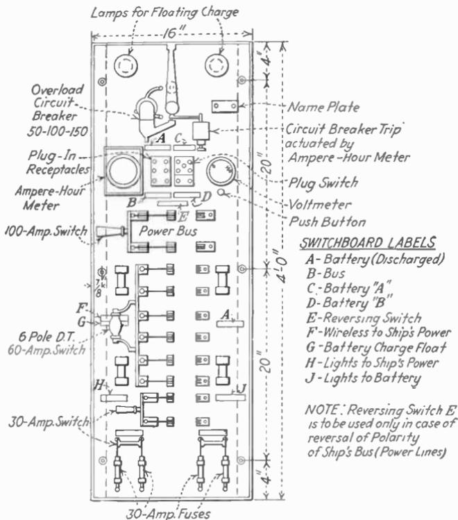
FIG. 66.—Front of switchboard (emergency equipment).
