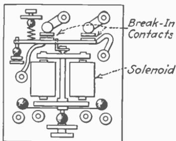
FIG. 164.—Leach break-in relay.
