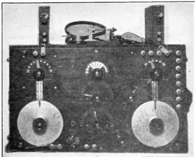
FIG. 167.—Navy standard type S.E. 143 tuner.
