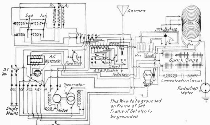
FIG. 191.—Cutting and Washington 2-kw. transmitter circuit diagram.
