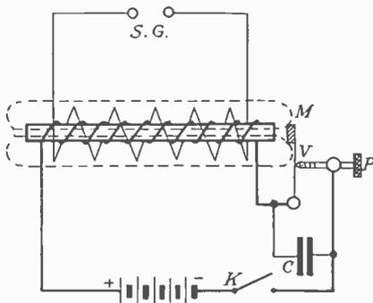
FIG. 70b.—Wiring diagram of an induction coil.
