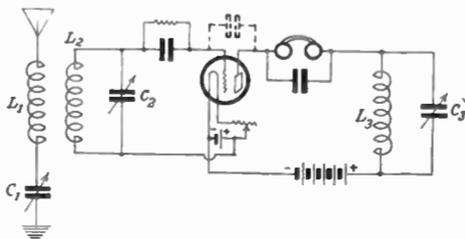
FIG. 129.—Regenerative circuit (tuned-plate method).
