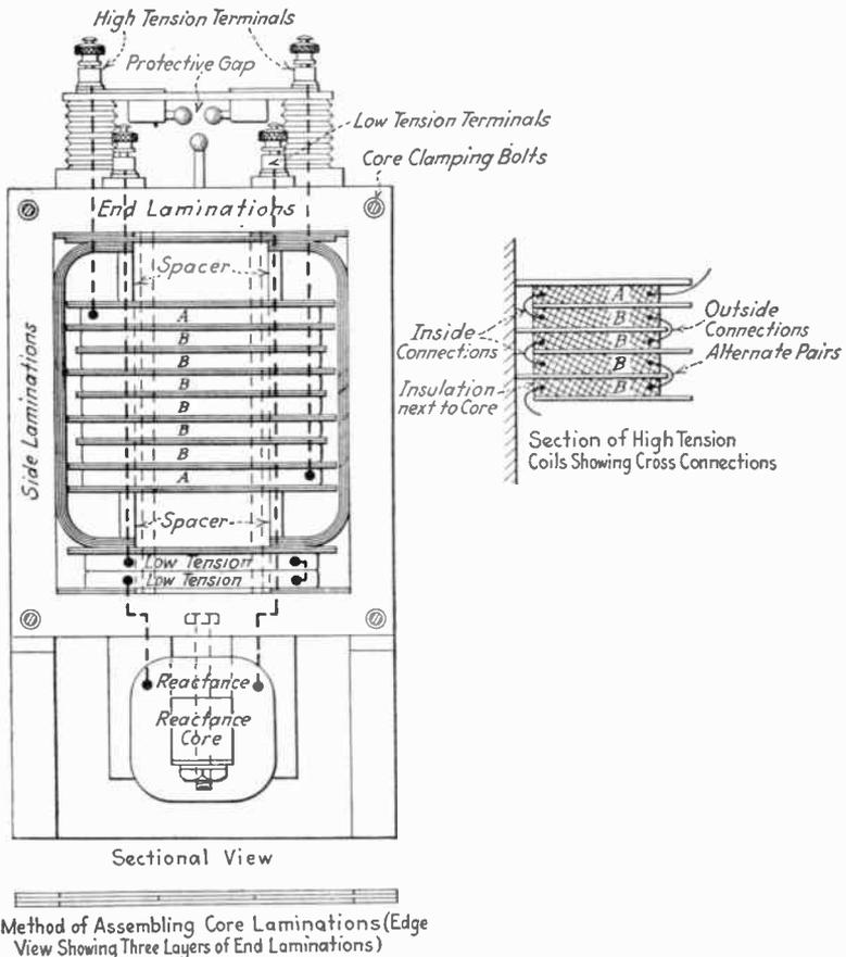
FIG. 71b.—Assembly and connections of a standard transformer.
