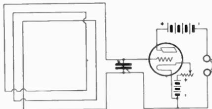
FIG. 204.—Simple radio compass.
