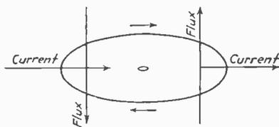
FIG. 63.—Results of current flow in watt-hour meter.
