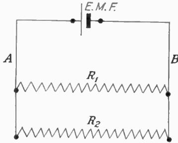
FIG. 12.—A simple parallel circuit (two resistances in parallel).
