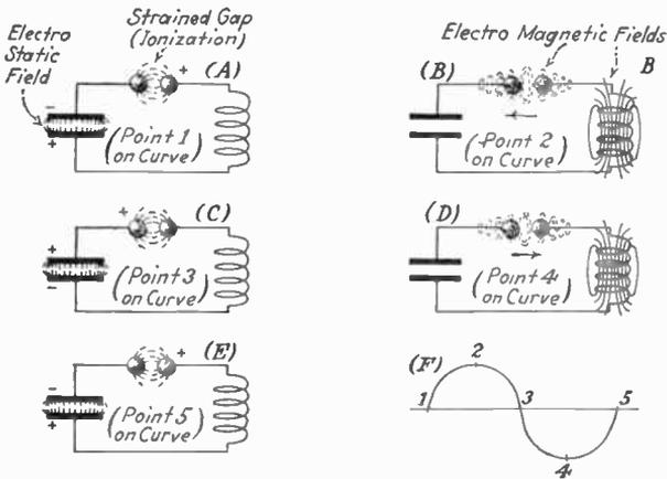
FIG. 85a.—Complete cycle of a condenser charge and discharge.
