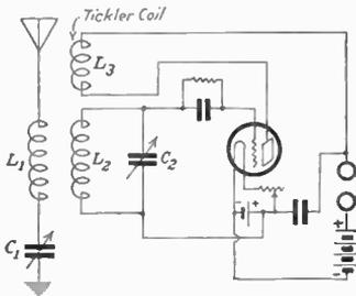
FIG. 127.—Simple regenerative circuit (tickler method).
