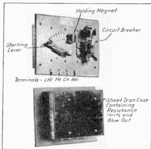
FIG. 151.—Two-kw. motor-starting panel.
