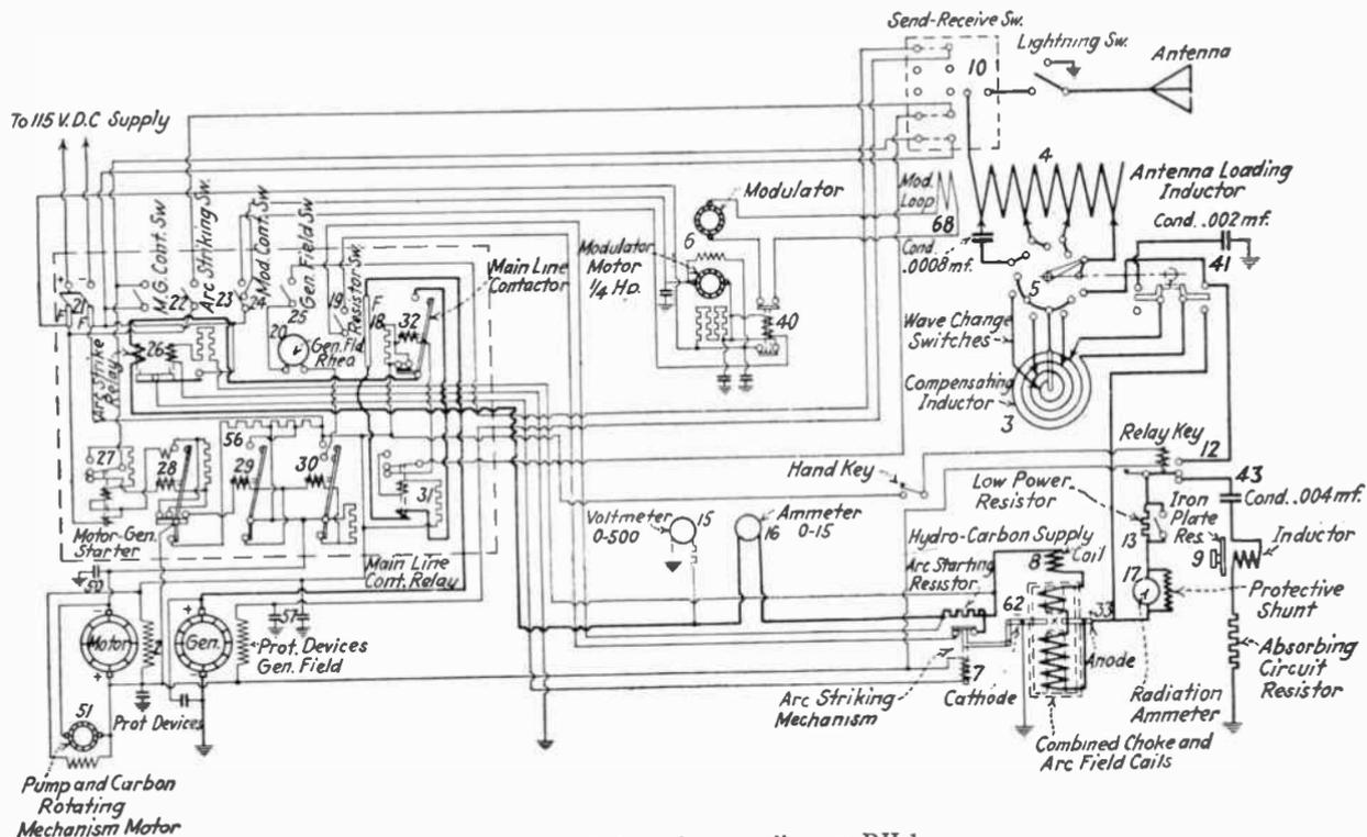
FIG. 157.—Independent arc diagram RH 1.
