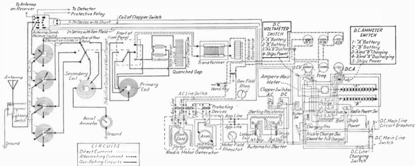
Fig. 192b.—Navy standard 1-kw. spark transmitter circuit diagram.
