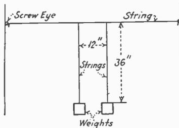
FIG. 93.—Mechanical analogy of coupled circuits.
