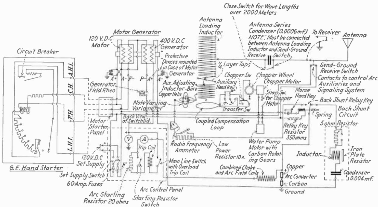
FIG. 153.—Complete Federal arc circuit diagram, type Q.
