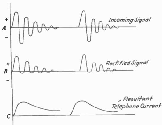
Fig. 108.—Graphs showing rectifying effect of crystal detector.
