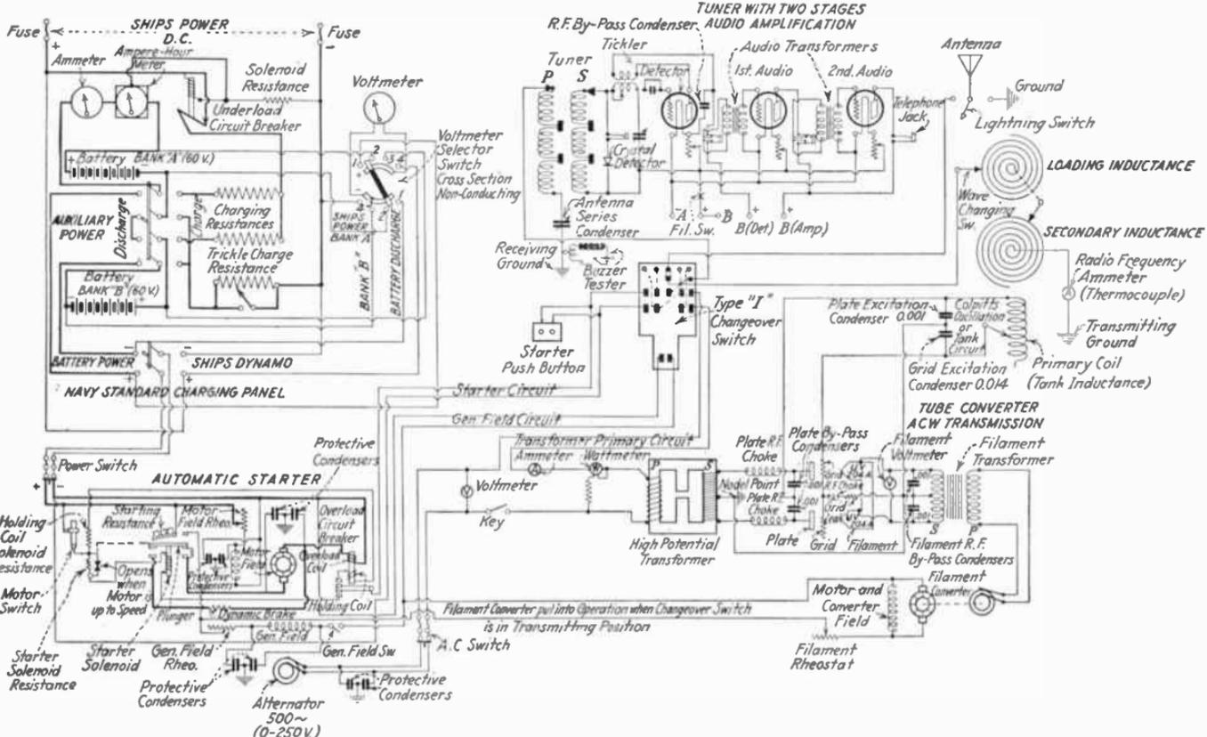
FIG. 161.—Commercial diagram of the P-8 transmitter with tube attachment for the production of full wave A. C. W. transmission.
