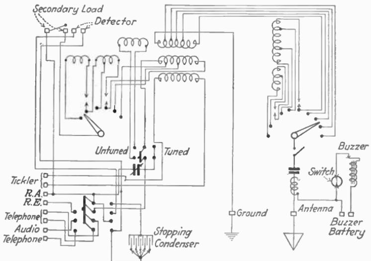
FIG. 194.—Navy standard S.F. 143 tuner circuit diagram.
