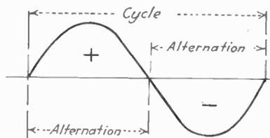
FIG. 20.—One cycle of alternating current.
