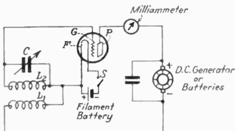
FIG. 131.—Simple vacuum-tube oscillator.
