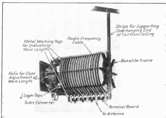
FIG. 144.—Two-kw. antenna-loading inductance.
