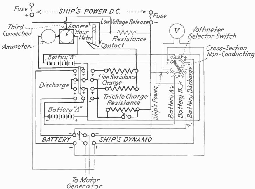
FIG. 68.—Schematic wiring diagram, Navy standard charging panel.
