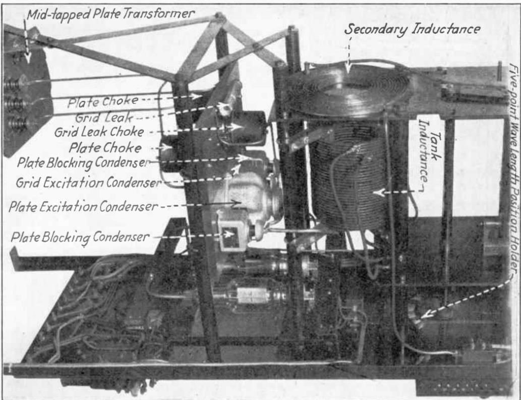
Fig. 160.—P-8 RCA transmitter with tube converter, rear view.
