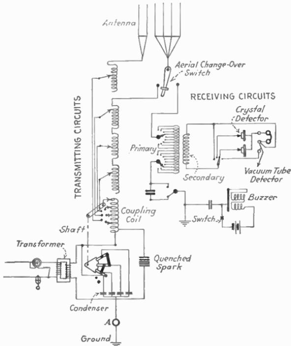
FIG. 180.—Diagram of Simpson radio telegraph transmitter and receiver
