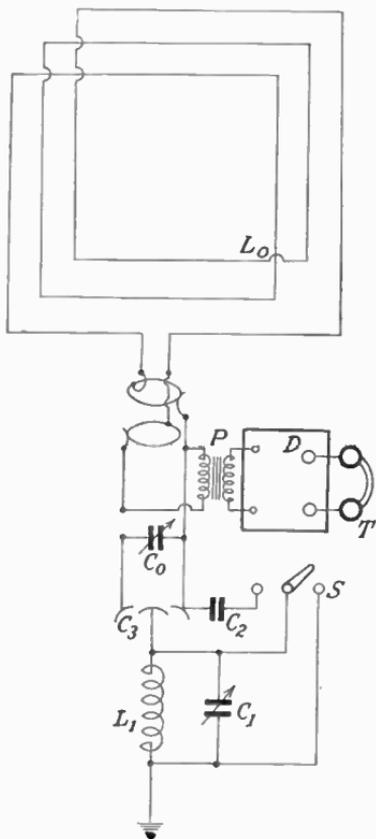
FIG. 209.—Standard radio compass circuit.
