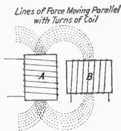
FIG. 18b.—Minimum e.m.f. induced in *B*.
