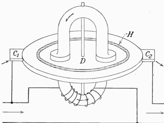
FIG. 62.—Principle of Sangamo ampere-hour meter. (See Fig. 65a.)
