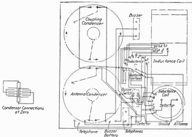
FIG. 185.—Complete wiring diagram independent type A-1 receiver.
