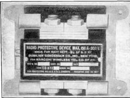
FIG. 69.—Protective condenser.
