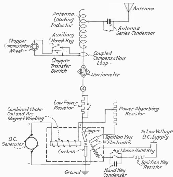
FIG. 139.—“Ignition-key” signaling system.
