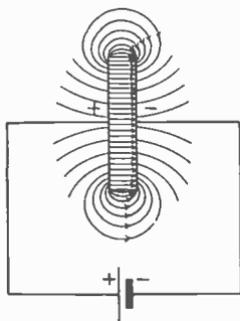
FIG. 73b.—Electrostatic field in a condenser.
