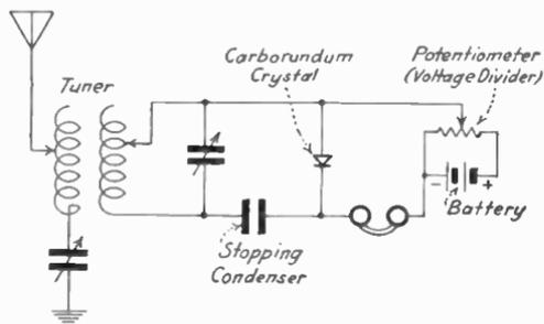
Fig. 109.—Carborundum crystal detector circuit.
