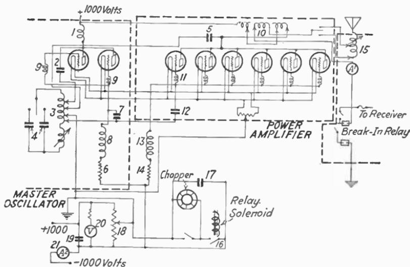
Fig. 166.—Circuit model 3626A tube transmitter RCA.
