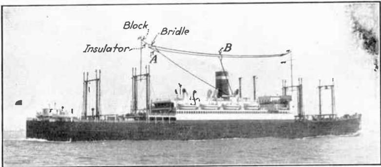
FIG. 100.—*T* or *L* type antenna.
