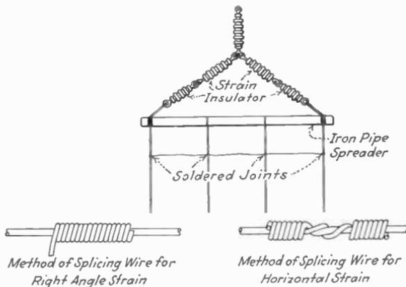
FIG. 103a.—Methods of splicing antenna wire.
