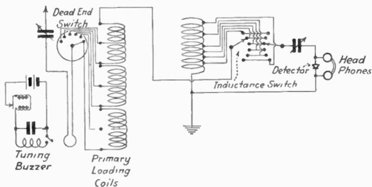
FIG. 189.—Circuit diagram Cutting and Washington receiver.
