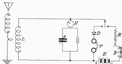
FIG. 177.—Circuit diagram of Kolster decremeter.
