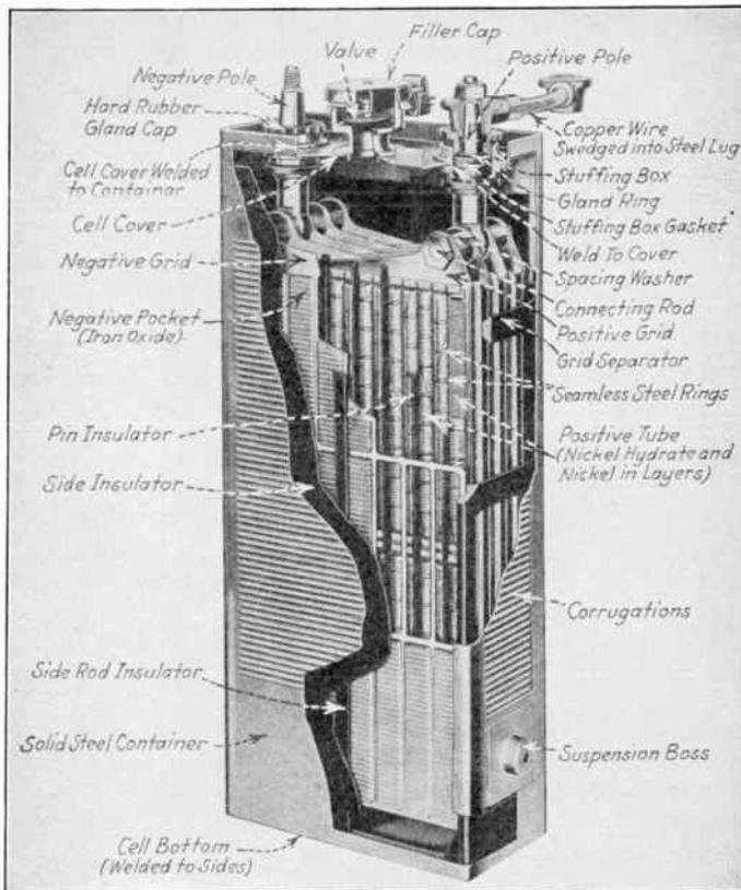
FIG. 48.—Cross-section Edison cell.
