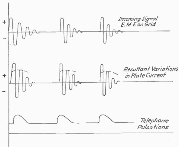
FIG. 125.—Graph of plate rectification without grid condenser.
