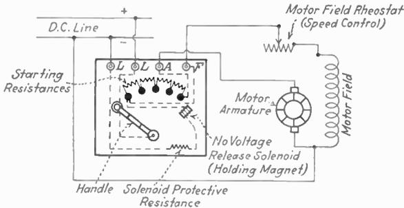
FIG. 32.—General Electric starting box and shunt motor.
