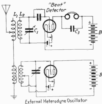
FIG. 130a.—Heterodyne oscillator with beat detector.
