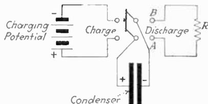
FIG. 78.—Arrangement for charging and discharging a condenser.
