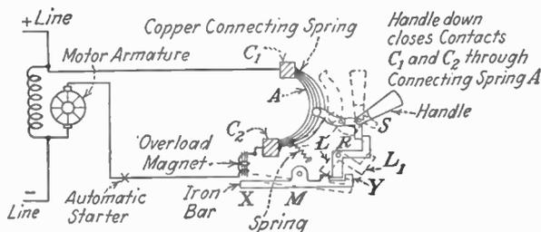
FIG. 64.—Electrical and mechanical arrangement overload circuit breaker.
