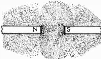
FIG. 2*a*.—Magnetic attraction between two unlike poles.
