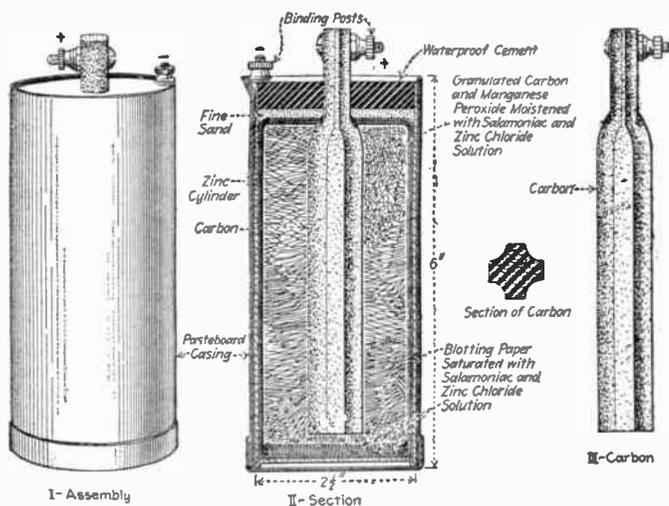
FIG. 37.—The simple primary dry cell.
