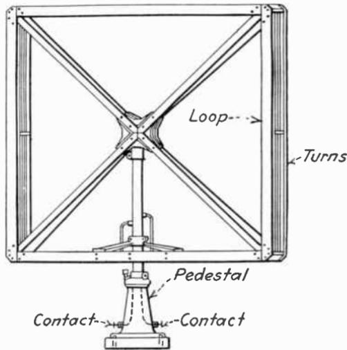
FIG. 102.—Loop antenna.
