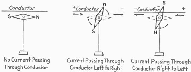
FIG. 14.—Magnetic field about a wire carrying current.
