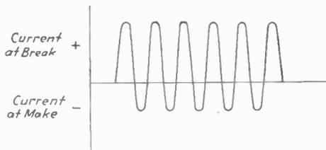
FIG. 70*a*.—Alternating-current wave form, induction coil.
