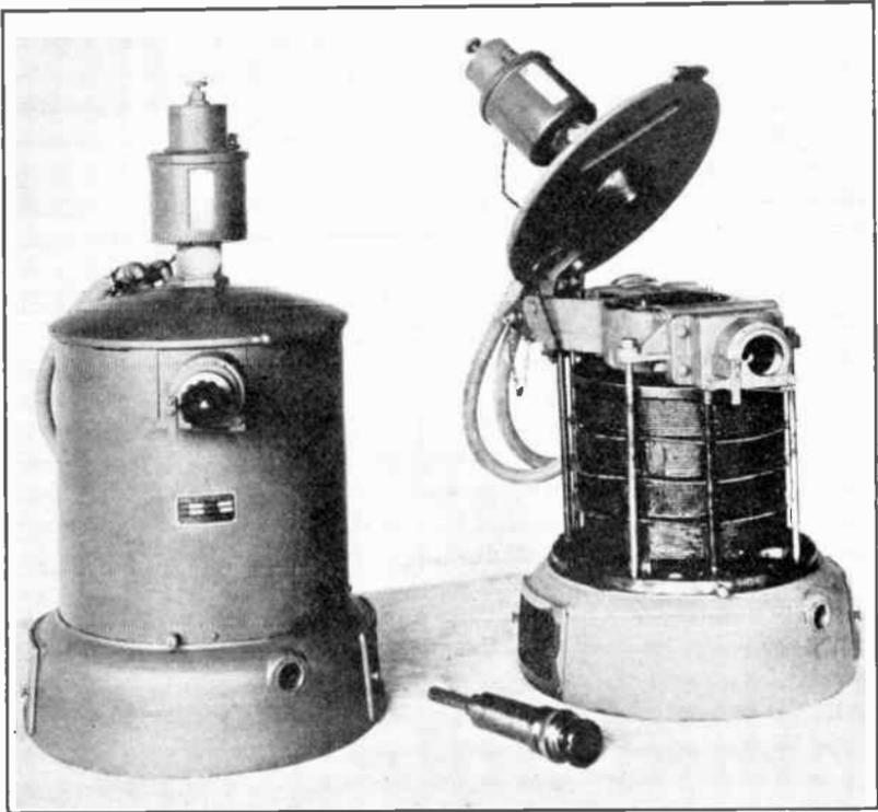
FIG. 155c.—Federal two-kw. arc converter unit type CM 1201.
