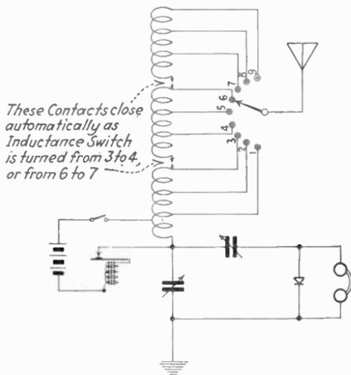
FIG. 183.—Schematic circuit diagram independent receiver, type A-1.
