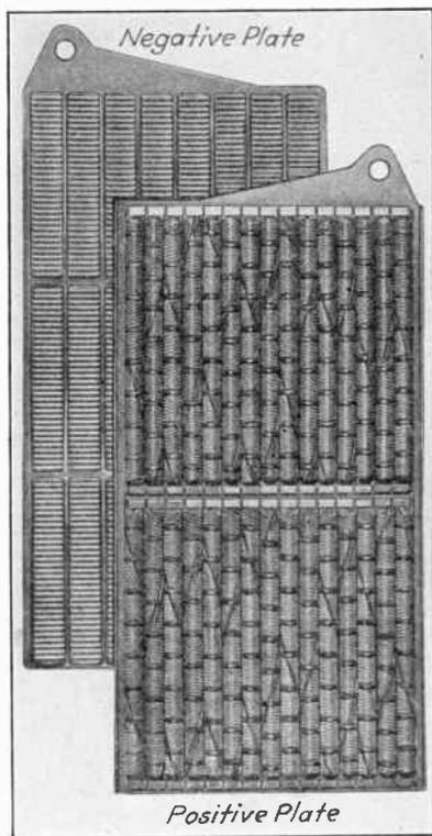
FIG. 49.—Plates of an Edison cell.
