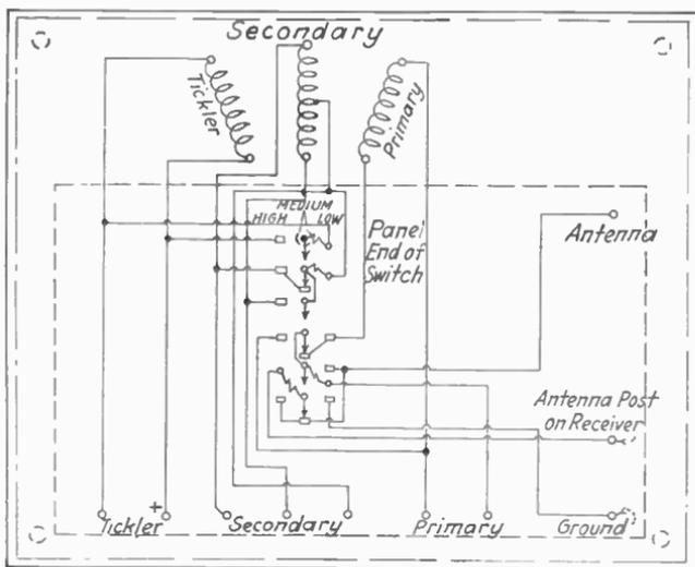
FIG. 199.—R.C.A. long wave attachment for IP501 receiver.
