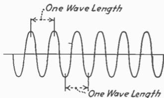
FIG. 88.—Illustrating one wave length.
