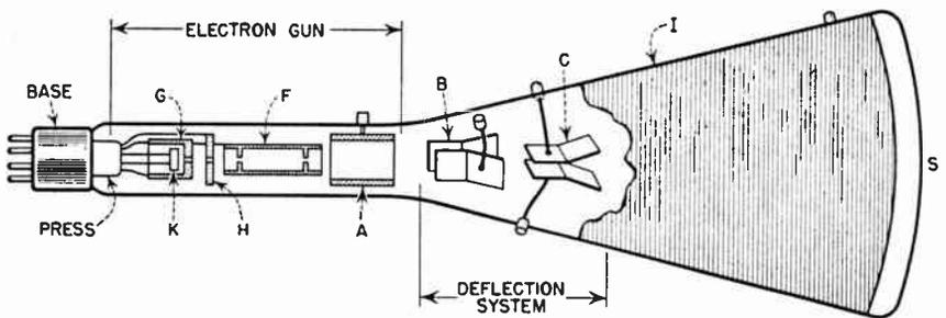
FIG. 2.1 Cathode-ray tube employing electrostatic deflection system.
