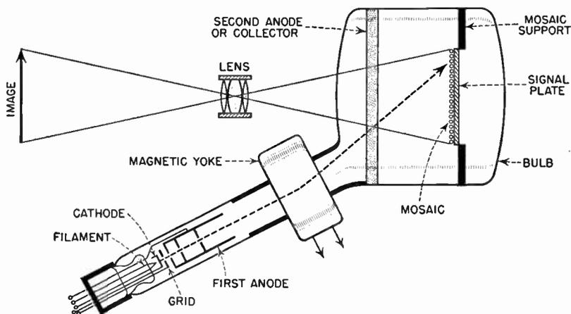
FIG. 4.2 Schematic diagram of R.C.A. Iconoscope.
