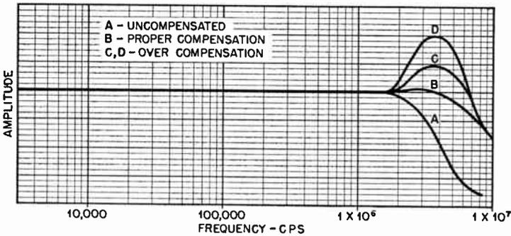
FIG. 6.12 Curves illustrating the effects of high-frequency compensation upon the band-pass characteristic of a video amplifier.
