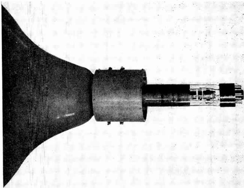
FIG. 8.64 Magnetic deflection yoke about the neck of a cathode-ray tube. (Courtesy of Allen B. Du Mont Labs., Inc.)
