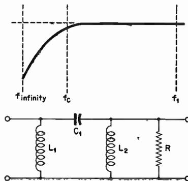
HIGH PASS FILTER AND CURVE INDICATING TRANSMISSION CHARACTERISTIC
