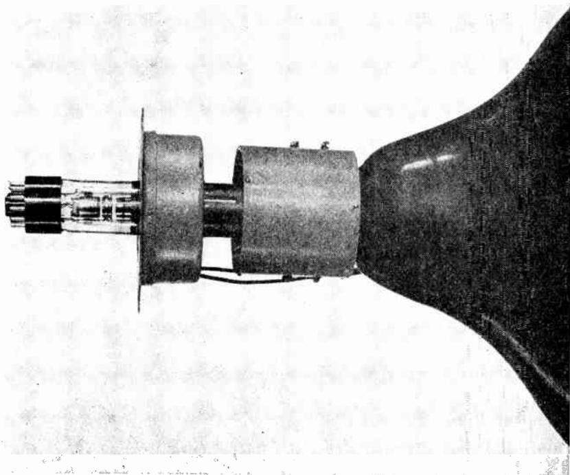
FIG. 2.23 Focusing coil and magnetic-deflection yoke in relative positions about the neck of the cathode-ray tube gun. The focusing coil is located in the direction of the tube's base. The deflection yoke is at the upper end of the gun assembly, near the large glass bulb of the tube. (Courtesy of Allen B. Du Mont Labs., Inc.)
