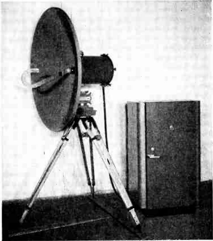
FIG. 9.27 R.C.A.'s microwave-link equipment for television relaying. (Courtesy of Radio Corporation of America.)
