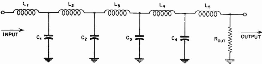
Fig. 5.41 Multisection low-pass filter used as a time-delay network in the television system.
