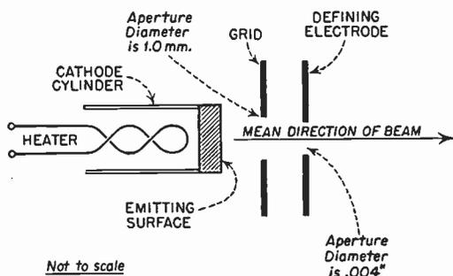
FIG. 4.14 Schematic diagram of Orthicon gun construction.
