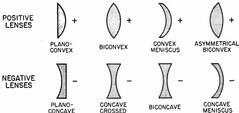
FIG. 1.7 The eight typical lens elements used in various combinations to construct the television camera lens.
