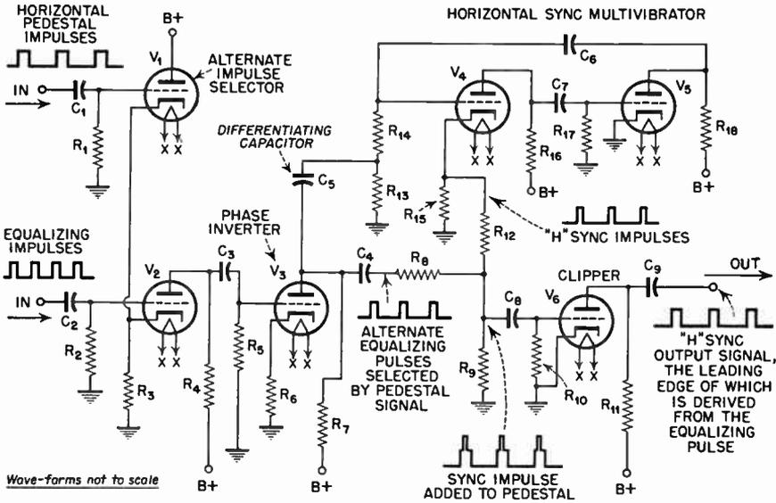
FIG. 5.43 System employed to generate the horizontal synchronizing impulse.
