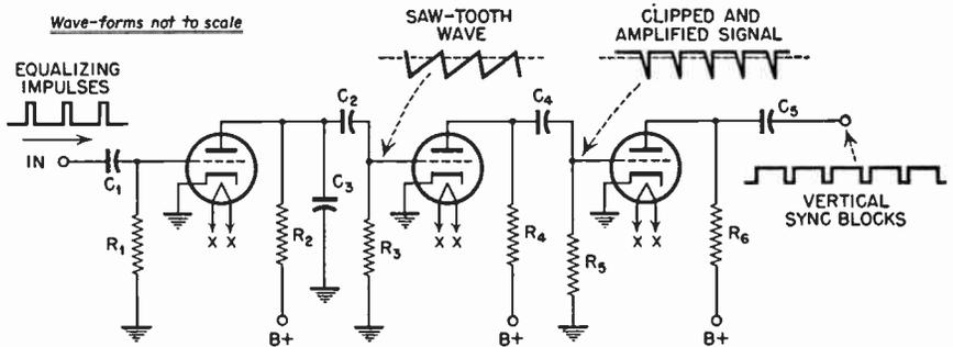
FIG. 5.44 Circuit used in generating and shaping the vertical synchronizing blocks.
