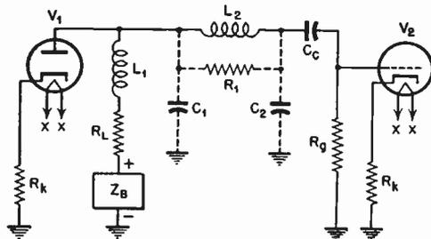
FIG. 6.18 Simple electrical equivalent of combination peaked video stage.
