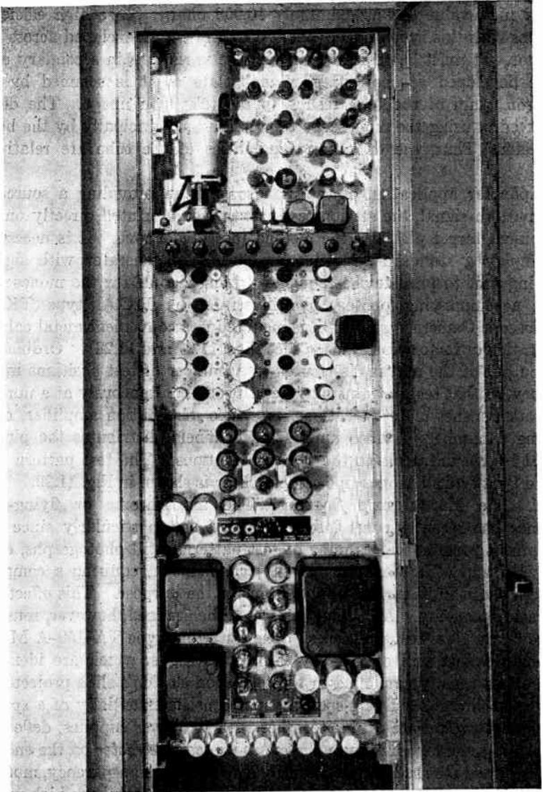
FIG. 11.27 Television test unit for broadcast stations and production lines. (Courtesy of Radio Corporation of America.)
