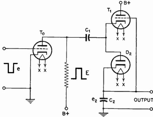
200 : 1. By increasing the negative bias potential, this ratio can be increased, the limit to which the count-down ratio can be extended being a function of permissible grid bias. In a commercial version of this counter-circuit timer, two such counters were employed to achieve a
