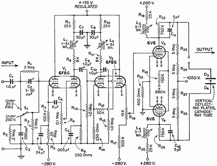
FIG. 3.5 Vertical deflection and parphase amplifiers, Du Mont type 208 oscillograph.
