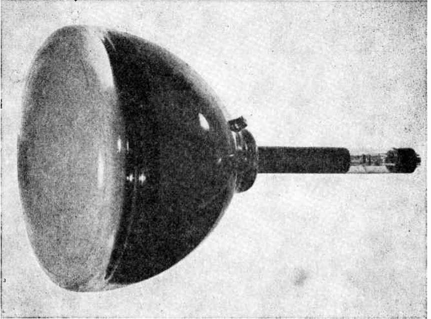
FIG. 2.13 Du Mont type 12DP4 12-in. television cathode-ray tube requiring electromagnetic deflection and focusing. The conductive electrical coating imparted to the inner walls of the envelope may be clearly seen. (Courtesy of Allen B. Du Mont Labs., Inc.)
