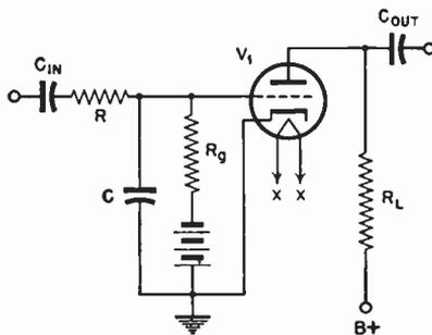
FIG. 5.32 Integrating, or delaying, circuit.
