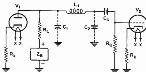
Fig. 6.16 Electrical equivalent of series-peaked video stage.
