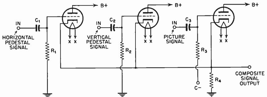
FIG. 5.55 Diagram of one method by which the horizontal pedestal signal may be modulated by the vertical blanking signal and mixed with the picture signal.
