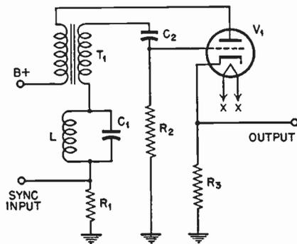
FIG. 5.14 Blocking-tube oscillator employing resonant stabilizer.
