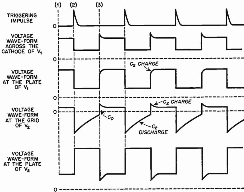
FIG. 5.8 Waveforms present in the one-shot multivibrator.
