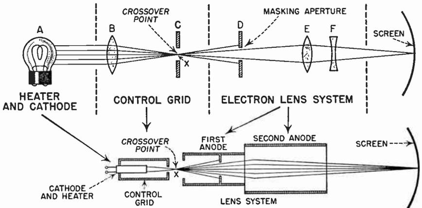
FIG. 2.11 Comparison of optical and electron focusing systems.
