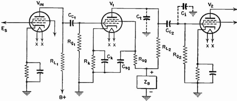
FIG. 6.3 Conventional  $RC$ -coupled amplifier stage.
