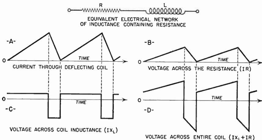
FIG. 4.6 Diagram of the development of the voltage waveform necessary to produce saw-toothed current in a coil containing resistance.
