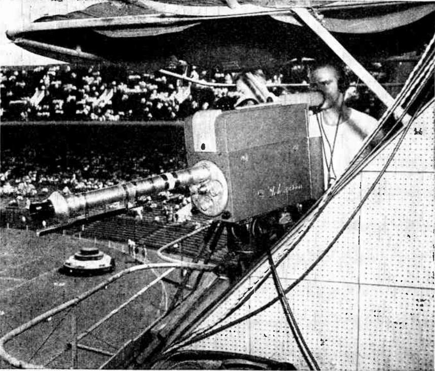
FIG. 1.20 Zoomar lens as mounted on the turret of an R.C.A. Image Orthicon field camera and as first used in televising a football game. (Courtesy of Station WFIL-TV, Philadelphia.)
