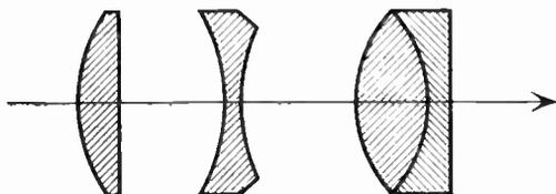
FIG. 1.8 The camera lens for one type of Eastman Ektar (f/3.5, 10.7 cm.). The television camera lens is constructed of a number of lens elements.
