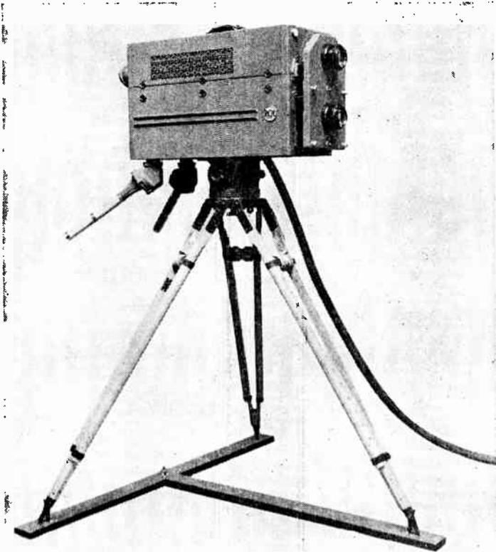
FIG. 4.13 Early R.C.A. field camera for use with the Orthicon pickup tube. (Courtesy of Radio Corporation of America, Tube Division.)
