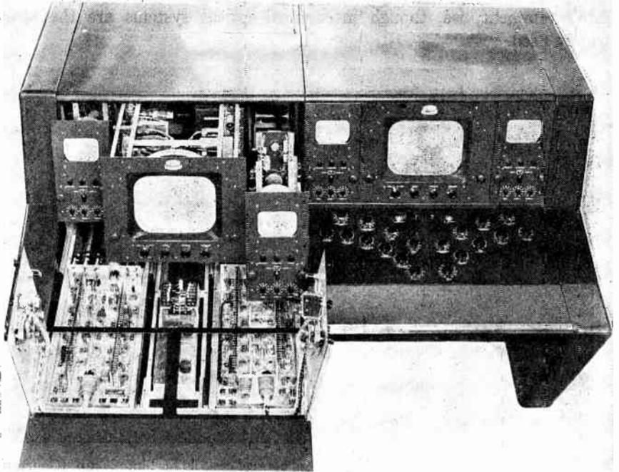
FIG. 9.26 The various units on "railways" so that they may be pulled out for inspection or servicing. (Courtesy of Allen B. Du Mont Labs., Inc.)
