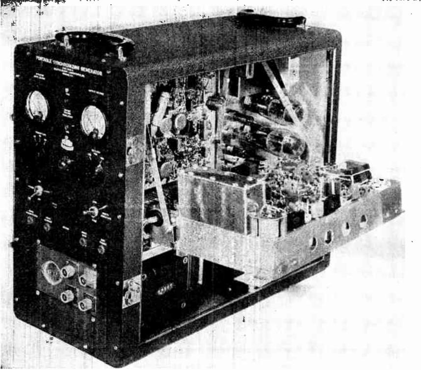
FIG. 9.21 The Du Mont portable synchronizing generator with side panels removed and chassis in position for servicing. (Courtesy of Allen B. Du Mont Labs., Inc.)
