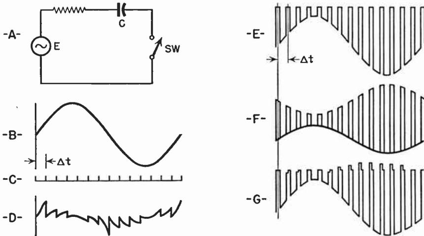
FIG. 5.62 An idealized clamping circuit and pertinent waveforms.
