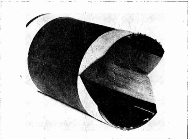
FIG. 4.23 Horizontal deflection coil used with the Farnsworth Image Dissector. The unique construction results in excellent horizontal scanning. (Courtesy of Farnsworth Television and Radio Corp.)
