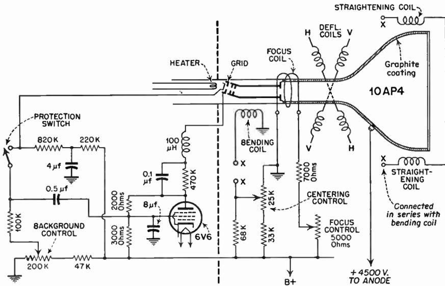
FIG. 2.35 Bent-gun type of cathode-ray tube and associated circuits.
