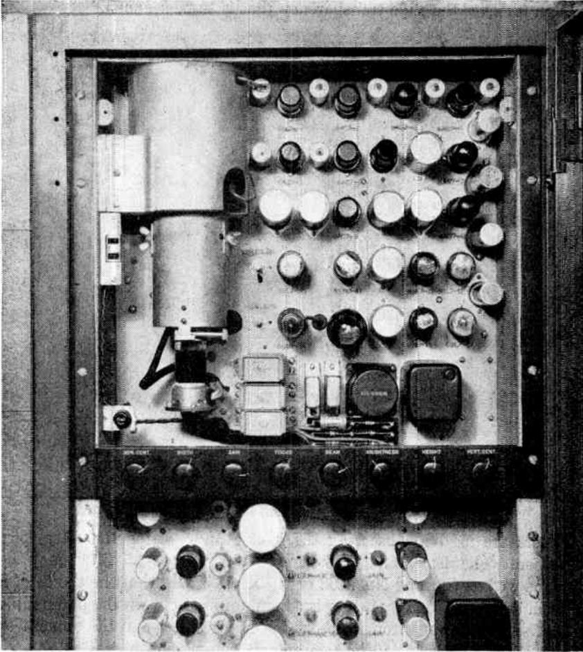
FIG. 11.28 R.C.A. Monoscope camera aids quality testing of television equipment. (Courtesy of Radio Corporation of America.)
