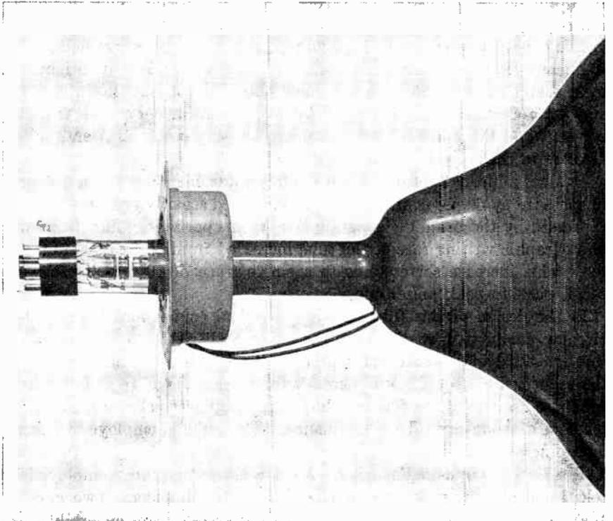
FIG. 2.18 Electromagnetic focusing coil in position along the neck of the cathode-ray tube gun. (Courtesy of Allen B. Du Mont Labs., Inc.)
