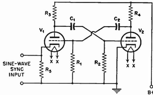
FIG. 5.11 Multivibrator in which the sine-wave synchronizing voltage is applied to the cathode.
