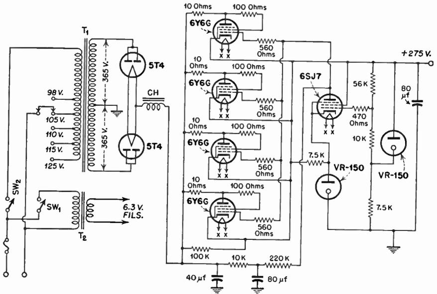
FIG. 5.29 Regulated power supply providing d-c potential to a portable television synchronizing generator.
