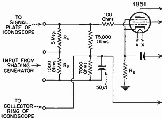
FIG. 5.48 Diagram of the method of introducing shading voltages at low level in the video system.
