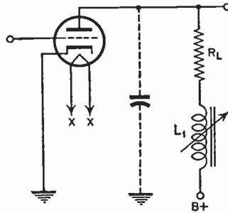
FIG. 3.9 High-frequency plate-circuit compensation.
