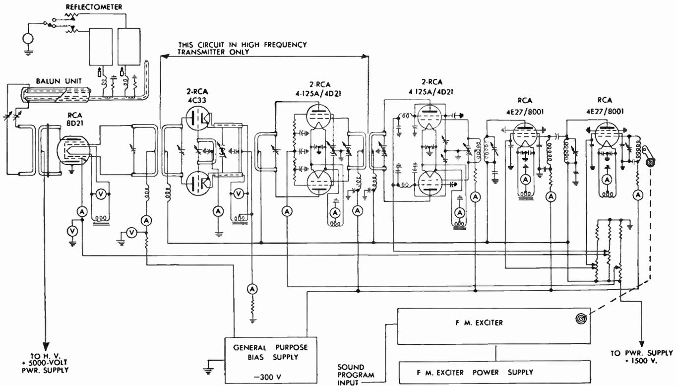
FIG. 10.14 Schematic of R.C.A. TT-5A sound transmitter.
