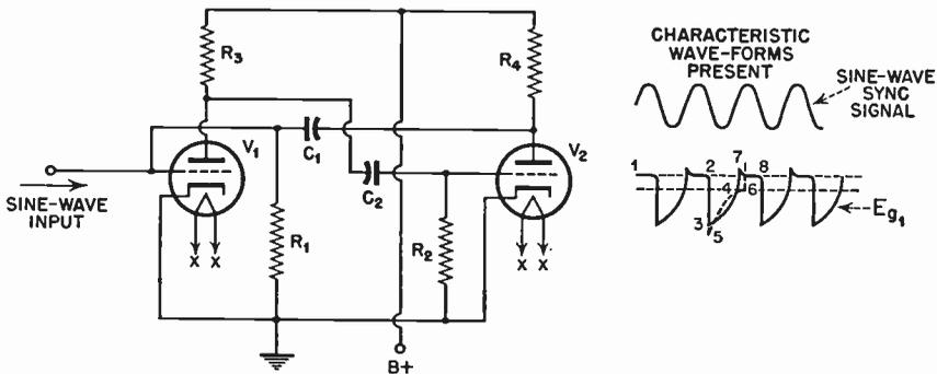
FIG. 5.10 Simple multivibrator synchronized with sine-wave signal.
