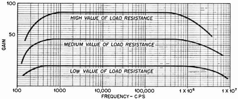
Fig. 6.8 Variation of voltage amplification with frequency in a typical video amplifier stage as the value of plate-load resistance ( $R_L$ ) is changed.
