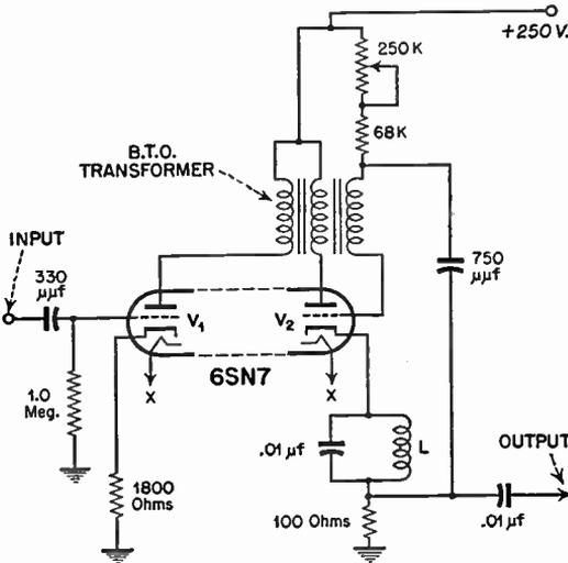
FIG. 5.17 Cathode-stabilized blocking-tube oscillator, as used in the timing unit of a Du Mont synchronizing generator.
