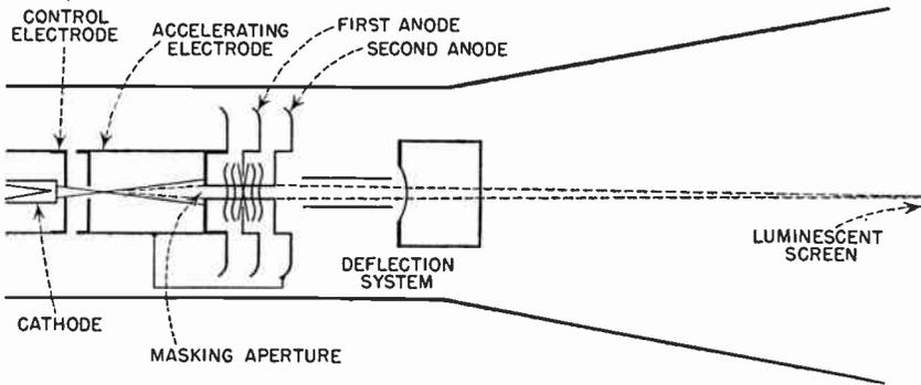
FIG. 2.21 Improved gun design based on zero first-anode current. (After L. E. Swedlund, Radio Corporation of America.)
