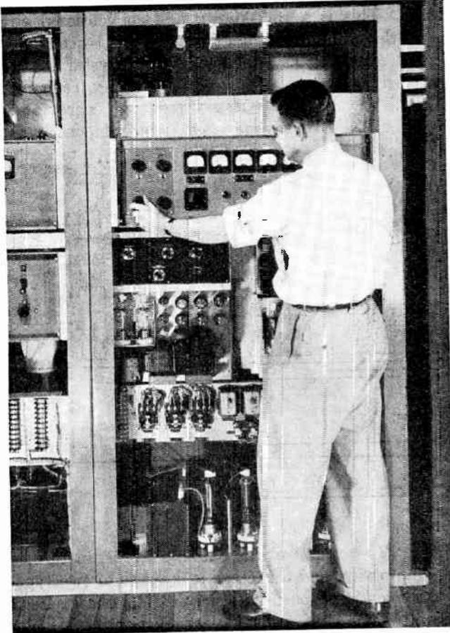
FIG. 10.5 Tuning up the video exciter unit of the Du Mont master series TV transmitter. The front panels and "skin" have been removed to facilitate final factory test. (Courtesy of Allen B. Du Mont Labs., Inc.)
