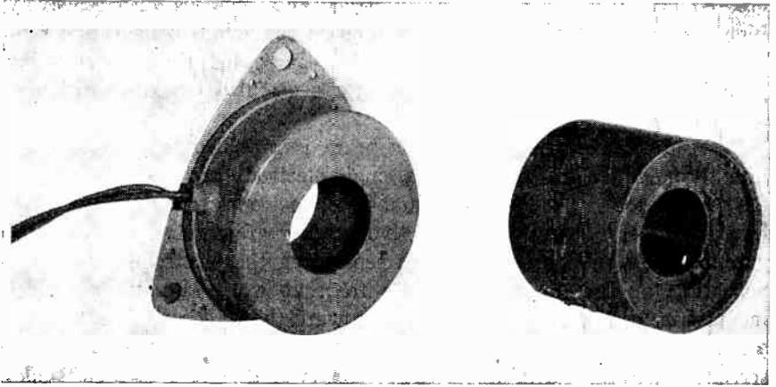
FIG. 2.17 Left, a typical electromagnetic focusing coil; right, the magnetic-deflection yoke. (Courtesy of Allen B. Du Mont Labs., Inc.)
