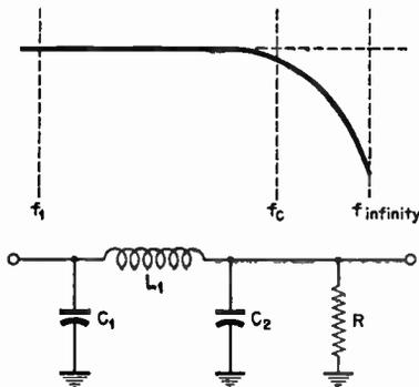
LOW PASS FILTER AND CURVE INDICATING TRANSMISSION CHARACTERISTIC
