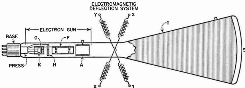
•FIG. 2.4 Cathode-ray tube employing electromagnetic deflection system.
