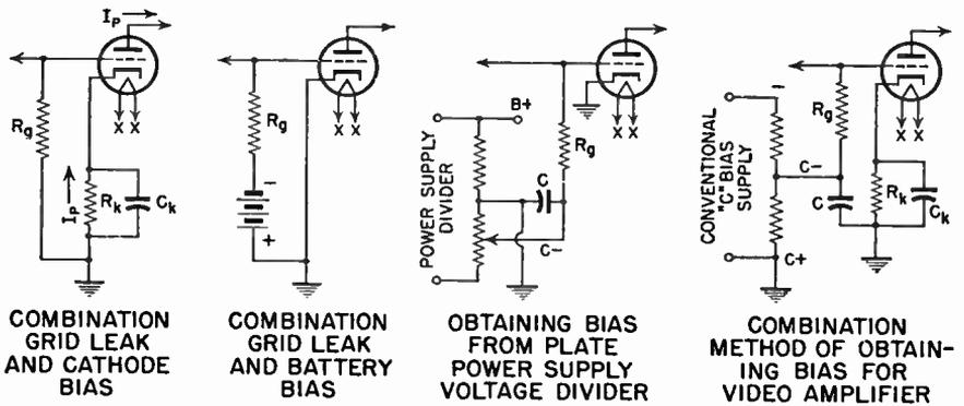
FIG. 6.10 Diagrams of four methods of obtaining bias for the video amplifier.
