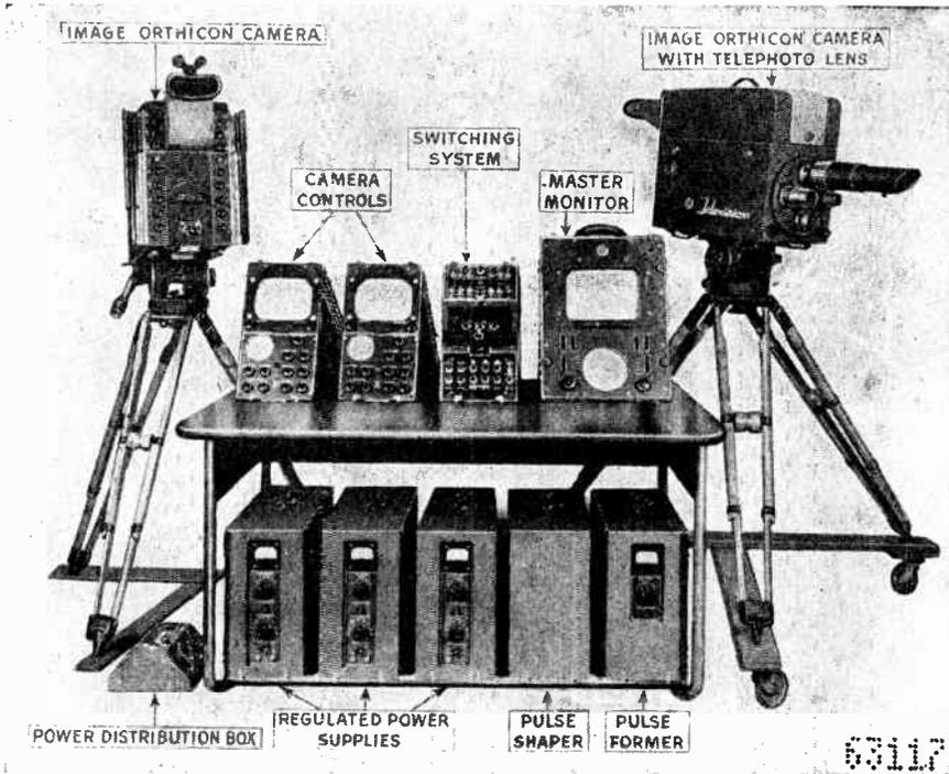
Fig. 9.1 An R.C.A. dual Image Orthicon camera chain. (Courtesy of R.C.A.-Victor.)
