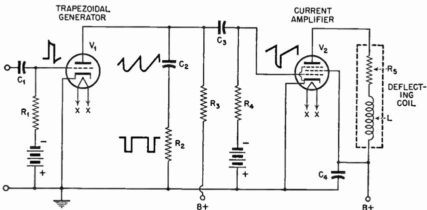
FIG. 4.7 Circuit for development of saw-toothed current wave required for electromagnetic deflection.
