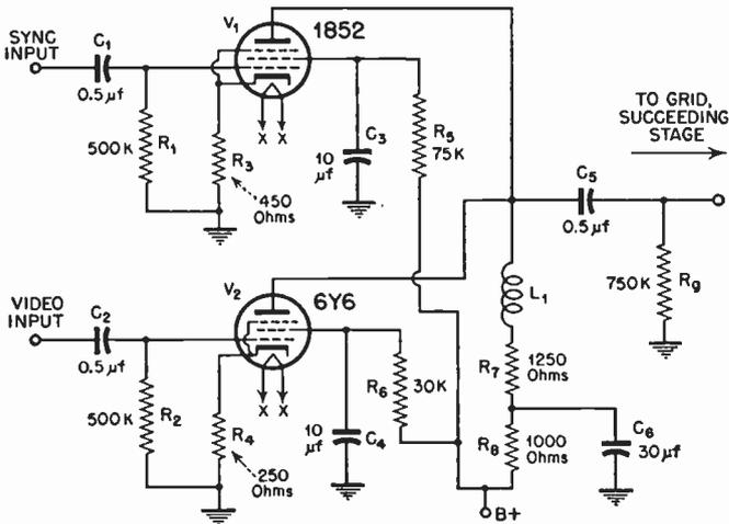
FIG. 5.49 Circuit employed in mixing video and synchronizing voltages.
