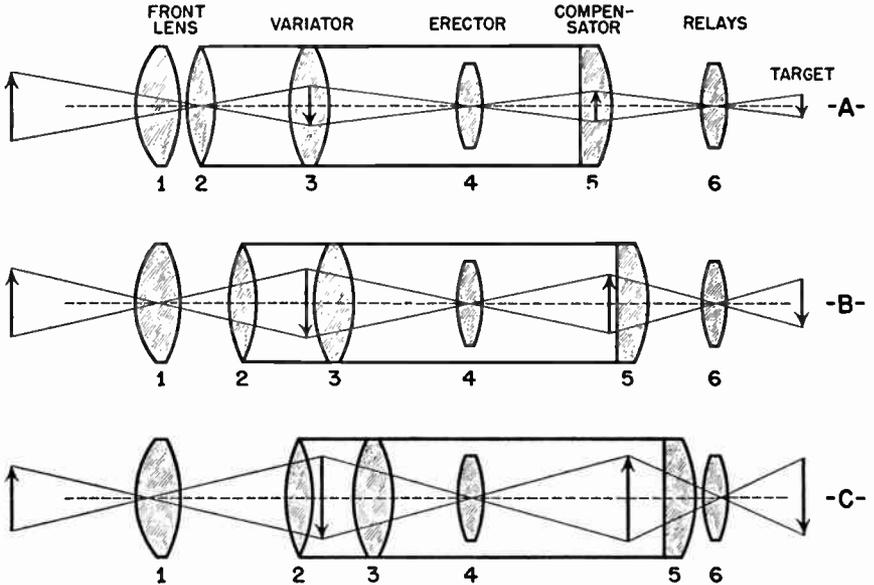
FIG. 1.21 Simplified schematic of the Zoomar lens in three operating positions: wide angle, medium, and telephoto.
