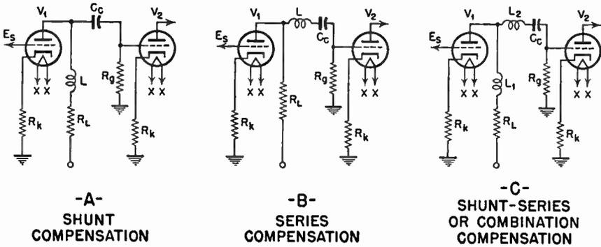
FIG. 6.11 Diagrams of three methods of high-frequency compensation.
