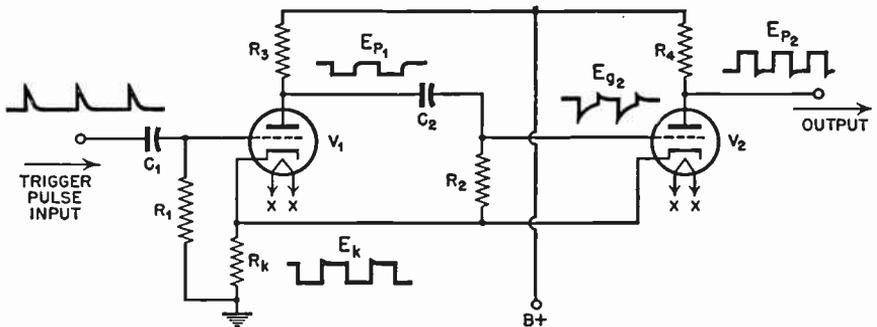
FIG. 5.7 Modified Eccles-Jordan multivibrator circuit.
