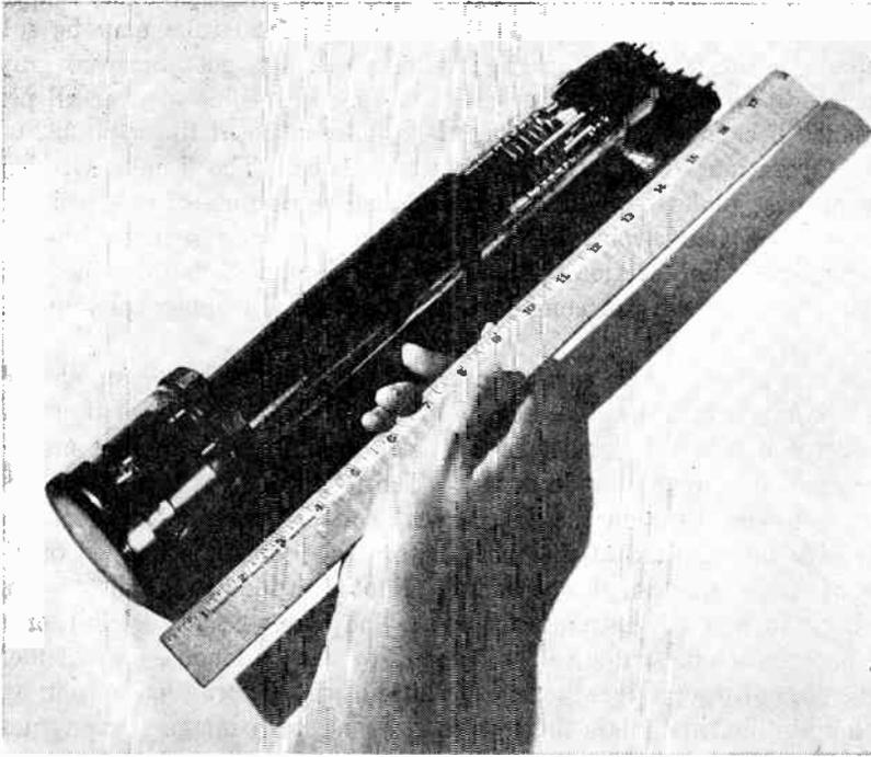
FIG. 4.16 Early commercial version of the Image Orthicon. (Courtesy of Radio Corporation of America, Tube Division.)
