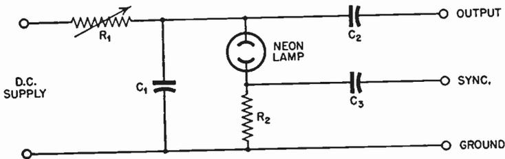
Fig. 3.2 Elementary neon time base.
