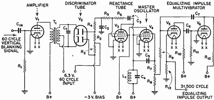
FIG. 5.26 Automatic-frequency-control system of a television synchronizing generator and the equalizing impulse multivibrator.
