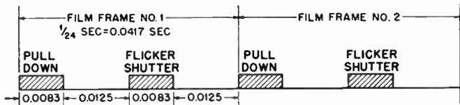
A. 35-MM MOTION PICTURE PROJECTOR WITH 72 DEGREE SHUTTER, 24 FRAMES PER SECOND
