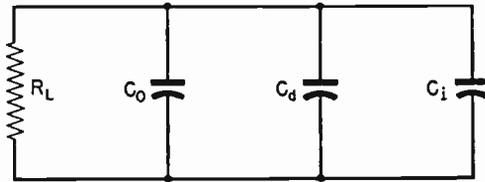
FIG. 6.13 Diagram of an equivalent network, combining  $R_L$ ,  $C_o$ ,  $C_d$ , and  $C_i$  into a common impedance, which effects high-frequency response.
