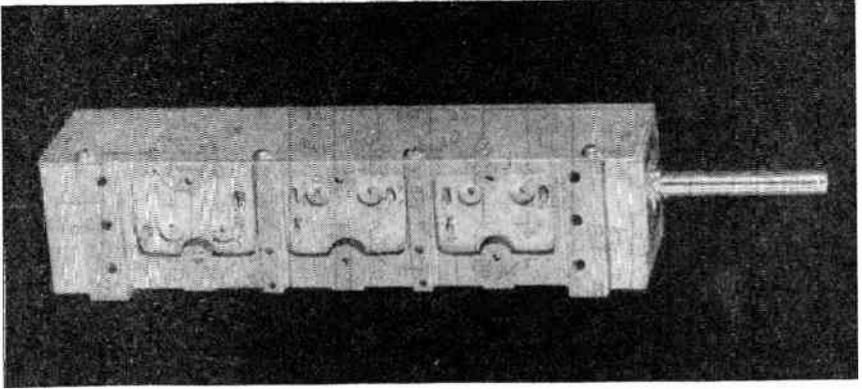
FIG. 8.19 The Inductuner is enclosed in a die-cast housing. The external connections to each coil assembly may be seen. The coils are not grounded. (Courtesy, Allen B. Du Mont Labs., Inc.)
