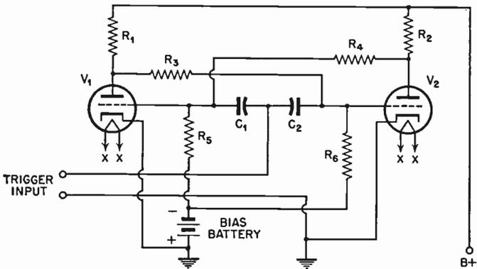
FIG. 5.6 Eccles-Jordan "flip-flop" circuit.
