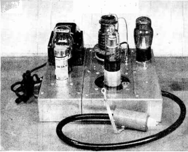
FIG. 8.72 High-voltage radio-frequency power supply, model 10HFP-2. (Courtesy of U.S. Television Corp.)
