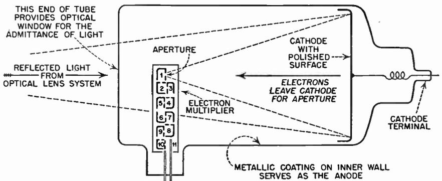
FIG. 4.20 Simplified schematic diagram of the Farnsworth Image Dissector.
