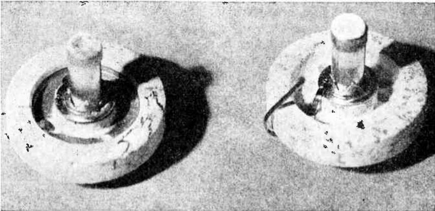
FIG. 2.9 Enlarged photograph of typical cathode construction. The cathode is fixed upon a ceramic support which ensures mechanical rigidity when mounted in the gun assembly. The flat cylindrical end of the cathode is coated with strontium and barium oxides. It is from this surface that the electrons are copiously emitted. (Courtesy of North American Philips Company, Inc.)
