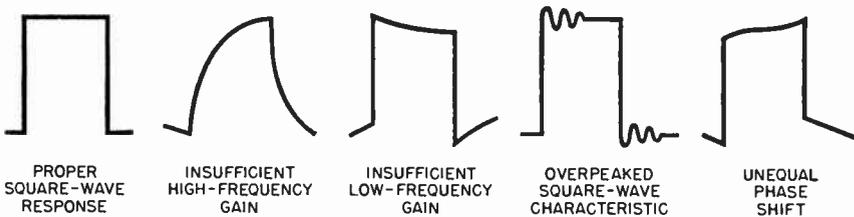
Fig. 3.10 Types of square-wave distortion introduced in poorly designed or adjusted oscillograph or video amplifiers.
