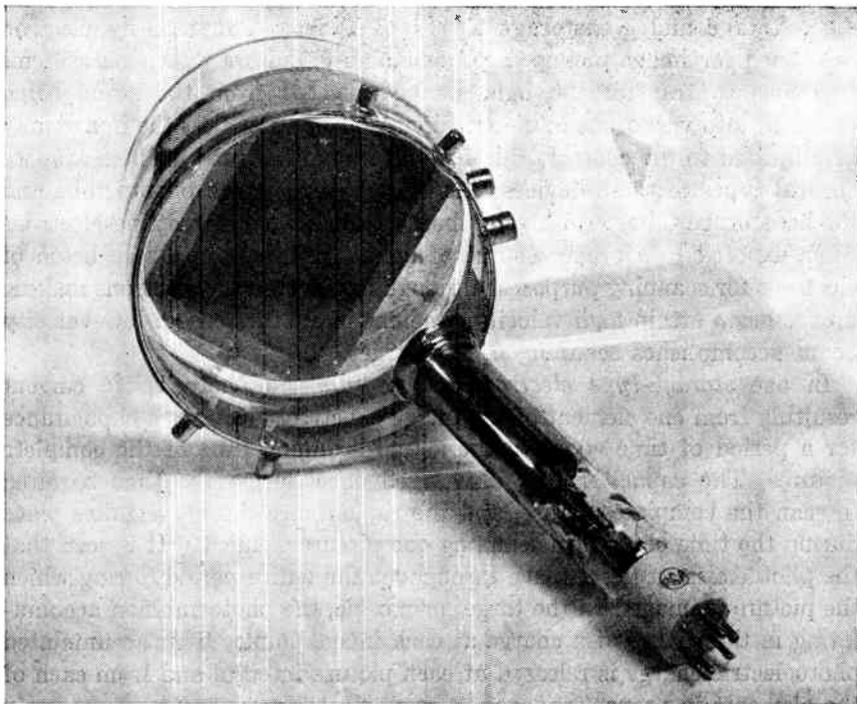
FIG. 4.1 R.C.A. type 1850-A Iconoscope. Location of the sensitive mosaic within the large glass bulb of the device is clearly shown. (Courtesy of Radio Corporation of America, Tube Division.)
