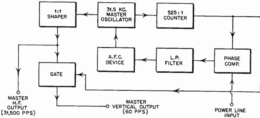
FIG. 5.25 Block diagram of suggested timer using the Hallmark counter.
