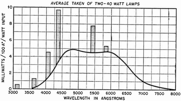
Fig. 1.4A Spectral energy distribution-daylight fluorescent. (Courtesy of General Electric Company, Nela Park, Cleveland.)
