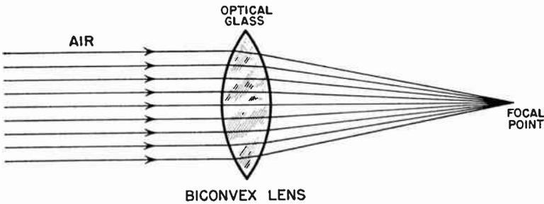
FIG. 1.15 Diagram of the way in which light rays are bent or refracted in passing through a medium of greater density than the density of air.
