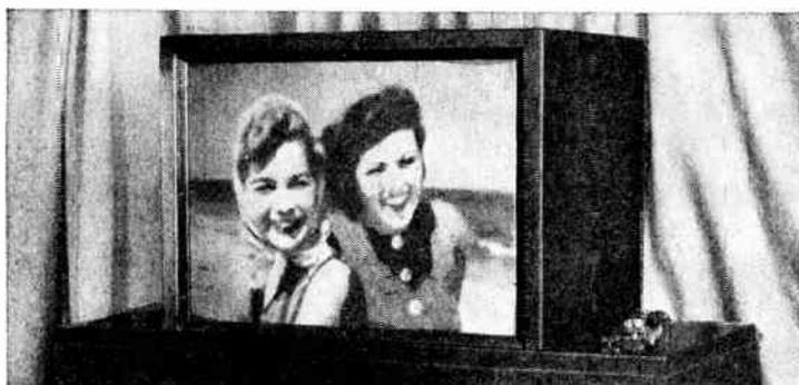
FIG. 8.80 An early R.C.A. projection receiver employing the Schmidt optical system. Only the translucent projection screen is shown here. (Courtesy of Radio Corporation of America.)
