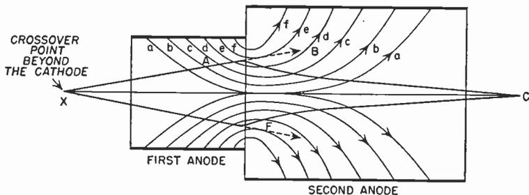
FIG. 2.12 Electrostatic field at first and second anodes.
