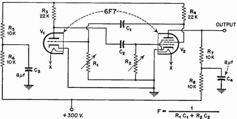
FIG. 5.12 Simple multivibrator circuit.
