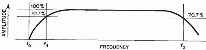
FIG. 6.4 Gain versus frequency characteristic of a typical  $RC$ -coupled amplifier.
