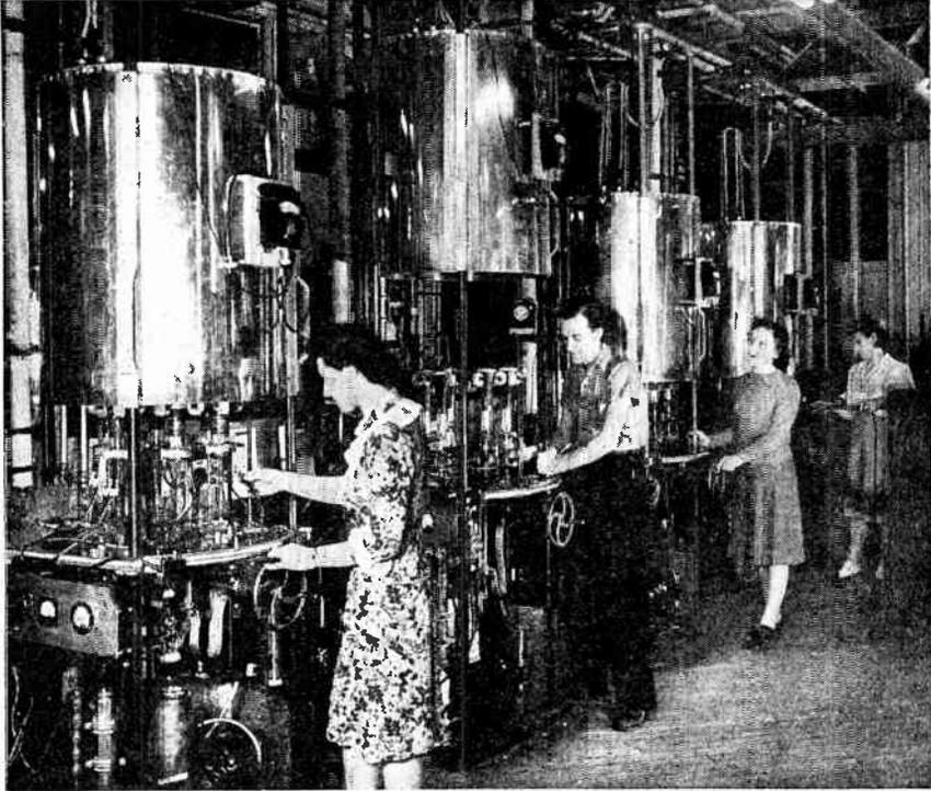
FIG. 2.38 Procedure after sealing. The tubes are baked, the cathodes broken down, and the mount parts radio-frequency bombarded in vacuum to liberate residual gases which are evacuated from the tube. (Courtesy of Allen B. Du Mont Labs., Inc.)
