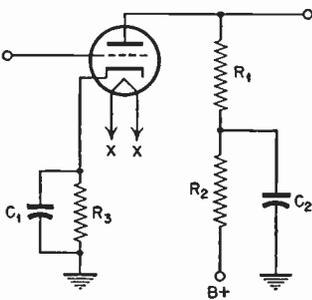
FIG. 3.8 Low-frequency plate-circuit compensation.
