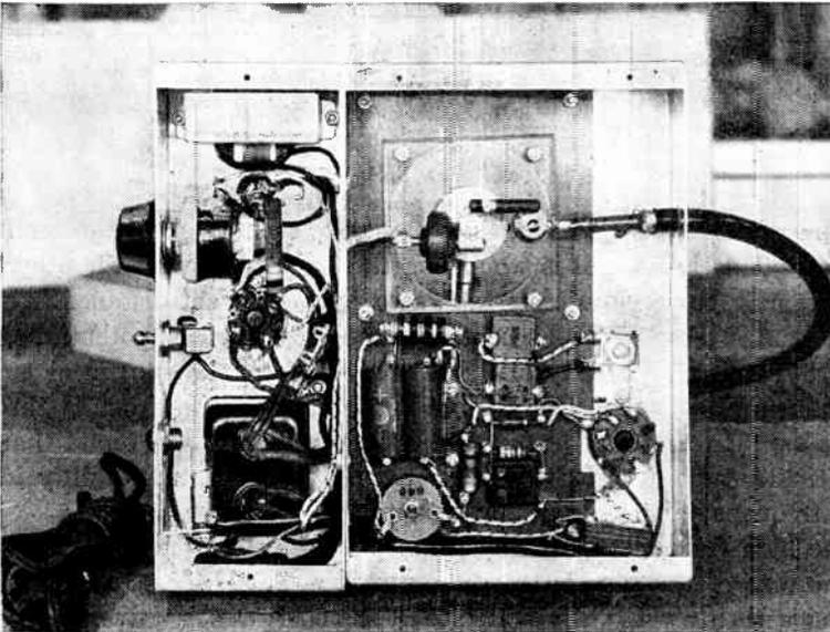
FIG. 8.73 High-voltage radio-frequency power supply, bottom view of chassis, model 10HFP-2. (Courtesy of U.S. Television Corp.)
