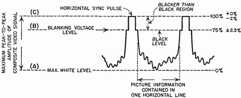
FIG. 5.1 The composite TV signal as interpreted in one line of horizontal picture information, with blanking voltage level and horizontal synchronizing impulses indicated.
