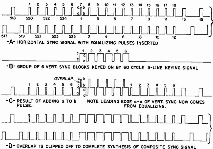
FIG. 5.54 Insertion of the vertical synchronizing blocks into the composite synchronizing signal. (After A. R. Applegarth.)
