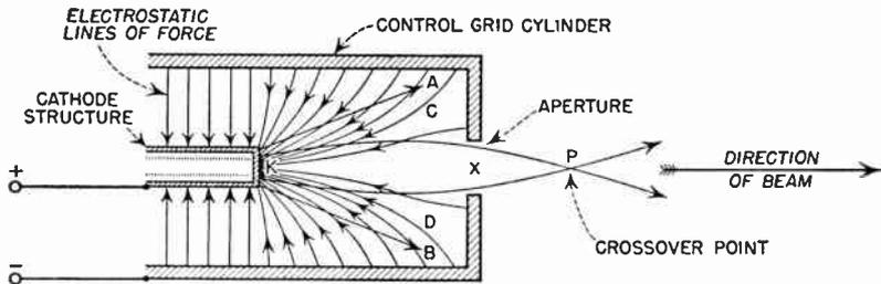
FIG. 2.10 Electron optics at control-grid lens, where electrons are first concentrated into a small beam.
