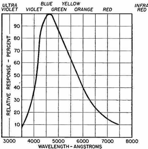
Fig. 4.4 Spectral sensitivity characteristic of the R.C.A. type 1850-A Iconoscope and the type 1840 Orthicon.
