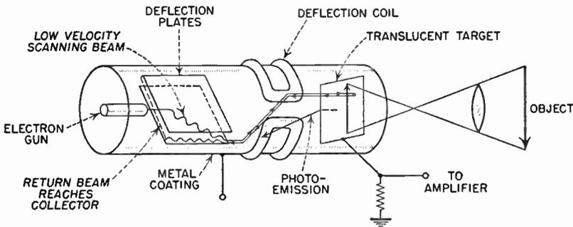
The focusing coil surrounding the tube is not shown
