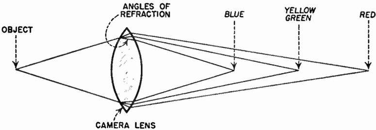
FIG. 1.11 Angles of refraction of different colors of light. Since each color of light has a different wavelength, each results in a different angle of refraction when passing through an uncorrected camera lens. The result is that not all colors focus in the same plane to form a sharp image.
