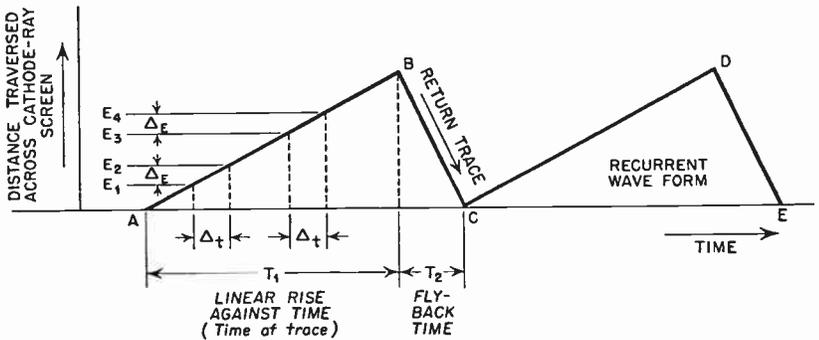
FIG. 3.1 Ideal saw-toothed-voltage waveform.
