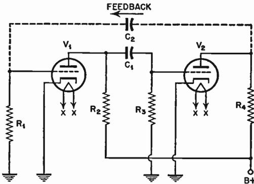
FIG. 5.9 Basic circuit-free running multivibrator.
