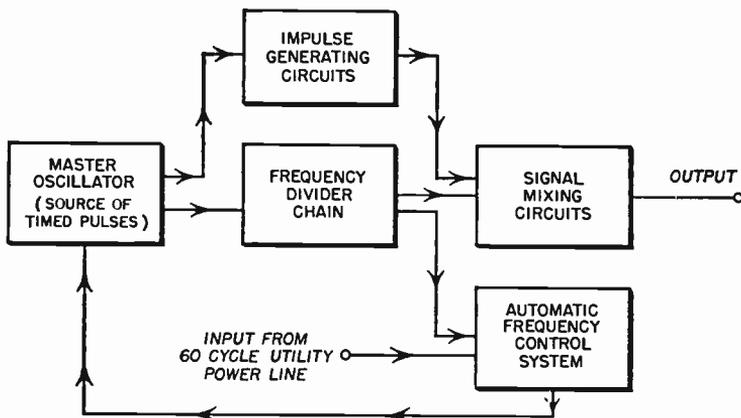
FIG. 5.4 Simplified block schematic of a typical synchronizing generator.
