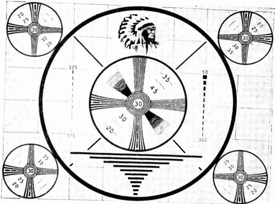
Fig. 11.29 Monoscope-tube test pattern. (Courtesy of Radio Corporation of America.)
