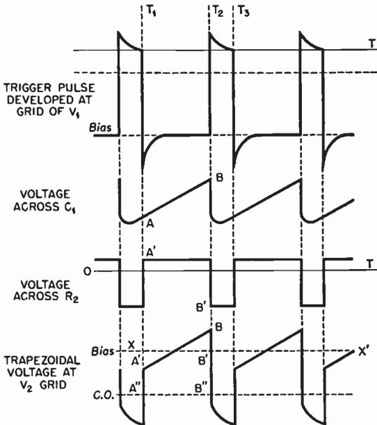
FIG. 4.8 Waveforms present in the circuit in Fig. 4.7.
