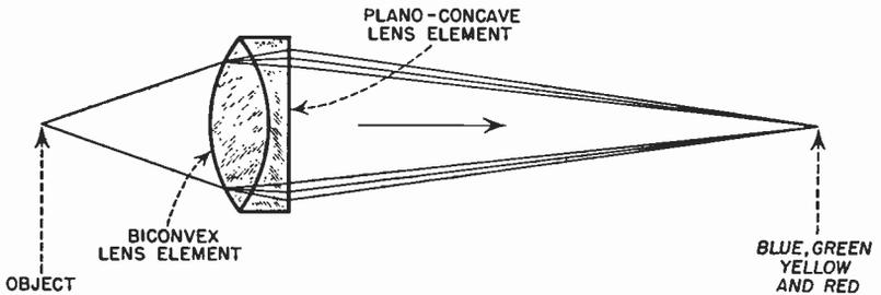
FIG. 1.12 Overcoming chromatic aberration by means of a doublet, in which the glass of the convex lens element is of a dissimilar refractive index from that of the concave lens element. In color correction all the rays of different wavelength (color) are brought into focus on an identical focal plane.
