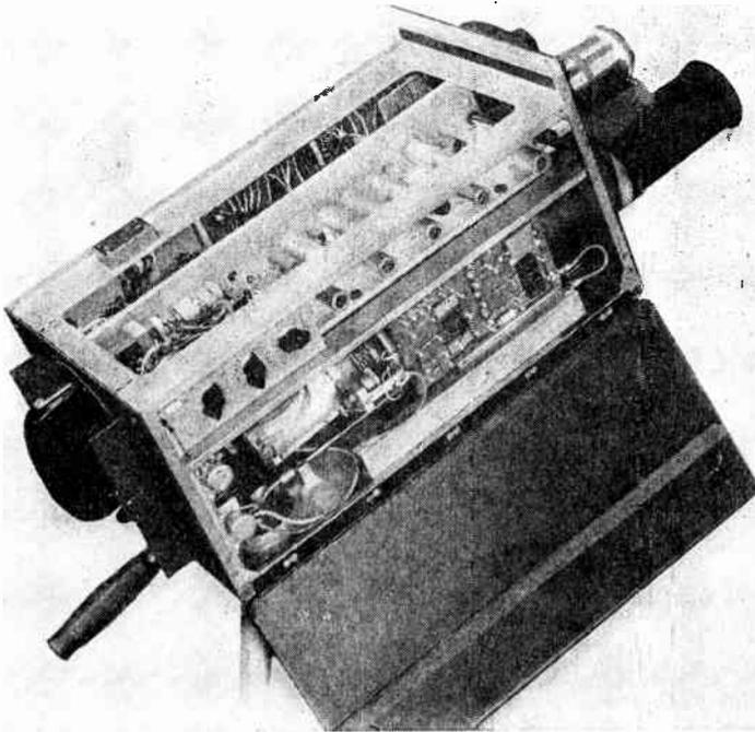
FIG. 9.5 Du Mont Orthicon camera head with electronic viewfinder detached (left-side and top views). The covers are removed for inspection of the circuits. (Courtesy of Allen B. Du Mont Labs., Inc.)
