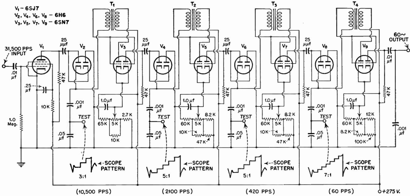
FIG. 5.22 Frequency-divider chain employing counter circuit timers.
