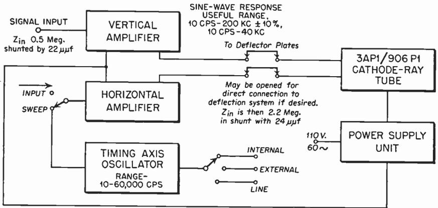
FIG. 3.16 Block diagram of R.C.A. type 155-C cathode-ray oscillograph.
