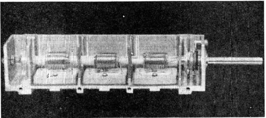
FIG. 8.20 The Inductuner is shown with the cover removed. It will be noted that the No. 2 and No. 3 inductors are wound in opposite directions so as to facilitate close positioning of the end inductors. (Courtesy, Allen B. Du Mont Labs., Inc.)
