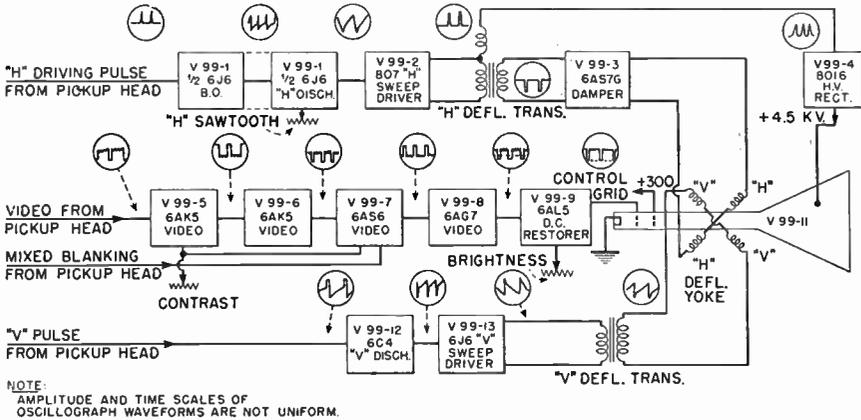
Fig. 9.9 Block schematic diagram of the type 5099-A electronic viewfinder.
