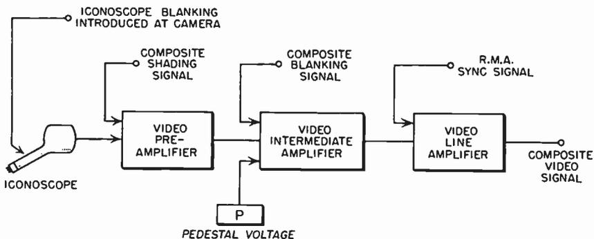
FIG. 5.46 Block schematic indicating where various signal voltages are injected in a typical Du Mont Iconoscope camera chain to result in the composite television signal.
