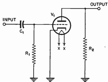
FIG. 5.31 *CR* differentiator circuit. It narrows the pulse, since *C* acts to discriminate against the low frequencies.
