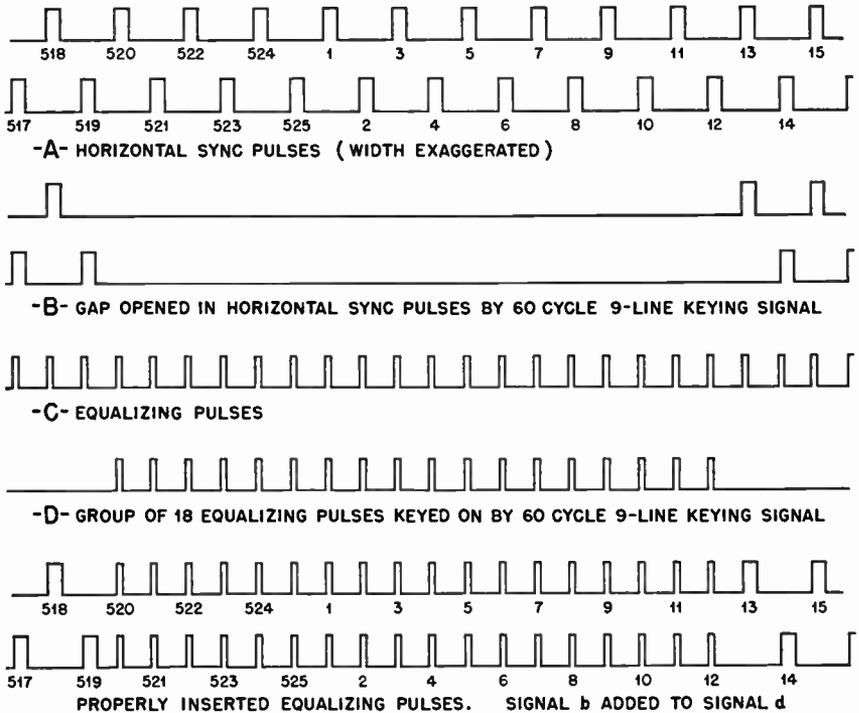
FIG. 5.53 Insertion of the equalizing signal into the horizontal synchronizing signal. (After A. R. Applegarth.)
