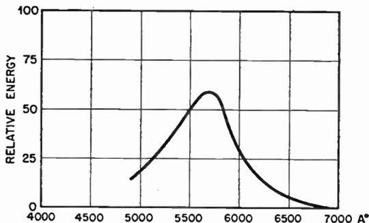
FIG. 2.26 Spectral characteristics of a fluorescent screen coated with artificial willemite  $[(\text{ZnO} + \text{SiO}_2): \text{Mn}]$ , the material having been quenched rapidly from a melt. This screen demonstrates a distinctly *yellow* luminescence.
