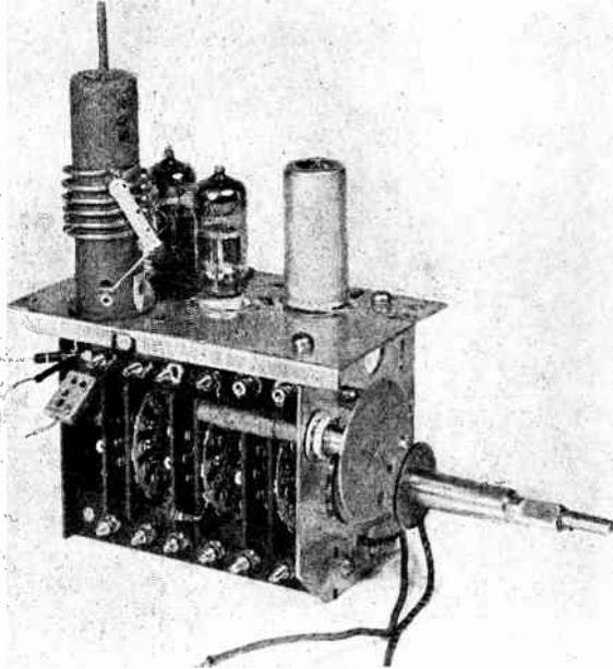
FIG. 8.5 External view of an R.C.A. Victor television tuning unit showing switch wafers and coils. Unit contains circuits tuned to cover each of the channels assigned by the F.C.C. to commercial television. (Courtesy of Radio Corporation of America.)
