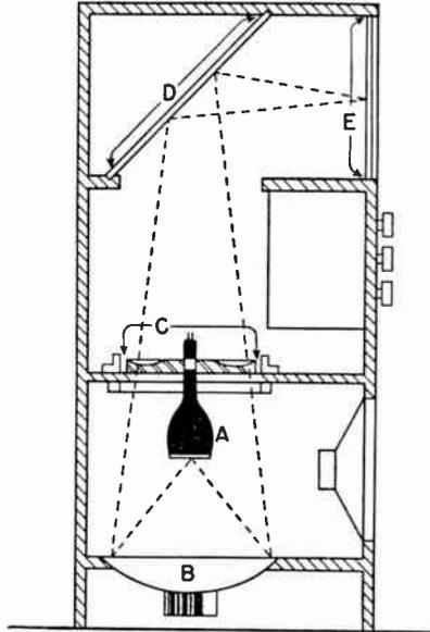
Two R.C.A. projection receivers using the Schmidt optical system are illustrated in Figs. 8.80 and 8.81, and the general arrangement of the projection system is shown in Fig. 8.82. The R.C.A. system makes use of a spherical front surface mirror and an aspherical lens that is positive in the central portion and gradually changes into negative near its periphery. A gain in screen illumination of about 6 : 1 or 7 : 1 is obtained as compared with a conventional  $f/2$  lens.
