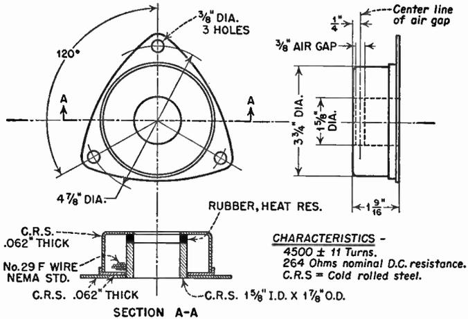
FIG. 2.24 Diagram of the construction of a typical focus coil.
