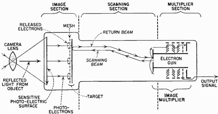
FIG. 4.17 Schematic diagram of the Image Orthicon.
