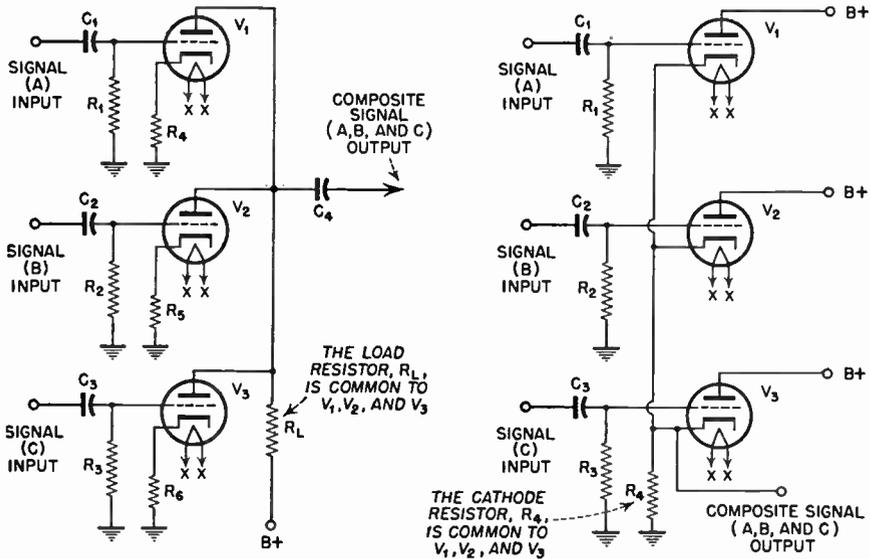
FIG. 5.45 Two methods for combining several signals into a composite signal, either a commonplate-load resistor or a common cathode resistor being employed.
