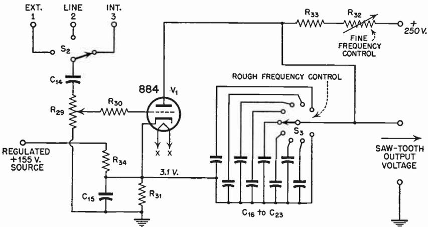
Fig. 3.3 Thyatron saw-toothed sweep generator, Du Mont type 208 oscillograph.
