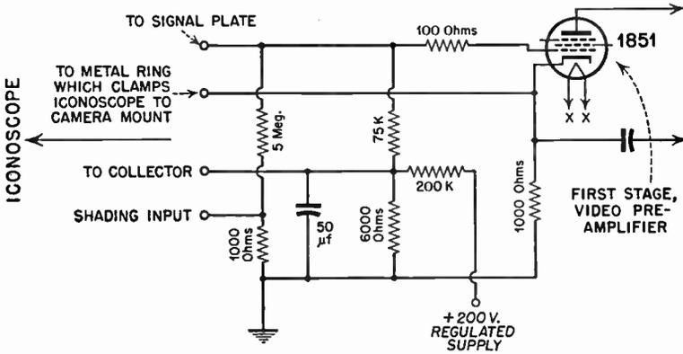
Fig. 4.3 Coupling circuit at input to video preamplifier at camera. Shading is introduced into system at low level.
