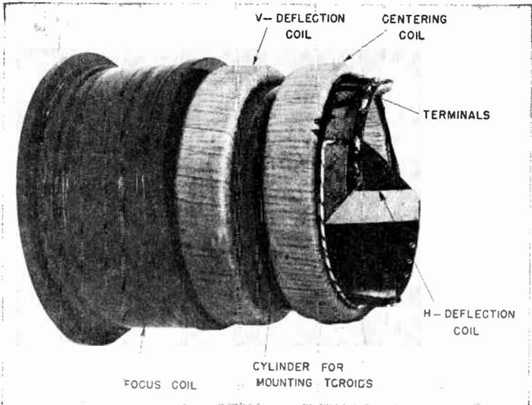
FIG. 4.22 Deflection-coil assembly associated with the Farnsworth Image Dissector. (Courtesy of Farnsworth Television and Radio Corp.)
