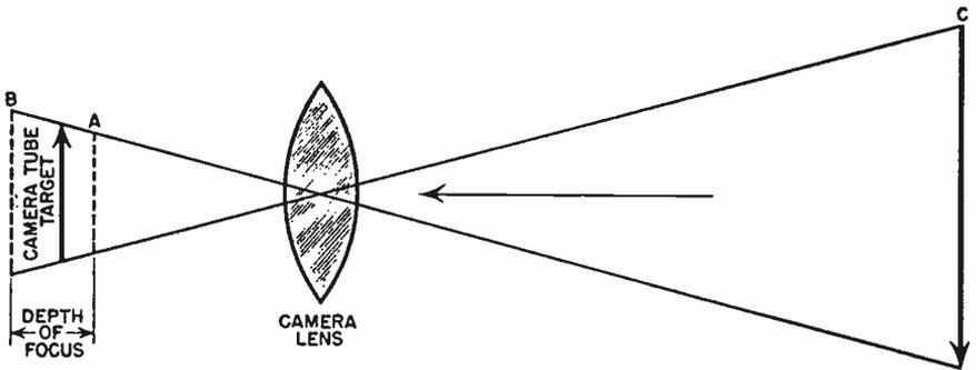
FIG. 1.14 Depth of focus. The depth of focus is the distance between the nearest image to the lens, focus *A*, and the most distant image from the lens, focus *B*, when the camera lens is focused on a given point *C*.
