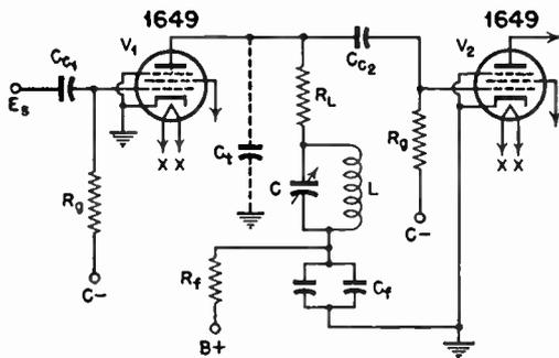
The resonant frequency  $F_r$  of the tuned circuit  $LC_t$  is  $\omega_r/2\pi$ , and  $\omega_h$  equals  $0.7\omega_r$ .
