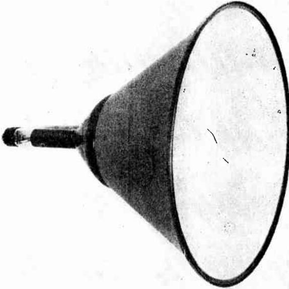
FIG. 2.34 Type 19AP4 metal-cone picture tube, the largest diameter cathode-ray tube in current commercial production employing a metal cone of chrome steel. The plate-glass face is treated with a P4 (white) phosphor, and it is designed for use in large-screen television receivers making use of direct viewing. (Courtesy of Allen B. Du Mont Labs., Inc.)
