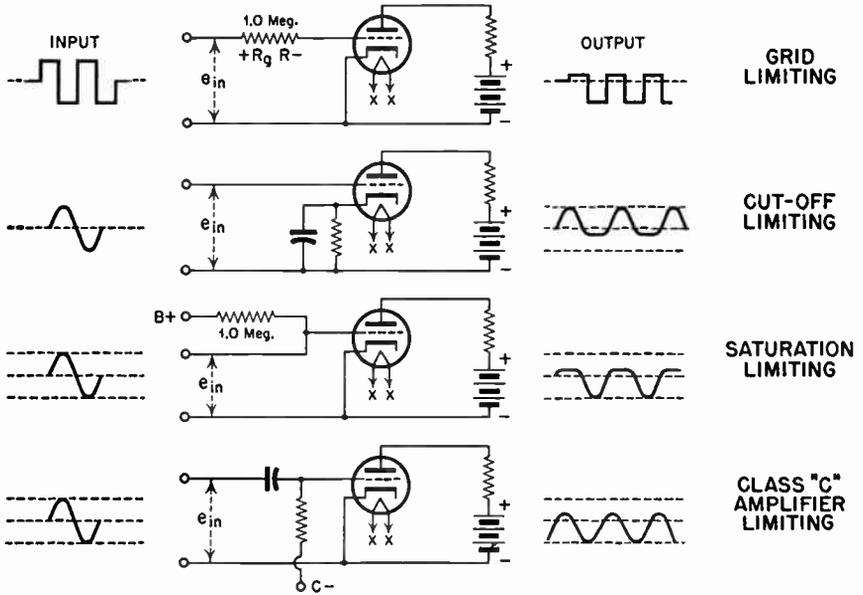
FIG. 5.30 Four types of limiting, or clipping, circuits.
