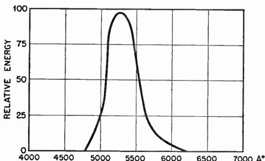
exhibits a green or yellow luminescence depends upon the temperature to which the synthetic material is heated and the manner in which it is cooled in the process of manufacture. If the material is cooled slowly, the resultant phosphor will exhibit a bright-green luminescence; but if it is quenched rapidly from a melt, the luminescence will be yellow.
