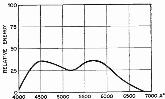
FIG. 2.29 Spectral characteristics of a *white* fluorescent screen coated with zinc cadmium sulphide and silver-activated zinc sulphide.
