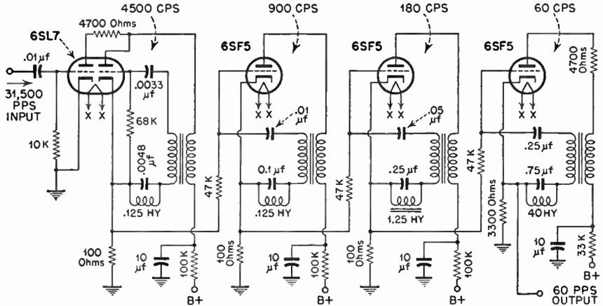
FIG. 5.15 Frequency-divider chain employing stabilized blocking-tube oscillators.
