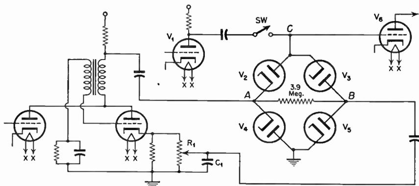
FIG. 5.63 Line-to-line clamping circuit.
