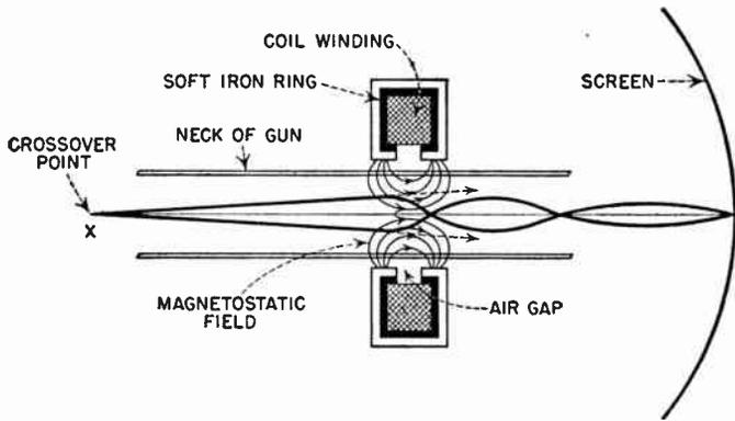
Fig. 2.20 Magnetostatic field set up in cathode-ray tube by short focus coil.
