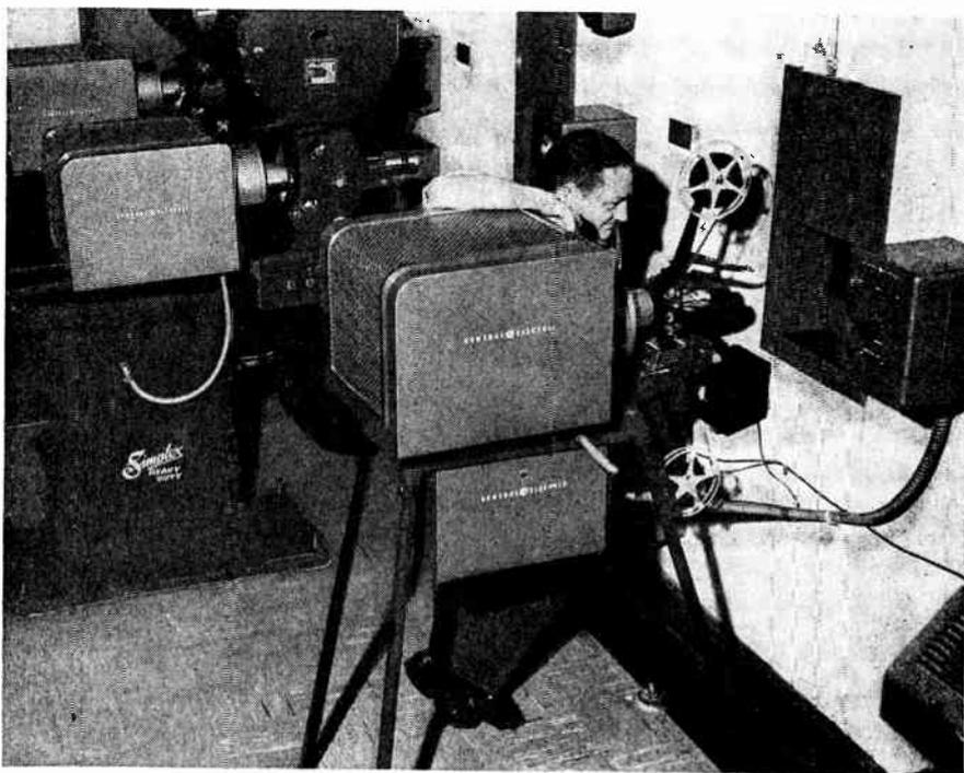
FIG. 11.31 The film-projection room of Station WGN-TV in Chicago. In the background are two 35-mm. projectors and in the foreground a 16-mm. projector. In this booth, movies or slides are projected through portholes to film cameras on the opposite side of the wall. A slide projector is shown at the lower right-hand corner. (Courtesy of General Electric Company.)
