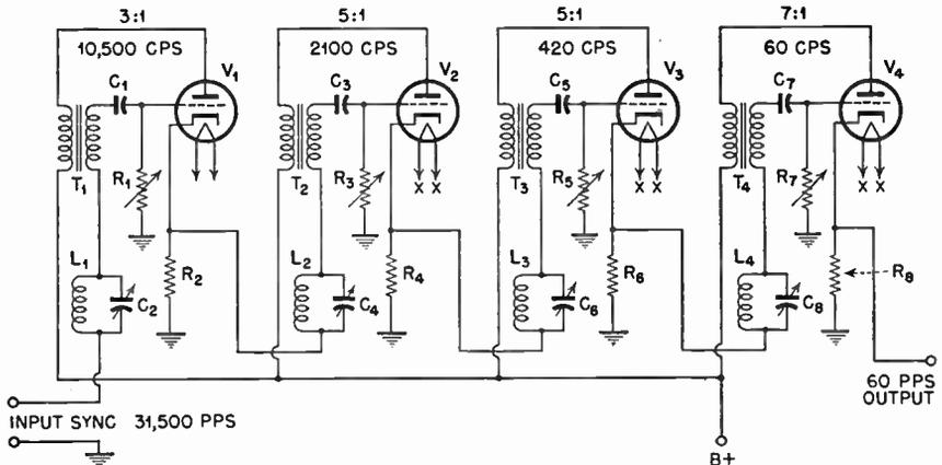
FIG. 5.16 Synchronizing-generator frequency-divider chain making use of stabilized blocking-tube oscillators.
