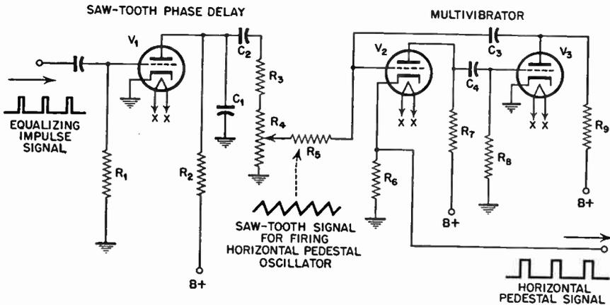
Fig. 5.42 Horizontal pedestal multivibrator system of a synchronizing generator.
