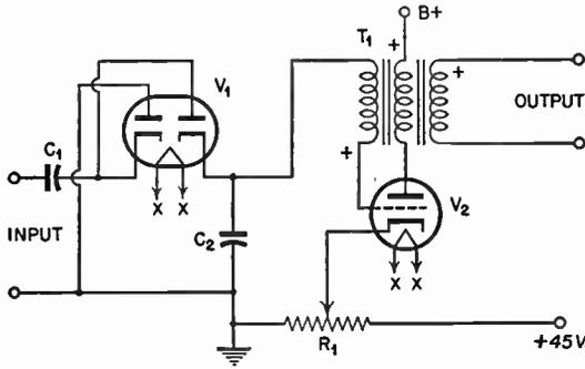
FIG. 5.20 Blocking-tube oscillator triggered by counter circuit.
