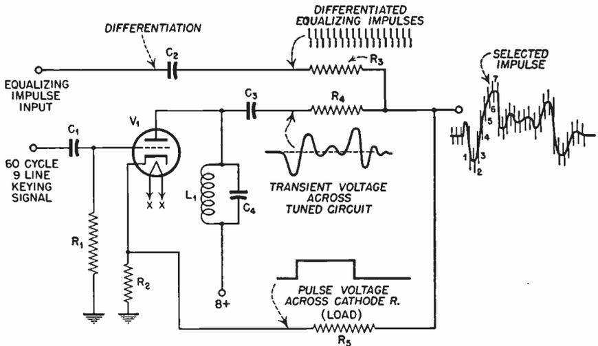
FIG. 5.40 Applegarth's precision time-delay system.
