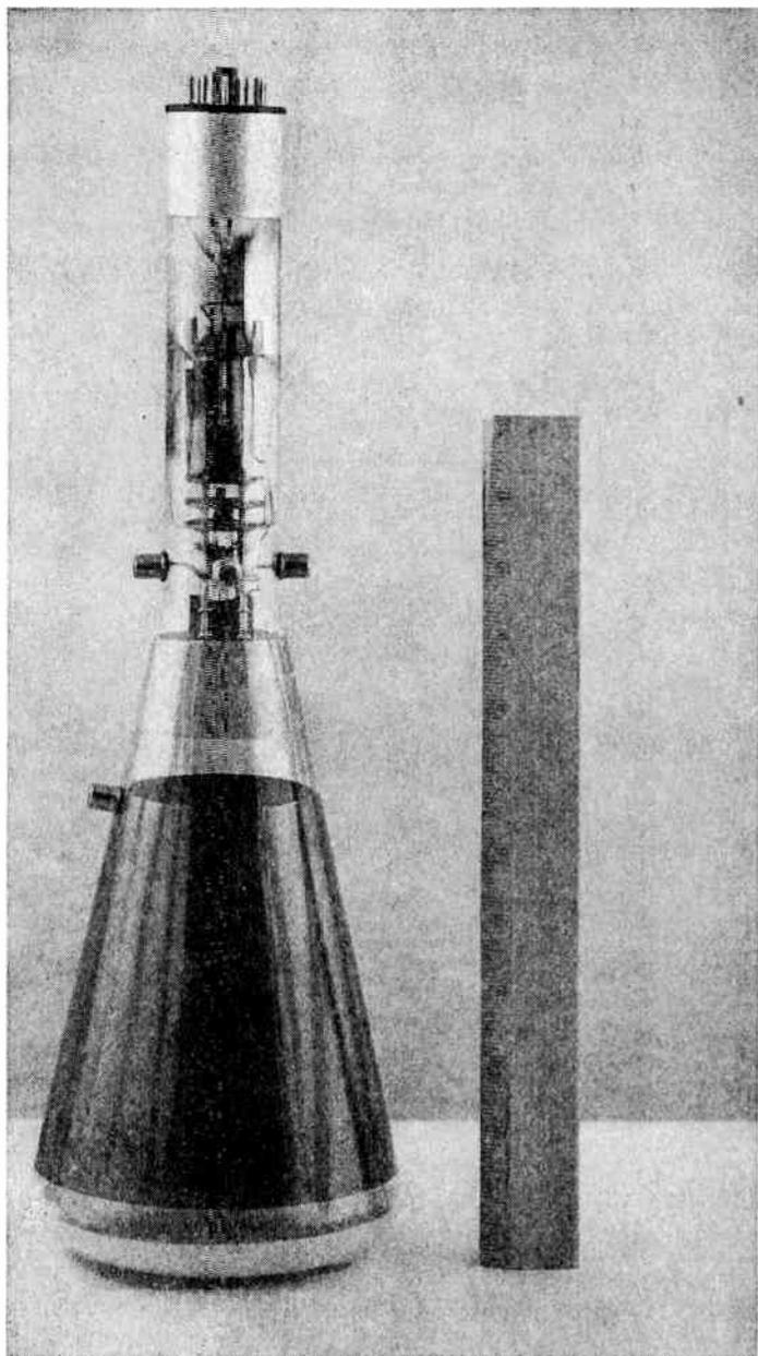
FIG. 2.2 Norelco type 5JP1 5-in. cathode-ray tube. This tube employs an electrostatic deflection system. Typical operating characteristics are:  $E_f$ : 6.3 v., 0.6 amp.;  $E_b$ , or  $E_{g2}$ : 1,000 v. maximum;  $E_{b1}$ : 2,000 v maximum;  $E_{b2}$ : 4,000 v. maximum; grid cutoff volts:  $-56 \pm 25$ . (Courtesy of North American Philips Company, Inc.)
