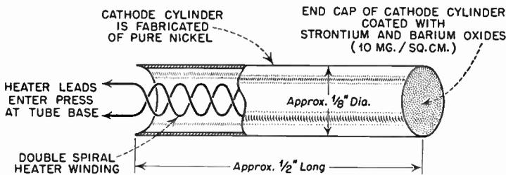
FIG. 2.7 Modern cathode-ray tube heater and cathode design.
