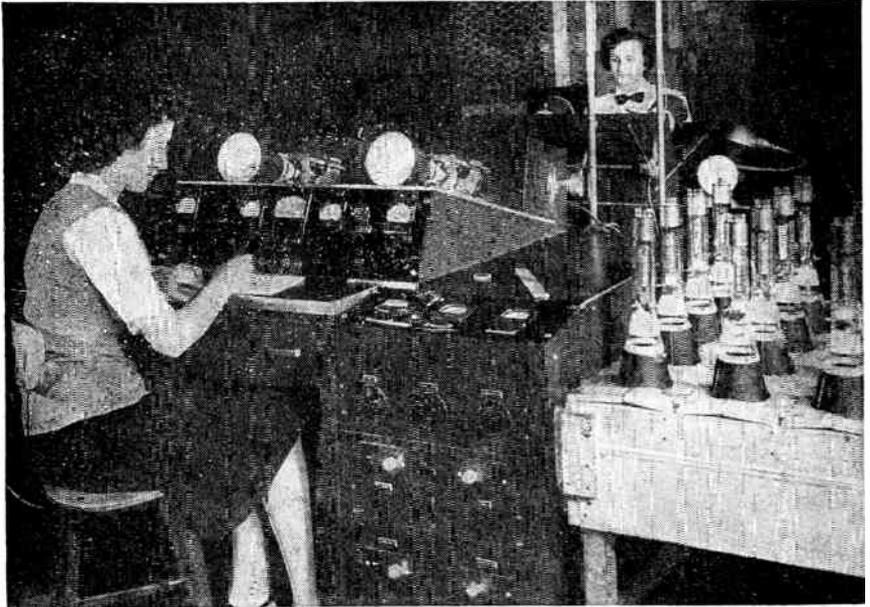
FIG. 2.39 Typical test console. The Du Mont cathode-ray tube must pass 18 electrical and 12 mechanical tests after manufacture. (Courtesy of Allen B. Du Mont Labs., Inc.)
