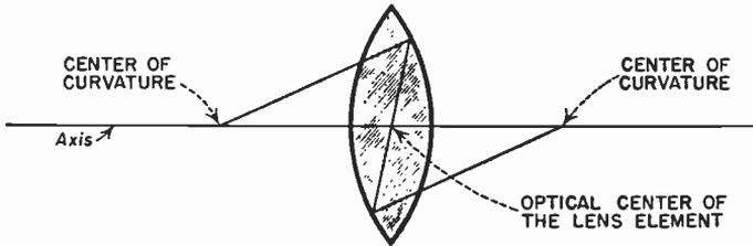
FIG. 1.17 Optical center. Parallel lines are drawn through the centers of curvature of the lens to meet the lens surfaces. The line joining these intersections crosses the lens axis at a point termed the "optical center."
