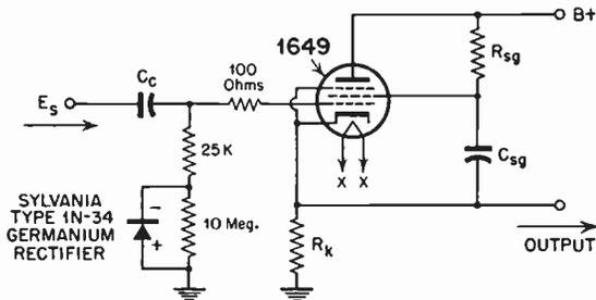
FIG. 6.7 Anti-“bounce” circuit employed at cathode-follower output stage of video preamplifier.
