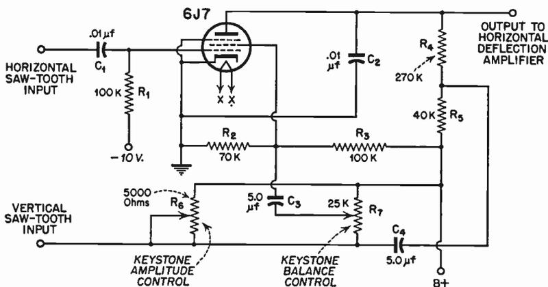
FIG. 5.61 Keystone-correction circuit.
