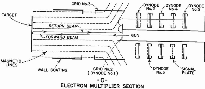
FIG. 4.18 The three important sections of the Image Orthicon tube.
