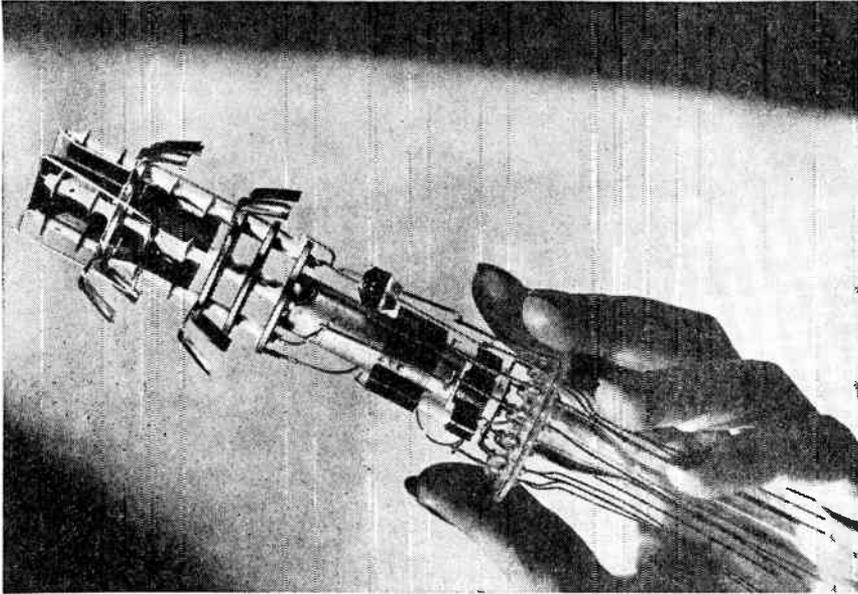
FIG. 2.6 Electron gun of a Norelco cathode-ray tube employing electrostatic deflection. (Courtesy of North American Philips Company, Inc.)
