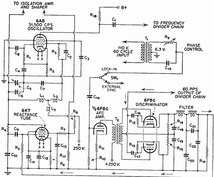
FIG. 5.27 Automatic-frequency-control system as used in a commercial synchronizing generator.
