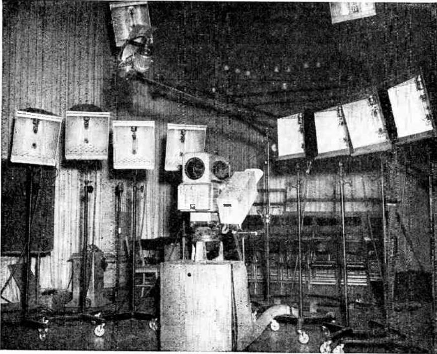
FIG. 1.3 Westinghouse type AII-12 1,000-w. mercury vapor lamps in olivettes of spun aluminum provide a suitable high-intensity cold light source where Image Orthicon or Iconoscope cameras are used. Here, some of the lamps are mounted on portable floor stands, some are suspended overhead on a pipe grid. Some supplementary incandescent lighting is used to provide the full color range. (Courtesy of Du Mont Television Network.)
