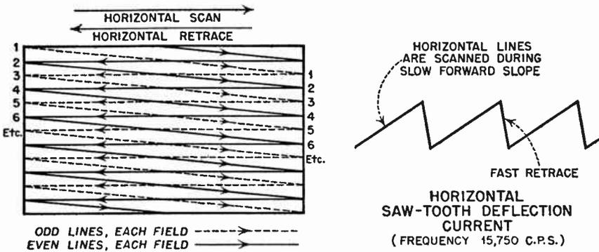
FIG. 1.23 Interlaced scanning as employed in a modern high-definition all-electronic television system (262.5 horizontal lines are scanned for each field. Two fields interlaced are required to make one frame, and 30 frames of 525 lines each are transmitted each second).
