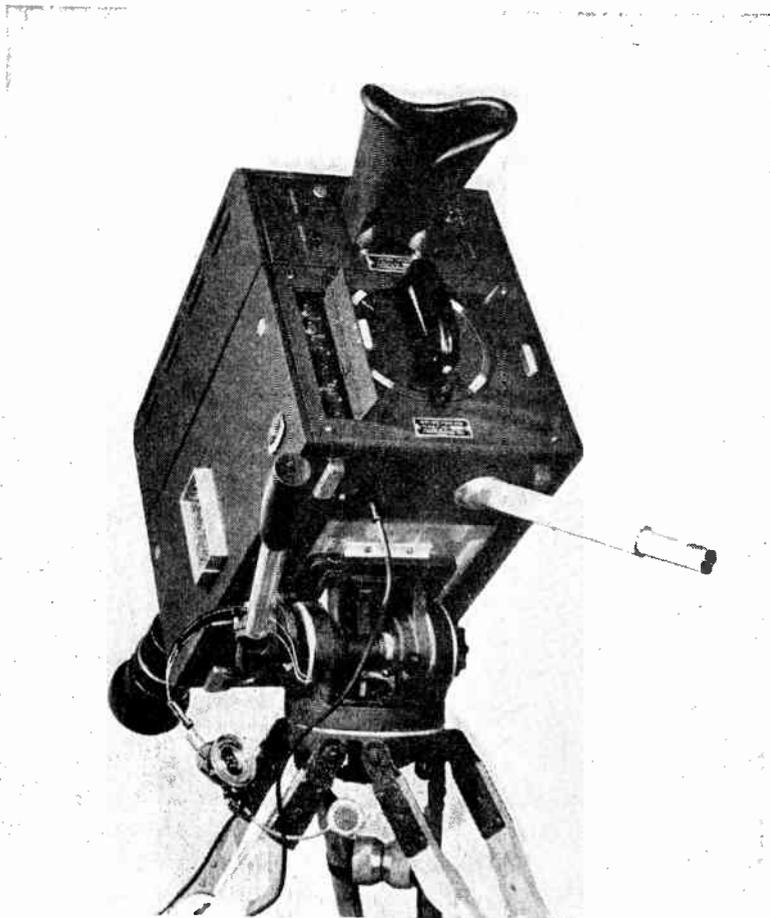
Fig. 9.4 Du Mont Orthicon pickup head with electronic viewfinder attached (rear view). (Courtesy of Allen B. Du Mont Labs., Inc.)
