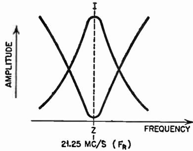
The elements of the series-resonant rejector circuit can be so proportioned that the susceptance curve is very sharp at the sound intermediate carrier frequency. It thus results in maximum current flow at this frequency, since the minimum impedance obtains at resonance. Because
