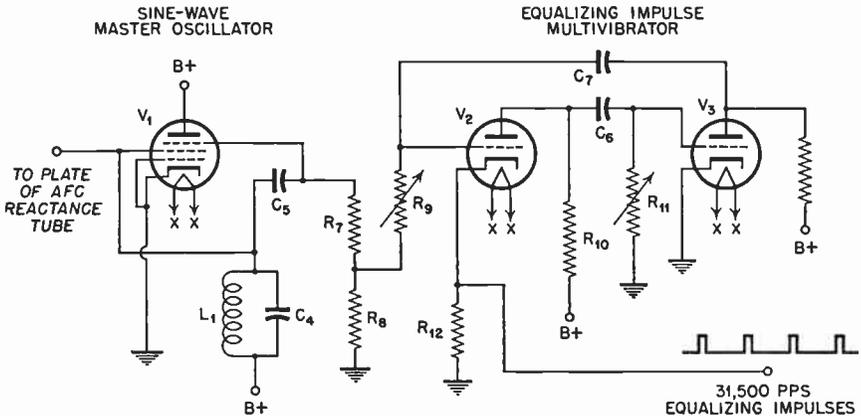
FIG. 5.36 Sine wave master oscillator and the equalizing impulse multivibrator.
