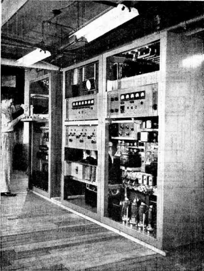
FIG. 10.4 Three frames housing the video exciter, 5-kw. video final amplifier, and 5-kv. power supply. The units are set up for test. A metal cover, or "skin," houses the complete transmitter. (Courtesy of Allen B. Du Mont Labs., Inc.)
