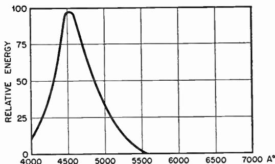
decay period, the light output suffering a reduction from full brilliance to 10 per cent in  $10^{-7}$  sec. Since its emission is highly actinic and its decay period short, it is often applied to the screen of tubes used for photographic purposes. The efficiency is low, being about 0.3 lumen per w. The peak radiation of calcium tungstate applied to a screen departs quite radically from the peak of the curve indicating luminous response
