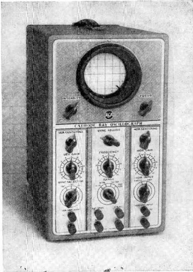
FIG. 3.15 R.C.A. type 155-C cathode-ray oscillograph. This is an example of the type of test instrument available to the television engineer and technician for simple routine equipment testing and maintenance. (Courtesy of Radio Corporation of America.)
