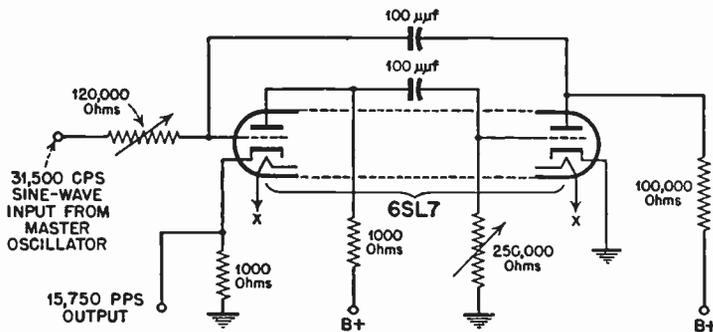
FIG. 5.37 Equalizing impulse multivibrator.
