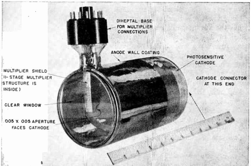
FIG. 4.19 Farnsworth Image Dissector. Location of the photosensitive cathode and the electron multiplier within the large containing glass envelope is indicated. It is an excellent tube for motion-picture film scanning. (Courtesy of Farnsworth Television and Radio Corp.)
