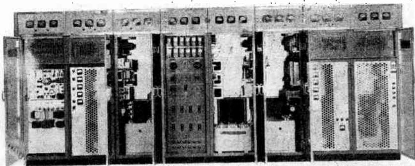
FIG. 10.11 Front view of RCA TT-5A transmitter with all doors open. (Courtesy of Radio Corporation of America.)
