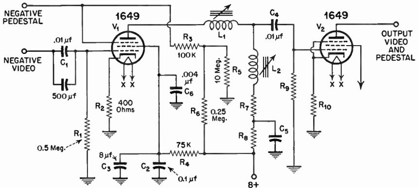
FIG. 5.51 Diagram of method of using suppressor injection to combine video and pedestal voltages.
