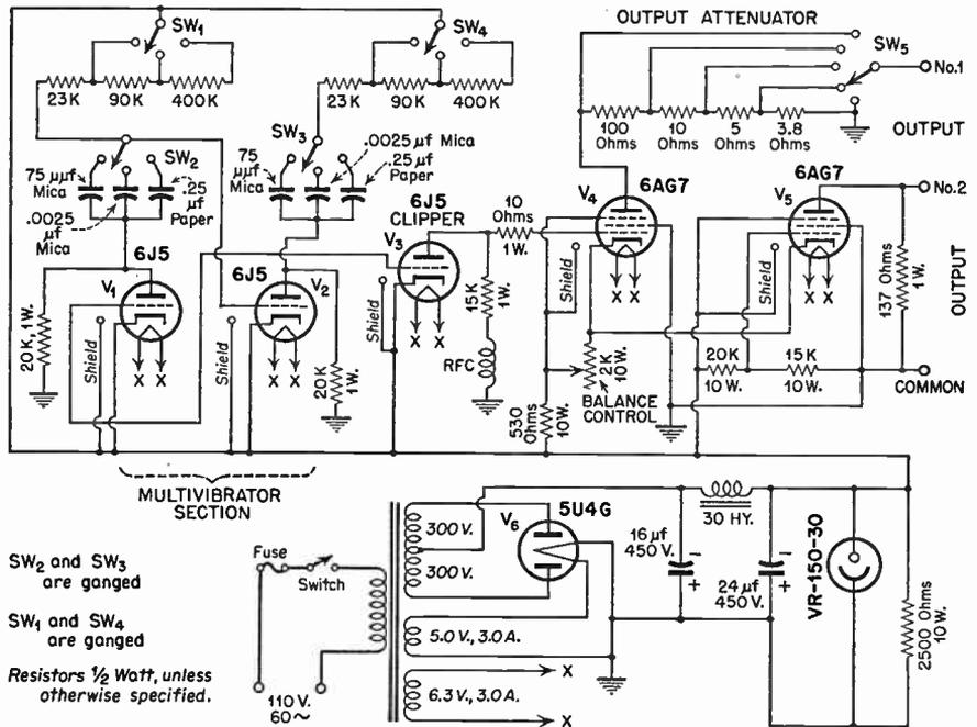
FIG. 3.7 Square-wave generator incorporating multivibrator and clipper; Range 2 c.p.s. to above 100,000 c.p.s.
