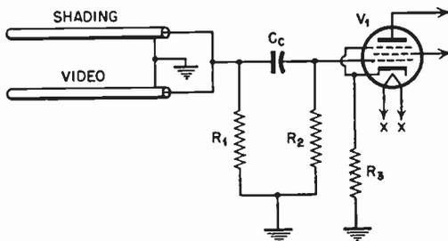
FIG. 5.47 Circuit employed in combining the outputs of the shading amplifier and video pre-amplifier when mixing is accomplished at high level.
