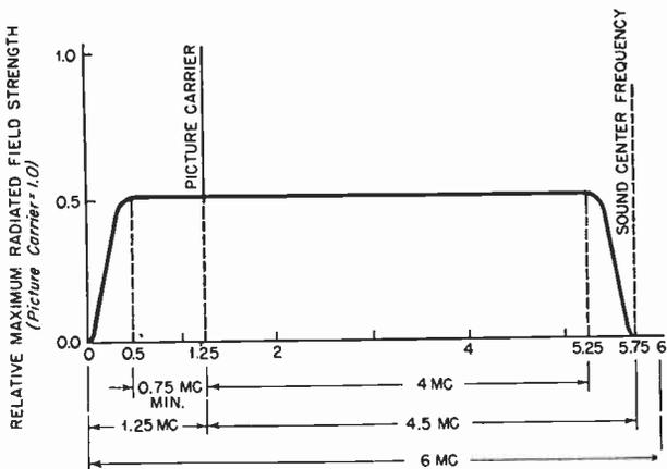
FIG. 10.1 A channel 6 mc. wide is provided by the licensing authority for television broadcasting purposes. The figure illustrates the relative positions of the picture and sound carriers and also the approximately single sideband transmission involved. Actually, the lower sideband is attenuated 20 db. at 1.25 mc. below the visual carrier.
