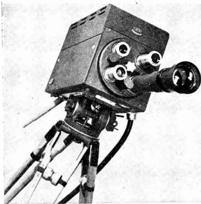
FIG. 1.19 Du Mont Mark II Image Orthicon field camera. Four lenses are mounted on a turret which may be rotated to select any lens desired. (Courtesy of Allen B. Du Mont Labs., Inc.)
