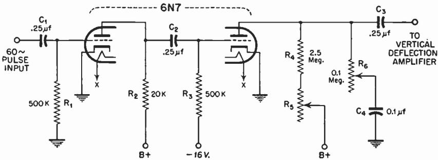
FIG. 5.57 Vertical saw-toothed deflection generator.
