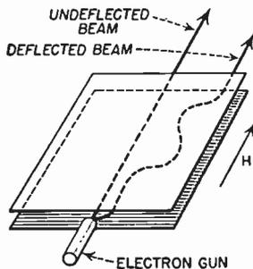
Fig. 4.15 Diagram of the path of an electron beam in electric and magnetic fields. (After A. Rose and H. Iams.)
