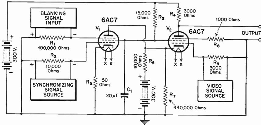
FIG 5.50 Diagram of signal-mixing system. (After Madison Cawein.)
