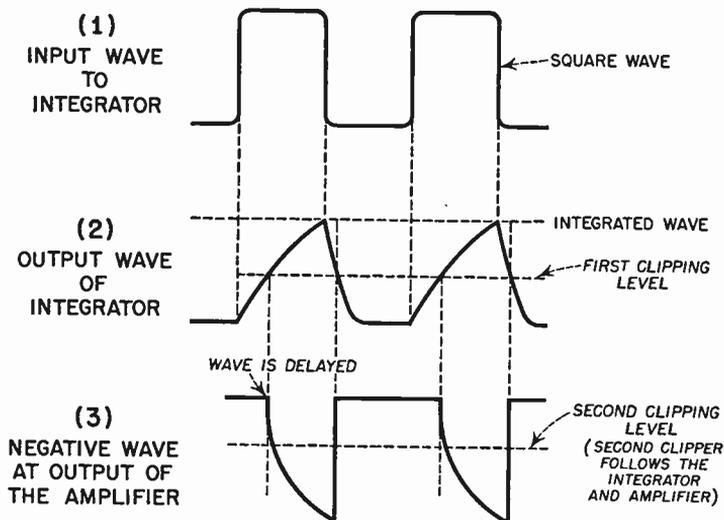
FIG. 5.33 Waveforms which obtain at the input of the integrator, at the output of the integrator, at the output of the amplifier and clipper (in the input circuit of which the integrator is connected), and the clipping level of a succeeding limiter are indicated.
