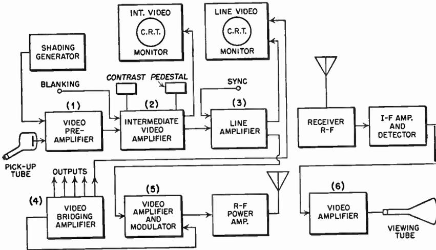
Fig. 6.1 Block diagram showing relative positions of video amplifiers in a typical high-definition television system.
