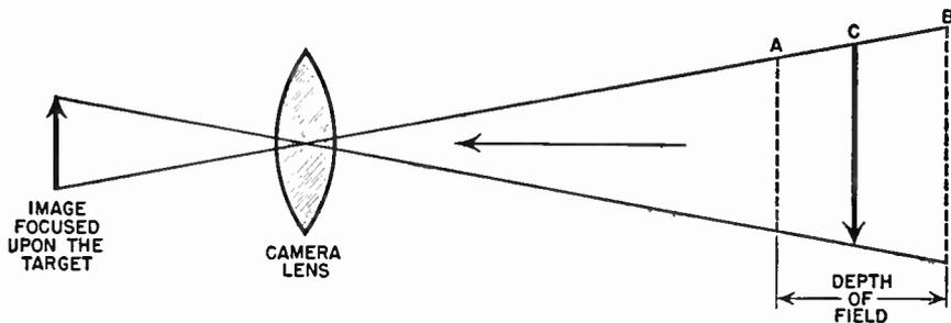
FIG. 1.13 Depth of field. The depth of field is the distance between the nearest object to the lens, focus A, and the most distant object from the lens, focus B, when the camera lens is focused on point C.
