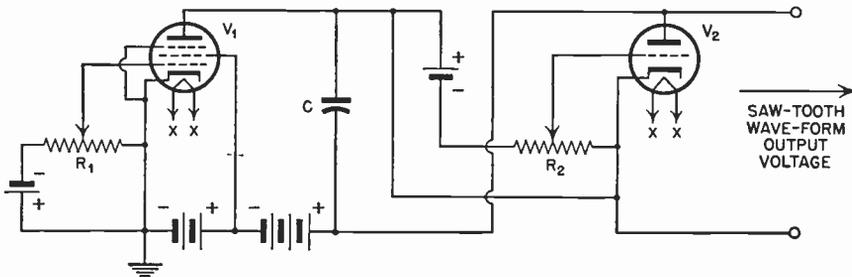
Fig. 3.4 Controlled charging-current saw-toothed generator.
