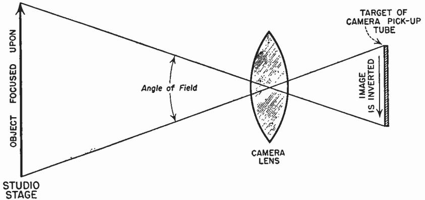
FIG. 1.16 Diagram of the way in which light reflected from the studio stage is imaged upon the target of the pickup tube in the television camera. The angle of field is that angle formed at the camera lens by the beams of light from the outer boundaries of the studio stage.
