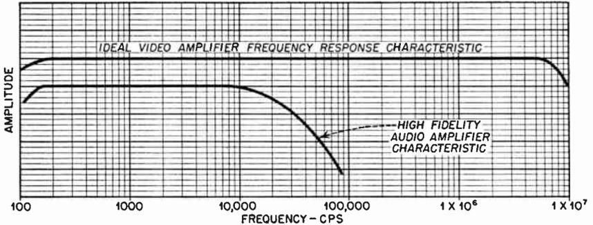
FIG. 6.2 Comparative gain-frequency characteristics of a high-fidelity audio amplifier and an ideal video amplifier employed in television systems.
