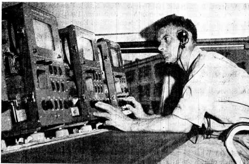
FIG. 9.29 Pictured above is a technician operating portable camera monitors inside a mobile television truck. The monitor at the extreme right is the master monitor. (Courtesy of General Electric Company.)
