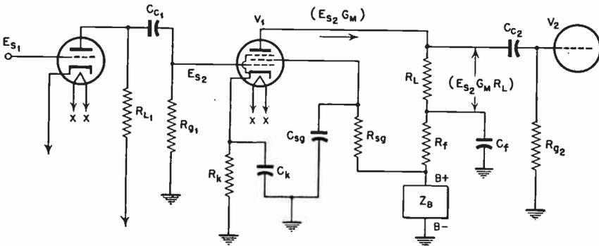
FIG. 6.9 Video-amplifier stage with low-frequency correction.
