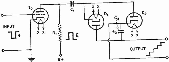
FIG. 5.23 Conventional counter of frequency-divider system.
