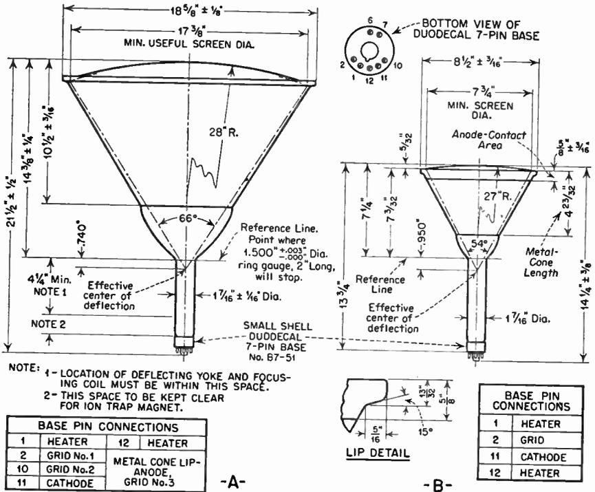
FIG. 2.33 A. Type 19AP4 metal-cone 19-in. picture tube. B. Type 8AP4 metal-cone 8-in. picture tube.
