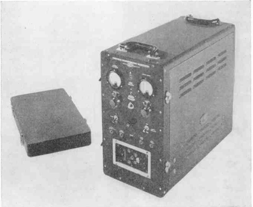
Fig. 9.20 Du Mont type 5030-A portable synchronizing generator. (Courtesy of Allen B. Du Mont Labs., Inc.)
