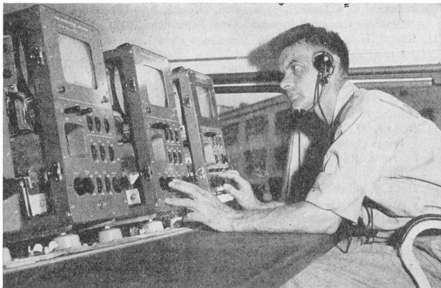
FIG. 9.29 Pictured above is a technician operating portable camera monitors inside a mobile television truck. The monitor at the extreme right is the master monitor. (Courtesy of General Electric Company.)
