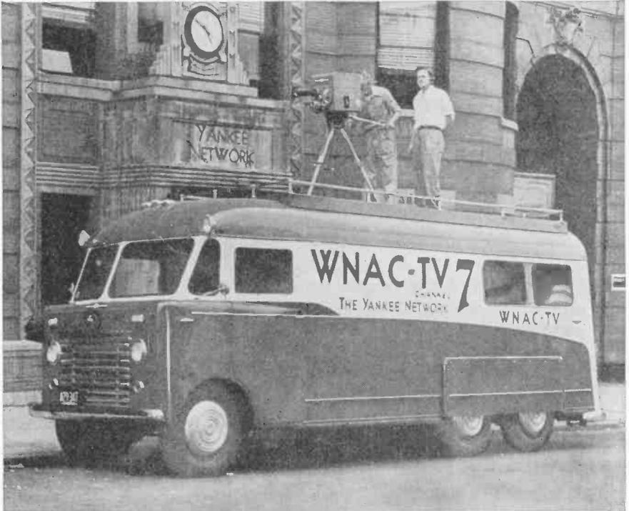
FIG. 9.28 A mobile television truck which is used to cover such events as baseball games, parades, etc., for television audiences. Atop the truck are two technicians operating the television camera. (Courtesy of General Electric Company.)
