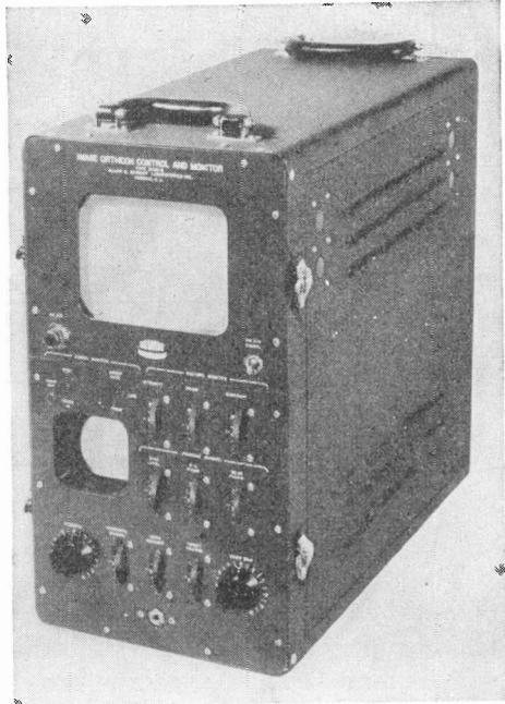
FIG. 9.13 Du Mont type 5028-B Image Orthicon control and monitor unit. (Courtesy of Allen B. Du Mont Labs., Inc.)
