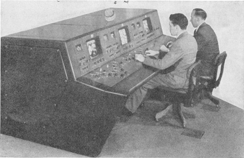
**Fig. 9.25** Du Mont dual Iconoscope camera control console for film pickup. (Courtesy of Allen B. Du Mont Labs., Inc.)
