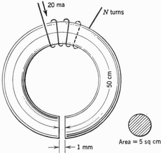
FIG. 7. An iron bar bent in the form of a ring presents an interesting problem in magnetic circuits.
