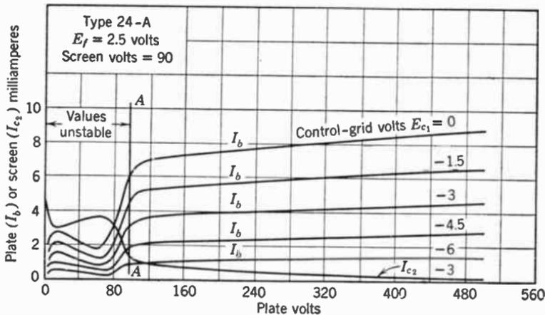
FIG. 11. Characteristic curves of typical screen-grid tube.
