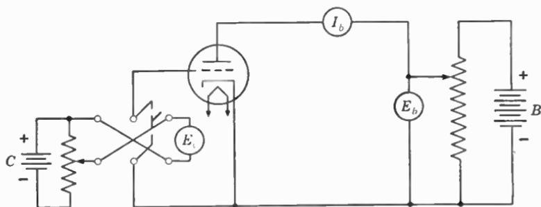
FIG. 8. Circuit for studying triode characteristics. The DPDT switch reverses the polarity of the grid voltage. The filament is held at its rated value, since that is the normal operation.
