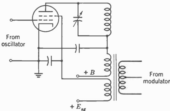
FIG. 8. Circuit in which both plate and screen voltages are modulated.
