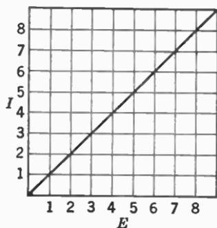
FIG. 4. In a circuit obeying Ohm's law, the current is directly proportional to the voltage.
