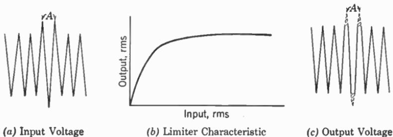
FIG. 8. A limiter eliminates variations in amplitude.
