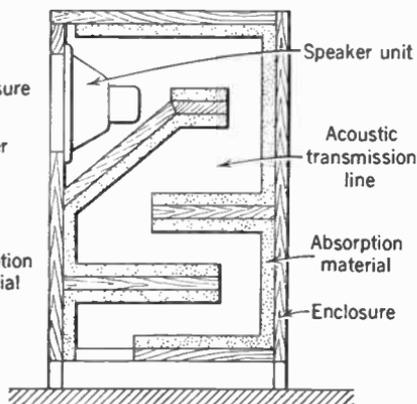
FIG. 17. Construction of the labyrinth enclosure for dynamic speaker.
