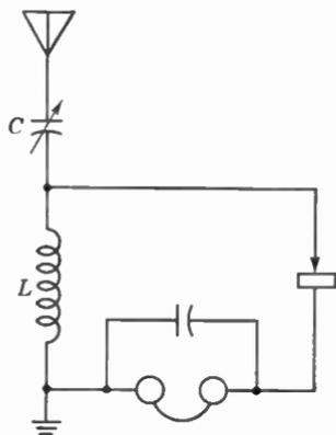
FIG. 1. A simple radio receiver.
