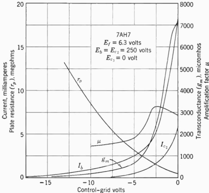
FIG. 14. Characteristics of a variable-mu or super-control tube.
