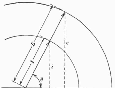
FIG. 12. Current and voltage in phase. Here the maximum value of the voltage is greater than the maximum value of the current, or it is drawn to a different scale.
