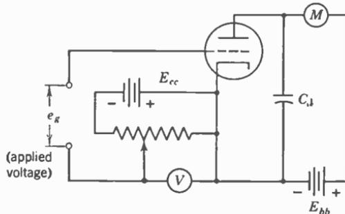
FIG. 5. Slide-back voltmeter. In operation, the grid bias,  $V$ , is adjusted to give a chosen value of plate current. The signal voltage which is to be measured is then applied. This increases the plate current. Finally, the bias voltage is increased to return the plate current to its original value.
