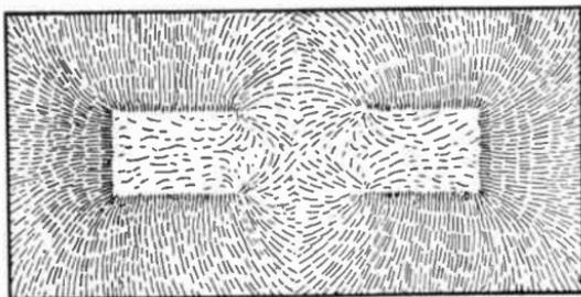
FIG. 1. How iron filings show the lines of force surrounding a bar magnet.
