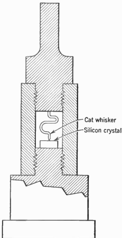
FIG. 4. Details of crystal detector rectifier.
