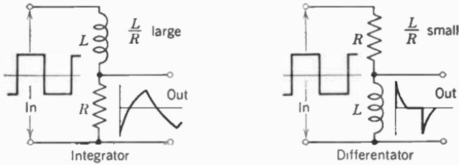
FIG. 6.  $RL$  integrating and differentiating circuits.
