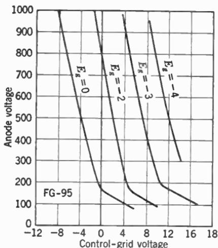
Fig. 3. Characteristics of shield-grid thyatron. Note that various starting voltages are possible, depending upon voltage of shield grid.
