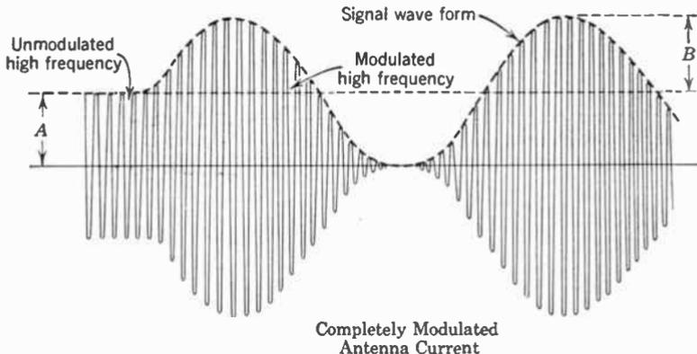
FIG. 6. Radio-frequency wave before and after modulation.
