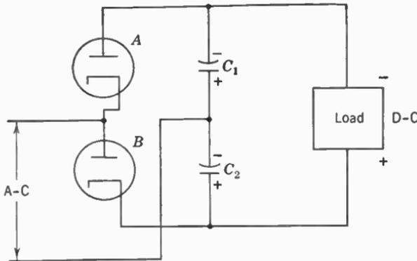
FIG. 7. Use of two diodes in a full-wave voltage-doubling circuit.
