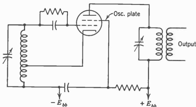
FIG. 9. Electron-coupled oscillator.
