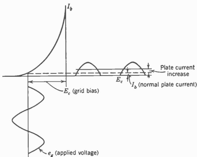
FIG. 2. Grid biased at or near cut-off in plate-circuit detector used as a voltmeter.
