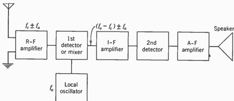
Fig. 5. Block diagram of a superheterodyne receiver.
