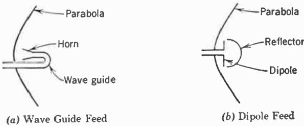
FIG. 14. Parabolic reflectors.
