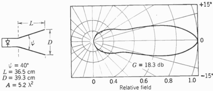
FIG. 13. Directional characteristics of a metal horn-type antenna operating on 15.3-cm wavelength.
