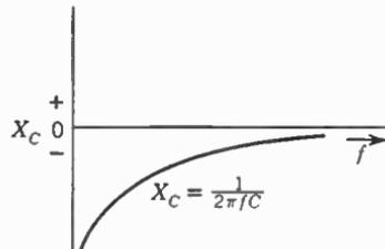
FIG. 8. Reactance curve for a capacitance.
