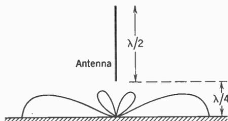
FIG. 11. Radiation pattern of a vertical doublet  $\frac{1}{4}\lambda$  above ground.
