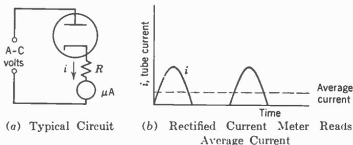
FIG. 6. Simple average-reading diode voltmeter. \*
