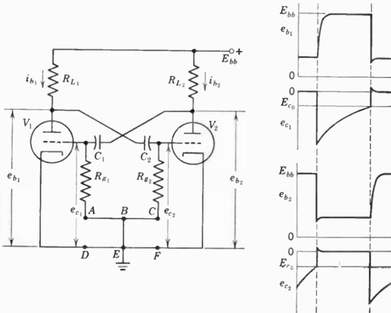
FIG. 11. Plate-coupled multivibrator.
