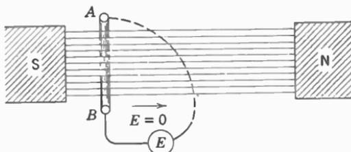
FIG. 12. If  $A-B$  is a conductor and if it is moved so that it "cuts" the lines of force between the magnet poles, then a voltage will appear across the ends of the conductor. If  $A-B$  moves in the direction of the lines of force, then no voltage will be produced.
