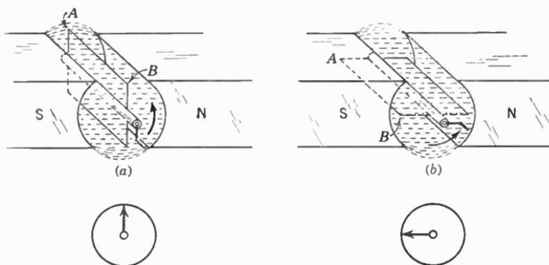
FIG. 14. Elements of a simple electric generator, in this case producing alternating current.
