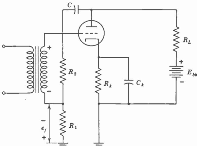
FIG. 20. A voltage-feedback circuit.
