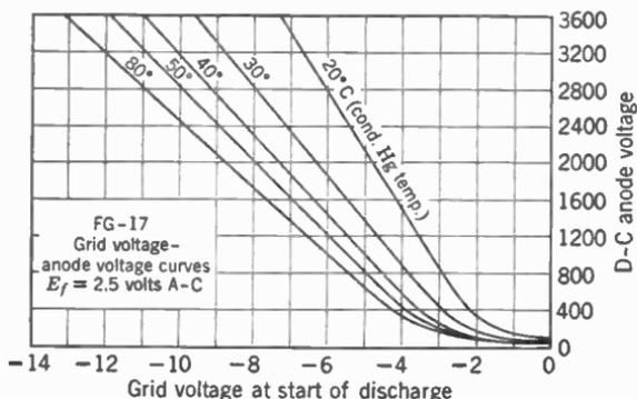
Fig. 2. Characteristics of mercury-vapor thyatron. Note that the temperature affects the starting voltage.
