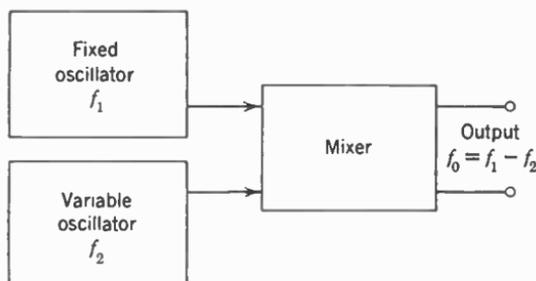
FIG. 25. Block diagram of a beat-frequency oscillator.
