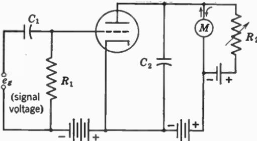
FIG. 4. Use of battery and rheostat for balancing out the steady no-signal current.
