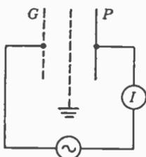
FIG. 9. A grounded shield between plate and grid reduces a-c current flow from plate to grid.
