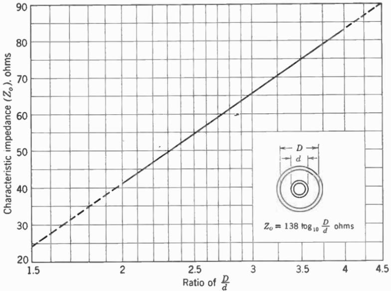
Impedance of Air-Filled Coaxial Line
