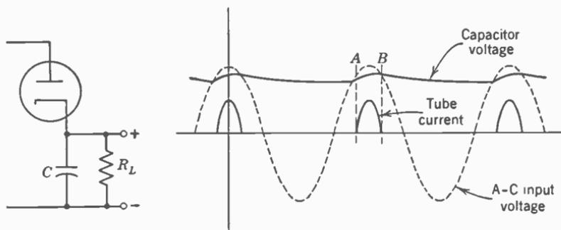
FIG. 10. Current and voltage for a shunt capacitor filter. The time constant  $R_L C$  is greater than the period of the a-c wave.
