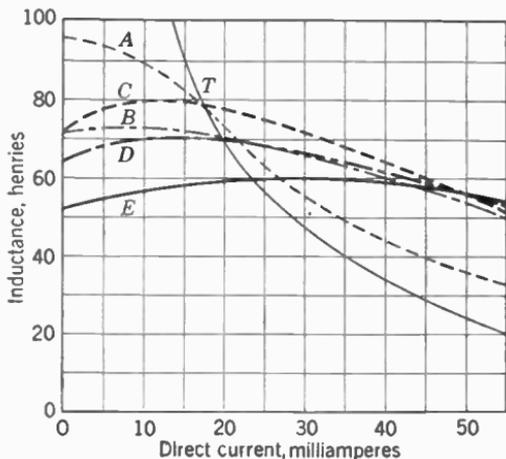
FIG. 14. Variation of inductance with air gap.
