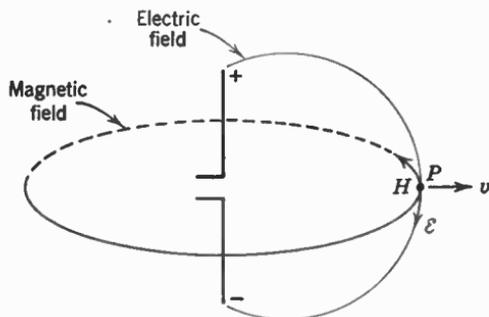
FIG. 23. Direction of electric and magnetic fields around a dipole antenna.
