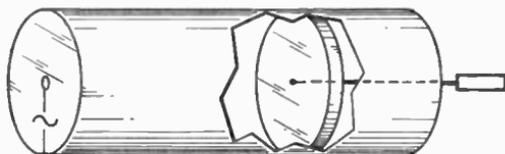
FIG. 4. Elements of cavity resonator. If the frequency of the energy introduced and the position of the plunger are correctly related, standing waves will be set up in the chamber, which then acts like an anti-resonant circuit of very high  $Q$ .
