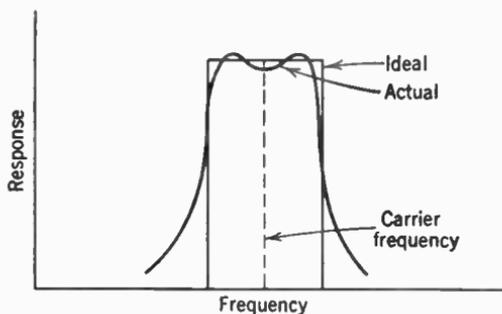
FIG. 9. Ideal and actual response of band-pass amplifier.
