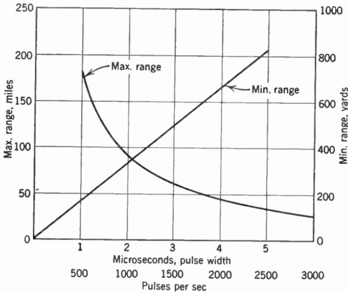
FIG. 5. The minimum range increases as pulse width in microseconds increases; the maximum range, however, decreases with wider pulses.
