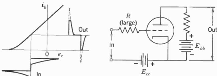
FIG. 10. Triode circuit which clips both peaks.
