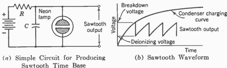
FIG. 13. Sawtooth generator.
