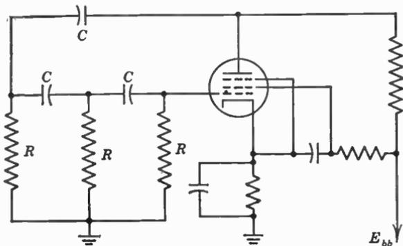
FIG. 17. Phase-shift oscillator.
