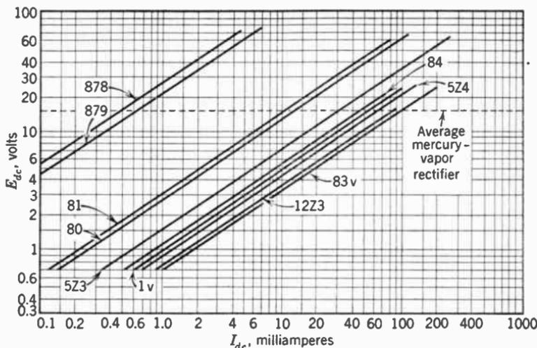
FIG. 1. Voltage drop versus current through several types of rectifier tubes. Note the dotted curve for the mercury-vapor rectifier.
