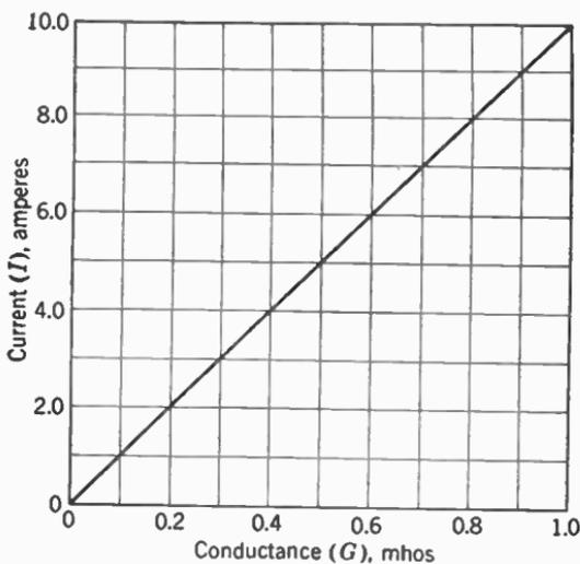
FIG. 6. The greater the conductance (lower resistance) the greater will be the current, as this curve shows.
