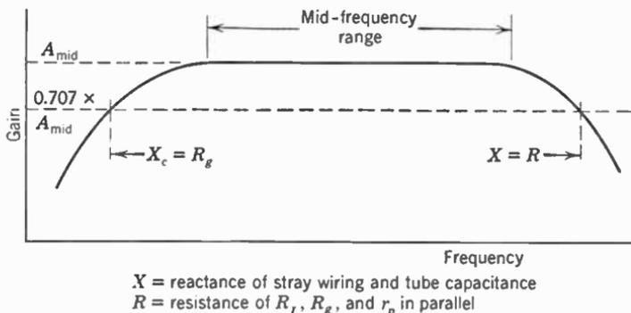
Fig. 4. Typical frequency-response curve of an  $RC$  amplifier.
