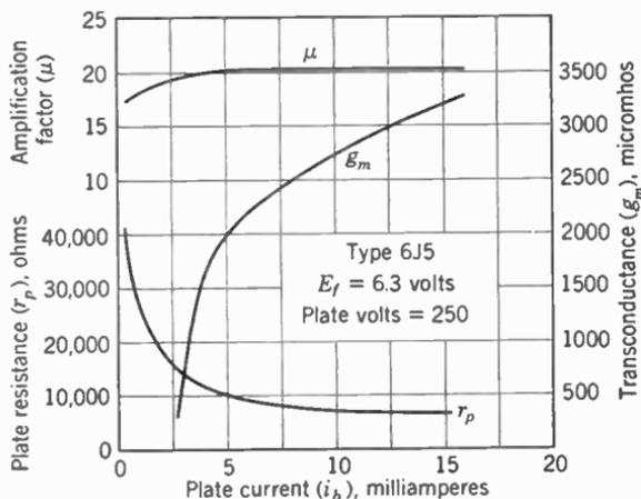
FIG. 12. Dependence of  $r_p$ ,  $g_m$ , and  $\mu$  on the plate current. Note that  $\mu$  is almost constant in value and that  $g_m$  increases as  $r_p$  decreases.
