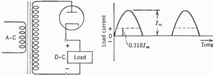
FIG. 5. A half-wave rectifier circuit. The load current is for a resistance load.
