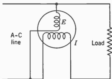
FIG. 11. Connections of a wattmeter into a circuit.
