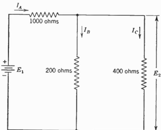
FIG. 17. A problem in series and parallel circuits.
