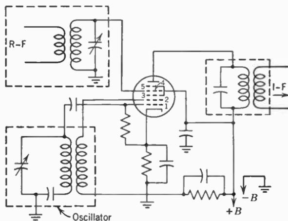
FIG. 6. Pentagrid converter circuit for frequency changing.
