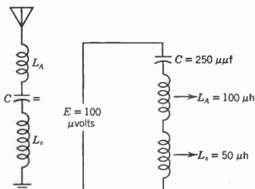
FIG. 23. An antenna and its equivalent circuit.
