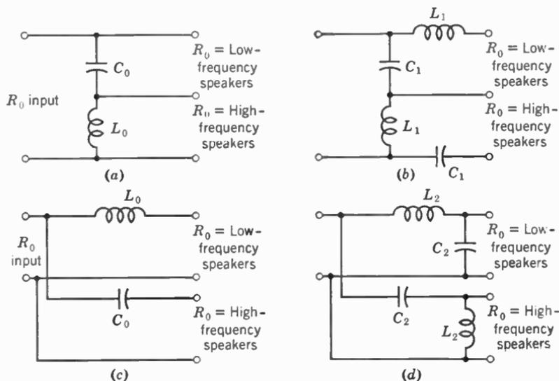
FIG. 18. Dividing networks to keep low frequencies out of high-frequency speaker, and vice versa.
