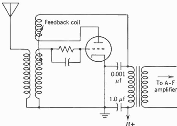
FIG. 2. Regenerative detector. Voltage fed back from plate to grid circuit increases sensitivity and selectivity.
