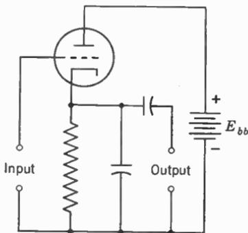
FIG. 13. Infinite input impedance detector.
