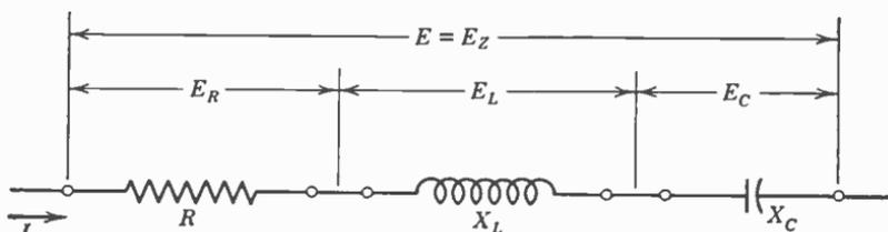
FIG. 25. Voltages across elements of an impedance.
