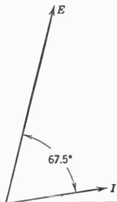
FIG. 14. Vector diagram showing lagging current. Same conditions as Fig. 13.
