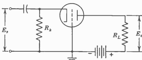
FIG. 22. Grounded-grid amplifier.
