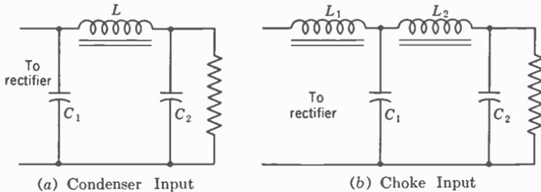
FIG. 11. Typical power supply filters.
