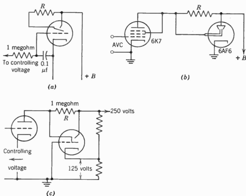
FIG. 13. Electron-ray tuning indicator tube circuits. In (b) and (c) separate d-c amplifiers are used, whereas in (a) the triode amplifier is in the same envelope with the indicator element.
