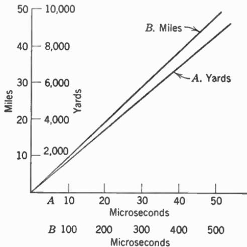
FIG. 2. Relation between transit time from radar to plane to radar and distance between plane and radar.
