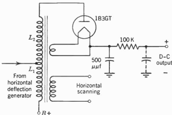
FIG. 10. Flyback power supply.
