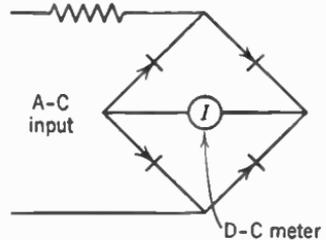
FIG. 3. Copper oxide rectifier meter.
