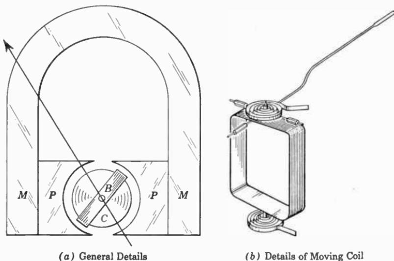
FIG. 1. Essential parts of a d'Arsonval moving-coil movement.
