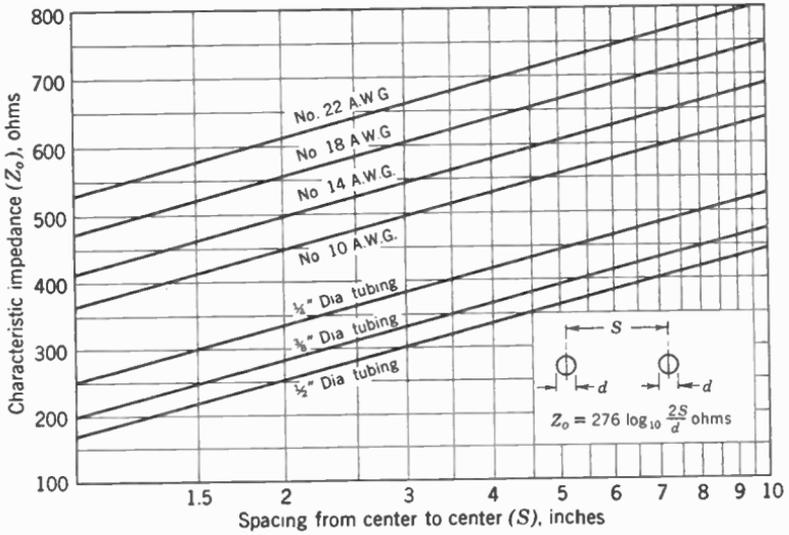
Impedance of Two-Wire Transmission Lines
