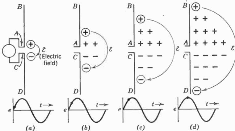
FIG. 22. Charges move out along a half-wave dipole antenna as the voltage rises.
