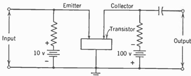
FIG. 15. Typical circuit connection of a transistor amplifier.
