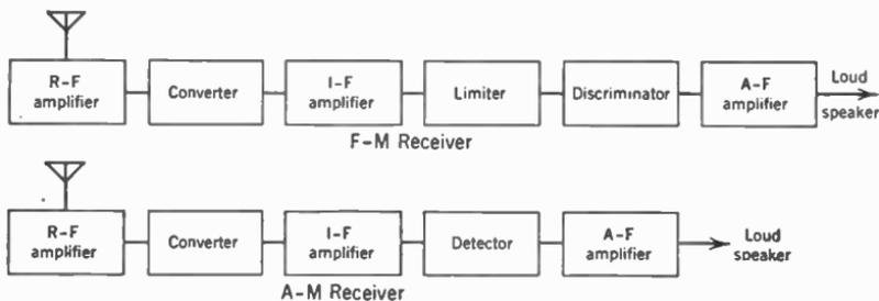
FIG. 7. Comparison of f-m and a-m receivers.
