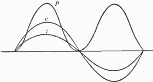
FIG. 29. In a resistive circuit, all power delivered by the generator is consumed by the external circuit. Voltage and current are in phase. The curve of instantaneous power has twice the frequency of the voltage and current curves.
