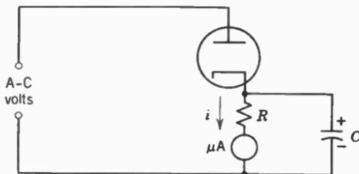
FIG. 7. Simple peak-reading diode voltmeter.
