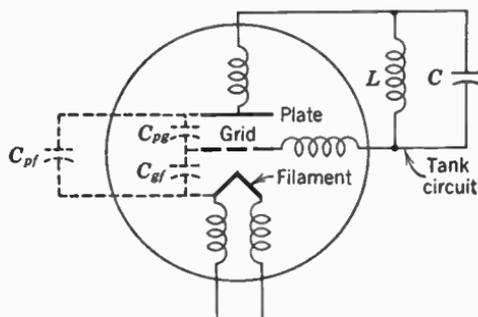
FIG. 1. Interelectrode capacitances and inductances inherent in tube.
