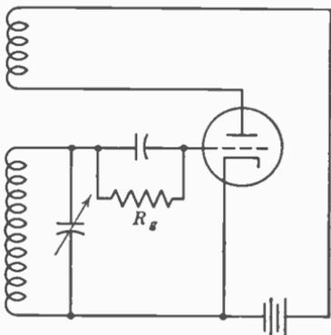
FIG. 1. Tuned-grid oscillator.
