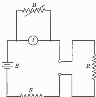
FIG. 13. Circuit of a series-type ohmmeter.
