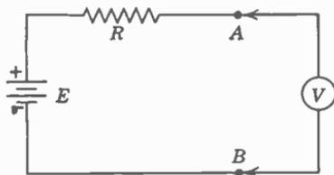
FIG. 17. The terminal voltage,  $V$ , depends upon the internal resistance.
