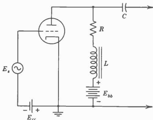
FIG. 5. Elements of impedance-coupled amplifier.
