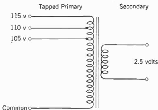
FIG. 10. Transformer with tapped primary.
