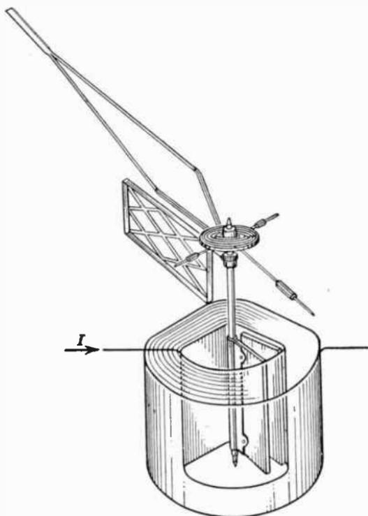
FIG. 5. Iron-vane type of meter for alternating currents.
