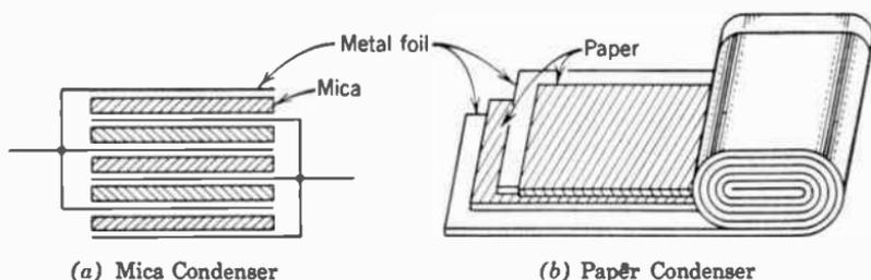
FIG. 3. Simple fixed condensers.
