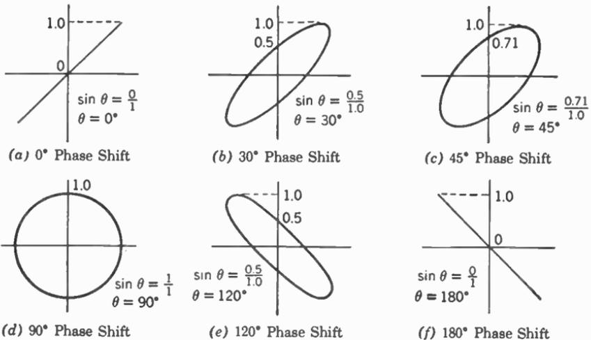
FIG. 18. Patterns produced for various phase differences between horizontal and vertical voltages.
