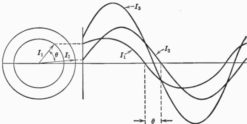
FIG. 7. Curve  $I_3$  is the sum of  $I_1$  and  $I_2$  at each instant.
