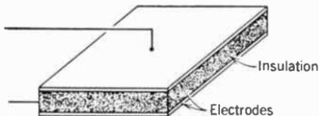
FIG. 1. Elements of a simple condenser.
