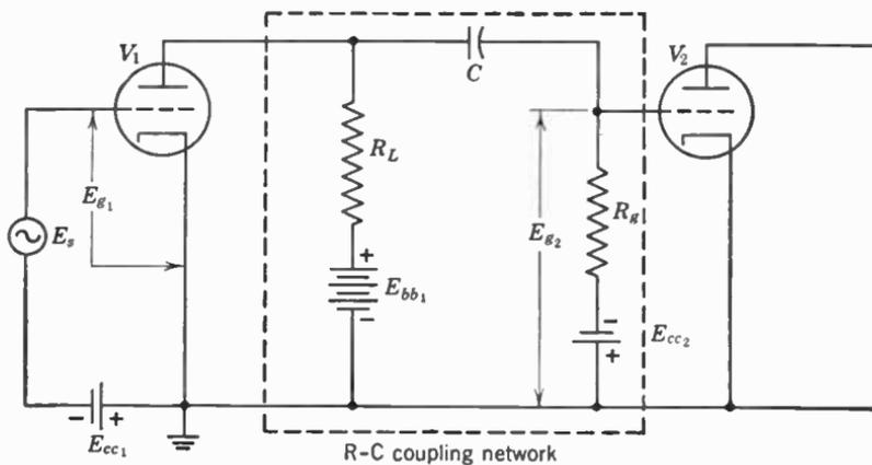
FIG. 2. Resistance-capacitance coupling of two amplifier stages.
