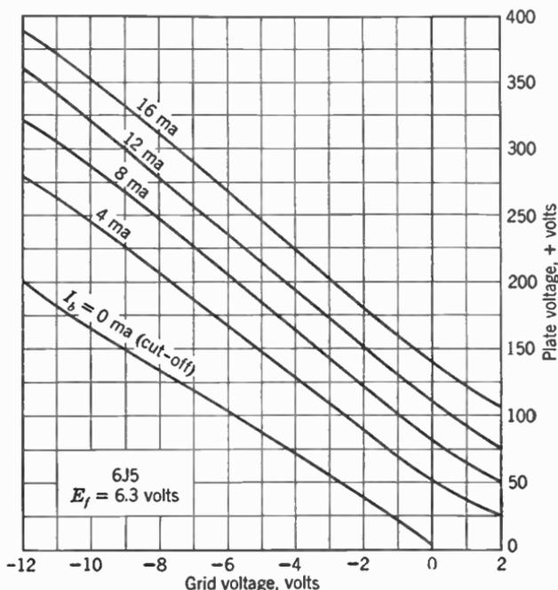
FIG. 11. Typical constant-current characteristics of a triode.
