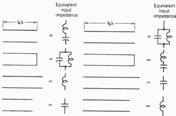
FIG. 5. Equivalent input impedance of several transmission line configurations.
