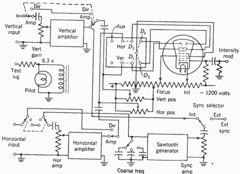
FIG. 16. Circuit of a typical cathode-ray oscillograph.
