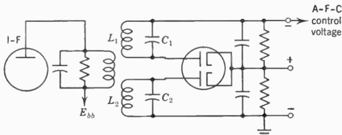
FIG. 12. Basic circuit for automatic frequency control.
