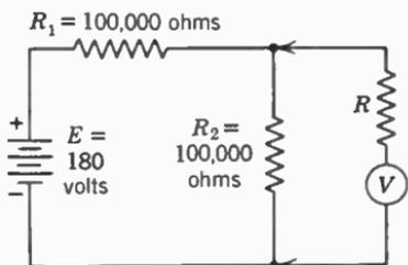
FIG. 10. An example of voltmeter "loading" so that different voltages are obtained.
