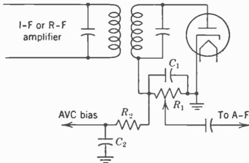
FIG. 15. Typical a-v-c circuit.
