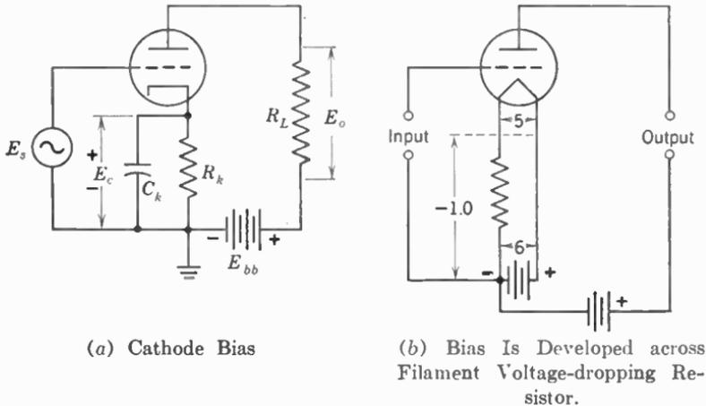
FIG. 20. Methods of biasing the grid negative.
