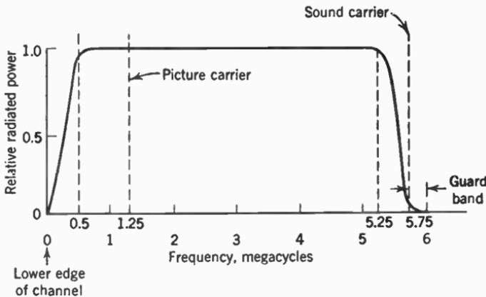
FIG. 6. Television transmitter channel with vestigial sideband transmission.
