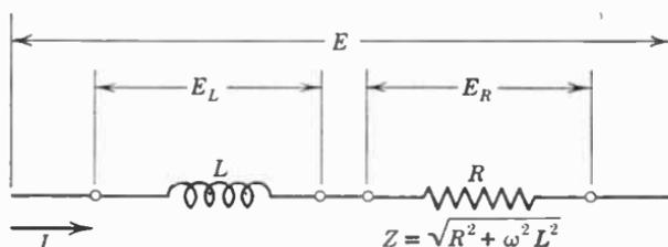
FIG. 24. A series circuit:  $\omega = 6.28 \times f$ .
