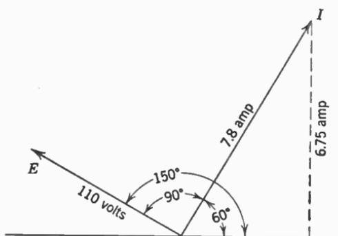
FIG. 17. Current lagging voltage by  $90^\circ$ .
