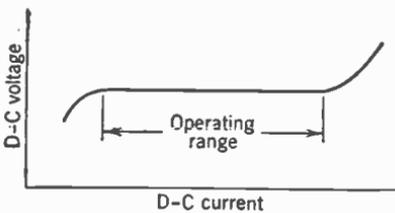
FIG. 18. Typical characteristics of a voltage-regulator tube.
