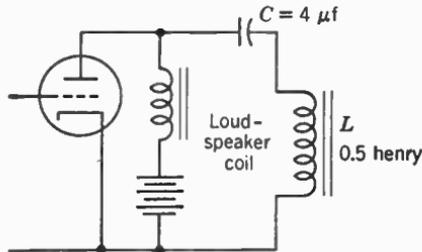
FIG. 11. An example of a resonant circuit.
