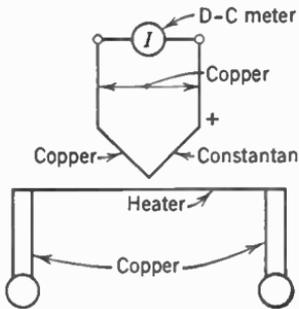
FIG. 2. Elements of thermocouple meter.
