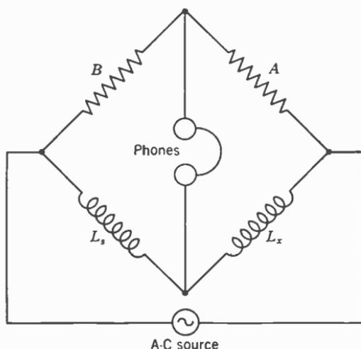
FIG. 7. Wheatstone bridge arranged to compare inductances. Here  $L_s$  is a known "standard" inductance to which the unknown inductance,  $L_x$ , is to be compared. One of the ratio arm resistances must be adjustable unless  $L_s$  is adjustable. The bridge is balanced when no sound is heard in the telephones, and at this adjustment the unknown inductance can be determined by the formula in the text.
