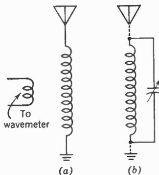
FIG. 7. To measure the capacitance of an antenna.
