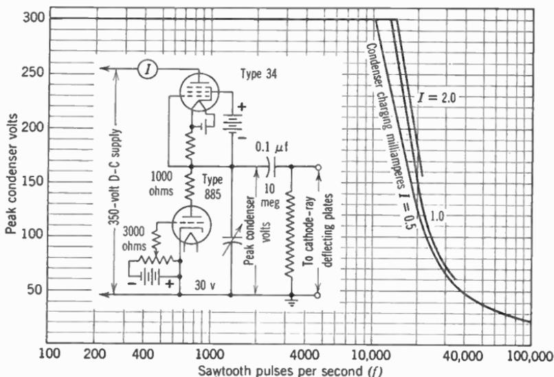
Fig. 14. Complete sweep-voltage oscillator circuit and its characteristic. (From RCA.)
