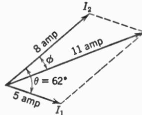
FIG. 9. Vector diagram of two sine waves combined to produce a new sine wave of 11 amp maximum value.
