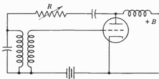
FIG. 6. Circuit often used in low- (audio-) frequency oscillators. Feedback is provided by resistance, which also loads up the plate circuit and straightens out the  $E_g-I_p$  characteristic.
