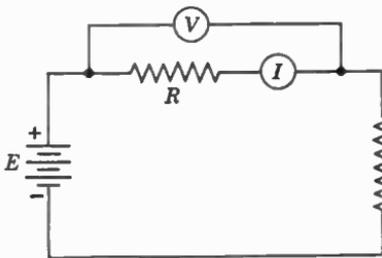
Fig. 12. Ammeter-voltmeter method of measuring resistance.
