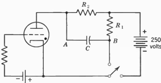
FIG. 7. An  $RC$  circuit for switching a thyatron.
