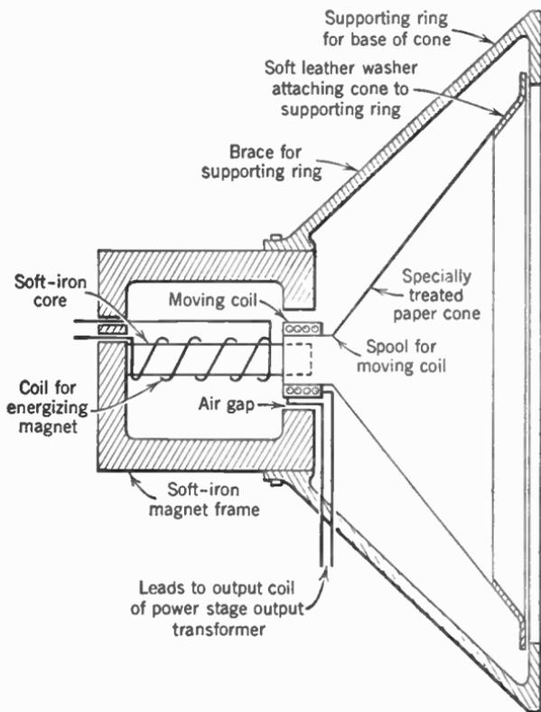
FIG. 14. Modern "dynamic" or moving-coil loud speaker.
