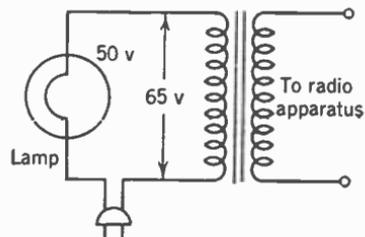
FIG. 19. Use of current regulator or ballast tube.
