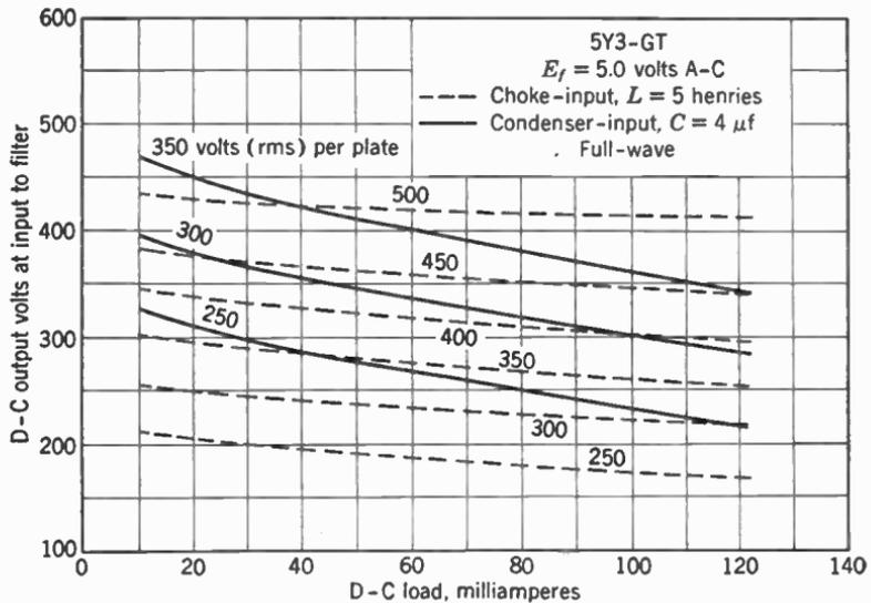
FIG. 13. Comparison of condenser-input and choke-input filter systems. Voltage drops due to resistance of filter chokes must be added to these regulation curves if complete regulation data are desired.
