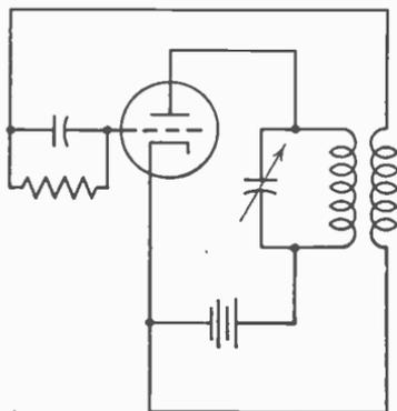
FIG. 2. Tuned-plate oscillator.
