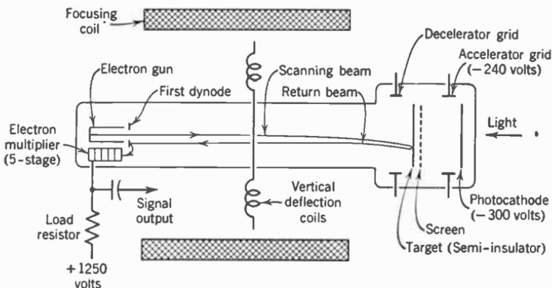
FIG. 3. Image orthicon, simplified diagram.
