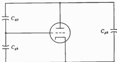
FIG. 6. Tube interelectrode capacitances.
