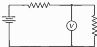
FIG. 8. Voltmeter goes across circuit being measured.
