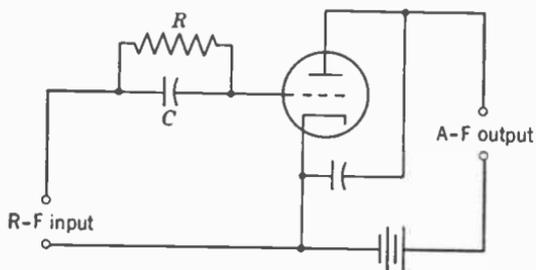
FIG. 14. Grid-leak and condenser detector.
