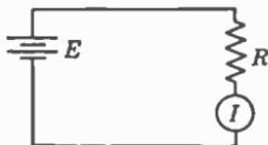
FIG. 7. Proper connection for measuring current.
