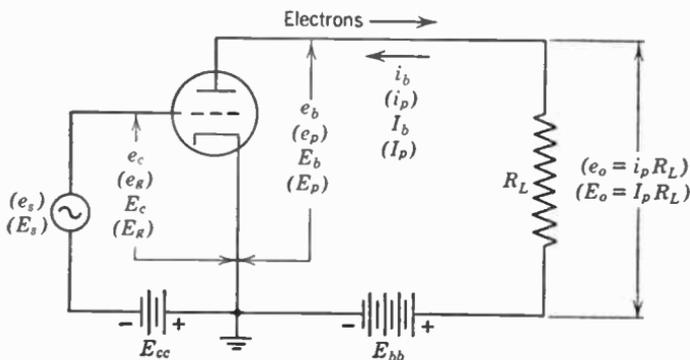
FIG. 3. Unbracketed lower-case letters  $i_p$ ,  $e_c$ , etc., indicate instantaneous total values; bracketed lower-case letters ( $i_p$ ), ( $e_p$ ), etc., indicate instantaneous value of a-c component; unbracketed capital letters,  $E_b$ ,  $E_c$ , etc., indicate d-c or average values; and bracketed capital letters ( $E_p$ ), ( $I_p$ ), etc., indicate rms a-c values. Brackets are not used in general practice.
