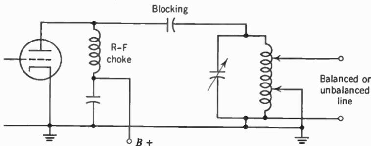
(d) Coupling for Balanced or Unbalanced Line
