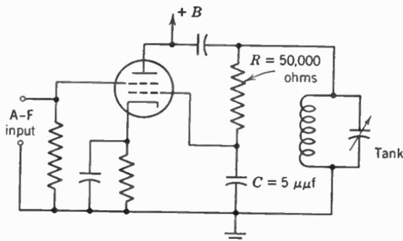
FIG. 5. A workable reactance-tube modulator which affects the resonant frequency of the tank as though a variable inductance were shunted across the tank.
