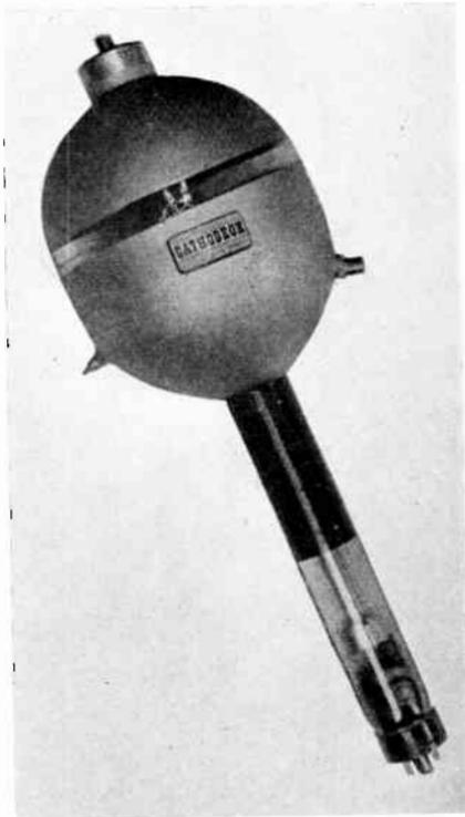
FIG. 10.3C. A STILL PICTURE GENERATOR TUBE
