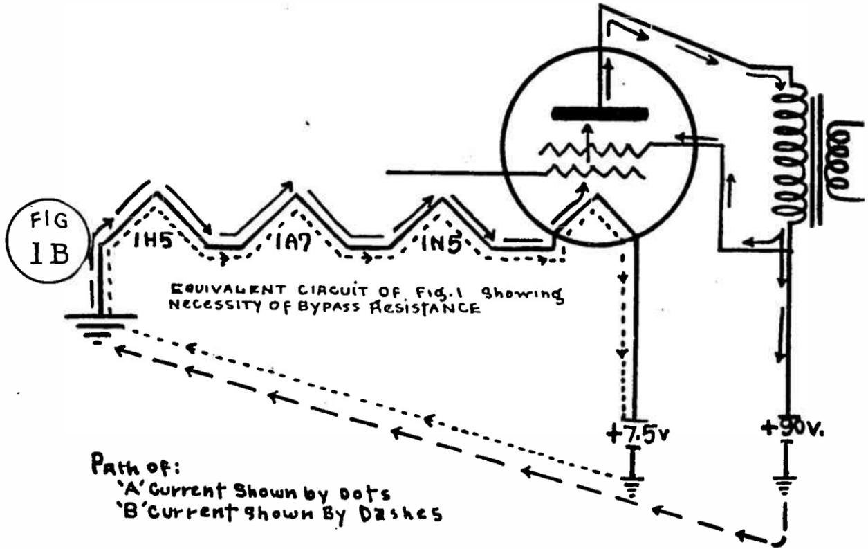
EQUIVALENT CIRCUIT OF FIG.1 showing
