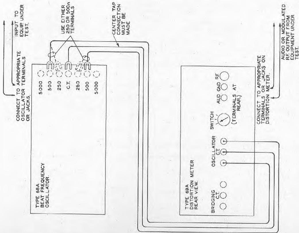
DISTORTION METER CONNECTIONS
