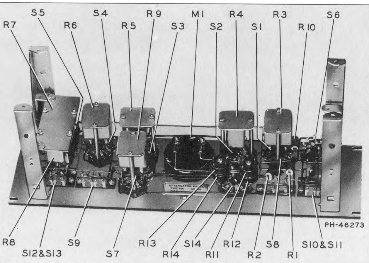
FIGURE 2 - ATTENUATOR PANEL
