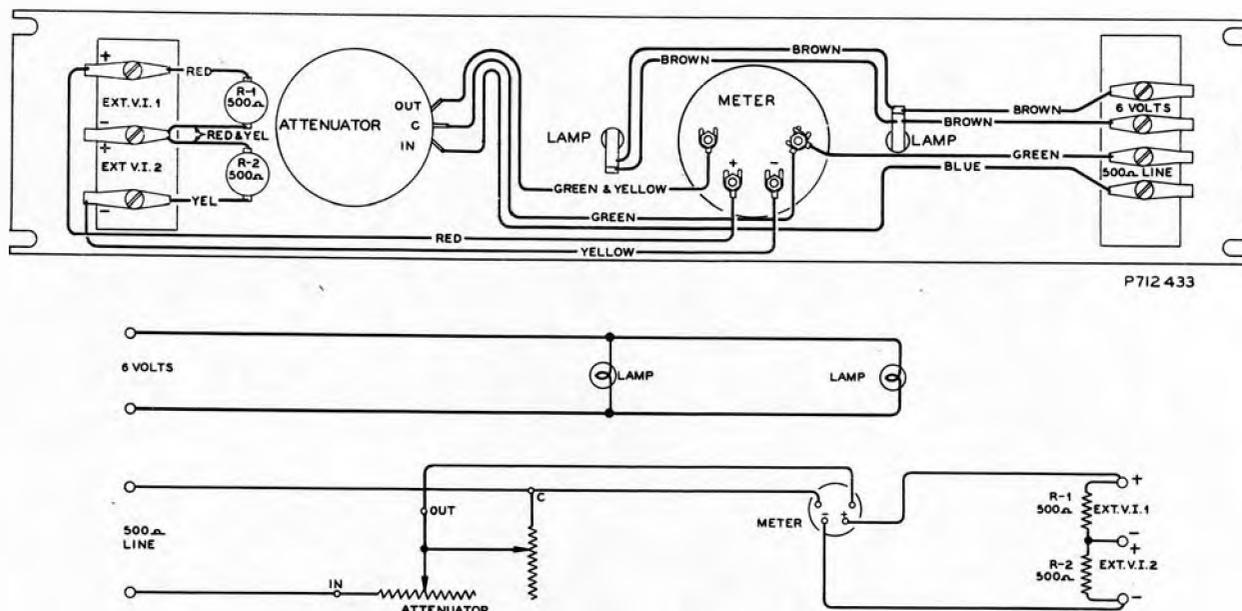
Figure 2 - Schematic and Wiring - MI-3115-A
