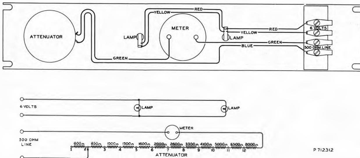
Figure 1 - Schematic and Wiring - MI-3115
