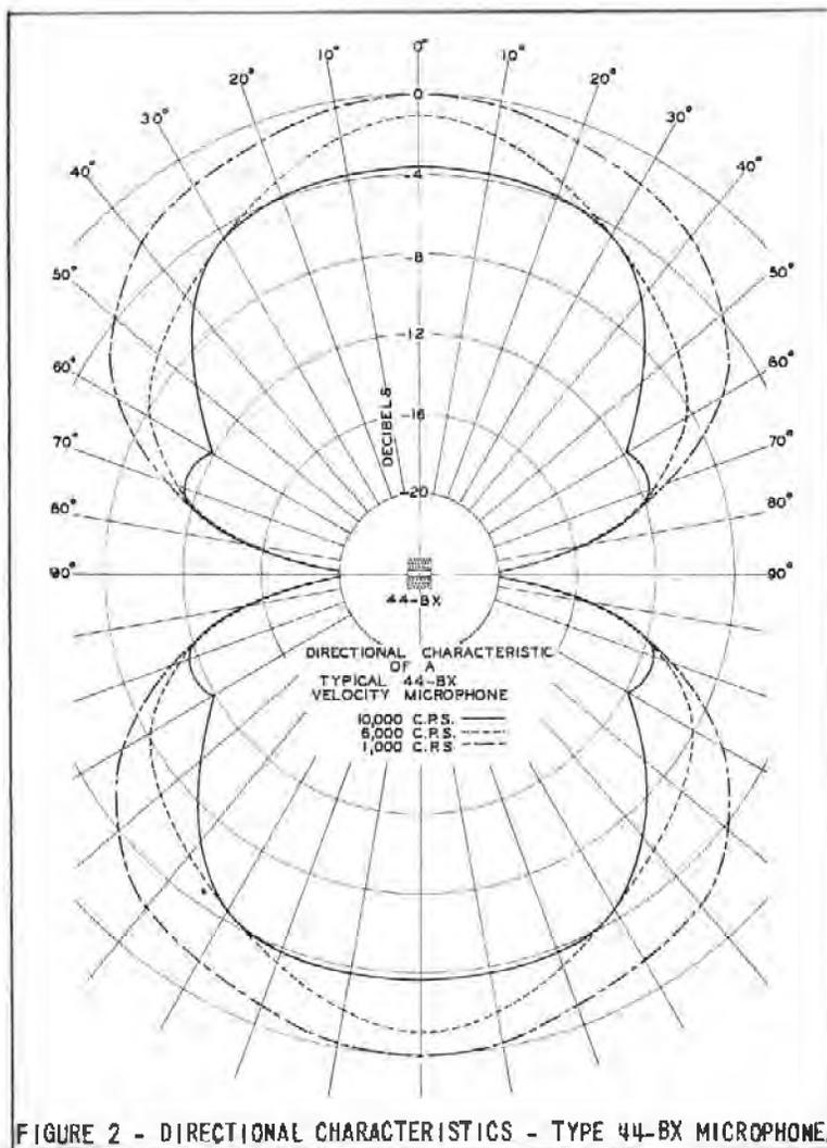
FIGURE 2 - DIRECTIONAL CHARACTERISTICS - TYPE 44-BX MICROPHONE.
