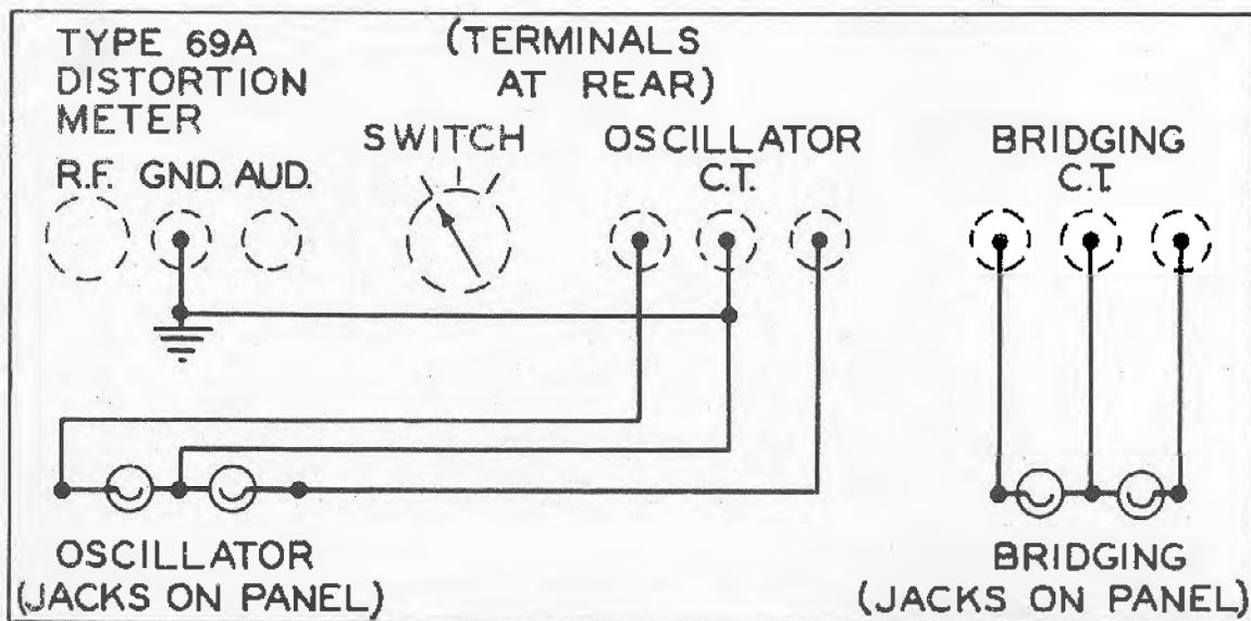
FIGURE 2 - INTERNAL WIRING
