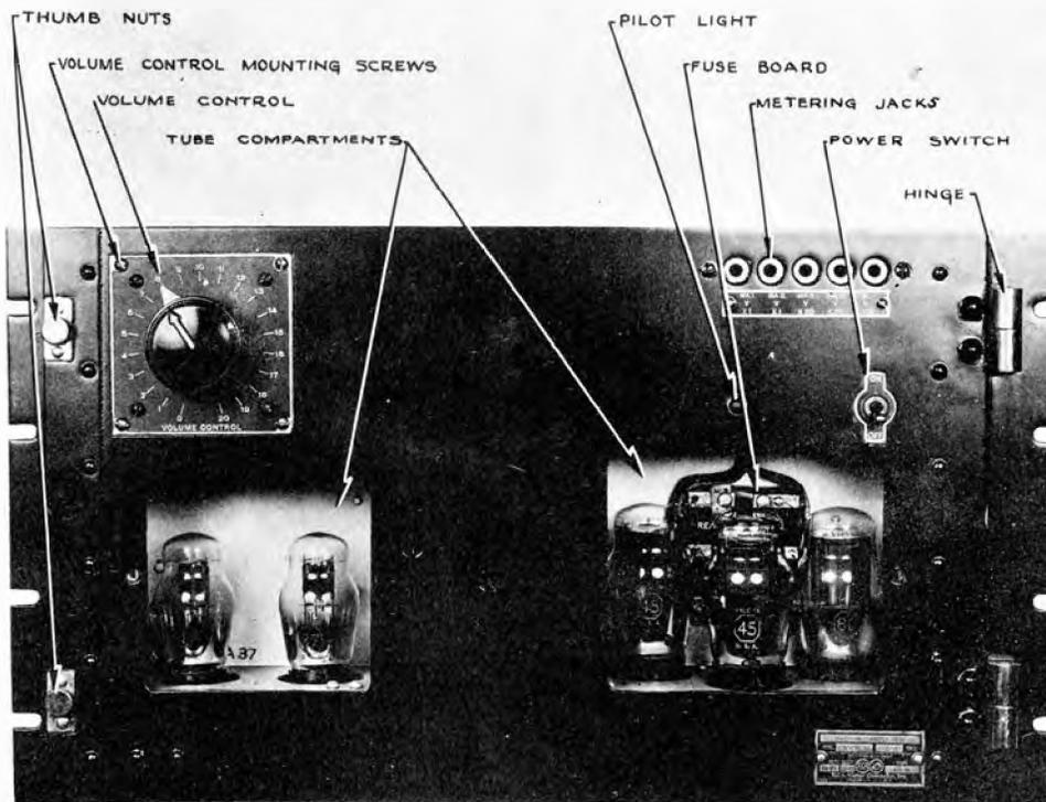
FIGURE 3—FRONT VIEW OF MODEL PA109A1 BRIDGING AMPLIFIER (MI-3223)
