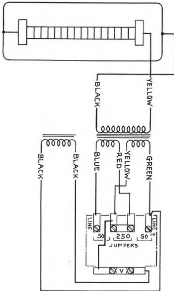
FIGURE 5—SCHEMATIC DIAGRAM OF VELOCITY MICROPHONE
