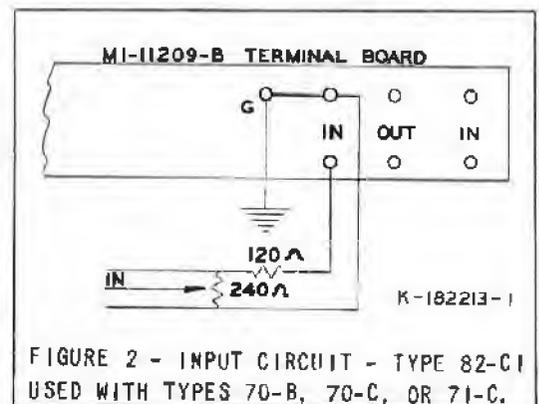
All audio input leads should be MI-64 shielded cable, or a shielded twisted pair, insulated for 200-volts, and need not be larger than No. 19 A.W.G. To prevent undesirable pickup, the leads should
