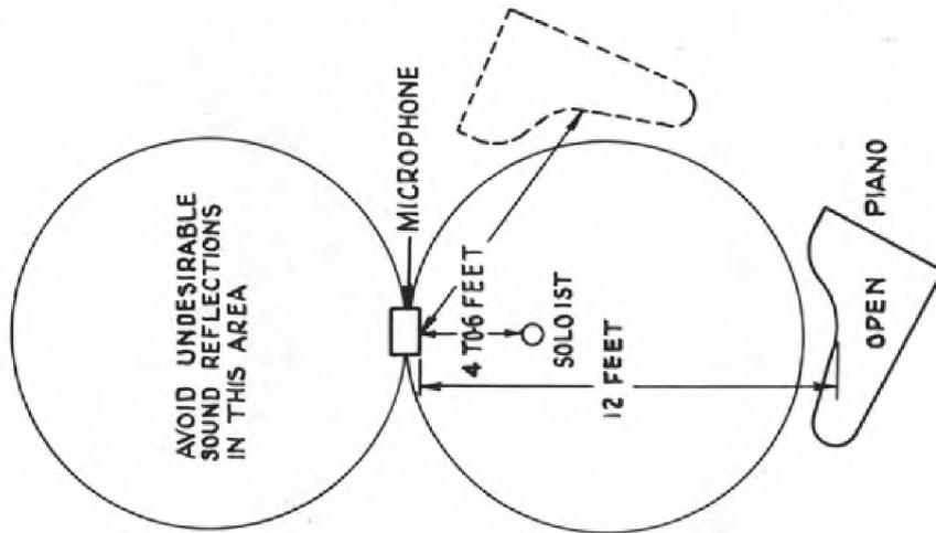
FIGURE 8 —MICROPHONE SETUP FOR SOLOIST WITH PIANO
