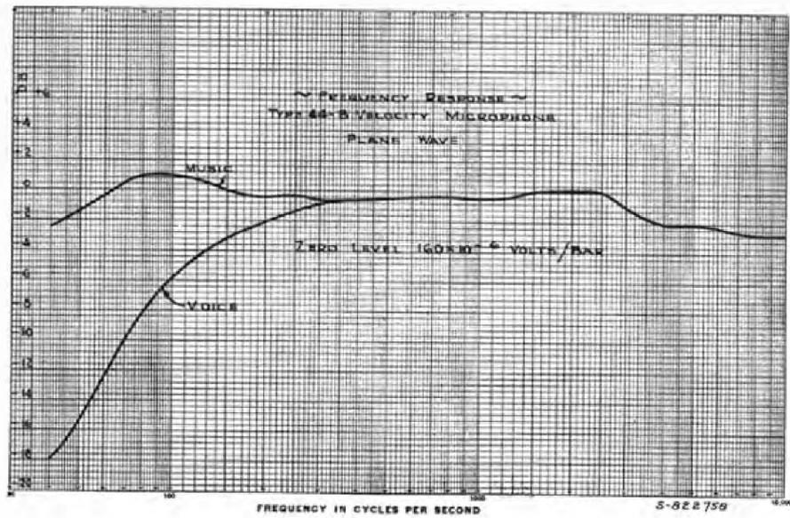
FIGURE 6—RESPONSE CHARACTERISTICS OF VELOCITY MICROPHONE
