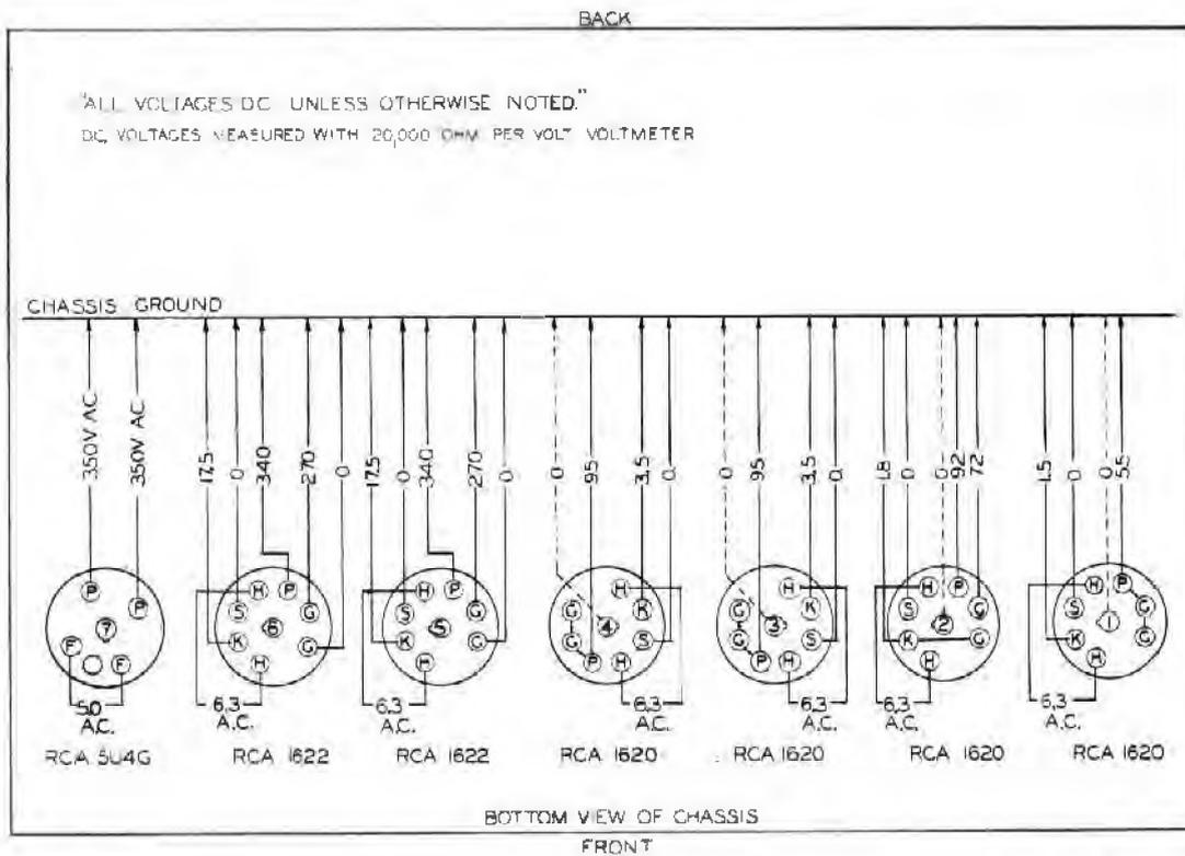
FIGURE 7 - TUBE SOCKET VOLTAGES - TYPE 82-C1 AMPLIFIER.
