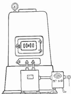
A. This interference is usually heard as a loud roaring noise, which may continue from 15 to 60 seconds, or during the entire period during which the oil burner is in operation. The duration of the interference from the ignition system will be dependent upon the type of electric ignition employed.
