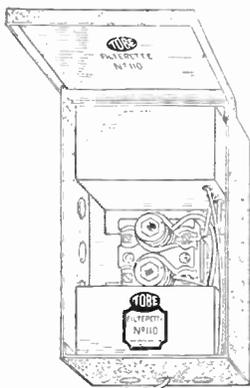
Filterettes of this type should be connected in series with the leads to the interference creating apparatus, and should be mounted as close as possible to it. The return wire from a Filterette of this type should, of course, be as short as possible, and should be connected to a carefully cleaned part of the frame of the machine.
