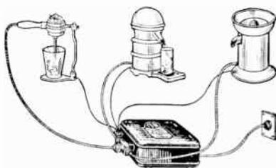
The Tobe Filterette No. 110 P. O. is recommended for use on large radio sets as a direct line filter. This Filterette when attached direct to the radio serves as an effective blocking device to prevent all electrical disturbances from entering the set from the power line.
