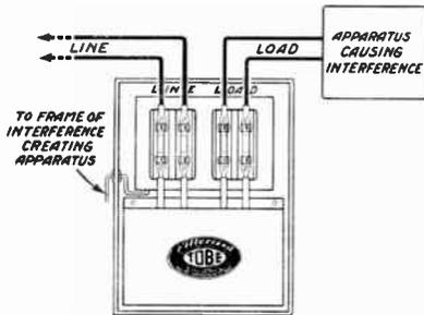
The return wire from the Filterette should be connected in the most direct manner possible to a carefully cleaned part of the motor frame.
