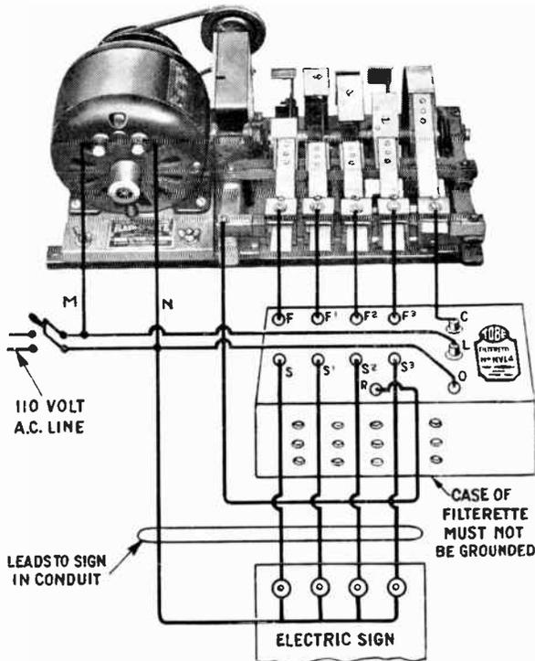
WIRING AND CONNECTIONS, FILTERETTE TYPE NYL-4
