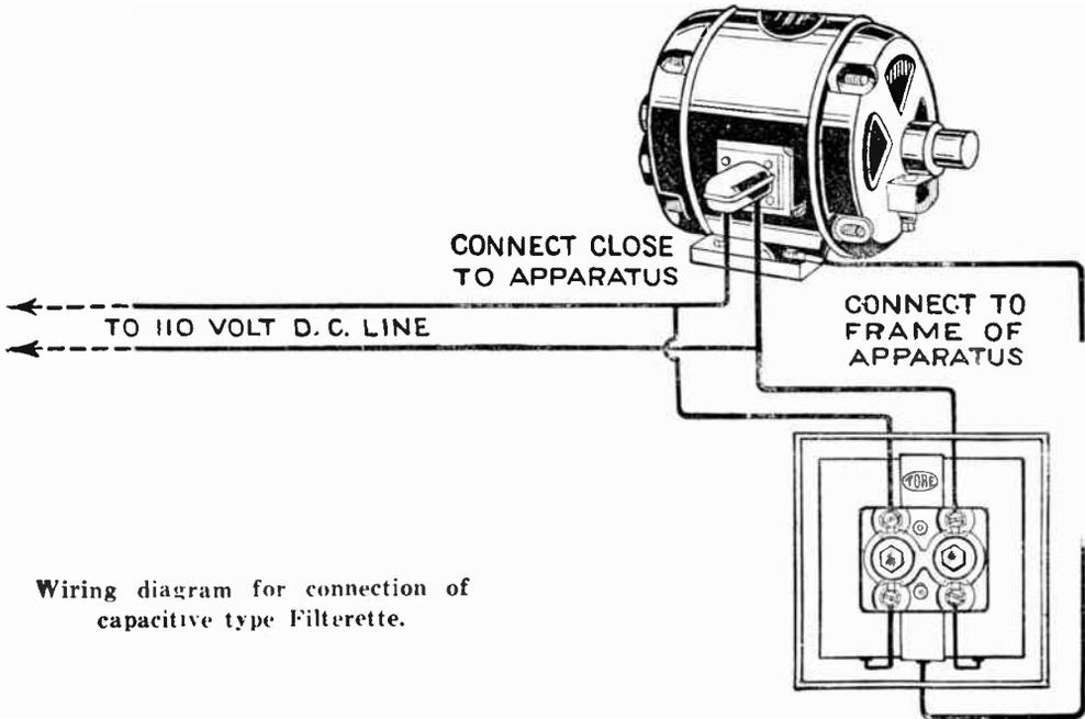
Wiring diagram for connection of capacitive type Filterette.
