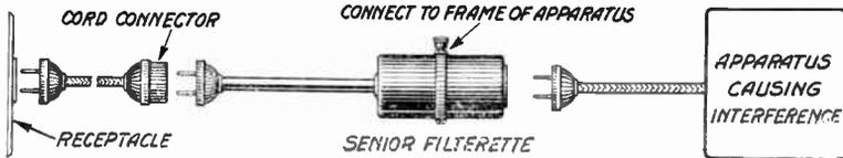
Maximum benefit is obtained from the use of this Filterette when it is located as close as possible to the source of the interference. This installation may best be accomplished by inserting a separable cord connector (Hubbell No. 6116, Benjamin No. KT-130, Bryant KT-130, or equivalent) in the attachment cord of the apparatus, and connecting the Filterette as shown in the above sketch.
