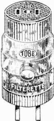
An ideal Filter for small motors such as are used for electric fans, hair dryers, barbers' clippers, vacuum cleaners, cash registers, etc. Plugs into the line, and it is necessary only to run a small wire from the binding post on the Filterette to any part of the motor frame. Interference is eliminated at once.
