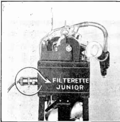
Provided the receiver or antenna lead-in is in close proximity to the interference creating appliance, such installation of the Filterette may not prove satisfactory. Under these circumstances it will probably be necessary to locate the Filterette closer to the source of the interference. This is accomplished by cutting the attachment cord of the appliance and inserting the Filterette at the point where the cord is cut.
