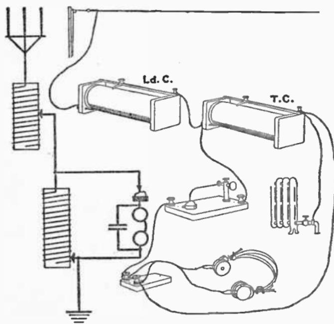
FIG. 23.—A LOADING COIL IN THE AERIAL CIRCUIT.
