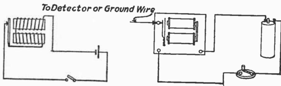
FIG. 22.—HOOK-UP FOR THE TEST BUZZER.
