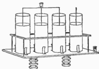
FIG. 88.—A TRANSMITTING CONDENSER MADE UP OF JARS.
