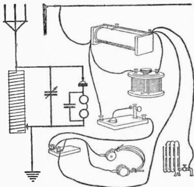
FIG. 27.—TUNING COIL CRYSTAL DETECTOR SET WITH VARIABLE CONDENSER IN PARALLEL WITH BOTH THE AERIAL CIRCUIT AND THE LOCAL CIRCUIT.
