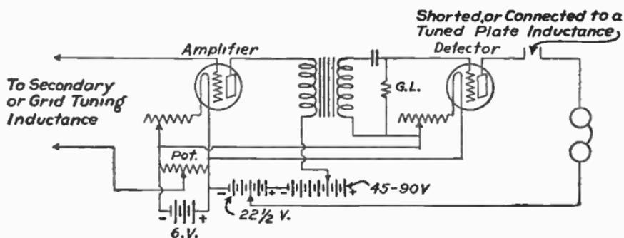
FIG. 80.—HOOK-UP FOR ONE STAGE OF RADIO-FREQUENCY AMPLIFICATION AND A DETECTOR.
