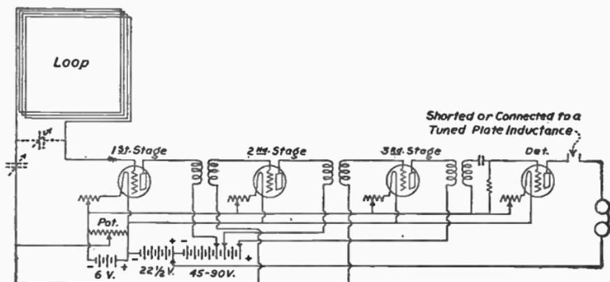
FIG. 81.—COMPLETE HOOK-UP FOR A LOOP AERIAL, THREE STAGES OF RADIO-FREQUENCY AMPLIFICATION AND A DETECTOR.
