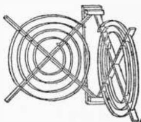
FIG. 86.—A PANCAKE OSCILLATION TRANSFORMER.
