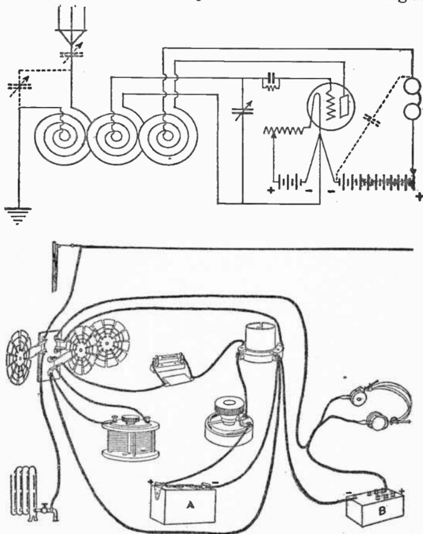
FIG. 66.—HOOK-UP FOR THREE SPIDERWEB COILS IN A REGENERATIVE SET.
