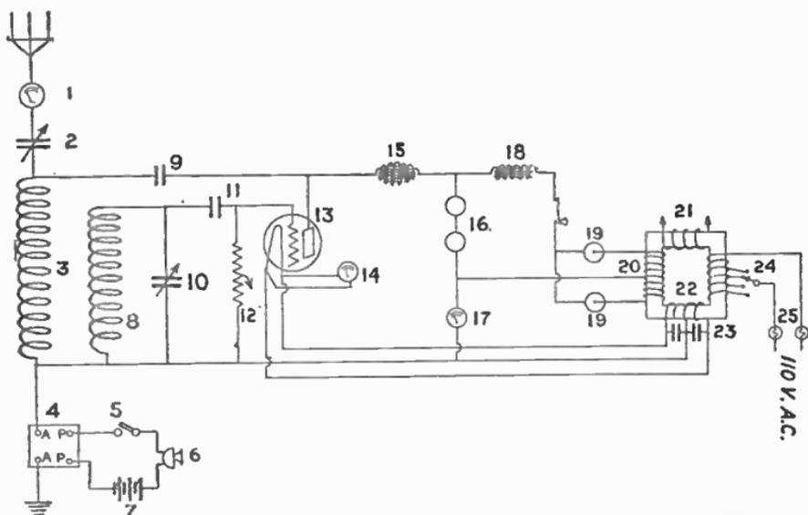
FIG. 94.—COMPLETE HOOK-UP FOR A VACUUM TUBE TRANSMITTER.
