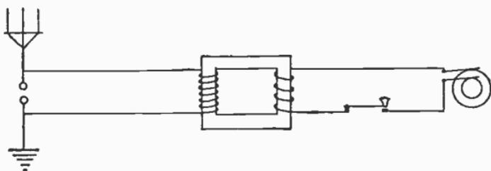
FIG. 85.—ELEMENTS OF A SPARK TRANSMITTER.
