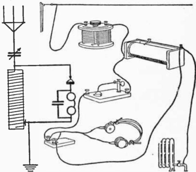
FIG. 28.—CRYSTAL DETECTOR SET WITH A VARIABLE CONDENSER IN SERIES IN THE AERIAL CIRCUIT.
