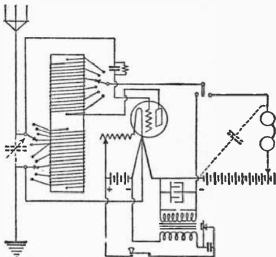
FIG. 93.—USE OF A SPARK COIL TO INCREASE THE POWER OF THE RECEIVER TYPE OF TRANSMITTER.
