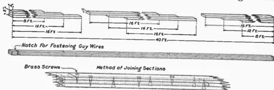
FIG. 7.—METHOD OF CONSTRUCTING A 40-FOOT LAMINATED MAST.
