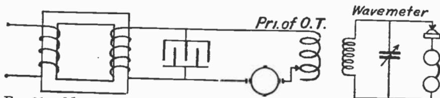
FIG. 91.—METHOD OF COUPLING THE WAVE METER TO THE PRIMARY OF THE OSCILLATION TRANSFORMER.
