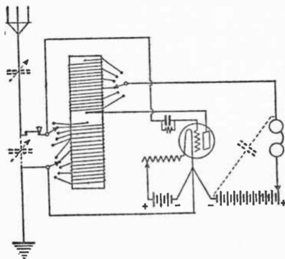
FIG. 92.—THE REGENERATIVE RECEIVING SET HOOKED UP AS A TRANSMITTER.
