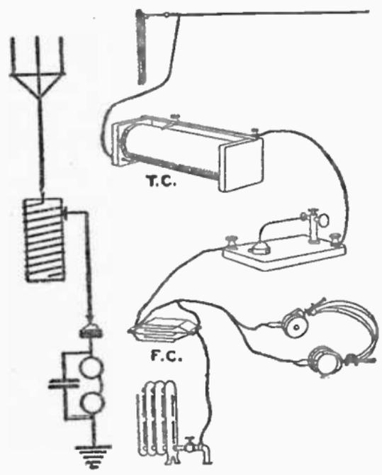
FIG. 16.—THE SIMPLE RECEIVING SET WITH A TUNING COIL AND A FIXED CONDENSER ADDED TO THE CIRCUIT.
