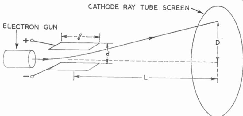
FIG. 10.—ELECTROSTATIC DEFLECTION OF AN ELECTRON BEAM.
