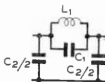
FIG. 46.—SHUNT-DERIVED  $\pi$  SECTION.
