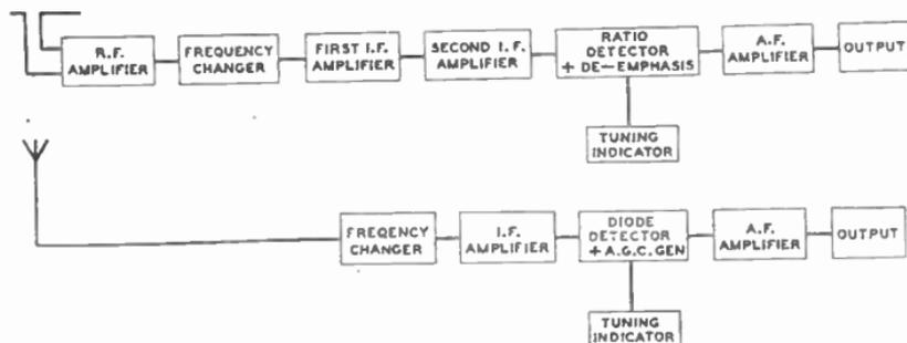
FIG. 29.—SCHEMATIC CIRCUIT DIAGRAM OF F.M./A.M. RECEIVER.
