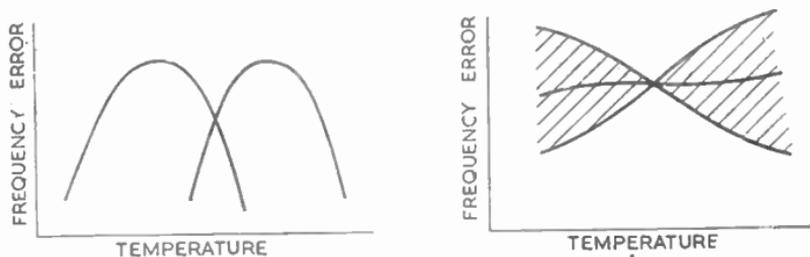
(a) B.T. CUT CRYSTALS
