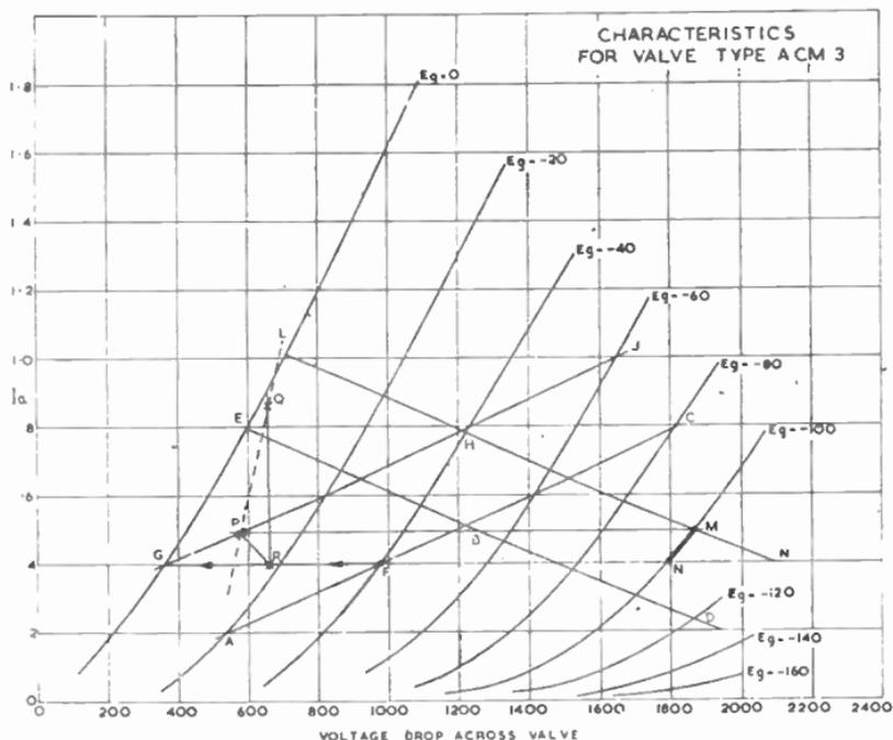
FIG. 36.—VOLTAGE EXCURSIONS FOR A SHUNT-REGULATED AMPLIFIER.
