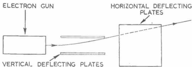
FIG. 11.—ARRANGEMENT OF VERTICAL AND HORIZONTAL DEFLECTING PLATES IN A CATHODE-RAY TUBE.
