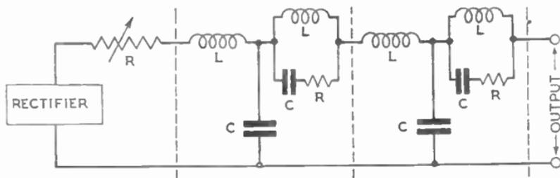
FIG. 46.—IMPROVED FORM OF "BUILT-OUT" FILTER.
