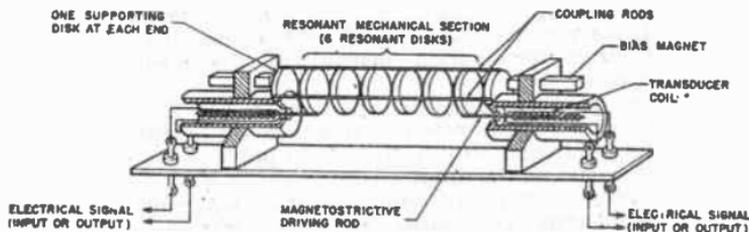
FIG. 6.—FUNCTIONAL DIAGRAM OF A MECHANICAL FILTER.
