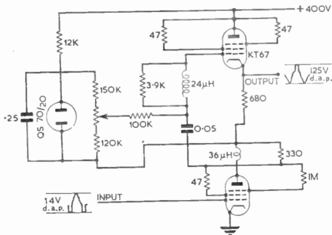
FIG. 39.—PRACTICAL SHUNT-REGULATED AMPLIFIER.
