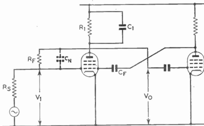
FIG. 26 (a).—CIRCUIT GIVING "OPTIMAL FEEDBACK".
