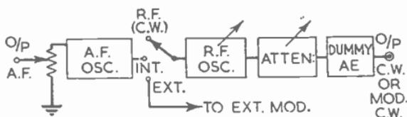
FIG. 19.—BLOCK SCHEMATIC LAYOUT OF A TEST OSCILLATOR.
