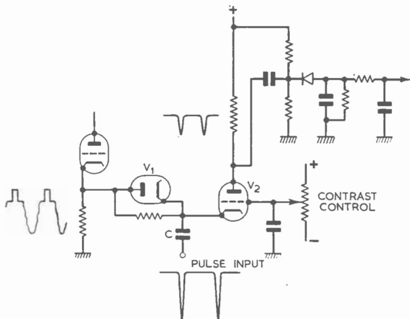
FIG. 48.—AUTOMATIC PICTURE CONTROL.
