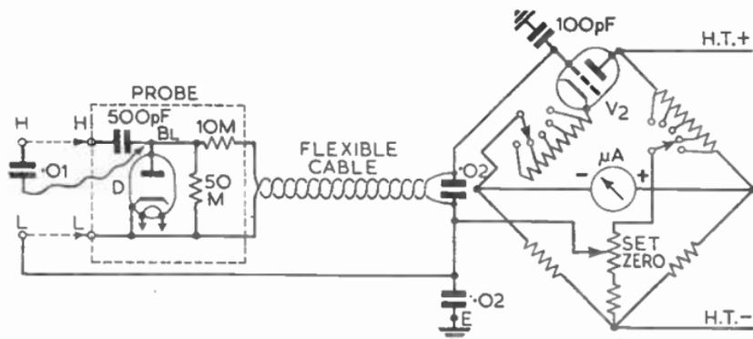
FIG. 16.—TYPICAL VALVE VOLTMETER AND PROBE UNIT.
