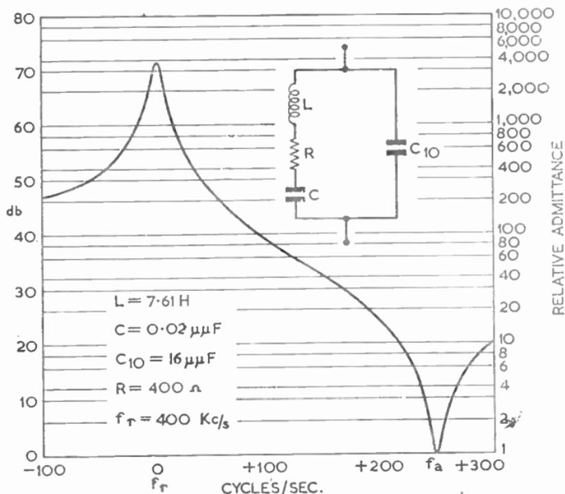
FIG. 3.—RESONANCE CURVE FOR A QUARTZ CRYSTAL.
