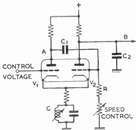
FIG. 39 (top).—CATHODE-COUPLED MULTI-VIBRATOR AND ASSOCIATED WAVEFORMS. (below) A COMMON VARIANT OF THE BASIC MULTI-VIBRATOR, ELIMINATING THE USE OF A DOUBLE VALVE.
