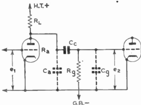
FIG. 60.—RESISTANCE-CAPACITANCE COUPLING.
