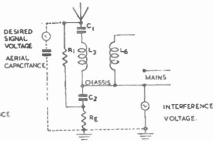
FIG. 11.—ALTERNATIVE AERIAL INPUT CIRCUIT FOR REDUCTION OF MAINS-BORNE INTERFERENCE.
