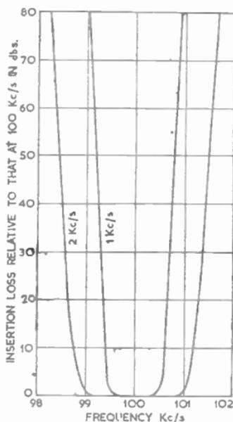
FIG. 15 (right).—CRYSTAL FILTER RESPONSE CURVES.
