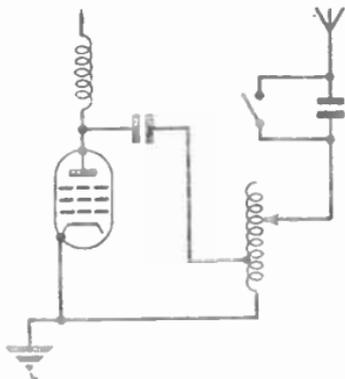
FIG. 12.—"ANODE TAP" OUTPUT.
