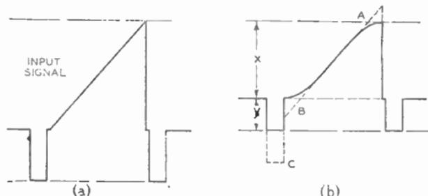
FIG. 61.—(a) UNDISTORTED LINE SAW-TOOTH WAVEFORM; (b) WAVEFORM DISTORTED DUE TO TRANSMITTER VALVE CHARACTERISTICS.
