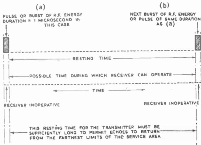
FIG. 18.—RELATION OF PULSE LENGTH TO REPETITION FREQUENCY.
