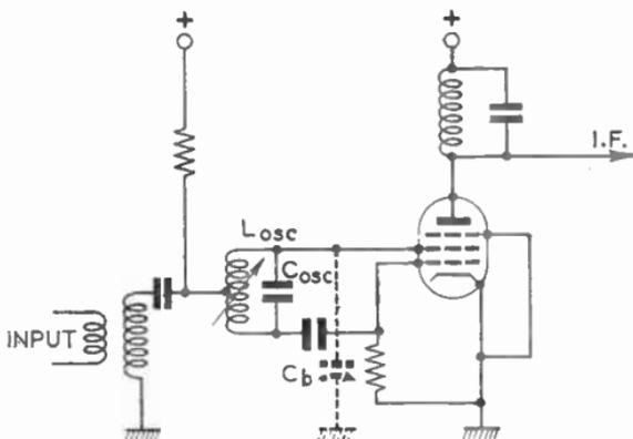
FIG. 8.—SELF-OSCILLATING MIXER.
