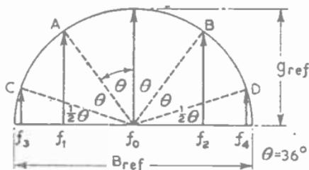
FIG. 20.—CALCULATION OF CIRCUIT IMPEDANCES AND TUNING FREQUENCIES.
