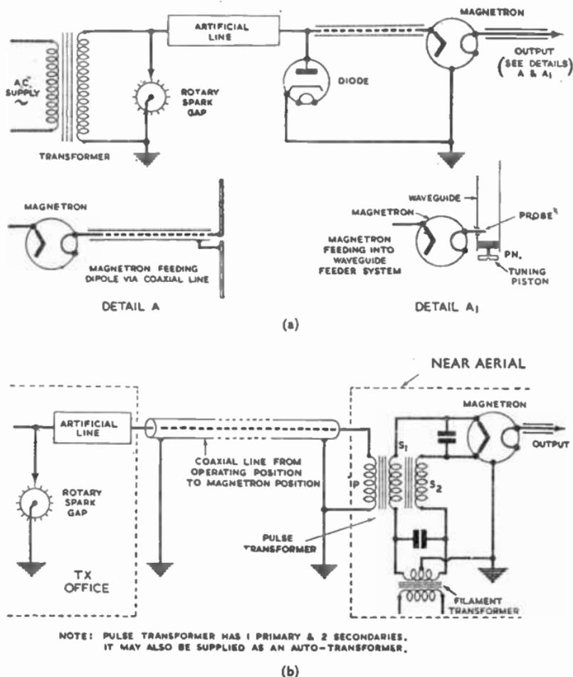
FIG. 44.—INPUT AND OUTPUT CIRCUITS FOR MAGNETRON R.F. GENERATOR.
