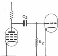
FIG. 33.—TYPICAL LOW-FREQUENCY RESPONSE-DETERMINING COUPLING ELEMENTS.
