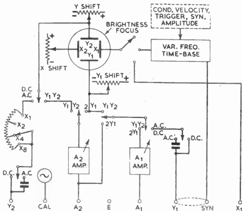
FIG. 44.—SWITCHING AND INPUT CIRCUIT OF A TYPICAL OSCILLOSCOPE.
