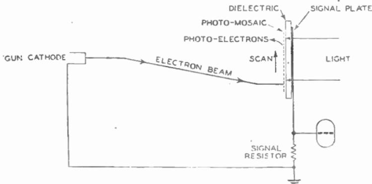
FIG. 23.—THE BASIC PRINCIPLE OF THE C.P.S. EMITRON.
