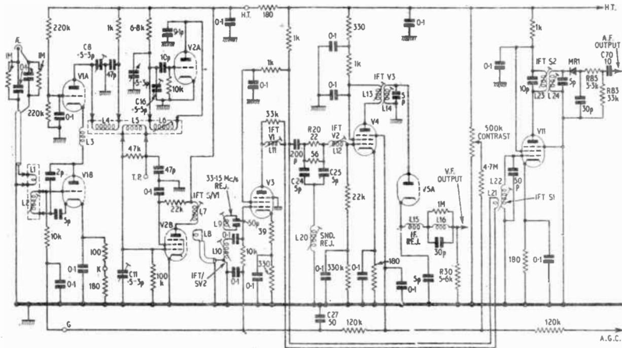
FIG. 7 ( ).—Circuit Diagram of the Turret Tuner Unit and I.F. Stages of an R.C.D. Receiver.
