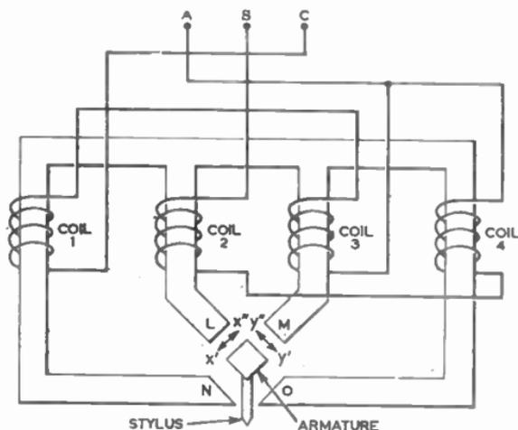
FIG. 22.—ONE ARRANGEMENT OF VARIABLE-RELUCTANCE STEREO CARTRIDGE.
