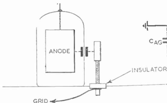
FIG. 12 (left).—METHOD OF OBTAINING SMALL NEUTRALIZING CAPACITANCE.
