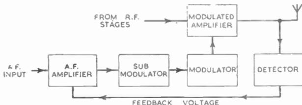
FIG. 23.—METHOD OF APPLYING OVERALL FEEDBACK TO A TRANSMITTER.
