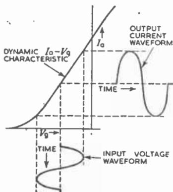
FIG. 2.—ILLUSTRATING CLASS A OPERATION.
