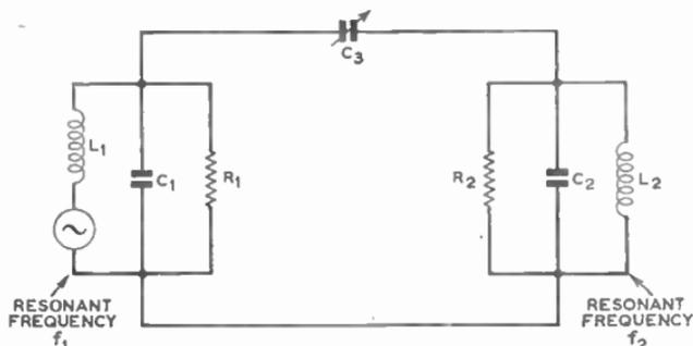
FIG. 29.—TWO CIRCUITS COUPLED BY A TIME-VARYING CAPACITOR.
