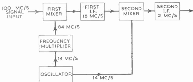
FIG. 26.—ALTERNATIVE METHOD OF DOUBLE MIXING.
