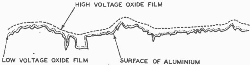
FIG. 5.—ETCHED-FOIL CROSS-SECTION SHOWING LOW- AND HIGH-VOLTAGE OXIDE FILMS.
