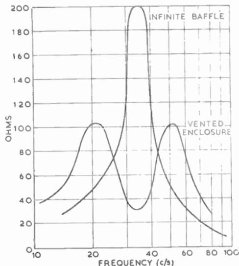
FIG. 16.—IMPEDANCE, FREQUENCY CHARACTERISTICS OF A LOUDSPEAKER MOUNTED ON AN INFINITE BAFFLE COMPARED WITH MOUNTING IN A VENTED ENCLOSURE.
