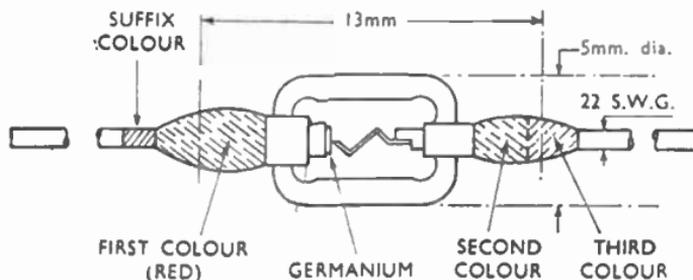
FIG. 10.—ARRANGEMENT OF TYPICAL GERMANIUM CRYSTAL UNIT.
