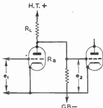
FIG. 59.—RESISTANCE COUPLING.
