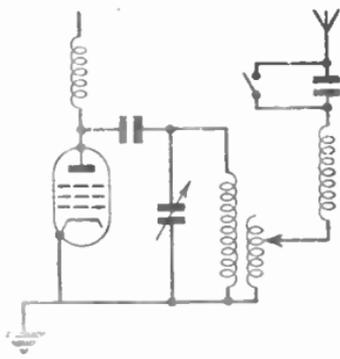
FIG. 11.—INDUCTIVE OUTPUT COUPLING.
