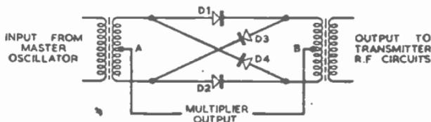
FIG. 9.—RING MODULATOR WHICH CAN BE USED IN THE DIVIDER CIRCUIT OF FIG. 8.
