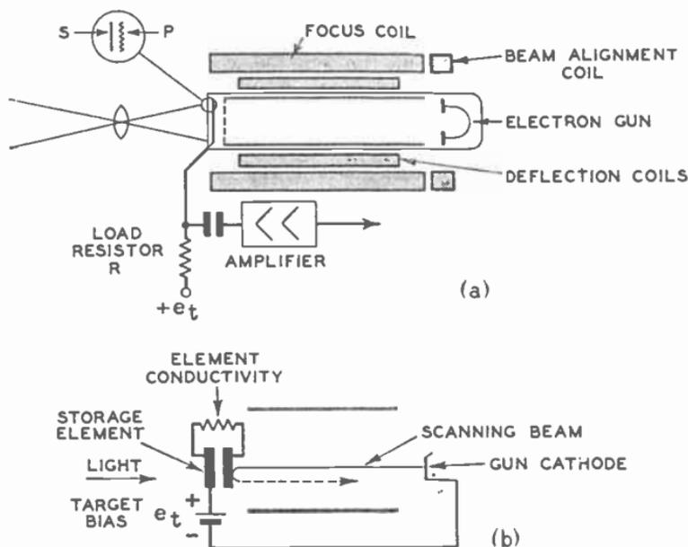
FIG. 9.—FUNCTIONAL DIAGRAM OF A PHOTOCONDUCTIVE TYPE OF CAMERA TUBE.
