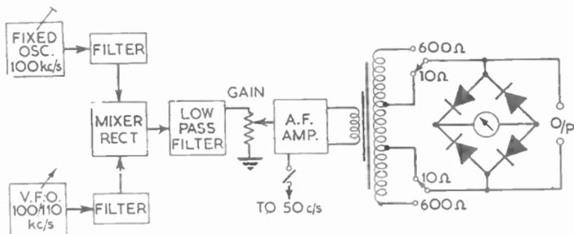
FIG. 18.—BLOCK SCHEMATIC LAYOUT OF A B.F.O.
