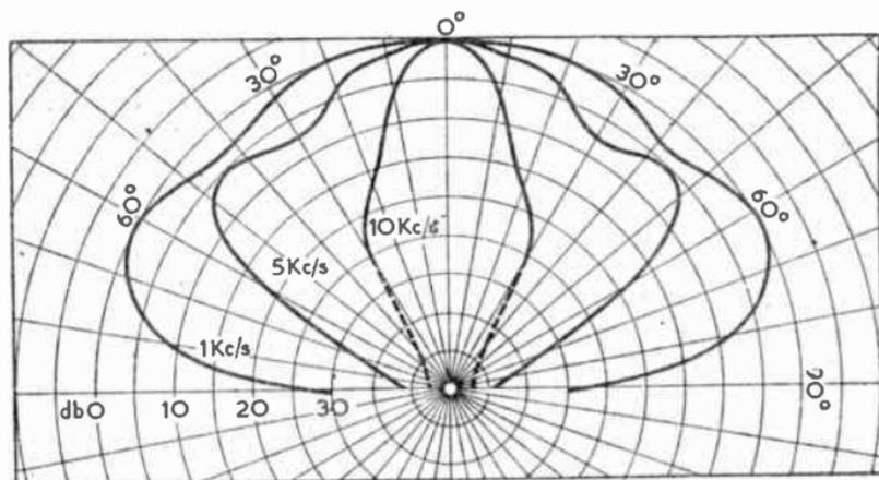
FIG. 14.—TYPICAL LOUDSPEAKER POLAR RESPONSE.
