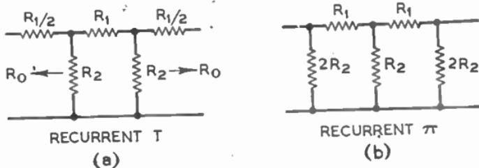
FIG. 41.—RECURRENT ATTENUATOR NETWORKS. (2 SECTIONS).
