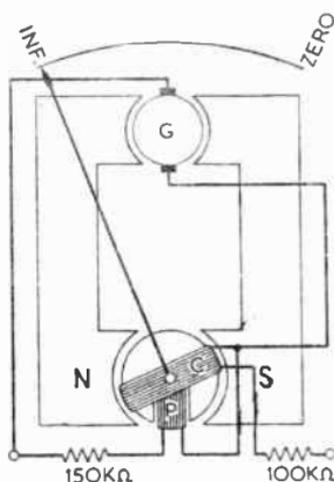
FIG. 14 (right).—"MEGGER" INSULATION TESTER.
