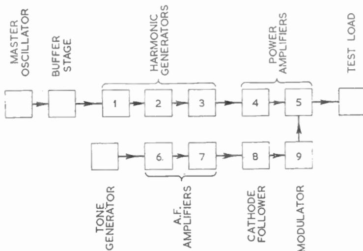
FIG. 4.—ALIGNMENT SEQUENCE FOR AN AMPLITUDE-MODULATED TRANSMITTER.
