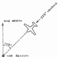
FIG. 4.—V.O.R. INSTRUMENT READINGS FOR AIRCRAFT IN POSITION AND HEADING AS SHOWN (left).
