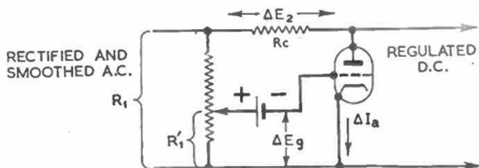
FIG. 111.—THERMIONIC VOLTAGE REGULATOR.
