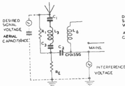
FIG. 10.—AERIAL INPUT CIRCUIT FOR NON-ISOLATED CHASSIS.
