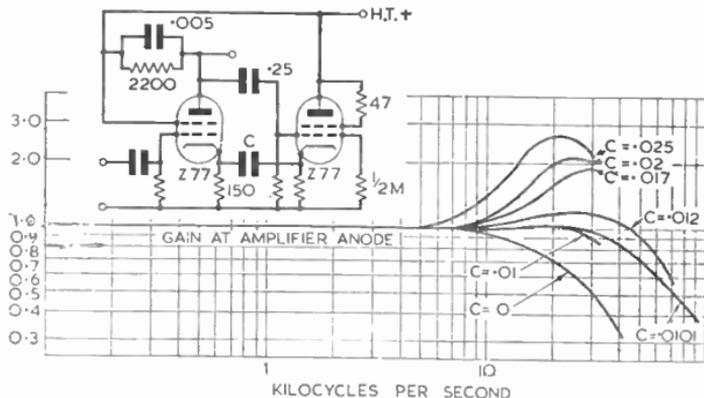
FIG. 27.—EXPERIMENTAL FORM OF "OPTIMAL FEEDBACK" CIRCUIT.
