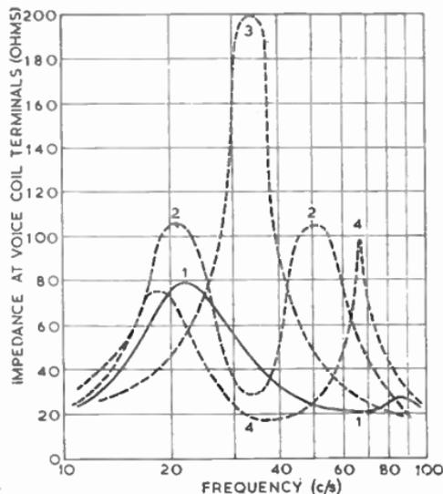
FIG. 19.—COMPARATIVE FREQUENCY/IMPEDANCE CHARACTERISTICS: (1) FRICTION LOADED ENCLOSURE; (2) REFLEX CABINET; (3) INFINITE BAFFLE; (4) AS (1) BUT WITH  $R_f$  OPEN CIRCUIT.
