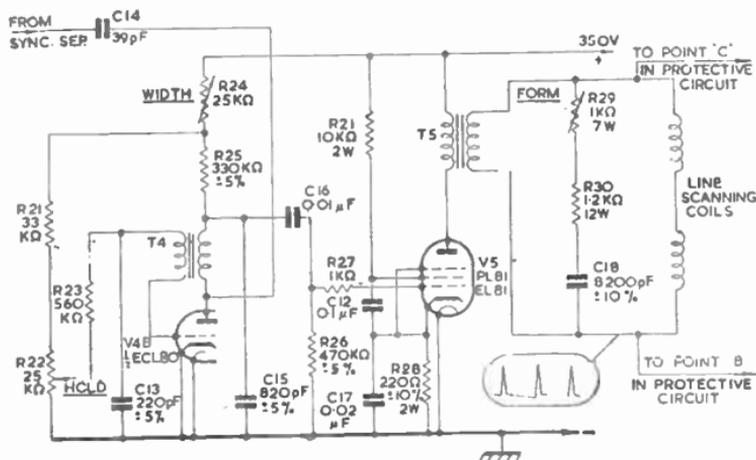
FIG. 8.—LINE TIME-BASE GENERATOR CIRCUIT.
