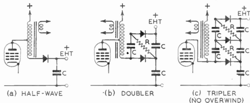
FIG. 23.—HALF-WAVE, DOUBLER, AND TRIPLER PULSE-DRIVEN RECTIFIER MULTIPLIERS.
