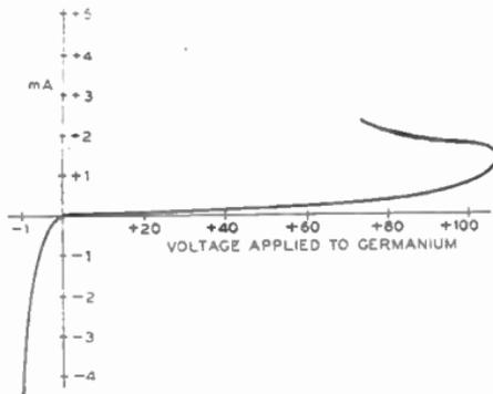
FIG. 2.—VOLTAGE/CURRENT CURVE OF TYPICAL GERMANIUM RECTIFIER.
