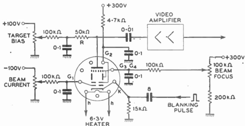
FIG. 10.—THE SUPPLIES NECESSARY TO OPERATE A VIDECON OR STATICON TYPE OF CAMERA TUBE.
