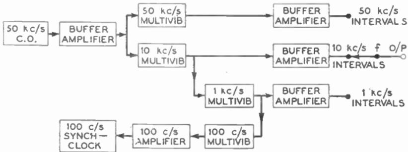
FIG. 35.—BLOCK ARRANGEMENT OF A STANDARD FREQUENCY-METER.
