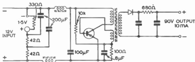
FIG. 23.—LOW POWER CONVERTER.
