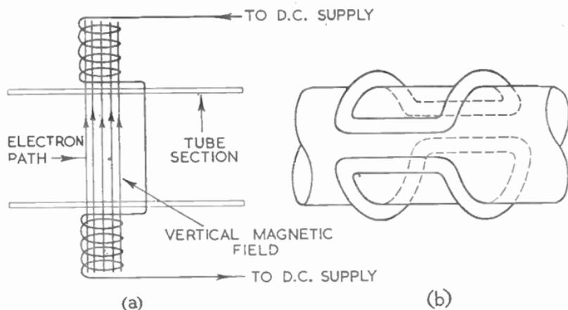
FIG. 18.—THEORETICAL DIAGRAM ILLUSTRATING THE MECHANISM OF MAGNETIC DEFLECTION IS SHOWN IN (a) AND A PRACTICAL FORM FOR SCANNING COILS FOR HORIZONTAL DEFLECTION IS SHOWN IN (b).
