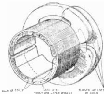
FIG. 20.—TYPICAL YOKE ASSEMBLY CUT IN HALF TO SHOW SECTIONS OF WINDINGS.
