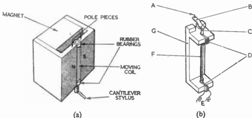
FIG. 17.—CANTILEVER MOVING-COIL PICK-UP.
