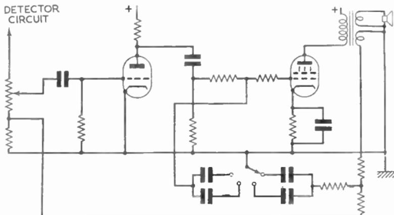
FIG. 25.—TONE CONTROL CIRCUIT PROVIDING TWO POSITIONS OF TREBLE RISE AND TWO OF TREBLE CUT USING A FOUR-WAY ONE-POLE SWITCH (IRRELEVANT PARTS OMITTED).
