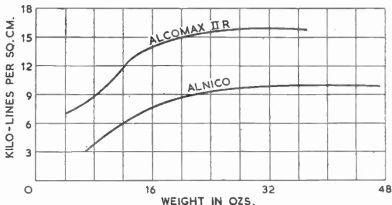
FIG. 5.—FLUX DENSITIES OF TYPICAL MAGNETIC MATERIALS.
