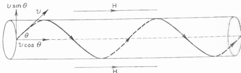
FIG. 13.—PATH TRACED BY AN ELECTRON ENTERING A PARALLEL MAGNETIC FIELD AT AN ANGLE  $\theta$ .
