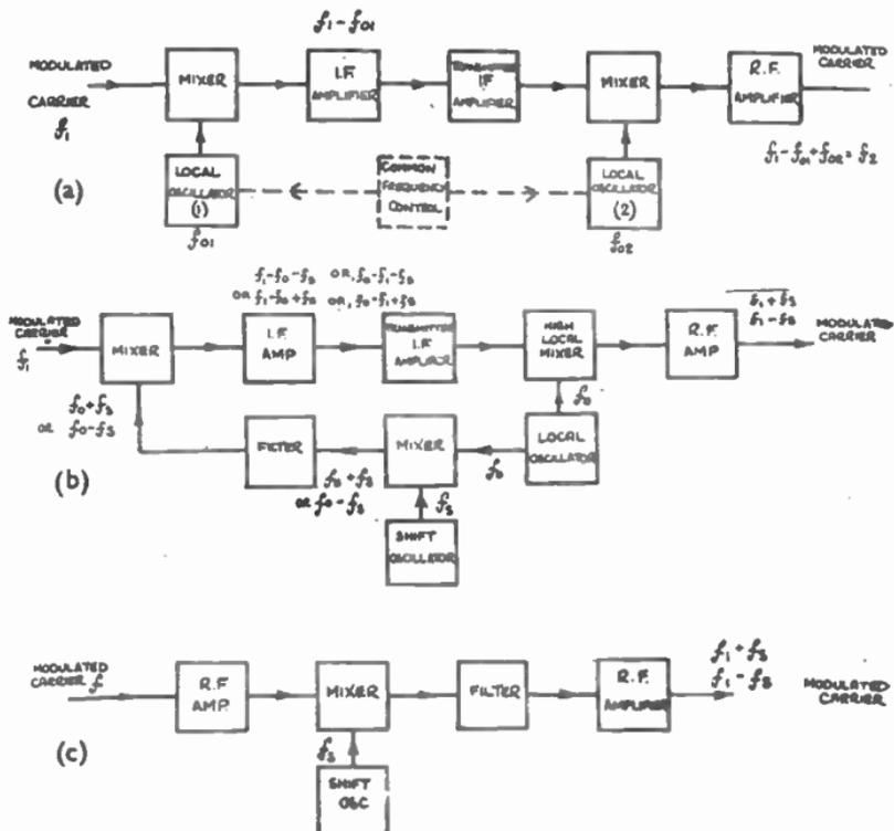
FIG. 5.—TYPICAL NON-DEM. ULATING REPEATERS.
