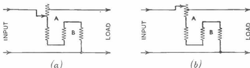
FIG. 12.—SINGLE-PHASE AUTO-TRANSFORMER VOLTAGE REGULATOR.
