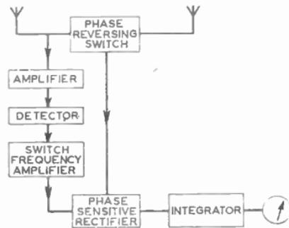
FIG. 18.—THE RYLE PHASE-SWITCHING RECEIVER.
