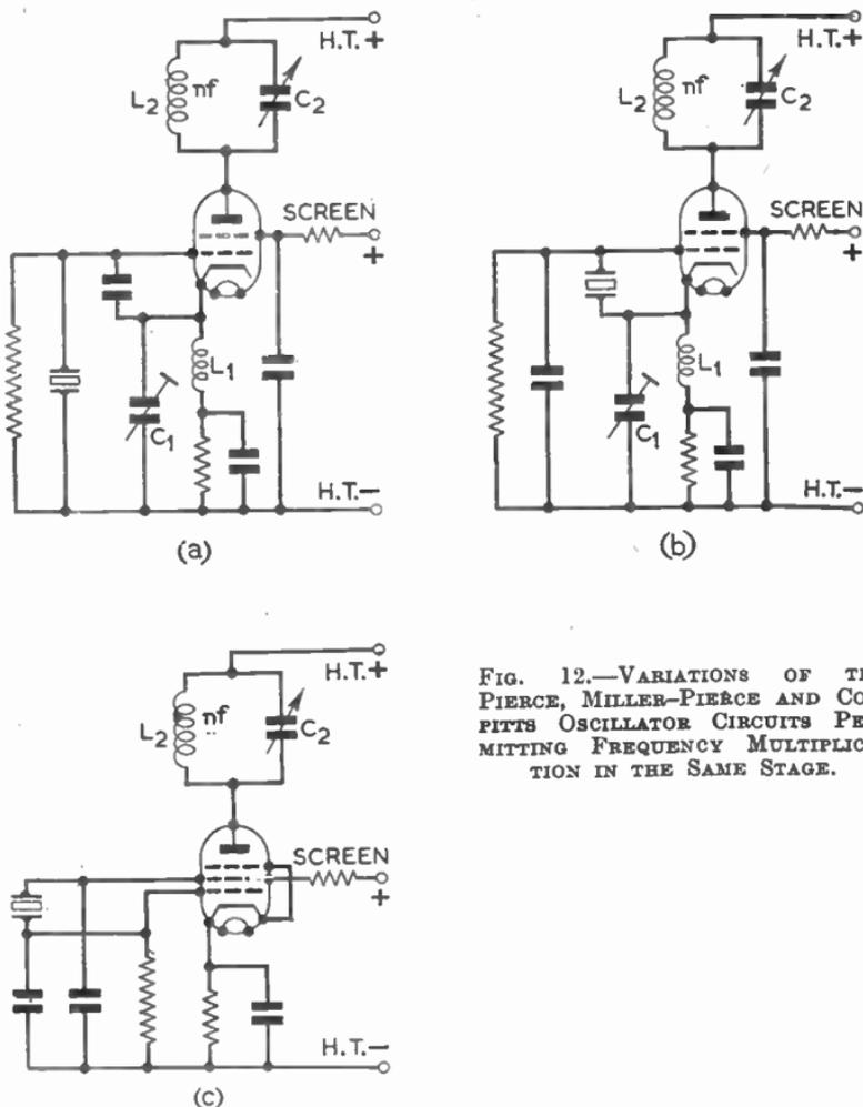
FIG. 12.—VARIATIONS OF THE PIERCE, MILLER-PIERCE AND COLPITTS OSCILLATOR CIRCUITS PERMITTING FREQUENCY MULTIPLICATION IN THE SAME STAGE.
