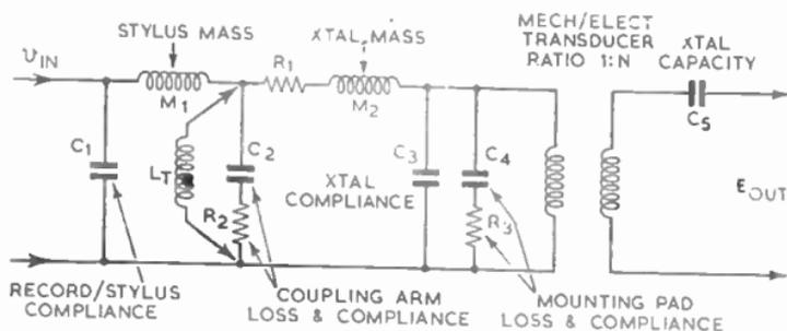
FIG. 14.—SIMPLE ANALOGUE FOR CRYSTAL PICK-UP CARTRIDGE.
