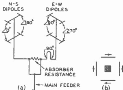
having a characteristic impedance of  $\sqrt{[r_1 \sqrt{(r_1 + r_2)}]}$  and the second of  $\sqrt{[r_2 \sqrt{(r_1 + r_2)}]}$ . Any further correction of susceptance variations is done at selected points on the feeders by introducing, at those points, lengths of line having equal and opposite variations after the manner adopted for the compensation of dipoles.
