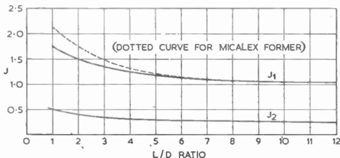
FIG. 16.—ACCEPTOR AND REFLECTOR RESONANCES ON SINGLE LAYER COILS.
