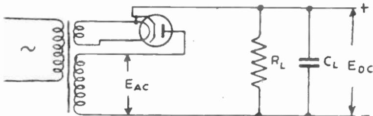
FIG. 8.—HALF-WAVE CIRCUIT RESERVOIR CAPACITOR.
