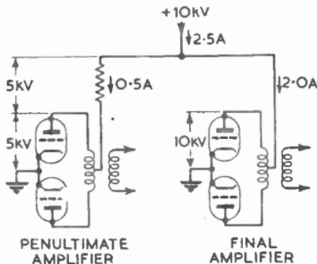
FIG. 27.—POWER AMPLIFIERS FED BY A COMMON RECTIFIER.
