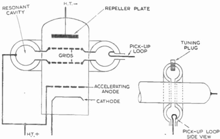
FIG. 24.—REFLEX KLYSTRON.
