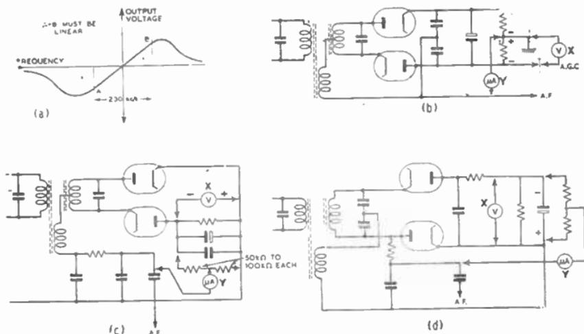
FIG. 15.—ALIGNMENT OF BALANCED AND UNBALANCED RATIO DETECTORS.
