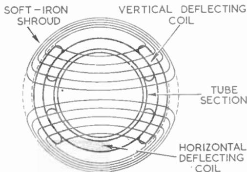
FIG. 19.—CROSS-SECTION OF TUBE FITTED WITH SADDLE COILS, FOR VERTICAL AND HORIZONTAL DEFLECTION, AND A SHROUD. THE FIELD ILLUSTRATED IS DUE TO THE VERTICAL DEFLECTION COILS.
