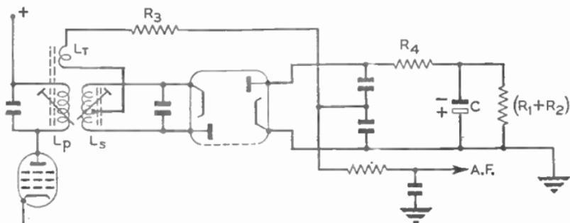
FIG. 38.—PRACTICAL RATIO DETECTOR, UNBALANCED CIRCUIT.
