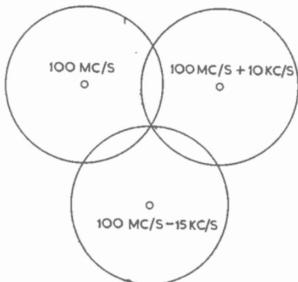
FIG. 34.—DIVERSITY SYSTEM FOR LARGE AREA COVERAGE.
