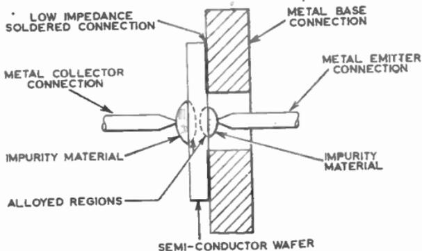
FIG. 4. TYPICAL ALLOYED JUNCTION TRANSISTOR.
