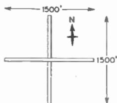
FIG. 20.—PLAN OF 85 Mc/s "MILLS CROSS". EACH ARM CONSISTS OF 250 PAIRS OF DIPOLES ALIGNED EAST-WEST ABOVE A REFLECTOR.
