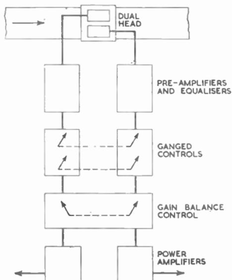
FIG. 24.—BLOCK DIAGRAM OF A "STEREOSONIC" REPRODUCER.
