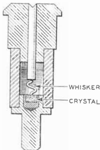
FIG. 5.—CONSTRUCTION OF TYPICAL SILICON DETECTOR.
