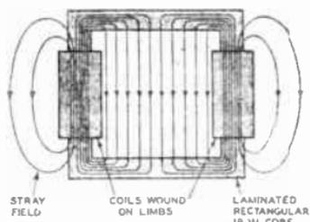
FIG. 14.—RECTANGULAR IRON-CORE COIL PRODUCING UNIFORM DEFLECTING FIELD.
