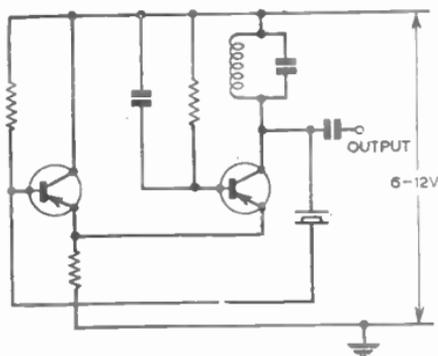
FIG. 9—TWO TRANSISTOR CRYSTAL OSCILLATOR.
