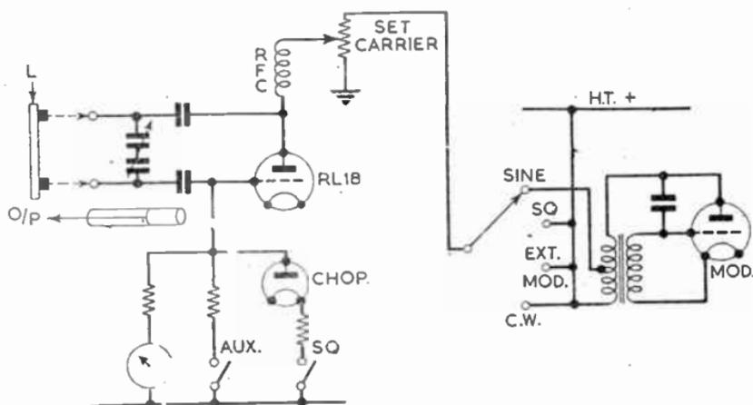
FIG. 21.—V.H.F. SIGNAL GENERATOR.
