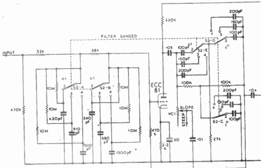
FIG. 21.—SWITCHED LOW-PASS FILTER CIRCUIT USING "PARALLEL T" NETWORK.
