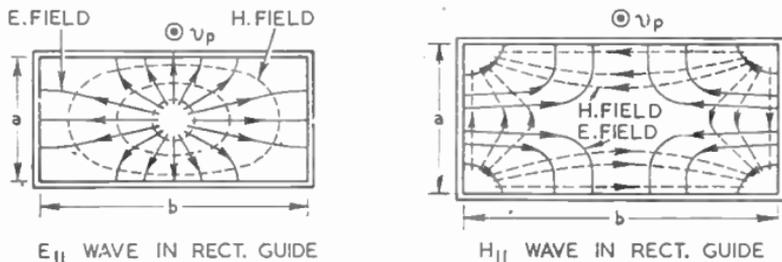
FIG. 18.—E<sub>11</sub> AND H<sub>11</sub> WAVES IN A RECTANGULAR GUIDE.
