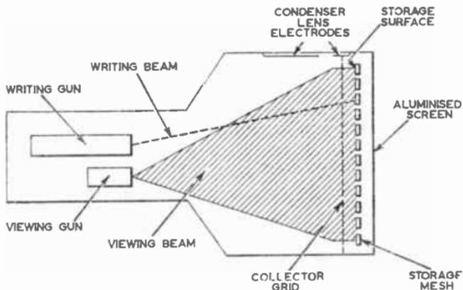
FIG. 24.—DIRECT-VIEWING STORAGE TUBE.
