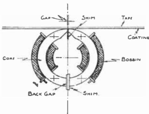
FIG. 2.—TYPICAL HEAD ASSEMBLY.
