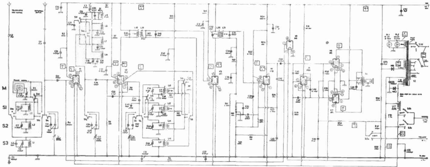
FIG. 20.—PORTABLE A.C. MAINS BATTERY RECEIVER FOR MEDIUM AND SHORT WAVES, WITH R.F. AMPLIFIER.
