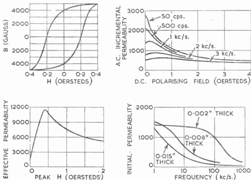
FIG. 1.—TYPICAL CHARACTERISTICS OF MAGNETIC LAMINATIONS.
