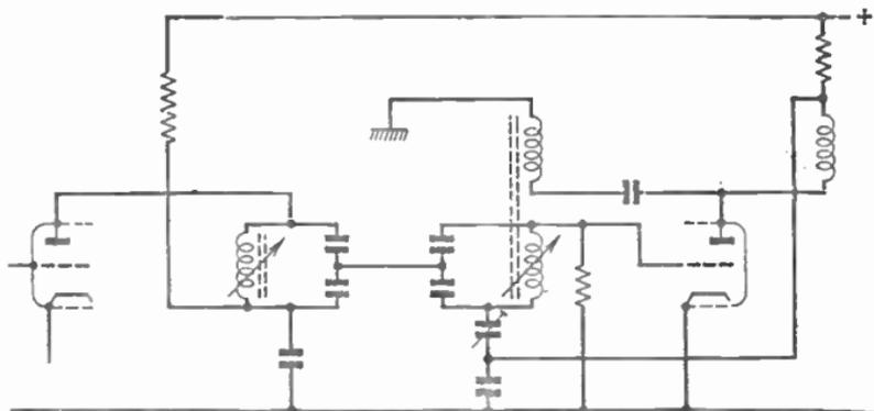
FIG. 32 (above).—R.F. AMPLIFIER AND MIXER, USING DOUBLE TRIODE AND PERMEABILITY TUNER.
