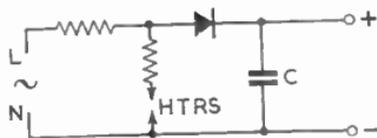
FIG. 20.—A.C./D.C. RADIO RECEIVER RECTIFIER CIRCUIT (SEE TABLE 3).
