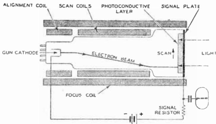
FIG. 27.—THE BASIC PRINCIPLE OF THE PHOTO-CONDUCTIVE TUBE.
