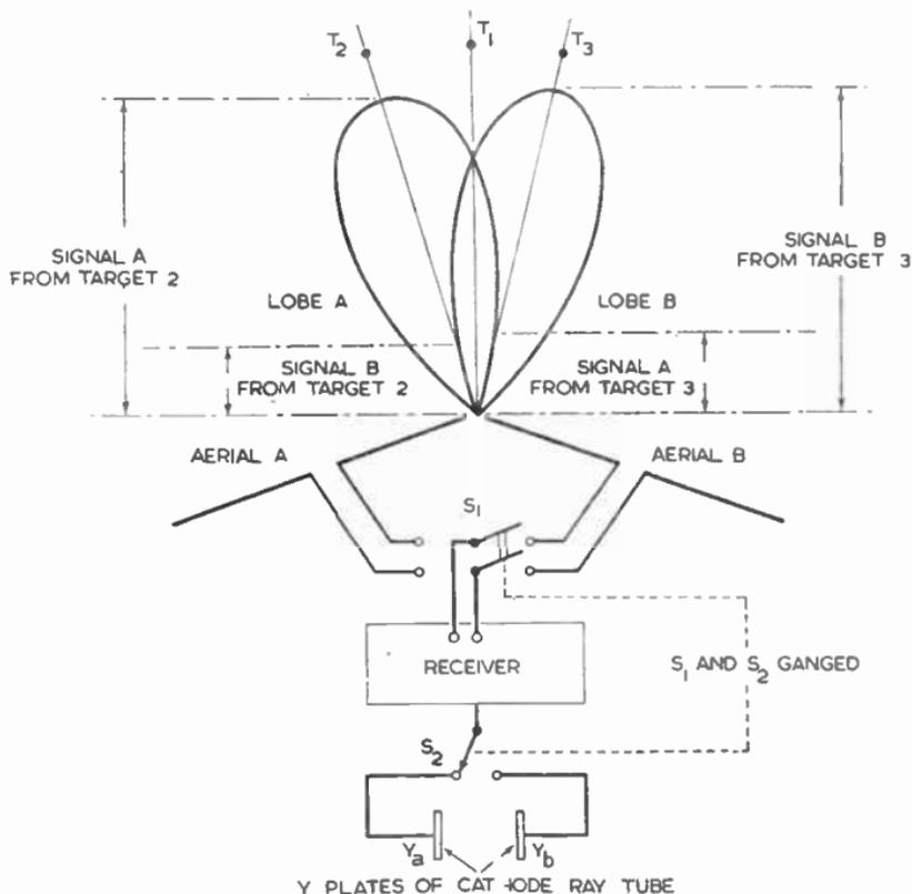
FIG. 28.—BEAM SWITCHING.
