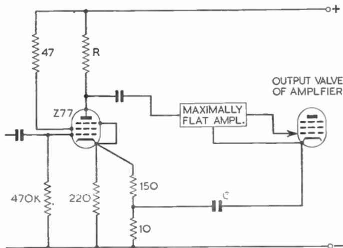
FIG. 32.—ALTERNATIVE ARRANGEMENT FOR SUPPLYING OVERALL OPTIMAL FEEDBACK.
