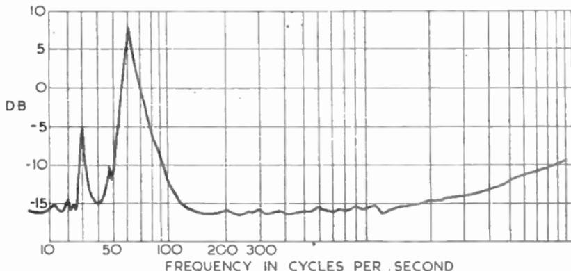
FIG. 3.—ELIMINATION OF CABINET BOOM—I.
