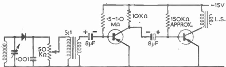
FIG. 31.—CRYSTAL DETECTOR FOLLOWED BY A TWO-STAGE TRANSISTOR AUDIO-FREQUENCY AMPLIFIER.
