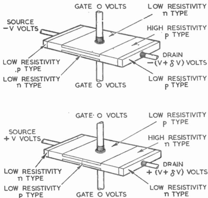
FIG. 16.—DIAGRAMMATIC CONSTRUCTION OF UNIPOLAR TRANSISTORS.
