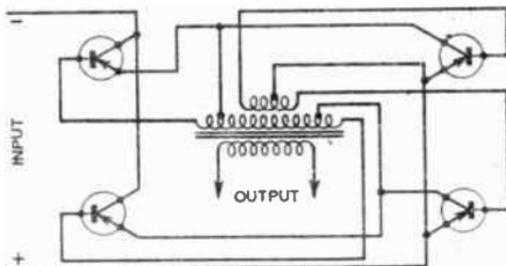
FIG. 22.—POLARITY CHANGER D.C. CONVERTER.
