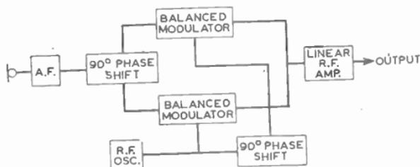
FIG. 7.—BLOCK DIAGRAM OF S.S.B. GENERATOR USING PHASING SYSTEM.
