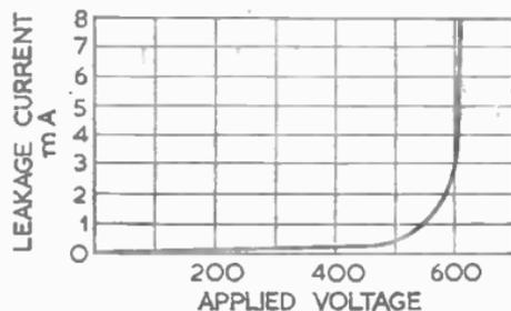
FIG. 7.—TYPICAL LEAKAGE CURRENT-VOLTAGE CURVE FOR CAPACITOR RATED AT 500 VOLTS D.C. WORKING 600 VOLTS SURGE.
