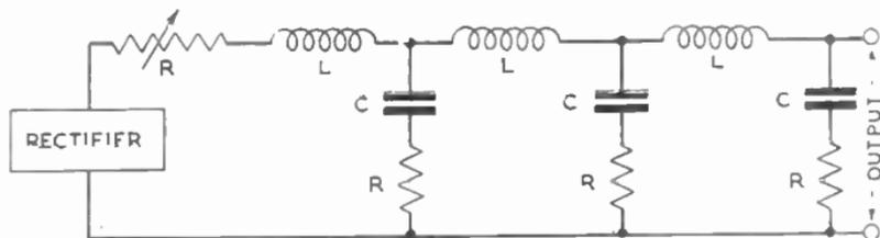
FIG. 45.—“ BUILT-OUT ” FILTER.
