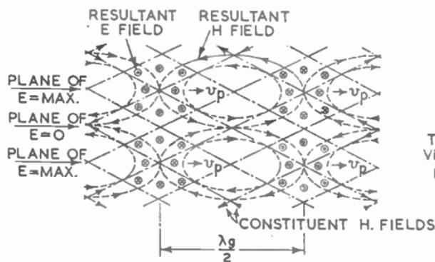
SYNTHESIZED H WAVE (OR T.E. WAVE) TRAVELLING WITH VELOCITY  $v_p$  FROM LEFT TO RIGHT
