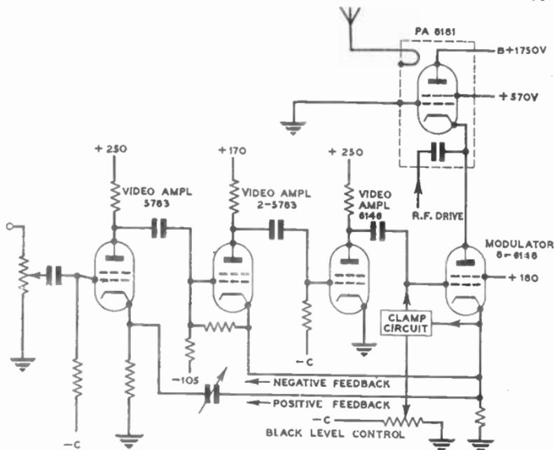
FIG. 6 (b).—MODULATOR ARRANGEMENT FOR CATHODE-MODULATED 1-kW TRANSMITTER.
