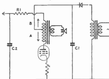
FIG. 22.—HUM CANCELLATION WINDING ON OUTPUT TRANSFORMER.
