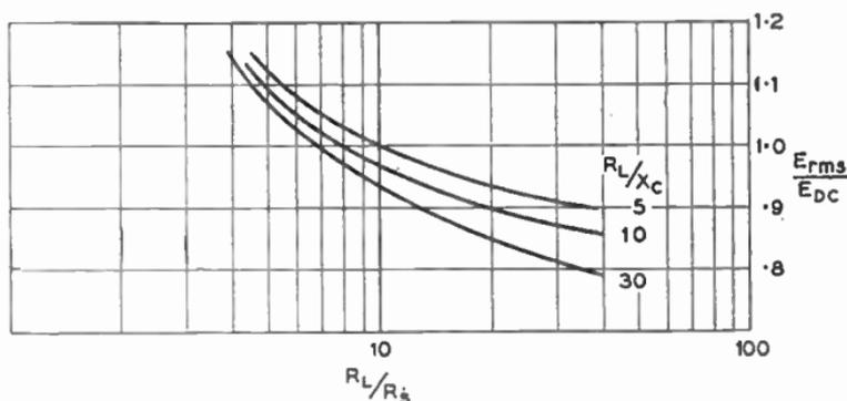
FIG. 15.— $E_{rms}/E_{DC}$  AS A FUNCTION OF  $R_L/R_s$  AND  $R_L/R_B$  FOR THE FULL-WAVE RECTIFIER CIRCUIT.
