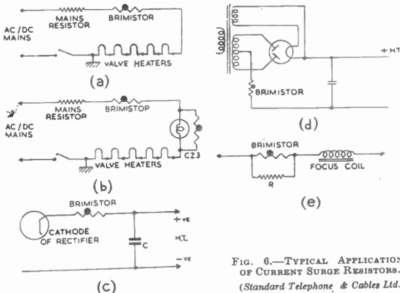
FIG. 6.—TYPICAL APPLICATIONS OF CURRENT SURGE RESISTORS.
