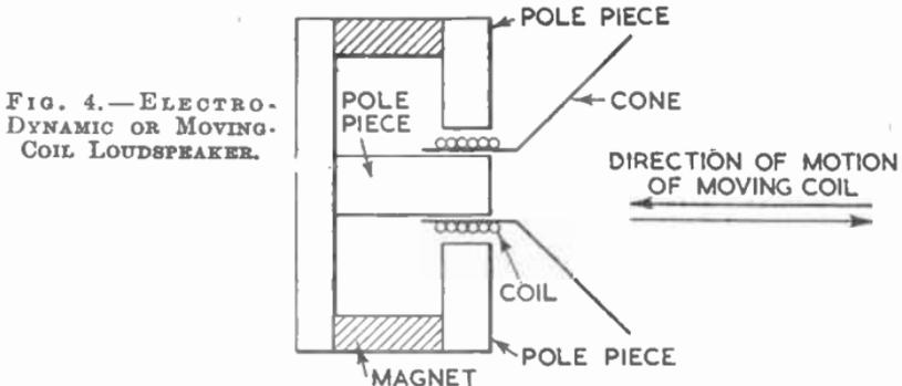
FIG. 4.—ELECTRO-DYNAMIC OR MOVING-COIL LOUDSPEAKER.
