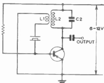
FIG. 8.—TRANSISTOR CRYSTAL OSCILLATOR.
