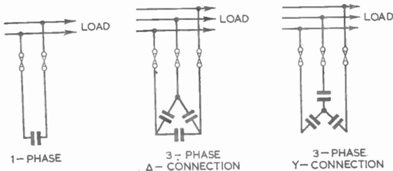
FIG. 104.—CAPACITORS FOR POWER FACTOR CORRECTION.
