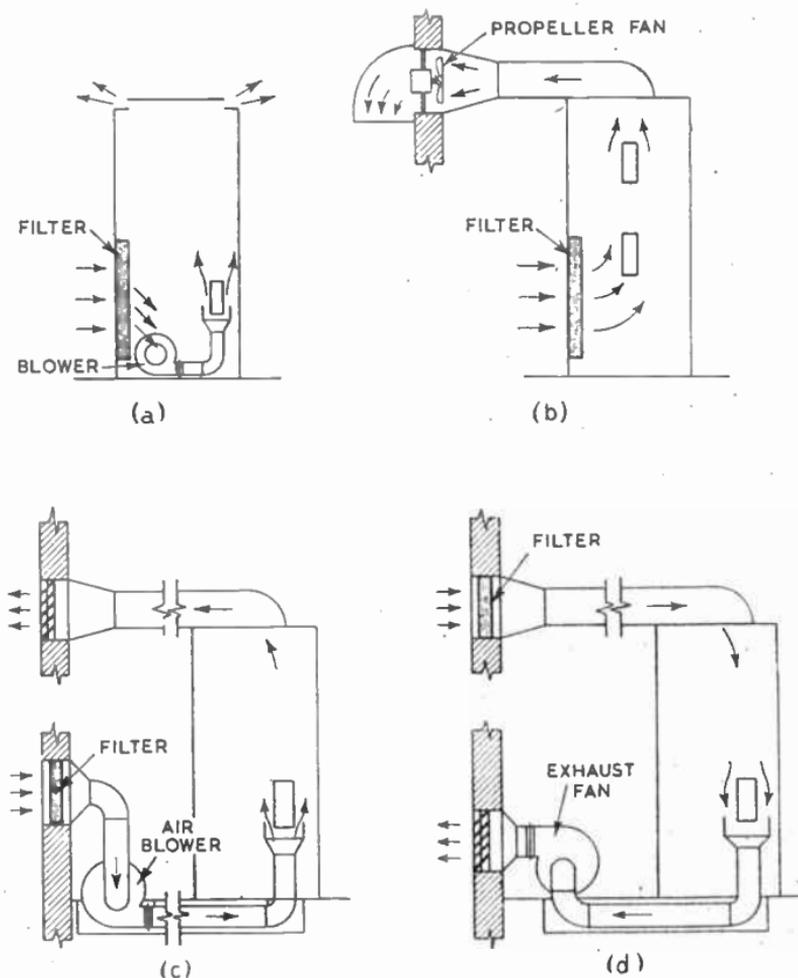
FIG. 20.—FORCED-AIR COOLING SYSTEMS.
