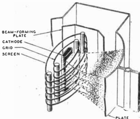
FIG. 9.—BEAM TETRODE VALVE.
