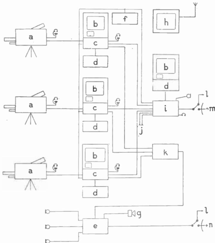
FIG. 21.—FACILITIES DIAGRAM FOR MOBILE TELEVISION CONTROL ROOM.
