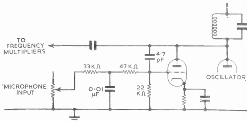
FIG. 22.—PHASE MODULATOR USING REACTANCE VALVE.
