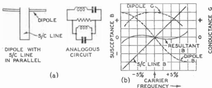
FIG. 21.—BAND-WIDTH OF DIPOLE WITH SHORT-CIRCUIED LINE IN PARALLEL.
