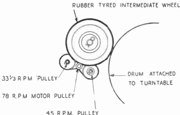
FIG. 2.—THREE-SPEED DRIVE USING BELTS.
