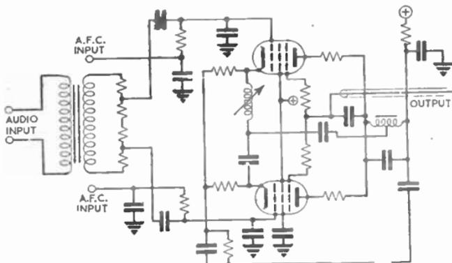
FIG. 39.—MODERN VERSION OF REACTANCE-CONTROLLED OSCILLATOR CAPABLE OF WIDE DEVIATION WITH LOW DISTORTION.
