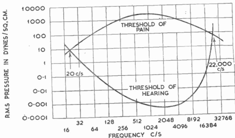
FIG. 42.—THRESHOLD CURVES.
