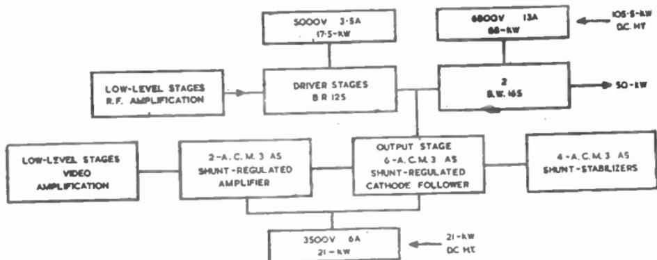
FIG. 4.—SCHEME FOR 50-KW HIGH-LEVEL MODULATED TRANSMITTER.
