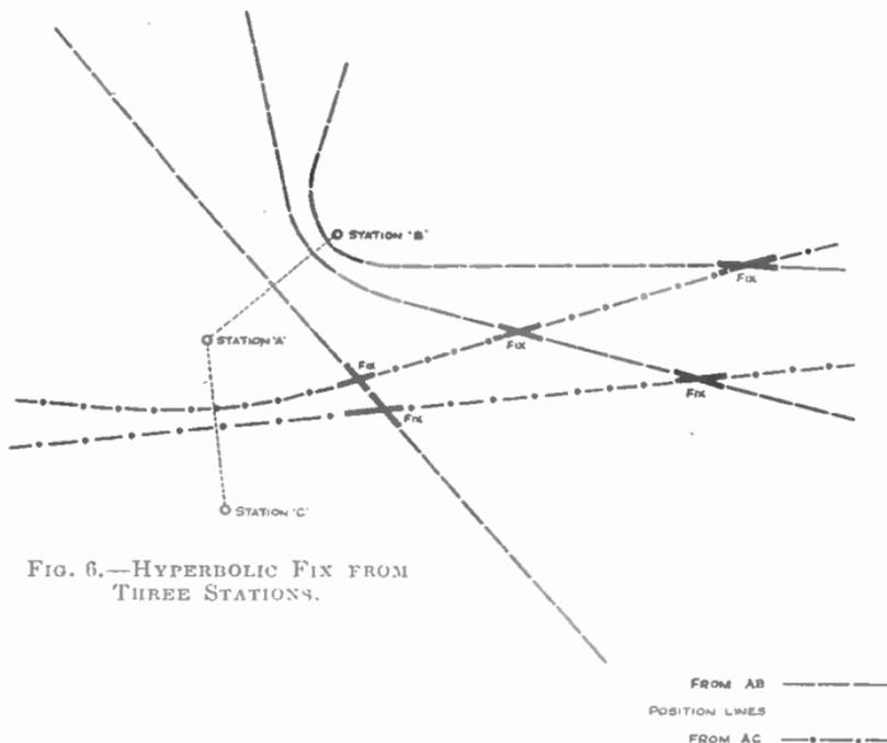
FIG. 6.—HYPERBOLIC FIX FROM THREE STATIONS.
