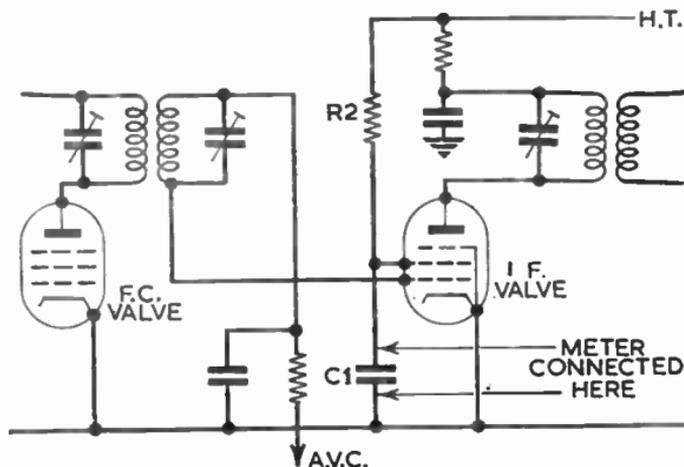
FIG. 13.—INTERMEDIATE-FREQUENCY STAGE OF A BATTERY-OPERATED RECEIVER.
