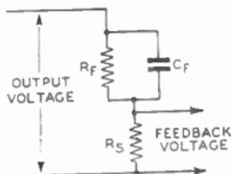
FIG. 21.—FEEDBACK NETWORK WITH CAPACITANCE.
