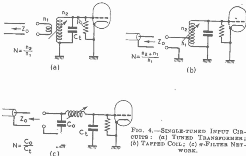
FIG. 4.—SINGLE-TUNED INPUT CIRCUITS: (a) TUNED TRANSFORMER; (b) TAPPED COIL; (c)  $\pi$ -FILTER NETWORK.
