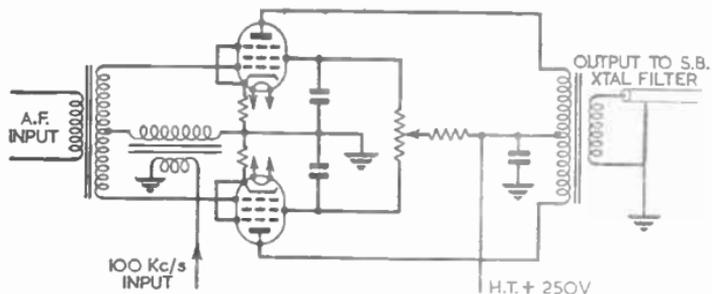
FIG. 19.—SIMPLIFIED CIRCUIT OF TYPICAL BALANCED MODULATOR.
