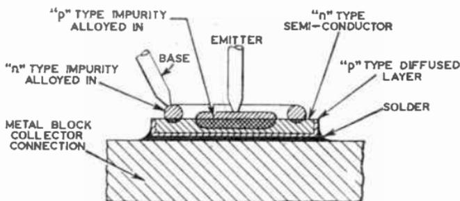
FIG. 8.—POWER JUNCTION TRANSISTOR.
