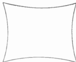
FIG. 15.—PIN-CUSHION DISTORTION INTRODUCED BY FLAT-FACED SCREEN, USING UNIFORM DEFLECTING FIELD.
