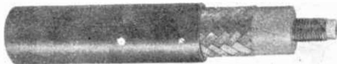
FIG. 4.—A HELICALLY WOUND DELAY CABLE.
