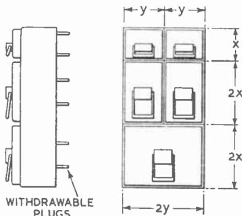
FIG. 18.—ARRANGEMENT OF UNITS IN UNIT ASSEMBLY SWITCHBOARD.
