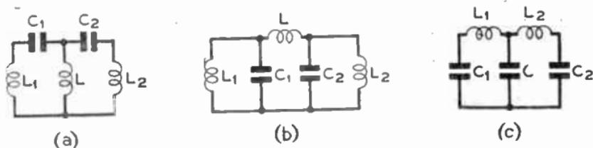
FIG. 35.—INDUCTANCE OF COUPLED CIRCUITS.
