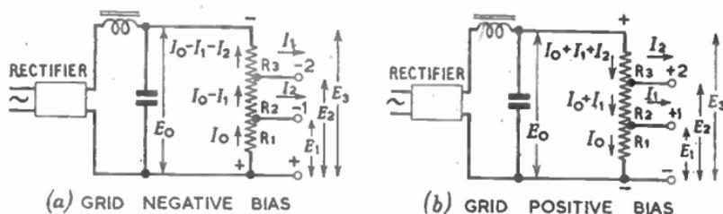
FIG. 31.—GRID-BIAS RECTIFIER WITH VOLTAGE DIVIDER.
