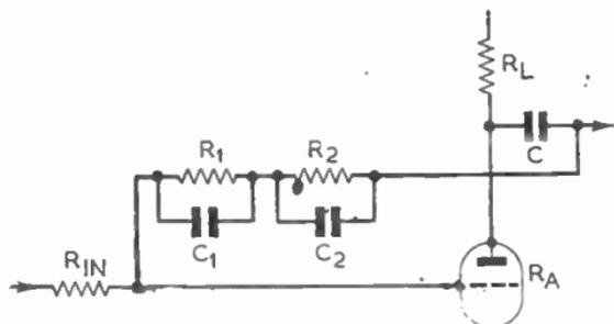
FIG. 17.—FEEDBACK EQUALIZER.
