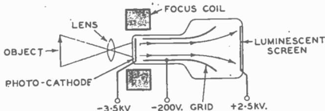
FIG. 13.—FUNCTIONAL DIAGRAM OF AN IMAGE CONVERTER.
