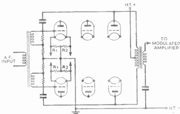
FIG. 22 —ONE METHOD OF APPLYING NEGATIVE FEEDBACK TO A MODULATOR.
