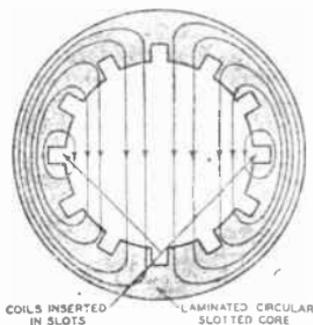
FIG. 17.—SLOTTED IRON-CORE DEFLECTING COIL.
