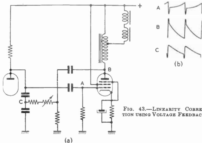
FIG. 43.—LINEARITY CORRECTION USING VOLTAGE FEEDBACK.
