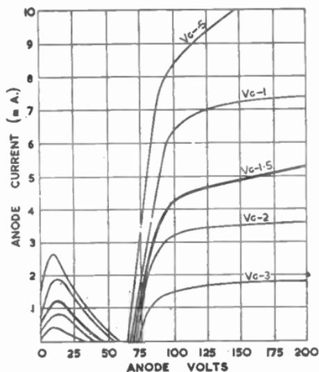
FIG. 8.—CHARACTERISTIC CURVE OF TYPICAL SCREEN-GRID VALVE.
