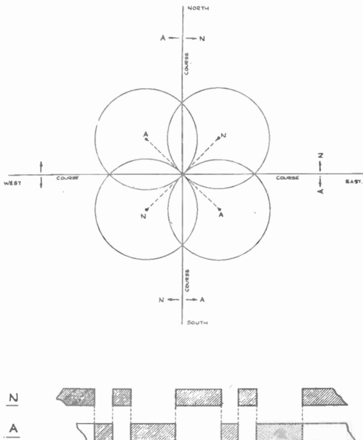
FIG. 1.—MEDIUM-FREQUENCY FOUR-COURSE RANGE: POLAR DIAGRAM AND INTERLOCKING MORSE CHARACTERS.
