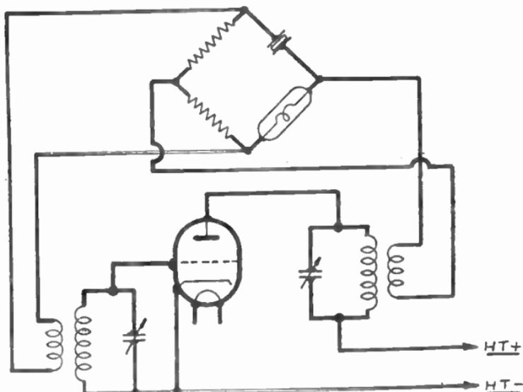
FIG. 13.—MEACHAM BRIDGE CRYSTAL OSCILLATOR.
