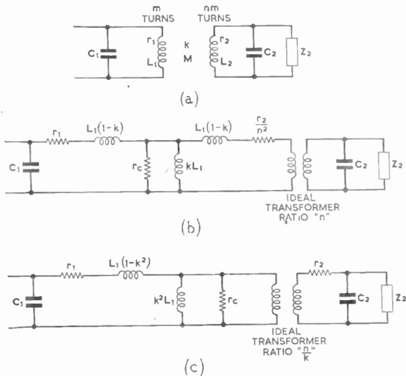
FIG. 3.—NETWORK APPROXIMATIONS TO THE PRACTICAL TRANSFORMER.
