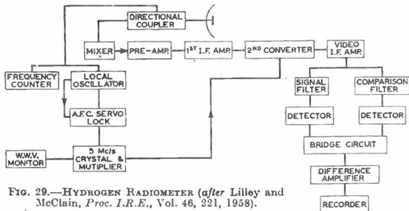
FIG. 29.—HYDROGEN RADIOMETER (after Lilley and McClain, *Proc. I.R.E.*, Vol. 46, 221, 1958).
