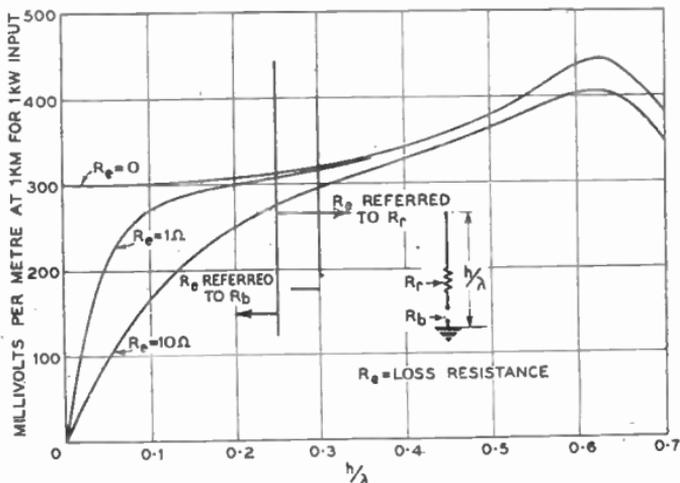
FIG. 7.—FIELD STRENGTH OF VERTICAL AERIALS.
