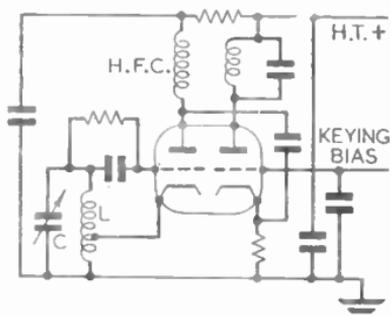
FIG. 6.—TWIN-VALVE KEYED E.C.O.
