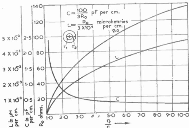
FIG. 13.—C-R CENTRIC FEEDER DATA.
