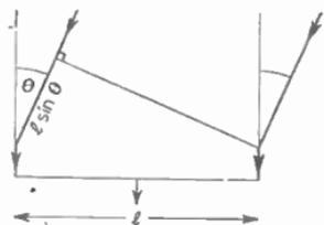
FIG. 16.—SPACED AERIALS INTERFEROMETER.
