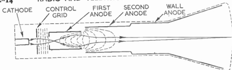
FIG. 8.—ELECTROSTATIC FOCUSING SYSTEM OF A CATHODE-RAY TUBE.
