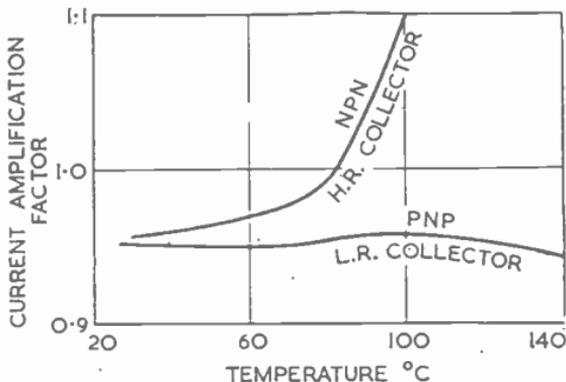
FIG. 11.—TYPICAL VARIATION OF CURRENT AMPLIFICATION FACTOR FOR JUNCTION TYPE TRANSISTORS.
