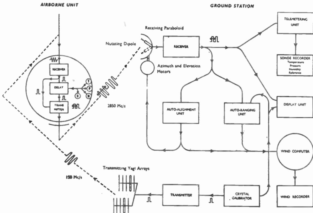
FIG. 48.—SCHEMATIC DIAGRAM OF COMPLETE RADAR WIND AND RADAR SONDE THEODOLITE.
