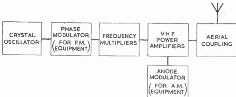
FIG. 1.—BLOCK DIAGRAM OF A V.H.F. TRANSMITTER.
