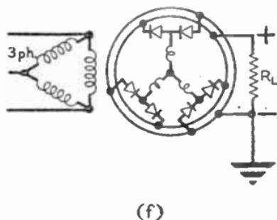
FIG. 106.--(a) SINGLE-PHASE, FULL WAVE; (b) SINGLE-PHASE, FULL-WAVE BRIDGE; (c) THREE-PHASE, HALF WAVE; (d) THREE-PHASE, HALF-WAVE INTERCONNECTED STAR; (e) THREE-PHASE, FULL-WAVE DOUBLE Y; (f) THREE-PHASE, FULL-WAVE SINGLE Y.
