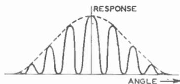
FIG. 15.—THE DIRECTIVITY OF A TWIN-AERIAL INTERFEROMETER.
