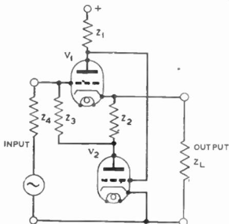
FIG. 43.—DOUBLE-SHUNT-REGULATED CATHODE FOLLOWER.
