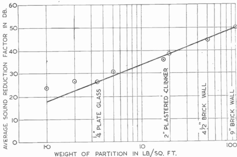
FIG. 2.—AVERAGE TRANSMISSION LOSSES OF BUILDING MATERIALS.
