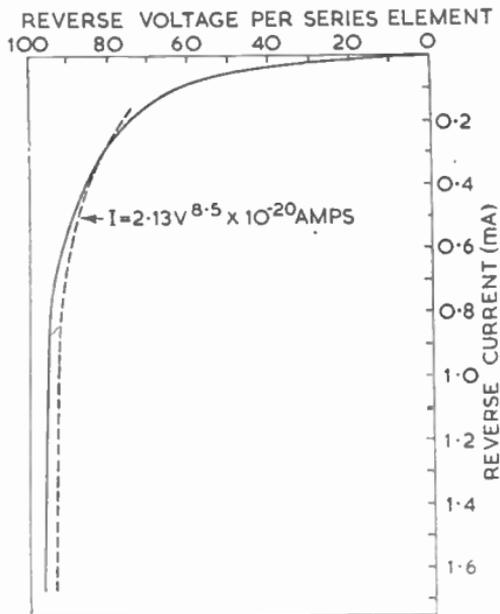
FIG. 27.—REVERSE CHARACTERISTIC OF A SINGLE QUADRUPLE-VOLTAGE (36EHT) DISC, ILLUSTRATING THE SHARP TURNOVER.
