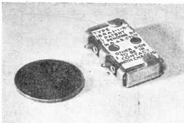
FIG. 28.—CONDUCTION COOLED RECTIFIER. OUTPUT 140 VOLTS, 60 mA.
