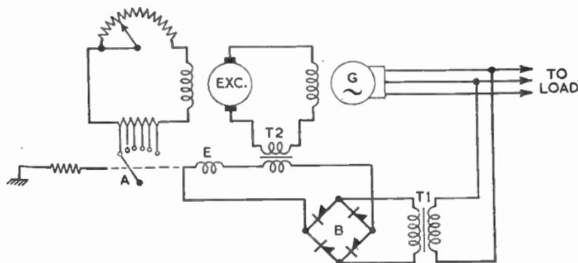
FIG. 16.—AUTOMATIC RHEOSTATIC VOLTAGE REGULATOR FOR CONTROL OF ALTERNATOR.
