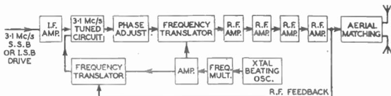
FIG. 22.—BLOCK SCHEMATIC DIAGRAM OF 4-KW TRANSMITTER USING RADIO-FREQUENCY NEGATIVE FEEDBACK.
