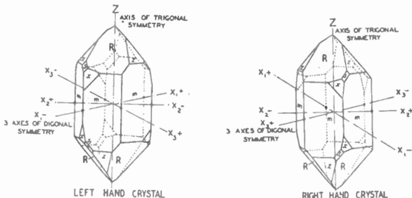
FIG. 1.—THE FORM OF QUARTZ CRYSTALS.
