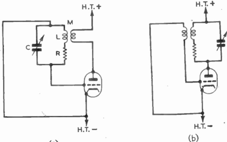
(a) FIG. 70.—VALVE OSCILLATORS.
