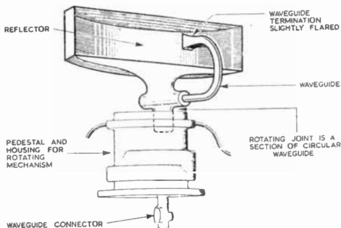
FIG. 29.—PARABOLIC REFLECTOR AERIAL.
