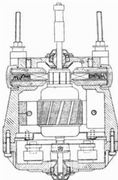
FIG. 6 (right).—SECTIONAL VIEW OF A UNIVERSAL MOTOR FOR USE WITH GRAMOPHONE UNITS.
