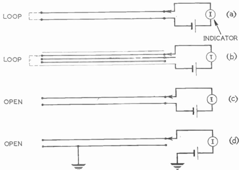
FIG. 1.—WIRING TESTS FOR CONTINUITY, SHORT-CIRCUIT, EARTH AND LOW INSULATION RESISTANCE.
