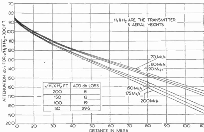
FIG. 8.—V.H.F. PROPAGATION LOSSES BETWEEN HALF-WAVE DIPOLES.
