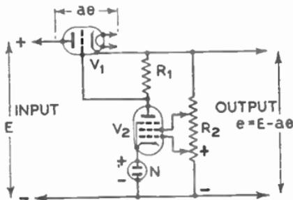
FIG. 14.—D.C. THERMIONIC VOLTAGE STABILIZER.
