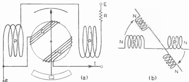
FIG. 12.—DYNAMOMETER TYPE WATTMETER.
