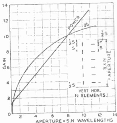
FIG. 20.—GAIN OF STACKED RADIATORS.
