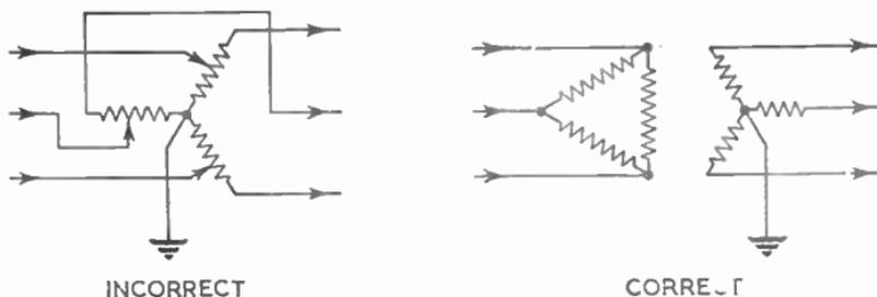
FIG. 9.—THREE-PHASE AUTO-TRANSFORMER—THREE-WIRE SUPPLY, NEUTRAL REQUIRED.
