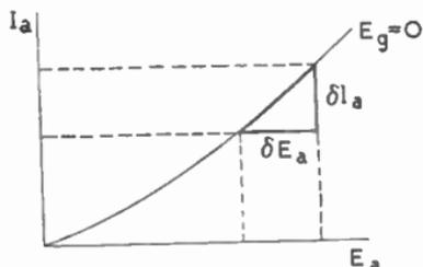
FIG. 134.—DETERMINATION OF VALVE CONSTANTS.
