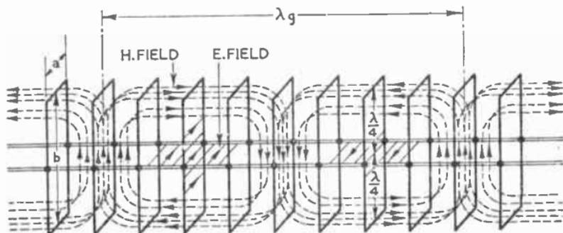
FIG. 7.—MAGNETIC AND ELECTRIC FIELD DISTRIBUTION ALONG AN OPEN-WIRE TRANSMISSION LINE ENCLOSED BY  $\lambda/4$  STUBS ABOVE AND BELOW THE LINE. STANDING WAVE CONDITION.
