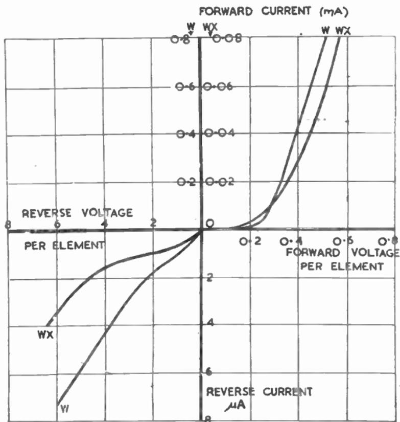
FIG. 29.—D.C. CHARACTERISTICS OF WESTECTORS TYPES W1 AND WX1 (i.e., FOR ONE SERIES ELEMENT ONLY).
