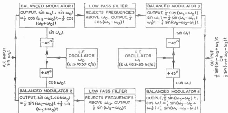
FIG. 25.—BLOCK DIAGRAM OF PORTABLE S.S.B. GENERATOR.
