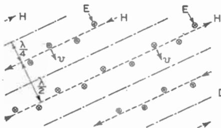
PLANE WAVE TRAVELLING WITH VELOCITY  $v$  DIAGONALLY DOWNWARDS
