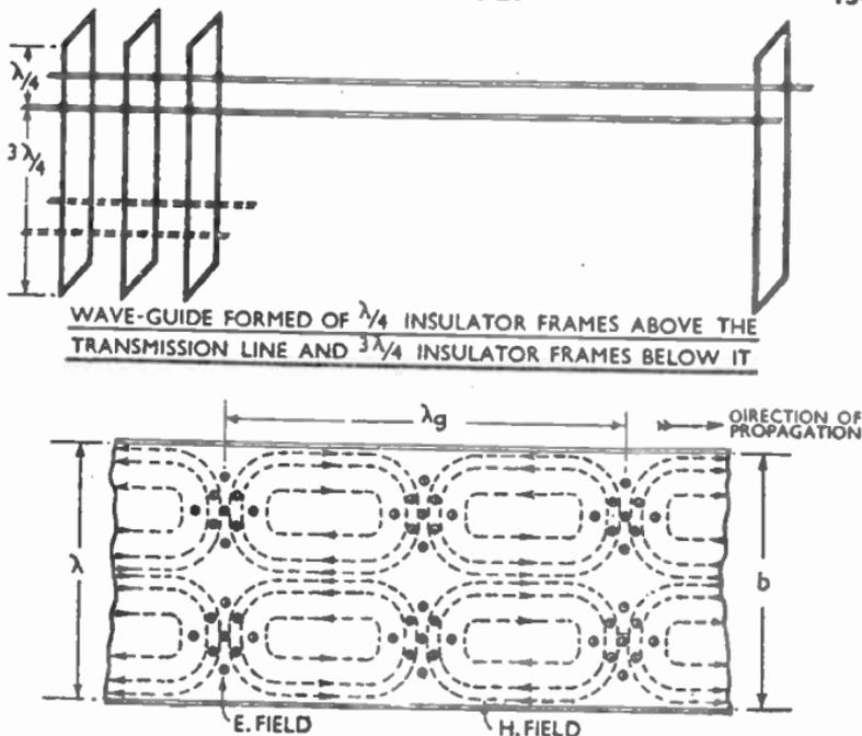
FIG. 8.—ELECTROMAGNETIC WAVE IN A RECTANGULAR GUIDE WHEN  $b > \lambda$ .
