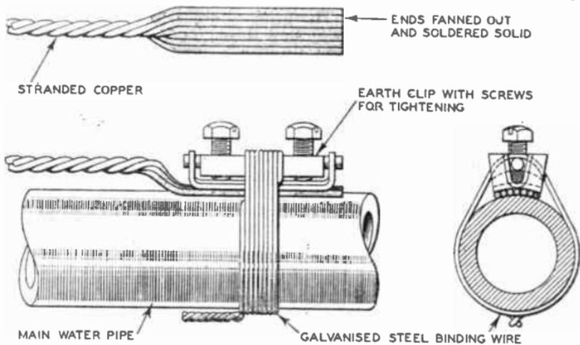
FIG. 18.—METHOD OF BONDING EARTH WIRE TO MAIN WATER PIPE.
