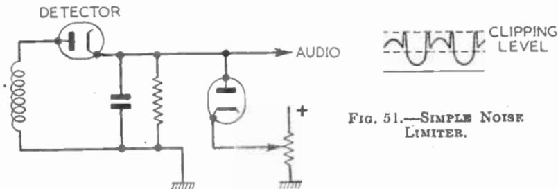
FIG. 51.—SIMPLE NOISE LIMITER.
