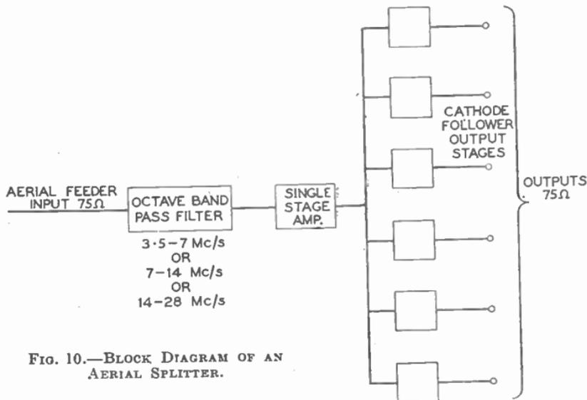
FIG. 10.—BLOCK DIAGRAM OF AN AERIAL SPLITTER.
