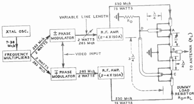
FIG. 7.—PHASE-TO-AMPLITUDE MODULATION SYSTEM USED AT U.H.F.
