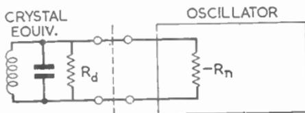
FIG. 19.—DIAGRAMMATIC REPRESENTATION OF A PARALLEL MODE CRYSTAL OSCILLATOR.
