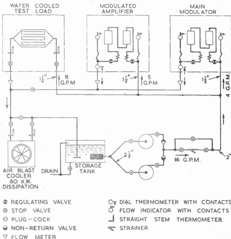
FIG. 24.—SCHEMATIC ARRANGEMENT OF VALVE WATER-COOLING SYSTEM.
