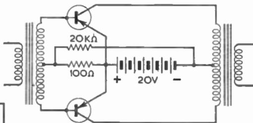
FIG. 33 (left).—COMMON COLLECTOR CLASS B OUTPUT CIRCUIT.
