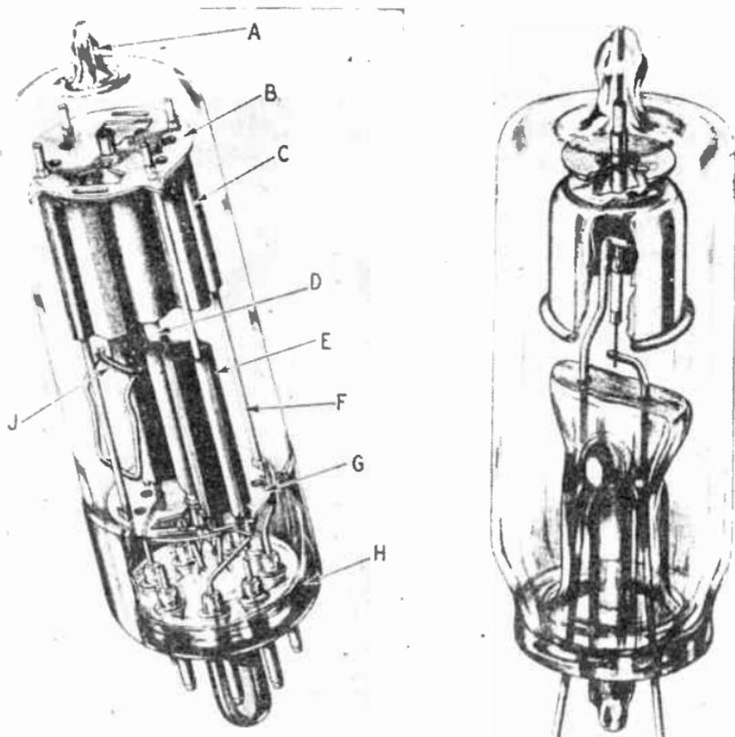
FIG. 4 (left).—CONSTRUCTIONAL DETAILS OF THE MAZDA UU9.
