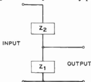
FIG. 33 (above).—DIVIDER NETWORK, FIRST STAGE.
