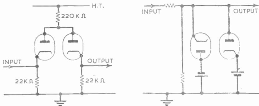
FIG. 19.—CLIPPING CIRCUITS.
