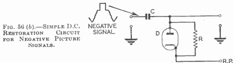
FIG. 56 (b).—SIMPLE D.C. RESTORATION CIRCUIT FOR NEGATIVE PICTURE SIGNALS.
