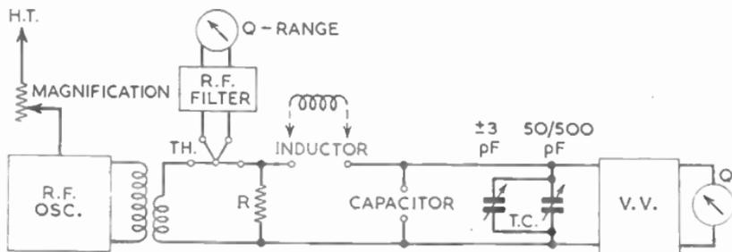
FIG. 26.—BLOCK LAYOUT DIAGRAM OF TYPICAL Q-METER.
