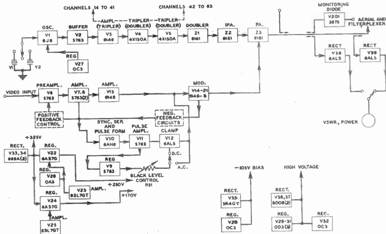
FIG. 6 (a).—SCHEMATIC DIAGRAM OF A CATHODE-MODULATED 1-kW U.H.F. TRANSMITTER.
