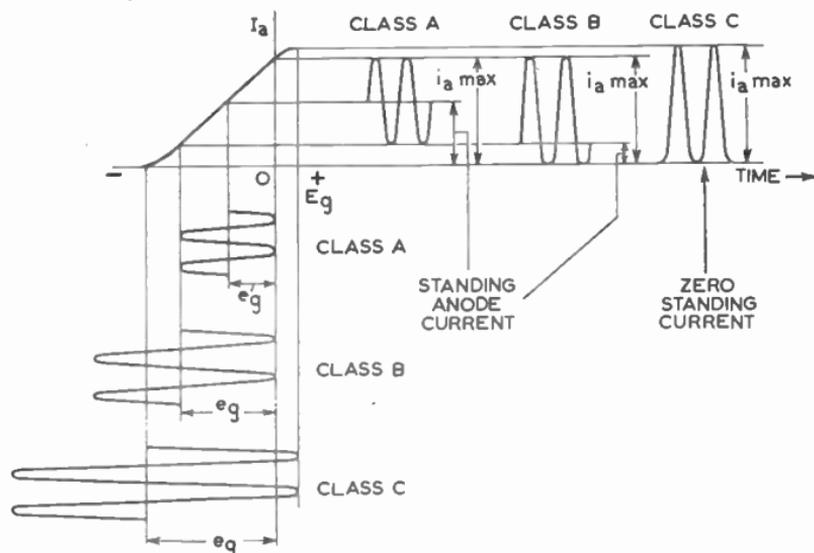
FIG. 56.—CLASS A, B, AND C AMPLIFICATION.
