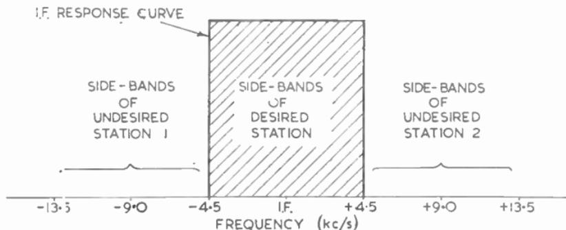
FIG. 6.—IDEAL INTERMEDIATE-FREQUENCY RESPONSE.
