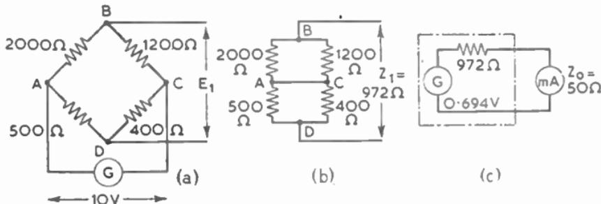
FIG. 19.—SOLUTION OF EXAMPLE 3.
