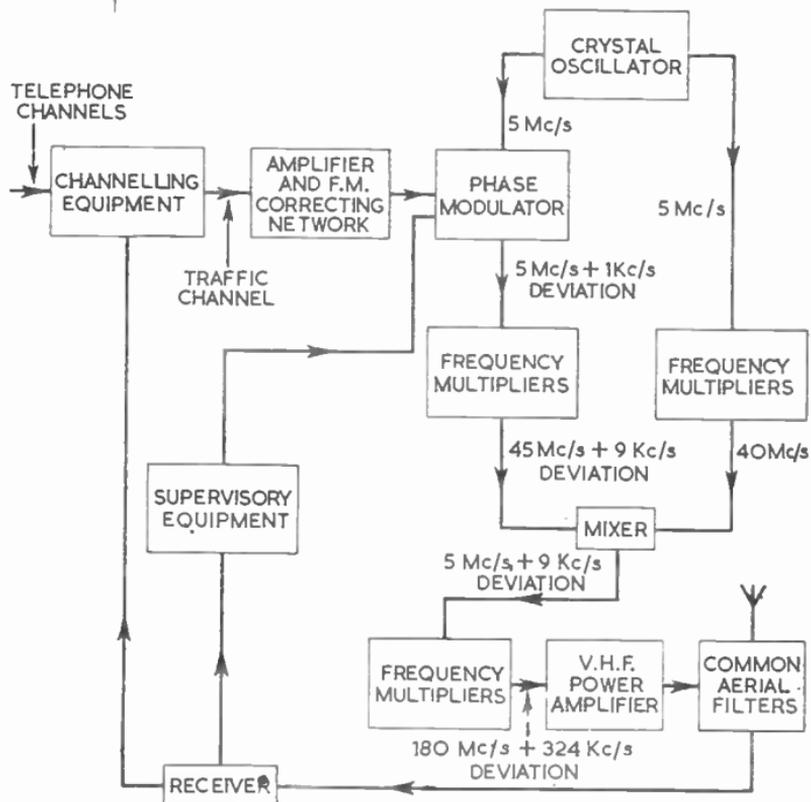
FIG. 35.—MULTI-CHANNEL TERMINAL TRANSMITTER AND RECEIVER.
