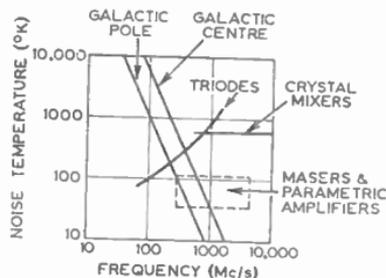
FIG. 11.—NOISE TEMPERATURES IN RELATION TO FREQUENCY.
