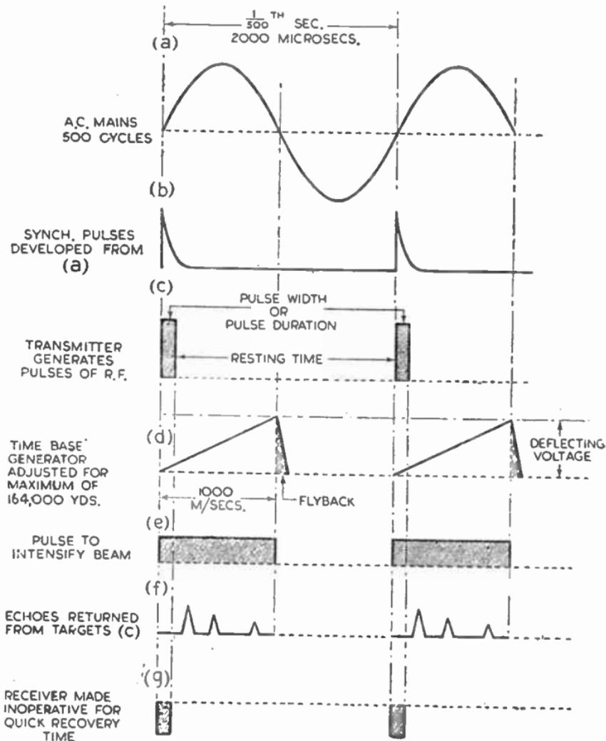
FIG. 20.—TIME RELATIONSHIPS IN BASIC RADAR SYSTEM.
