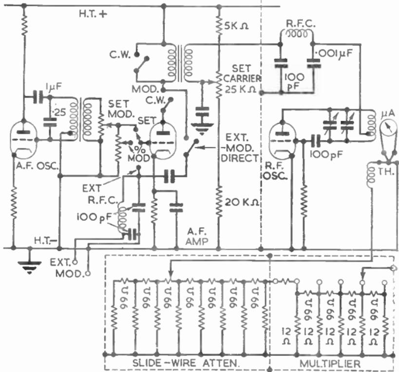
FIG. 20.—TYPICAL CIRCUIT OF A SIGNAL GENERATOR.
