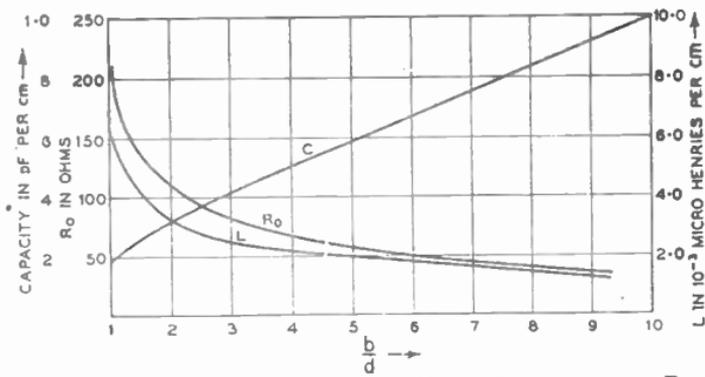
FIG. 15.—INDUCTANCE, CAPACITANCE AND SURGE IMPEDANCE OF PARALLEL TAPES.
