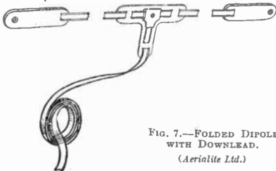
FIG. 7.—FOLDED DIPOLE WITH DOWNLEAD.
