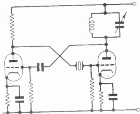
of the valve amplifier, which can then operate strictly in the linear mode. Provided that the phase change in the amplifier is constant, the crystal alone determines the frequency, since there are no other reactive elements in the bridge. Using this circuit, long-term stabilities better than one part in a hundred millions have been obtained.
