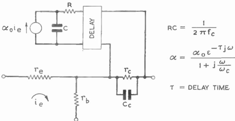
FIG. 23.—APPROXIMATE EQUIVALENT CIRCUIT FOR TRANSIENT ANALYSIS OF JUNCTION TRANSISTORS.
