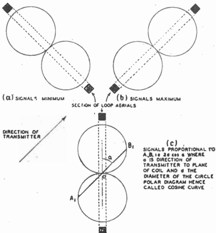
FIG. 3.—FIGURE-OF-EIGHT POLAR DIAGRAM OF LOOP AERIAL.
