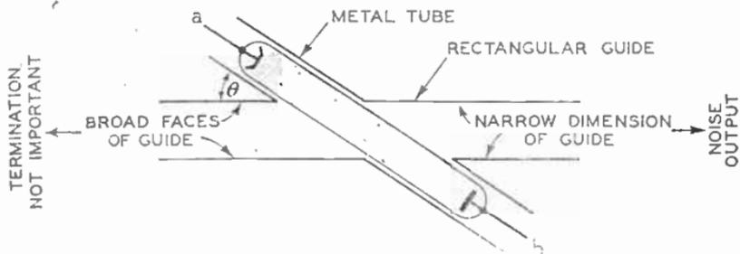
FIG. 4.—SIMPLIFIED DRAWING OF FLUORESCENT-TUBE NOISE SOURCE.
