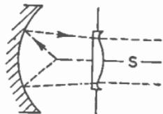
FIG. 1.—BASIC PRINCIPLE OF THE SCHMIDT OPTICAL SYSTEM.
