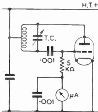
FIG. 34.—GRID-DIP OSCILLATOR.
