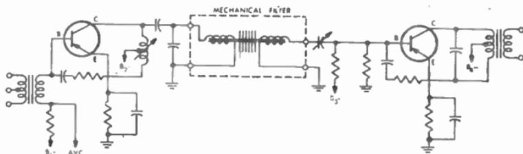
FIG. 8.—TRANSISTOR I.F. AMPLIFIER WITH MECHANICAL FILTER.
