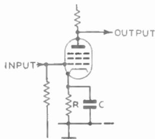
FIG. 7.—EXAMPLE OF A CIRCUIT FOR EFFECTING AFTERGLOW CORRECTION FOR A FLYING-SPOT SCANNER.
