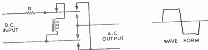
FIG. 15.—CIRCUIT FOR OBTAINING APPROXIMATELY THE SAME OUTPUT AS THE INPUT VOLTAGE.
