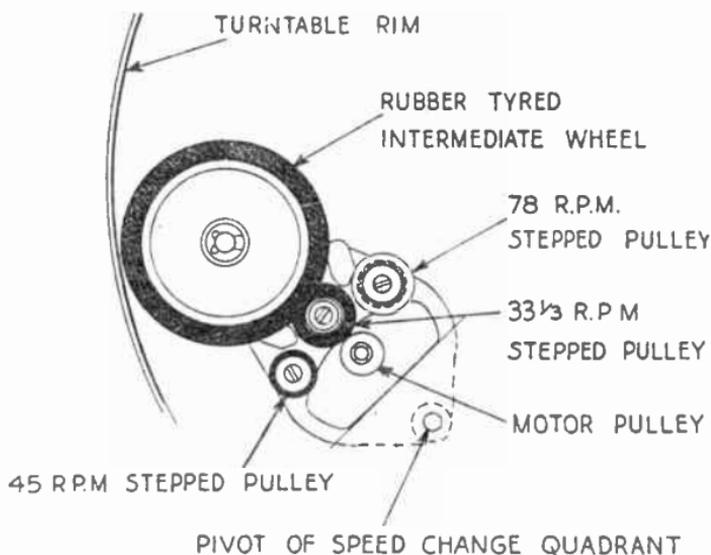
FIG. 3.—THREE-SPEED DRIVE USING THREE STEPPED PULLEYS.
