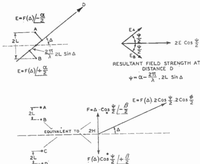
FIG. 16.—DERIVATION OF VERTICAL RADIATION PATTERNS.
