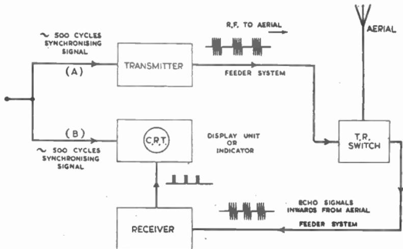
FIG. 19.—BASIC RADAR SYSTEM.
