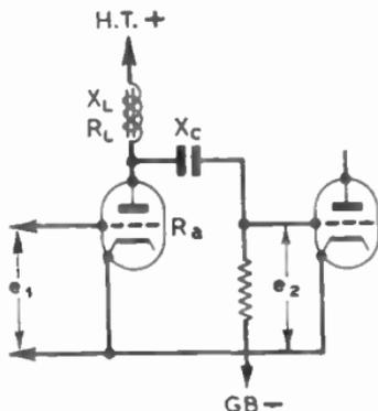
FIG. 61.—CHOKE COUPLING.
