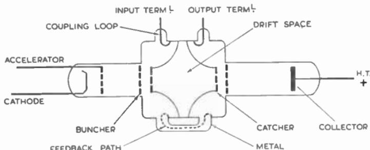
FIG. 23.—KLYSTRON WITH CAVITY RESONATORS.
