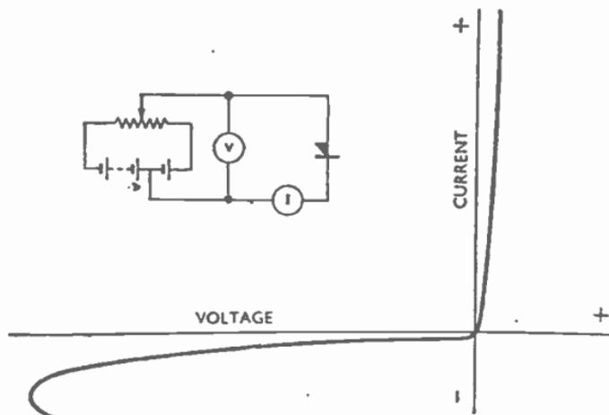
FIG. 3.—USUAL FORM OF PRESENTATION OF TYPICAL GERMANIUM RECTIFIER CHARACTERISTIC.
