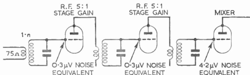
FIG. 2.—THE SIGNAL-TO-NOISE RATIO THROUGH THE FIRST STAGES OF THE RECEIVER.
