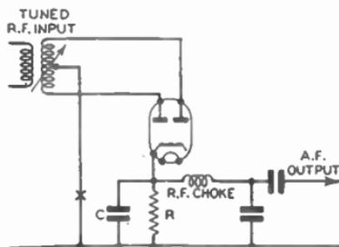
FIG. 4.—PUSH-PULL DIODE DETECTOR.
