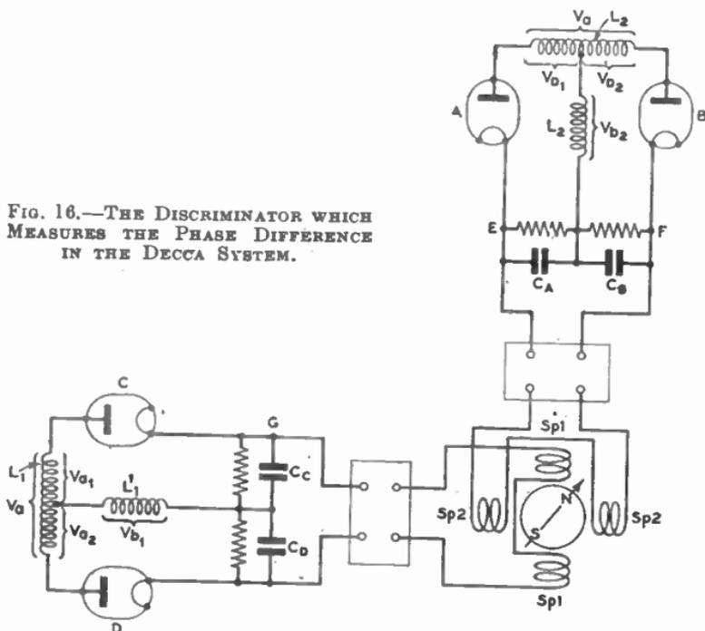
FIG. 16.—THE DISCRIMINATOR WHICH MEASURES THE PHASE DIFFERENCE IN THE DECCA SYSTEM.
