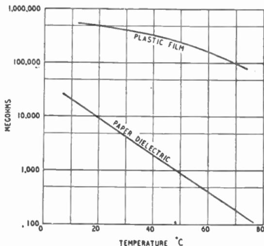
FIG. 8.—VARIATIONS OF INSULATING RESISTANCE WITH TEMPERATURE FOR TYPICAL 1- $\mu$ F CAPACITORS OF THE PLASTIC FILM AND PAPER DIELECTRIC TYPES.
