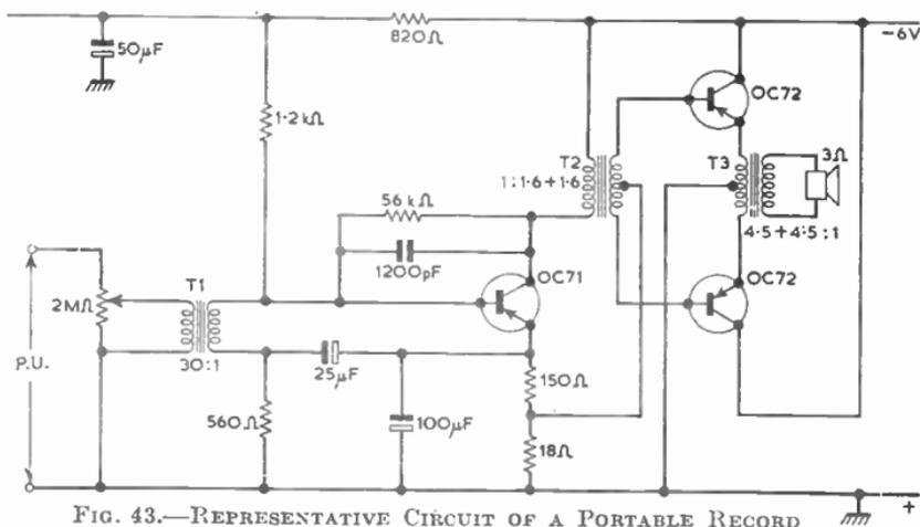
FIG. 43.—REPRESENTATIVE CIRCUIT OF A PORTABLE RECORD REPRODUCER.
