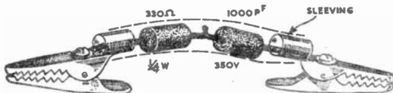
FIG. 9.—DAMPING DEVICE.
