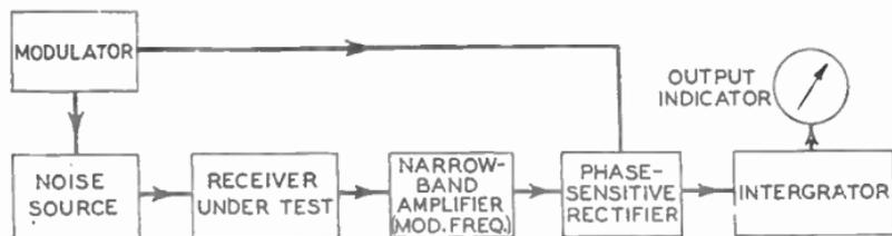
FIG. 7.—SKETCH SHOWING APPLICATION OF DICKE METHOD TO THE MEASUREMENT OF RECEIVER SENSITIVITY.
