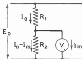
FIG. 123.—VOLTMETER WITH POTENTIAL DIVIDER.
