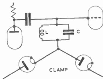
FIG. 72.—CLAMPING CIRCUIT FOR N.T.S.C. CIRCUITS.
