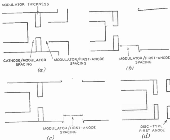
FIG. 3.—TRIODE ASSEMBLIES FOR CATHODE-RAY TUBES.
