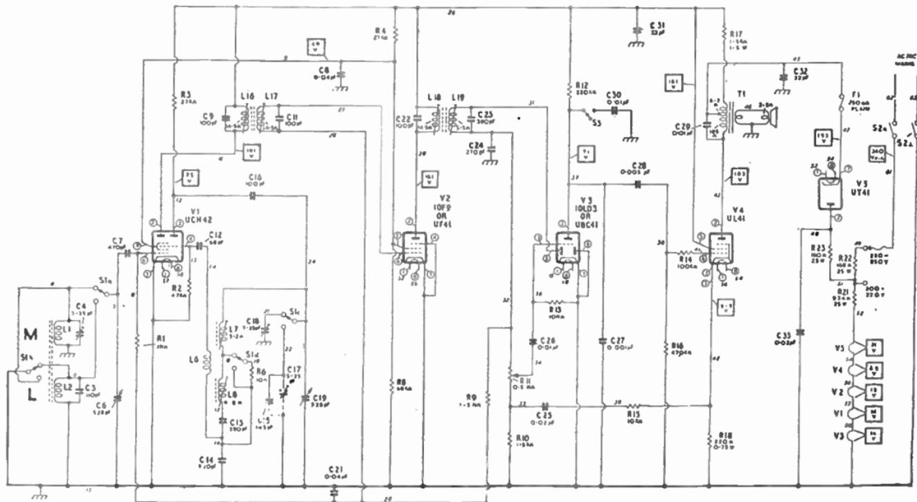
FIG. 17.—TYPICAL SMALL A.C./D.C. RECEIVER WITH FERRITE-ROD AERIAL.
