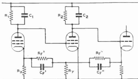
FIG. 29.—TWO-STAGE SIMPLIFIED AMPLIFIER WITH "APERIODIC FEEDBACK".
