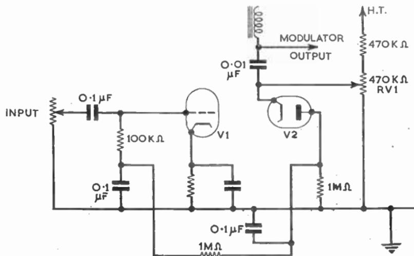
FIG. 17.—MODULATOR A.G.C. CIRCUIT.
