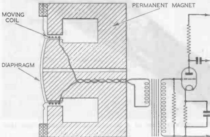
FIG. 6.—A MOVING-COIL MICROPHONE IN CIRCUIT.
