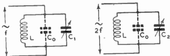
FIG. 131.—DETERMINATION OF SELF-CAPACITANCE OF INDUCTOR L.
