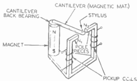
FIG. 20.—SCHEMATIC DIAGRAM OF A VARIABLE RELUCTANCE CARTRIDGE.
