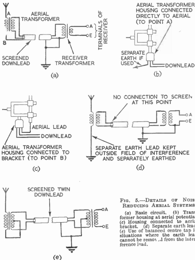
FIG. 5.—DETAILS OF NOISE REDUCING AERIAL SYSTEMS.
