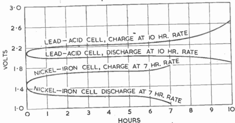
FIG. 10.—CHARGE AND DISCHARGE VOLTAGE CURVES OF LEAD-ACID AND NICKEL-IRON CELLS.
