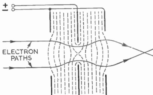
FIG. 9.—SYMMETRICAL OR UNIVOLTAGE ELECTRON LENS.
