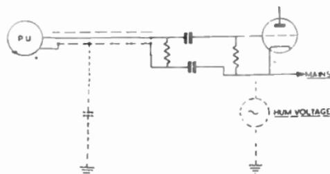
FIG. 27 (left).—TWO-SOCKET PICK-UP CONNECTION FOR NON-ISOLATED CHASSIS—UN-SUITABLE OWING TO HUM VOLTAGE.
