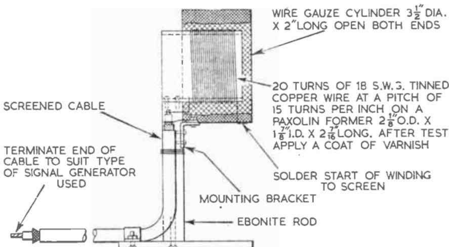
FIG. 12.—CONSTRUCTION OF A SHIELDED COIL.
