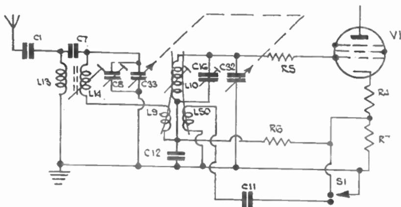
FIG. 13.—BAND-PASS TUNING CIRCUIT FOR RADIO-FREQUENCY AMPLIFIER.
