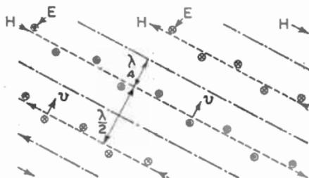
PLANE WAVE TRAVELLING WITH VELOCITY  $v$  DIAGONALLY UPWARDS
