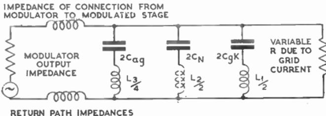
FIG. 11.—INPUT IMPEDANCE OF THE MODULATED STAGE.
