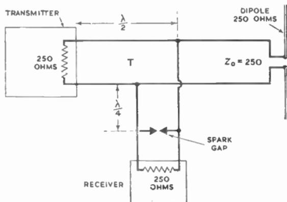
FIG. 35.—ELEMENTARY ARRANGEMENT FOR T.R. SWITCHING.
