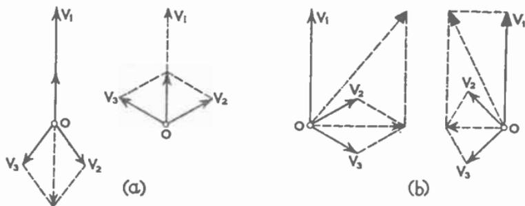
FIG. 31.—(a) VECTORIAL REPRESENTATION OF AMPLITUDE MODULATION; (b) VECTORIAL REPRESENTATION OF FREQUENCY MODULATION.
