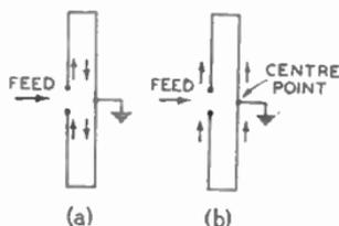
FIG. 22.—THE FOLDED DIPOLE.
