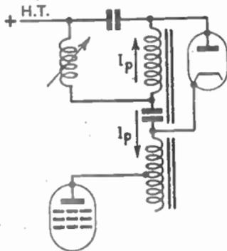
FIG. 47.—DESATURATED TRANSFORMER.
