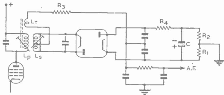
FIG. 37.—PRACTICAL RATIO DETECTOR, BALANCED CIRCUIT.
