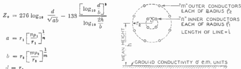
FIG. 15.—MULTI-WIRE UNBALANCED TRANSMISSION LINE.
