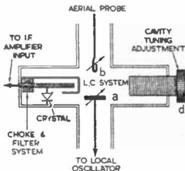
FIG. 45 (a) (above).—CRYSTAL MIXER IN A RESONANT CAVITY.
