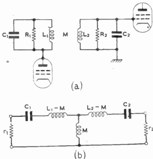
FIG. 7.—TRANSFORMER AS BAND-PASS FILTER: (a) PRACTICAL APPLICATION OF TRANSFORMER AS BAND-PASS FILTER; (b) APPROXIMATE EQUIVALENT OF TUNED BAND-PASS TRANSFORMER.
