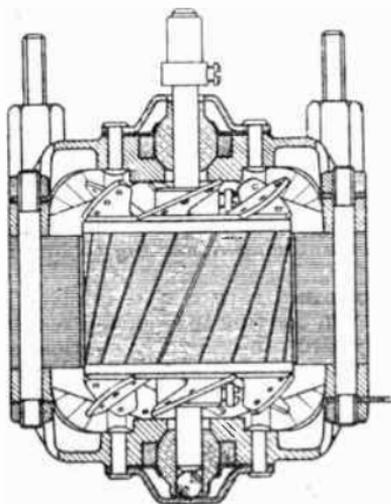
FIG. 5 (above).—SECTIONAL VIEW OF OF A TYPICAL INDUCTION MOTOR USED ON GRAMOPHONE UNITS.
