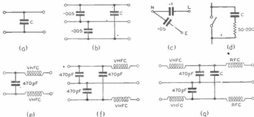
FIG. 1.—BASIC INTERFERENCE-SUPPRESSION DEVICES.
