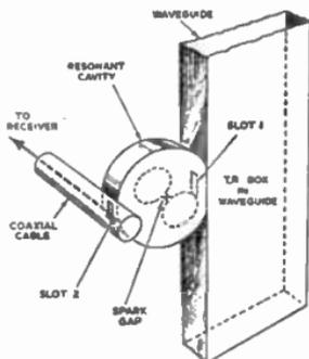
FIG. 37.—T.R. SWITCHING FOR WAVEGUIDE SYSTEMS.
