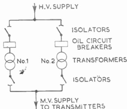
FIG. 5.—DUPLICATION OF SUPPLY TRANSFORMERS.
