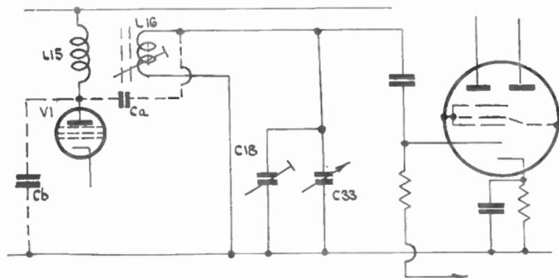
FIG. 15.—INTERSTAGE COUPLING FOR 3-9-Mc/s BAND.
