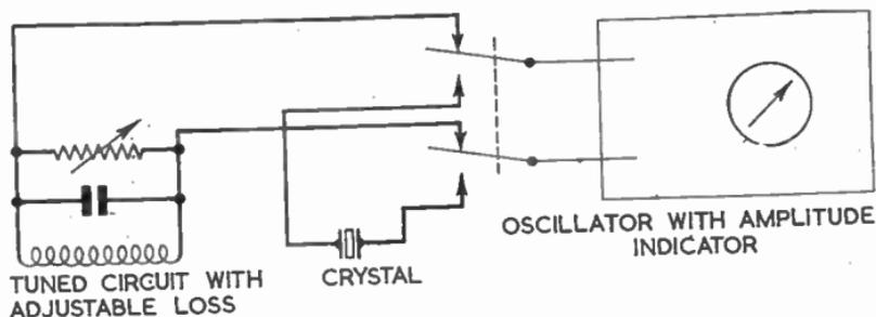
FIG. 22.—DIAGRAMMATICAL ARRANGEMENT FOR MEASURING THE EQUIVALENT PARALLEL RESISTANCE OF A CRYSTAL.
