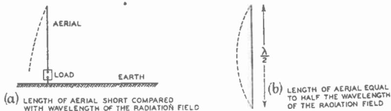
FIG. 11.—CURRENT DISTRIBUTION IN ROD AERIALS.
