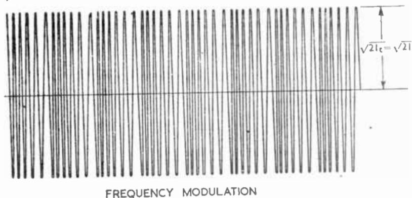
FIG. 79.—CARRIER ENVELOPE SHOWING FREQUENCY MODULATION
