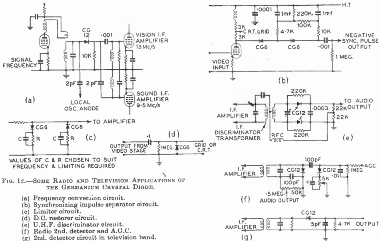
FIG. 12.—SOME RADIO AND TELEVISION APPLICATIONS OF THE GERMANIUM CRYSTAL DIODE.
