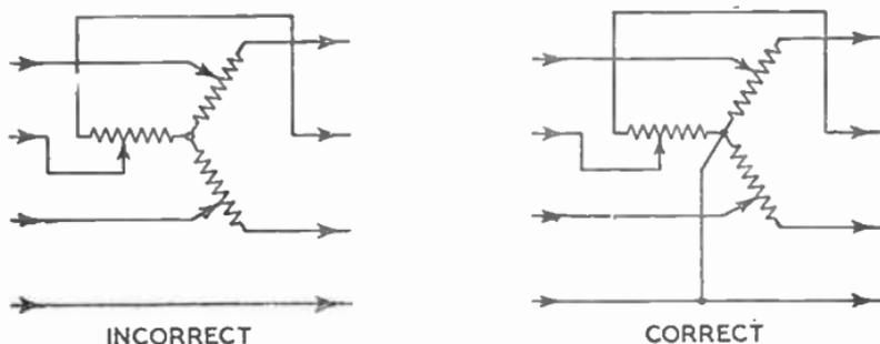
FIG. 8.—THREE-PHASE AUTO-TRANSFORMER—THREE-PHASE, FOUR-WIRE SUPPLY.
