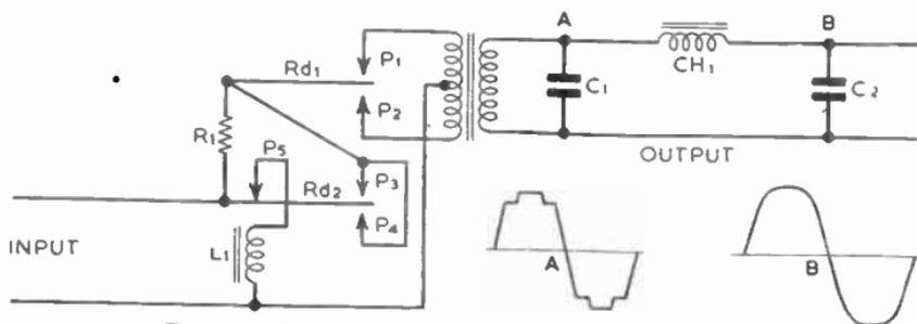
FIG. 16.—TYPICAL VIBRATOR CONVERTER CIRCUIT.
