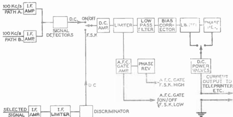
FIG. 16.—BLOCK DIAGRAM OF THE D.C. CIRCUITS OF A TYPICAL TELEGRAPH RECEIVER.
