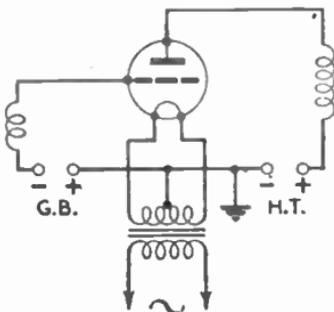
FIG. 33.—CENTRE TAP FEED RETURN FOR ELIMINATING GRID-CATHODE MODULATION BY A.C.
