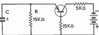
rod aerial and achieves extra gain by reflex use of one transistor for both intermediate-frequency and audio-frequency amplification. The total current consumption is 7 mA at 15 volts for the H.T., plus 1 mA at 1.25 volts for the bias. Fixed tuning is employed and an intermediate frequency of 165 kc/s is chosen, so that long-wave coils may be used for the intermediate-frequency transformers.
