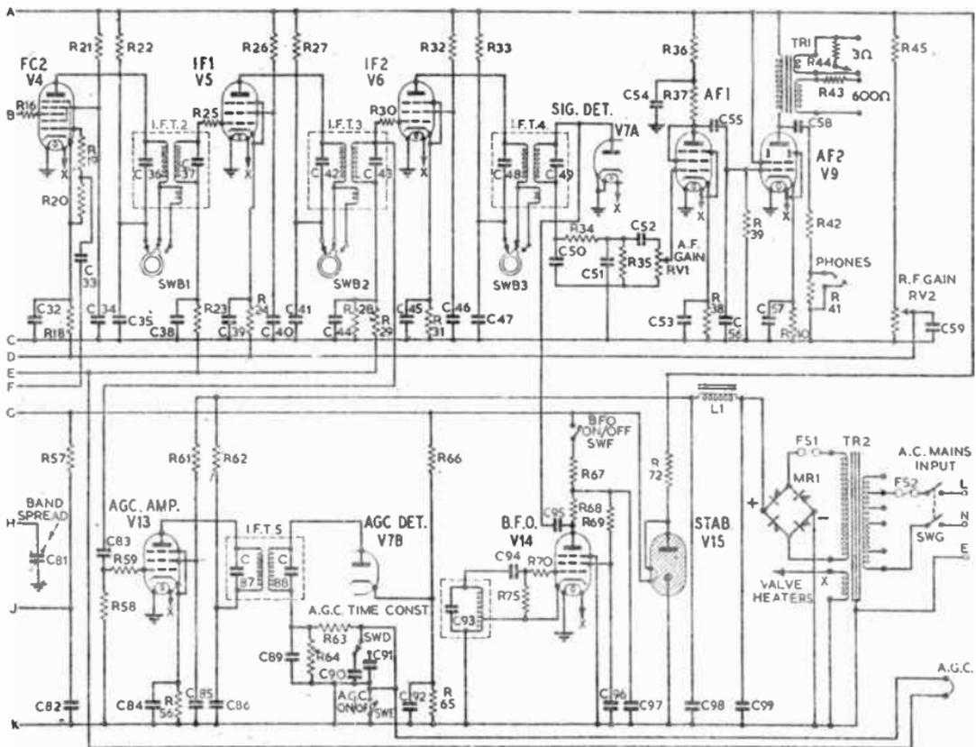
FIG. 13 (b).—INTERMEDIATE-FREQUENCY AND AUDIO-FREQUENCY SECTION OF TYPICAL DOUBLE-CONVERSION COMMUNICATION RECEIVER.
