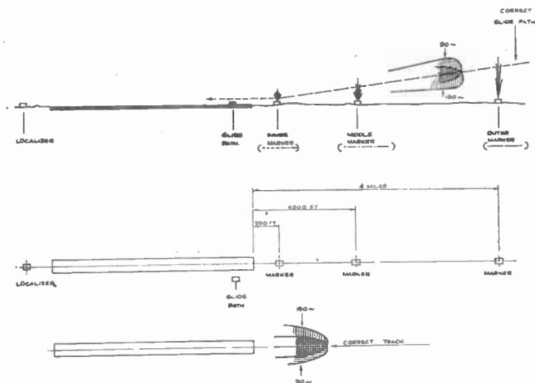
FIG. 11.—INSTRUMENT LANDING SYSTEM LAYOUT.
