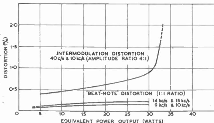
FIG. 5.—INTERMODULATION DISTORTION MEASUREMENTS ON MODERN HIGH-FIDELITY AMPLIFIER.
