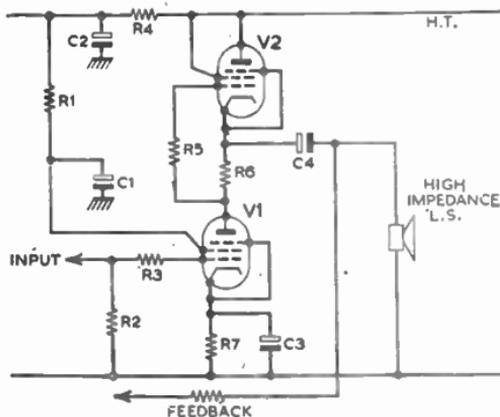
FIG. 9.—ONE PRACTICAL ARRANGEMENT FOR THE ELIMINATION OF THE OUTPUT TRANSFORMER.
