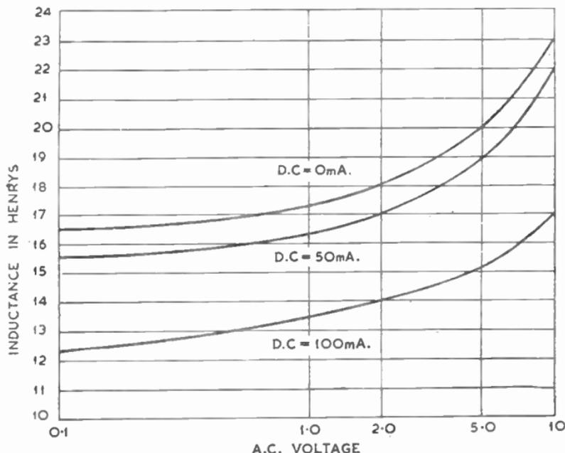
FIG. 47.—EFFECT OF INPUT VOLTAGE ON INDUCTANCE.
