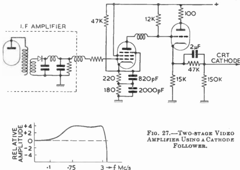
FIG. 27.—TWO-STAGE VIDEO AMPLIFIER USING A CATHODE FOLLOWER.
