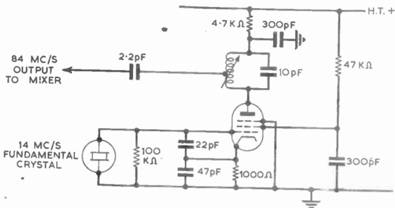
FIG. 27.—COMBINED OSCILLATOR AND FREQUENCY MULTIPLIER.
