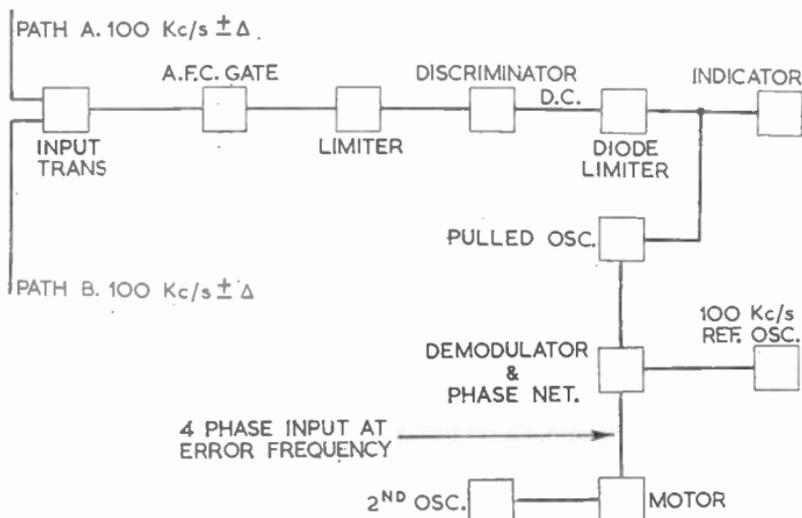
FIG. 19.—BLOCK DIAGRAM OF A TELEGRAPH RECEIVER A.F.C. SYSTEM.
