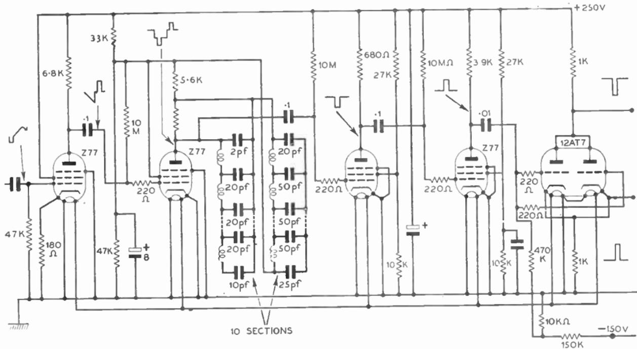
of the separator consists of a short-circuited delay line  $D_1$  with transmission time of, say, 3 microseconds.
