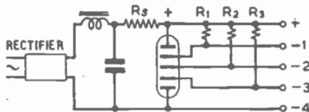
FIG. 32.—GRID-BIAS RECTIFIER WITH GLOW-GAP DIVIDER.
