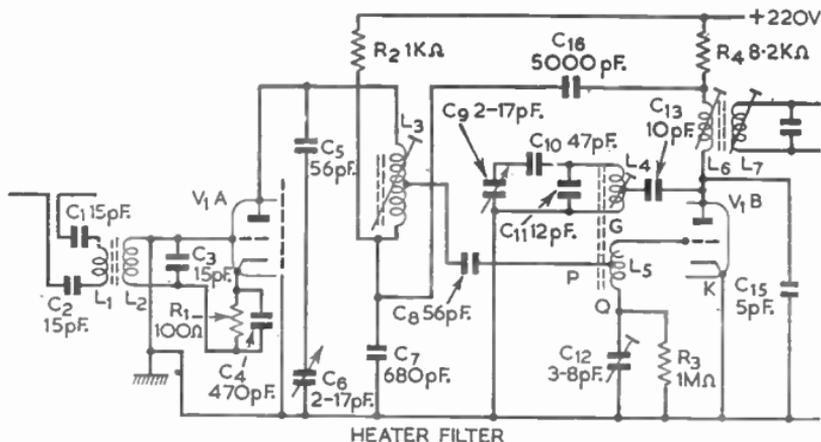
FIG. 30 (above).—V.H.F. R.F. AMPLIFIER AND MIXER, USING DOUBLE TRIODES WITH GANGED CAPACITOR TUNING. L8 is self-resonant at 104 Mc/s.
