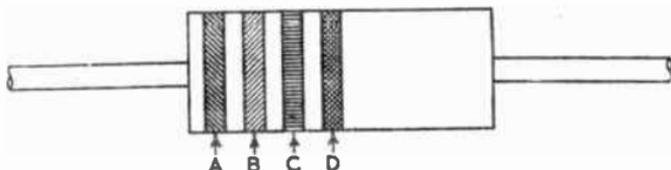
FIG. 1.—RESISTOR COLOUR CODING.
