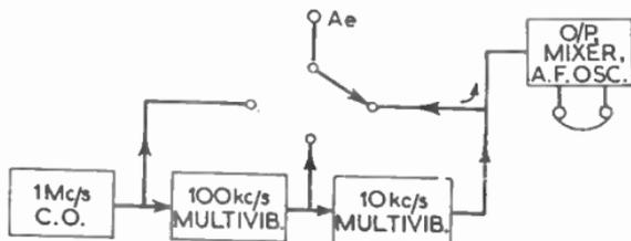
FIG. 33.—BLOCK SCHEMATIC LAYOUT OF A CRYSTAL CALIBRATOR.
