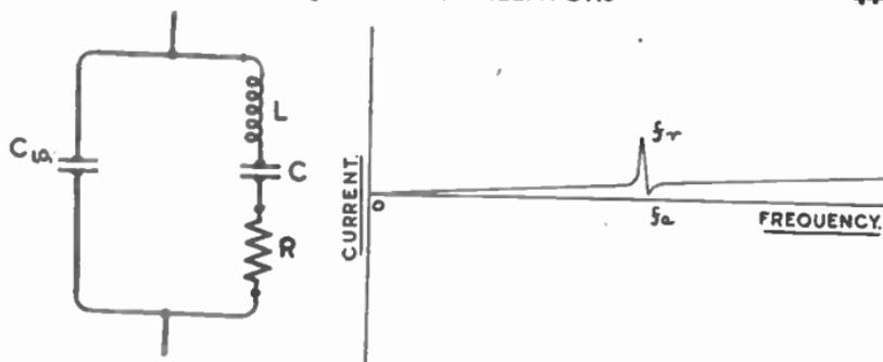
FIG. 2.—THE EQUIVALENT CIRCUIT OF A QUARTZ CRYSTAL.
