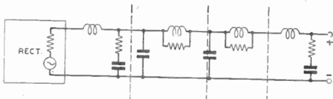
FIG. 68.—FORMS OF CONSTANT-IMPEDANCE NETWORKS AS SUPPLY FILTER.
