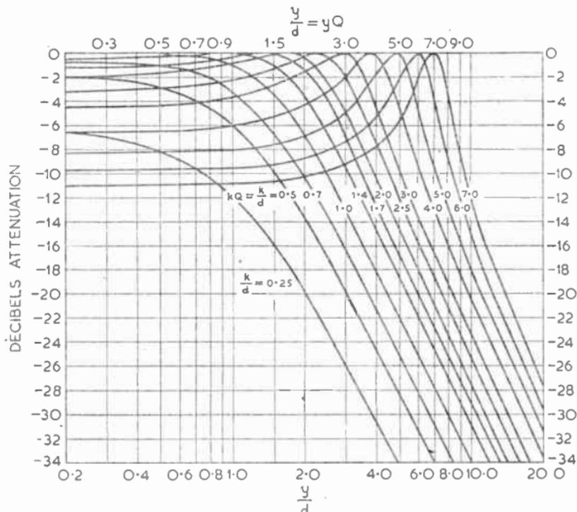
FIG. 6.—RESONANCE CURVES OF COUPLED CIRCUITS.
