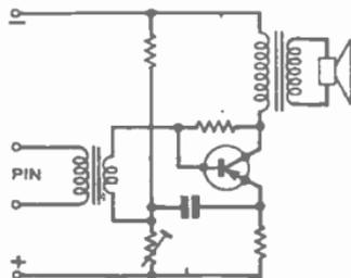
FIG. 49.—SINGLE TRANSISTOR CLASS A OUTPUT STAGE.
