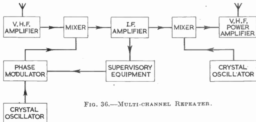
FIG. 36.—MULTI-CHANNEL REPEATER.
