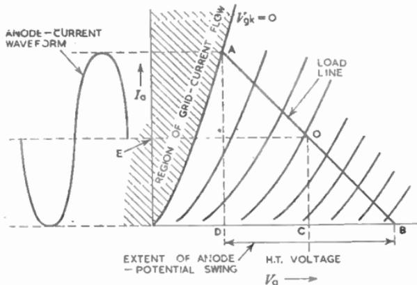
FIG. 3.—LIMITATION OF ANODE-POTENTIAL SWING BY GRID-CURRENT FLOW IN A CLASS A AMPLIFIER.
