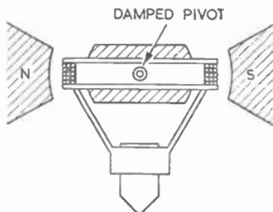
FIG. 8.—MOVING-COIL SYSTEM.
