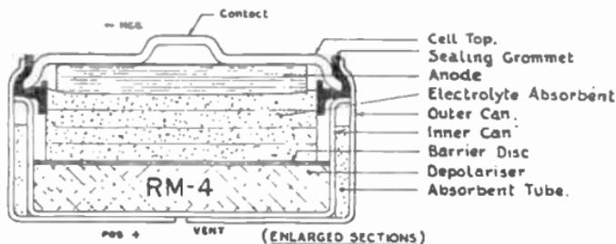
FIG. 8 (b).—POWDERED-ANODE-TYPE CELL.
