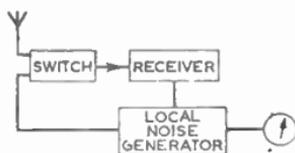
FIG. 14.—MACHIN, RYLEE AND VONBERG SERVO-CONTROLLED RADIOMETER.
