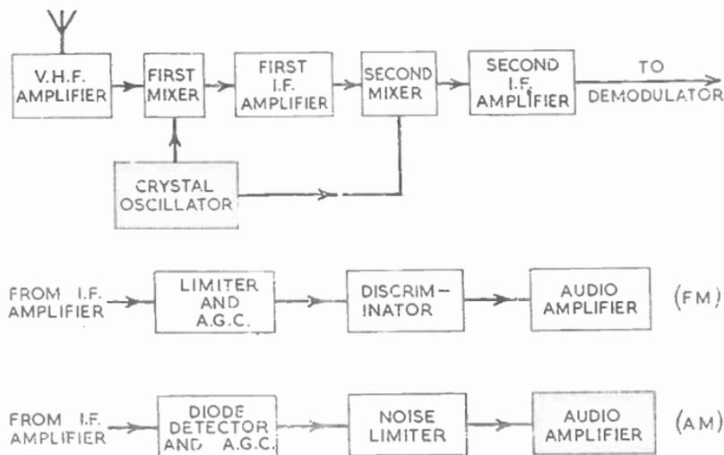
FIG. 23.—BLOCK DIAGRAM OF A V.H.F. RECEIVER.
