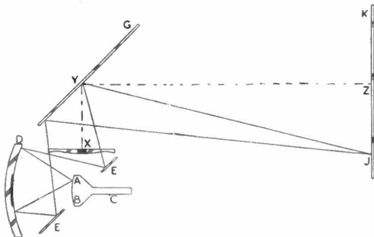
FIG. 3.—THE SCHMIDT "FOLDED OPTICAL" SYSTEM.
