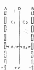
FIG. 21.—THE CONSTANT CHARGE PRINCIPLE.
