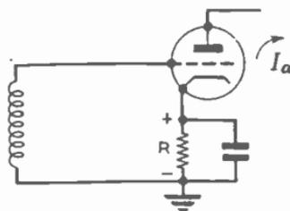
FIG. 30.—CATHODE RESISTANCE BIASING.
