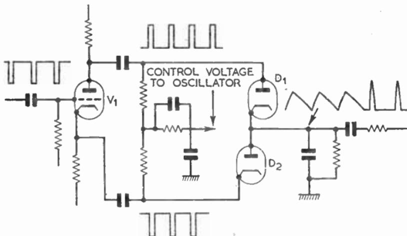
FIG. 34.—AN ALTERNATIVE CIRCUIT FOR AUTOMATIC PHASE CONTROL.
