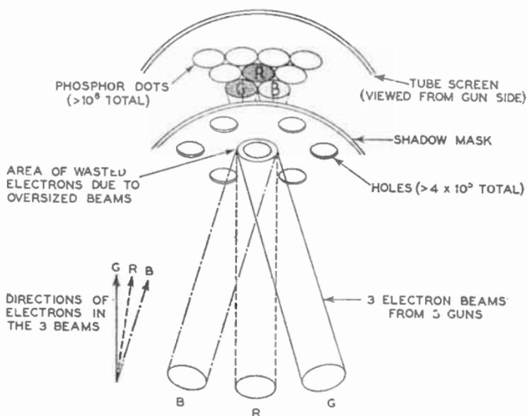
FIG. 21.—THREE-GUN DISPLAY TUBE USING SHADOW OR APERTURE MASK.
