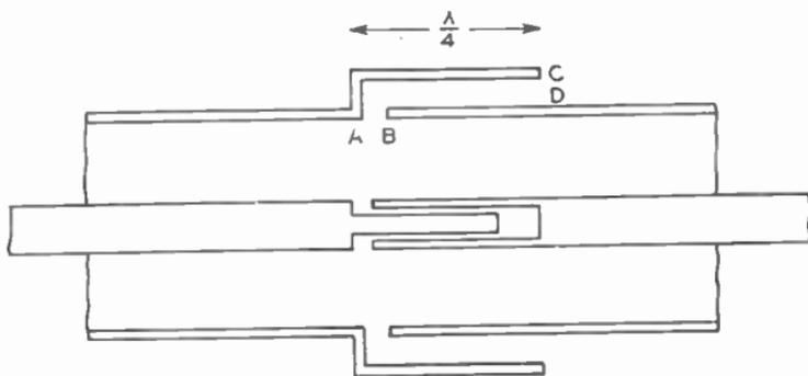
FIG. 34.—ROTATING JOINT FOR CO-AXIAL FEEDER.
