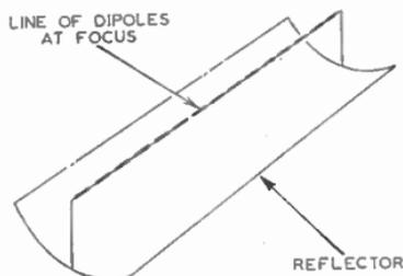
FIG. 3 (left).—A PARABOLIC TROUGH AERIAL.
