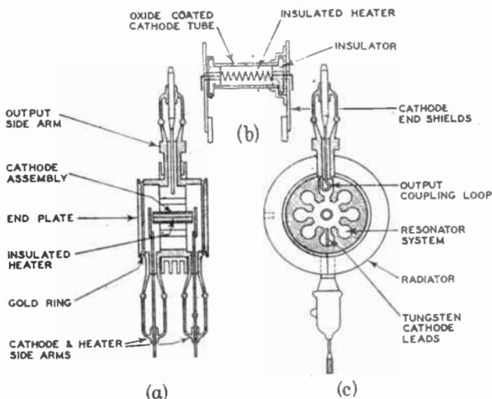
FIG. 21.—A MULTI-RESONANT MAGNETRON.
