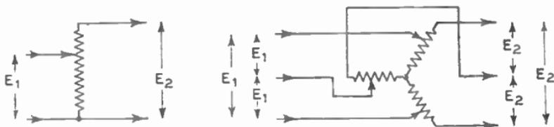
FIG. 7.—ONE-PHASE AND THREE-PHASE AUTO-TRANSFORMERS.
