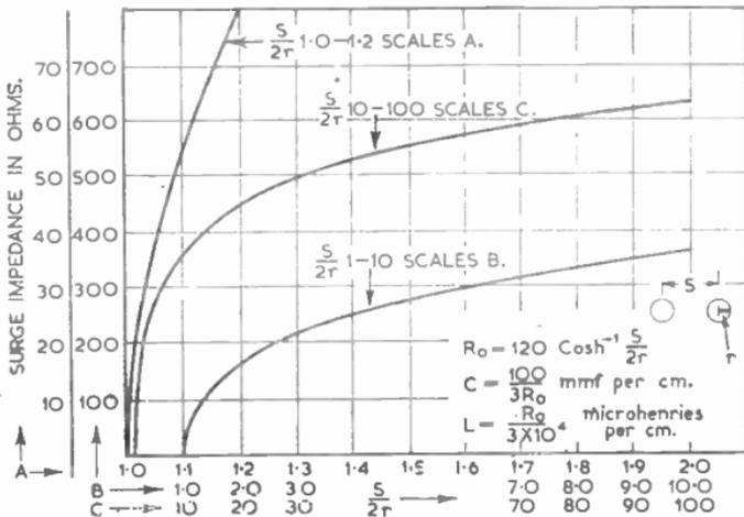
FIG. 14.—SURGE IMPEDANCE OF PARALLEL CYLINDERS—ANY SPACING.
