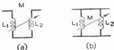
FIG. 34.—INDUCTANCE OF TWO COUPLED CIRCUITS.
