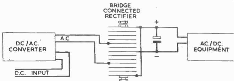
FIG. 17.—USE OF A D.C./A.C. CONVERTER WITH A.C./D.C. EQUIPMENT.
