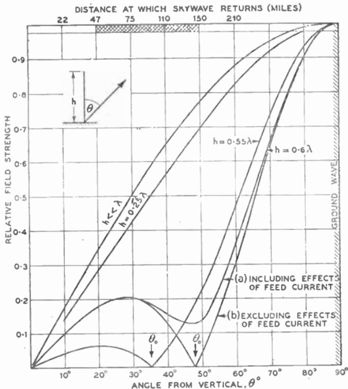
FIG. 11.—RADIATION FROM VERTICAL AERIALS.
