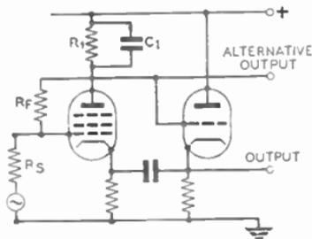
FIG. 26 (b).—ALTERNATIVE "OPTIMAL FEEDBACK" CIRCUIT.
