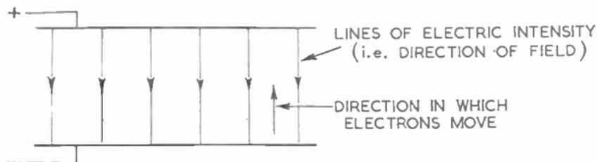
FIG. 2.—ELECTRIC FIELD BETWEEN TWO PARALLEL CHARGED PLATES.
