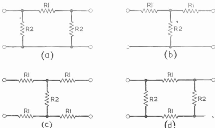
FIG. 13.—ATTENUATORS: (a) "pi" TYPE; (b) "T" TYPE; (c) "T" TYPE FOR BALANCED TWIN FEEDERS; (d) "pi" TYPE FOR BALANCED TWIN FEEDERS
