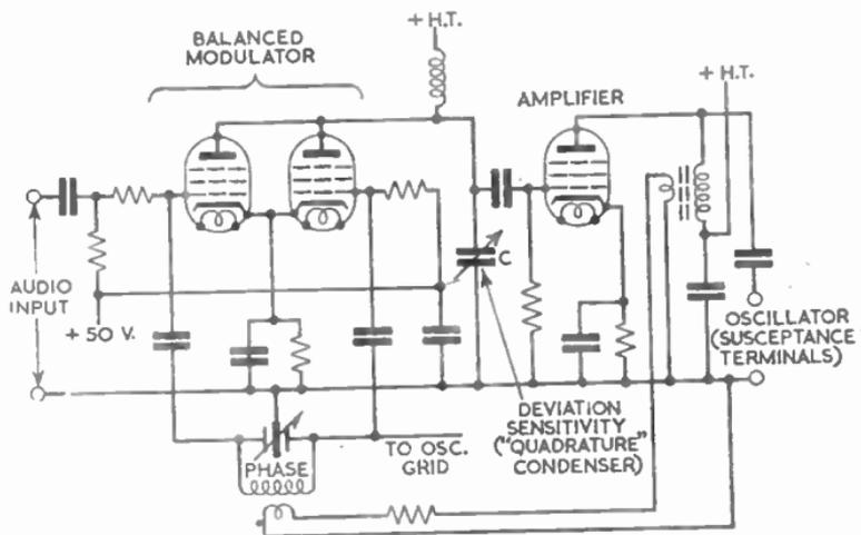
FIG. 42.—THREE-VALVE "SUSCEPTANCE MODULATOR" CIRCUIT.
