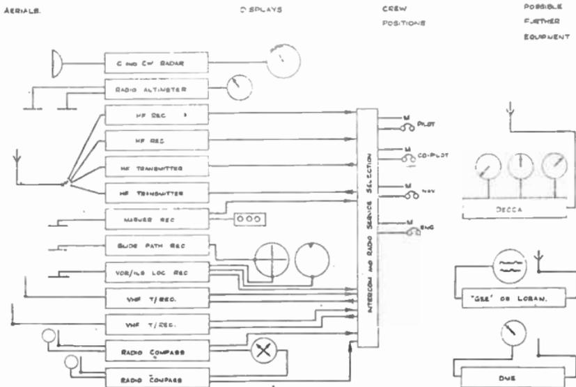
FIG. 12.—TYPICAL MAIN-LINE AIRCRAFT RADIO AND NAVIGATION INSTALLATION.
