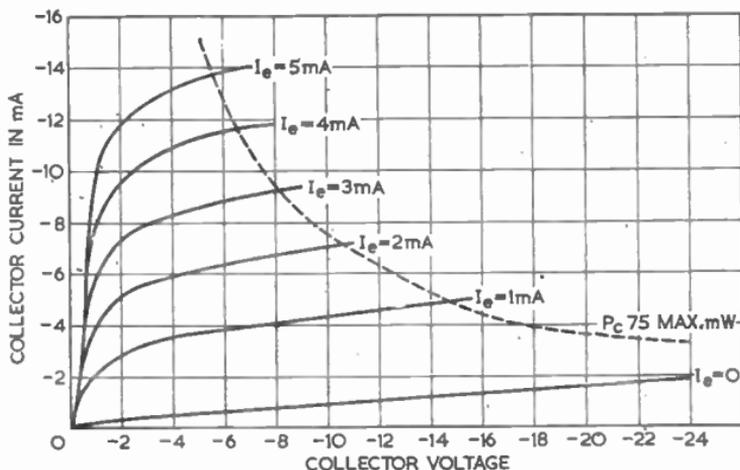
FIG. 26.—COMMON BASE CHARACTERISTICS OF A TYPICAL POINT-CONTACT TRANSISTOR, TYPE GET 2.
