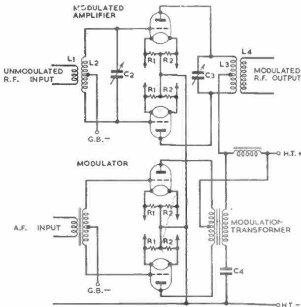
FIG. 20.—CLASS B MODULATOR WITH PARALLEL-FED MODULATION TRANSFORMER.
