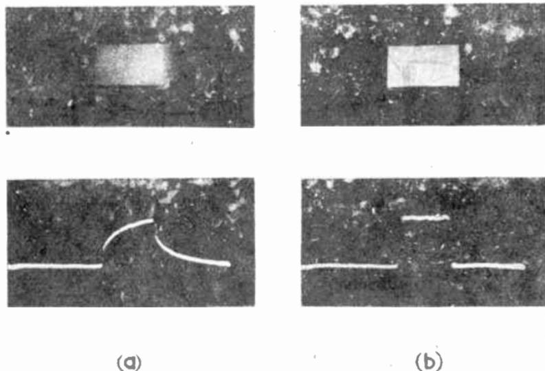
FIG. 6.—TELEVISION PICTURES AND OSCILLOGRAMS SHOWING THE EFFECTS OF SCANNING-TUBE PHOSPHOR AFTERGLOW: (a) UNCORRECTED; (b) CORRECTED BY SCREEN DIFFERENTIATING CIRCUITS.
