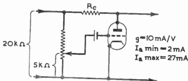
variation of supply voltage over which control will be effective. The anode current change obtainable is 2–27 mA,  $g = 10\text{ mA/volt}$ , and the resistance of the voltage divider is  $20\text{ k}\Omega$  tapped a quarter of the way up.
