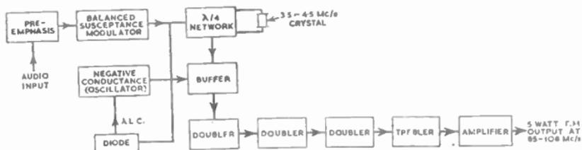
FIG. 41.—BLOCK SCHEMATIC DIAGRAM OF "F.M.Q." DRIVE.
