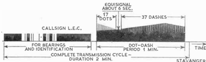
FIG. 11.—DIAGRAM OF THE SIGNAL STRENGTH DURING THE WHOLE TRANSMISSION CYCLE FROM STAVANGER, FOR ONE POSITION LINE.
