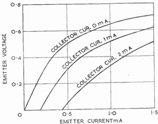
FIG. 2.—STATIC CHARACTERISTICS OF TYPICAL POINT-CONTACT TRANSISTOR.
