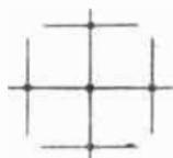
FIG. 24 (left).—THE LOBES OF THE CHRISTIANSEN INTERFEROMETER PROJECTED ON TO THE CELESTIAL SPHERE. THE RECEIVER RESPONDS ONLY TO SOURCES AT THE POINTS OF INTERSECTION.
