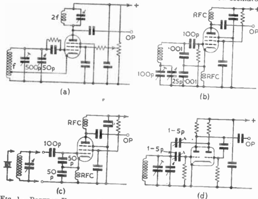
FIG. 1.—POPULAR VARIABLE FREQUENCY OSCILLATOR CIRCUITS: (a) E.C.O.; (b) "CLAPP"; (c) "COMO"; (d) "FRANKLIN".
