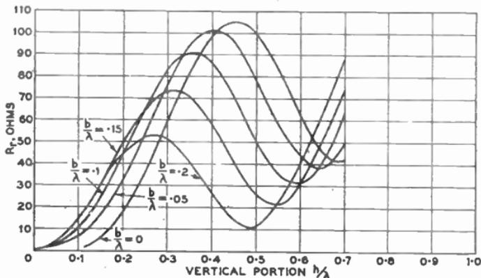
FIG. 9.—LOAD RADIATION RESISTANCE OF VERTICAL AERIAL.  $\lambda$  is the height of vertical portion;  $b$  is the equivalent length of top.
