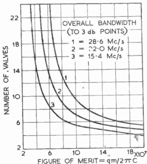
FIG. 9.—NUMBER OF VALVES REQUIRED TO OBTAIN A GAIN OF 90 db AS DETERMINED BY REQUIRED BAND-WIDTH AND FIGURE OF MERIT.
