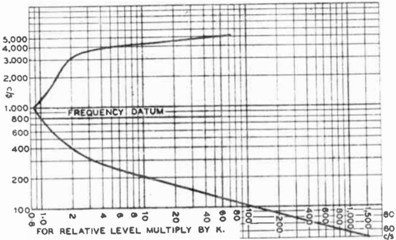
FIG. 43.—C.C.I.F. "WEIGHTING" CURVE FOR BROADCASTING SYSTEM.
