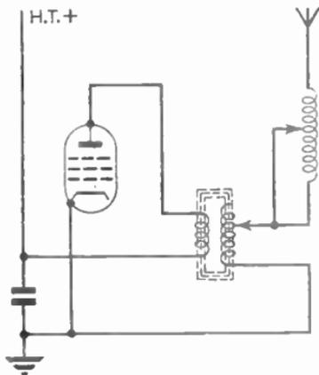
FIG. 14.—WIDE-BAND RADIO-FREQUENCY TRANSFORMER AERIAL COUPLING.
