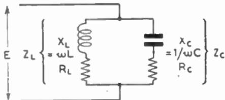
FIG. 31.—PARALLEL RESONANT CIRCUIT.
