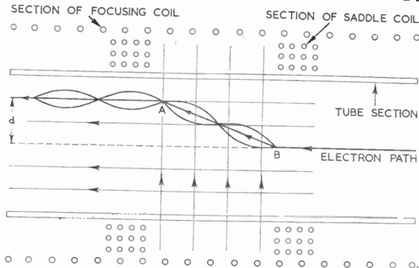
FIG. 20.—LONGITUDINAL SECTION OF TUBE WITH SADDLE AND FOCUSING COIL ILLUSTRATING THE PRINCIPLE OF ORTHOGONAL SCANNING.
