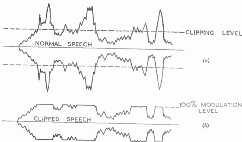
FIG. 18.—SPEECH WAVEFORMS SHOWING EFFECT OF CLIPPING.
