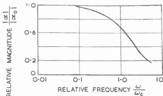
FIG. 10.—VARIATION OF CURRENT AMPLIFICATION FACTOR WITH FREQUENCY FOR JUNCTION TYPE TRANSISTORS.
