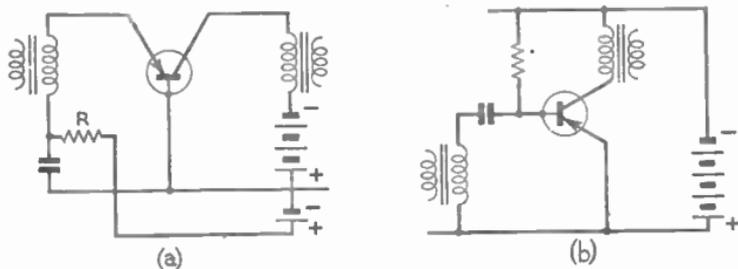
FIG. 27 (above).—(a) BIAS CIRCUIT FOR COMMON BASE CONNECTED TRANSISTOR. (b) BIAS CIRCUIT FOR COMMON EMITTER CONNECTED TRANSISTOR.
