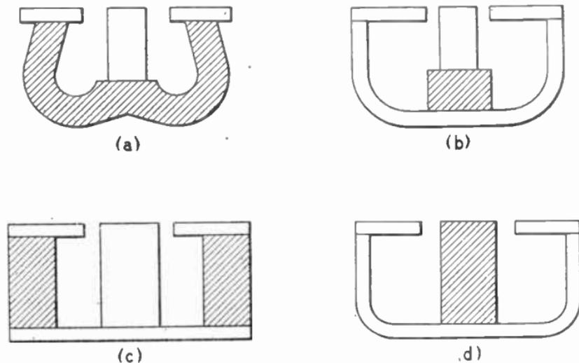
FIG. 6.—TYPES OF MAGNETS.
