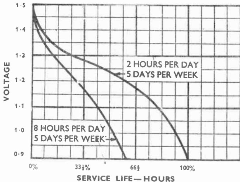
FIG. 6.—THE EFFECT OF THE TIME CYCLE ON A BATTERY'S LIFE.
