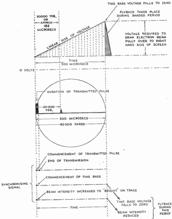
FIG. 25.—A RELATION OF RANGE TO FORM OF TIME-BASE VOLTAGE WAVE.
