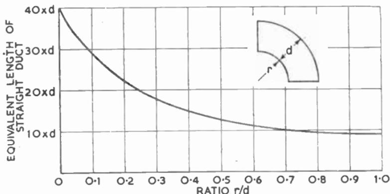
FIG. 22.—EQUIVALENT LENGTHS OF RADIUSSED BENDS IN AIR DUCTS.
