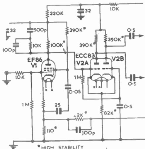
FIG. 12.—INPUT AND PHASE-SPLITTER STAGES OF A MODERN POWER AMPLIFIER.
