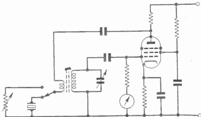
FIG. 21.—SIMPLIFIED CIRCUIT OF AN EQUIVALENT SERIES RESISTANCE MEASUREMENT SET.
