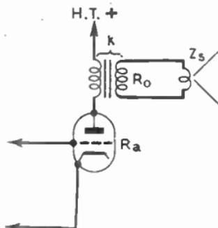
FIG. 63.—OUTPUT TRANSFORMER.
