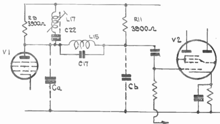
FIG. 14.—MEDIUM-WAVE INTERSTAGE COUPLING.
