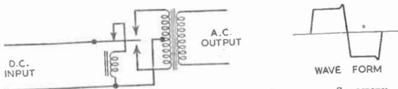
FIG. 14.—VIBRATOR CIRCUIT GIVING INCREASED FREQUENCY STABILITY.
