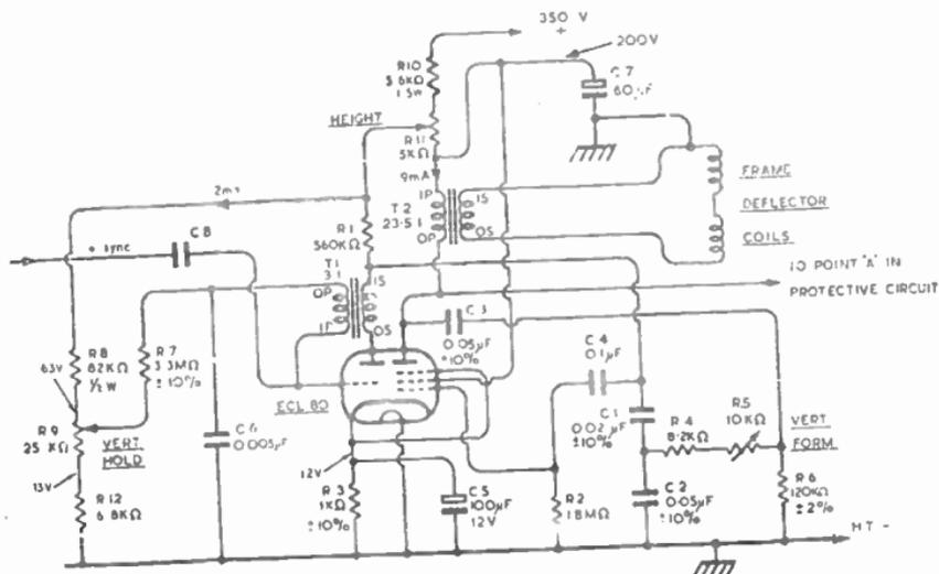
FIG. 7.—FRAME TIME-BASE GENERATOR CIRCUIT.
