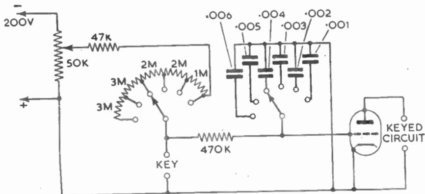
FIG. 10.—VALVE-KEYER WITH ADJUSTABLE LAG CHARACTERISTICS.
