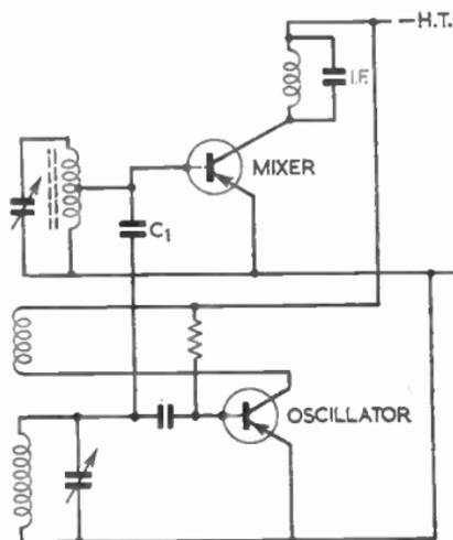
FIG. 38 (below).—EXPERIMENTAL SUPERHETERODYNE RECEIVER USING TWO POINT-CONTACT AND TWO JUNCTION TRANSISTORS. FIXED TUNING IS EMPLOYED.
