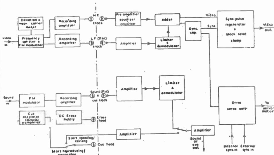
FIG. 5.—BLOCK DIAGRAM OF THE PRINCIPAL ELECTRONIC UNITS OF THE B.B.C. VISION ELECTRONIC RECORDING APPARATUS.
