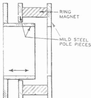
FIG. 3.—TYPICAL MAGNETIC FOCUSING ASSEMBLY FOR A TELEVISION CATHODE-RAY TUBE.
