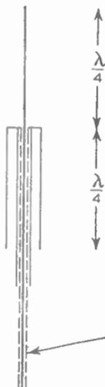
FIG. 32 (left).—CO-AXIAL HALF-WAVE DIPOLE AERIAL.
