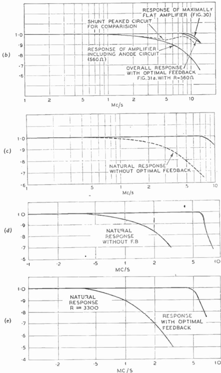
FIG. 31.—(b) RESPONSE CURVES FOR THE CIRCUIT GIVEN IN FIG. 31 (a).
