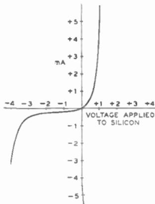
FIG. 1.—VOLTAGE/CURRENT CURVE OF TYPICAL SILICON RECTIFIER.
