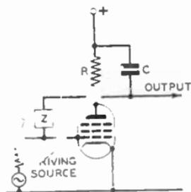
FIG. 20.—SINGLE STAGE WITH VOLTAGE FEEDBACK.
