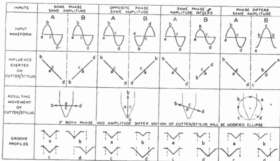
FIG. 26.—BASIC PRINCIPLES OF THE "45/45 OUT OF PHASE" DUAL-CHANNEL DISC RECORDING SYSTEM.
