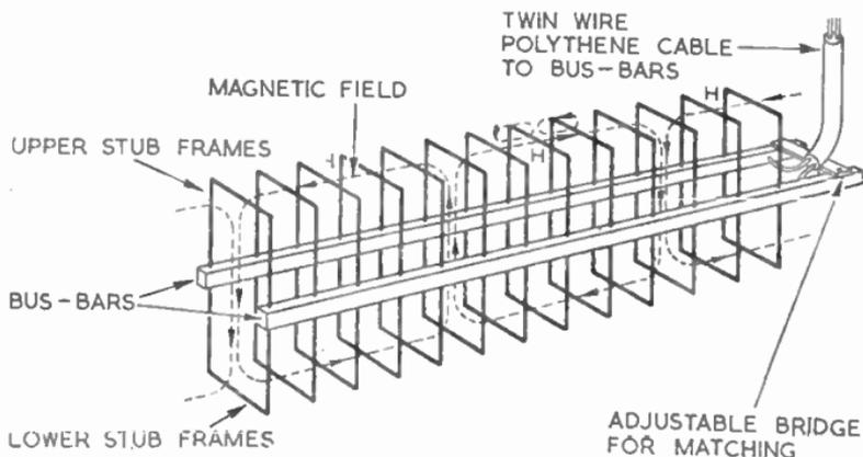
FIG. 5.—OUTLINE OF A SKELETON WAVEGUIDE SHOWING AN  $H_0$  TRAVELLING WAVE.
