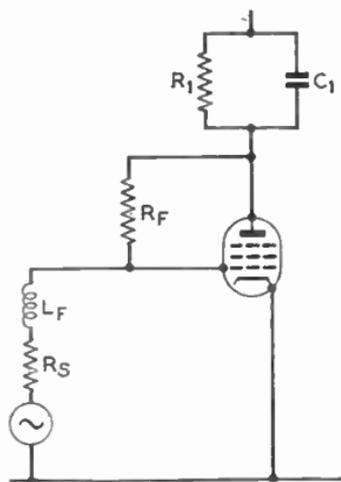
FIG. 24.—ALTERNATIVE FORM OF APERIODIC FEEDBACK WHERE  $R_S \ll R_F$  AND  $L_F/R_S = R_1 C_1$  (FIG. 23).
