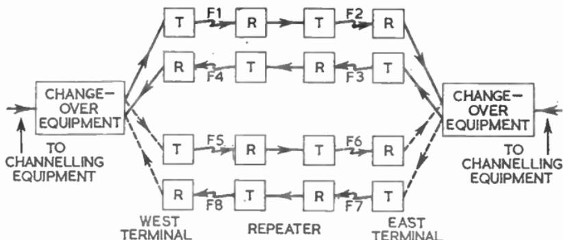
FIG. 37.—MULTI-CHANNEL SYSTEM WITH AUTOMATIC CHANGE-OVER FACILITIES.
