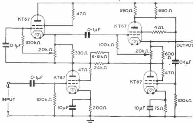
FIG. 44.—EXPERIMENTAL SHUNT-REGULATED AMPLIFIER.
