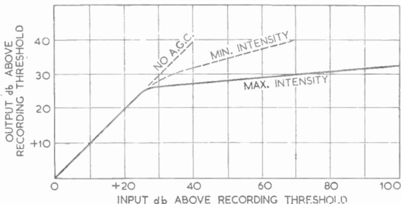
FIG. 18.--TELEGRAPH RECEIVER A.G.C. CHARACTERISTIC.
