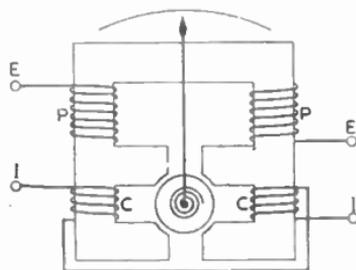
FIG. 13 (above).—INDUCTION-TYPE WATTMETER.
