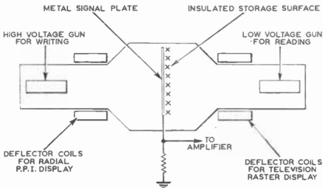
FIG. 25.—TWO GUN STORAGE TUBE FOR RADAR SCAN CONVERSION.
