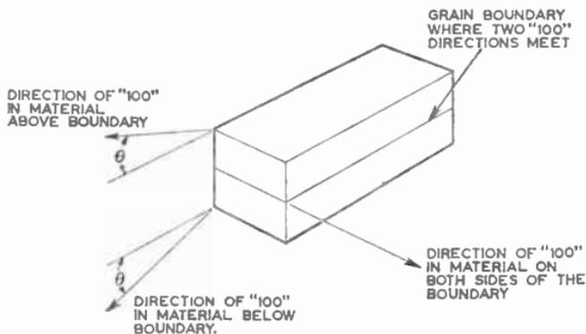
FIG. 20.—SEMI-CONDUCTOR WITH GRAIN-BOUNDARY.
