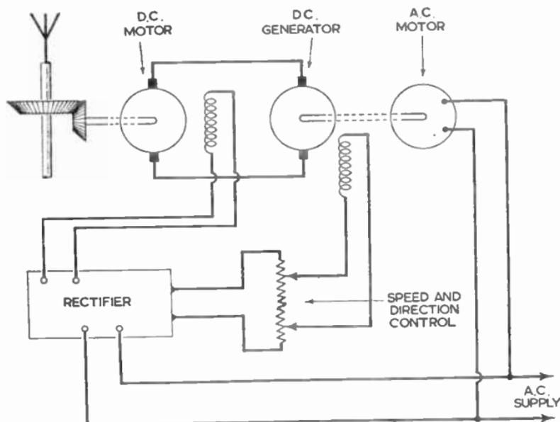
FIG. 38.—SIMPLE AERIAL DRIVING SYSTEM.
