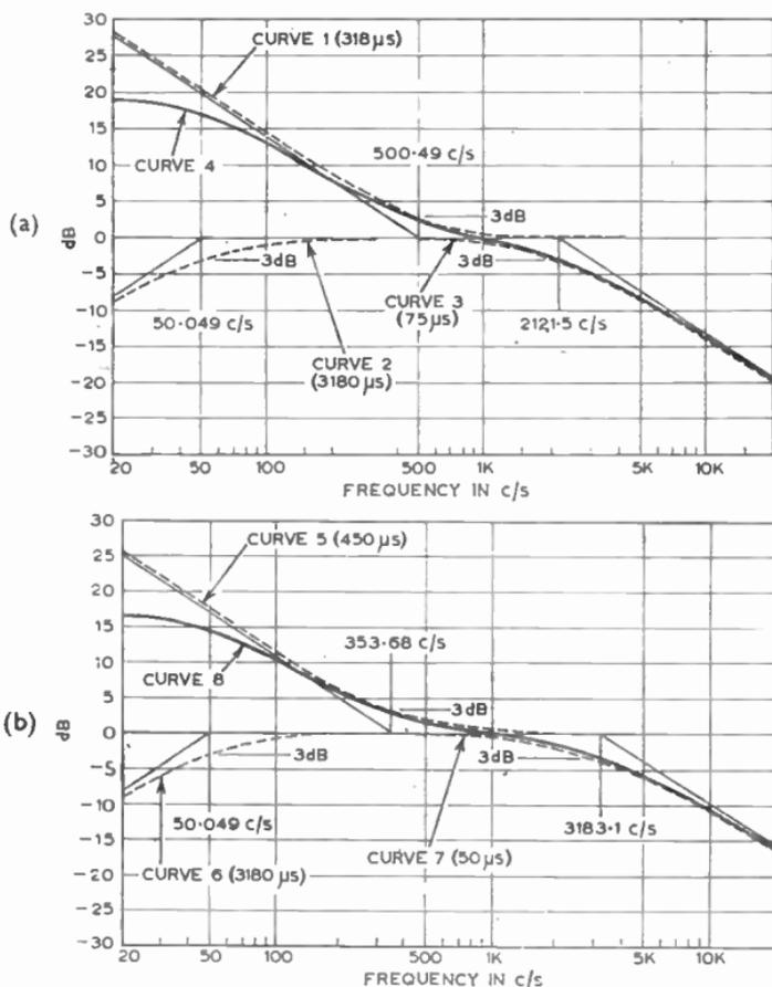
FIG. 15.—STANDARD PLAYBACK RESPONSE CURVES.
