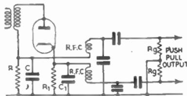
FIG. 5.—DIODE DETECTOR AS PHASE-SPLITTER.
