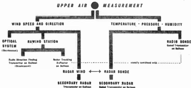
FIG. 47.—METHODS OF UPPER AIR MEASUREMENT.
