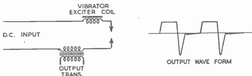
FIG. 12.—BASIC VIBRATOR CIRCUIT.
