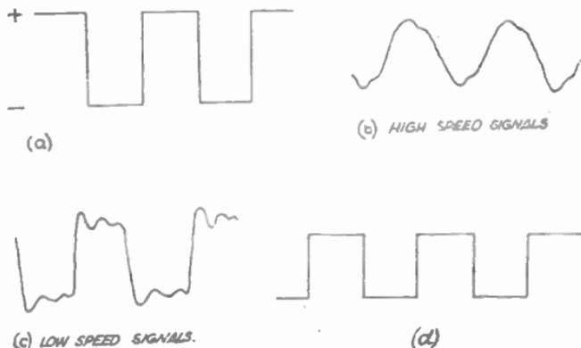
FIG. 17.—WAVEFORMS BEFORE AND AFTER FILTERING.
