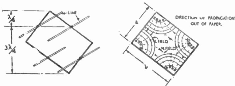
FIG. 9.—DEVELOPMENT OF A WAVE MODE OF HIGHER ORDER IN A RECTANGULAR GUIDE.
