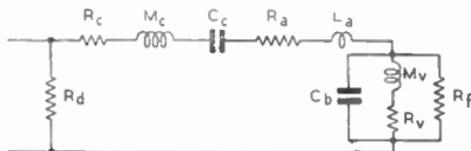
The port provides additional mass loading of the cone, and therefore reduces the effective resonant frequency; but, since the area of the port is small, it will not have sufficient radiation to produce cancellation of this frequency (see "vented enclosures" earlier). This resonance will be fairly well damped.
