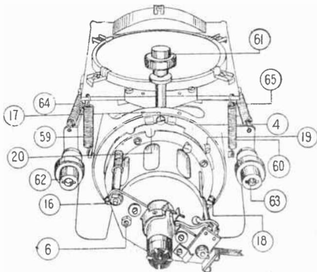
FIG. 12.—ADJUSTMENTS FOR MECHANICAL FOCUSING.
