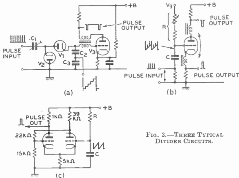
FIG. 3.—THREE TYPICAL DIVIDER CIRCUITS.
