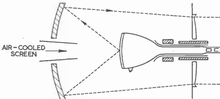
FIG. 2.—SCHMIDT OPTICAL SYSTEM APPLIED TO PROJECTION TELEVISION.
