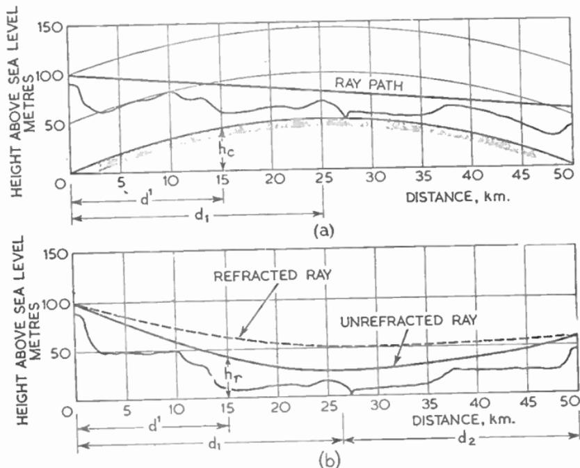
FIG. 33.—CONTOUR ELEVATIONS FOR V.H.F. COMMUNICATION LINKS.
