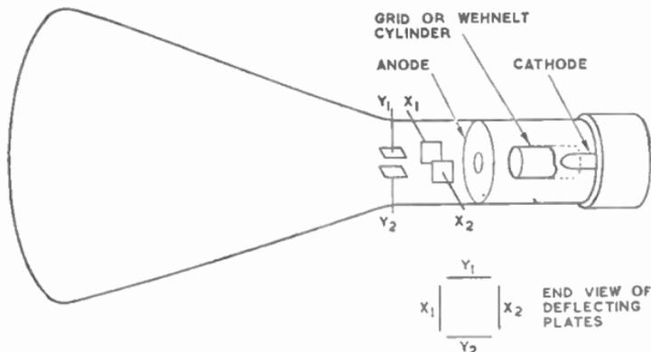
FIG. 1.—SIMPLE GAS-FOCUSED ELECTROSTATIC TUBE.
