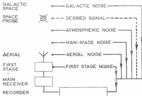
FIG. 30.—SOURCES OF NOISE COMPETING WITH THE DESIRED SIGNAL.
