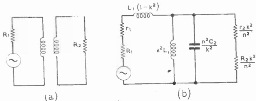
FIG. 5.—EQUALIZATION OF TRANSFORMER PASS-BAND: (a) LOADED TRANSFORMER; (b) EQUIVALENT BAND-PASS CIRCUIT.
