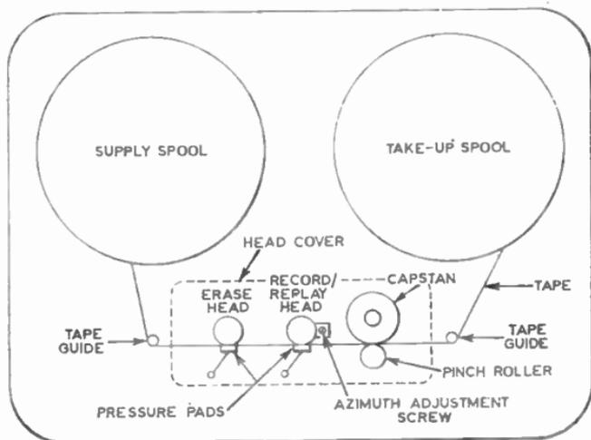
FIG. 23.—LAY-OUT OF TYPICAL TAPE DECK.
