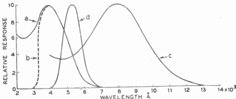
FIG. 12.—RELATIVE RESPONSE TO EQUAL AMOUNTS OF ELECTROMAGNETIC ENERGY OF THE HUMAN EYE AND VARIOUS PHOTOELECTRIC SURFACES.
