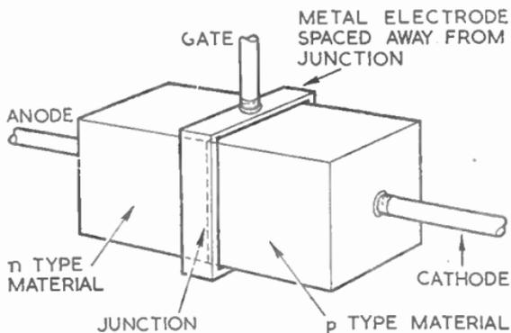
FIG. 18.—DIAGRAMMATIC CONSTRUCTION OF JUNCTION FIELD-ISTOR.
