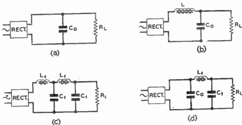
FIG. 108.—RIPPLE REDUCTION FACTOR.
