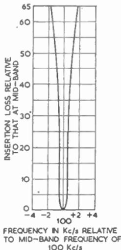
FIG. 22.—CARRIER FILTER RESPONSE CURVES.
