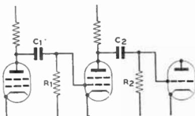
FIG. 34.—TWO-STAGE CIRCUIT WITH STAGGERED TIME CONSTANTS.
