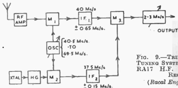
FIG. 9.—TRIPLE CONVERSION TUNING SYSTEM FITTED TO THE RA17 H.F. COMMUNICATIONS RECEIVER.
