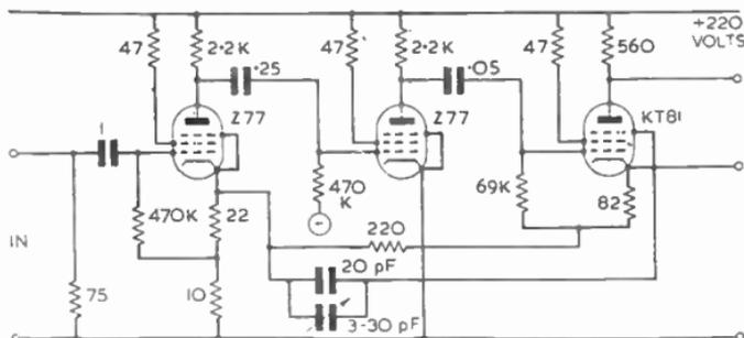
FIG. 30.—EXPERIMENTAL FORM OF TWO-STAGE MAXIMAL AND CRITICAL FEEDBACK AMPLIFIER.
