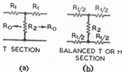
FIG. 39.—T AND BALANCED T ATTENUATORS.
