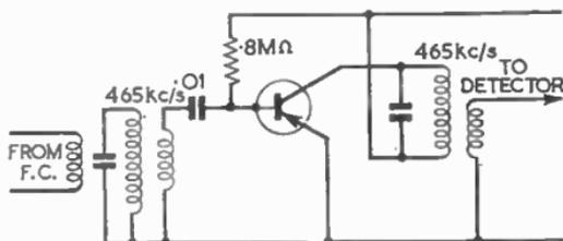
impedance negative, so reducing the damping of the tuned circuit to the point of self-oscillation. Bias is provided through  $R$ , and the blocking capacitor is to prevent damage to the transistor in the event of a short-circuit in  $V_c$ . This type of circuit is valuable to the experimenter who wishes to obtain utmost sensitivity at the expense of critical adjustment. Its use should be restricted to receivers with very small frame or ferrite-rod aeriels.
