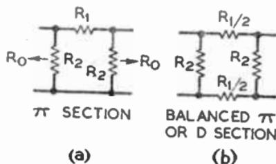
FIG. 40.—pi AND BALANCED pi ATTENUATORS.
