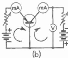
FIG. 24.—(a) COMMON BASE CHARACTERISTICS OF *pn*p JUNCTION TRANSISTOR TYPE EW 53/2. (b) CIRCUIT ILLUSTRATING CURRENT FLOW IN TRANSISTOR IN COMMON BASE ARRANGEMENT.
