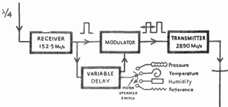
FIG. 50.—BLOCK SCHEMATIC OF THE AIRBORNE RADAR SONDE UNIT.
