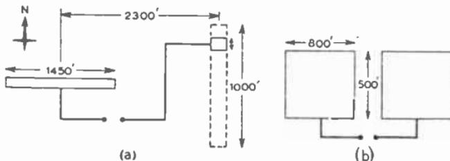
FIG. 26.—(a) PLAN OF THE 178 Mc/s RADIO STAR INTERFEROMETER EMPLOYING APERTURE SYNTHESIS (after Ryle. *Nature*, Vol. 180, 110, 1957).
