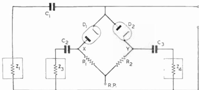
FIG. 60.—GENERALIZED TWO-DIODE CLAMP CIRCUIT.
