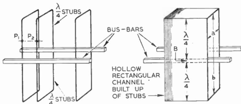
FIG. 4.—RECTANGULAR GUIDE BUILT UP OF TWO PARALLEL BUS-BARS WITH QUARTER-WAVELENGTH STUBS.
