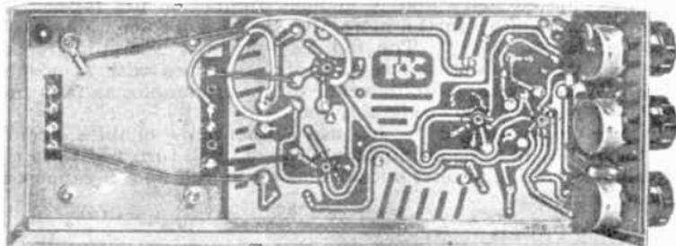
FIG. 9.—A TYPICAL PRINTED CIRCUIT, PREPARED WITH THE STENCIL SHOWN IN FIG. 8.
