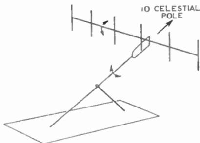
FIG. 9.—YAGI ARRAY IN EQUATORIAL MOUNTING.
