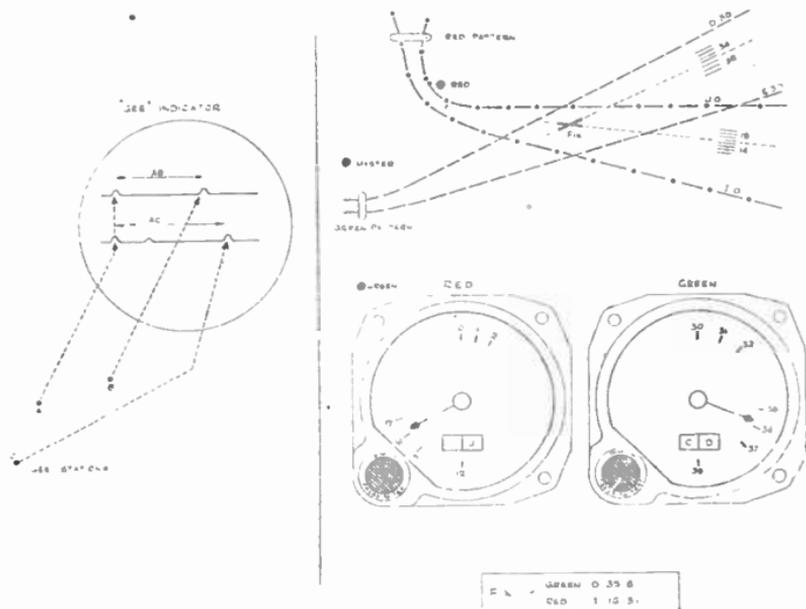
FIG. 7.—COMPARISON OF GEE REPRESENTATION (left) AND DECCA REPRESENTATION (right).
