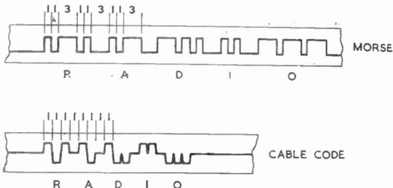
FIG. 77.—RELATIVE LENGTHS OF ELEMENTS IN MORSE AND CABLE MORSE KEYING.
