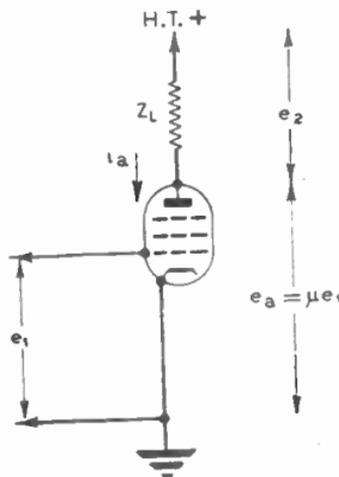
FIG. 57.—VOLTAGE AMPLIFICATION.
