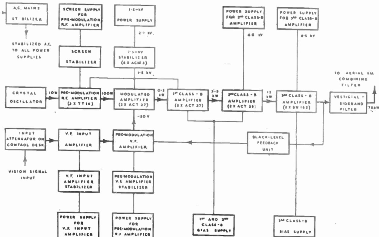
FIG. 5.—BLOCK DIAGRAM OF LOW-LEVEL MODULATED TRANSMITTER.
