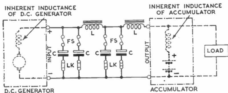
FIG. 41.—MACHINE FILTER.
