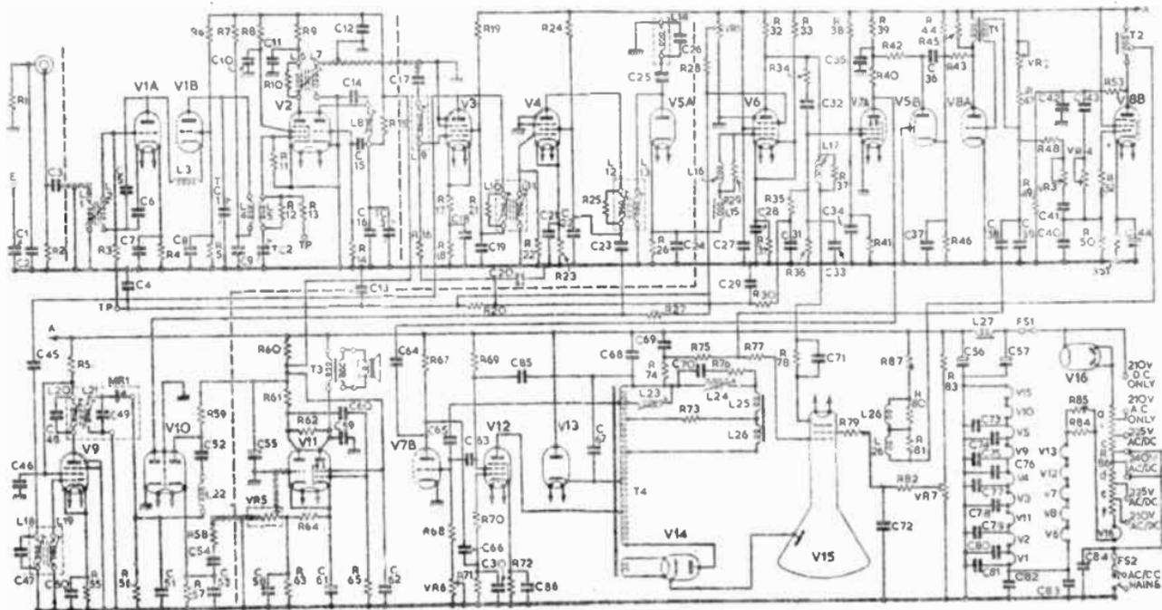
FIG. 1.--REPRESENTATIVE CIRCUIT OF A BAND I/III 17-IN. RECEIVER.
