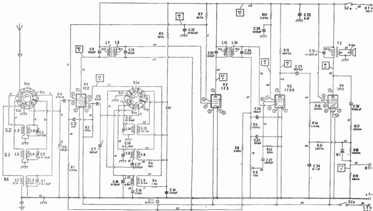
FIG. 19.—FOUR-VALVE, THREE-WAVEBAND RECEIVER WITH BATTERY ECONOMY CIRCUIT.
