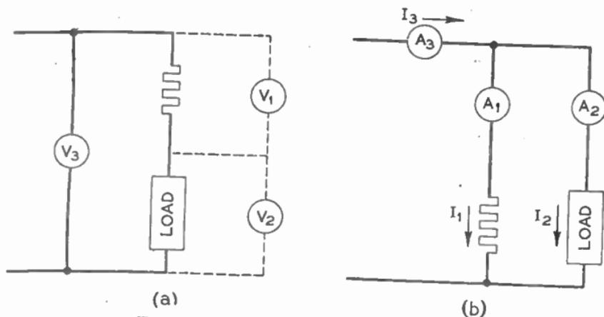
FIG. 102.—MEASUREMENT OF A.C. POWER.
