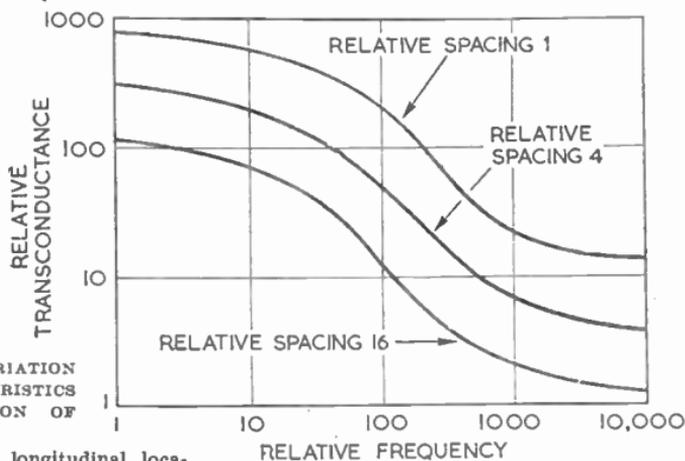
FIG. 19.—VARIATION OF CHARACTERISTICS WITH LOCATION OF GATE.
