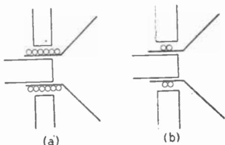
leakage field of the magnet, the flux density of which rapidly decreases as the distance from the gap increases. It has been stated that the force  $F = Bli$ , and therefore if the value of  $B$  varies in the space traversed by the moving coil, the driving force will not always be proportional to the current in the coil, and hence distortion will result.
