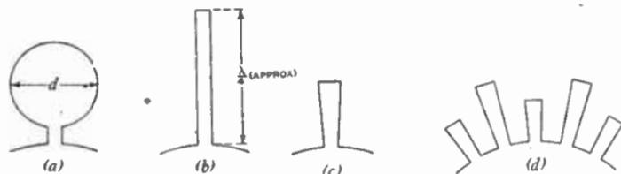
FIG. 20.—MAGNETRON CAVITIES.
