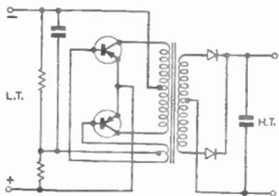
FIG. 48.—TYPICAL PUSH-PULL TRANSFORMER-COUPLED TRANSISTOR H.T. UNIT.
