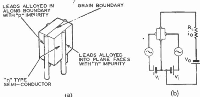
FIG. 21.—(a) GRAIN-BOUNDARY TRANSISTOR; (b) CIRCUIT OF GRAIN-BOUNDARY TRANSISTOR.
