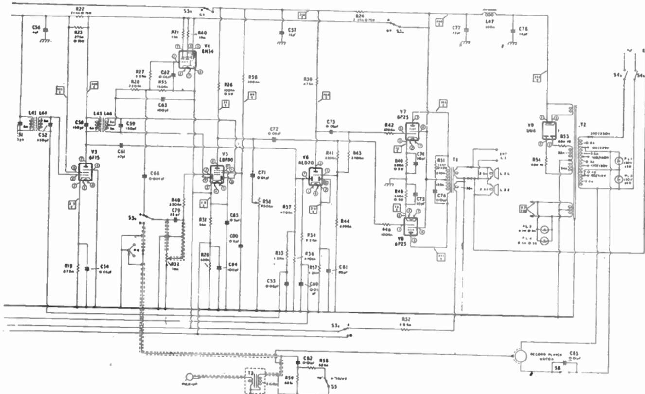
FIG. 24 (b).—INTERMEDIATE- AND AUDIO-FREQUENCY STAGES OF EXPORT RADIOGRAMOPHONE.
