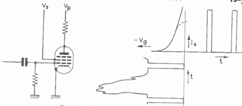
FIG. 28.—SYNCHRONIZING SEPARATOR.
