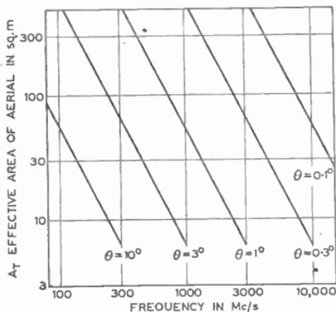
FIG. 34.—RELATIONSHIP BETWEEN  $A_t$ ,  $\theta$  AND FREQUENCY FOR A PENCIL BEAM AERIAL.
