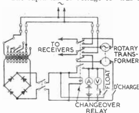
FIG. 11.—METHOD OF PROVIDING AN EMERGENCY A.C. SUPPLY WITH A FLOATING BATTERY.
