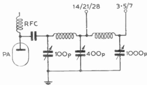
FIG. 2.—MULTI-BAND PI-COUPLING OUTPUT CIRCUIT.
