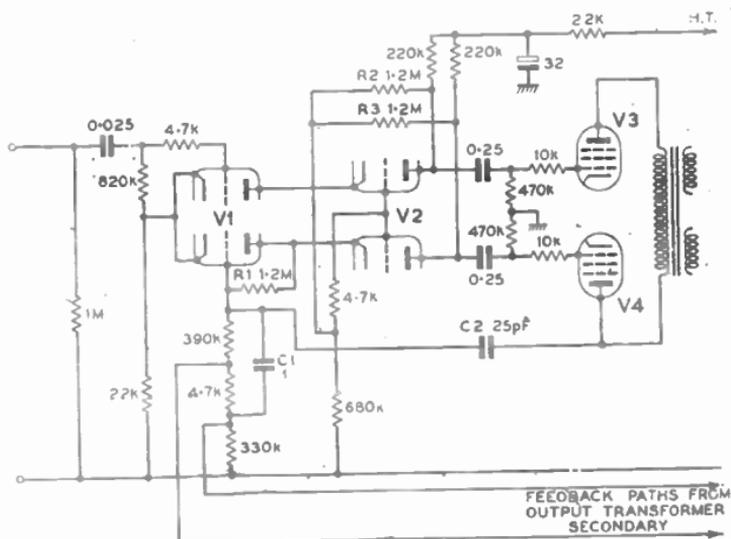
FIG. 11.—PHASE-SPLITTER AND DRIVER STAGES OF A MODERN POWER AMPLIFIER SHOWING USE OF MULTIPLE FEEDBACK PATHS.
