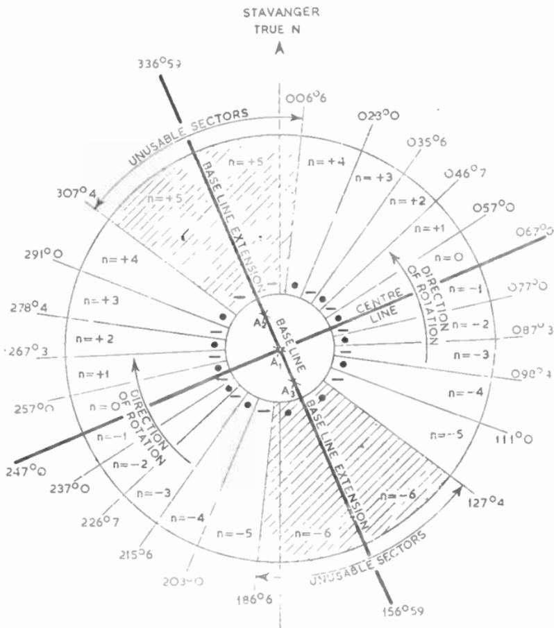
FIG. 10.—TRANSMISSION PATTERN OF THE CONSOL BEACON, AT STAVANGER, NORWAY.
