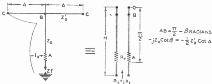
FIG. 8.—TOP-LOADED AERIAL AND EQUIVALENT TRANSMISSION LINE.
