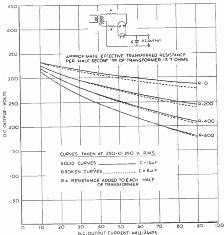
FIG. 16.—CHARACTERISTIC CURVES OF AVERAGE MAZDA VALVE UU6.
