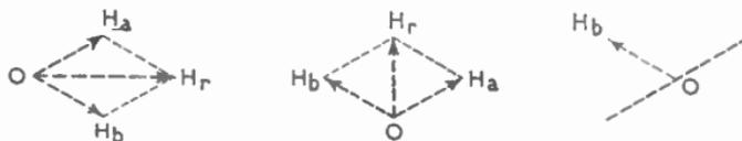
FIG. 13.—SYNTHESIS OF H WAVE FROM TWO PLANE WAVES MOVING DIAGONALLY ACROSS ONE ANOTHER.
