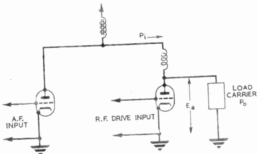
FIG. 75.—MODULATED AMPLIFIER.
