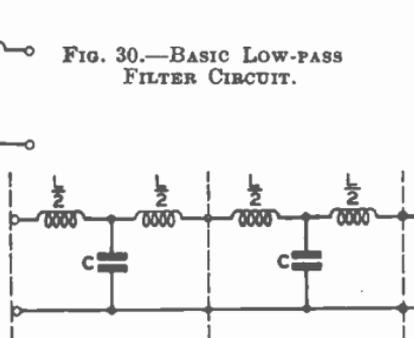
FIG. 30.—BASIC LOW-PASS FILTER CIRCUIT.
