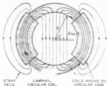
FIG. 16.—TOROIDAL AND CIRCULAR IRON-CORE DEFLECTING COIL.
