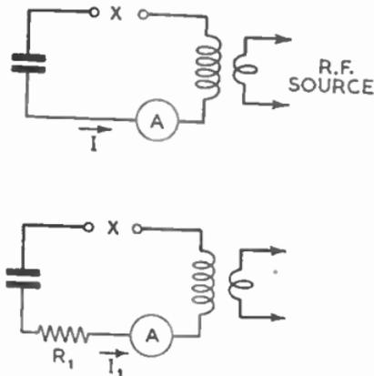
FIG. 133.—MEASUREMENT OF RADIO-FREQUENCY RESISTANCE
