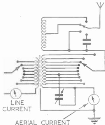
FIG. 15.—SIMPLE AERIAL COUPLING UNIT.
