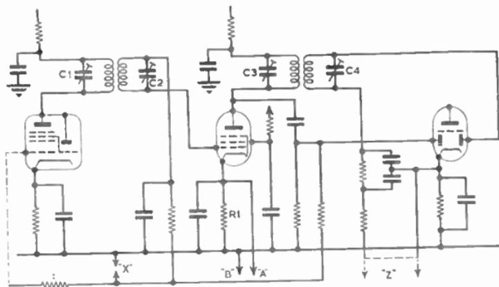
FIG. 10.—INTERMEDIATE-FREQUENCY STAGES OF A TYPICAL BROADCAST RECEIVER.
