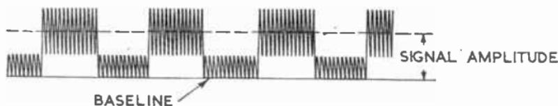
FIG. 25.—SQUARE-WAVE ADJUSTMENT FOR NOISE MEASUREMENTS.
