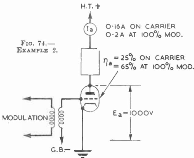
the efficiency falls to 25 per cent and the current to 0.16 ampere. Calculate the anode dissipation under both conditions and the average dissipation, if the average depth of modulation is 30 per cent and the dissipation decreases directly with depth of modulation.
