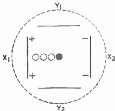
FIG. 2.—A POSITIVE POTENTIAL ON THE  $X_1$  PLATE CAUSES THE ELECTRON BEAM TO SWING TOWARDS THAT PLATE.
