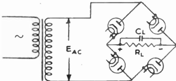
FIG. 11.—BRIDGE CIRCUIT.
