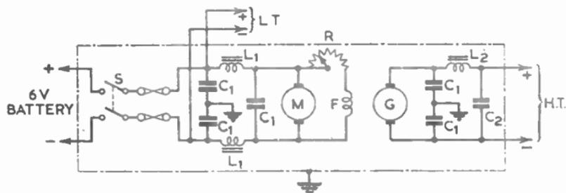
FIG. 18.—ROTARY TRANSFORMER FOR CONVERTING LOW-VOLTAGE D.C. TO HIGH-VOLTAGE D.C.
