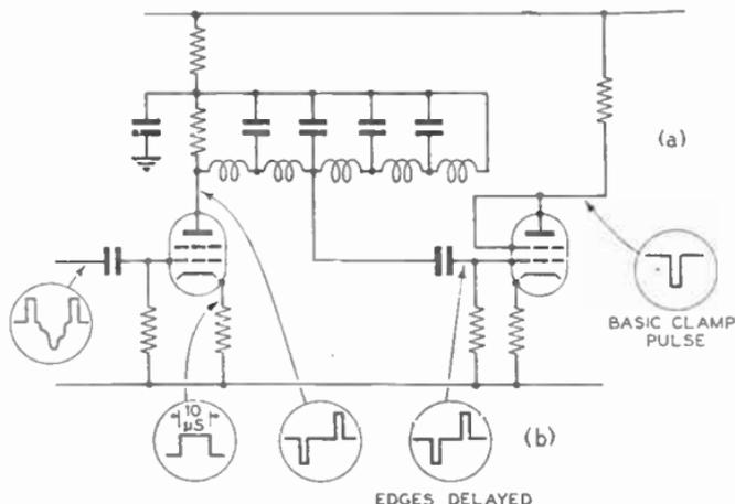
FIG. 64.—BASIC DELAY LINE TYPE CLAMP-PULSE GENERATOR.
