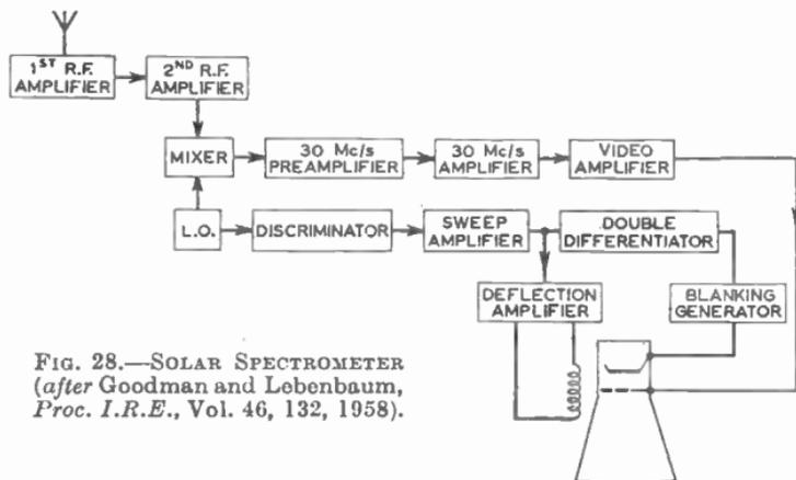
FIG. 28.—SOLAR SPECTROMETER (after Goodman and Lebenbaum, *Proc. I.R.E.*, Vol. 46, 132, 1958).
