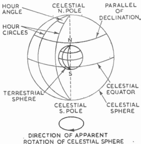
FIG. 29.—DECLINATION AND HOUR ANGLE.
