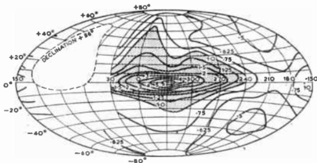
FIG. 31.—DISTRIBUTION OF RADIO BRIGHTNESS OVER THE SKY AT 100 Mc/s. Galactic Co-ordinates. Observations corrected for aerial smoothing. Unit 1000 degrees.
