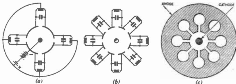
FIG. 19.—DEVELOPMENT OF THE RESONANT-CAVITY MAGNETRON.
