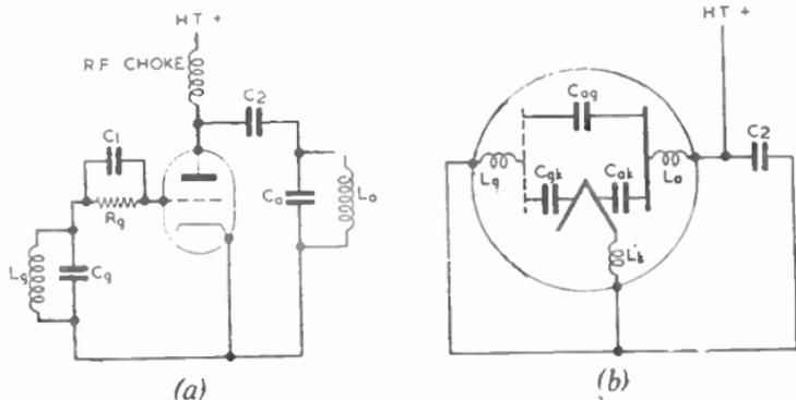
FIG. 13.—EFFECT OF INTERNAL INDUCTANCES AND CAPACITANCES AT VERY HIGH FREQUENCIES.
