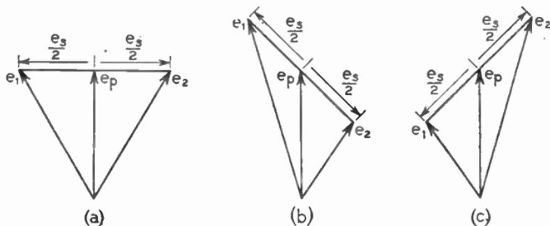
FIG. 36.—VECTOR DIAGRAMS FOR RATIO DETECTOR.
