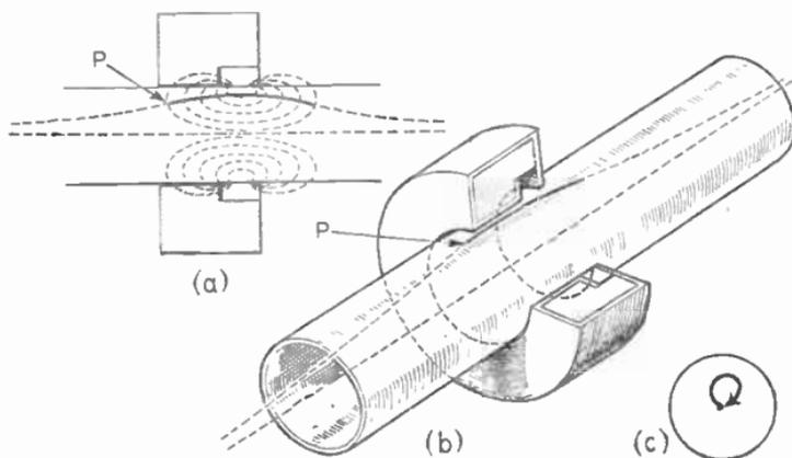
FIG. 8.—FOCUSING BY MEANS OF A SHORT COIL.
