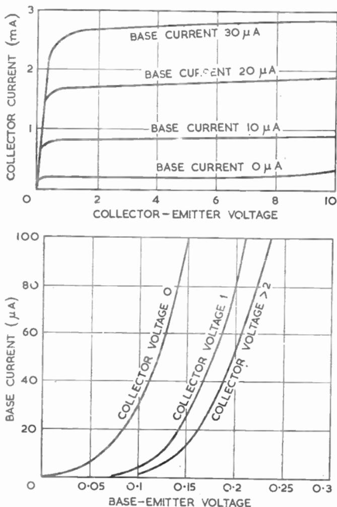
FIG. 9.—TYPICAL STATIC CHARACTERISTICS OF JUNCTION TRANSISTORS.
