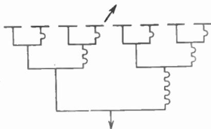
FIG. 8 (right).—BEAM SWINGING BY ALTERING RELATIVE PHASES OF ELEMENTS.
