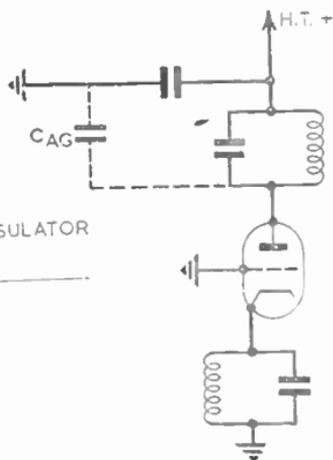
oscillation is described below to illustrate the type of problem which may be encountered. Fig. 11 (a) shows an amplifier stage, and Fig. 11 (b) shows the same circuit including the lead inductances and inter-electrode capacitances. It is seen that at some particular frequency above the working frequency—depending on the component values—the stage may oscillate as a tuned-grid, tuned-anode circuit.
