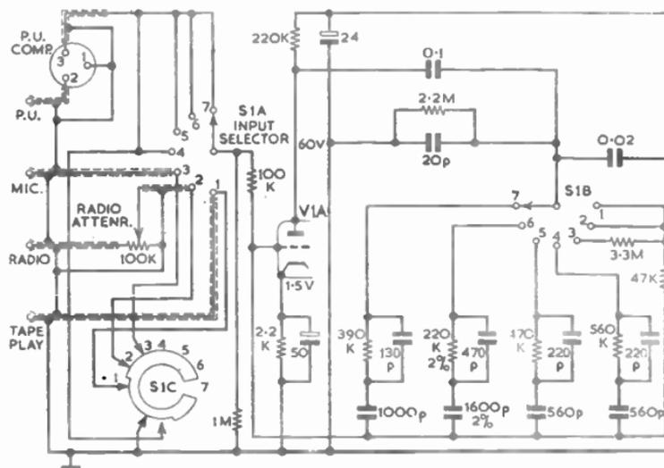
FIG. 14.—INPUT AND EQUALIZING CIRCUIT OF A MODERN PRE-AMPLIFIER. VIA is one section of an ECC40.
