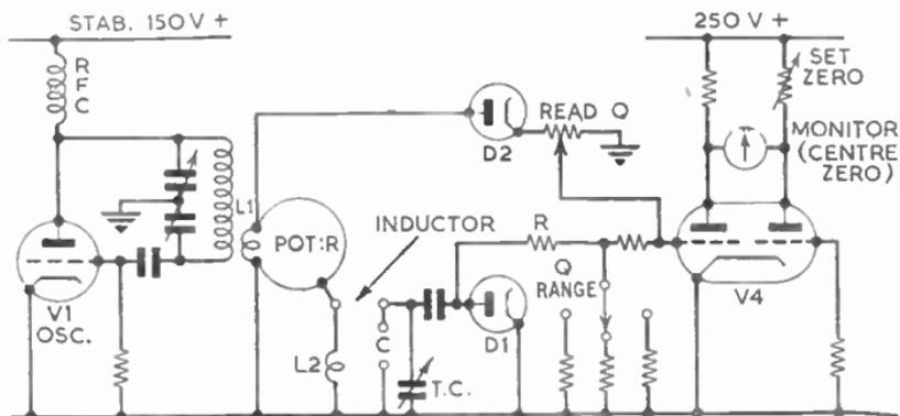
FIG. 27.—V.H.F. Q-METER CIRCUITRY (POWER SUPPLIES OMITTED).
