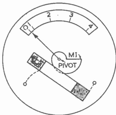
reversal of the actuating torque, it can be used only on a D.C. supply, and care must be exercised to observe the current polarity to its terminals. In its favour are a high degree of accuracy, the linear scale and negligible interference from external fields.
