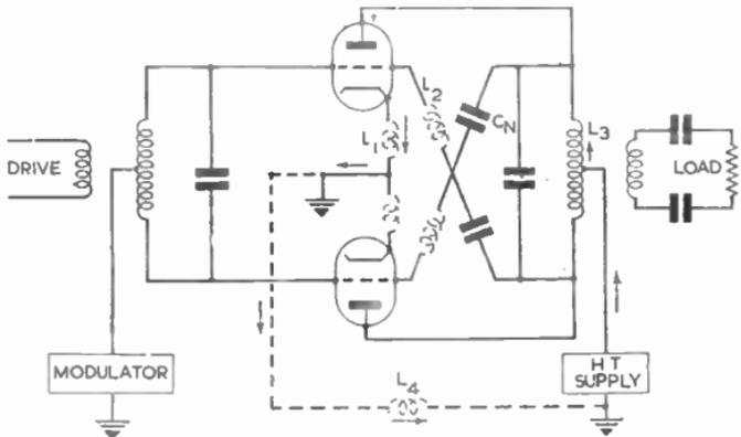
FIG. 10 (b).—SHOWING THE PATH OF VIDEO-FREQUENCY CHANGES OF ANODE CURRENT.
