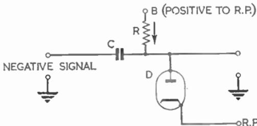
FIG. 57 (b).—(left) IMPROVED D.C. RESTORATION CIRCUIT FOR NEGATIVE PICTURE SIGNALS.
