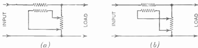
FIG. 13.—SINGLE-PHASE AUTO-TRANSFORMER VOLTAGE REGULATOR WITH BOOSTER TRANSFORMER.
