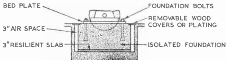
FIG. 15.—METHOD OF ISOLATING FOUNDATION BLOCK.
