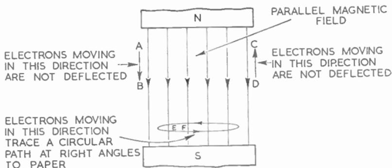
FIG. 12.—ILLUSTRATING THE FORCES ACTING ON ELECTRONS MOVING IN A PARALLEL MAGNETIC FIELD.
