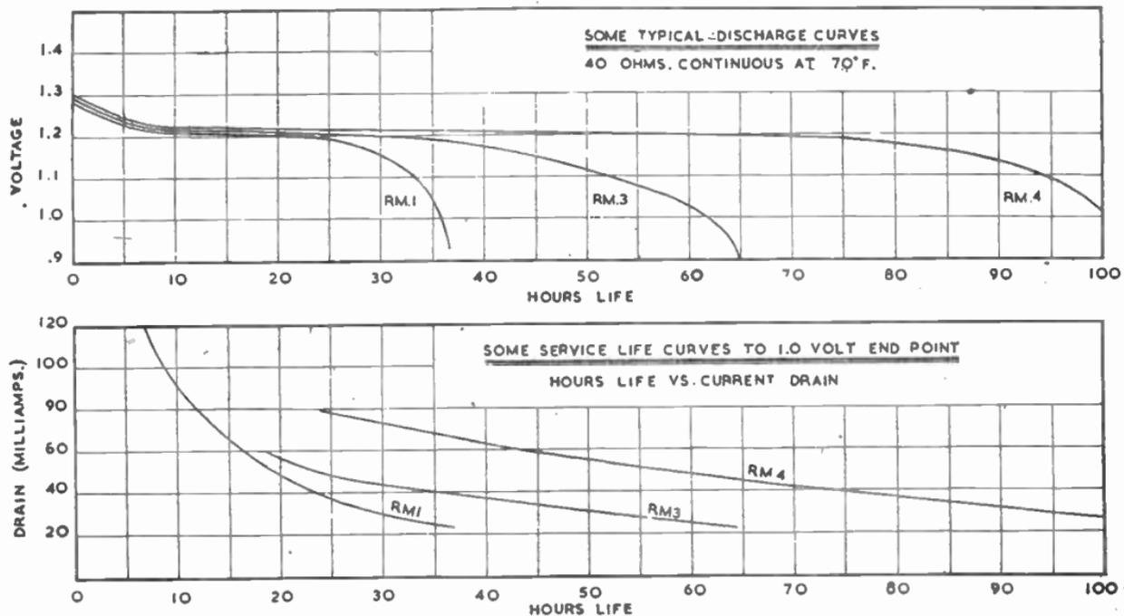
FIG. 9.—THE EFFECT OF SIZE ON THE MALLORY-TYPE DRY CELL.
