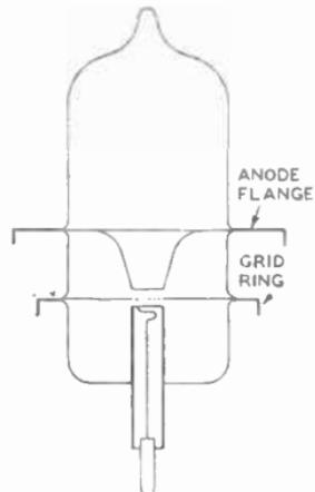
FIG. 17.—FORM OF CONSTRUCTION OF BRITISH DISC SEAL TRIODE.
