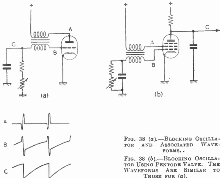
FIG. 38 (a).—BLOCKING OSCILLATOR AND ASSOCIATED WAVEFORMS.
