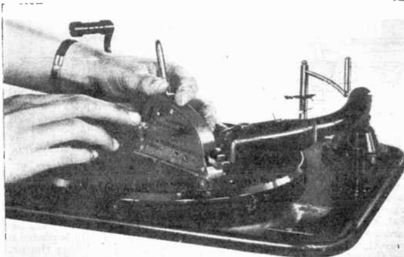
FIG. 17.—CHECKING STYLUS PRESSURE.
