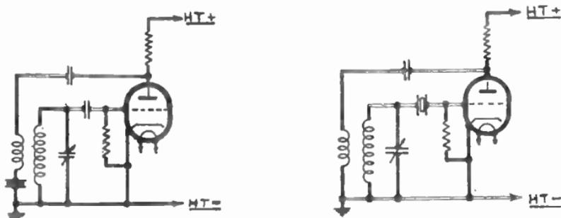
FIG. 14.—SERIES-MODE OSCILLATOR CIRCUITS.
