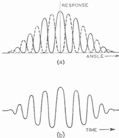
FIG. 19 (right).—(a) RECEPTION PATTERNS OF AN INTERFEROMETER WITH THE AERIALS CONNECTED IN AND OUT OF PHASE. (b) THE RESPONSE OF A PHASE-SWITCHING RECEIVER.
