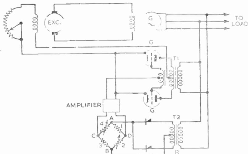
FIG. 17.—THERMIONIC VOLTAGE REGULATOR FOR CONTROL OF ALTERNATOR.
