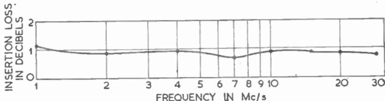
FIG. 9.—AERIAL TRANSFORMER RESPONSE CURVE.
