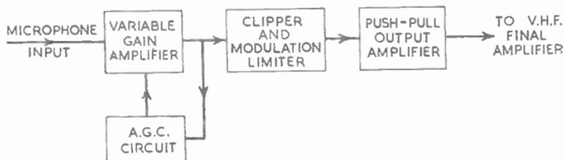
FIG. 20.—BLOCK DIAGRAM OF AN AMPLITUDE MODULATOR.
