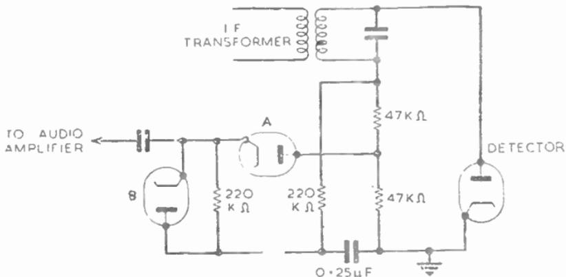
FIG. 28.—PEAK NOISE LIMITER FOR AN A.M. RECEIVER.
