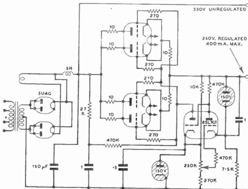
FIG. 69.—SERIES REGULATED POWER SUPPLY.
