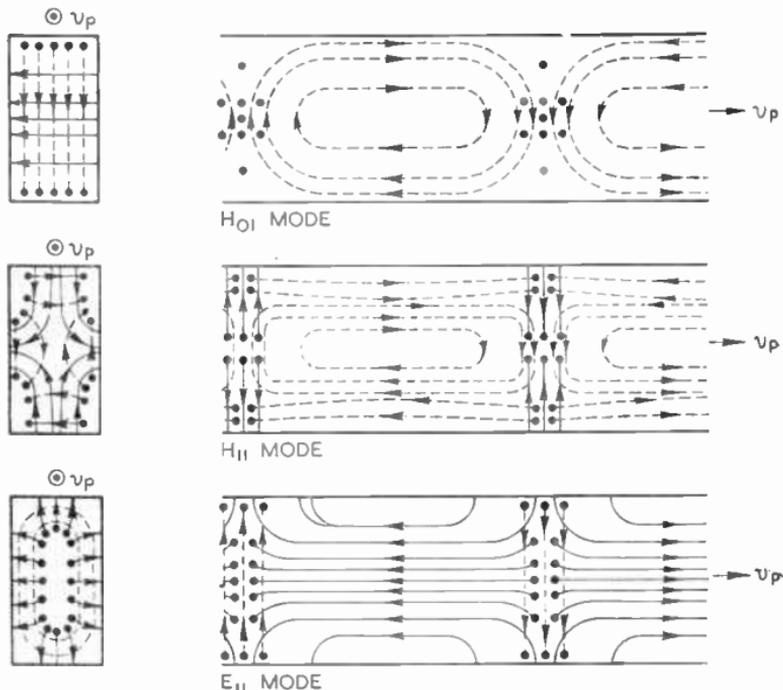
FIG. 19.—Wave Modes in a Rectangular Guide.
