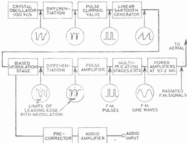
FIG. 36.—THE SERROSSOID SYSTEM OF PRE-CORRECTED PHASE DERIVED FREQUENCY MODULATION.
