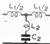
FIG. 45.—SERIES-DERIVED T SECTION.
