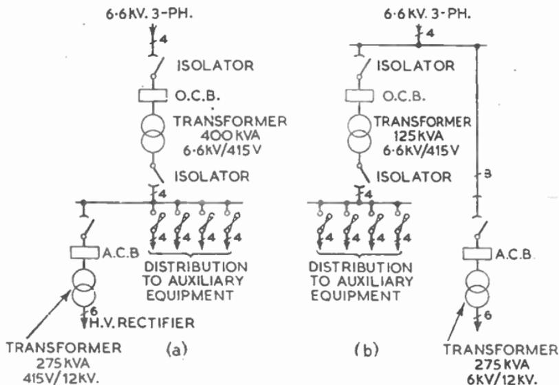
FIG. 6.—TWO TRANSFORMATION SCHEMES FOR HIGH-POWER TRANSMITTING EQUIPMENT.
