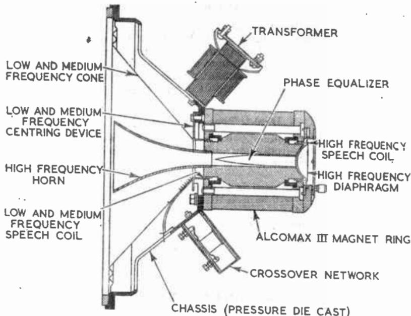
FIG. 12.—DUPLEX TYPE OF LOUDSPEAKER.
