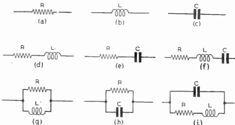
FIG. 8.—RESISTANCES AND REACTANCES IN SERIES AND PARALLEL.
