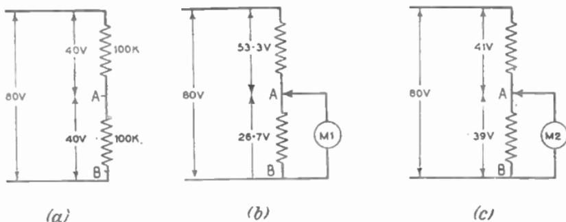
FIG. 1.—EFFECT OF METER RESISTANCE.
