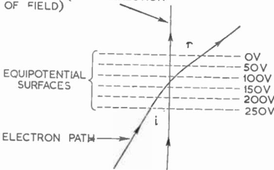
FIG. 6.—PATH TRACED BY AN ELECTRON BEAM ENTERING A PARALLEL ELECTRIC FIELD OBLIQUELY AND TRAVELLING DOWN THE POTENTIAL GRADIENT.
