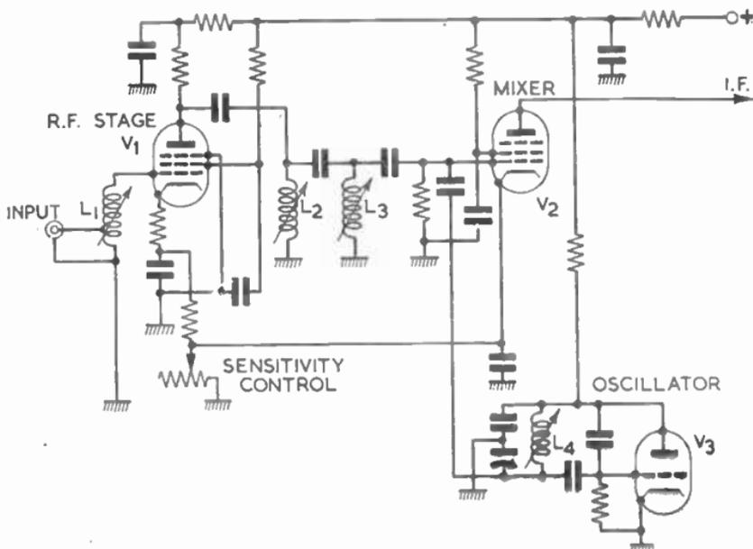
FIG. 11.—TYPICAL "FRONT-END" OF A BAND I RECEIVER.
