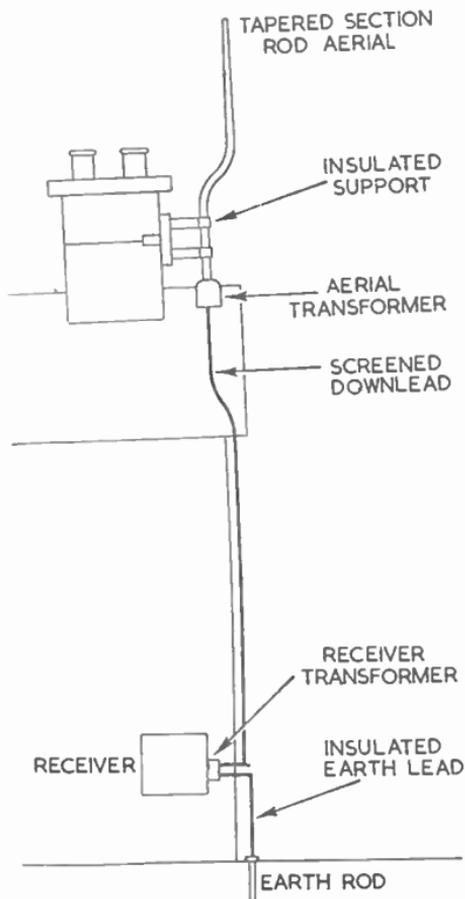
FIG. 4.—AN AERIAL INSTALLATION DESIGNED TO REDUCE NOISE.
