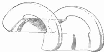
FIG. 18.—ONE SADDLE-SHAPED COIL FROM A DEFLECTING-YOKE.
