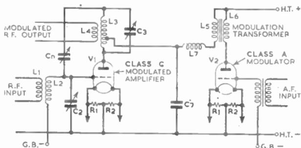
FIG. 19.—ANODE-MODULATION CIRCUIT INCLUDING A MODULATOR TRANSFORMER.
