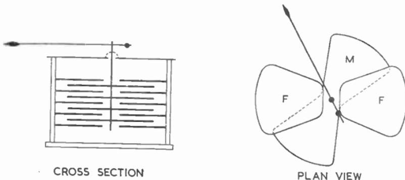
FIG. 7.—ELECTROSTATIC VOLTMETER.
