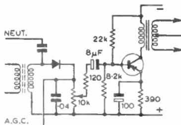
FIG. 42.—TYPICAL DETECTOR AND A.F. DRIVER.
