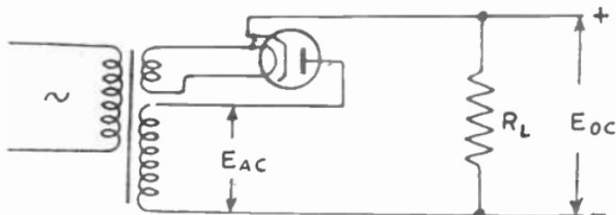
FIG. 7.—HALF-WAVE CIRCUIT WITH RESISTANCE LOAD.
