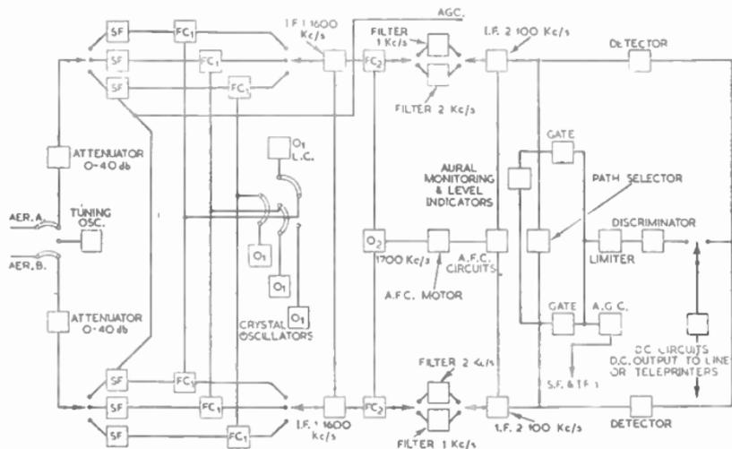
FIG. 11.—SIMPLIFIED BLOCK DIAGRAM OF A TELEGRAPH RECEIVER.
