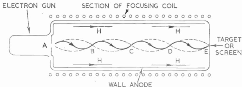
FIG. 14.—ACTION OF A LONG MAGNETIC LENS.
