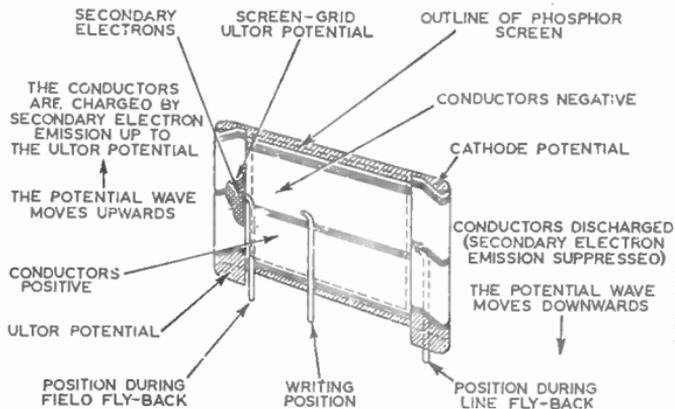
FIG. 13.—THE PRINCIPLE OF SELF-SCANNING BY WRITING BEAM.
