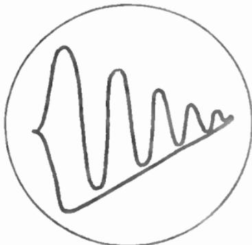
FIG. 14.—OSCILLOSCOPE TRACE WITH CORRECT ADJUSTMENT OF AUDIO-FREQUENCY GENERATOR.
