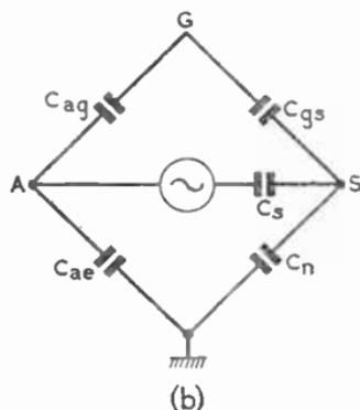
FIG. 34.—I.F. AMPLIFIER NEUTRALIZATION. (a) CIRCUIT; (b) EQUIVALENT BRIDGE CIRCUIT.
