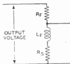
FIG. 22.—FEEDBACK NETWORK WITH INDUCTANCE.
