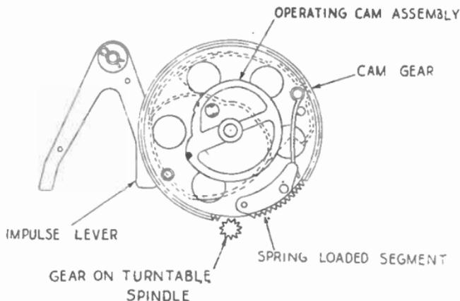
FIG. 14.—CAM GEAR AND DRIVE.
