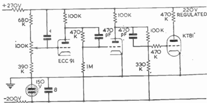
FIG. 70.—SHUNT-REGULATED POWER SUPPLY.
