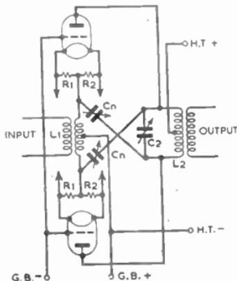
FIG. 15.—SIMPLIFIED CIRCUIT DIAGRAM OF TRANSMITTER RADIO-FREQUENCY STAGE USING TWO NEUTRALIZED INVERTED AMPLIFIERS IN PUSH-PULL.
