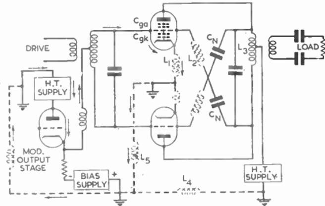
FIG. 10 (a).—SHOWING PATH OF TRANSMITTER GRID CURRENT (FOR ONE VALVE ONLY) AND THE IMPEDANCES IN THE PATH OF THE VIDEO FREQUENCY CURRENT.
