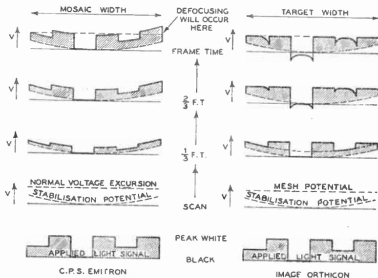
FIG. 28.—BUILD-UP OF THE CHARGE IMAGE.
