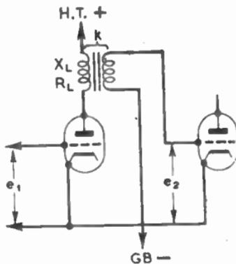
FIG. 62.—TRANSFORMER COUPLING.
