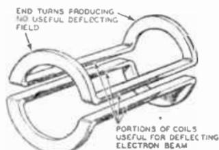
FIG. 19.—AIR-CORE COILS FOR TELEVISION. A FURTHER SET OF COILS IS SUPERIMPOSED AT RIGHT-ANGLES, AND THE ASSEMBLY SURROUNDED BY IRON WIRE.
