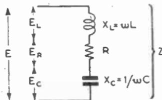
FIG. 28.—SERIES RESONANT CIRCUIT.
