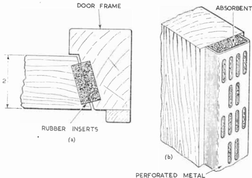
FIG. 1.—MEANS OF OBTAINING ACOUSTICALLY SEALED DOORWAYS.
