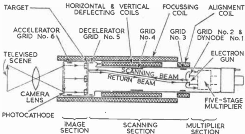
FIG. 19.—THE IMAGE ORTHICON CAMERA TUBE.
