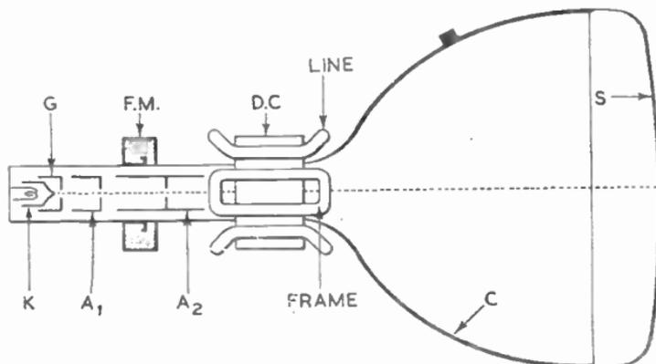
FIG. 6.—ARRANGEMENT OF A TYPICAL TETRODE PICTURE TUBE.
