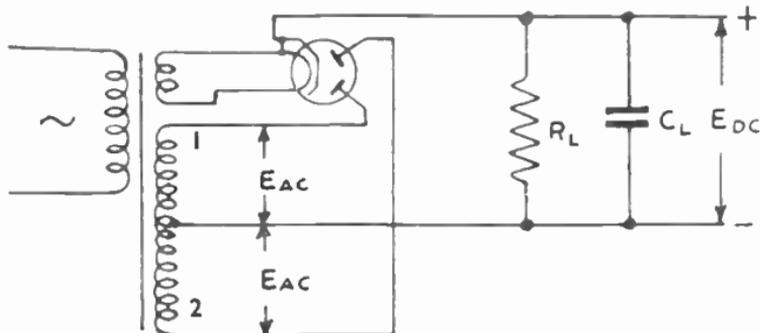
FIG. 10.—FULL-WAVE CIRCUIT WITH RESERVOIR CAPACITOR.
