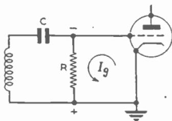
FIG. 29.—LEAKY GRID METHOD OF BIASING.
