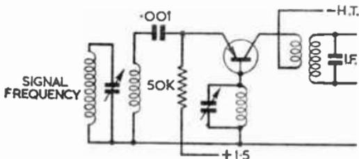
FIG. 36.—POINT-CONTACT TRANSISTOR USED AS A FREQUENCY CHANGER.
