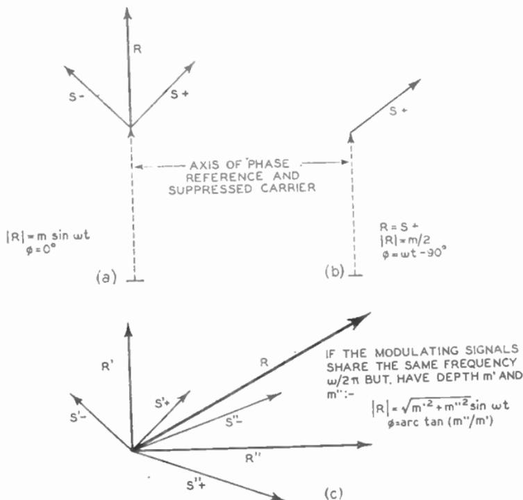
FIG. 23.—METHODS OF MODULATION.
