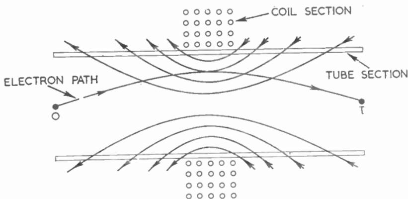
FIG. 15.—LONGITUDINAL SECTION THROUGH A TUBE WITH A SHORT MAGNETIC LENS SHOWING FIELD AND A TYPICAL ELECTRON PATH.
