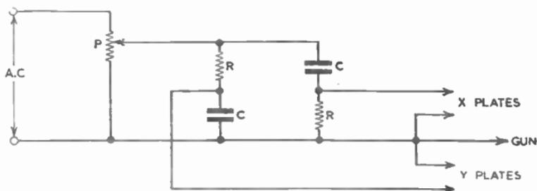
FIG. 46.—ESSENTIALS OF A CIRCULAR TRACE CIRCUIT.
