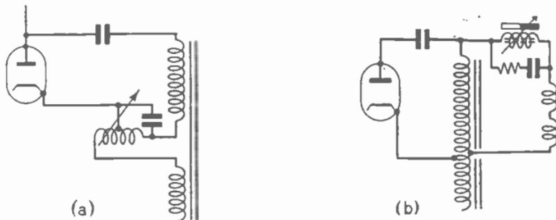
FIG. 46.—LINEARITY CORRECTION WITH BOOSTER DIODE.
