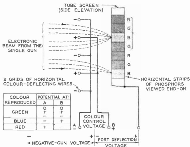
FIG. 22.—ONE-GUN DISPLAY TUBE USING COLOUR SELECTION BY DEFLECTION SWITCHING.
