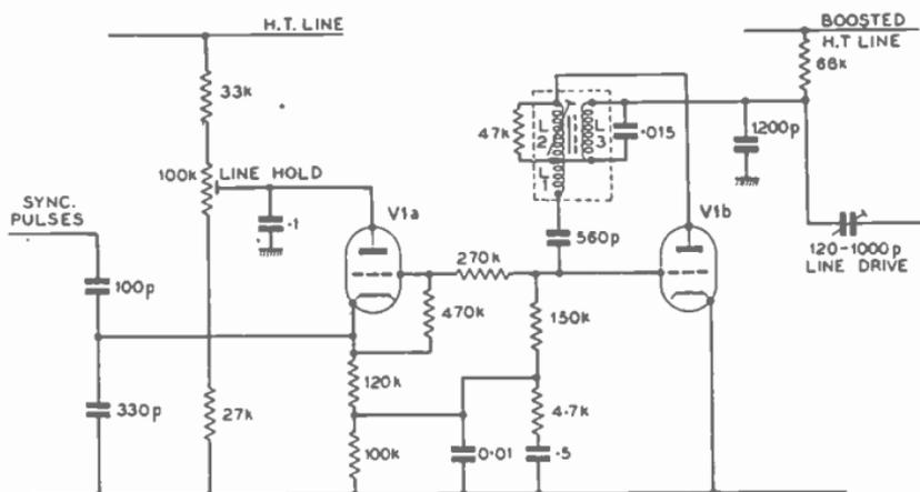
FIG. 37.—USE OF A TRIODE COMPARATOR VALVE ("SYNCHROGUIDE").
