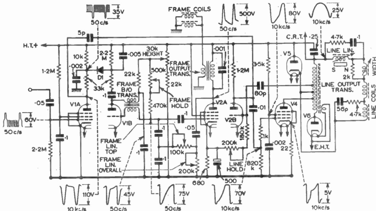
FIG. 11.—THE TIME-BASES OF A TYPICAL MODERN RECEIVER SHOWING THE WAVEFORMS TO BE EXPECTED AT VARIOUS POINTS.
