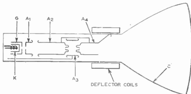
FIG. 7.—TYPICAL TELEVISION TUBE EMPLOYING ELECTROSTATIC FOCUSING.
