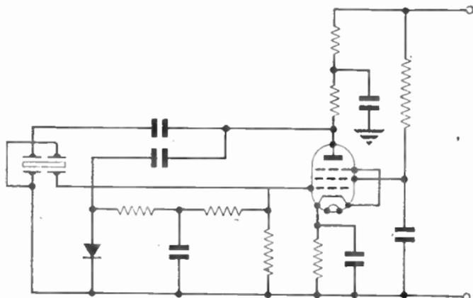
FIG. 17.—FORM OF OSCILLATOR USED FOR FLEXURAL CRYSTALS.
