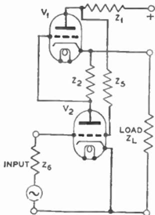
FIG. 42.—DOUBLE-SHUNT-REGULATED AMPLIFIER.
