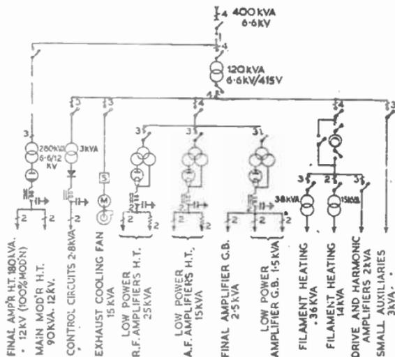
FIG. 4.—POWER DISTRIBUTION DIAGRAM FOR 150-kW M.F. BROADCAST TRANSMITTER.
