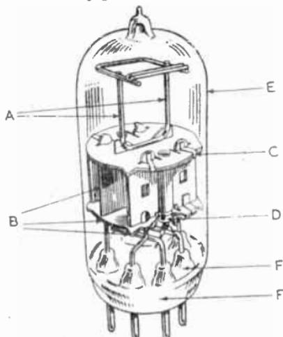
FIG. 11.—CONSTRUCTIONAL FEATURES OF A TYPICAL SPECIAL SERVICE VALVE.
