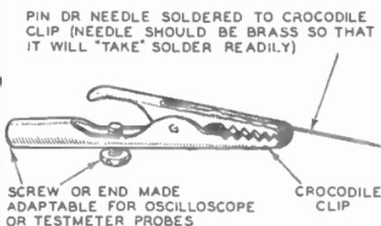
FIG. 16 (left).—DETECTION OF HAIR-LINE CRACKS.
