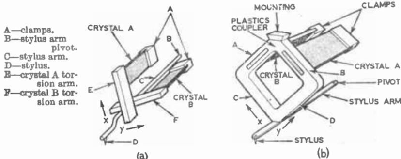
FIG. 15.—CRYSTAL STEREO PICK-UPS.
