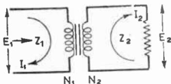
FIG. 113.—EQUIVALENT IMPEDANCE OF TRANSFORMER.
