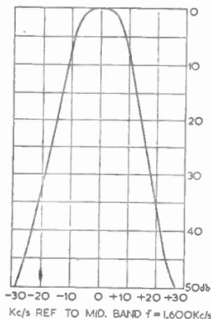
FIG. 14 (above).—TELEGRAPH RECEIVER FIRST INTERMEDIATE-FREQUENCY RESPONSE CURVE.
