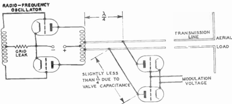
FIG. 8 (a).—ARRANGEMENT FOR ABSORPTION MODULATION.
