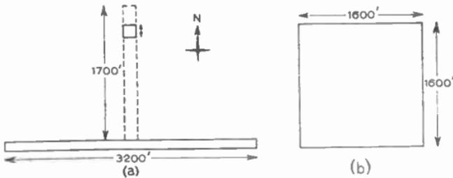
FIG. 27.—PLAN OF 38 Mc/s AERIAL PRODUCING  $1^\circ$  "PENCIL BEAM" BY APERTURE SYNTHESIS (after Ryle, *Nature*, Vol. 180, 110, 1957).
