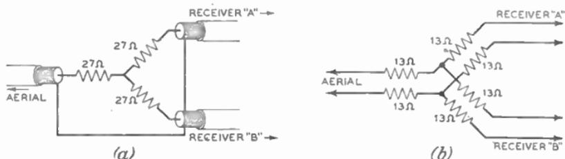
FIG. 14.—STAR NETWORKS: (a) CO-AXIAL FEEDER; (b) TWIN FEEDER.
