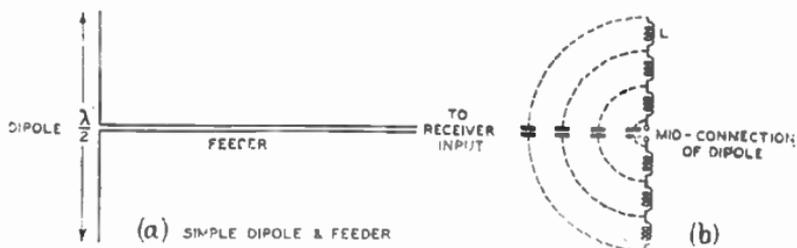
FIG. 12.—HALF-WAVE DIPOLE.
