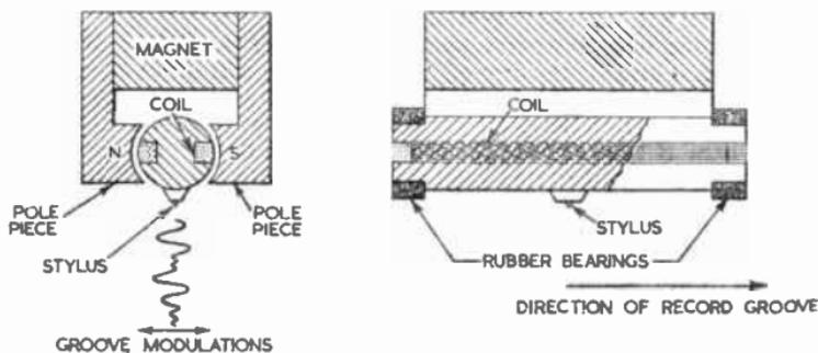
FIG. 16.—THE "LONG COIL" MOVING-COIL PICK-UP.
