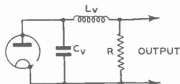
FIG. 3.—NOISE-DIODE EQUIVALENT CIRCUIT ILLUSTRATING EFFECT OF LEAD INDUCTANCE AND INTER-ELECTRODE CAPACITANCE.
