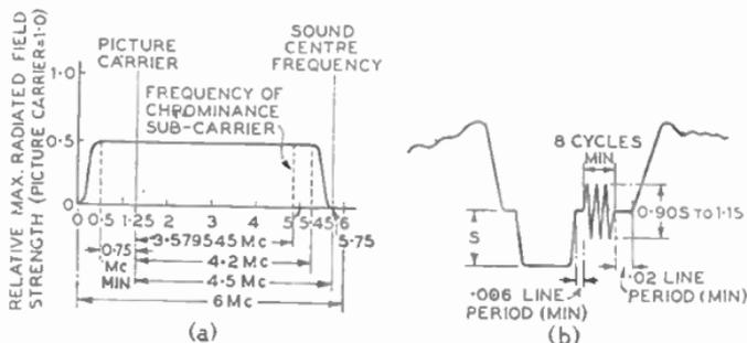
FIG. 71.—(a) N.T.S.C. IDEALIZED PICTURE TRANSMISSION AMPLITUDE CHARACTERISTIC; (b) N.T.S.C. LINE-SYNCHRONIZATION PULSE.
