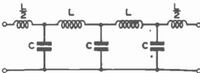
FIG. 31.—T-SECTION LOW-PASS FILTER CIRCUIT.
