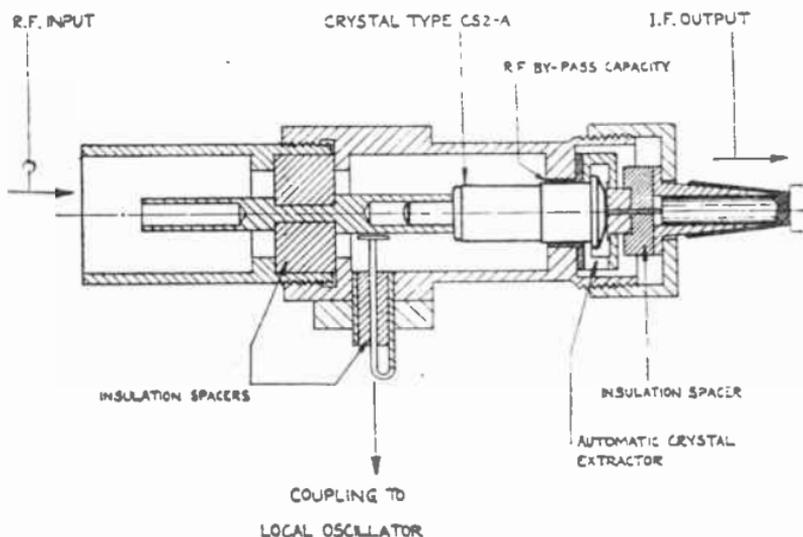
FIG. 9.—B.T.H. CS2-A RECTIFIER USED AS A MIXER.
