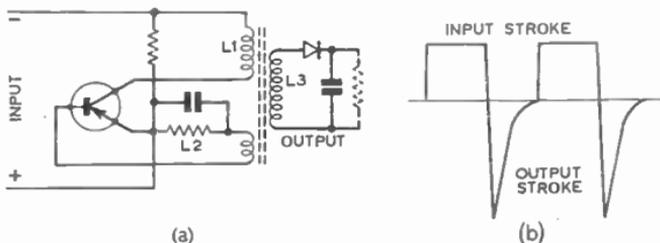
FIG. 20.—RINGING CHOKe D.C. CONVERTER.
