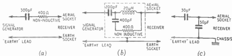
FIG. 11.—DUMMY AERIAL ARRANGEMENTS FOR RADIO-FREQUENCY ALIGNMENT.
