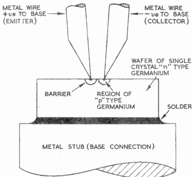
FIG. 1.—CONSTRUCTION OF POINT-CONTACT TRANSISTOR.
