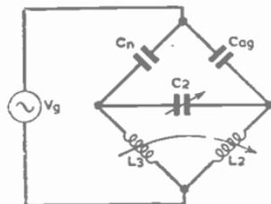
FIG. 13.—CIRCUIT OF FIG. 12 REDRAWN AS A BRIDGE CIRCUIT.
