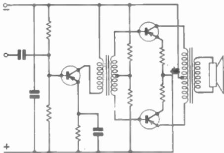
FIG. 50.—A.F. DRIVER AND CLASS B OUTPUT STAGES.
