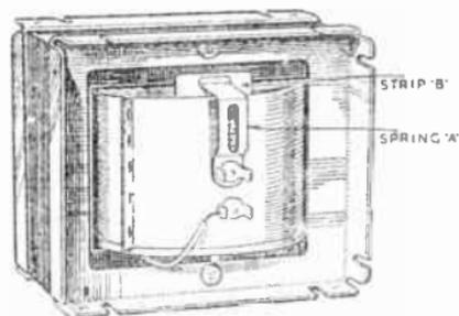
FIG. 9.—TEMPERATURE FUSE FITTED TO A MAINS TRANSFORMER.
