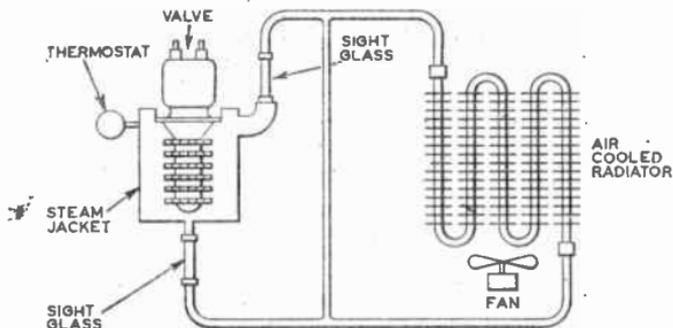
FIG. 26.—VAPOUR-COOLED VALVE SYSTEM.
