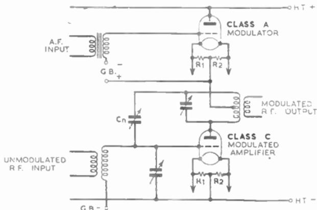
FIG. 24.—BASIC FEATURES OF SERIES MODULATION CIRCUIT.
