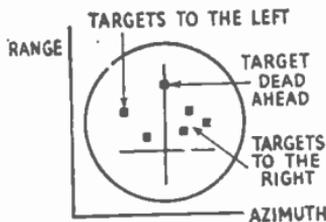
FIG. 23.—APPEARANCE OF THE "B" DISPLAY.
