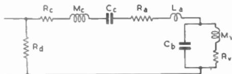
The analogous electrical circuit of a vented enclosure is shown in Fig. 17. If the impedance characteristic of this is plotted, it will be found to correspond to that shown in Fig. 16. The impedance of the parallel section, rising to a maximum at resonance, corresponds to that of the enclosure.
