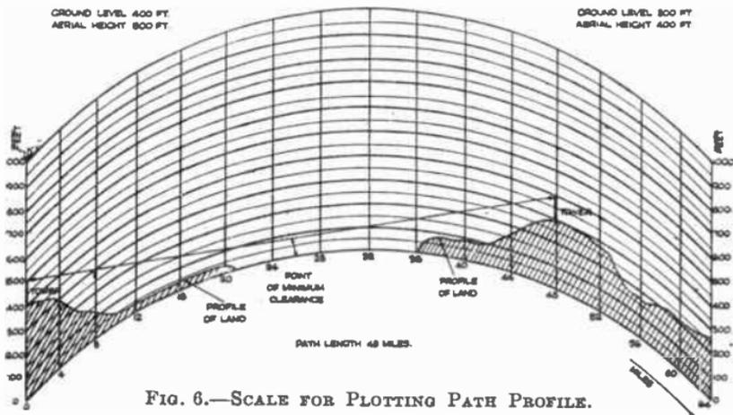
FIG. 6.—SCALE FOR PLOTTING PATH PROFILE.
