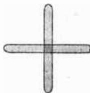
FIG. 21 (right).—THE TWO FAN BEAMS OF A "MILLS CROSS" AERIAL. THE PHASE SWITCHING RECEIVER RESPONDS ONLY TO THE DIAGONALLY-HATCHED REGION OF INTERSECTION.
