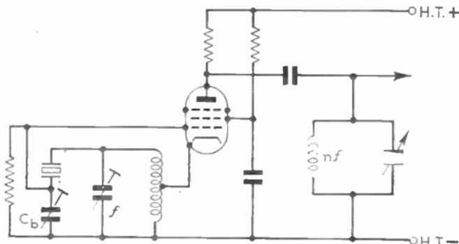
FIG. 18.—OSCILLATOR FOR USE AT OVERTONE FREQUENCIES.
