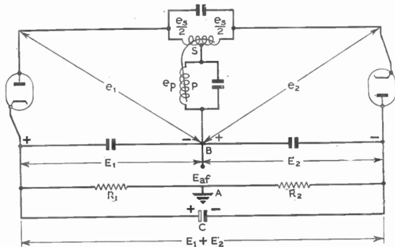
FIG. 35.—BASIC CIRCUIT OF RATIO DETECTOR.
