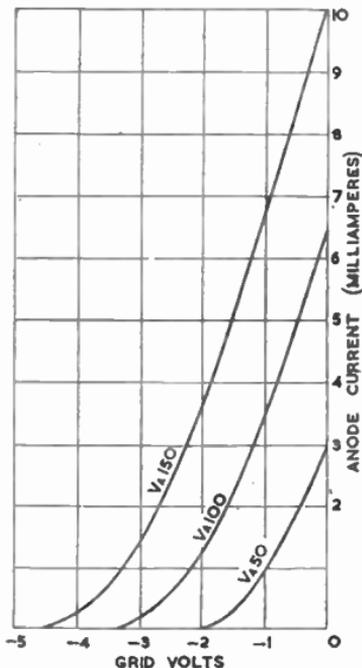
FIG. 7.—CHARACTERISTIC CURVE OF A TYPICAL SMALL TRIODE.
