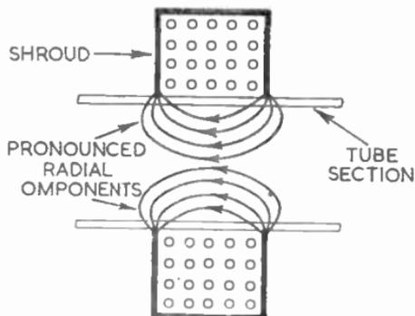
FIG. 17.—CROSS-SECTION OF ONE TYPE OF SHORT MAGNETIC LENS EMPLOYING A PERMANENT MAGNET.
