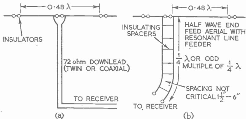
FIG. 6.—HORIZONTAL HALF-WAVE DIPOLE WITH SUITABLE MATCHING.
