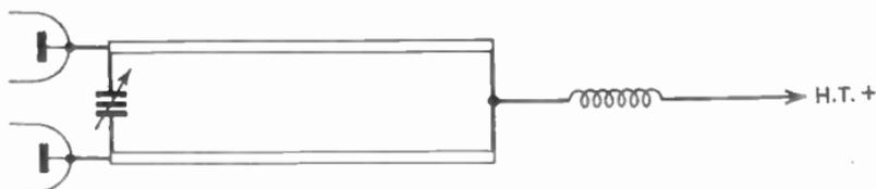
FIG. 9.—PARALLEL LINE WITH TUNING CAPACITANCE.
