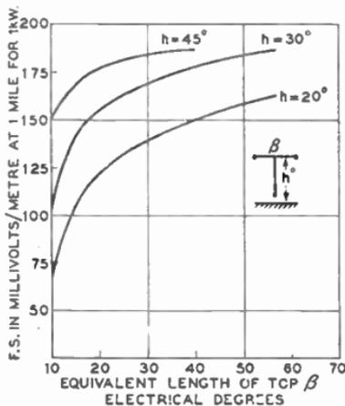
FIG. 10.—SHOWING THE IMPROVEMENT EFFECTED BY TOP CAPACITANCE LOADING OF A LOW AERIAL WITH A POOR EARTH SYSTEM.
