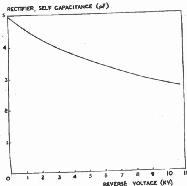
FIG. 22.—VARIATION OF APPARENT SELF-CAPACITANCE OF AN 11-kV TUBULAR E.H.T. RECTIFIER (36EHT130) WITH REVERSE VOLTAGE.
