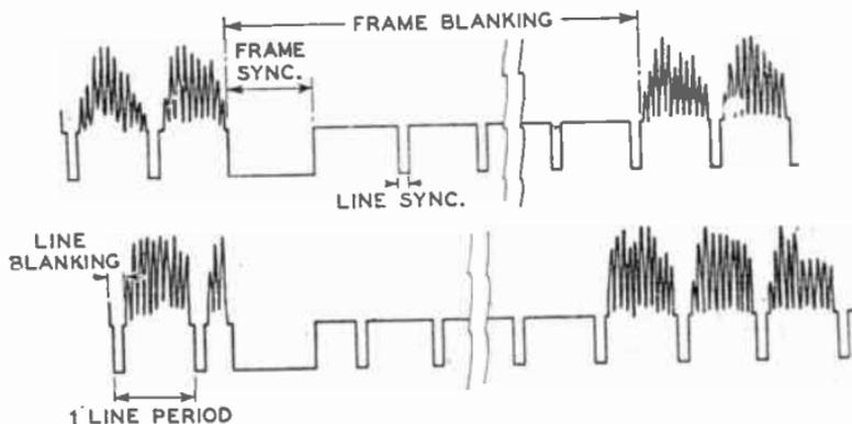
FIG. 1.—TWO SUCCESSIVE FIELDS OF A COMPOSITE WAVEFORM FOR AN INDUSTRIAL TELEVISION EQUIPMENT.
