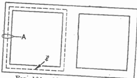
FIG. 121.—MAGNETIC PATH OF CHOKE.
