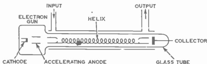
FIG. 25.—TRAVELLING-WAVE AMPLIFIER.
