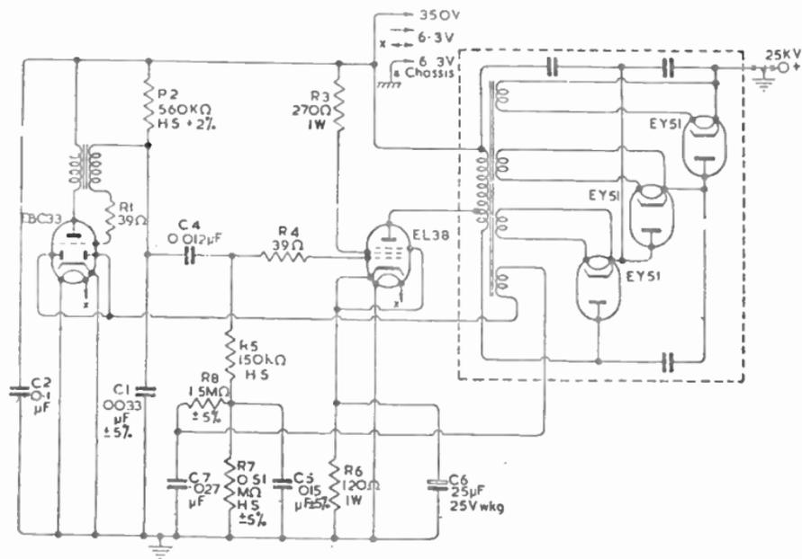
FIG. 11.—TYPICAL E.H.T. UNIT FOR PROJECTION TUBES.
