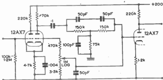
FIG. 22.—CONTINUOUSLY VARIABLE LOW PASS FILTER.
