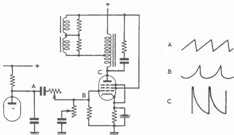
FIG. 42.—LINEARITY CORRECTION SUITABLE FOR A PENTODE VALVE.
