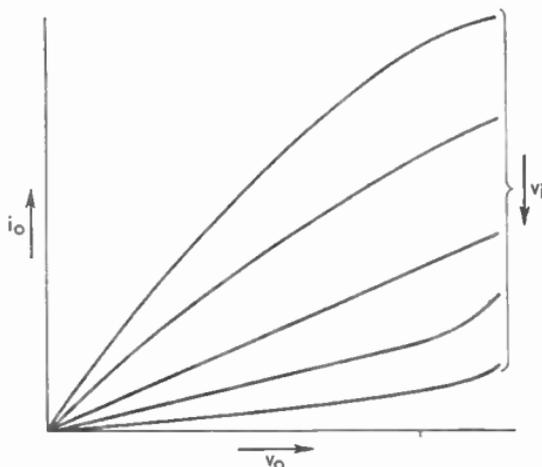
FIG. 22.—CHARACTERISTICS OF GRAIN-BOUNDARY TRANSISTOR.
