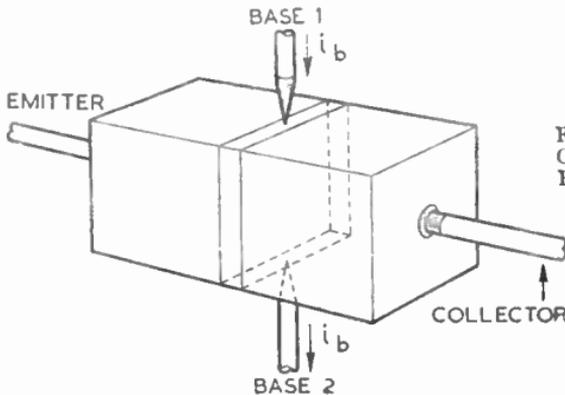
FIG. 13.—DIAGRAMMATIC CONSTRUCTION OF HIGH-FREQUENCY JUNCTION TETRODE.
