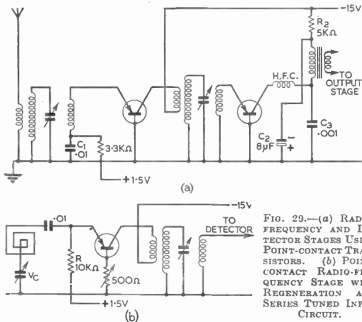
FIG. 29.—(a) RADIO-FREQUENCY AND DETECTOR STAGES USING POINT-CONTACT TRANSISTORS. (b) POINT-CONTACT RADIO-FREQUENCY STAGE WITH REGENERATION AND SERIES TUNED INPUT CIRCUIT.
