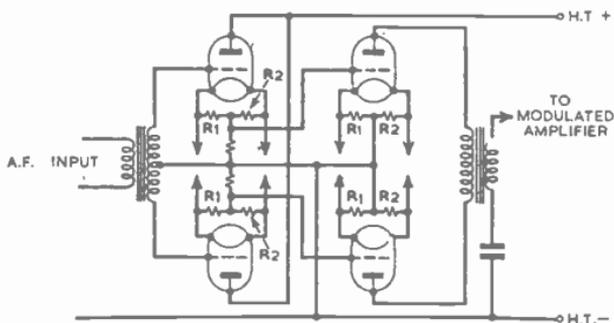
FIG. 21.—CATHODE FOLLOWERS USED AS DRIVERS OF A CLASS B MODULATOR. FOR SIMPLICITY SOURCES OF GRID BIAS ARE IGNORED.
