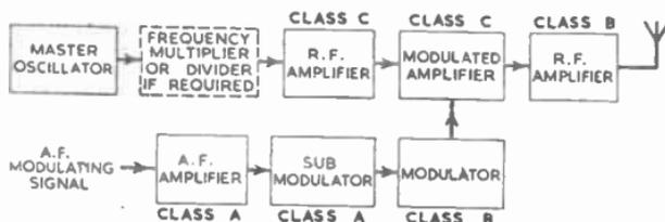
FIG. 16.—BLOCK SCHEMATIC DIAGRAM OF A LOW-POWER MODULATED TRANSMITTER.
