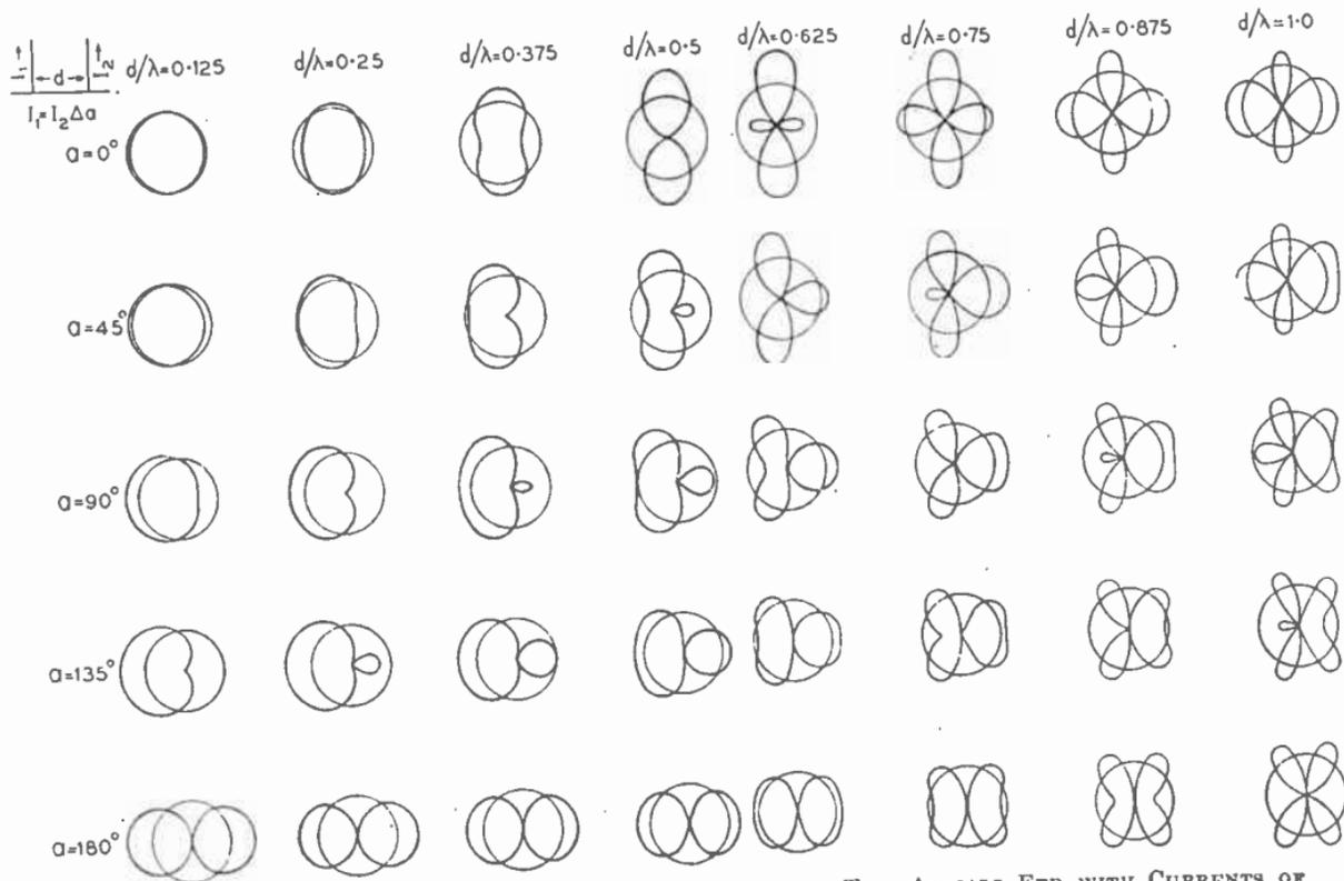
FIG. 14.—HORIZONTAL RADIATION PATTERNS FOR AN ARRAY OF TWO AERIALS FED WITH CURRENTS OF EQUAL MAGNITUDES.
