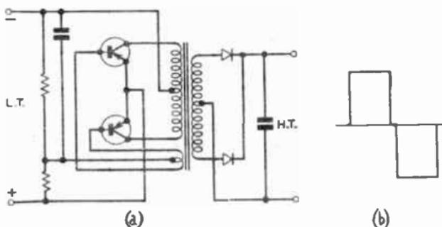
FIG. 21.—PUSH-PULL TRANSFORMER COUPLED D.C. CONVERTER.
