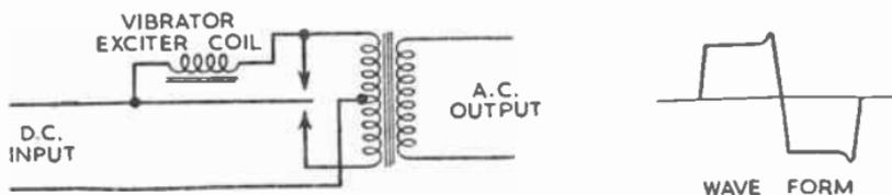
FIG. 13.—TYPICAL VIBRATOR CIRCUIT FOR LOADS UP TO 30 WATTS.
