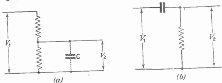
FIG. 45.—ATTENUATING NETWORKS SUBJECT TO FREQUENCY DISTORTION.
