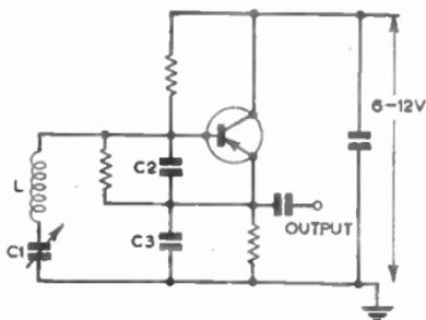
FIG. 7.—TRANSISTOR  $L-C$  OSCILLATOR.
