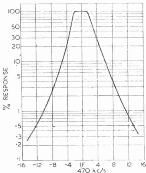
FIG. 7.—TYPICAL PRACTICAL INTERMEDIATE-FREQUENCY RESPONSE CURVE.
