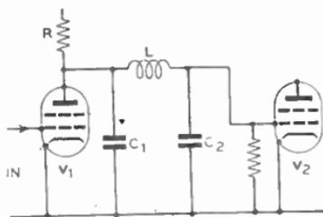
FIG. 19.—SIMPLE FORM OF FOUR-TERMINAL COUPLING NETWORK.
