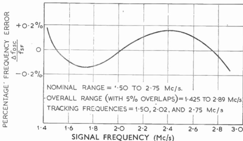
FIG. 4.—OSCILLATOR TRACKING MISMATCHING.
