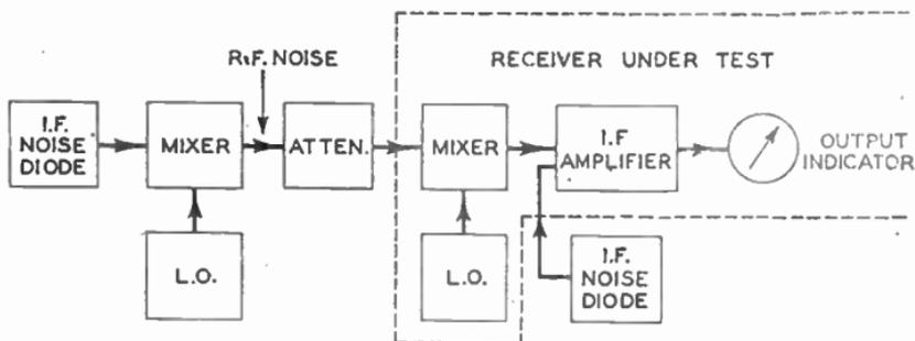
FIG. 6.—USE OF MIXER FOR OBTAINING MICRO-WAVE NOISE FROM AN INTERMEDIATE-FREQUENCY SOURCE.
