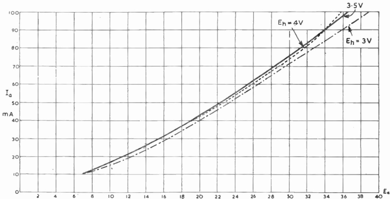
FIG. 2.—TYPICAL ANODE CURRENT/ANODE VOLTAGE CURVES AT LOW VALUES OF HEATER VOLTAGE =  $E_h$ .
