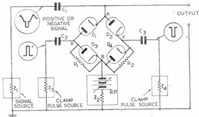
FIG. 59.—GENERALIZED CIRCUIT FOR A DIODE BRIDGE BLACK-LEVEL CLAMP.
