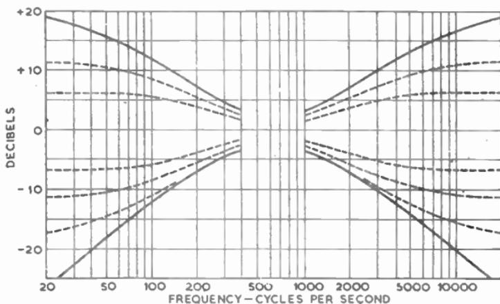
FIG. 16 (top).—FREQUENCY RESPONSE CURVES FOR PASSIVE TONE CONTROL.
