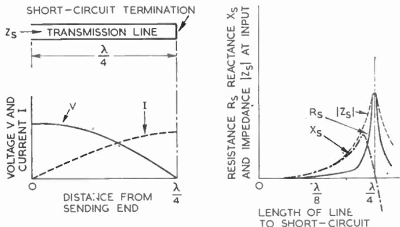
FIG. 3.—QUARTER-WAVELENGTH TRANSMISSION LINE CHARACTERISTICS.
