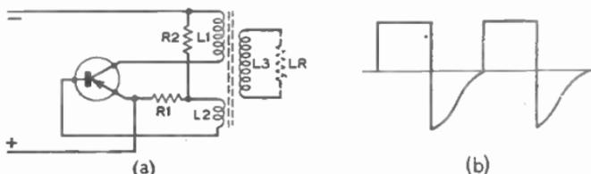
FIG. 19.—TRANSFORMER COUPLED, SINGLE TRANSISTOR D.C. CONVERTER.
