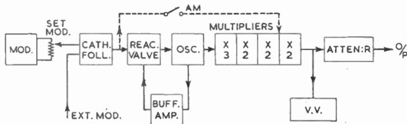
FIG. 22.—BLOCK SCHEMATIC LAYOUT OF AN F.M./A.M. SIGNAL GENERATOR.
