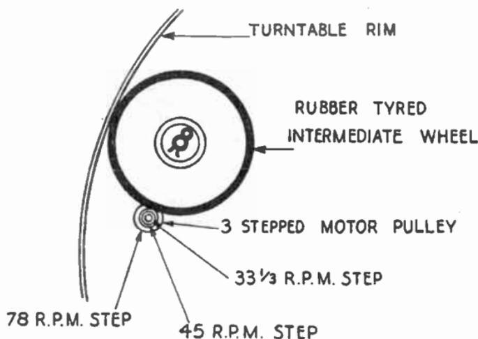
FIG. 4.—THREE-SPEED DRIVE USING STEPPED MOTOR PULLEY.
