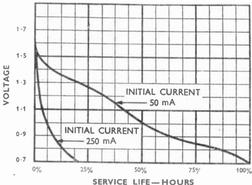
FIG. 5.—THE BEARING OF THE DISCHARGE RATE OF A BATTERY ON ITS LIFE.
