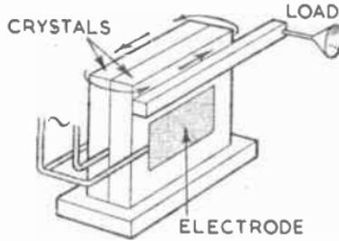
FIG. 3.—CRYSTAL LOUDSPEAKER.
