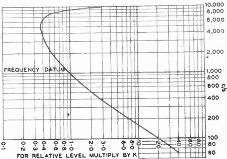
FIG. 44.—C.C.I.F. "WEIGHTING" CURVE FOR COMMUNICATION SYSTEM.
