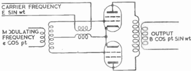
FIG. 35.—BALANCED MODULATOR.
