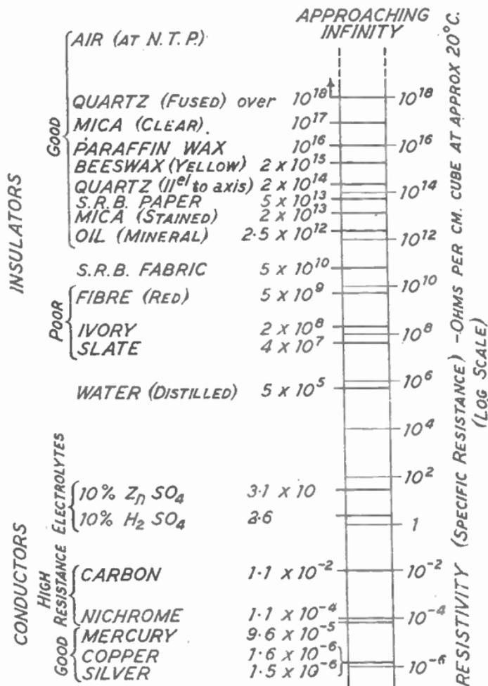
FIG. 5.—“SPECTRUM” OF ELECTRICAL RESISTIVITY OF MATERIALS.
