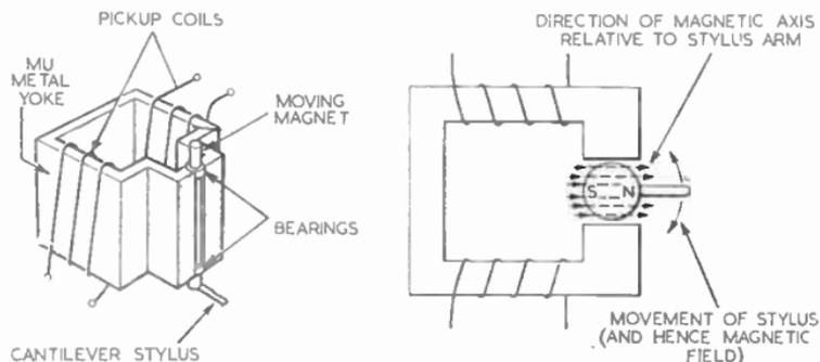
FIG. 19.—SCHEMATIC VIEW OF MOVING-MAGNET PICK-UP.
