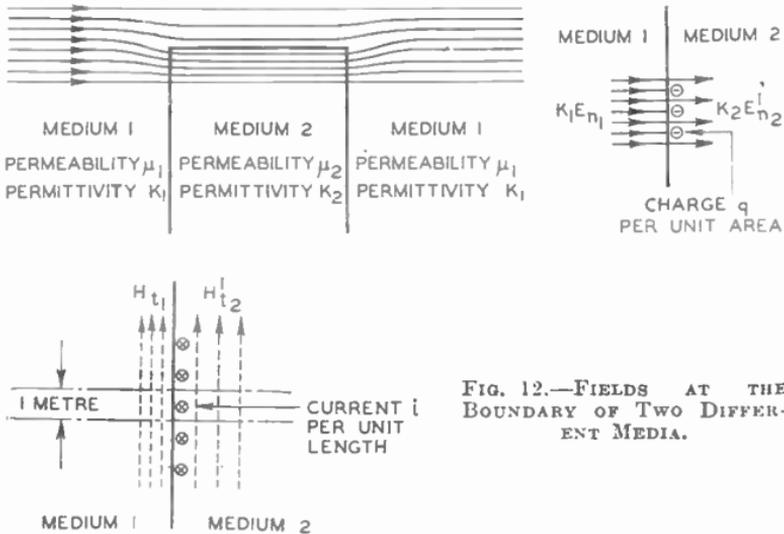
FIG. 12.—FIELDS AT THE BOUNDARY OF TWO DIFFERENT MEDIA.
