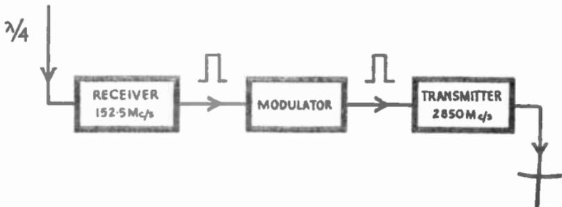
FIG. 49.—BLOCK SCHEMATIC OF THE AIRBORNE RADAR WIND UNIT.
