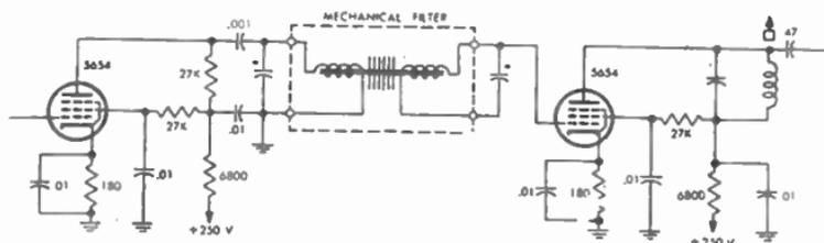
FIG. 7.—TYPICAL CONSTANT GAIN AMPLIFIER USING MECHANICAL FILTER.
