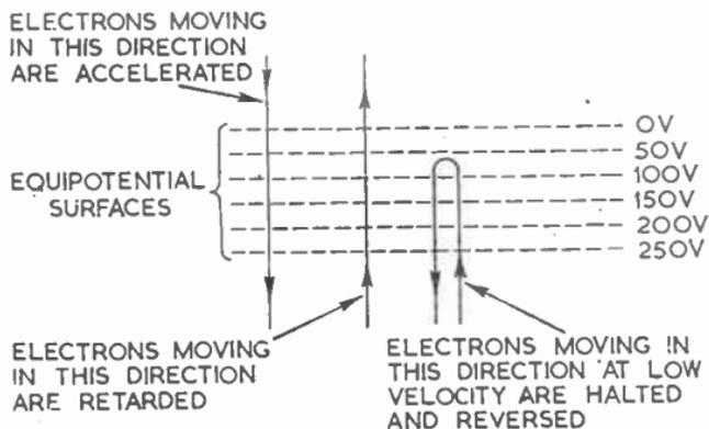
FIG. 4.—BEHAVIOUR OF AN ELECTRON BEAM ENTERING AN ELECTRIC FIELD NORMAL TO THE EQUIPOTENTIAL SURFACES.
