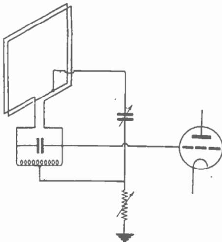
FIG. 6.—PRINCIPLE OF COMBINED OPEN AND LOOP AERIAL.
