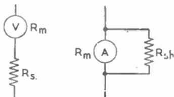
FIG. 122.—SERIES AND SHUNT MULTIPLIERS.
