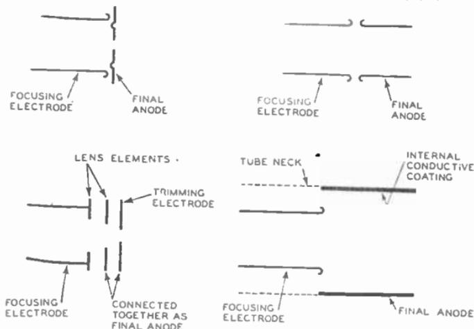
FIG. 5.—FORMS OF ELECTRODES FOR FOCUSING.
