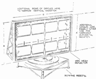
FIG. 30.—A COMMON TYPE OF AERIAL FOR USE WITH LONG-RANGE WARNING SETS, USING STACKED DIPOLES.
