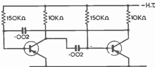
FIG. 39 (left).—MULTI-VIBRATOR CIRCUIT USING TWO JUNCTION TRANSISTORS.
