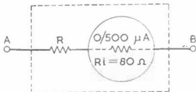
the old value by the addition of a series multiplier of six times the original value. Hence the value of additional multiplier  $R_m$  is given by
