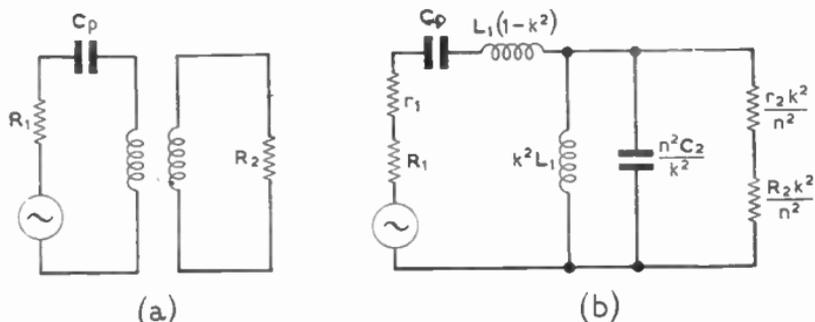
FIG. 6.—SERIES RESONANCE OF PRIMARY: (a) LOADED TRANSFORMER; (b) EQUIVALENT BAND-PASS CIRCUIT.
