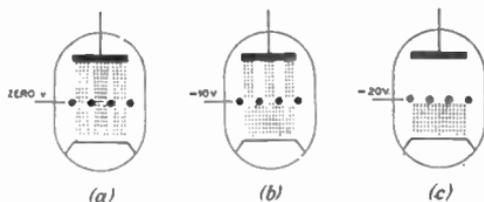
FIG. 6.—HOW THE GRID CONTROLS THE ELECTRON STREAM.
