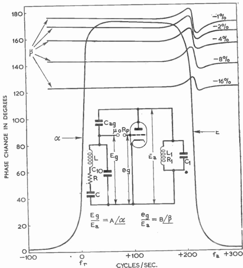
FIG. 8.—PHASE RELATIONS IN THE MILLER-PIERCE CIRCUIT.
