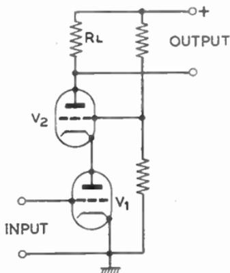
FIG. 2 (a) (left).—THE BASIC FORM OF CASCODE AMPLIFIER.
