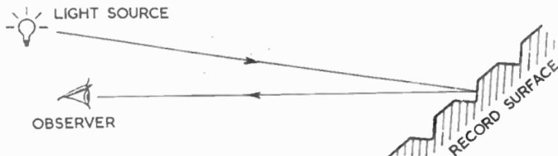
FIG. 12.—PRINCIPLE OF THE BUCHMANN AND MEYER OPTICAL SYSTEM.
