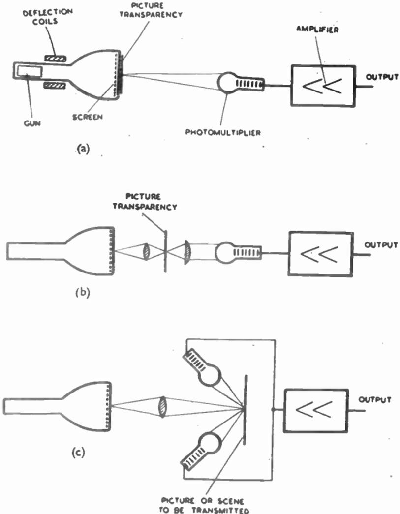
FIG. 5.—THREE EXAMPLES OF FLYING-SPOT SCANNING WITH CATHODE-RAY TUBES.
