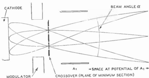
FIG. 4.—ELECTRON TRAJECTORIES.
