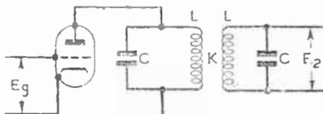
FIG. 5.—STAGE GAIN WITH COUPLED CIRCUITS.
