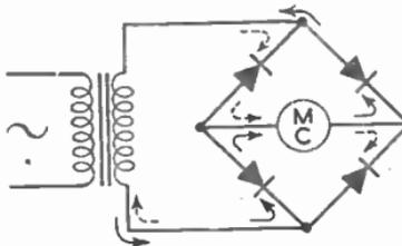
When used at radio frequencies, care must be exercised to minimize the distributed capacitances. Errors are incurred if the applied waveform is not pure sinusoidal, as the recorded deflection current must then be multiplied by the form factor to provide the true R.M.S. value.
