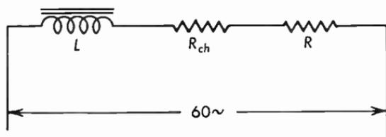
**Fig. 12.20** Circuit illustrating the measuring of inductance with a voltmeter (see text).
