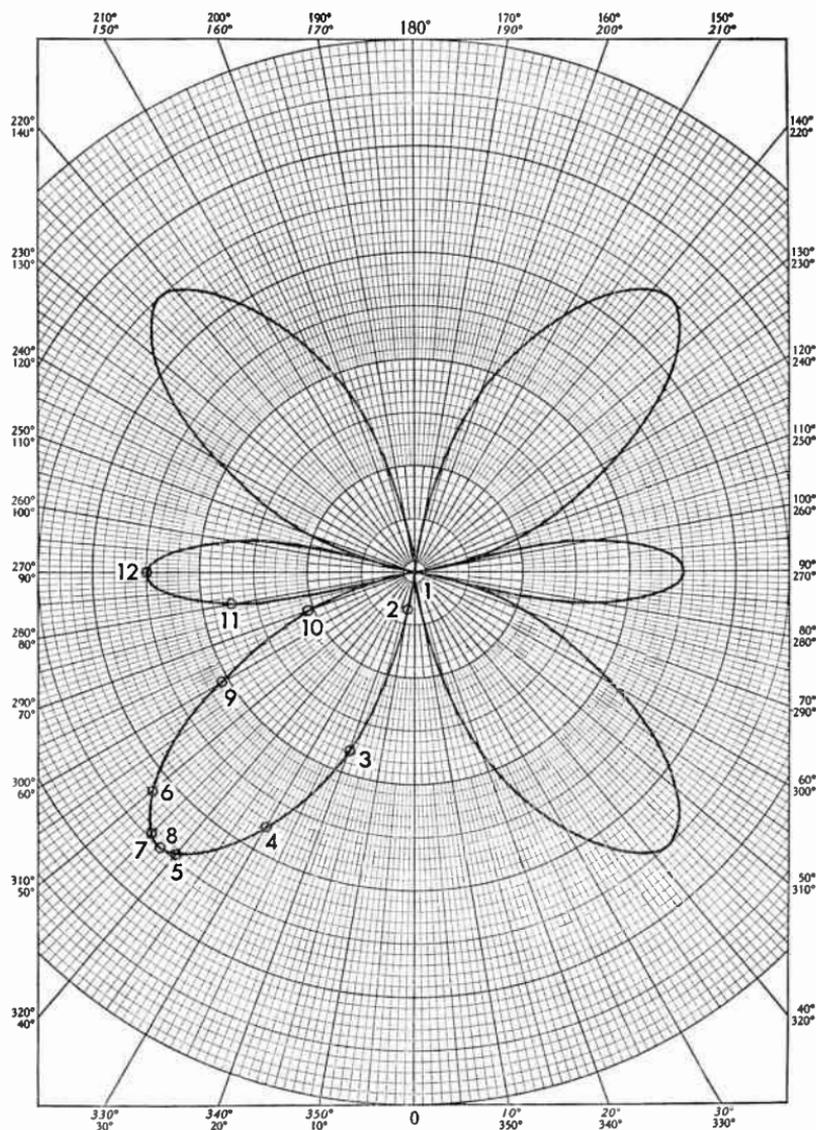
**Fig. 10.24** Field strength pattern of an antenna  $1\frac{1}{2}$  wavelengths long in a plane containing the wire.
