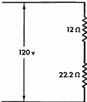
**Fig. 2.20b** Equivalent circuit. The 12-ohm resistance is equivalent to the resistance of the loop *BCED* of Fig. 2.20a; the 22.2-ohm resistance is equivalent to the resistance of loop *DEFG*.
