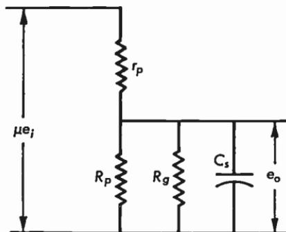
Fig. 5.02 Equivalent circuit of Fig. 5.01a for high frequencies (approx. 10,000 cycles).
