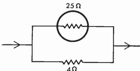
**Fig. 12.18** Equivalent circuit of ammeter with internal resistance and shunt.
