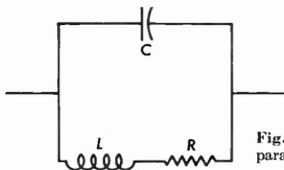
Fig. 3.19 Coil and Capacitor in parallel.
