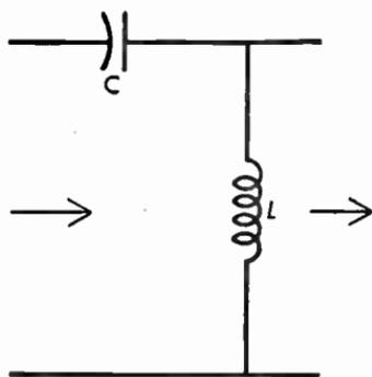
Fig. 4-3.61 High-pass filter.
