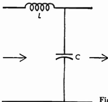
Fig. 4-3.62 Low-pass filter.
