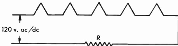
**Fig. 9.21** A-c/d-c filament hookup with lamp-cord resistor.
