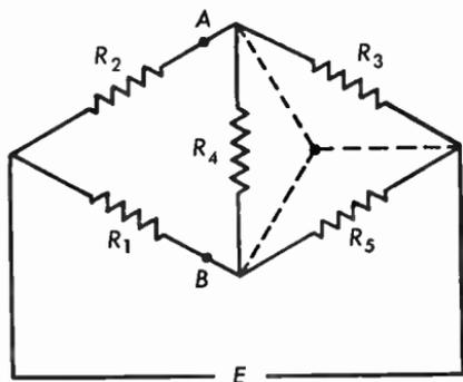
**Fig. 2.23a** Unbalanced bridge of Fig. 2.22a represented by two delta loops.
