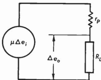
Fig. 13.14b Equivalent circuit of 13.14a.
