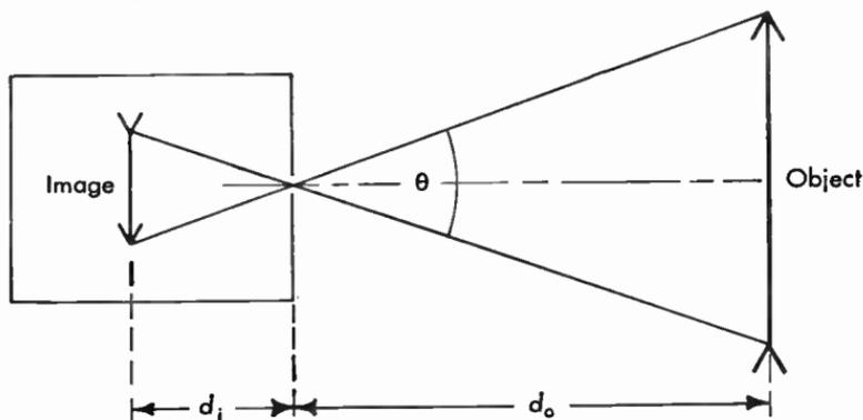
**Fig. 11.51** Camera angle  $\theta$  for a viewing distance of  $d_o$  feet.
