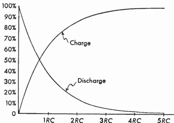
Fig. 11.22 Universal charge and discharge curves (see text).
