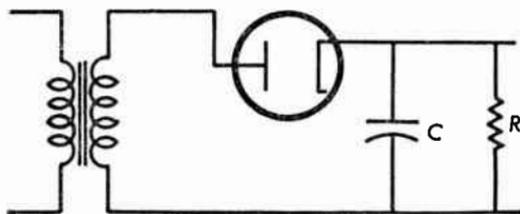
Fig. 11.33a High-voltage rectifier with resistance-capacitance filter.
