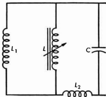
Fig. 8.02 Tank circuit with permeability tuning.
