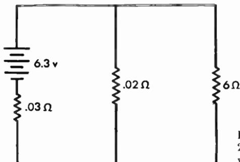
Fig. 2.21b Circuit of Fig. 2.21a, considering the 6.3-volt e.m.f. only.
