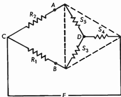
**Fig. 2.23b** The equivalent circuit of Fig. 2.23a, the right loop transformed to a star circuit.
