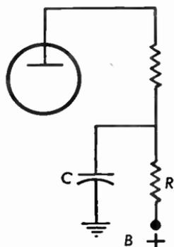
**Fig. 9.14a** Resistance-capacitance decoupling filter.
