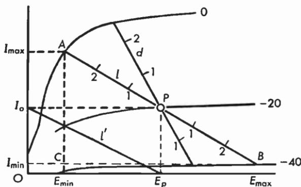
Fig. 4.23 Plate voltage-plate current characteristics of the pentode type 6F6. A scale intersecting the  $-20$  volts grid bias curve will have a nearly equal swing of approximately 3 units between the 0 and the  $-40$  curve, indicating a small amount of distortion.
