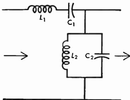
Fig. 4-3.63 Band-pass filter.
