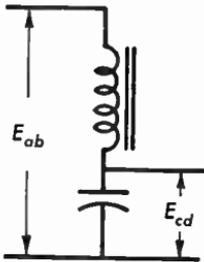
Fig. 9.01b Voltage-divider circuit of the filter output of Fig. 9.01a.
