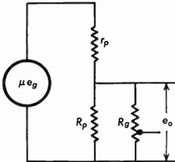
**Fig. 5.37b** Equivalent circuit of the output of the upper half of the 6N7 triode of Fig. 5.37a.
