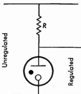
**Fig. 9.20** Voltage regulation by glow-discharge tube.
