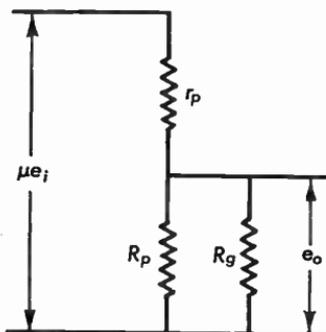
Fig. 5.04 Resistance-capacitance coupled amplifier at medium frequencies.
