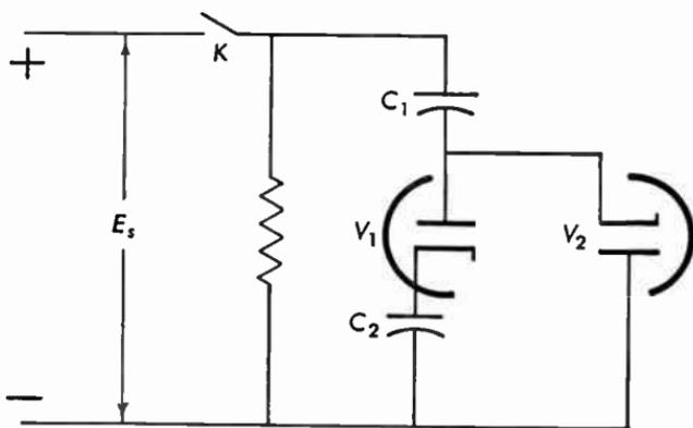
**Fig. 11.26** Electronic counter circuit, based on the principle of the voltage distribution of two capacitors in series. The voltage across the capacitor  $C_2$  is usually employed to unblock the grid of the tube of a discharge circuit.
