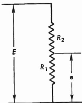
Fig. 4-2.26 Voltage division by tap in load resistor.
