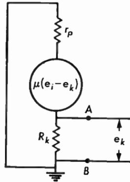
Fig. 11.40b Equivalent circuit of cathode follower.
