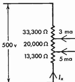
Fig. 2.16 Voltage divider with stated drain from taps.
