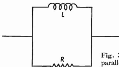
Fig. 3.17 Resistance and inductance in parallel.
