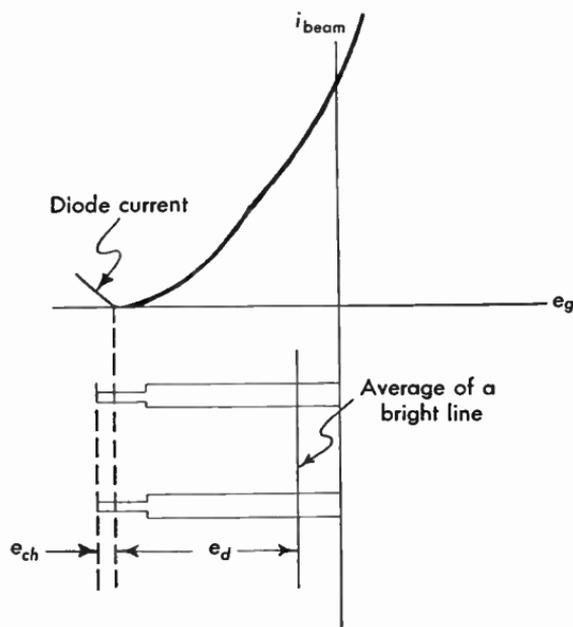
Fig. 11.59c Beam current-grid voltage characteristic of cathode-ray tube and bias conditions for a bright signal.
