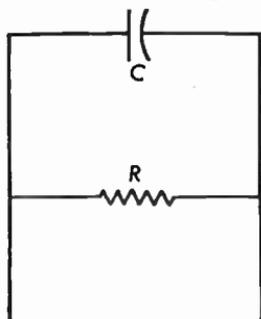
Fig. 3.15 Resistance and capacitance in parallel.
