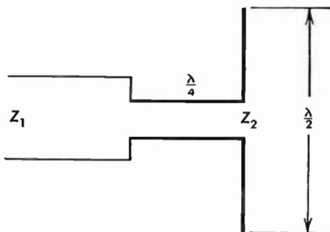
**Fig. 10.26** Quarter-wave matching stub, coupling a two-wire line into a dipole.
