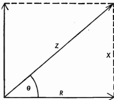
Fig. 3.14 Vector diagram for the total impedance of Fig. 3.13.
