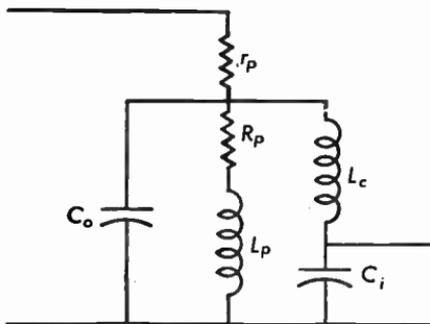
Fig. 11.38b Equivalent circuit of Fig. 11.38a.
