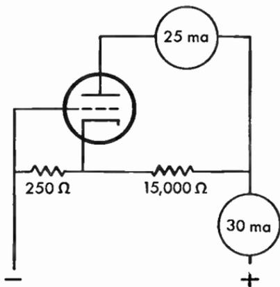
Fig. 12.17 Use of ammeter to find voltages when resistances are known.
