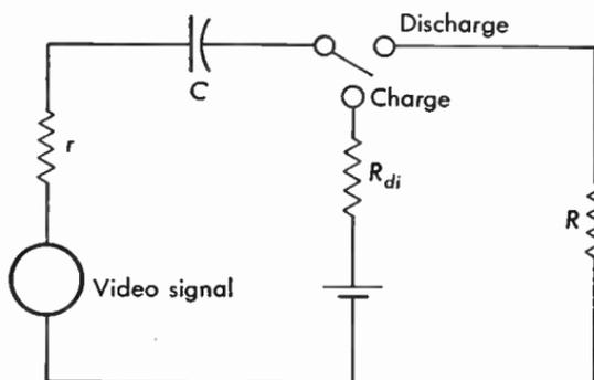
Fig. 11.59b Equivalent circuit of Fig. 11.59a.
