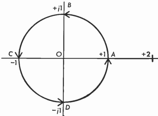
Fig. 3-6 Rotating vectors in the complex plane.
