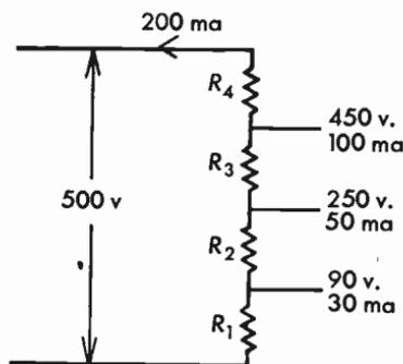
Fig. 9.17 Voltage divider.
