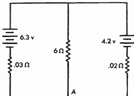
Fig. 2.21d Circuit of Fig. 2.21a, arranged to illustrate a right-hand and a left-hand loop, both containing a source of e.m.f.
