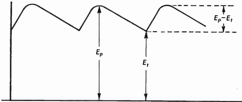
Fig. 11.33b Fluctuating direct voltage as obtained from the rectifier of Fig. 11.33a.
