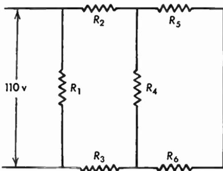
Fig. 2.19a Series-parallel circuit, conventional layout.
