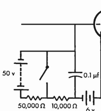
Fig. 7.02 Grid keying with click filter.
