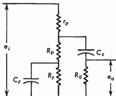
**Fig. 11.39b** Equivalent circuit of Fig. 11.39a.
