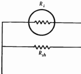
Fig. 12.14 Ammeter with shunt resistor extending the range of the meter.
