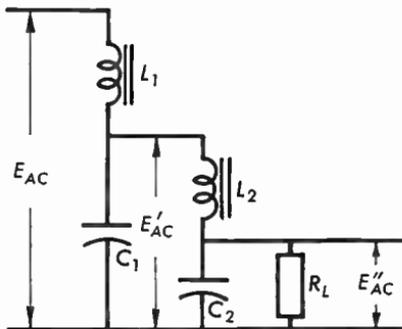
Fig. 9.06b Equivalent circuit of the filter sections of Fig. 9.06a.
