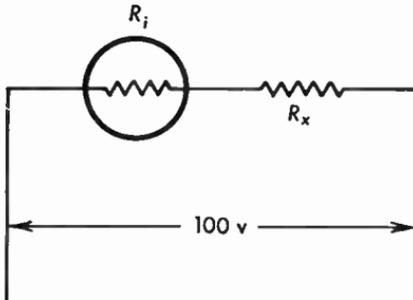
Fig. 12.13 Voltmeter with series resistor extending the range of the meter.
