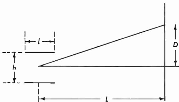
Fig. 11.11 Diagram illustrating the deflection of an electron beam by electrostatic deflection.
