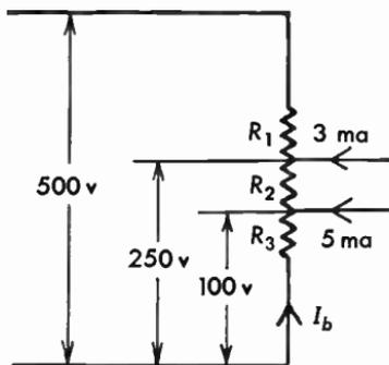
Fig. 2.17 Voltage divider with stated voltages and currents.
