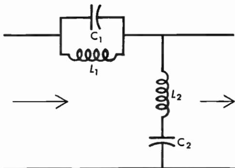
Fig. 4-3.64 Band-elimination filter (wave trap).
