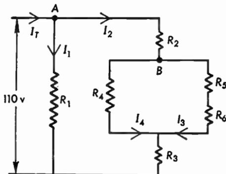
Fig. 2.19b Series-parallel circuit, equivalent to the circuit of Fig. 2.19a.
