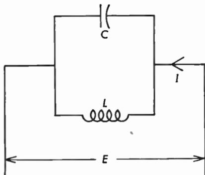
Fig. 3.16 Capacitance and inductance in parallel.
