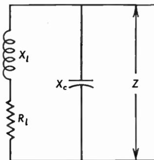
Fig. 3.26 Parallel-resonant circuit.
