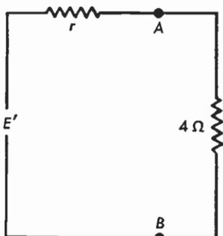
Fig. 2.25b Equivalent circuit. The circuit to the left of  $AB$  is "Thévenins generator."
