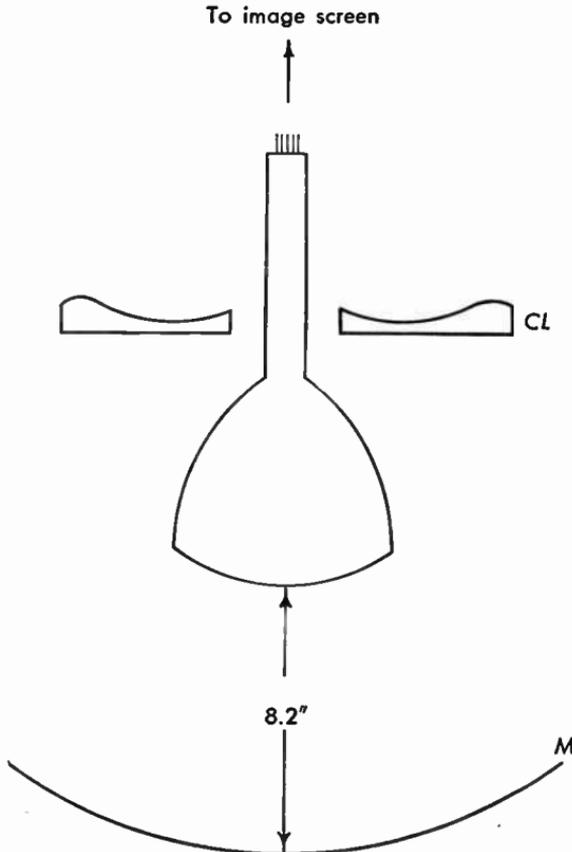
**Fig. 11.45** Reflective projection system. *CL* = correcting lens, *M* = concave mirror.
