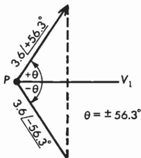
**Fig. 3-10** Two polar vectors of the same magnitude having a positive and a negative phase angle.
