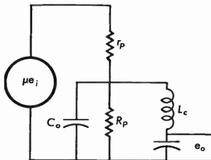
Fig. 11.37b Equivalent circuit of Fig. 11.37a.
