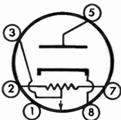
Fig. 9.24 Base connections of the 35Z5 rectifier tube. Prongs 2 and 7 are the heater terminals, prong 3 is the pilot-light tap.
