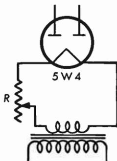
Fig. 2.05 Filament rheostat, used to cause a voltage drop since the voltage across the transformer secondary is too high.
