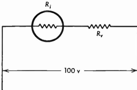
**Fig. 12.15** Ammeter with series resistor to make the meter read voltage.
