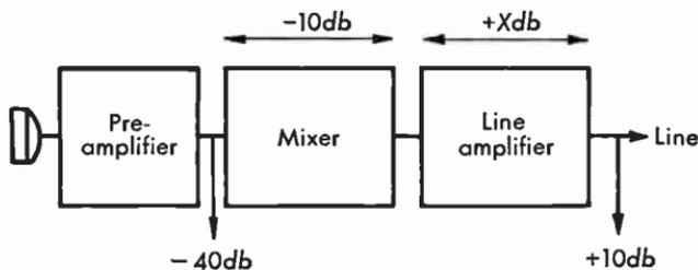
Fig. 5.14 Block diagram of audio equipment with line amplifier.
