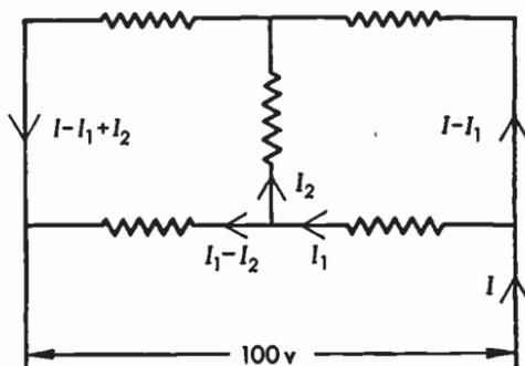
Fig. 2.22b Current layout on the unbalanced bridge.
