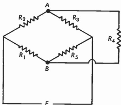
Fig. 2.25a Unbalanced bridge.  $R_4$  to be disconnected and the remainder of the network to be simplified to a source of e.m.f. with an internal resistance.
