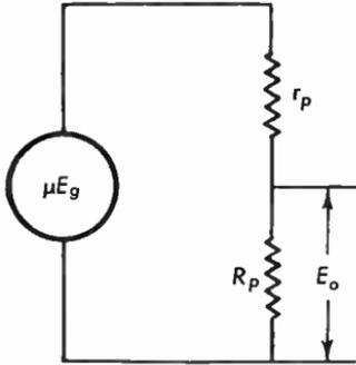
Fig. 4.08 Equivalent circuit of triode with resistive load.
