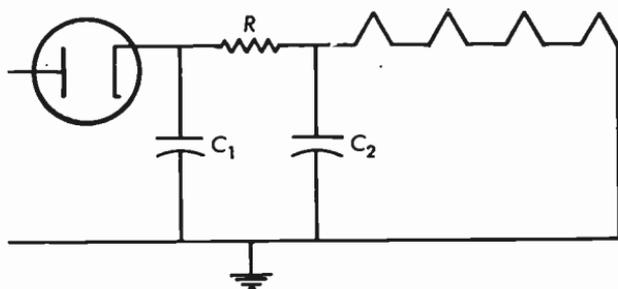
**Fig. 9.26** Power supply suitable for a-c, d-c, and battery supplies.
