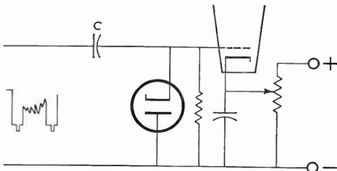
Fig. 11.59a D-c restorer using a diode tube.
