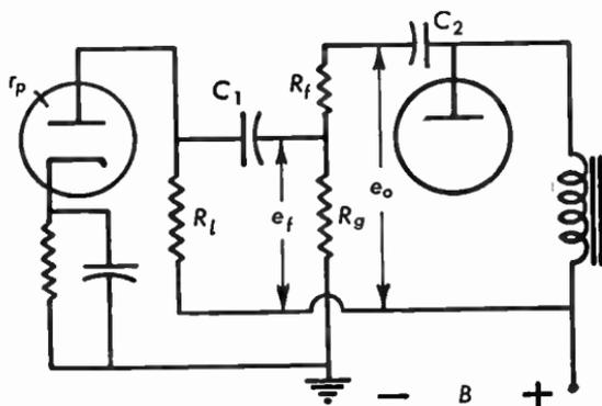
Fig. 8.22a Resistance-coupled amplifier with negative feedback.
