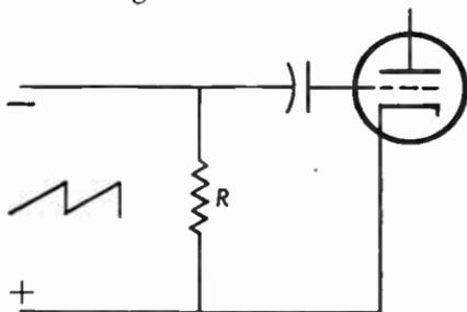
Fig. 13.03 Saw-tooth wave applied to thyatron tube through an  $R$ - $C$  circuit.
