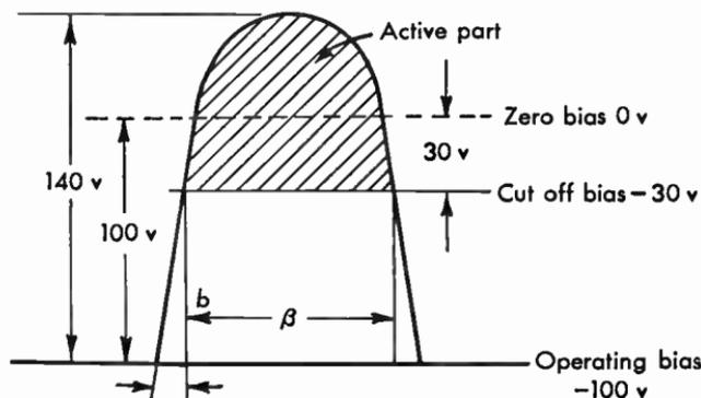
**Fig. 5.44** Diagram illustrating the bias conditions of a class C amplifier.
