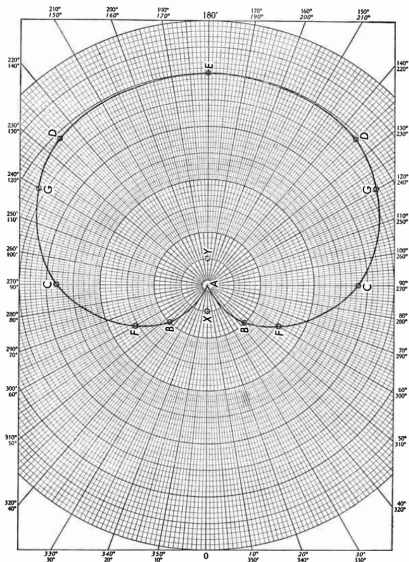
Fig. 10.25 Field strength pattern in a horizontal plane obtained by two vertical wires spaced  $\frac{1}{4}$  wavelength apart and fed 90 degrees out of phase.
