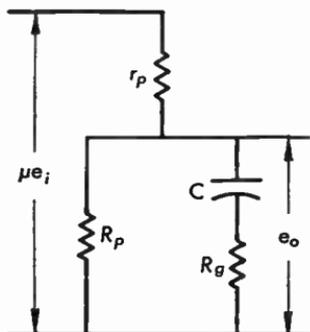
Fig. 5.08 Resistance-capacitance coupled amplifier at low frequencies.
