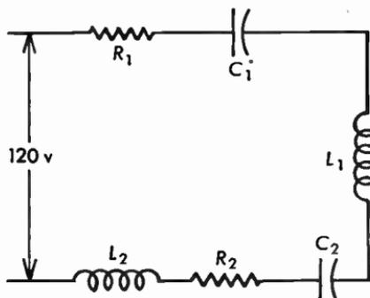
Fig. 3.13 Impedance elements in series.
