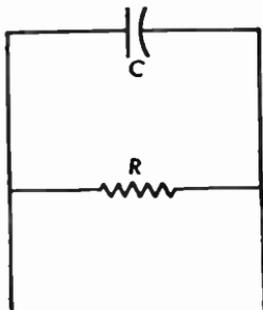
**Fig. 3.15** Resistance and capacitance in parallel.
