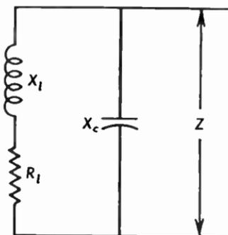
Fig. 3.26 Parallel-resonant circuit.
