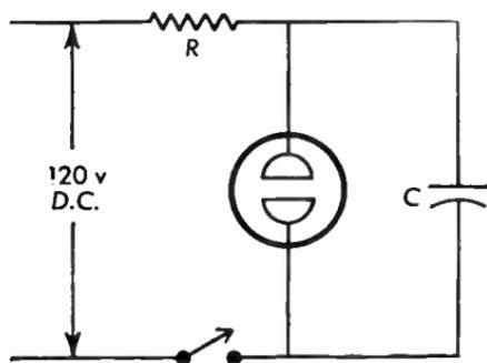
**Fig. 13.04** Saw-tooth oscillator using a neon bulb discharge path.
