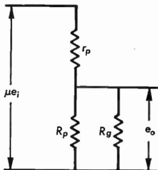
Fig. 5.01b Equivalent circuit of Fig. 5.06a for medium frequencies (approx. 1000 cycles).
