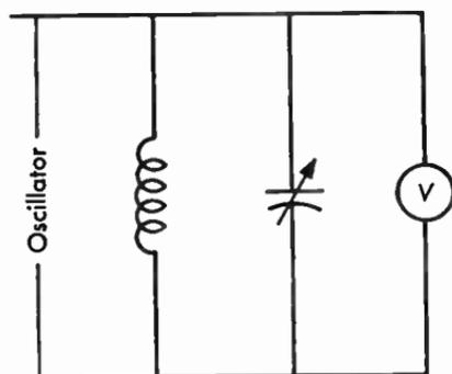
**Fig. 12.11** Circuit for measuring the inductance of an r-f coil.
