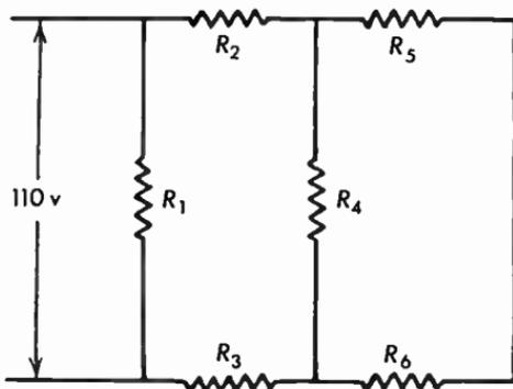
Fig. 2.19a Series-parallel circuit, conventional layout.
