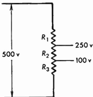
**Fig. 2.15** Voltage divider with negligible current drain from taps.
