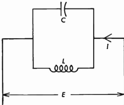
Fig. 3.16 Capacitance and inductance in parallel.
