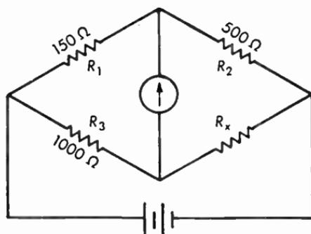
**Fig. 12.01** Wheatstone bridge, as used to measure unknown resistances.
