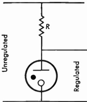
**Fig. 9.20** Voltage regulation by glow-discharge tube.
