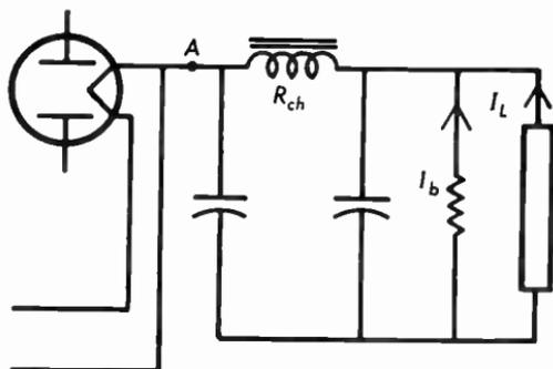
**Fig. 9.10** Filter with bleeder resistor.
