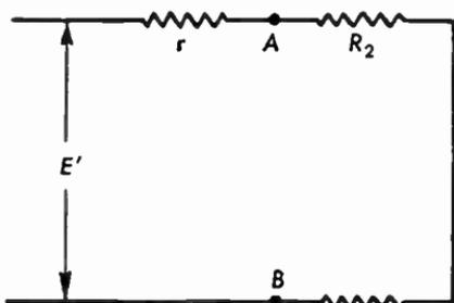
**Fig. 2.24b** Equivalent circuit. The network to the left of  $AB$  is represented by a "Thévenin generator" with an e.m.f. of  $E'$  volts and an internal resistance of  $r$  ohms.
