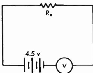
**Fig. 12.07** Circuit for measuring resistance with a voltage-indicating meter.
