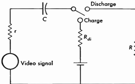
Fig. 11.59b Equivalent circuit of Fig. 11.59a.
