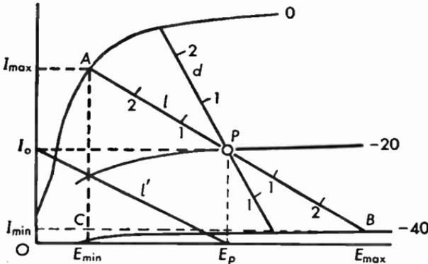
Fig. 4.23 Plate voltage-plate current characteristics of the pentode type 6F6. A scale intersecting the  $-20$  volts grid bias curve will have a nearly equal swing of approximately 3 units between the 0 and the  $-40$  curve, indicating a small amount of distortion.
