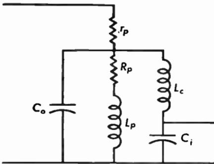
Fig. 11.38b Equivalent circuit of Fig. 11.38a.
