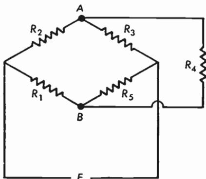
**Fig. 2.25a** Unbalanced bridge.  $R_1$  to be disconnected and the remainder of the network to be simplified to a source of e.m.f. with an internal resistance.
