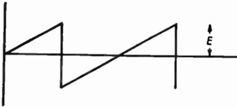
**Fig. 11.43** Saw-tooth wave.
