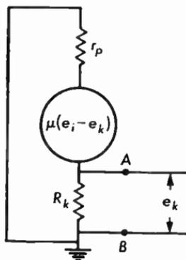
Fig. 11.40b Equivalent circuit of cathode follower.
