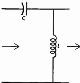
Fig. 4-3.61 High-pass filter.
