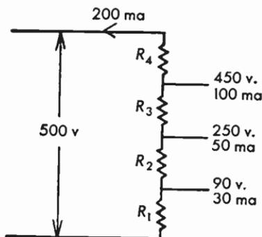
**Fig. 9.17** Voltage divider.
