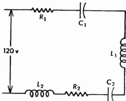
Fig. 3.13 Impedance elements in series.
