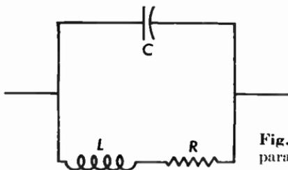
Fig. 3.19 Coil and Capacitor in parallel.
