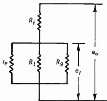
Fig. 8.22b Equivalent circuit at Fig. 8.22a.
