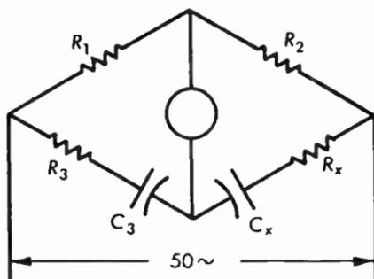
**Fig. 12.10** Capacitance-resistance bridge, suitable for measuring unknown capacitance and power factor. When  $C_x$  and  $R_x$  are connected in parallel the circuit is referred to as a *Wien bridge* (see also problem 12.12).
