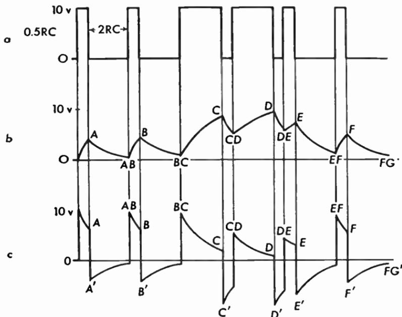
**Fig. 11.23** *a.* Rectangular pulses. The short intervals on the time axis are all  $\frac{1}{2} RC$  second, the long intervals all  $2 RC$  seconds.
