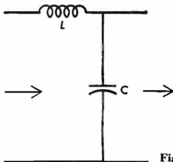
Fig. 4-3.62 Low-pass filter.
