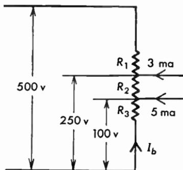
Fig. 2.17 Voltage divider with stated voltages and currents.
