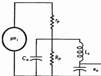
Fig. 11.37b Equivalent circuit of Fig. 11.37a.
