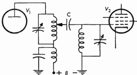
**Fig. 6.11** Capacitance-coupled r-f amplifier.
