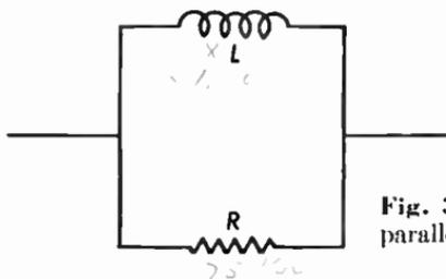
**Fig. 3.17** Resistance and inductance in parallel.
