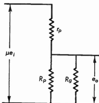
**Fig. 5.04** Resistance-capacitance coupled amplifier at medium frequencies.
