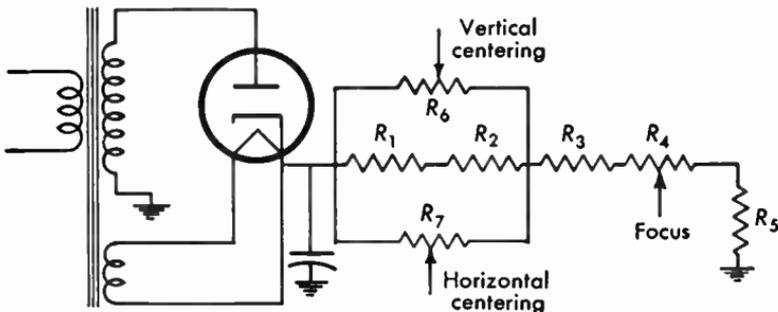
**Fig. 11.34** High-voltage rectifier with provisions for focusing and centering.
