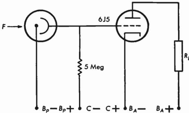
**Fig. 13.14a** Phototube with amplifier.
