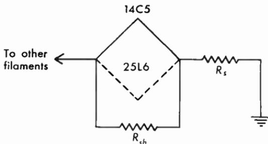
**Fig. 9.29** Diagram illustrating the substitution of a 25L6 beam-power tube by using the equivalent type 14C5.
