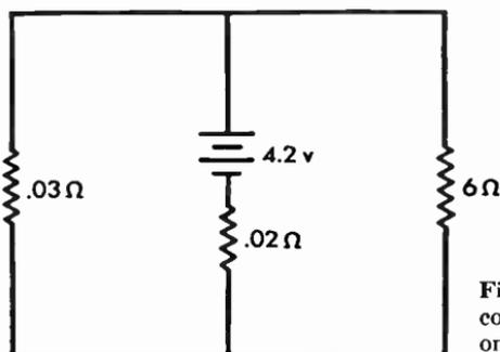
Fig. 2.21c Circuit of Fig. 2.21a, considering the 4.2-volt e.m.f. only.
