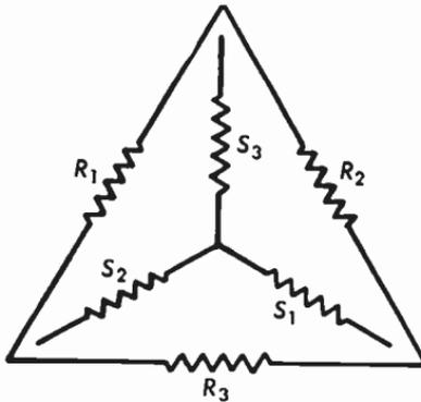
Fig. 4-2.25 Equivalent delta and star impedance elements.
