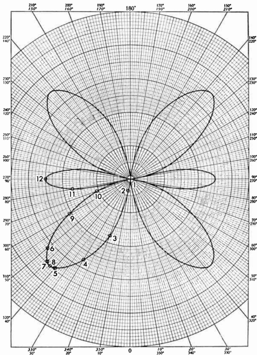
**Fig. 10.24** Field strength pattern of an antenna  $1\frac{1}{2}$  wavelengths long in a plane containing the wire.
