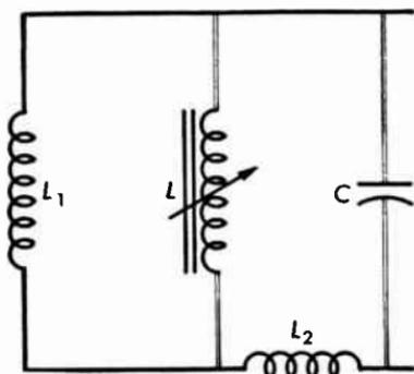
Fig. 8.02 Tank circuit with permeability tuning.
