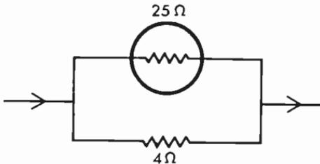
**Fig. 12.18** Equivalent circuit of ammeter with internal resistance and shunt.
