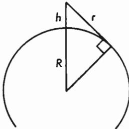
**Fig. 11.08** Distance of the horizon  $r$  as seen from an altitude  $h$ .
