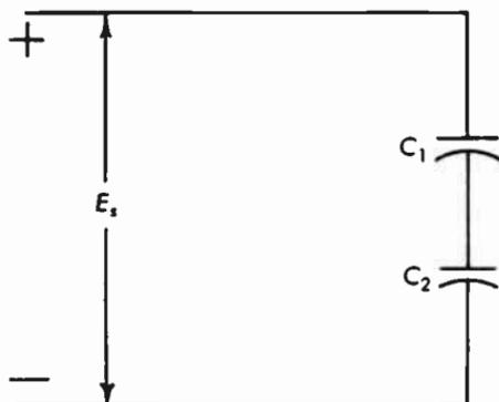
**Fig. 11.25** Direct voltage  $E_s$  applied across two capacitors in series.
