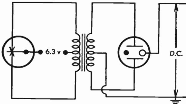
**Fig. 9.18** Vibrator-power supply with gas-filled rectifier tube.
