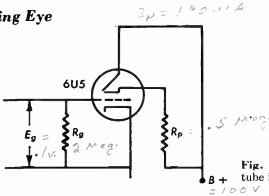
**Fig. 8.17** Electron-ray tube indicator.
