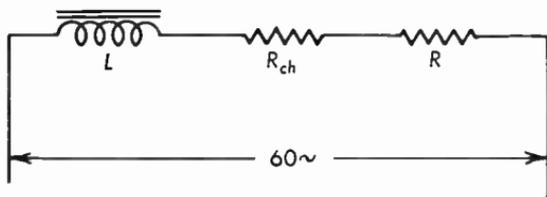
**Fig. 12.20** Circuit illustrating the measuring of inductance with a voltmeter (see text).
