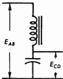
Fig. 9.03b Voltage-divider circuit of the filter output of Fig. 9.03a.
