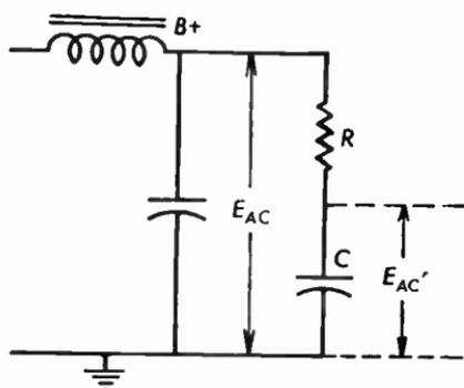
**Fig. 9.14b** Decoupling filter as connected across the B-supply.
