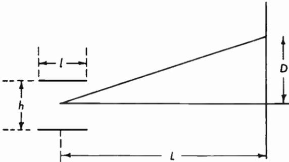
**Fig. 11.11** Diagram illustrating the deflection of an electron beam by electrostatic deflection.
