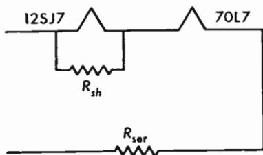
**Fig. 9.28** Series filament hookup for phonograph amplifier.
