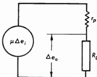
Fig. 13.14b Equivalent circuit of 13.14a.
