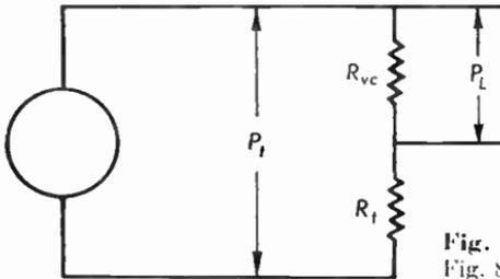
Fig. 8.27b Equivalent circuit of Fig. 8.27a.
