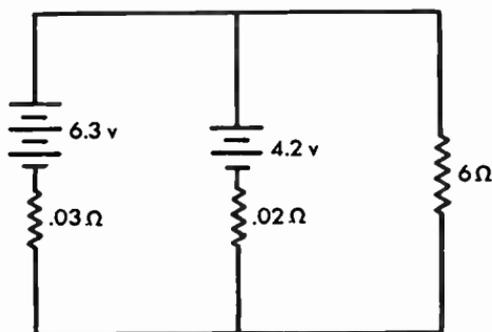
**Fig. 2.21a** Two sources of e.m.f. connected in parallel across a load of 6 ohms.
