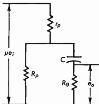
Fig. 5.03 Equivalent circuit of Fig. 5.01a for low frequencies (approx. 50 cycles).
