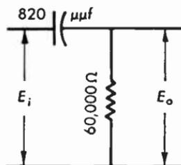
**Fig. 11.19** One-stage differentiating circuit.
