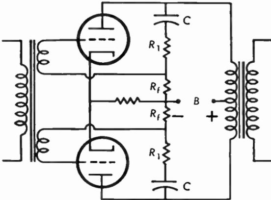
**Fig. 8.23** Push-pull circuit with negative feedback.
