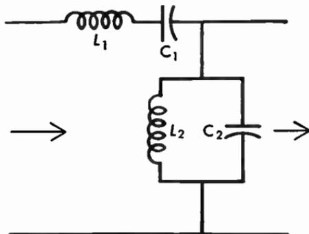
Fig. 4-3.63 Band-pass filter.
