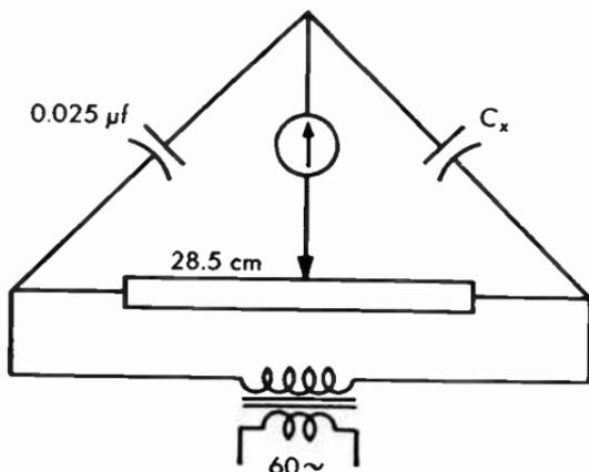
**Fig. 12.09** Slide-wire bridge used to measure an unknown capacitance.
