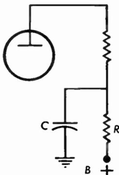
**Fig. 9.14a** Resistance-capacitance decoupling filter.
