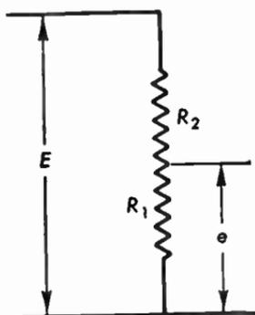
Fig. 4-2.26 Voltage division by tap in load resistor.
