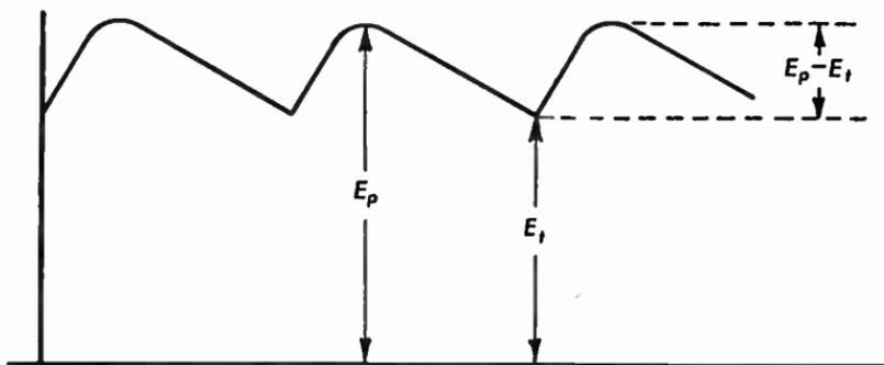
Fig. 11.33b Fluctuating direct voltage as obtained from the rectifier of Fig. 11.33a.
