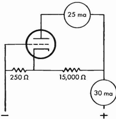
Fig. 12.17 Use of ammeter to find voltages when resistances are known.
