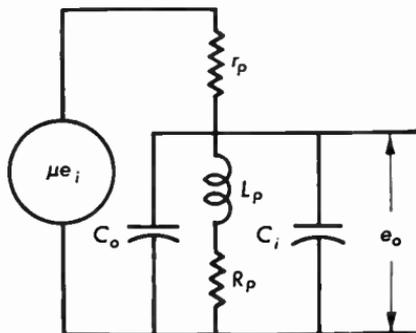
Fig. 11.36b Equivalent circuit of Fig. 11.36a.
