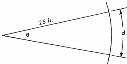
**Fig. 11.16** Distance  $d$  distinguishable when the viewing angle is  $\theta$ .
