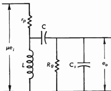
**Fig. 5.26** Equivalent circuit of an impedance-coupled audio amplifier.
