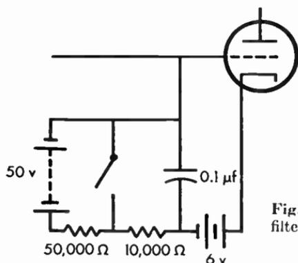
Fig. 7.02 Grid keying with click filter.
