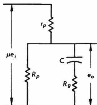
**Fig. 5.08** Resistance-capacitance coupled amplifier at low frequencies.
