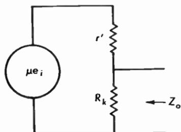
Fig. 11.41 Equivalent circuit of cathode follower for calculating the output impedance. The equivalent plate resistance  $r'$  and the equivalent generator  $\mu e_i$  make the circuit analogous to a plate coupled triode amplifier.
