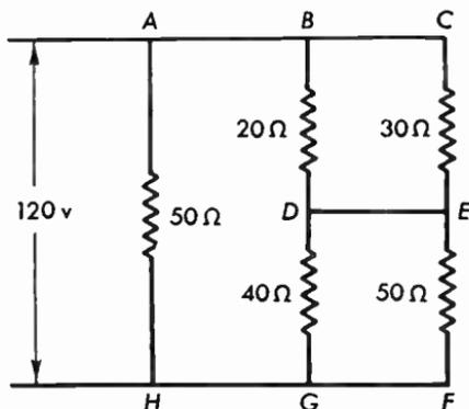
**Fig. 2.20a** Series-parallel circuit.
