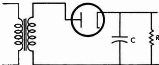
**Fig. 11.33a** High-voltage rectifier with resistance-capacitance filter.
