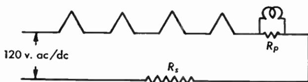
Fig. 9.22 A-c/d-c filament hookup with ballast resistor and pilot lamp.
