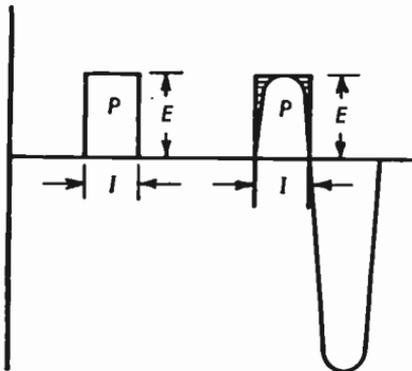
**Fig. 5.42** Diagram illustrating the driving power of a class C amplifier.
