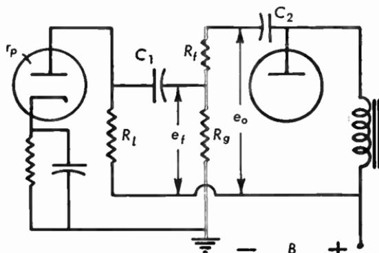
Fig. 8.22a Resistance-coupled amplifier with negative feedback.
