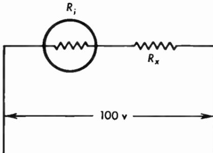
**Fig. 12.13** Voltmeter with series resistor extending the range of the meter.
