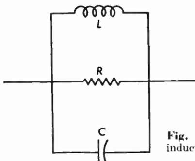
**Fig. 3.18** Resistance, capacitance and inductance in parallel.
