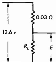
**Fig. 9.23b** Equivalent circuit of Fig. 9.23a.
