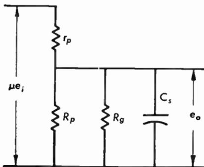
Fig. 5.06 Resistance-capacitance coupled amplifier at high frequencies.
