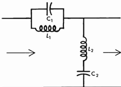
Fig. 4-3.64 Band-elimination filter (wave trap).
