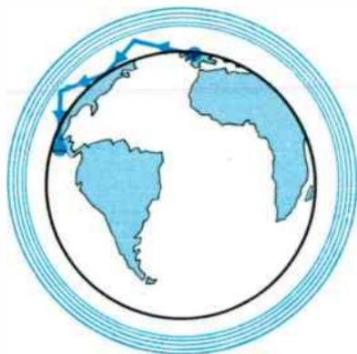
**1·18 Far left** Radio waves would not be expected to travel from England to America any more easily than light would travel a quarter way round a sphere of radius 3 cm from a point on its surface. Rayleigh showed this by comparing the radii with the wavelengths.
