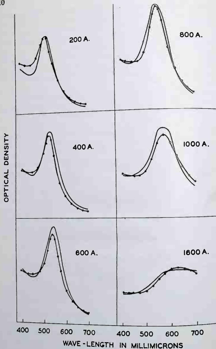
Fig. 9. Absorption spectrum of colloidal gold as a function of the diameter of the particle. The points are experimental while the full curve is the absorption spectrum predicted by G. Mie.
