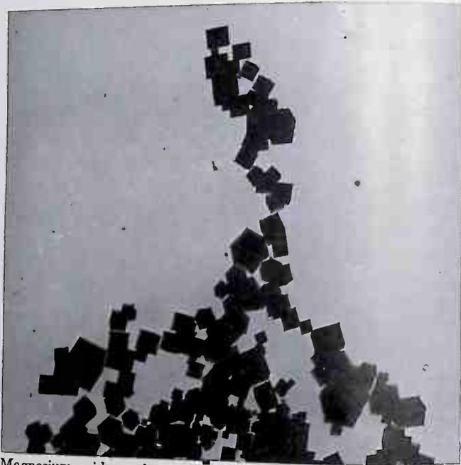
Fig. 1. Magnesium oxide smoke produced by burning magnesium in air. Note the cubic form and the mode of attachment. Magnification 26,000X.
