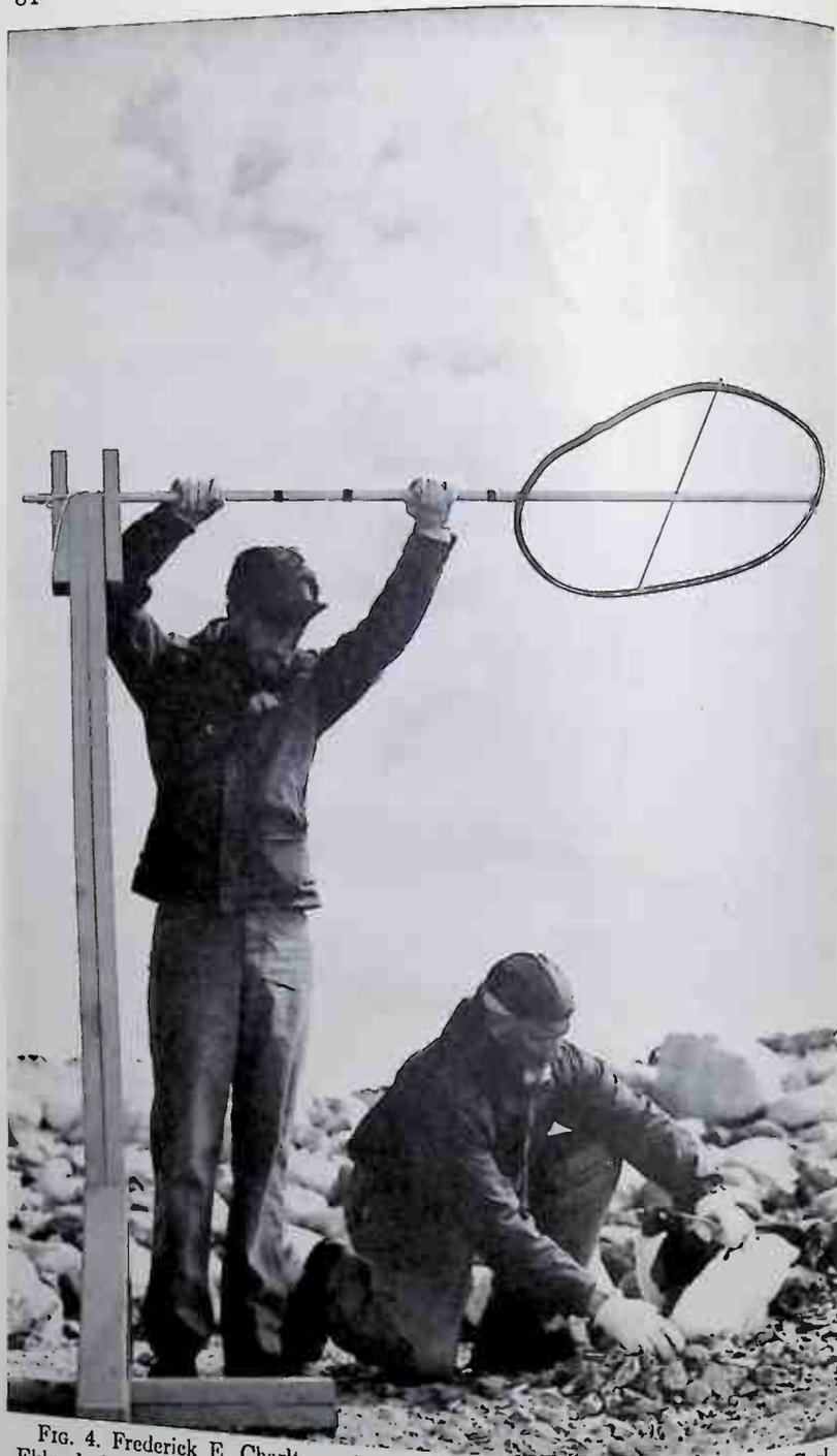
FIG. 4. Frederick E. Charlton orients loop antenna over penguin nest as Carl Eklund places egg containing telemeter under bird. Temperature signals picked up by the antenna are carried by a transmission line to a receiver located nearby.
