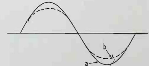
Fig. 3—Non-linear distortion changes the shape of a sine wave form from "a" to the flatter top type of "b".
