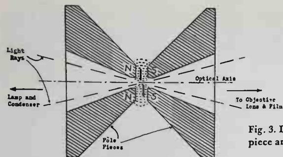
Fig. 3. Light-valve ribbon and pole piece arrangement; section at right angles to ribbons.
