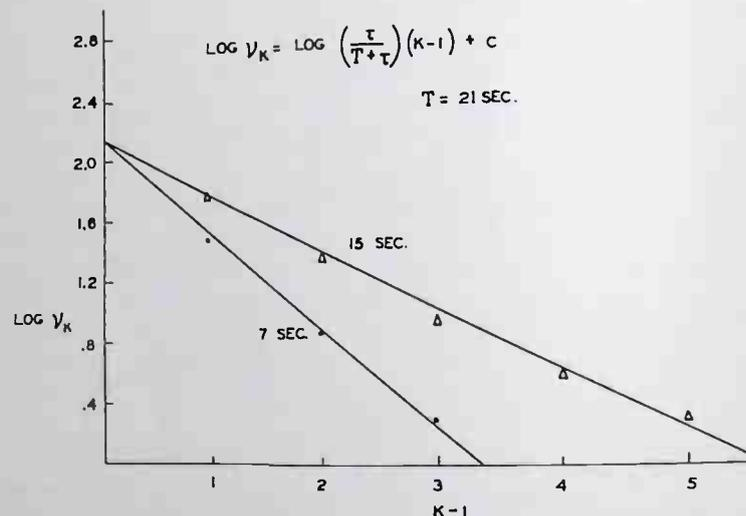
FIG. 13. Experimental verification of Smolouchowski relation between the number of clusters  $v_k$  containing  $k$  particles, and the number of  $k$  particles in a cluster, for two times during the process of aggregation.
