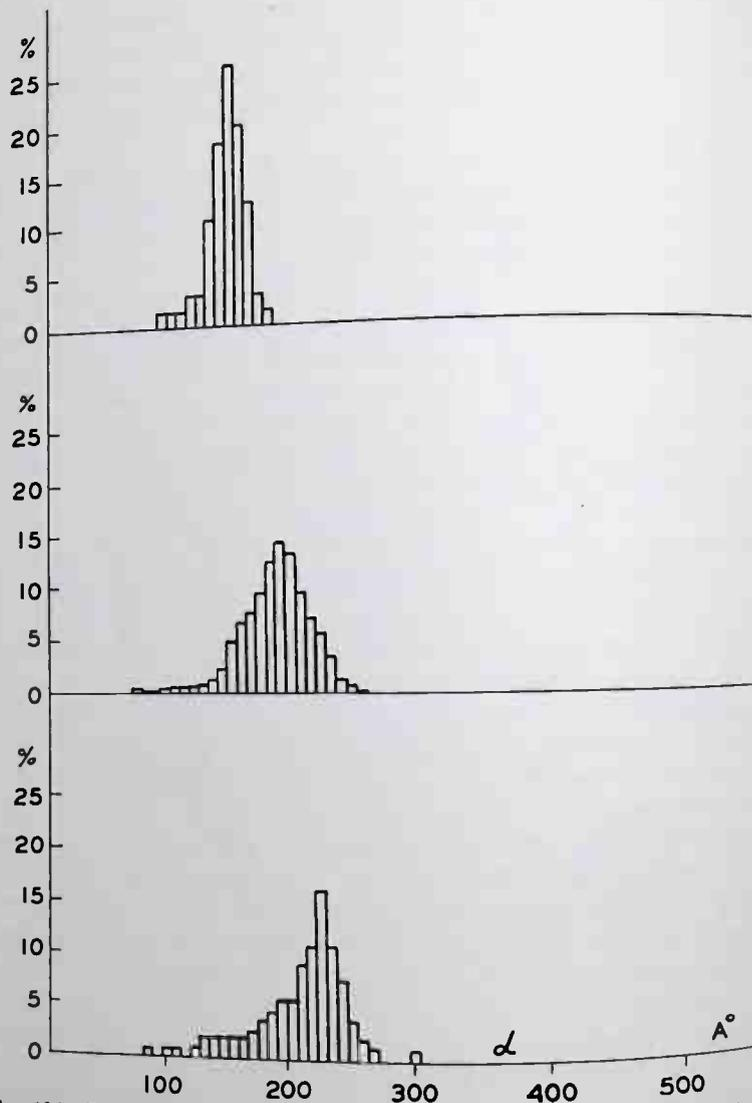
Fig. 10A. Particle size distribution curve of colloidal gold prepared at different concentrations.
