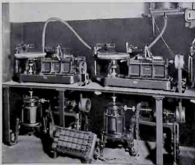
Fig. 4—Two recording machines arranged to be driven synchronously with cameras.
