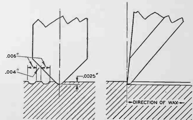
Fig. 5—Details of the stylus point of the recorder. Left, a radial section through the wax; right, a section looking from the stylus point to the center of the disc.
