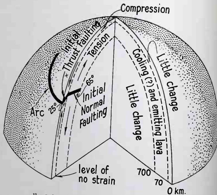
Fig. 6. Diagram of arc formation in a contracting Earth.
