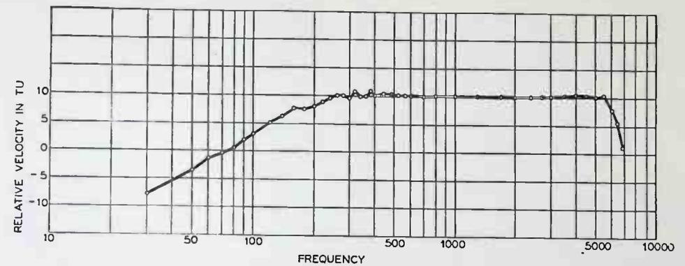
Fig. 2—Typical frequency characteristic of a commercial recorder.
