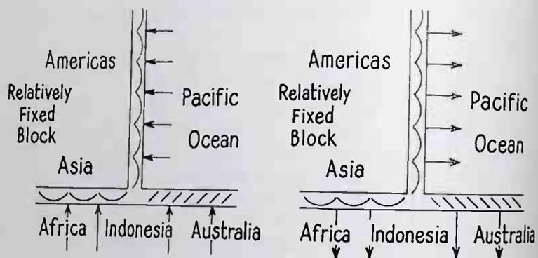
FIG. 7. Diagram of the pattern of continental fracture system which would result if created by forces (A) in the zone of compression above 70 km and (B) in the zone of relief of pressure between 70 and 700 km. The latter corresponds with Figure 3. Note the different orientation of the fractured arcs north of Australia.
