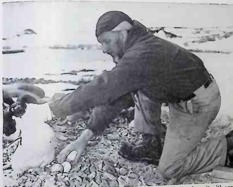
FIG. 3. Eklund removes one genuine egg from penguin nest and replaces it with egg containing telemeter.
