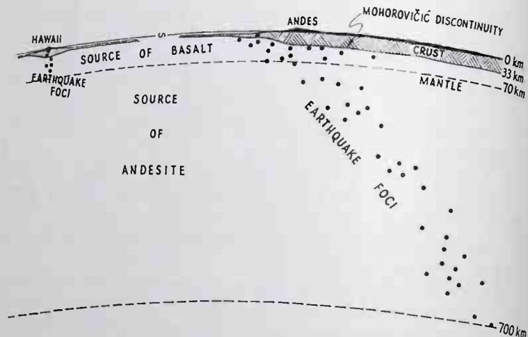
Fig. 5. Cross section of crust and upper mantle. (No vertical exaggeration.)
