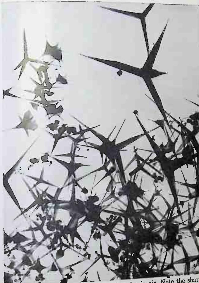
Fig. 2. Zinc oxide smoke produced by burning zinc in air. Note the sharp needles originating from plates. Magnification 25,000X.
