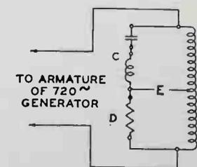
Fig. 2—The heart of the sound-picture governor. Potential E shifts 180° in phase as the speed changes from any value below 1200 r. p. m. to any value above it.
