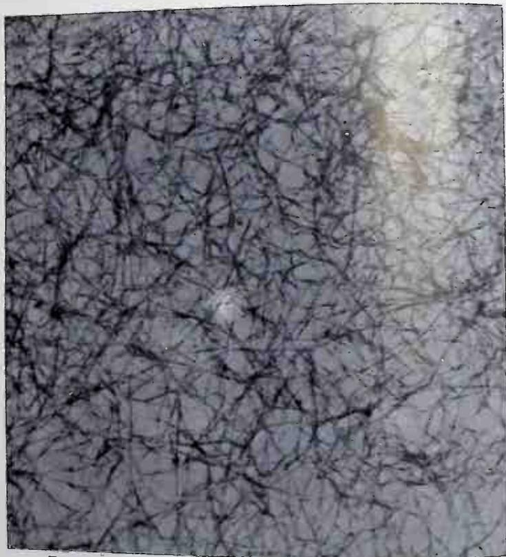
FIG. 4. Fibers of vanadium pentoxide. Magnification 166,667 $\times$ .
