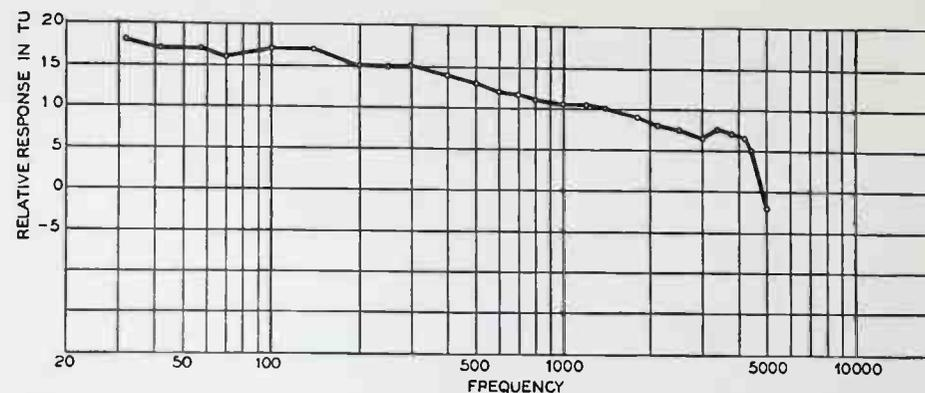
Fig. 10—Response of a 4-A pick-up driven by a constant-velocity pressing.
