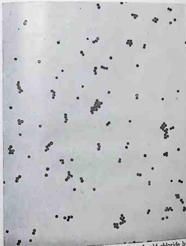
Fig. 7. Colloidal gold particles obtained by reduction of gold chloride by sodium citrate. Magnification 50,000 $\times$ .
