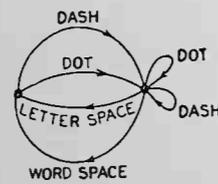
Fig. 2—Graphical representation of the constraints on telegraph symbols.
