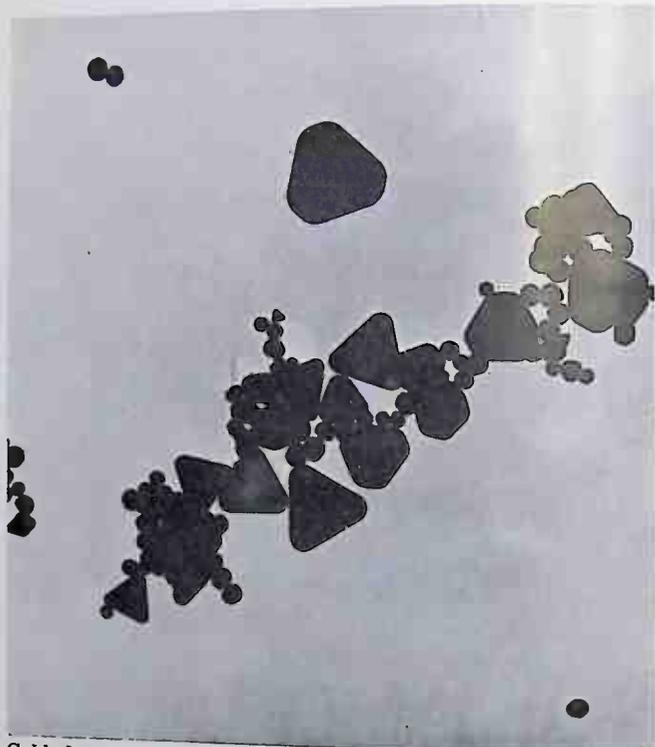
FIG. 8. Gold plates and spheres obtained by reduction of gold chloride by citric acid 25,000 X.
