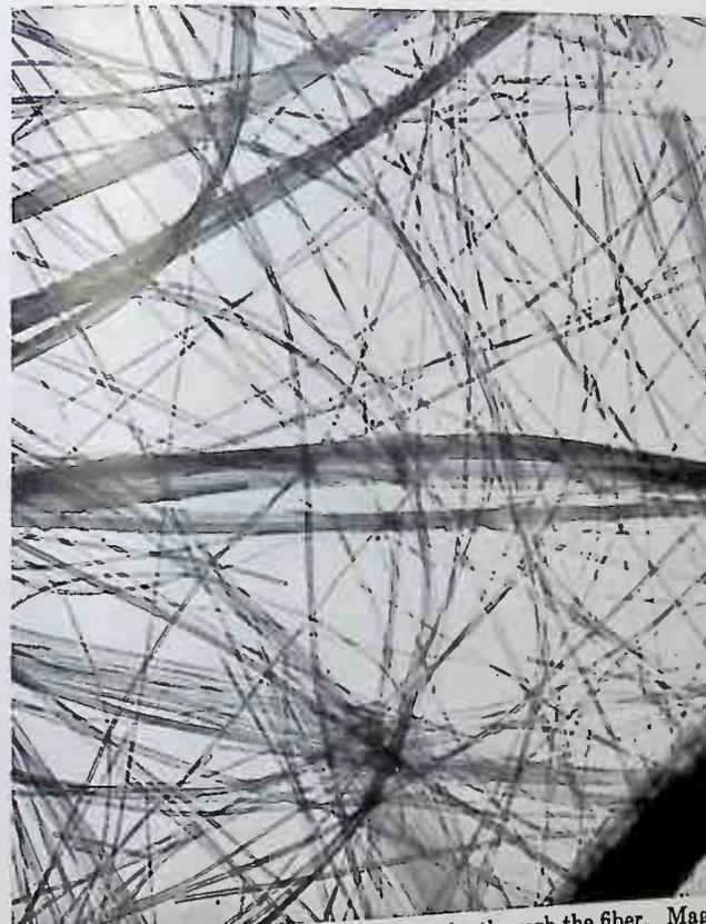
Fig. 3. Fibers of chrysotile asbestos. Note the tube through the fiber. Magnification 19,500X.
