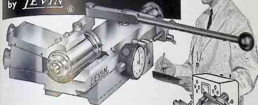
Levin micro-drilling equipment can be used with the smallest drills available. The drill can be retracted for chip removal and returned to position without striking the bottom of the hole. While commercial drills can be had as small as .0016" Levin equipment has successfully produced holes as small as .0006". Send for catalog M describing complete line of instrument lathes and accessories for the laboratory. LOUIS LEVIN & SON, INC., 3610 S. Broadway, Los Angeles 7, California
