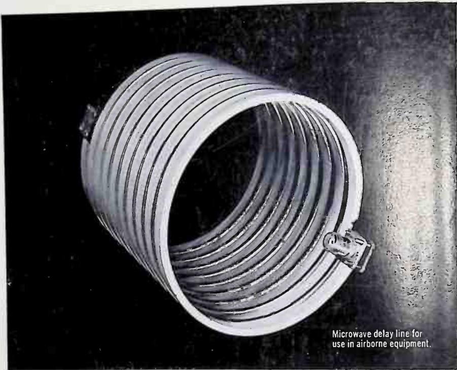
Microwave delay line for use in airborne equipment.
