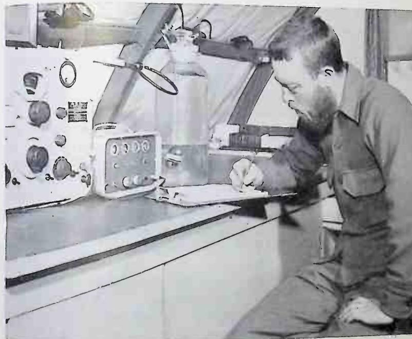
FIG. 5. Charlton calibrates temperature telemeter. Instruments shown, from left to right, are receiver, counter, and telemeter (in bottle).
