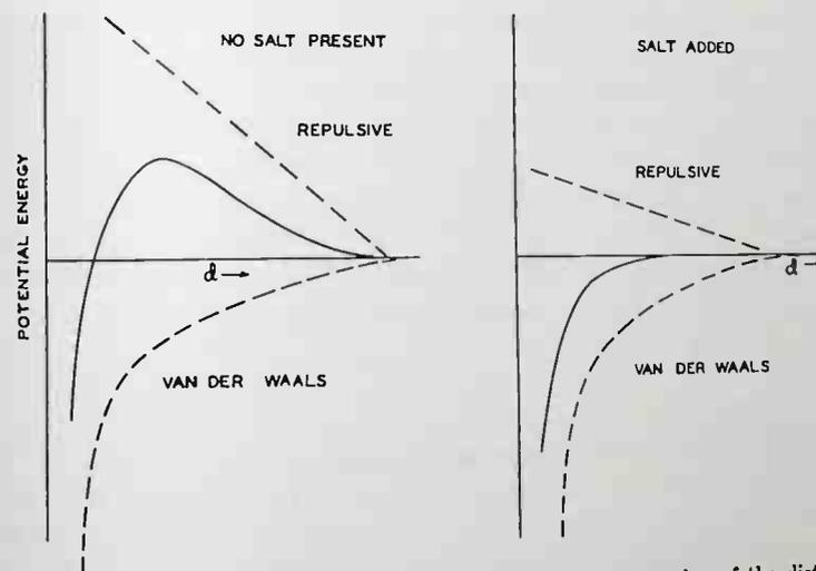
Fig. 11. The potential energy of two gold particles as a function of the distance between them (schematic). The dashed curves represent the two components of this potential—the repulsive of the diffuse double layer and the attractive van der Waals potential.
