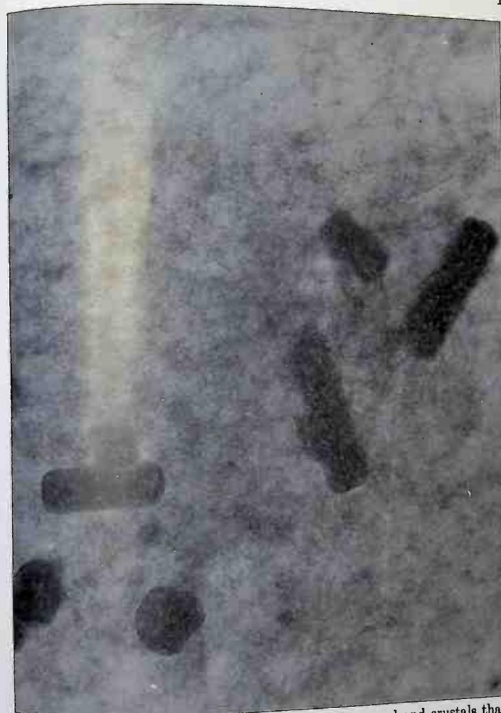
FIG. 5. Aged aluminum oxide sol. Note fibers in background and crystals that are formed from them. Magnification 166,667 $\times$ .
