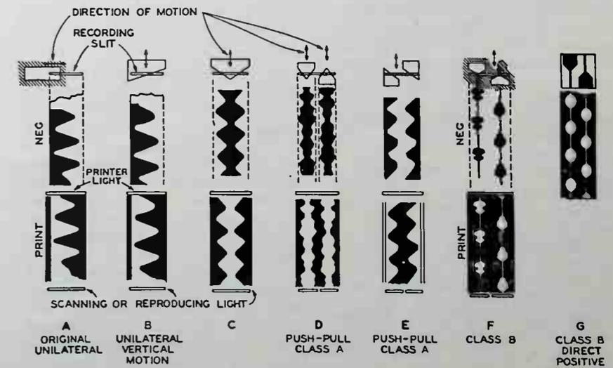
Fig. 14. Various types of area soundtracks, and light-spot shapes which produce them.
