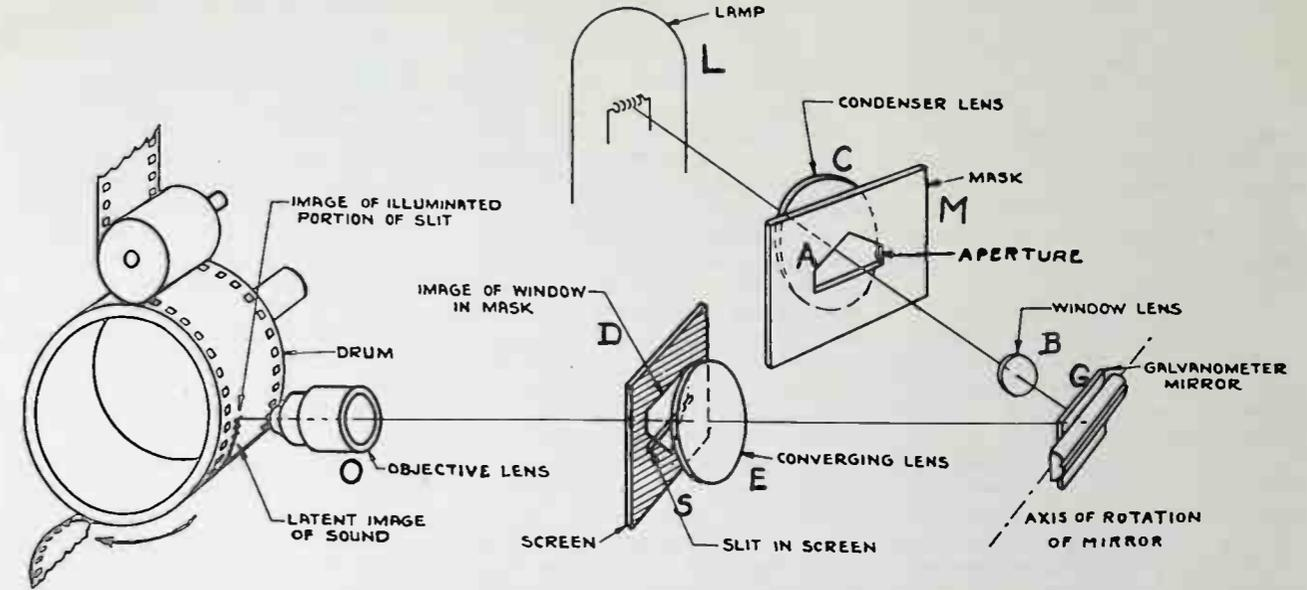
Fig. 13. Variable-area recording optical system. (Lens B images A on slit-plate D.)
