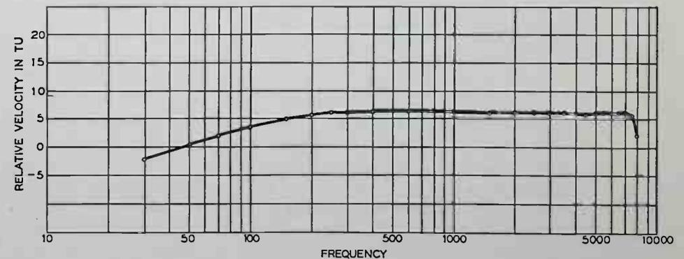
Fig. 3—Frequency characteristic of a recent laboratory recorder.
