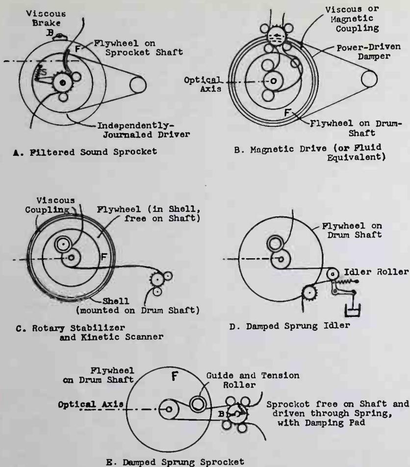
Fig. 4. Mechanical filter systems for reducing irregularities in film motion.
