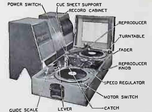
Fig. 9—Cabinet for reproducing from disc records not synchronized with pictures.
