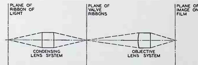
Fig. 2—Optical system for studio recording.
