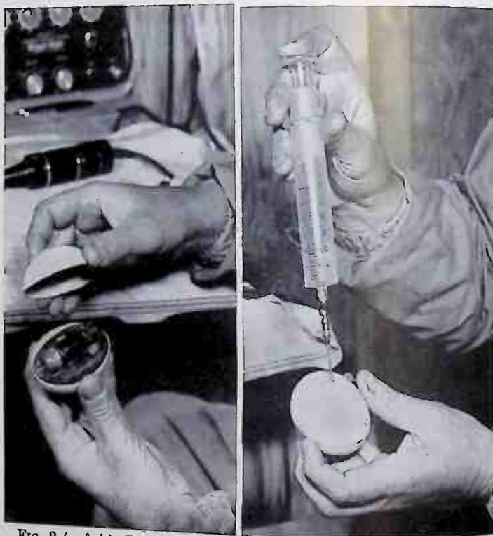
FIG. 2 (a & b). The radio thermometer and empty penguin egg shell are readied for use. Left, the telemeter is placed in shell. Right, albumen is injected into sealed shell.
