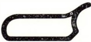
Figure 14-18. Typical shape of a coaxial coil.
