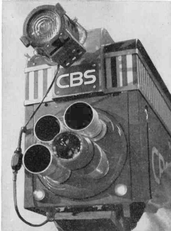
FIG. 14-12. A small incandescent spotlight mounted on the front of a television camera is an effective way to provide eyelight on close-ups. The two tally lights in the lower corners of the camera front provide a visual cue to performers indicating when the camera is in use.
