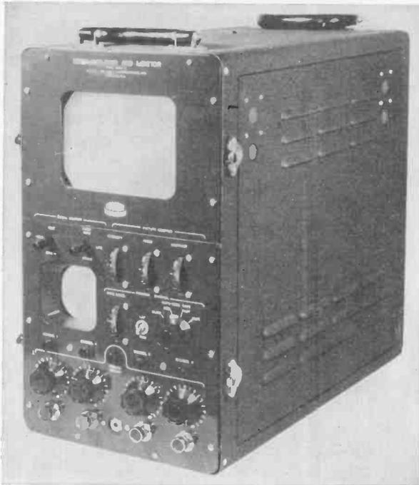
FIG. 3-3. A portable video switching unit that incorporates, in addition to the usual manual controls, automatic means for dissolving from one camera output to that of another. (Courtesy of Allen B. Du Mont Laboratories, Inc.)
