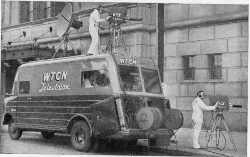
FIG. 3-16. A mobile television unit that has provisions for accommodating a two- or three-camera chain and a microwave relay-link transmitter (seen set up on the roof of the unit). (Courtesy of WTCN-TV, now WCCO-TV, Minneapolis.)
