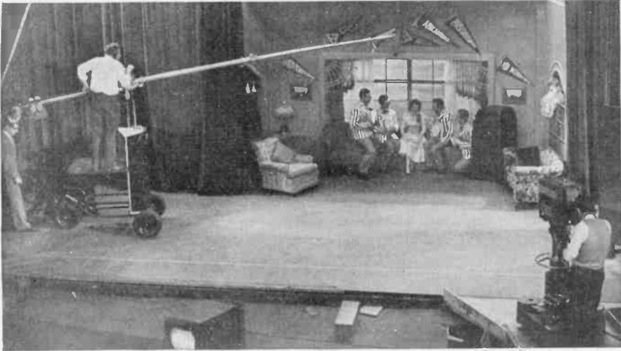
FIG. 6-19. This microphone boom is extended 17 ft, thereby placing a microphone over the scene of action without having to encroach upon the set.
