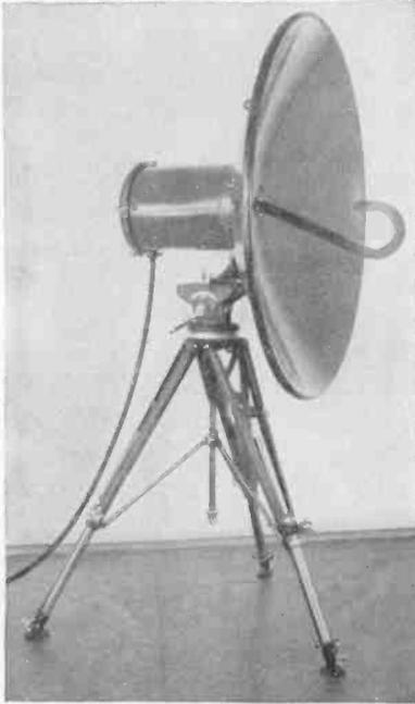
FIG. 3-25. A 4-ft-diameter parabolic reflector excited by means of a hook-shaped waveguide which, in turn, is fed by a microwave transmitter contained in a weatherproof cylindrical case mounted on the back of the reflector. (Courtesy of Radio Corporation of America.)
