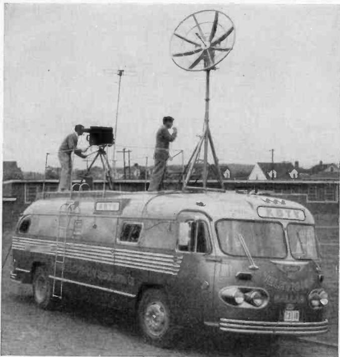
FIG. 3-20. A coach-type mobile unit that houses complete television pickup facilities which are installed, wired, and ready for use as soon as the associated cameras, microphones, and microwave transmitting antenna are set up on location. (*Courtesy of Allen B. Du Mont Laboratories, Inc.*)
