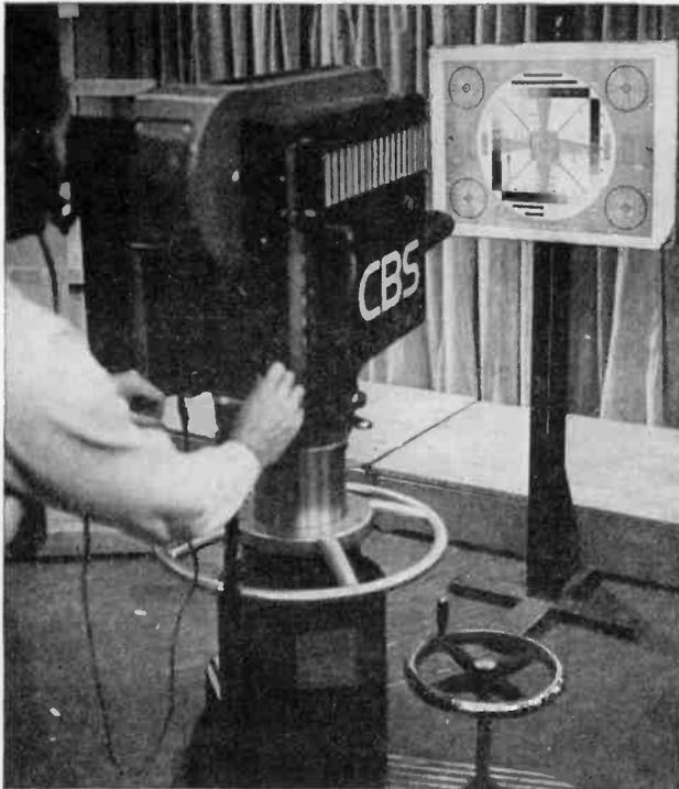
FIG. 16-15. A camera being trained on a standard test chart for resolution measurements and camera alignment purposes.
