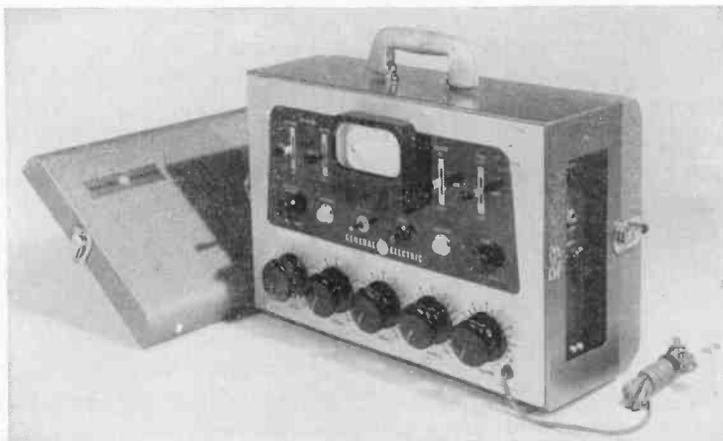
FIG. 3-14. A portable audio amplifier suitable for television field applications which incorporates four preamplifiers, an equal number of associated mixers, a suitable program amplifier, headphone monitoring facilities, and a standard volume-indicator instrument. (Courtesy of General Electric Company.)
