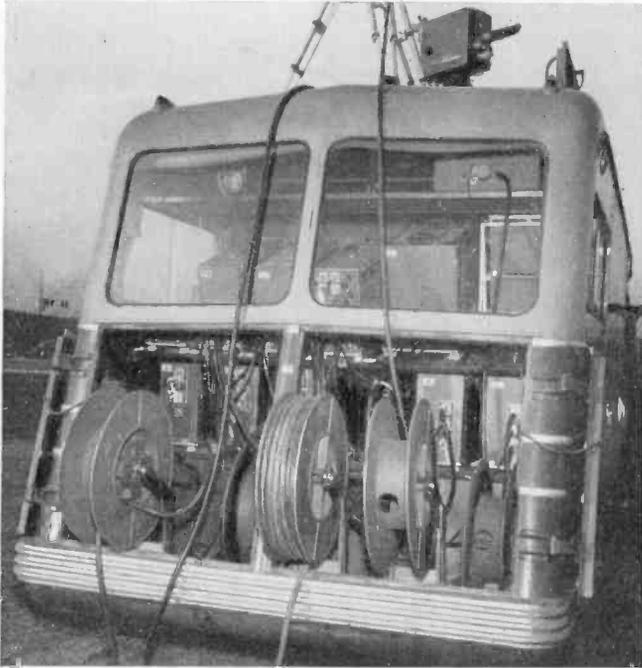
FIG. 3-18. Cable reels for accommodating camera and other cables associated with the mobile unit are carried on reels that swing out from the back of the vehicle to make them more readily accessible. (Courtesy of Radio Corporation of America.)
