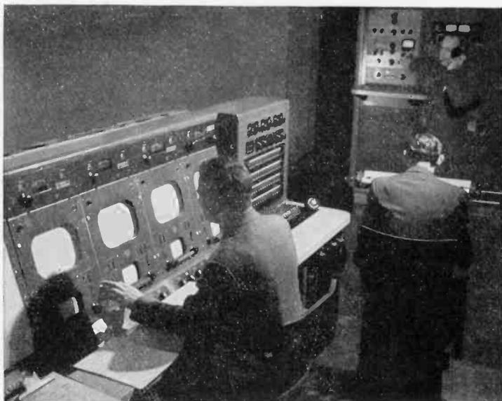
FIG. 14-28. An efficient master control outgoing-line switching console that places essential controls within easy reach of operating personnel. The functions of the various equipments are described in the text.
