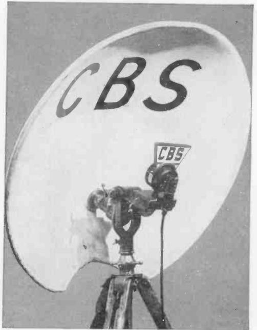
FIG. 3-10. Microphones placed in parabolic reflectors are sometimes useful for picking up distant musical bands or cheering sections at outdoor athletic events.
