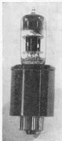
FIG. 5-8. This completely self-contained, plug-in binary scaler unit is only 1 $\frac{3}{8}$  in. in diameter and 3 $\frac{7}{8}$  in. high, including the tube that is plugged into the top of the device.
