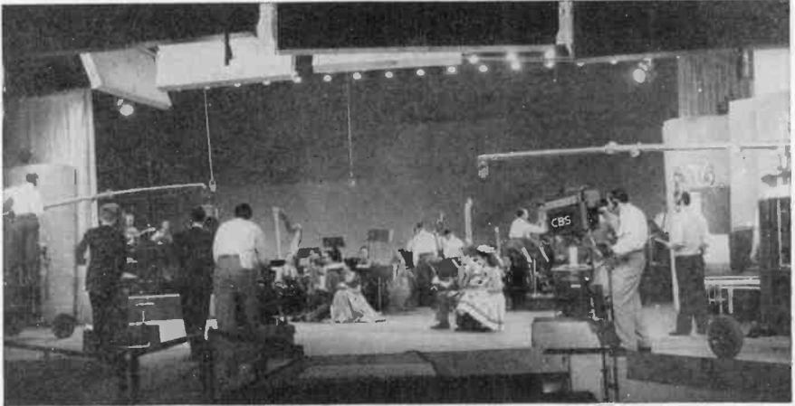
FIG. 6-2. This photograph taken during a rehearsal illustrates the large number of microphones sometimes used on a television program. Visible in this portion of the set are two microphones on booms, two hanging microphones, and two floor-stand microphones. In all, 12 microphones were actually employed.
