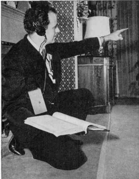
FIG. 6-26. This floor director wears an antenna over his shoulder that supports a low-frequency induction-field receiver whose output actuates the headphones he wears. Thus he is free to move anywhere on the studio floor and still be able to receive instructions from the program director in the control room.
