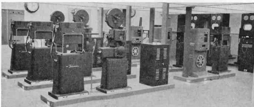
FIG. 14-2. Each of the three 35-mm projectors and the equal number of 16-mm projectors in this corner of the CBS Television City telecine room is provided with its own film camera chain.
