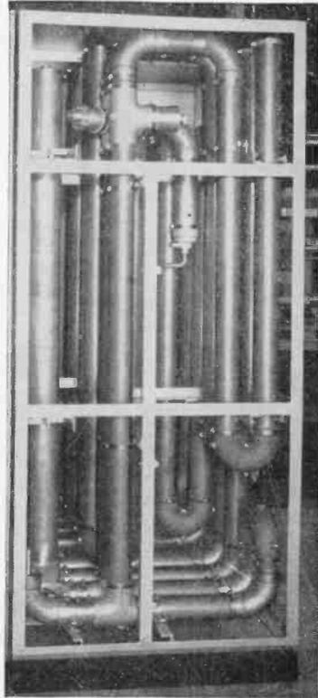
FIG. 13-3. A vestigial sideband filter for the low-frequency v-h-f channels. (Courtesy of Radio Corporation of America.)
