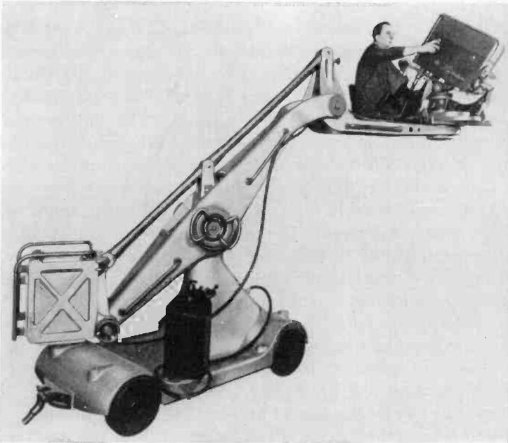
FIG. 6-16. A large camera crane which employs electric-drive motors for moving the unit across the studio floor. The platform carrying the camera and cameraman remains horizontal for all positions of the tongue. (Courtesy of Houston-Fearless Corp.)
