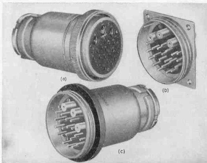
FIG. 15-5. A female camera cable connector is shown at (a) with a corresponding male chassis connector at (b). A male camera cable connector is shown at (c). (Courtesy of Cannon Electric Development Co.)
