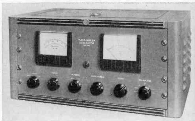
FIG. 16-11. A sweep-frequency generator that covers the spectrum from 100 kc to 10 Mc at a 60-cps rate. (Courtesy of Radio Corporation of America.)
