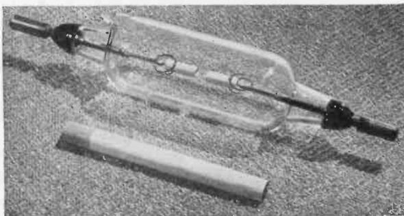
FIG. 9-10. This film-projector flash tube is filled with xenon gas and employs coiled tungsten-wire electrodes encased in ceramic shields. A cigarette is included in the photograph for size comparison. (Courtesy of General Electric Company.)
