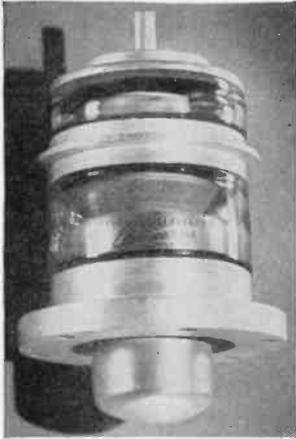
FIG. 13-23. The flanged end of this 9C24 grounded-grid power amplifier tube connects to its plate, the ring seal that separates the two glass portions of the envelope connects to its grid, and the metal cap connects to the cathode. The overall diameter of the tube is  $3\frac{7}{8}$  in. and its length  $7\frac{1}{2}$  in. (Courtesy of General Electric Company.)
