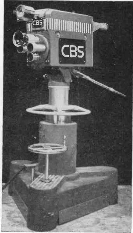
FIG. 6-14. A camera pedestal with the camera-supporting column partially raised. Units of this type are equipped with large rubber-tired wheels and can be readily moved across smooth studio floors by the cameraman.
