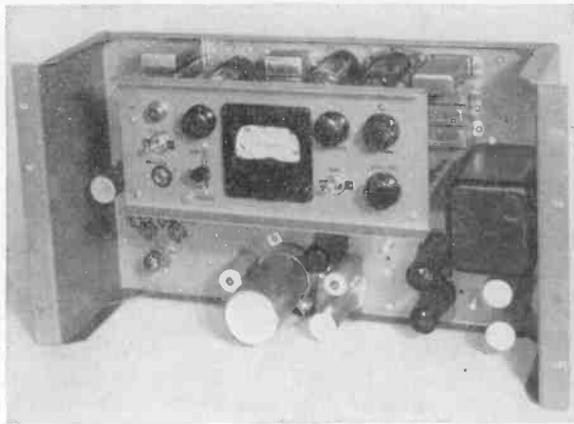
FIG. 3-29. This control chassis for the microwave receiver can be on either a rack or in a carrying case and located an appreciable distance from the microwave receiver and antenna assembly. (Courtesy of Radio Corporation of America.)
