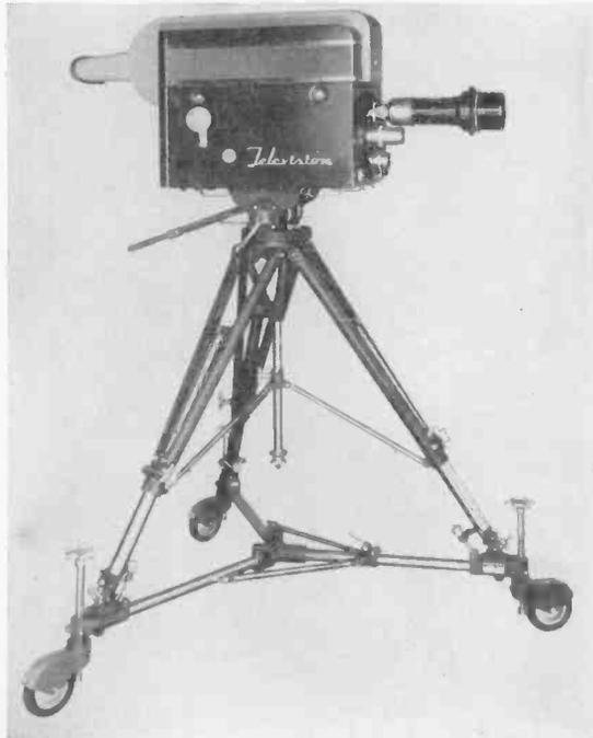
FIG. 3-7. A complete assembly consisting of an image orthicon camera, camera friction head, tripod, and tripod dolly primarily intended for field use but also satisfactory for some studio applications. (Courtesy of Houston-Fearless Corp.)
