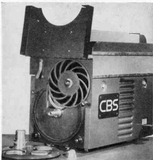
FIG. 17-6. The color filter disk assembly which is added to a monochrome camera to convert it for field sequential color-television operation.
