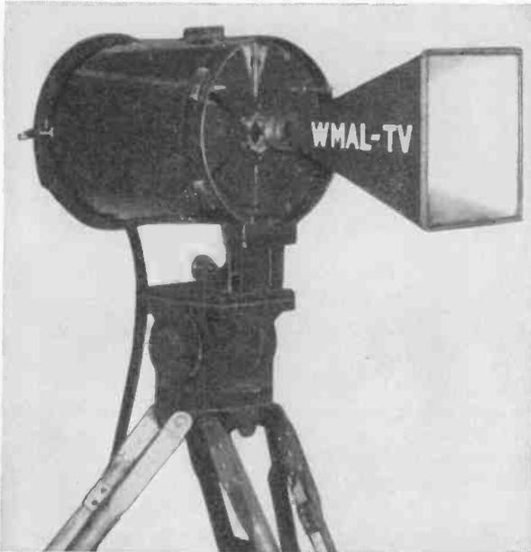
FIG. 3-26. For transmission over short distances, a conveniently small horn antenna of this type may provide all the directivity and gain required for satisfactory operation. (Courtesy of WMAL-TV, Washington.)
