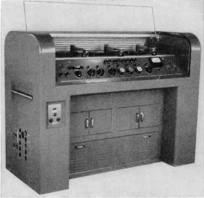
FIG. 6-23. This sound-effects console contains three turntables, continuously variable in speed from 10 to 130 rpm and four pickup arms so arranged that two arms can be used simultaneously on any one turntable. All mixing, amplifying, monitoring, and other supporting equipment is included within the completely self-contained unit.
