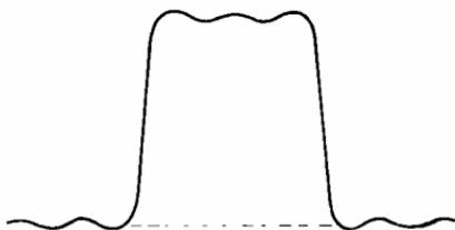
Fig. 2-12. Ideal pulse response of overall tv system.
