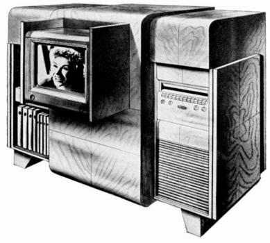
FIG. 8.26A. A DuMont television receiver employing a 20-ineh direct-viewing tube. When not in use, the tube is tilted back into the cabinet.
