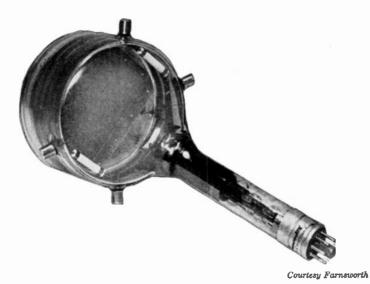
FIG. 1.5. An Iconoscope camera tube.
