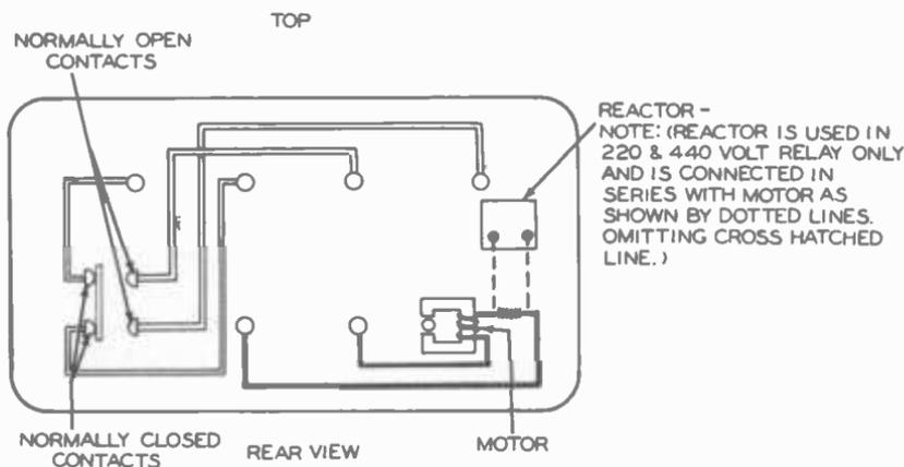
Fig. 8-15. Internal connections of Westinghouse six-terminal type TD (time delay) relay.
