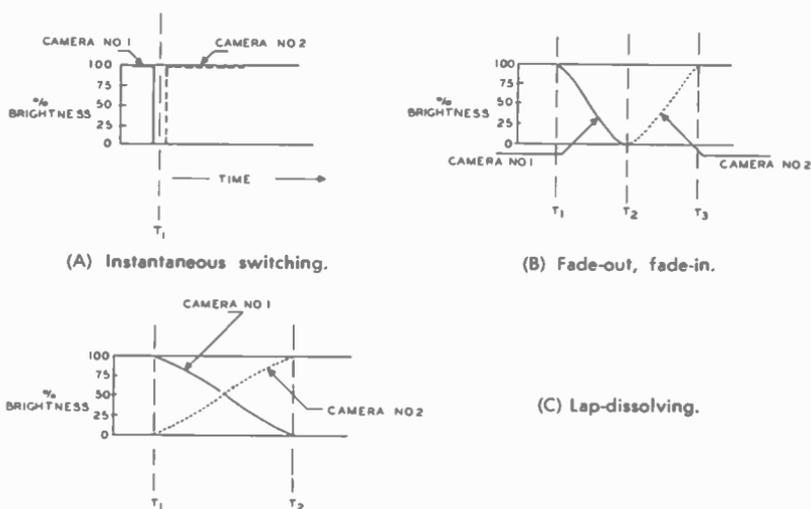
Fig. 4-3. Three of the most common types of video switching techniques.
