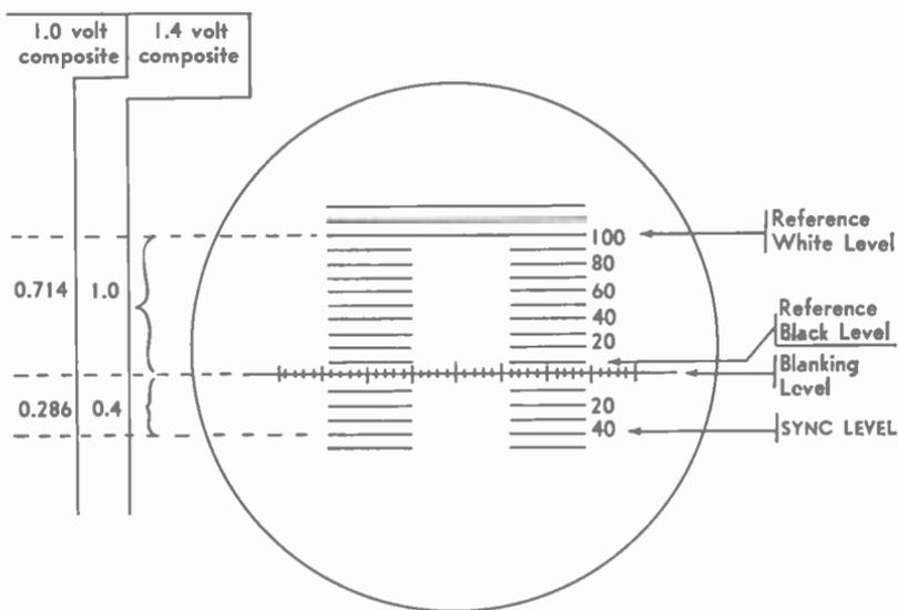
Fig. 2-2. Standard IRE scale showing correlation of 1.0-volt and 1.4-volt signals.
