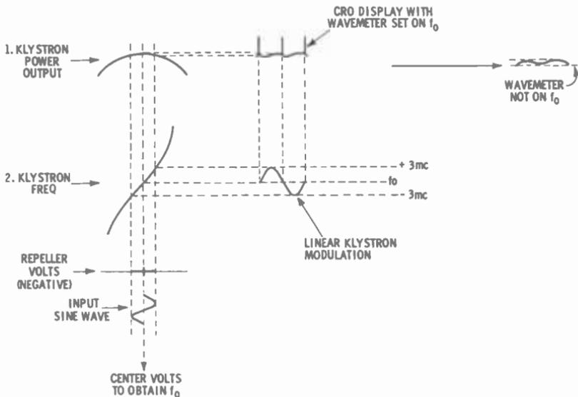
Fig. 7-9. Correct tuning of a transmitter klystron.
