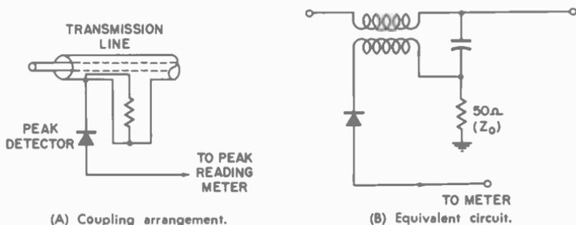
Fig. 8-7. Directional coupling principle.
