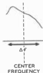
Fig. 8-10. Resultant frequency response curve of an over-coupled double-tuned circuit when the primary and secondary are tuned to different frequencies.
