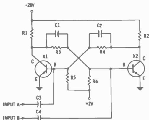
Fig. 3-14. A basic bistable multivibrator.
