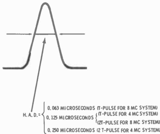
Fig. 5-34. The sine<sup>2</sup> pulse in terms of T and bandwidth.
