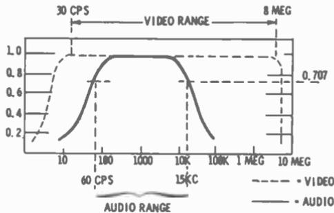
Fig. 5-1. Comparison between the ideal response curves of a video amplifier (dotted line) and an audio amplifier (solid line).
