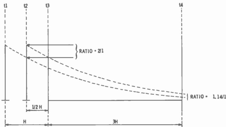
Fig. 3-2. Purpose of the 3H "equalizing interval" before vertical sync.
