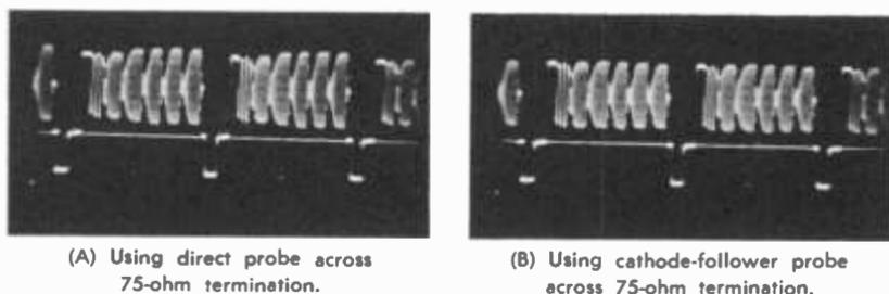
Fig. 1-3. Scope response to keyed sine-wave burst.
