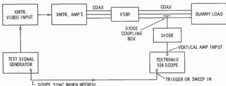
Fig. 8-24. Setup for measuring transmitter frequency response.
