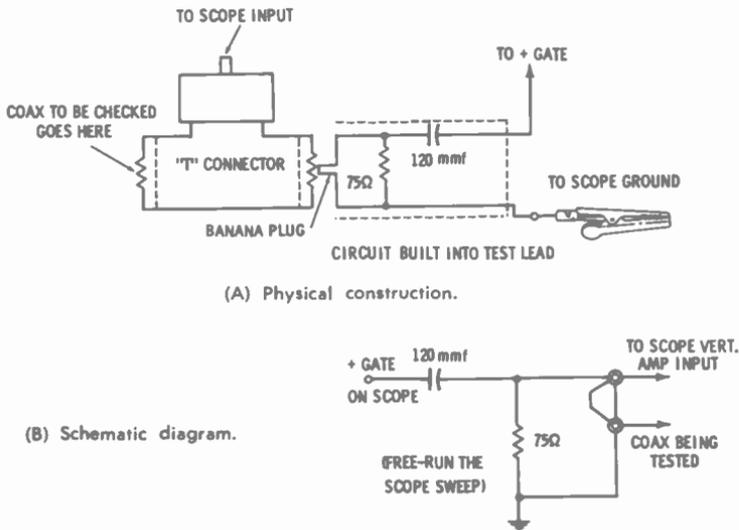
Fig. 3-28. Coaxial line tester for Tektronix 551 and similar scopes.
