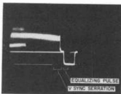
Fig. 1-14. Expanded horizontal sweep showing details of vertical sync serrations and equalizing pulse coincident with horizontal sync.
