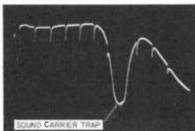
(A) Proper overall response when sound diplexer is used with a subcarrier frequency of 6.8 mc.
