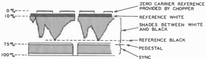
Fig. 8-18. Drawing of typical CRO display of half-tone video signal chopped at 120-cycle rate and displayed with scope sweep of frame frequency (30 cps).
