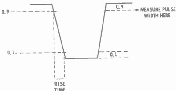
Fig. 3-21. Standard for measuring pulse width and rise time.
