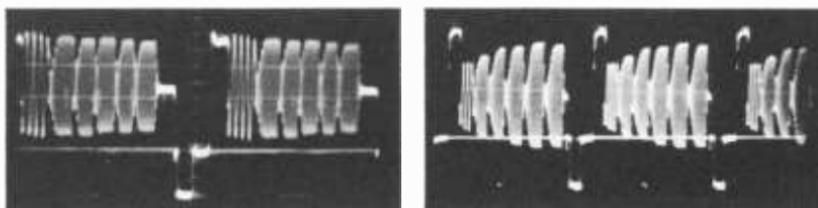
(A) Showing gradual roll-off of highs with increasing frequencies.
