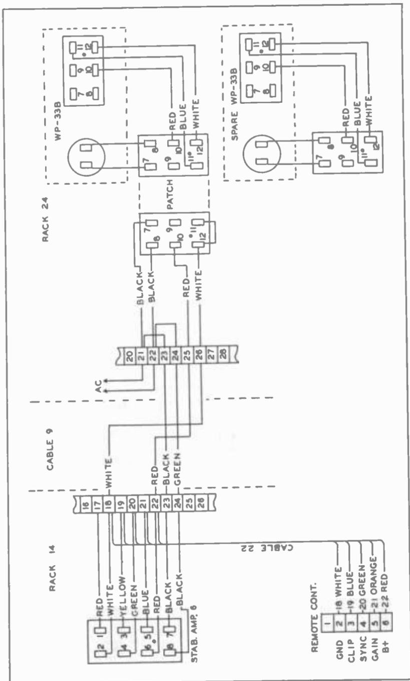
Fig. 2-18. Wiring diagram of the WISH-TV power supply patch system.
