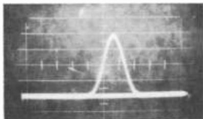
Fig. 5-28. The sine pulse used for phase distortion and transient response checks.
