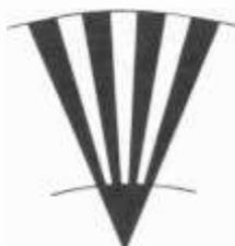
Fig. 5-21. Wedges for visual interpretation of horizontal resolution.
