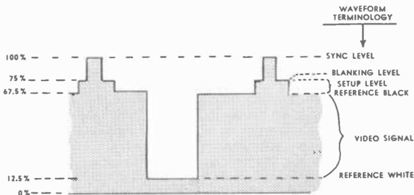
Fig. 2-1. Transmitter carrier representation when modulated with standard window signal.
