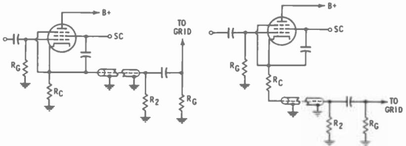
(A) Internal impedance high with respect to coupling network  $R_1$ - $R_2$ . (B) Internal impedance low with respect to coupling network  $R_1$ - $R_2$ .
