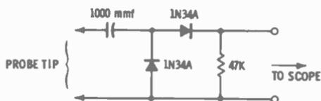
(A) Simplest type with a detected output that is approximately 75% of peak-to-peak value.
