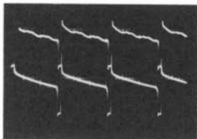
Fig. 3-17. Upper trace shows 31.5-kc waveform with MO on crystal control; lower trace is the same waveform with MO free running.
