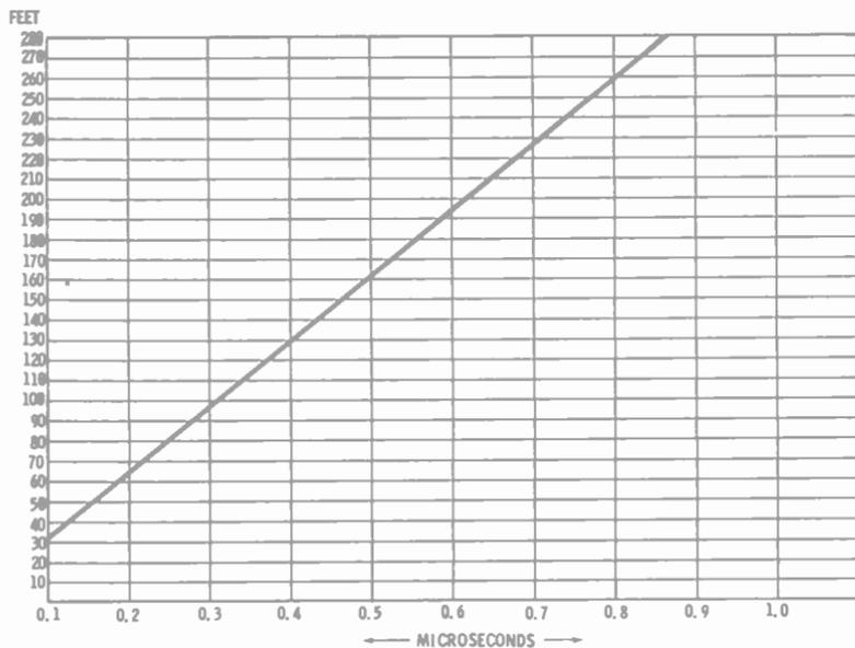
Fig. 3-30. Delay in microseconds versus cable lengths (10 to 280 feet) for propagation factor of 0.66.
