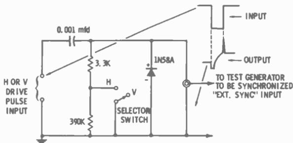
Fig. 5-24. Differentiating circuit designed to obtain positive sync trigger from trailing edge of horizontal or vertical drive.
