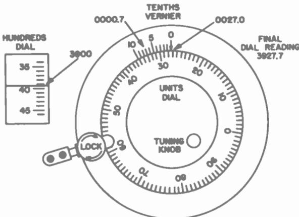
Fig. 1-10. Dial of a typical heterodyne frequency meter.
