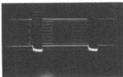
(B) 1-megacycle sine wave with station blanking.
