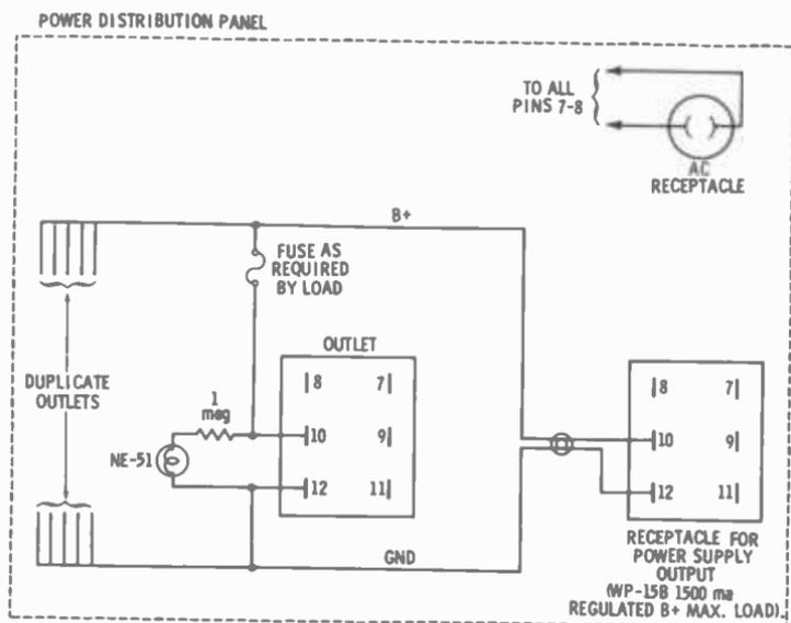
Fig. 2-19. Example of power supply distribution at station WTAE.
