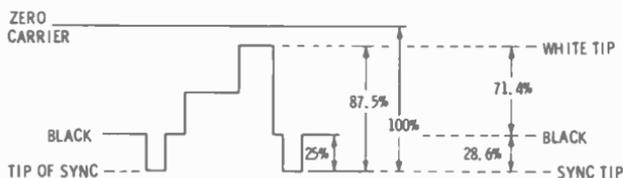
Fig. 8-5. Representation of a CRO display set to indicate depth of carrier modulation. Actual video-to-sync ratio transmitted is same as received, unless compression occurs.
