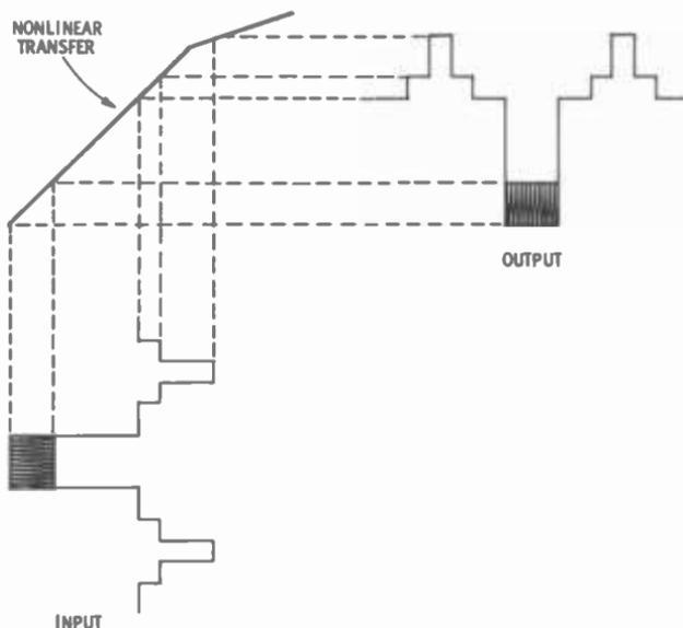
(B) Sync compression (no compression of RF component in white compression).
