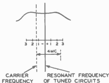
Fig. 8-9. One method of obtaining the required video bandpass while maintaining the proper attenuation of the lower sideband.
