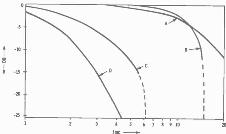
Fig. 1-1. The four major response curves with which the telecasting industry is concerned. (A) "Gaussian" or normal response—gradual roll-off (9 db/octave), rise time approximately 0.035 microsecond. (B) Flat response to 5 or 6 mc. More rapid roll-off than curve A. Rise time approximately 0.035 microsecond. (C) Old IRE curve. Rise time 0.175 microsecond. (D) New IRE curve. Rise time 0.3 microsecond.
