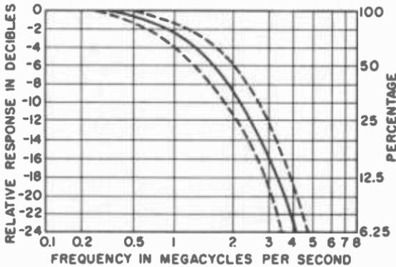
Fig. 2-6. Frequency response for standard oscilloscope (IRE roll-off).
