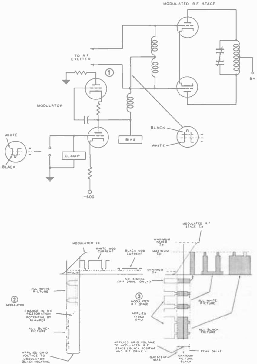
Fig. 8-3. Video modulation fundamentals.
