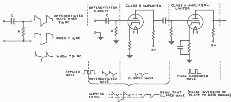
Fig 3-9. Method of obtaining the desired pulse waveshape.
