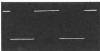
(A) Square wave—very effective for amplitude and phase response checks and setting tilt controls.
