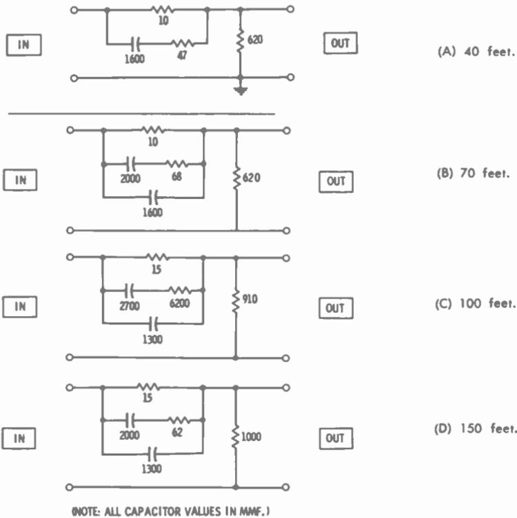
Fig. 4-23. Typical video equalizer circuits for various lengths of cable.
