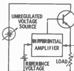
(C) Further stabilized by error gain (amplified correction).
