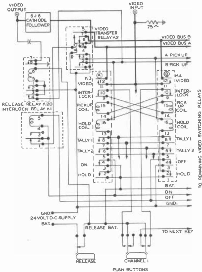
Fig. 4-B. Circuit details of RCA relay switching system.
