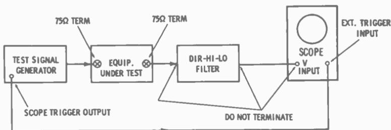
Fig. 6-11. Test setup for checking amplitude linearity and differential gain.
