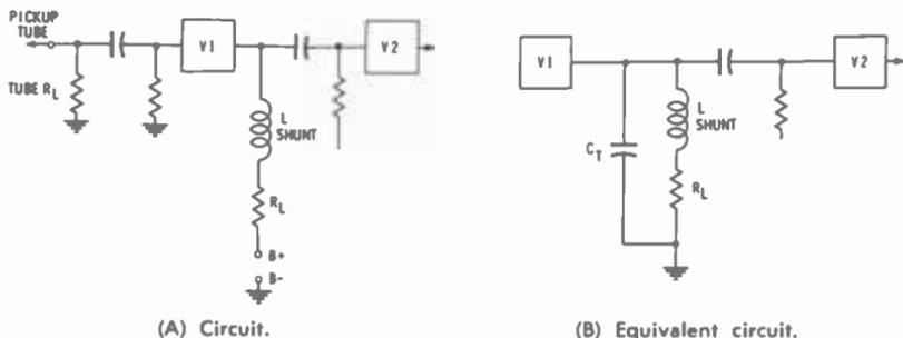
Fig. 5-11. Shunt-peaking compensation.
