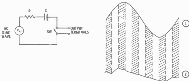
Fig. 5-48. Clamp circuit theory for sine waves.
