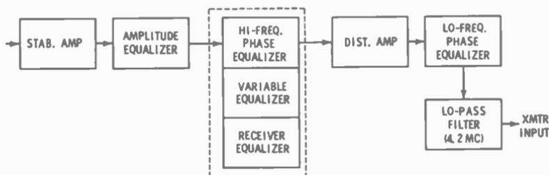
Fig. 8-28. Units employed for color transmitter equalization.
