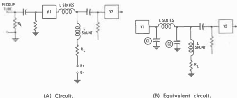
Fig. 5-13. Shunt-series peaking.
