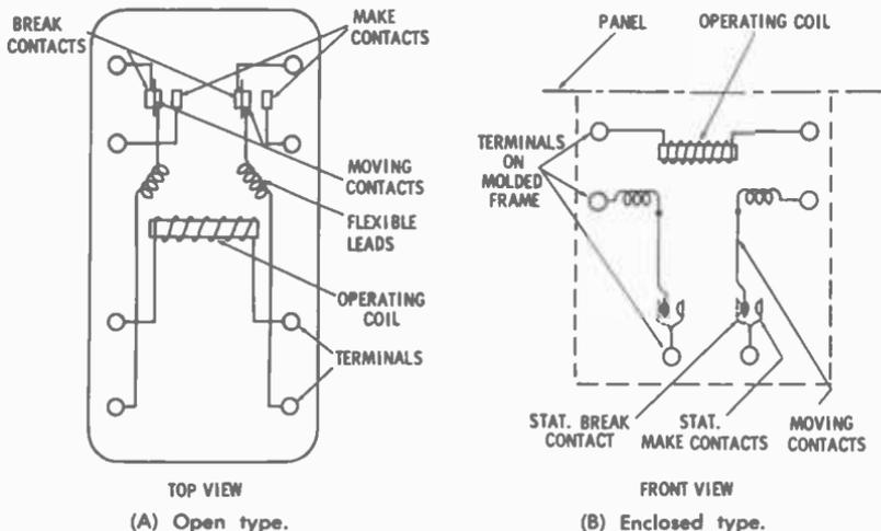
Fig. 8-14. Westinghouse type SG relay.
