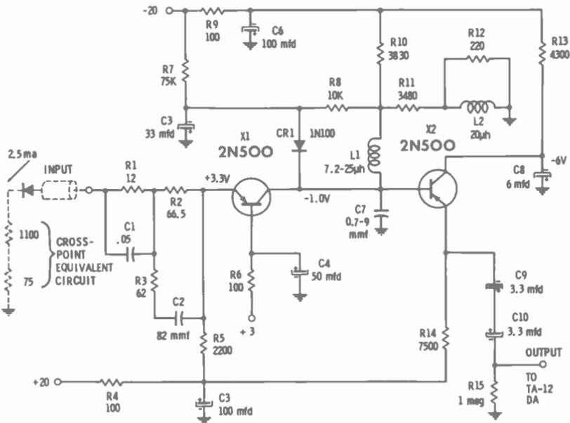
Fig. 4-22. Coupling circuit.
