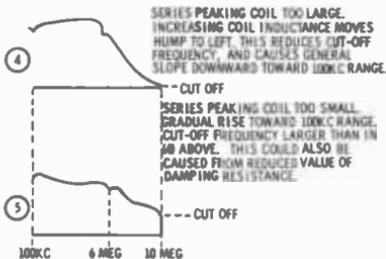
Fig. 5-44. Effect of series-peaking coil on response curve.
