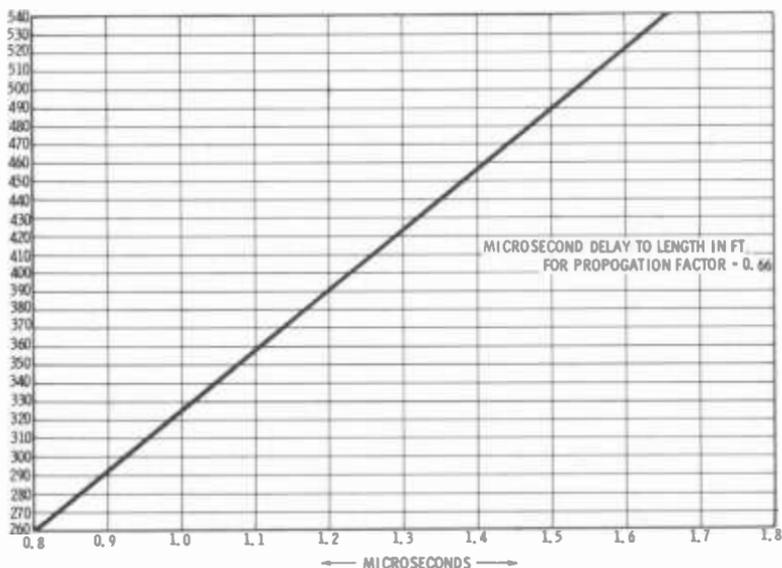
Fig. 3-31. Delay in microseconds versus cable lengths (260 to 540 feet) for propagation factor of 0.66.
