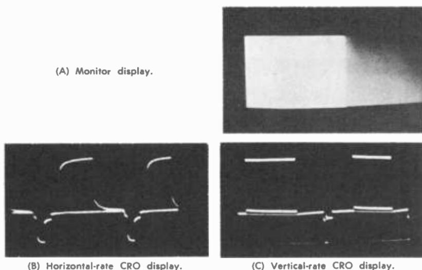
Fig. 5-31. Examples of positive streaking of a window signal.
