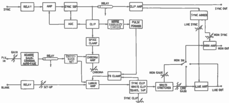
Fig. 5-53. Simplified block diagram of the RCA Model TA-9 stabilizing amplifier.
