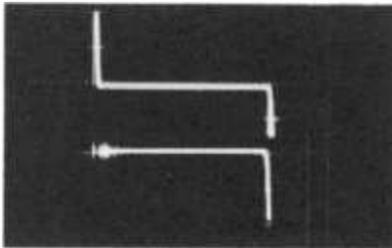
Fig. 2-14. Upper trace shows CRO display of zener diode response; in the lower display the forward trace is eliminated.
