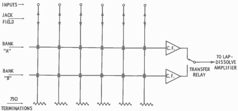
X - RELAY SWITCH FOR PICKUP OF AN INPUT ON A OR B BUS
