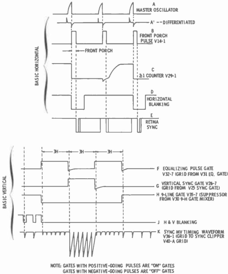
Fig. 3-7. Derivation of pulses with the RCA TG-2A sync generator.
