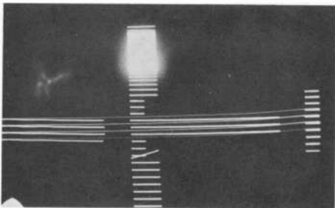
Fig. 3-27. Interlaced pulse-cross display when sync generator has lost interlace. Note the apparent loss of one field.
