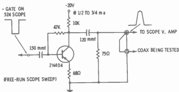
(A) Schematic of the coaxial-line tester.
