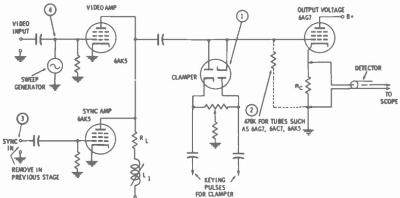
**Fig. 5-51. Typical sync injection and clamping circuit.**
