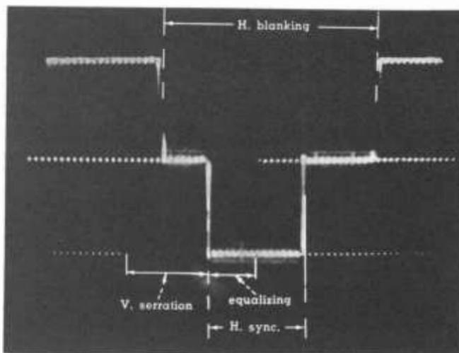
Fig. 3-22. Cross-mixed sync and blanking with 0.005H markers.
