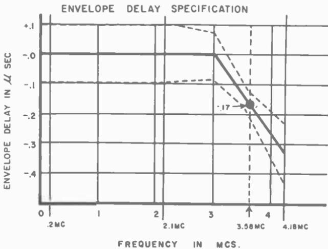
Fig. 8-29. FCC specifications for the transmitter envelope delay curve for color TV transmissions.
