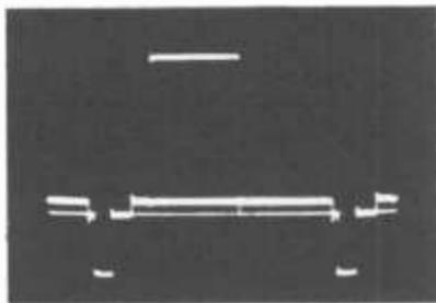
Fig. 5-33. CRO display at horizontal rate showing excessive high-frequency response.
