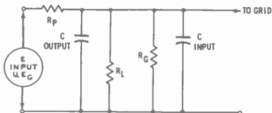
Fig. 5-3. Equivalent circuit for RC-coupled amplifier at high frequencies.
