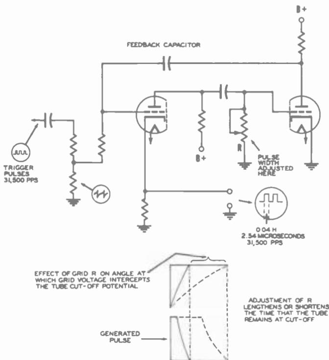
Fig. 3-11. Basic MV circuit employing width control. The timing shown here is for equalizing pulses.
