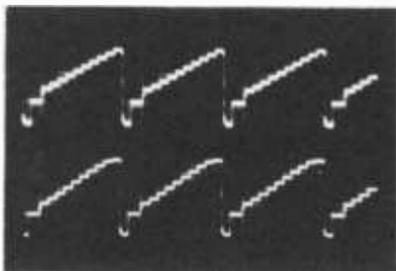
Fig. 6-12. CRO displays through a low-pass filter. Upper trace is input signal; lower trace shows filter output with white compression.
