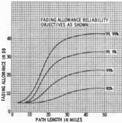
Fig. 7-4. Graph showing fading allowance.
