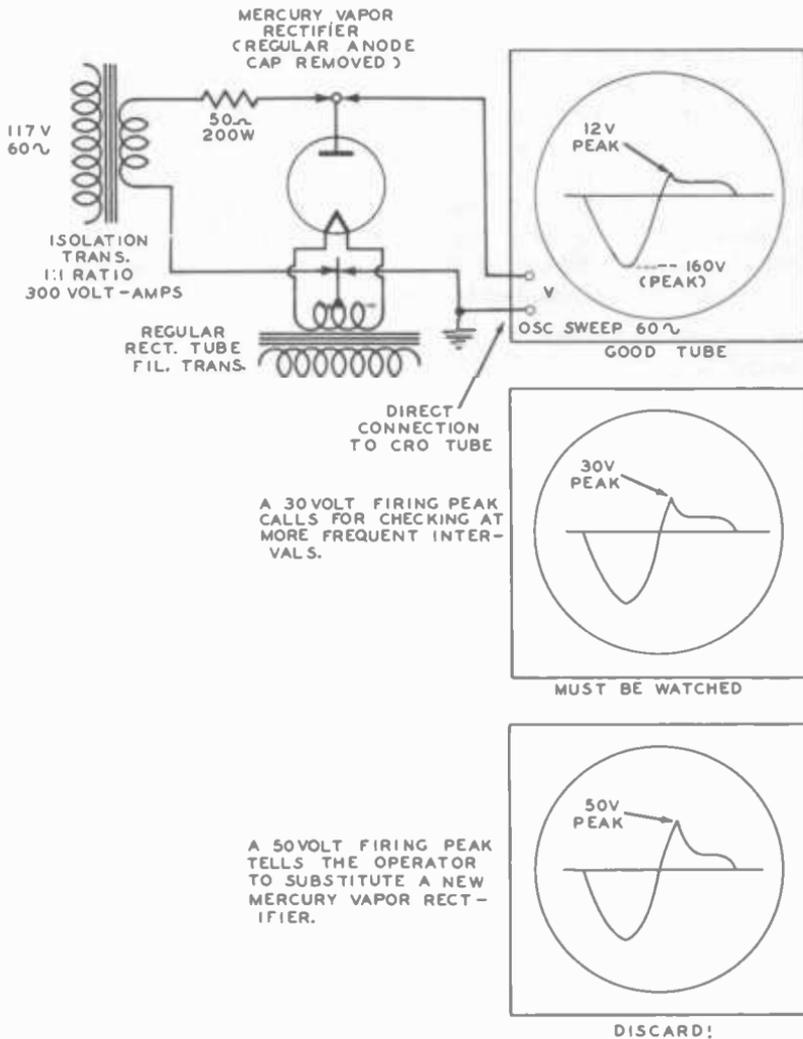
Fig. 8-13. Method of checking mercury vapor rectifier tubes and typical scope displays indicating tube conditions.
