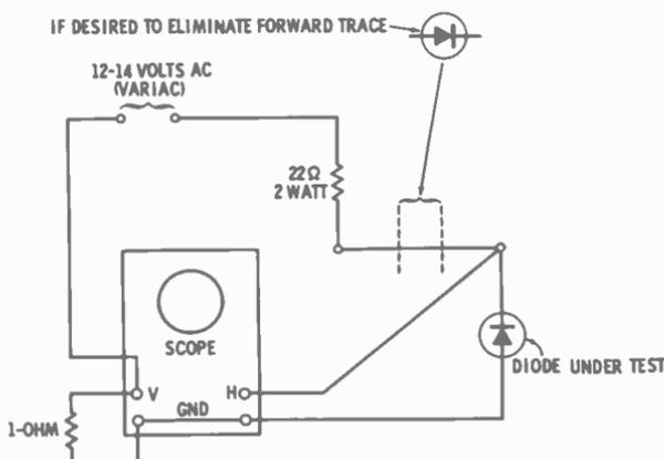
Fig. 2-13. Test setup for checking zener (or any other type) diode.
