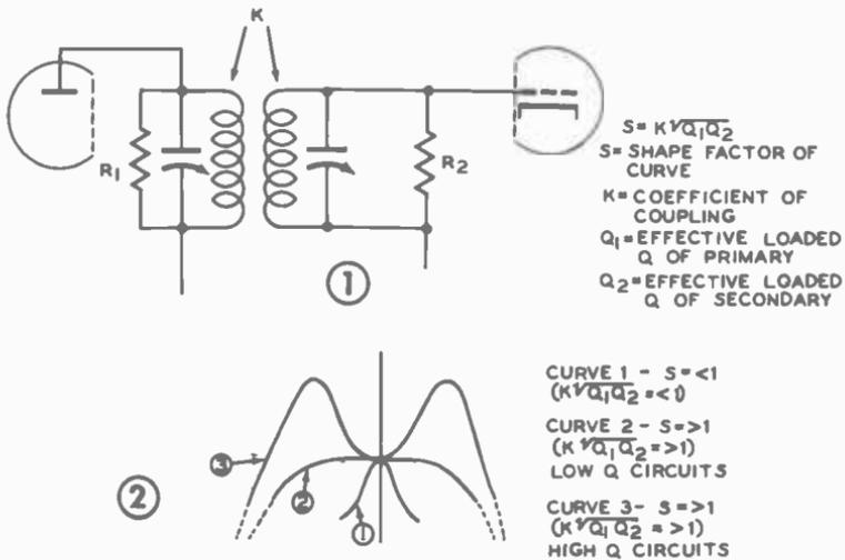
Fig. 8-8. Variable factors of double-tuned circuits.
