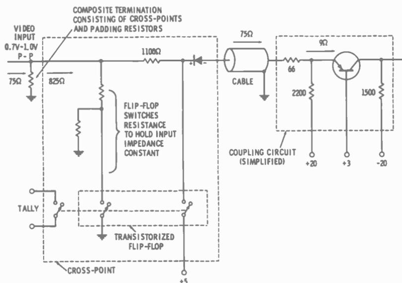
Fig. 4-17. Basic circuit of the RCA TS-40 switcher.
