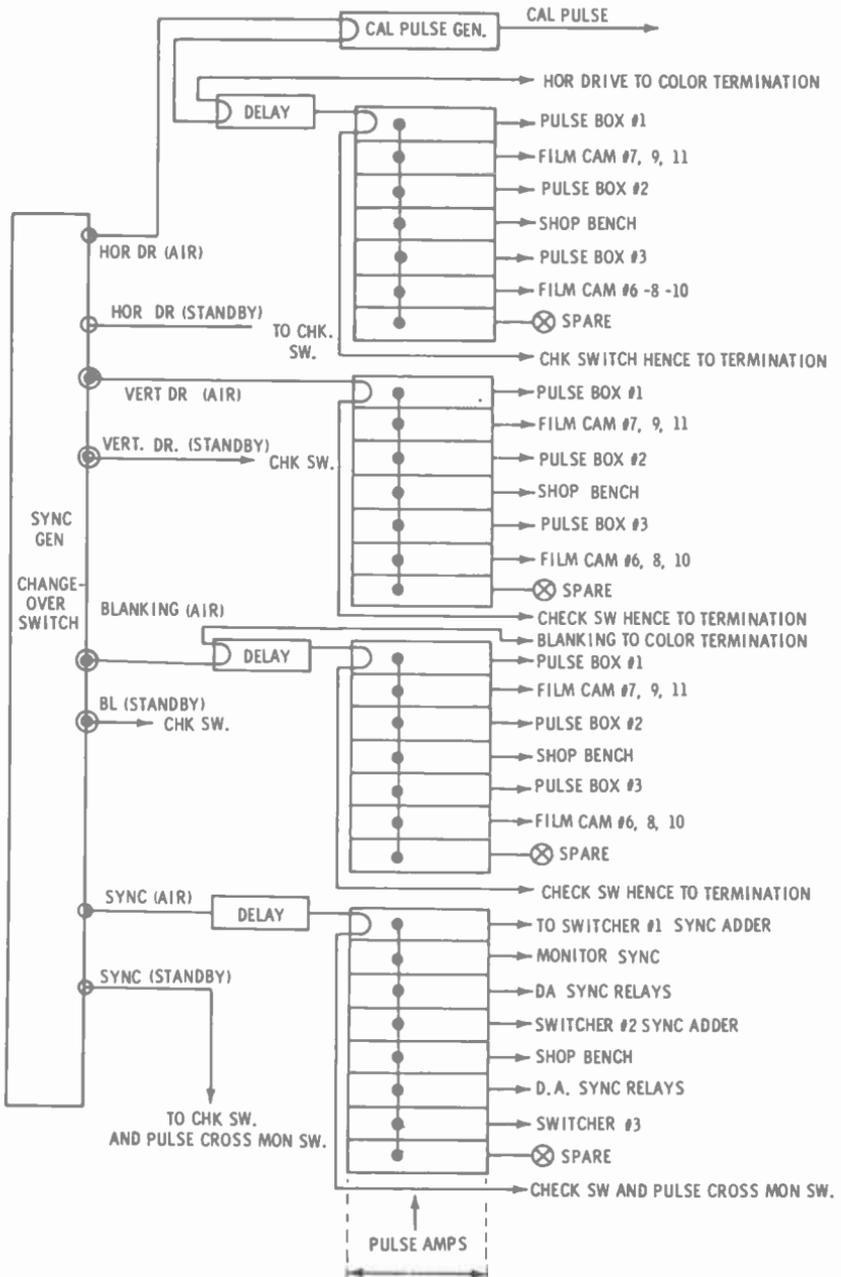
Fig. 3-33. Pulse distribution system of station WTAE.
