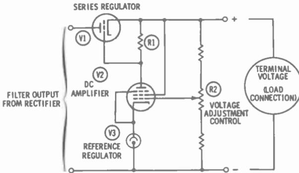
Fig. 2-9. Basic vacuum-tube regulator circuit.
