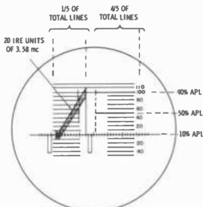
Fig. 6-4. Sawtooth (15.75 kc) with superimposed 3.58 mc at 20 IRE units. When provided with variable APL, the saw occurs once every five lines with fixed levels on alternate sets of four lines to simulate required APL.
