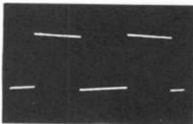
(B) 60-cycle square wave with scope on AC position.
