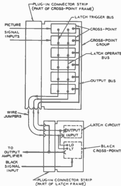
Fig. 4-15. Interconnections between cross-point group and latch-circuit plate.
