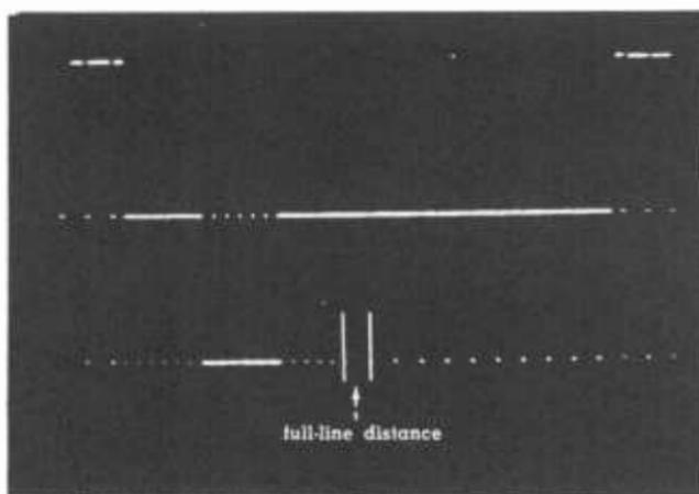
Fig. 3-23. Vertical blanking interval (waveform P of Fig. 3-1) adjusted to  $1.9H$ .
