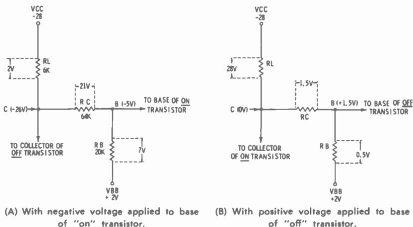
Fig. 3-15. Voltage division of multivibrator circuit for "off" and "on" transistors.
