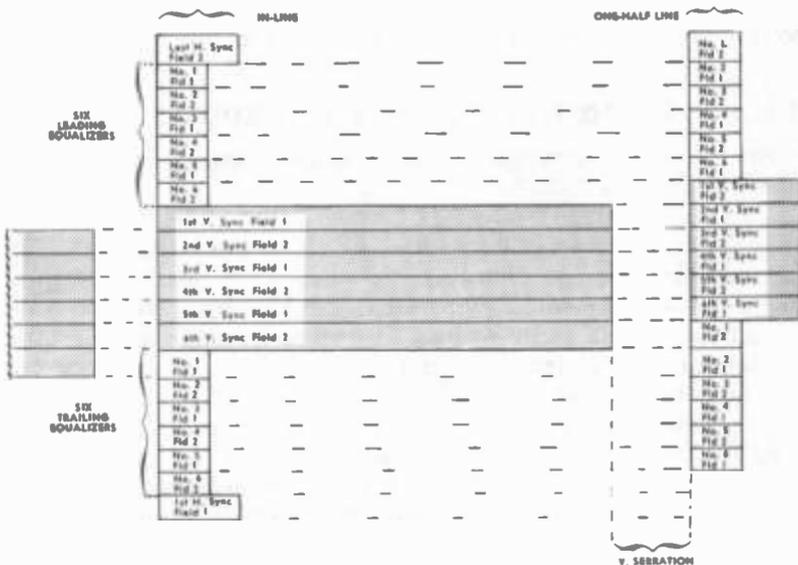
Fig. 3-26. Exploded view of pulse cross with pulse identification.
