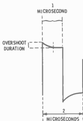
Fig. 1-8. Vacuum-tube cathode interference distortion of a 500-kc square wave.
