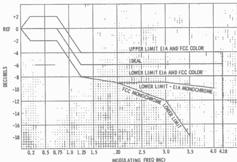
Fig. 8-26. Example of graph plotted to show frequency response characteristics of monochrome and color transmitters.
