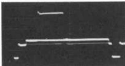
(B) Window—convenient for checking low and middle-frequency response at multiples of line scanning frequency.
