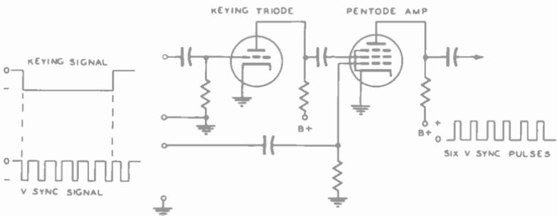
(B) Commercial-type keying-in circuit.
