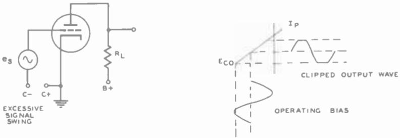
(B) Plate-current cutoff and saturation clipper.
