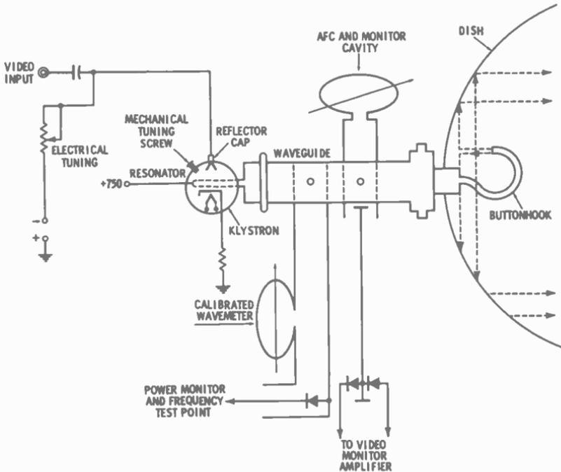
Fig. 7-5. Basic microwave "plumbing."
