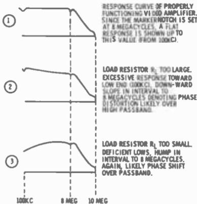
Fig. 5-43. Effect of  $R_L$  on demodulated sweep-generator test signal.
