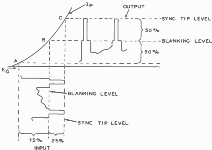
Fig. 5-47. Basic action of sync stretcher.
