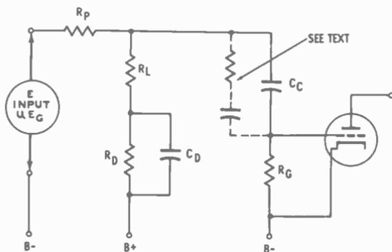
Fig. 5-6. Equivalent circuit of video amplifier at low frequencies with addition of low-frequency decoupling (boost) circuit. To provide equal time constants of the two parallel branches of the load circuit;  $R_L C_D = C_C R_G$ .
