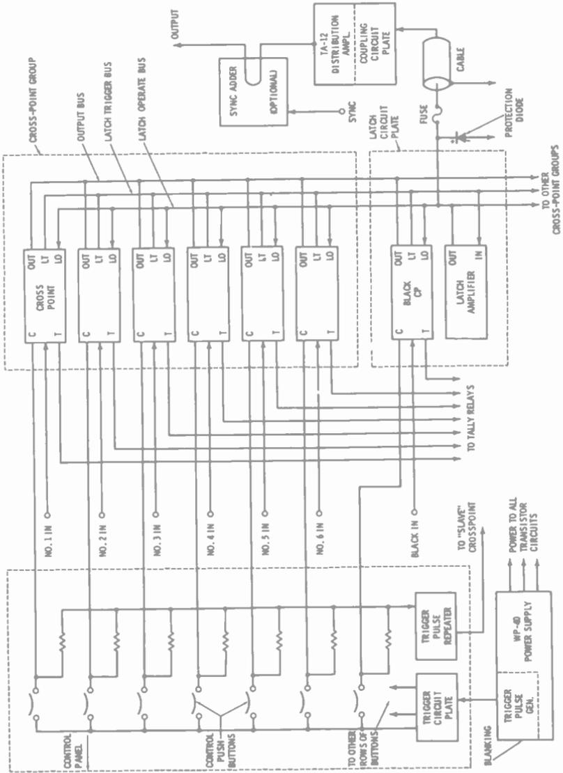
Fig. 4-16. Block diagram of a simple TS-40 system.
