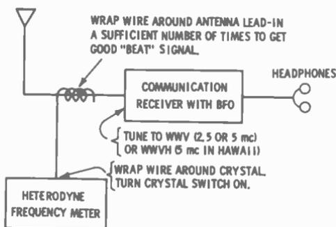
Fig. 1-12. Test setup for zero-beating frequency-standard crystal with National Bureau of Standards transmission.
