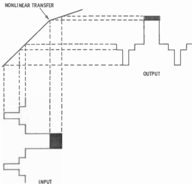
(A) Compression of RF component in the white direction (no sync compression).
