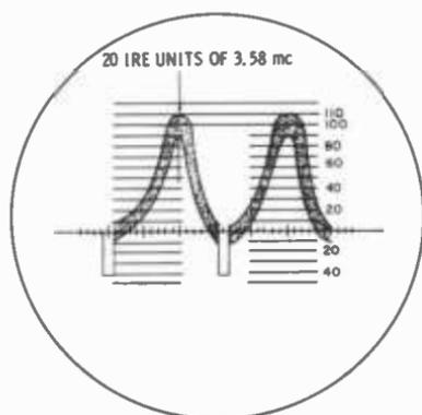
Fig. 6-3. A test signal with a sinusoidal waveform phased with sync to represent a black-to-white transition (and return to black) within a single-line period.
