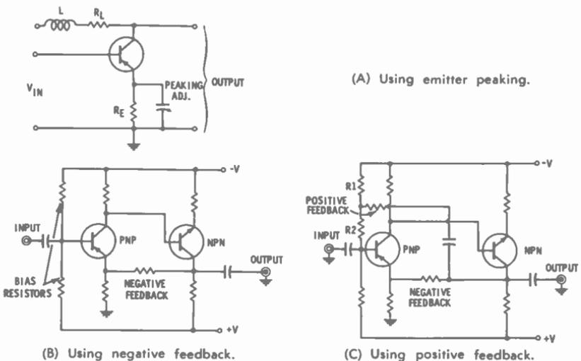
Fig. 5-18. Typical transistor circuits.
