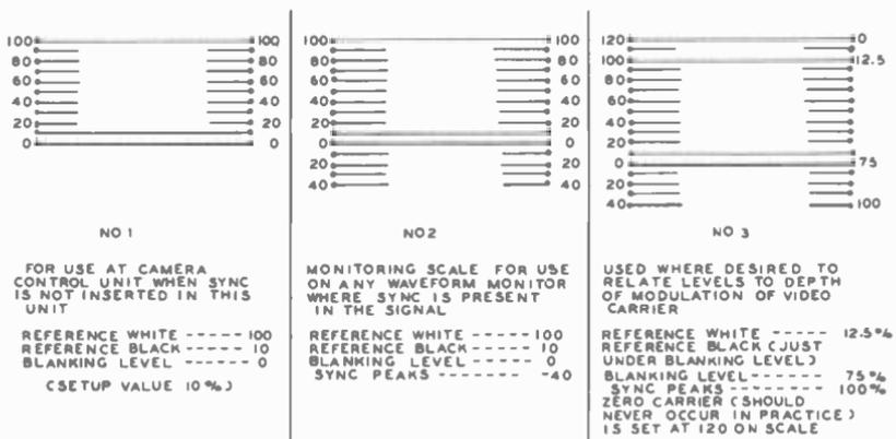
Fig. 2-3. Video level measuring scales recommended by IRE Standards (black negative polarity).
