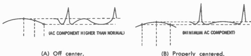
Fig. 7-10. Waveform displays indicating klystron centering.
