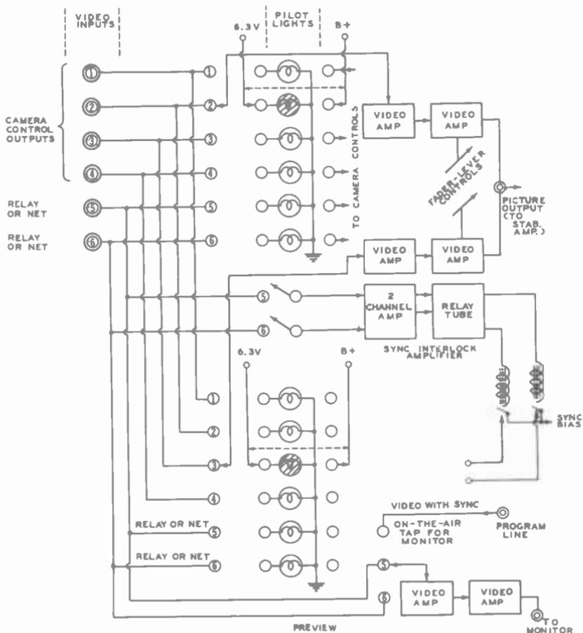
Fig. 4-2. Block diagram of the RCA TS-10 switching system.
