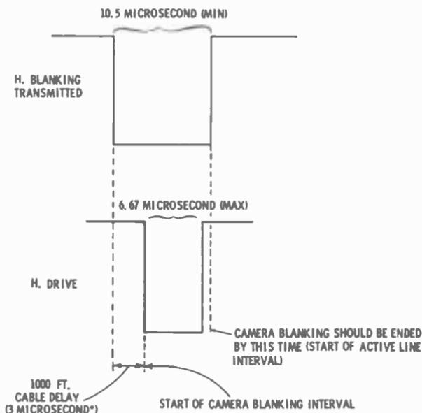
\*SINCE CABLE DELAY IS APPROX 1.5 MICROSECONDS PER 1000 FT, TOTAL DELAY (TO AND FROM CAMERA) IS 3 MICROSECONDS.
