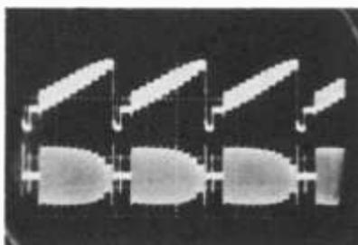
Fig. 6-13. Differential gain in white region. Upper trace shows output signal with filter in "Direct" position; lower trace is output signal with filter in "Hi-Pass" position with increased scope gain.
