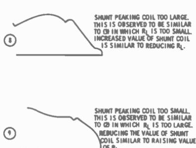
Fig. 5-46. Effect of shunt-peaking coil on response curve.
