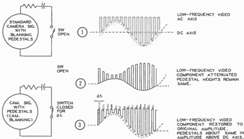
Fig. 5-49. Clamp circuit action for waves broken up by pedestals at a fixed level.
