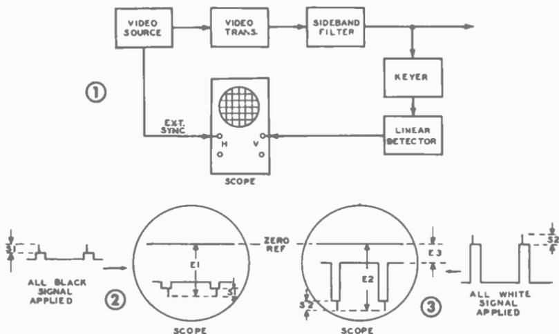
Fig. 8-2. Measuring modulation characteristics.
