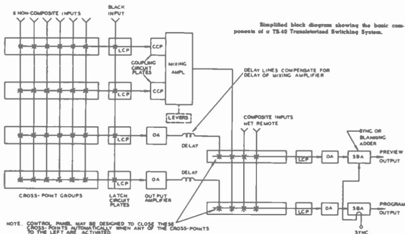
Fig. 4-9. Simplified block diagram of the RCA TS-40 transistorized switching system.
