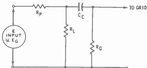
Fig. 5-4. Equivalent circuit of RC-coupled amplifier at low frequencies.
