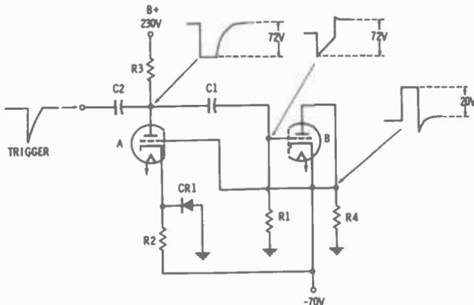
Fig. 3-4. Basic multivibrator circuit.
