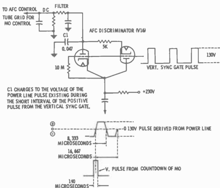
Fig. 3-6. AFC action to maintain constant master-oscillator frequency.
