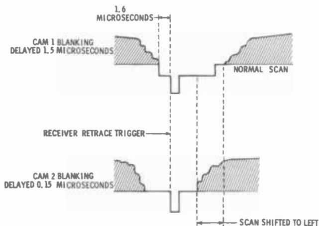
(B) Effect of cable length on scan waveform.
