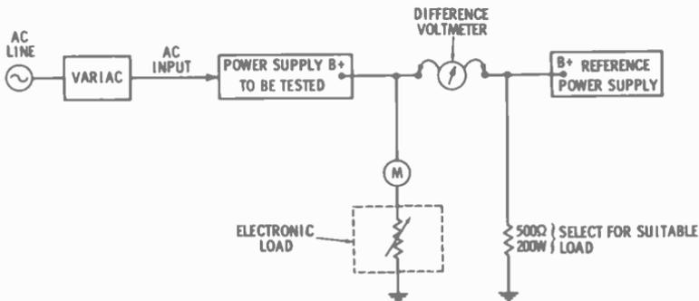
Fig. 2-12. Test setup for checking power supply regulation.
