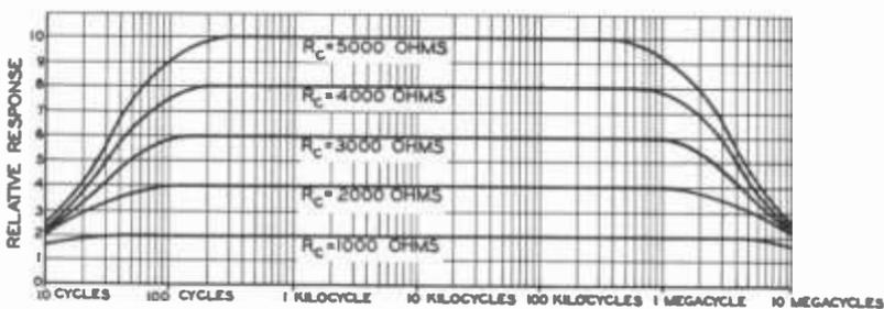
Fig. 5-5. Effect of plate coupling resistor on gain and bandwidth for typical high-transconductance pentode.
