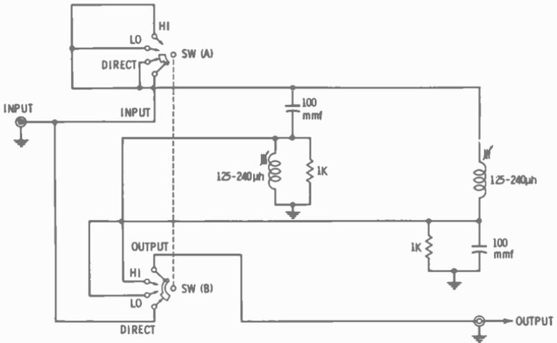
Fig. 6-6. Standard crossover filter for 3.58-mc frequency checks on stairstep.
