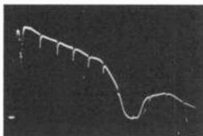
(B) Display showing detected sweep on system with excessive roll-off characteristics.
