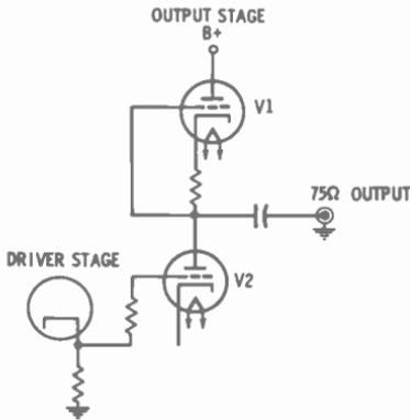
Fig. 5-17. Single-ended, push-pull, output stage.
