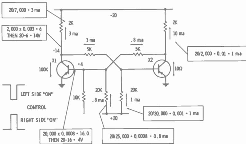
Fig. 4-18. Basic transistorized flip-flop circuit.
