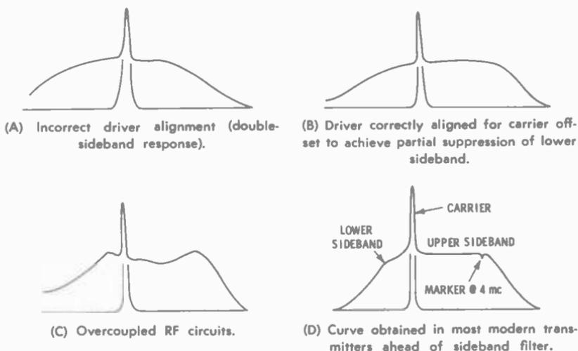
Fig. 8-21. Transmitter tuning with sideband response analyzer.
