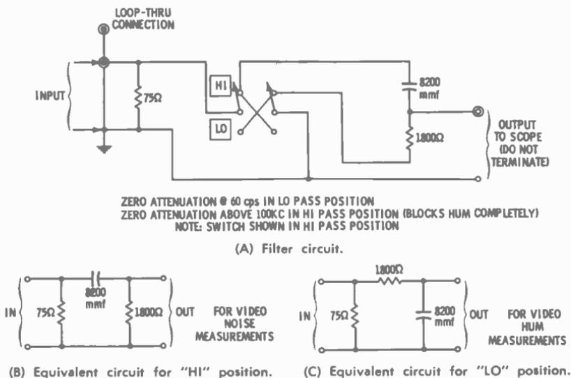
Fig. 7-14. Video filter for STL signal-to-noise measurements.
