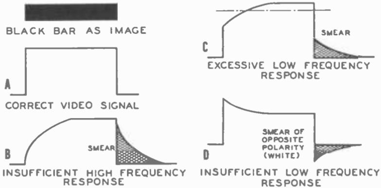
Fig. 5-7. Square-wave video signals showing the effect of amplifier deficiencies.
