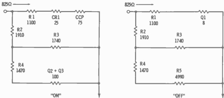
Fig. 4-20. Input equivalent circuits for a cross point.
