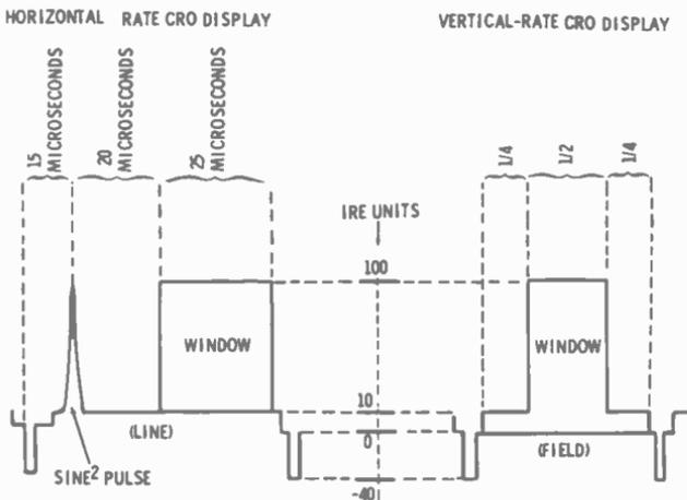
Fig. 5-35. The horizontal and vertical-rate CRO display of the Telechrome Model TMC 1073-D2 Sine<sup>2</sup> Pulse Window Generator.
