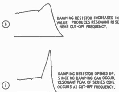
Fig. 5-45. Effect of damping resistor on response curve.
