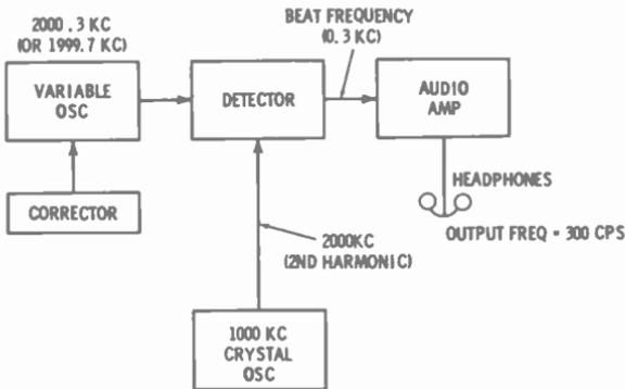
Fig. 1-9. Typical setup for calibrating a heterodyne frequency meter.
