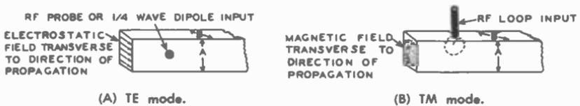
Fig. 7-7. The method of introducing RF energy in a wave guide determines the mode of operation.
