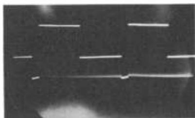
(A) 60-cycle square wave with station blanking.
