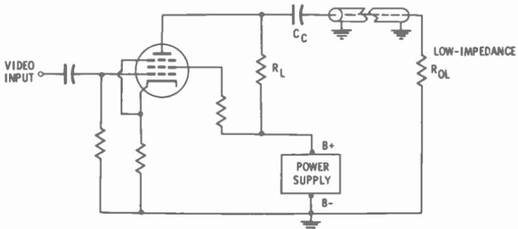
Fig. 5-16. Schematic of typical plate-loaded, video output stage.
