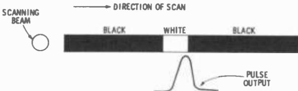
Fig. 5-20. Scanning beam encountering sharp vertical line.
