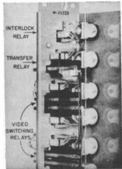
Fig. 4-7. Video switching relays.
