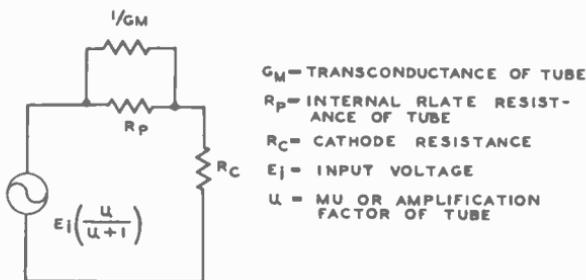
Fig. 5-14. Equivalent circuit of cathode follower.
