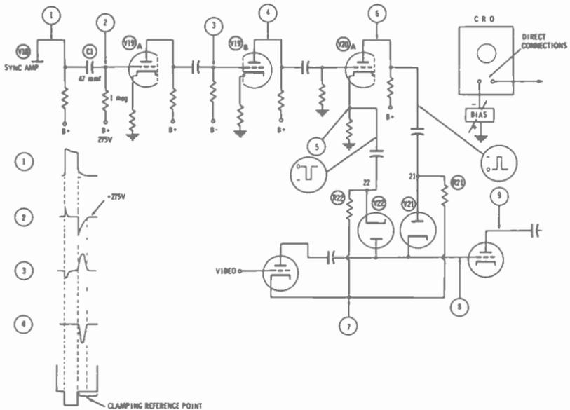
Fig. 5-52. Simplified schematic of one of the clamping circuits in a stabilizing amplifier.
