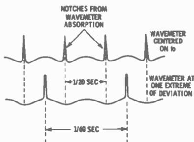
Fig. 7-11. CRO display of wavemeter indication of deviation from center frequency with 60-cycle test signal.
