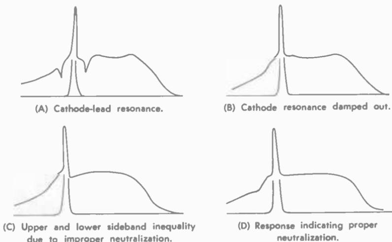
Fig. 8-20. Transmitter adjustments by means of sideband response analyzer.
