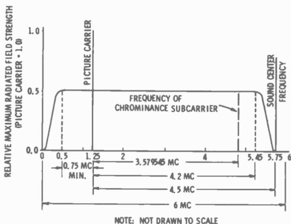
Fig. 8-27. Ideal picture transmission amplitude characteristic.
