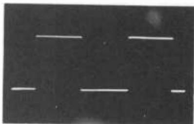
(A) 60-cycle square wave with scope on DC position.
