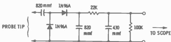
(B) Probe with additional isolation and filtering providing detected output of approximately 50% of peak-to-peak value.
