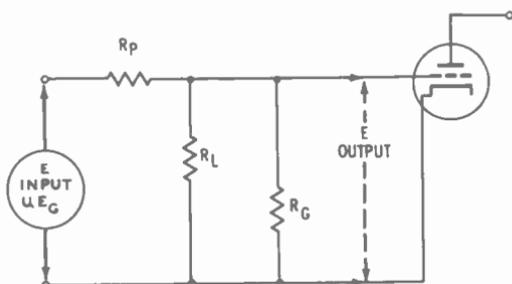
Fig. 5-2. Equivalent circuit for RC-coupled amplifier in mid-frequency range.
