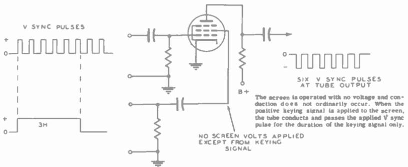
(A) Basic function of keying-in circuit.
