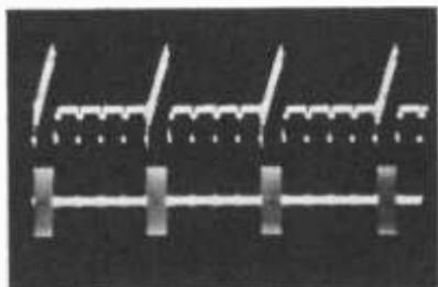
Fig. 6-14. Output of stairstep generator with variable APL adjusted to equal 10% APL. Upper trace shows 1-line-in-5 stairstep signal; lower trace is same signal through high-pass filter.
