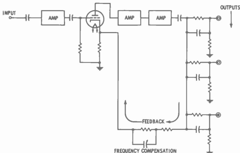
Fig. 5-10. Typical video amplifier circuit with negative-feedback frequency compensation.
