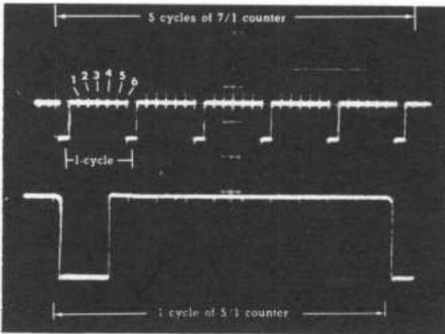
Fig. 3-20. Upper trace is five cycles of 7/1 counter; lower trace shows one cycle of 5/1 counter.
