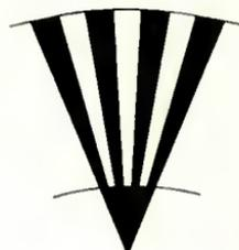
Horizontal resolution is the ability to define vertical lines in the image. The essentially round shape of the scanning spot and the fact that it is not infinitely small places an immediate limitation on the ability to reproduce rapid picture transitions. Thus, when the beam suddenly encounters the sharp vertical line representing transition from black to white (Fig. 1-4), the resulting signal is not a square wave, but more nearly a sine wave.
