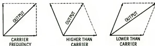
Fig. 4-31. Vector analysis of delay-line demodulator.
