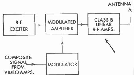
FIG. 36 Block Diagram, Low-Level Modulation TV Transmitter
