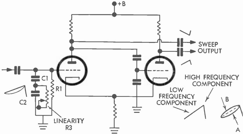
FIG. 170 Linearity Control with  $R-C$  Compensating Circuits
