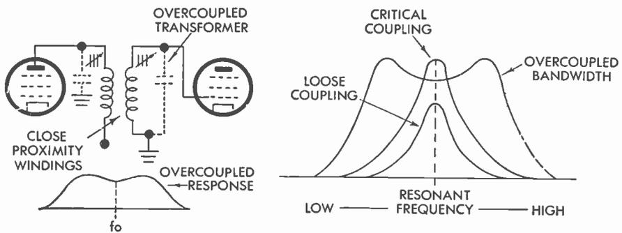
FIG. 40 Overcoupled Transformer
