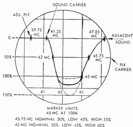
FIG. 73f GE Alignment Curve
