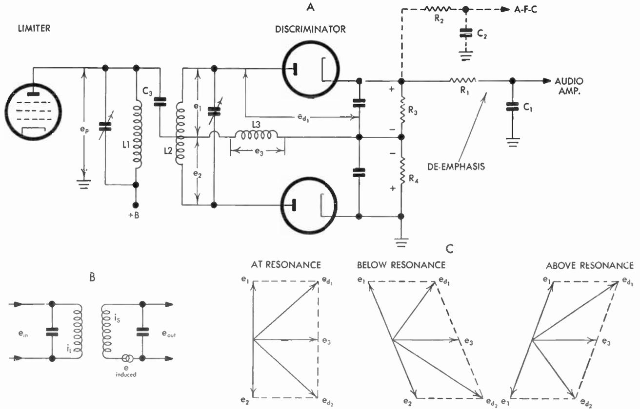
FIG. 198 Conventional Discriminator and Voltage Vectors
