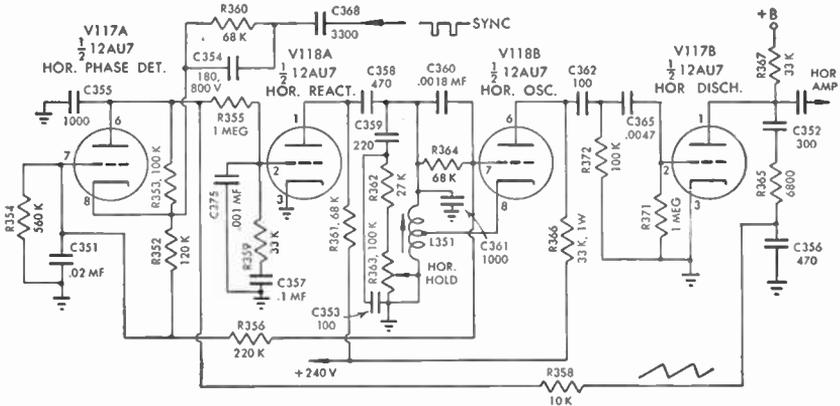
FIG. 150d Phase-Detector AFC (GE)
