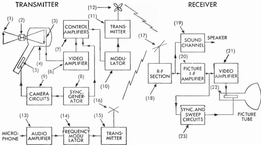
FIG. 1 Functional Diagram of Basic Television System
