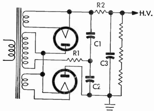
FIG. 125 Voltage-Doubler Supply
