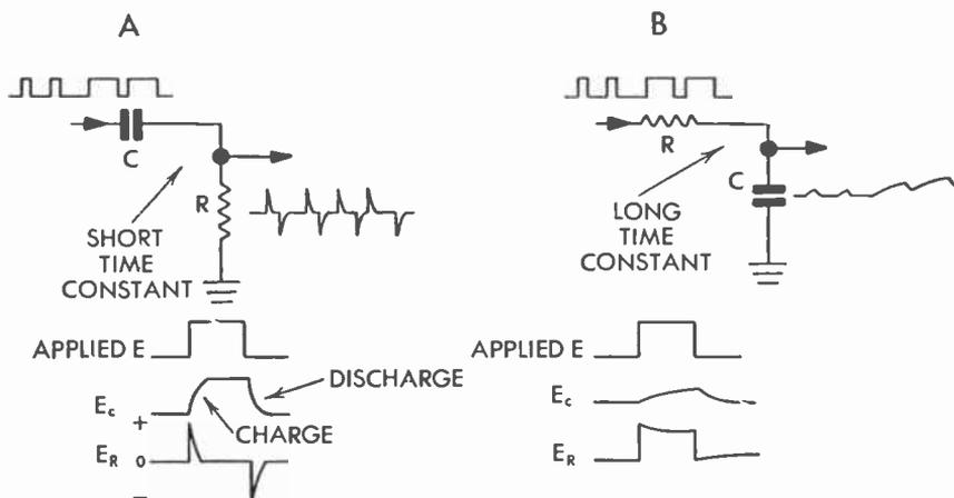
FIG. 142 Differentiating and Integrating Circuits
