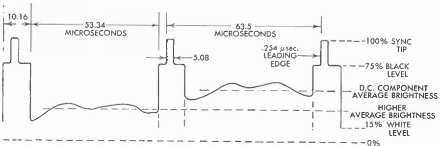
Fig. 24 Signal Distribution for Two-Line Interval, Showing Blanking and Sync Pulses
