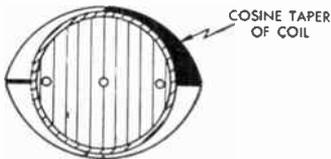
FIG. 185 Uniform Field of Cosine Yoke
