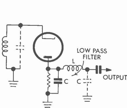
FIG. 82 Bandpass Filter in Output of Video Detector
