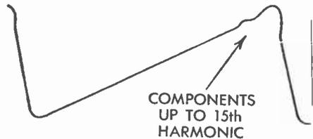
FIG. 13 Components of a Sawtooth
