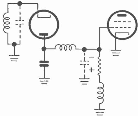
FIG. 83 Direct-Coupling from Video Detector
