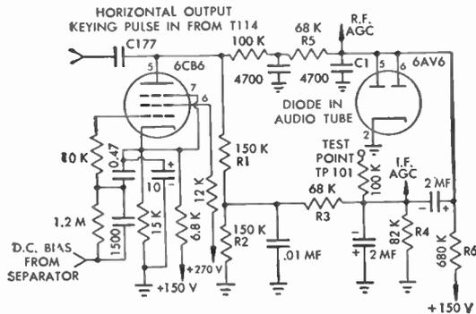
FIG. 104 RCA Keyed A-G-C Circuit
