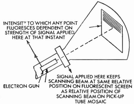
FIG. 3 Scanning at Picture Tube
