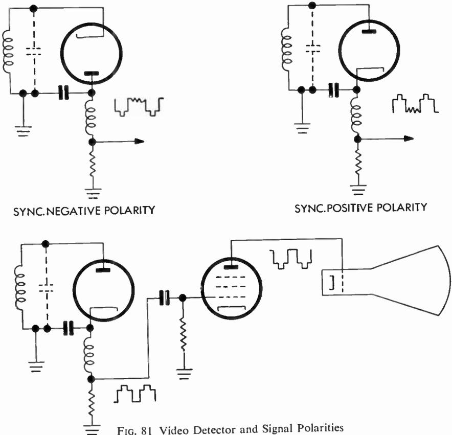
FIG. 81 Video Detector and Signal Polarities
