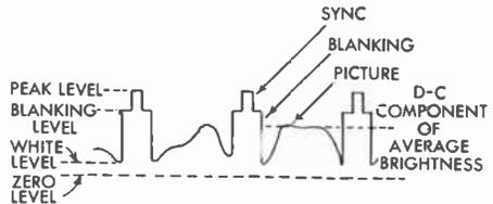
FIG. 15 Portion of Television Signal Showing Uni-Polarity Voltage
