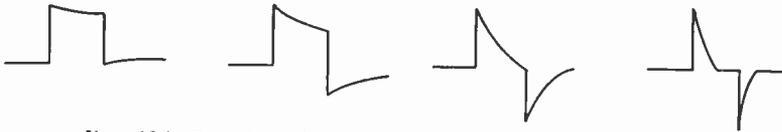
FIG. 136 Poor Low-Frequency Response and Pulse Distortion
