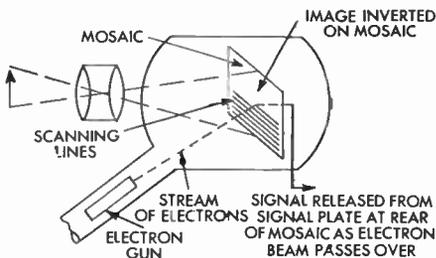
FIG. 2 Scanning with Electrons
