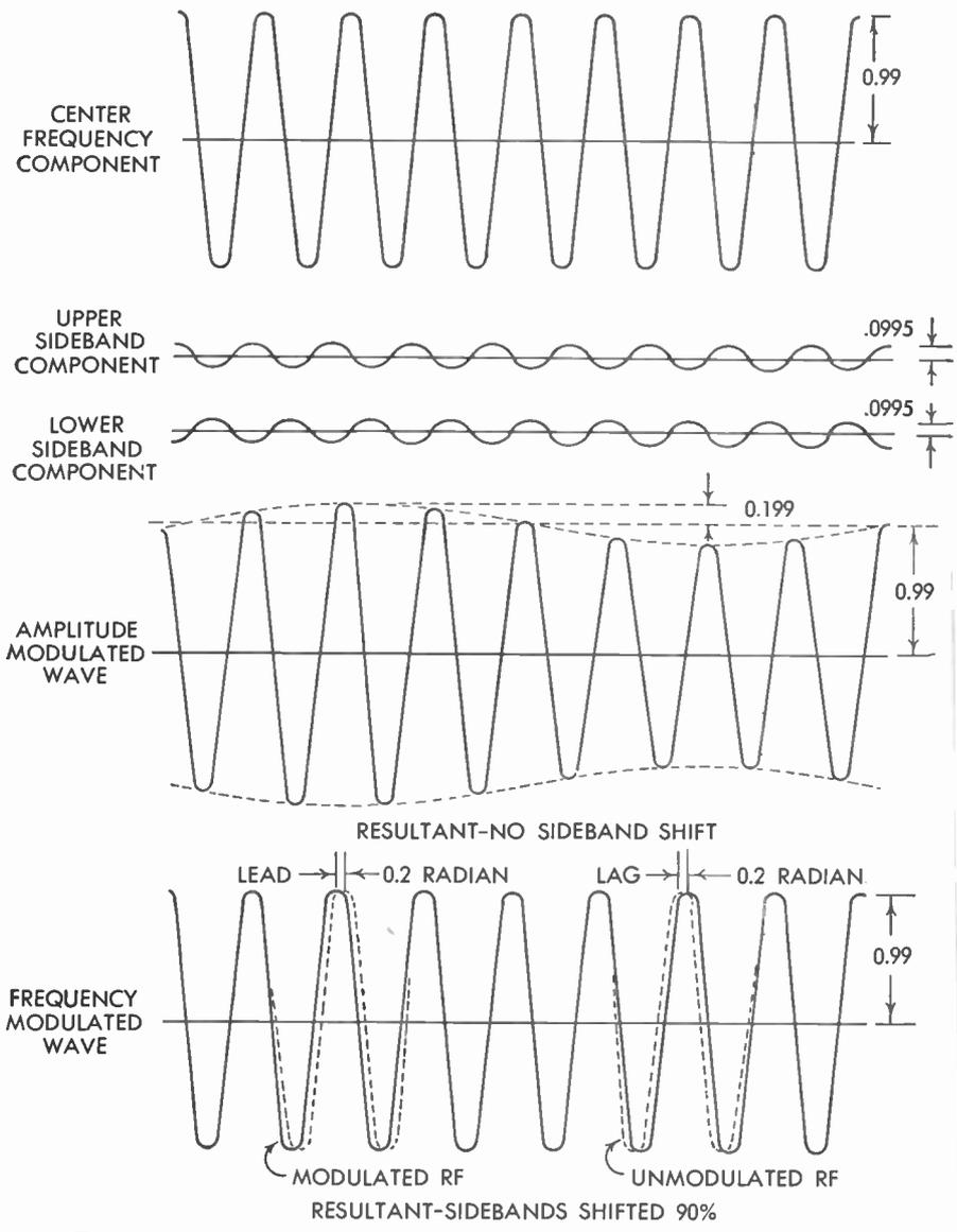
FIG. 192 Comparison of AM Wave and PM Frequency-Modulated Wave
