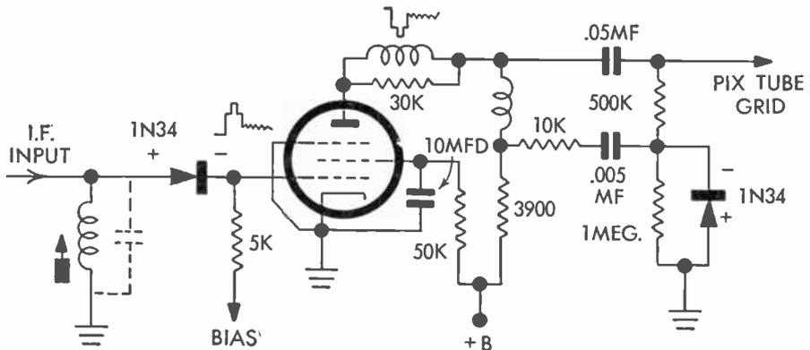
FIG. 94 Crystal Diodes in Video Section
