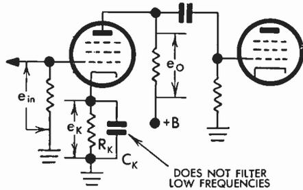
FIG. 76 Loss of Low Frequencies by Cathode Degeneration
