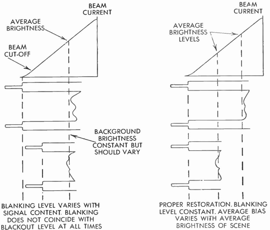
FIG. 91 Signal Distribution on Grid of Picture Tube with and without Proper Restoration
