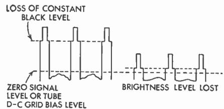
FIG. 33 Loss of Level When Coupling with a Capacitor
