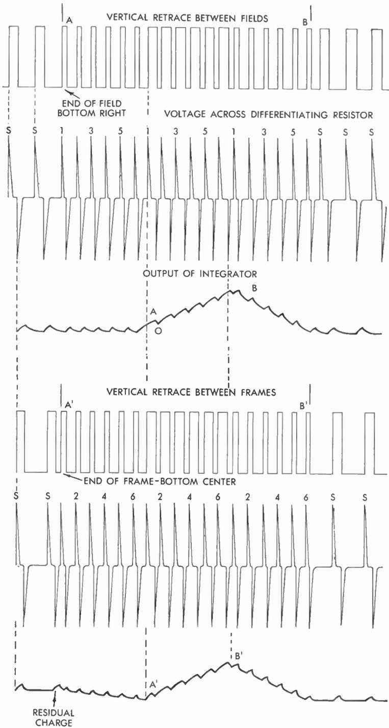
FIG. 144 Horizontal and Vertical Synchronization between Fields and Frames
