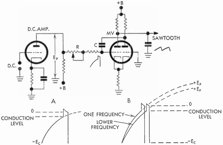
FIG. 165 D-C Control of Multivibrator Frequency
