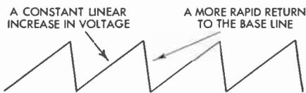
FIG. 12 Sawtooth Waves
