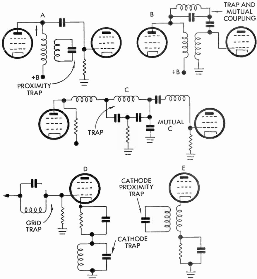
FIG. 45 Insertion of Wavetraps
