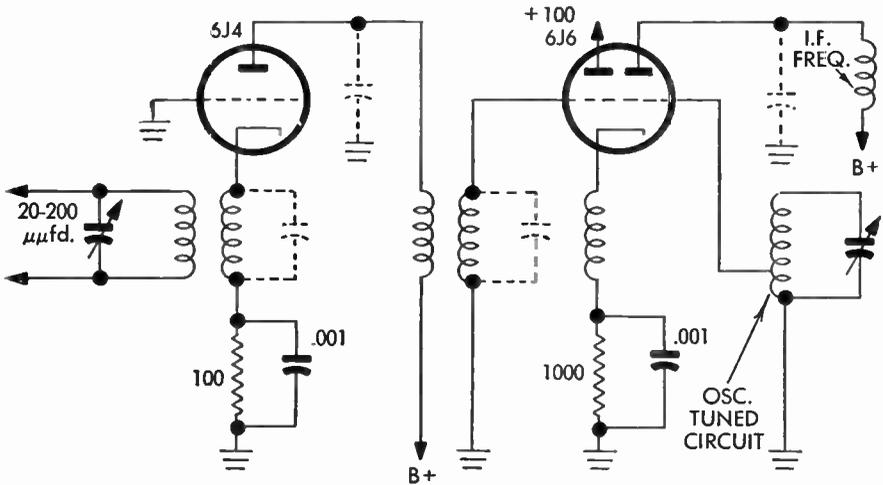
FIG. 50 Cathode-Coupled Mixer and Oscillator
