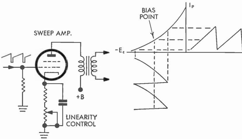
FIG. 180 Linearity Control by Biasing on Nonlinear Portion of Curve
