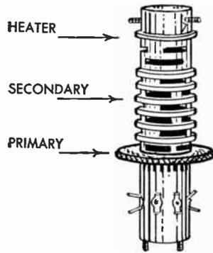
FIG. 127 R-F Transformer Assembly
