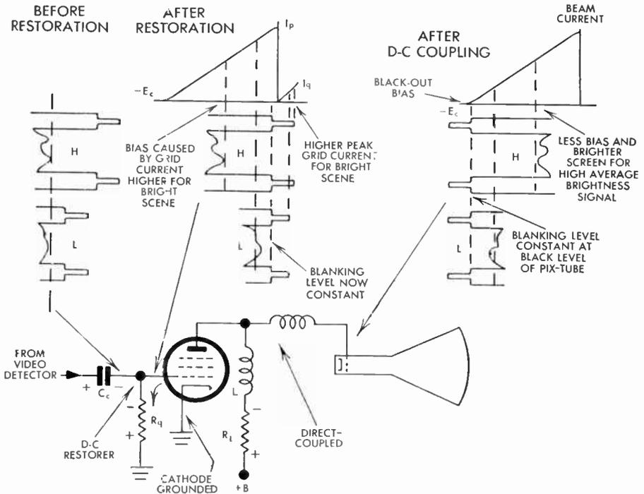
FIG. 92 Grid-Rectifier D-C Restorer and Waveforms
