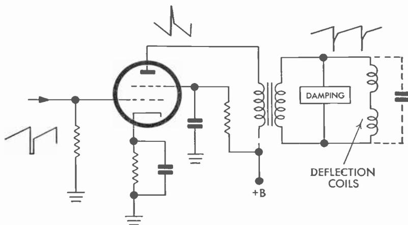
FIG. 172 Sweep Amplifier for Magnetic Deflection
