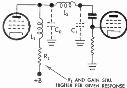
FIG. 79 Series-Shunt Peaking
