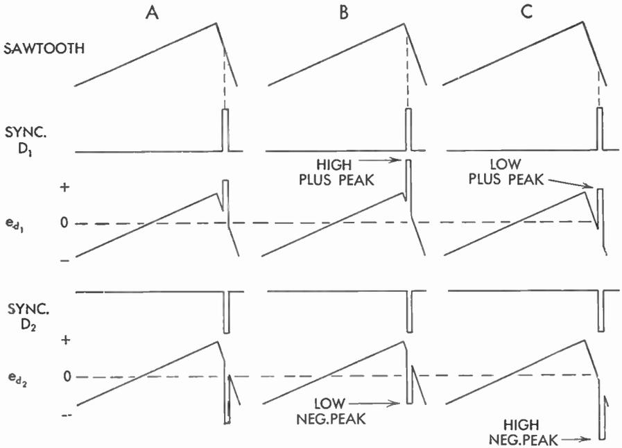
FIG. 150 Sync Control Waveforms
