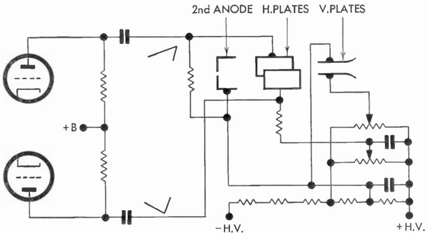
Fig. 115 Balanced Deflection Circuit
