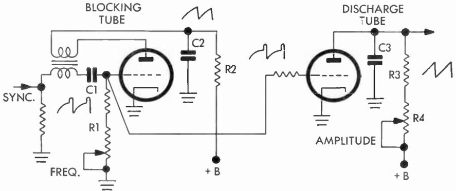
FIG. 160 Blocking-Tube Oscillator and Discharge Tube
