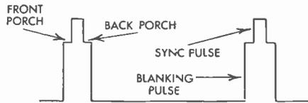
FIG. 11 Short-Duration Pulse on a Pedestal
