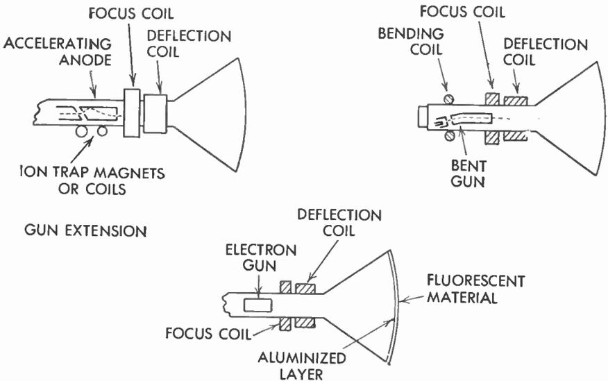
FIG. 119 Ion Spot Removal
