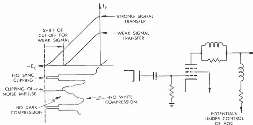
Fig. 98d Signal Level and Noise Clipping
