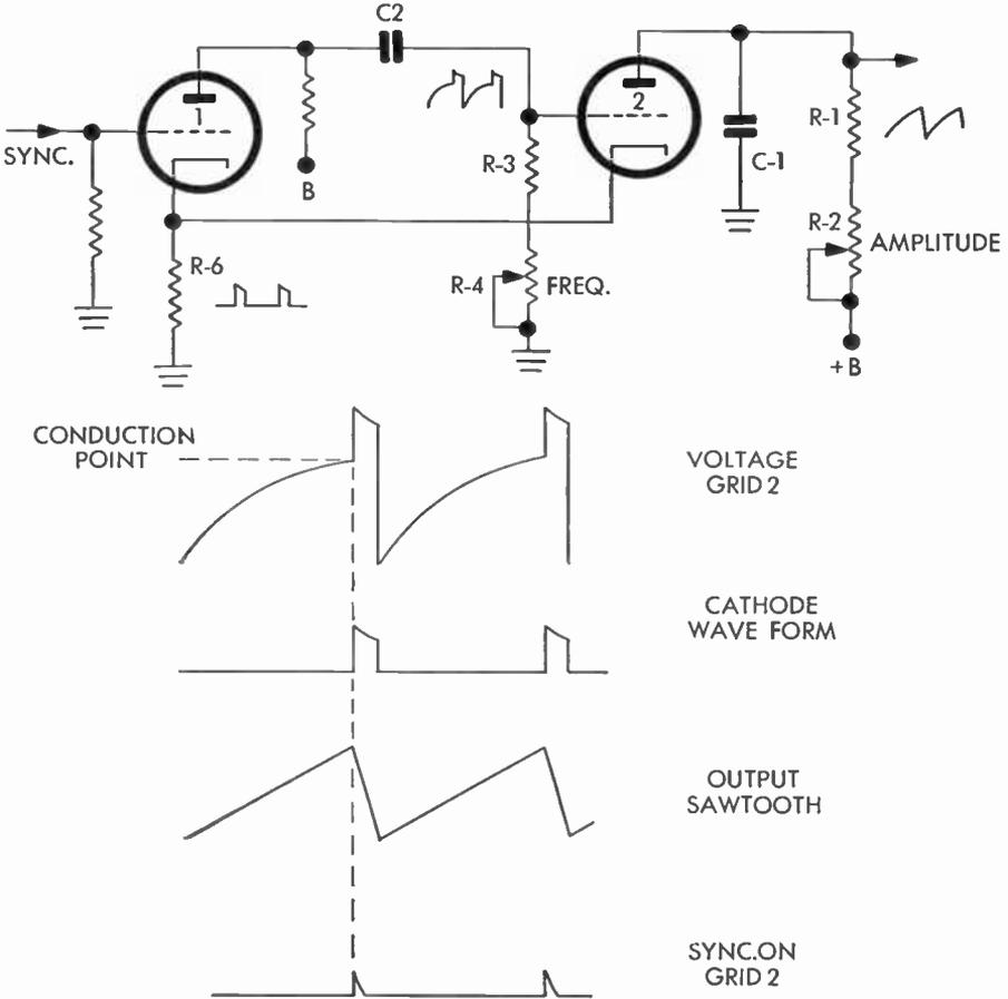
FIG. 162 Multivibrator Sawtooth Generator
