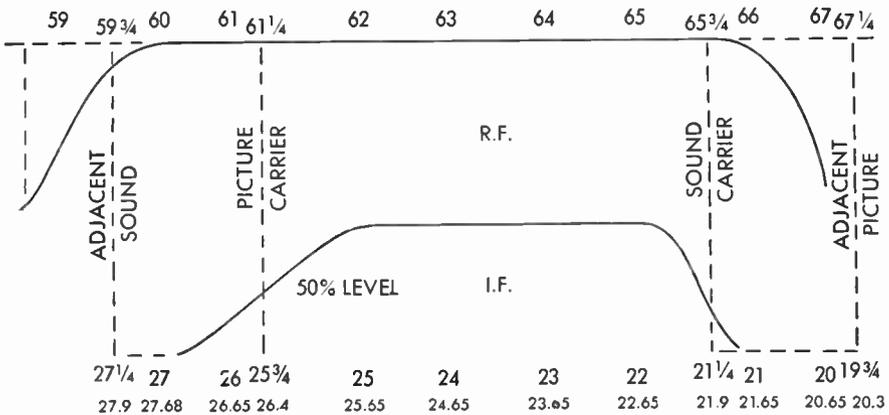
FIG. 67 Ideal R-F and I-F Bandpass. Local Oscillator on 87 or 87.65 Megacycles
