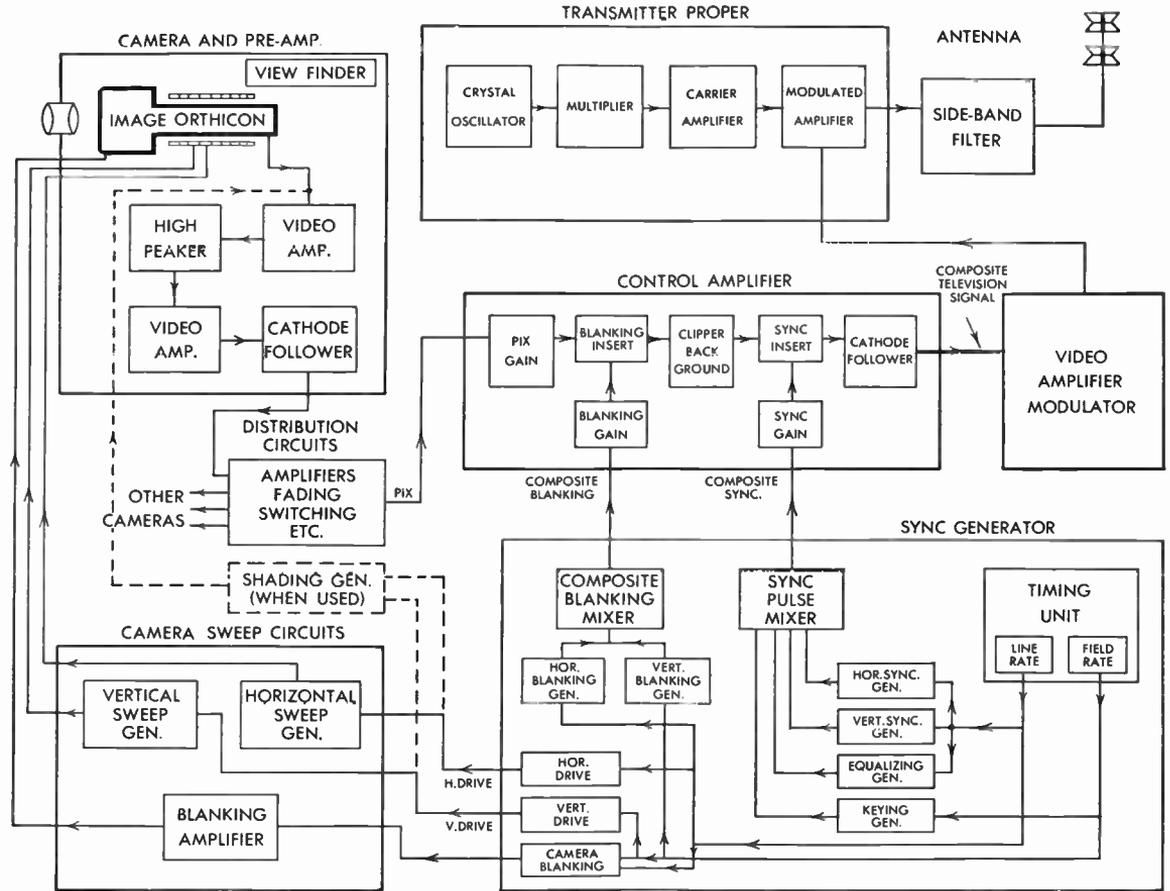
Fig. 29 Functional Block Diagram of Television Transmitter
