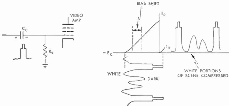
FIG. 98b Compression of Whites by Bias Shift on Bright Scene
