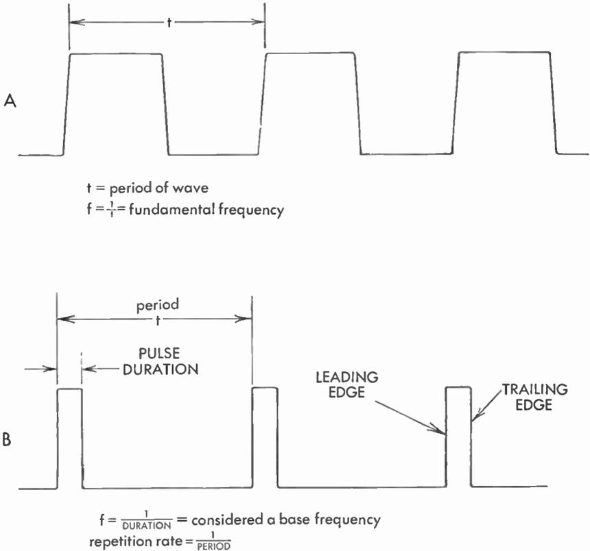
FIG. 9 Characteristics of Rectangular Pulses
