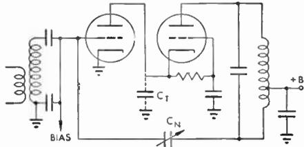
FIG. 51a. Basic Cathode Circuit
