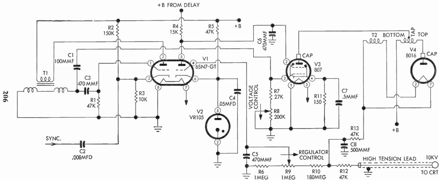
FIG. 129 DuMont Pulsed High-Voltage Supply
