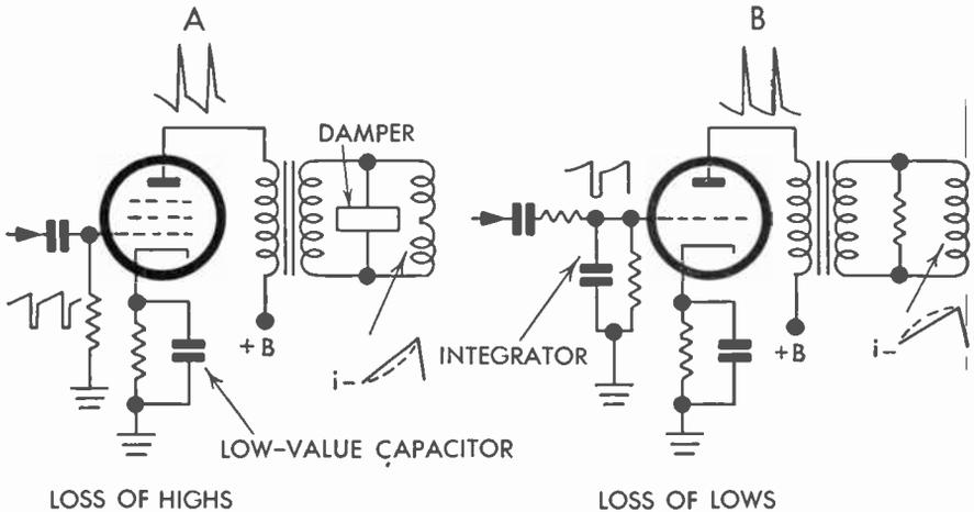
FIG. 179 Frequency Response Correction of Nonlinearity
