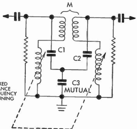
FIG. 59 Overcoupled Inductuner
