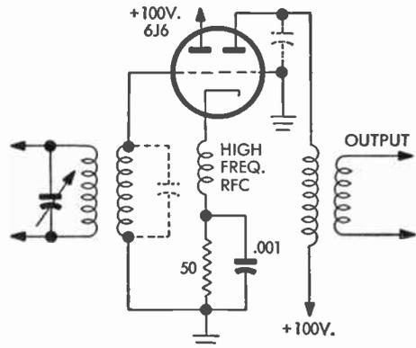
FIG. 49 Cathode-Coupled R-F Amplifier
