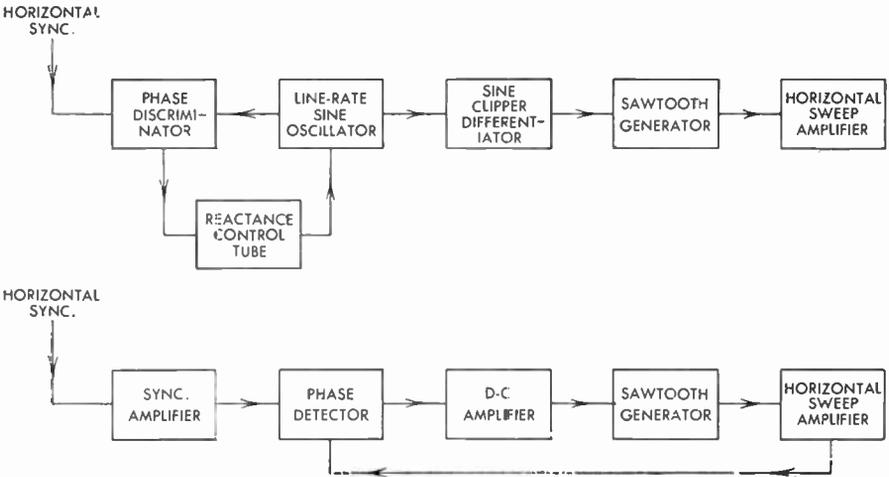
FIG. 146 Horizontal Sync Control Systems
