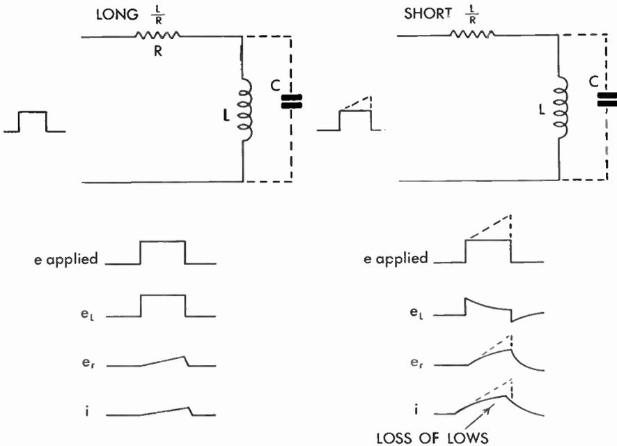
FIG. 176 Time Constant of  $R$ - $L$  Combination and Its Effect on Series Current
