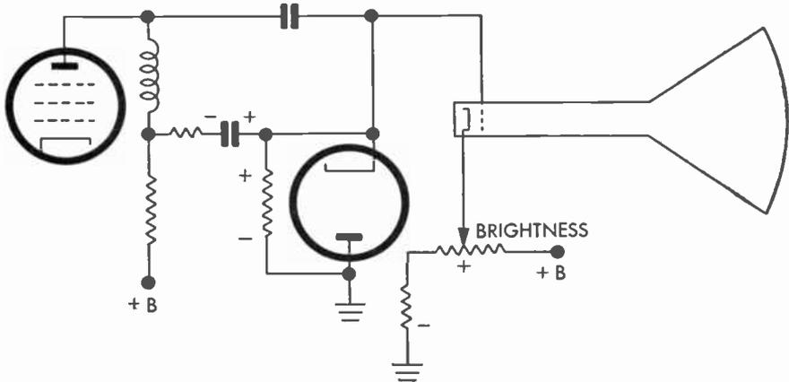
FIG. 96 Signal and Bias System with Diode-Restorer Circuit
