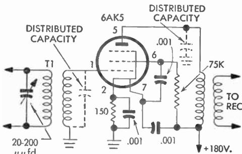
FIG. 47 Typical R-F Stage, T1 Overcoupled
