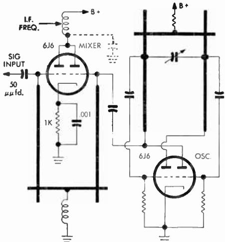
FIG. 51 Push-Pull Mixer-Oscillator
