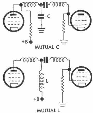
FIG. 42 Bandpass T Broad-Band Coupling
