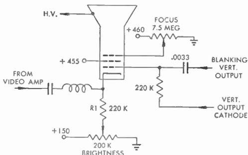
FIG. 131 Zenith Picture-Tube Circuit
