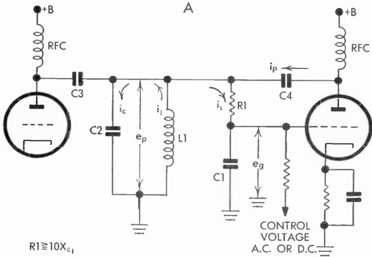
FIG. 203 Basic Reactance-Tube Circuit
