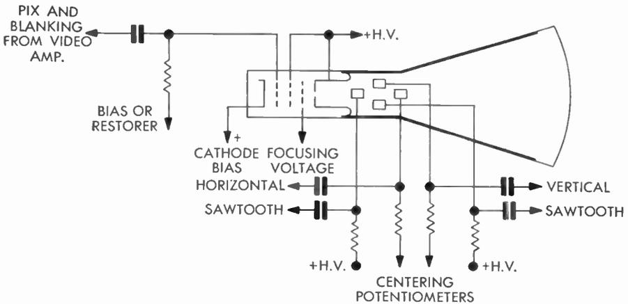
FIG. 122 Picture-Tube Circuit, Electric Deflection and Focusing
