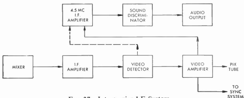
FIG. 37a Intercarrier I-F System
