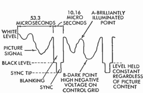
FIG. 21 Signal on Control Grid of Picture Tube
