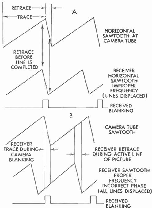
FIG. 166 Frequency and Phase of Receiver Sawtooth in Relation to Blanking
