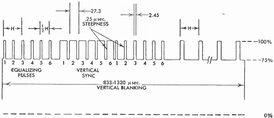
FIG. 25 Vertical Retrace Interval
