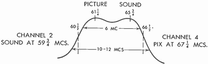
FIG. 63 Channel 3 Response of a Tuner
