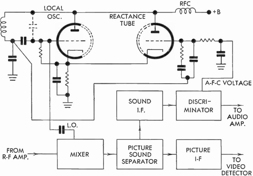
FIG. 66 Philco A-F-C Control of Local Oscillator
