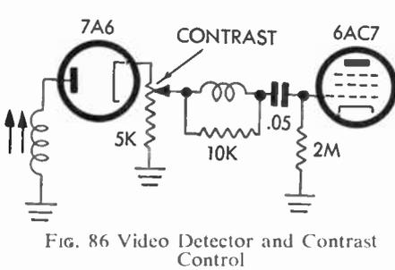
Fig. 86 Video Detector and Contrast Control
