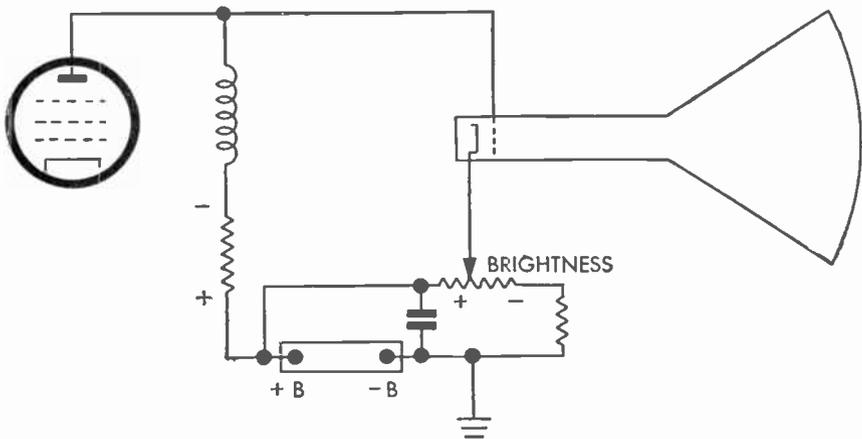
FIG. 95 Signal and Bias System of Picture Tube with D-C Coupling
