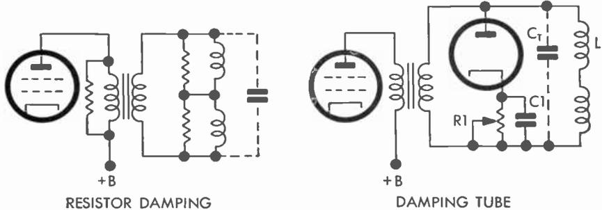
FIG. 177 Transient Voltage Damping Systems
