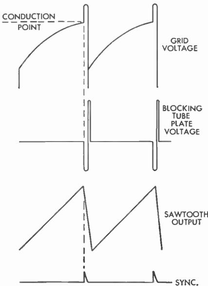
FIG. 161 Blocking-Tube Waveforms
