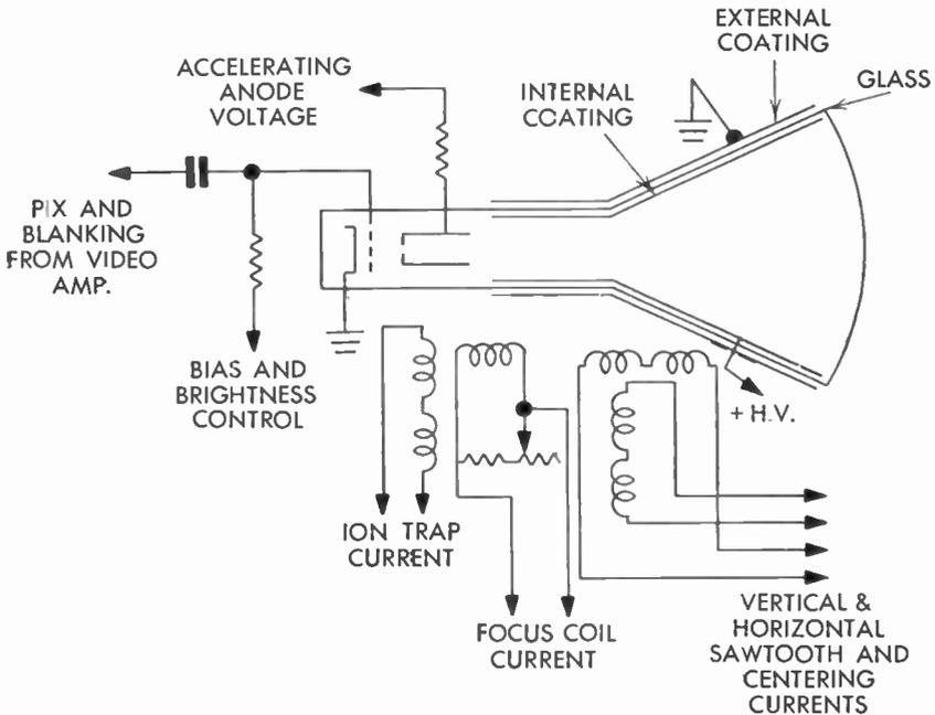
FIG. 121 Picture-Tube Circuit, Magnetic Deflection and Focusing
