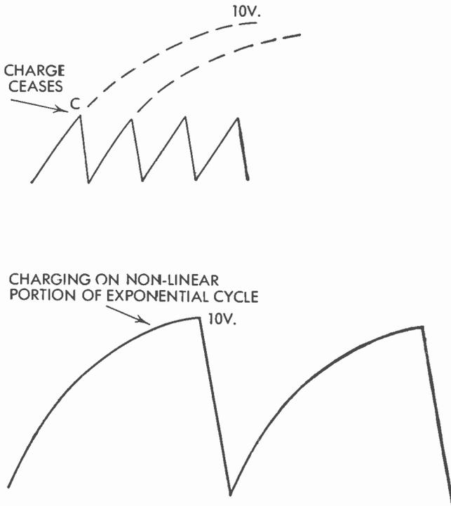
FIG. 158 Generation of a Sawtooth
