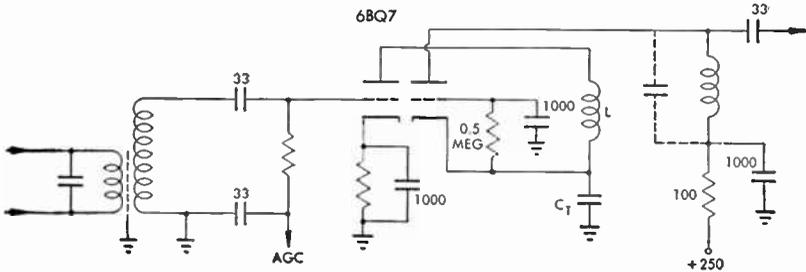
FIG. 51b Cascode Amplifier with No Neutralization
