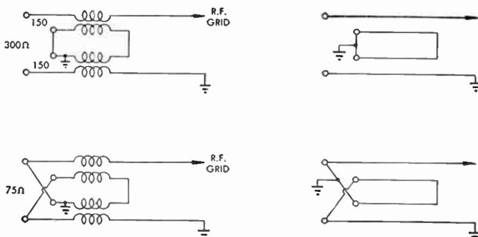
FIG. 64d Elevator Transformer Action
