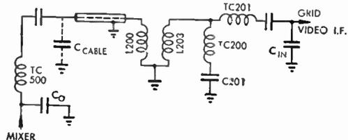
Fig. 73d Philco Tuner to I-F Coupling
