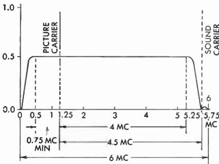
FIG. 5 Signal Distribution. Standard Television Channel
