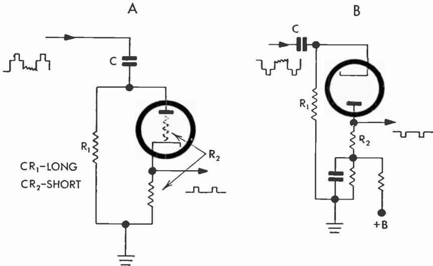
FIG. 140 Diode Separators—Positive and Negative
