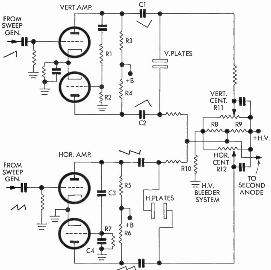
FIG. 171 Horizontal and Vertical Sweep Amplifiers
