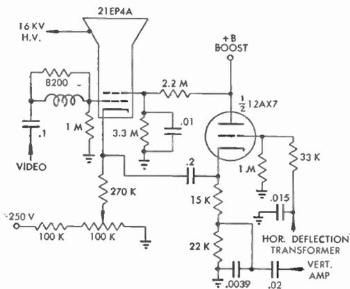
FIG. 132 GE Picture-Tube Circuit
