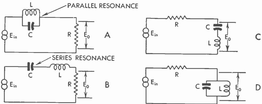
FIG. 68 Fundamentals of Resonant Circuits
