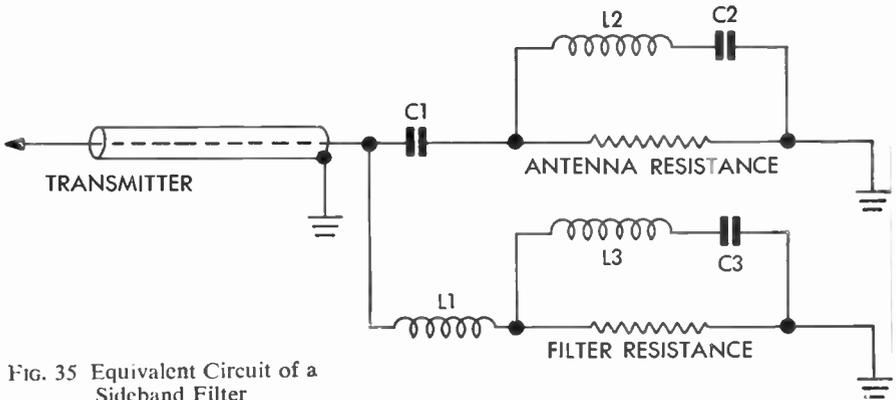
FIG. 35 Equivalent Circuit of a Sideband Filter
