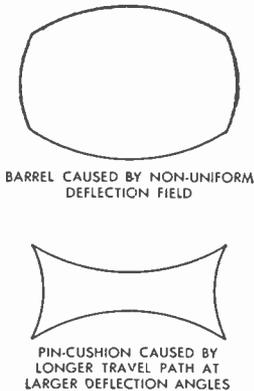
FIG. 186 Distortion of Deflection Field and Raster
