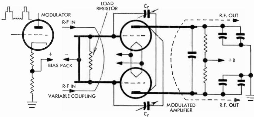
Fig. 34 Direct-Coupled Grid Modulation
