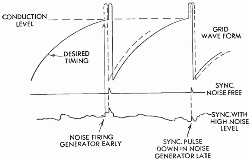
Fig. 164 Effects of Noise on Synchronization Time
