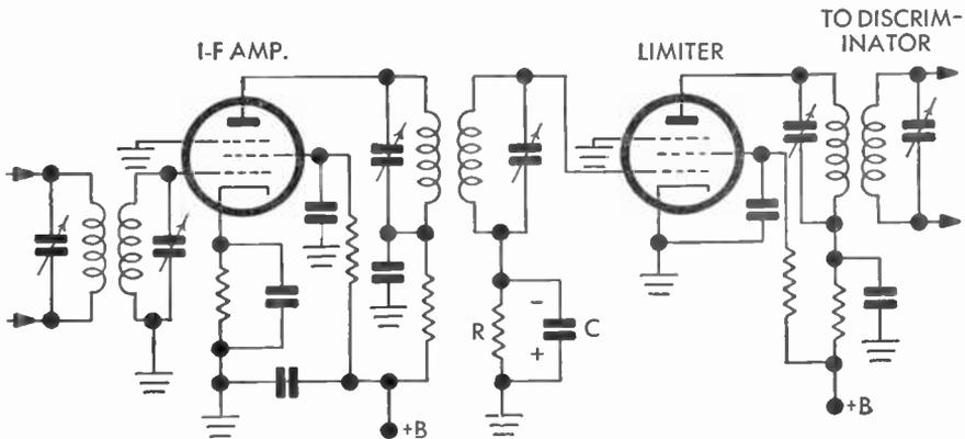
FIG. 196 Sound I-F Amplifier and Limiter
