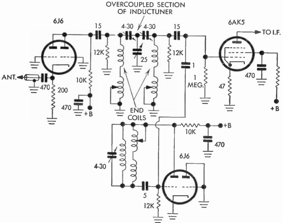
FIG. 57 DuMont Inductuner Circuit
