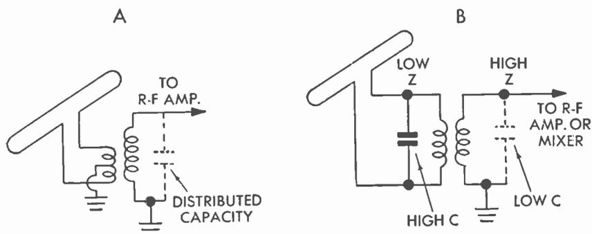
FIG. 60 Antenna Matching Methods
