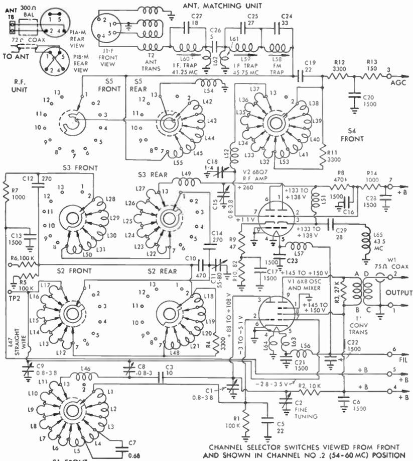
Fig. 64c RCA Cascode Tuner
