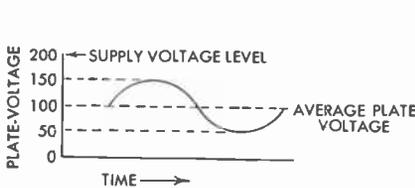
FIG. 14 A-C and D-C Plate Current Components
