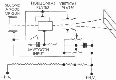
Fig. 114 Horizontal Deflection by Sawtooth Voltage
