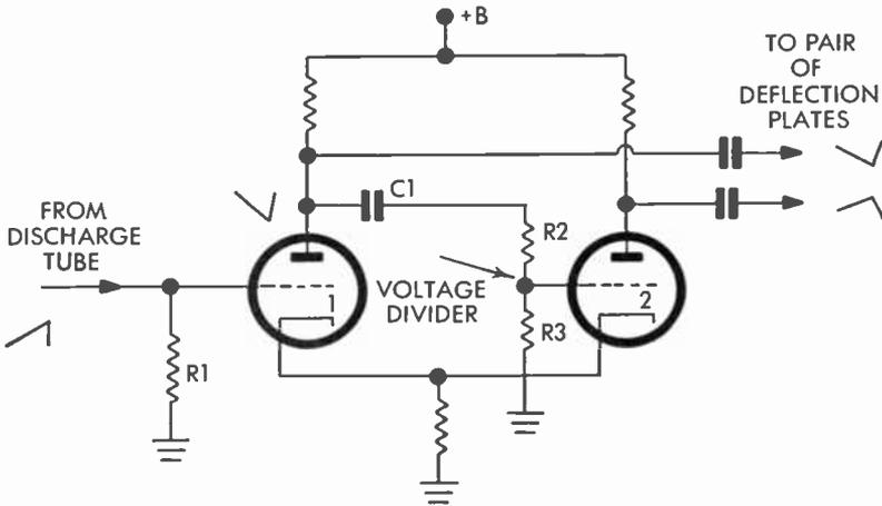
FIG. 168 Electrostatic Sweep Amplifier
