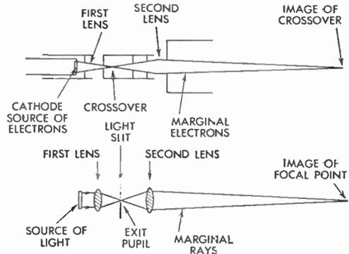
FIG. 107 Comparison of Electronic and Optical Lens Systems
