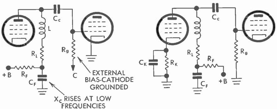
FIG. 80 Low-Frequency Compensation
