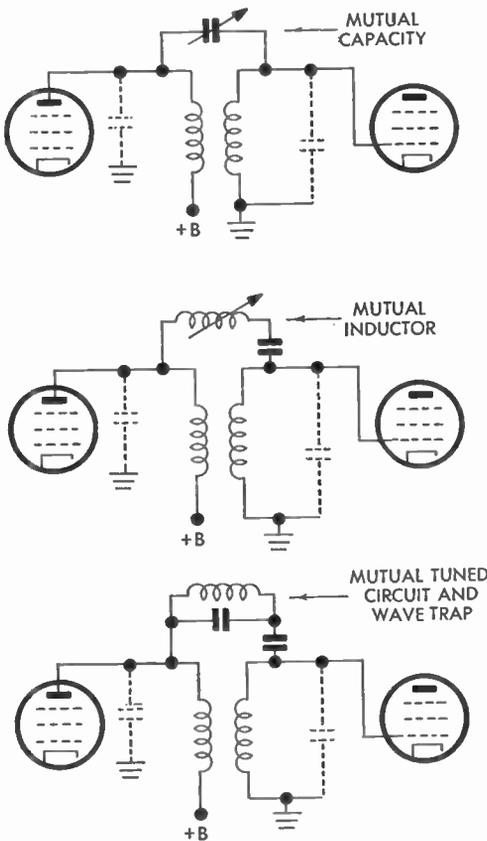
FIG. 41 Overcoupling Methods
