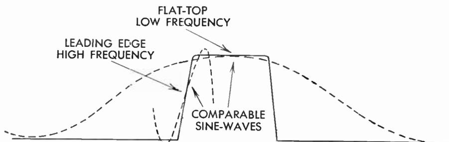
FIG. 134 High- and Low-Frequency Characteristics of a Pulse
