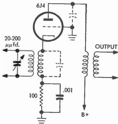
FIG. 48 Grounded-Grid R-F Amplifier
