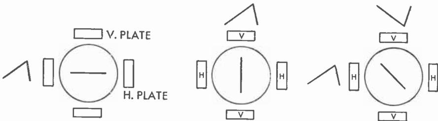
FIG. 16 Scanning Process
