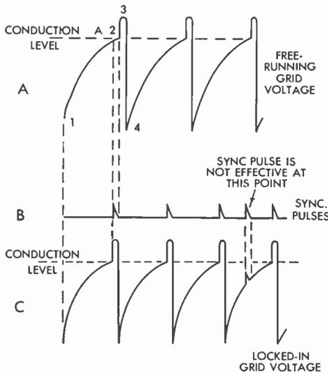
FIG. 163 Synchronization of a Blocking Tube
