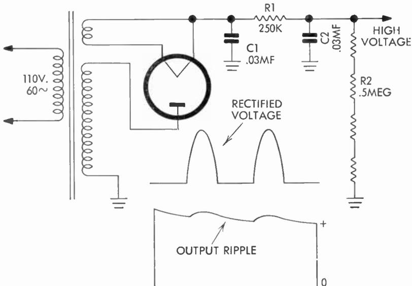
FIG. 124 Transformer High-Voltage Supply
