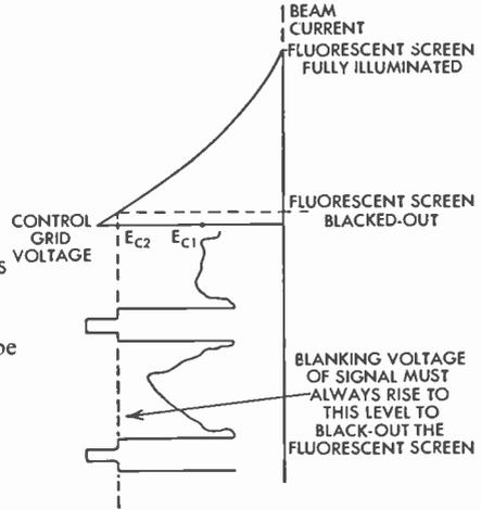
FIG. 22 Positioning of Signal on Picture-Tube Characteristic
