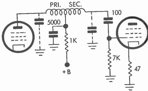
Fig. 72a Single-Winding I-F Transformer
