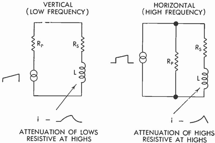
FIG. 178 Distortion of Horizontal and Vertical Sweep Currents
