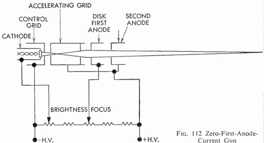
FIG. 112 Zero-First-Anode-Current Gun
