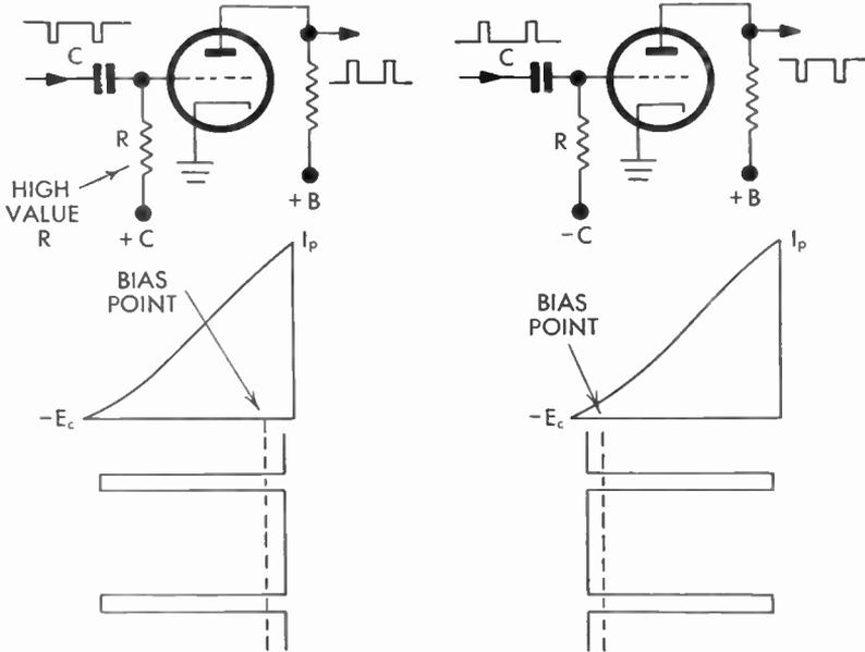
FIG. 153 Biasing a Pulse Stage
