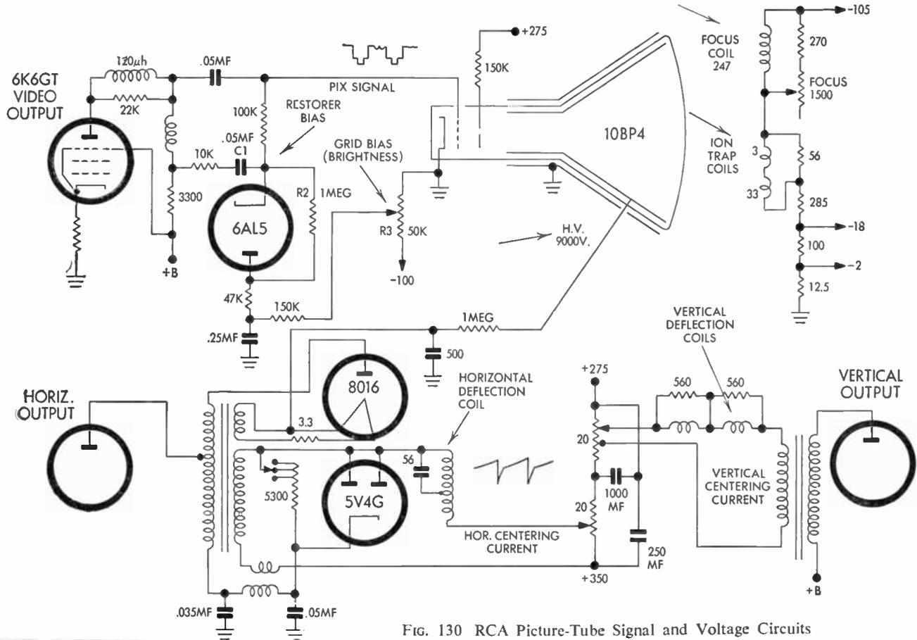
FIG. 130 RCA Picture-Tube Signal and Voltage Circuits
