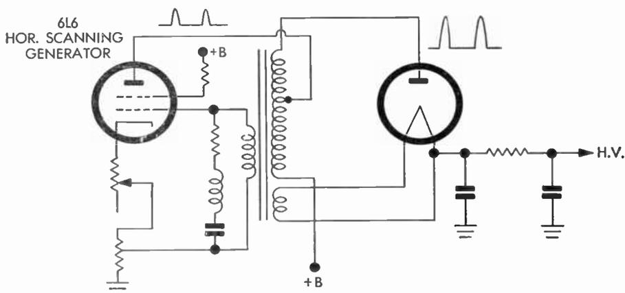
FIG. 128 Beam-Relaxor High-Voltage Supply
