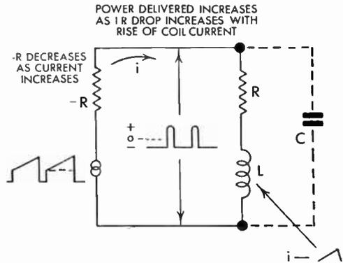
FIG. 175 Equivalent Circuit of Deflection System
