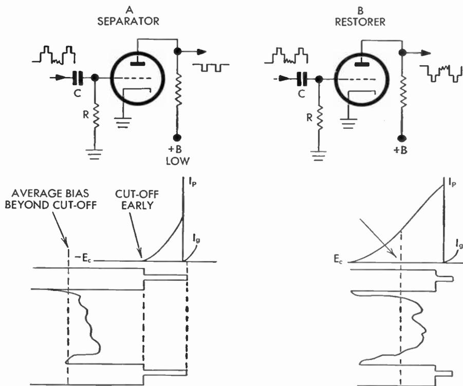
FIG. 141 Triode Sync Separator and Grid-Type Restorer
