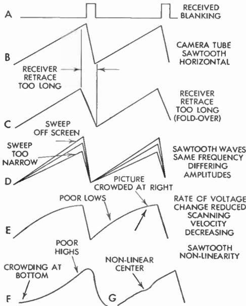
FIG. 167 Sweep Waveform Defects
