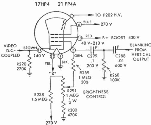
FIG. 133 DuMont Self-Focus Circuit
