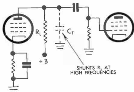
FIG. 74 Loss of Highs through Shunt Capacity
