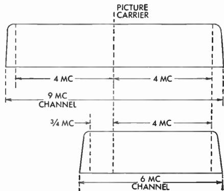
FIG. 6 Reduction of Channel Width by Partial Suppression of One Sideband
