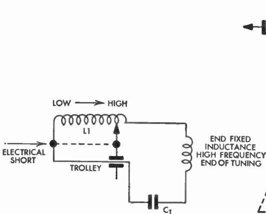
FIG. 58 Basic Inductuner Circuit
