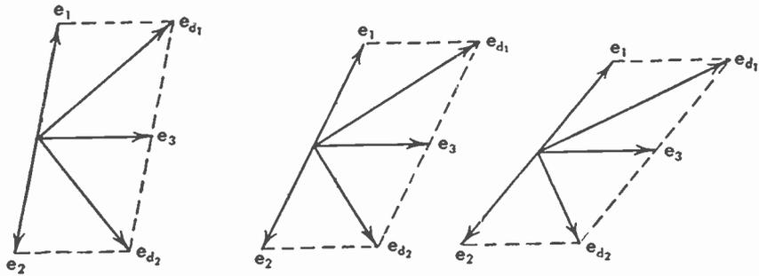
FIG. 199 Increase in Output as Frequency Departs from Center Frequency,  $e_{d1}$ - $e_{d2}$
