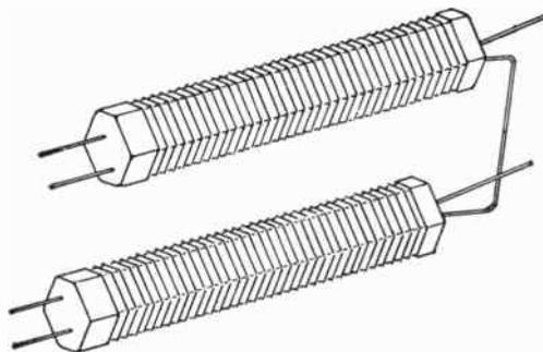
FIG. 64c Coil Plan of RCA Elevator Transformer
