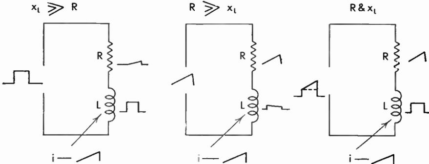
FIG. 173 Modification of Waveform to Obtain Sawtooth Current in Coil
