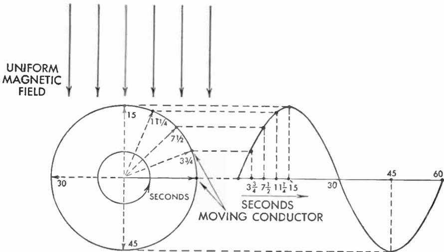
FIG. 8 Generation of a Sine Wave
