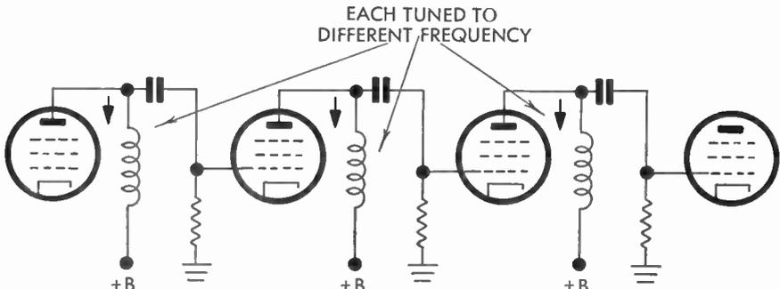
FIG. 44 Stagger-Tuned, Single-Tuned Transformer
