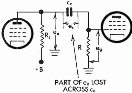
FIG. 75 Loss of Lows across Coupling Capacitor
