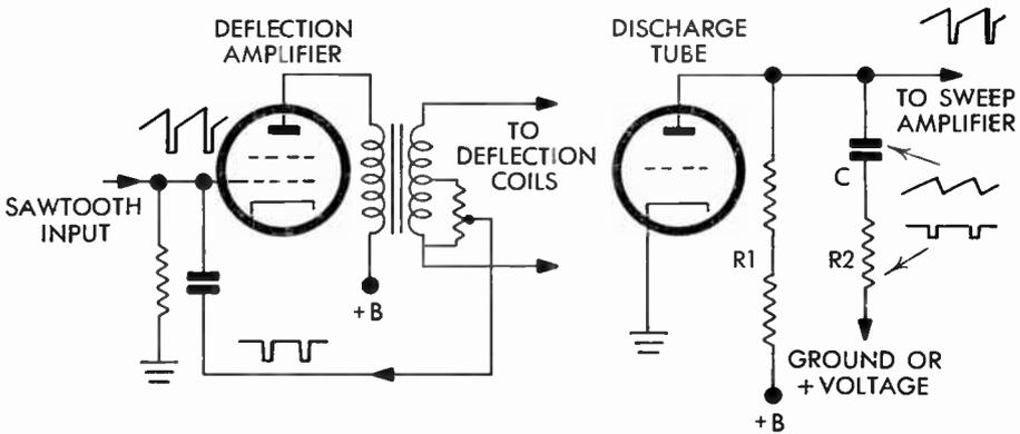
FIG. 174 Modification of Sweep Sawtooth for Magnetic Deflection
