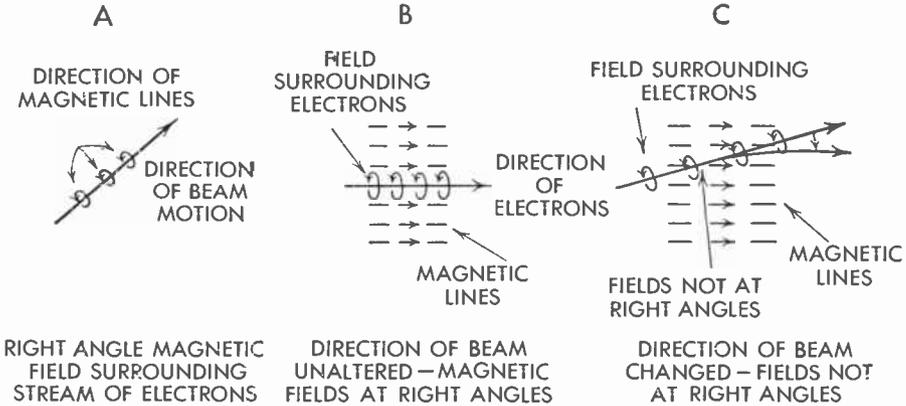
FIG. 110 Magnetic Fields and Beam Motion
