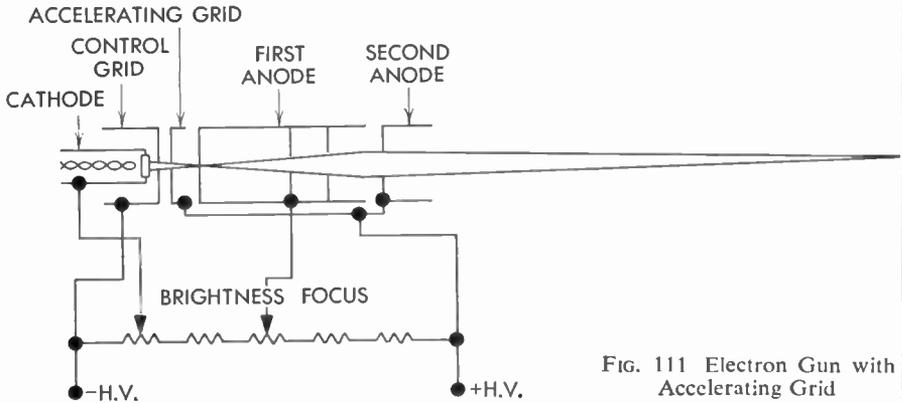
FIG. 111 Electron Gun with Accelerating Grid
