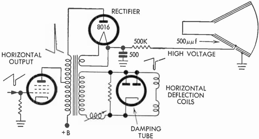
FIG. 123 Flyback High-Voltage Supply
