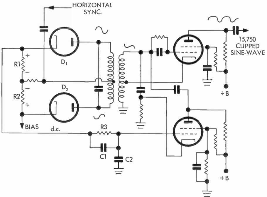
FIG. 147 RCA Sync-Lock System
