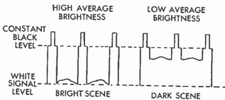
FIG. 32 Composite Signal with High and Low Average Brightness
