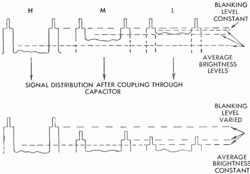
FIG. 90 Loss of Average Brightness and Blanking Levels through Capacitor Coupling
