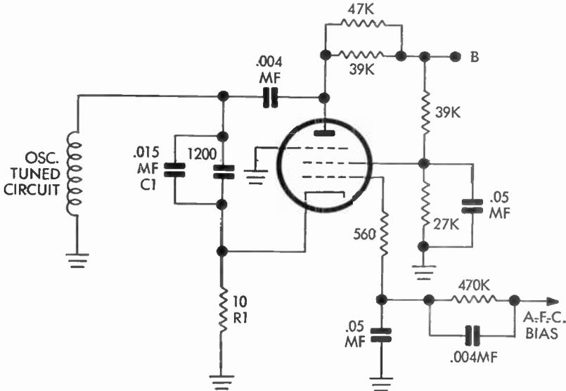
FIG. 207 Reactance Tube of RCA Sync Control
