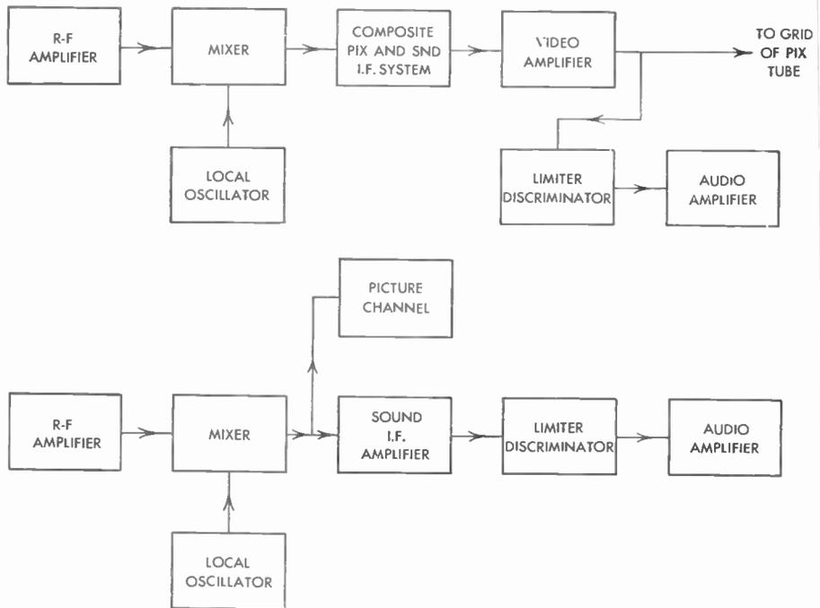
FIG. 193 Television Receiver FM Sections
