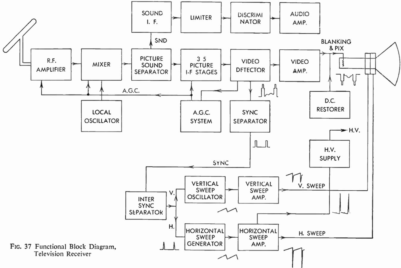
Fig. 37 Functional Block Diagram, Television Receiver
