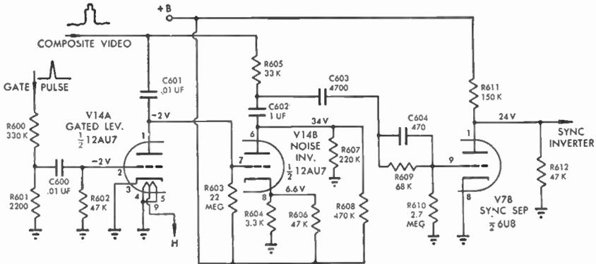
FIG. 156 Noise-Inverter and Sync Separator
