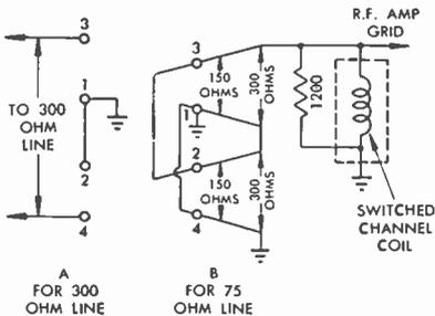
FIG. 64g Philco Tapered-Line Input
