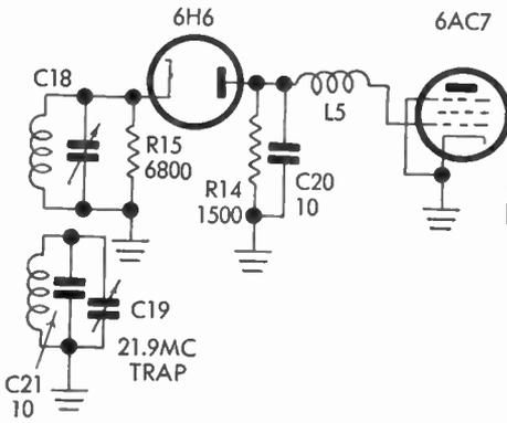
Fig. 84 GE Direct-Coupled Video Detector
