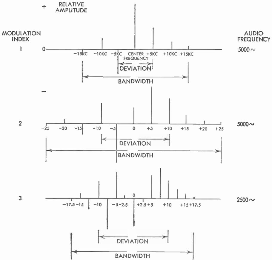
FIG. 190 Components of an FM Wave According to Modulation Index
