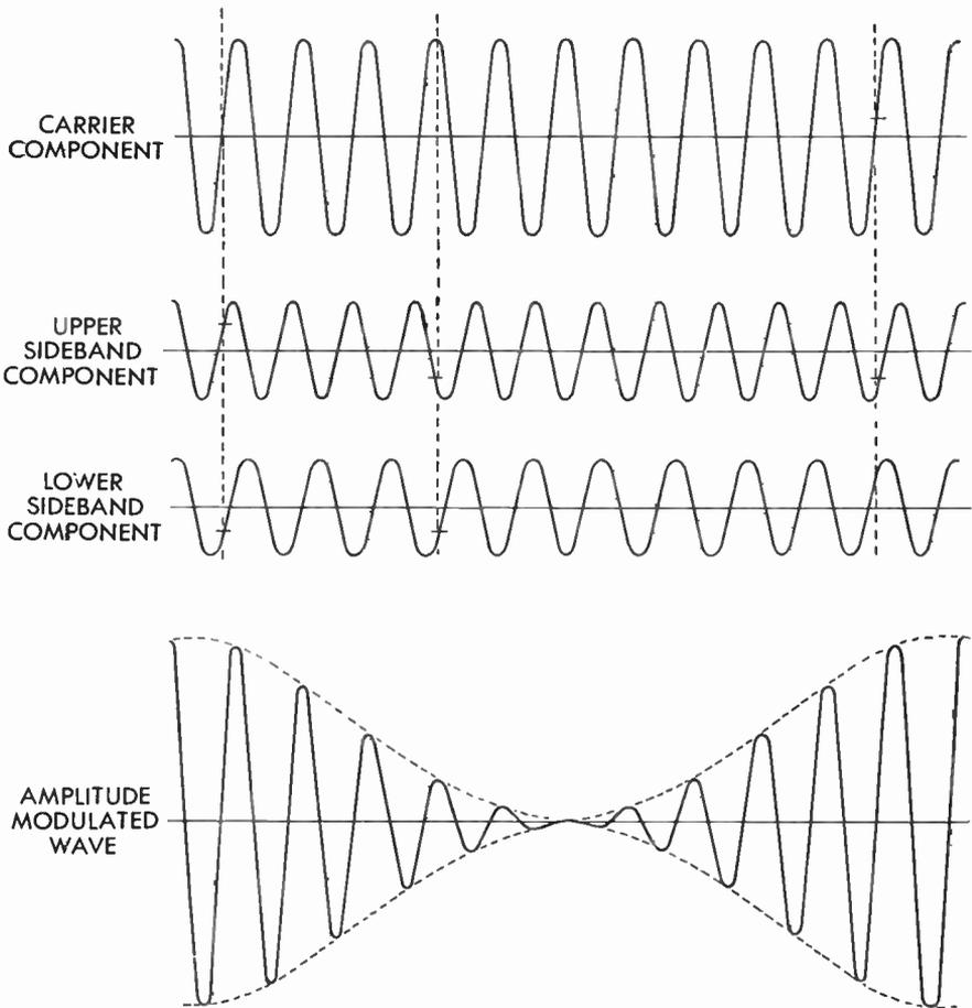
FIG. 189 Components of a 100% Amplitude-Modulated Wave
