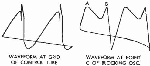
FIG. 150c Syncroguide Waveforms
