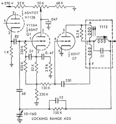
FIG. 150b RCA Synchroguide
