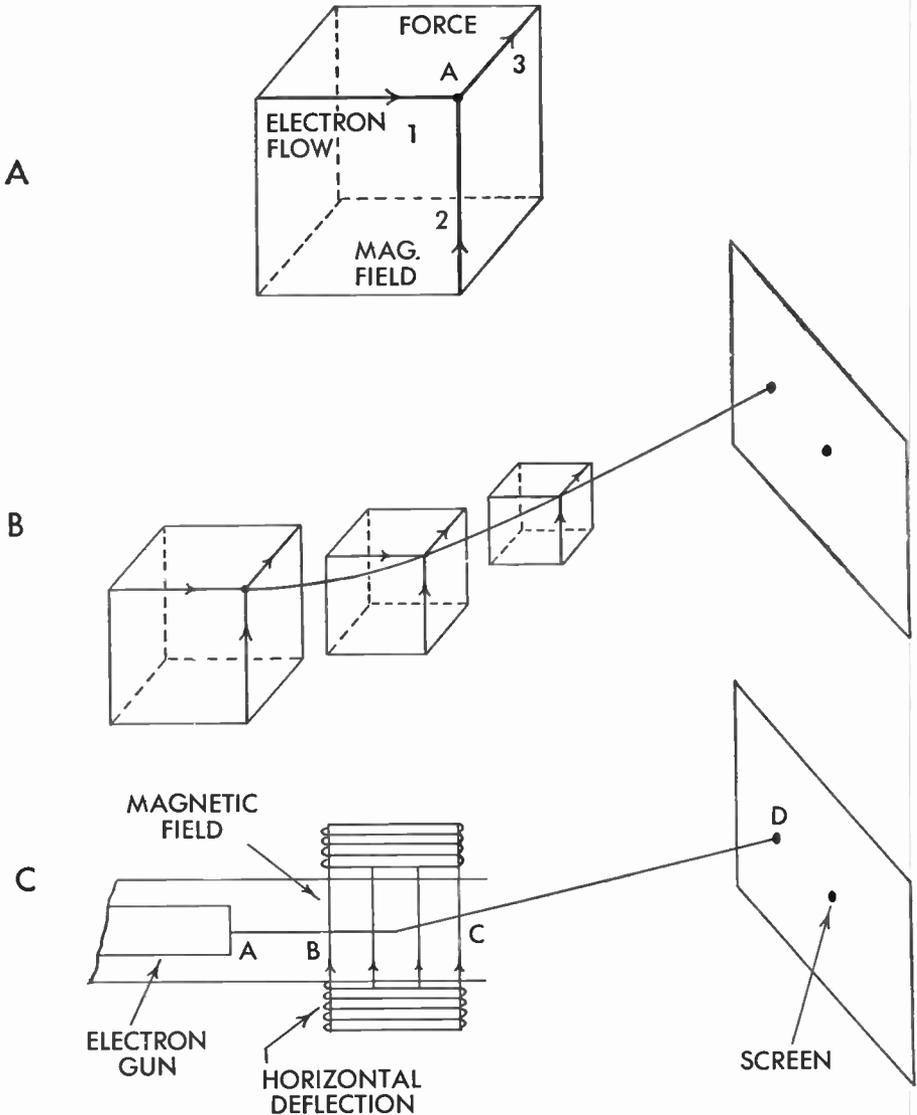
FIG. 117 Principles of Magnetic Deflection
