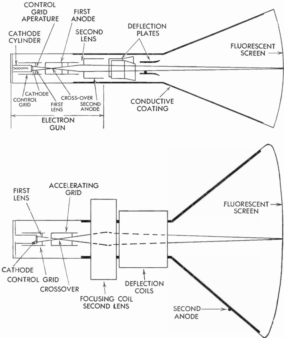
Fig. 106 Electric and Magnetic Focusing and Deflection for Picture Tubes
