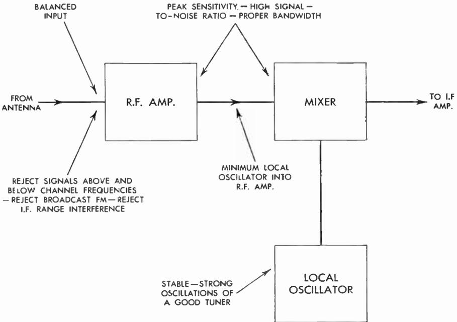
FIG. 62 Features of a Good Tuner
