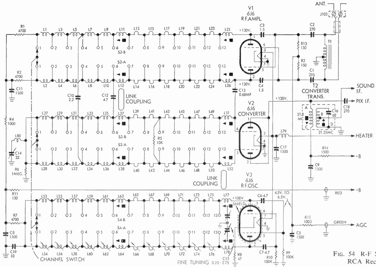
FIG. 54 R-F Section, RCA Receiver
