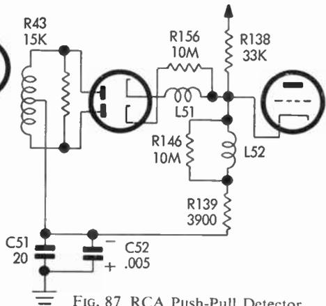
Fig. 87 RCA Push-Pull Detector
