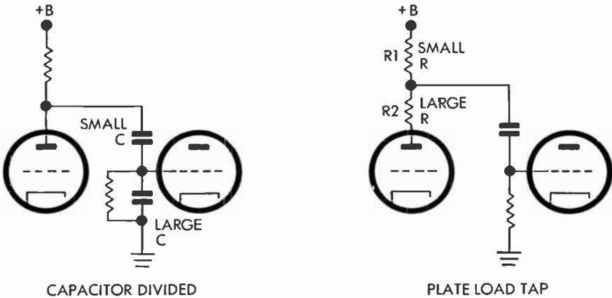
Fig. 169 Voltage Division Methods for Horizontal Sweep Amplifier
