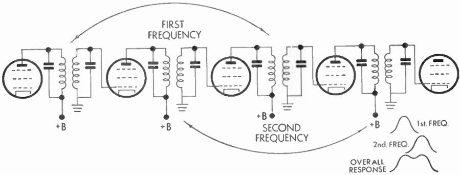
FIG. 43 Stagger-Tuned Wide-Band Amplifier
