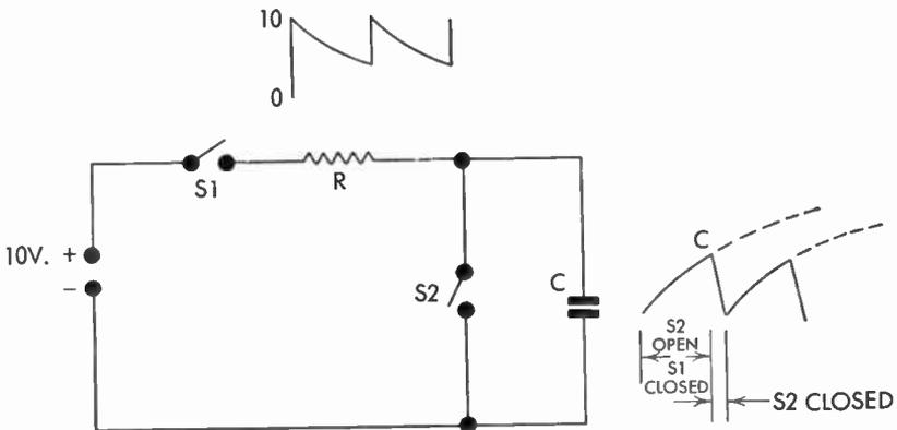
FIG. 157 Simple Sawtooth Generator
