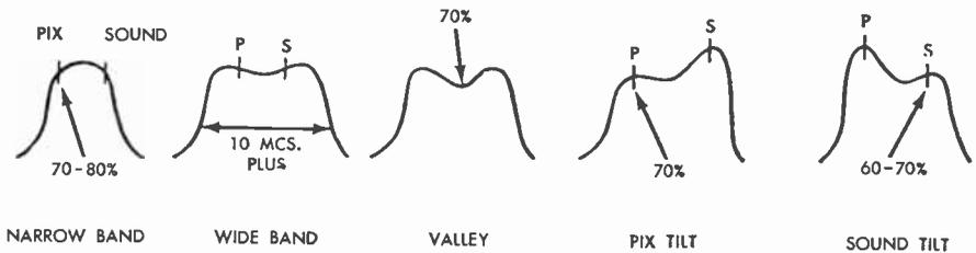
FIG. 64b Tuner Response Limits
