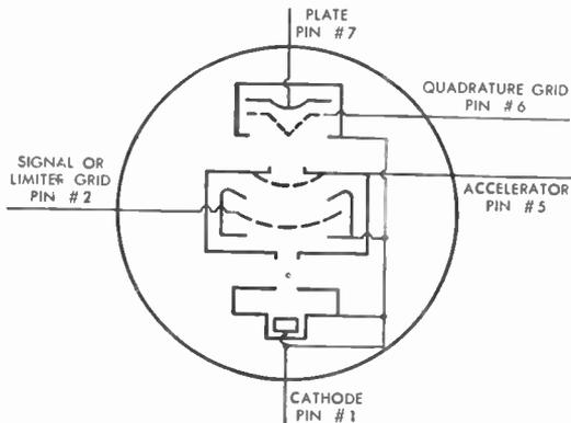
FIG. 209a Grated-Beam Tube
