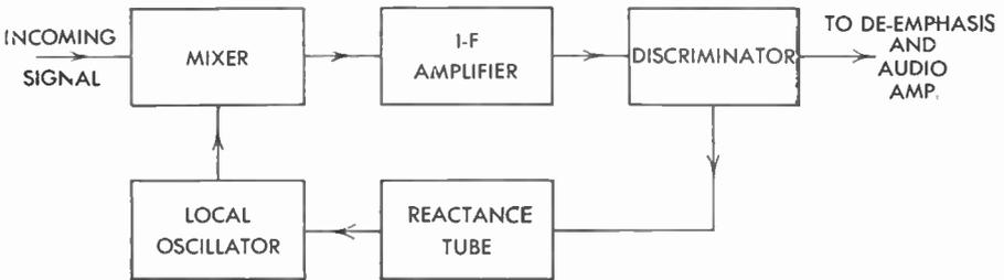
FIG. 202 Block Diagram, Automatic Frequency Control
