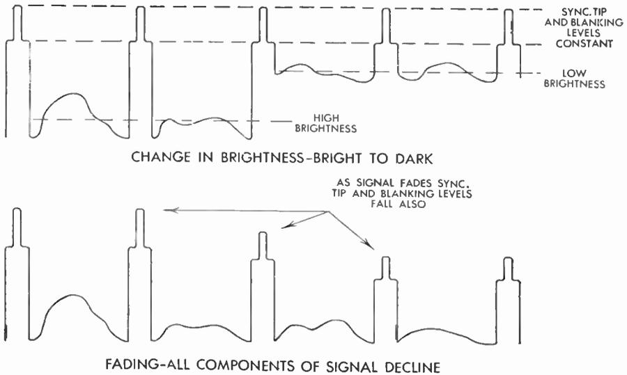
FIG. 100 Change in Signal Distribution with Changes in Average Brightness and Fading
