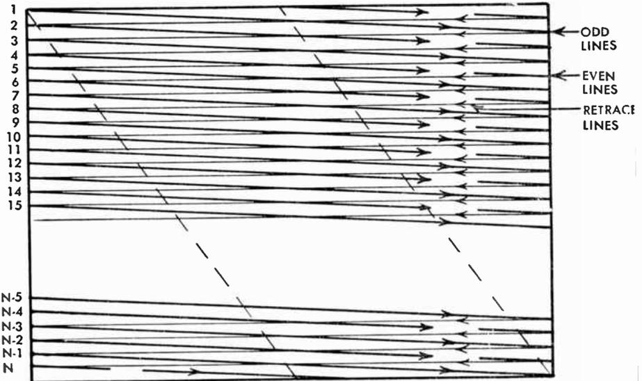
FIG. 19 Scanning Raster Showing Interlaced Pattern
