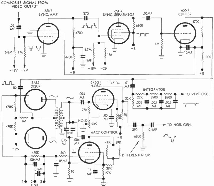
FIG. 151 RCA Sync and Inter-Sync System
