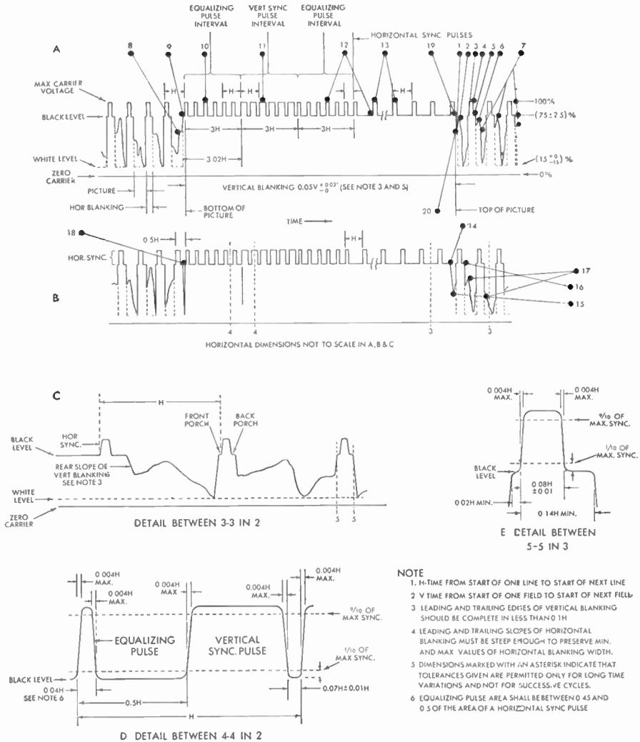
Fig. 23 Composite Television Signal
