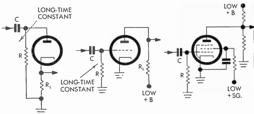
FIG. 139 Typical Sync Separators
