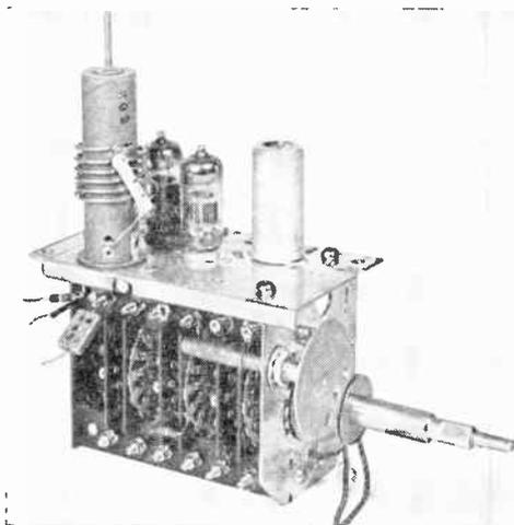
Fig. 52 RCA Selector Tuner
