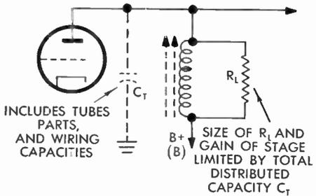
FIG. 46 Output Circuit of Wide-Band R-F or I-F Amplifier
