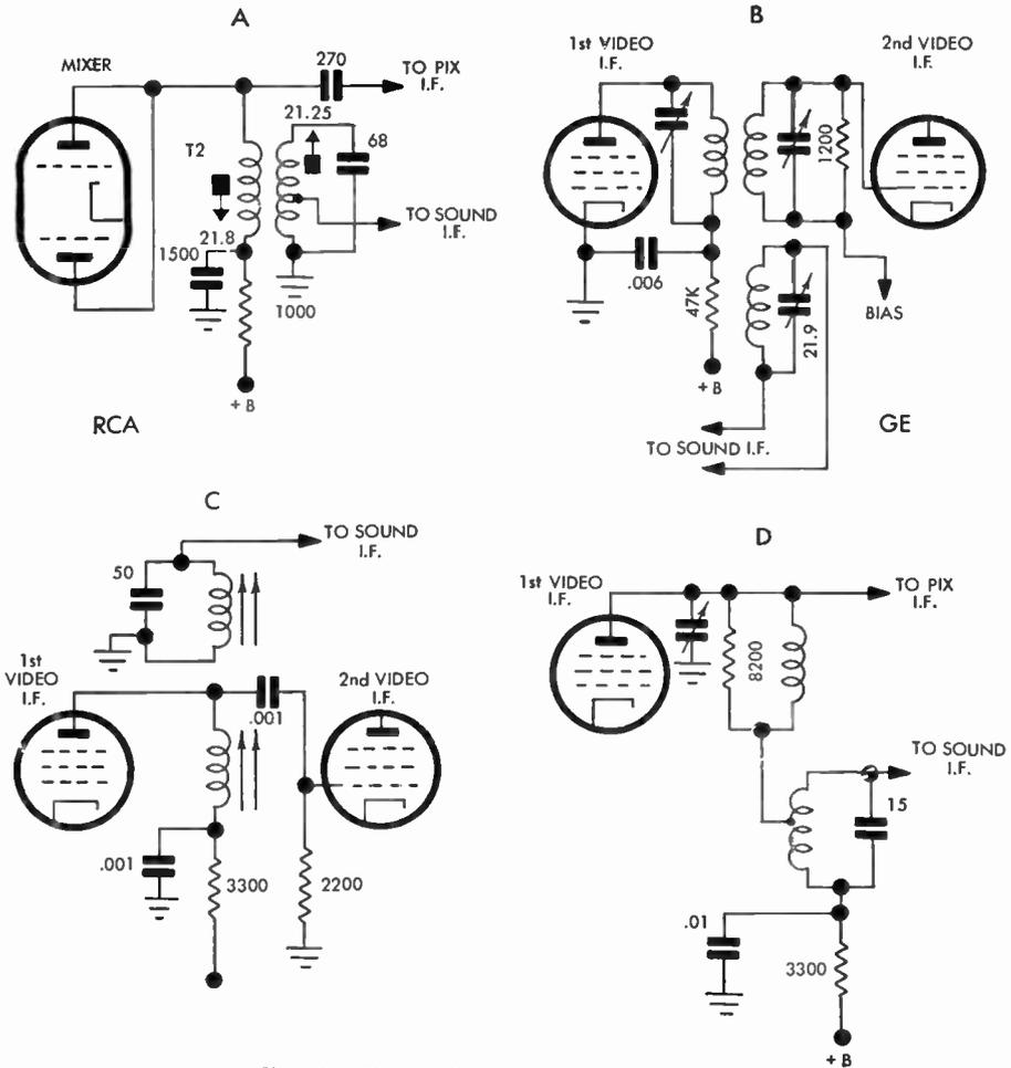
FIG. 69 Picture-Sound Separating Systems
