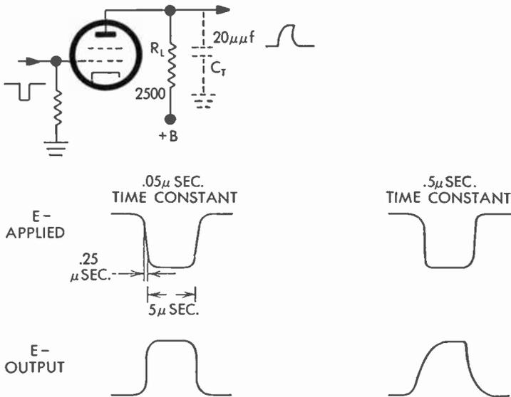
FIG. 137 Time Constant and Pulse Leading Edge
