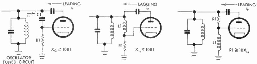
FIG. 205 Reactance-Tube Phase Shifters
