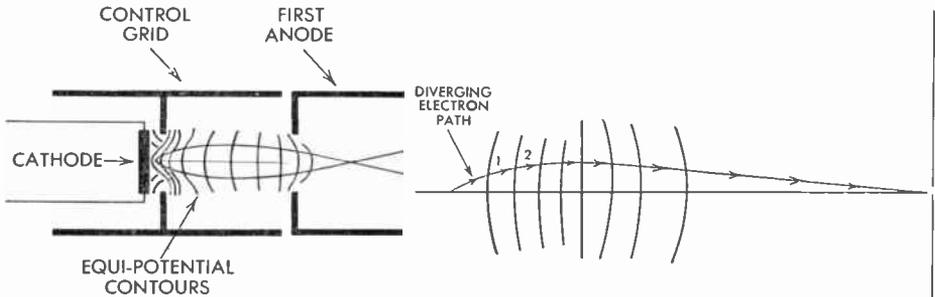
FIG. 108 Voltage Gradients of First Lens
