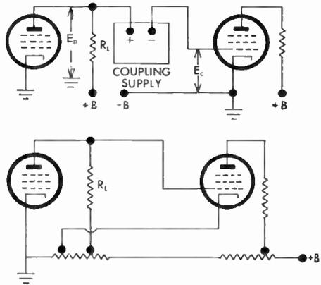
FIG. 93a Basic D-C Amplification
