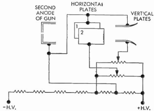
FIG. 113 Simple Deflection System as Used for Centering
