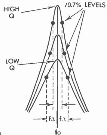
FIG. 39 Circuit  $Q$  and Bandwidth
