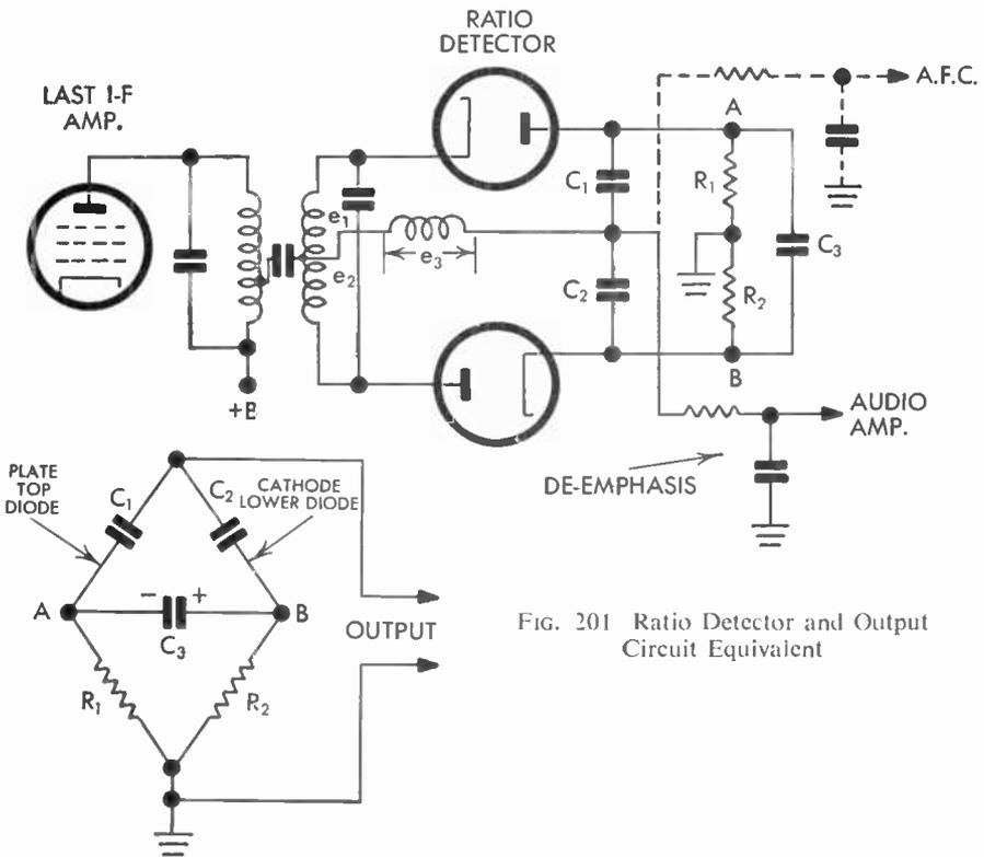
FIG. 201 Ratio Detector and Output Circuit Equivalent
