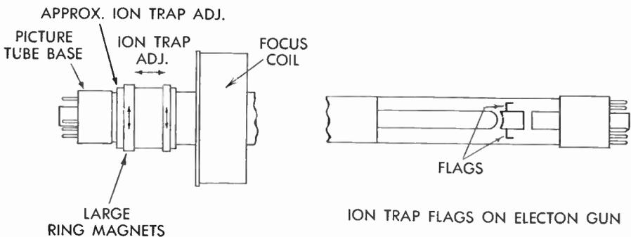
SIDE VIEW SHOWING ION TRAP ADJUSTMENT
