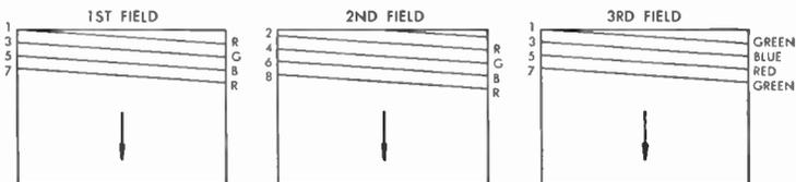
FIG. 8 Line Sequential Color Scanning
