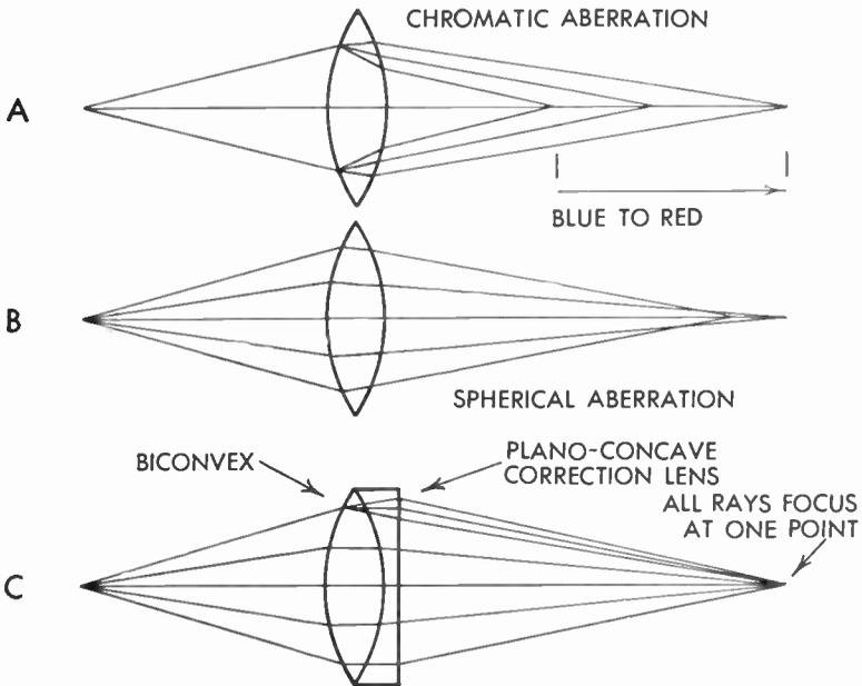
FIG. 222 Correction of Spherical and Chromatic Aberrations
