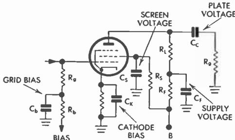
FIG. 347 Supply-Voltage Points RC Filtering
