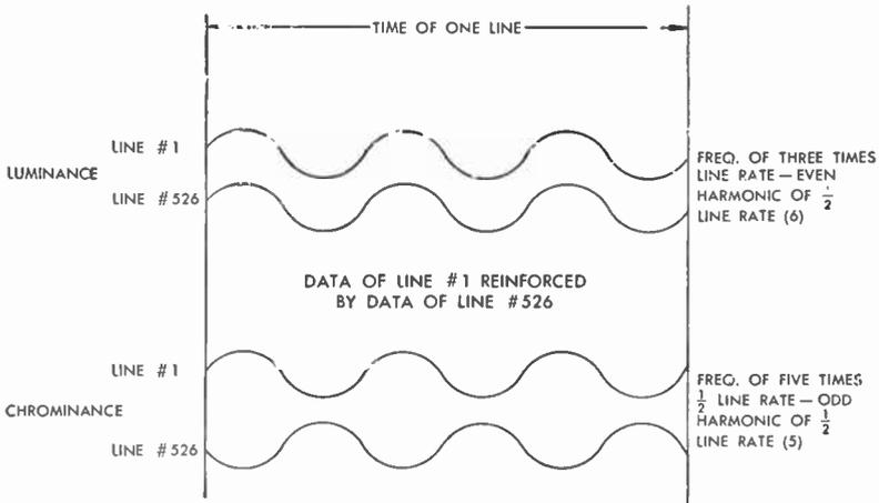
FIG. 13 Frequency Interference Cancellation of Chrominance Crosstalk in Luminance Channel
