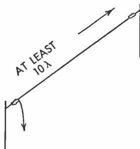
FIG. 265 Long-Wire Antenna
