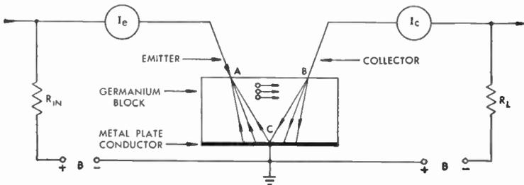
FIG. 416 Basic Transistor Circuit
