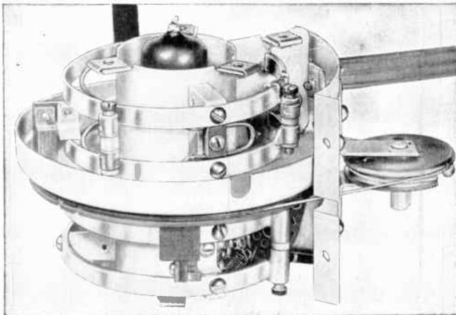
Fig. 394 Tuned Resonant Lines
