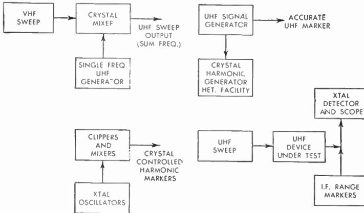
Fig. 414 Sweep Alignment and Marker Generator Systems
