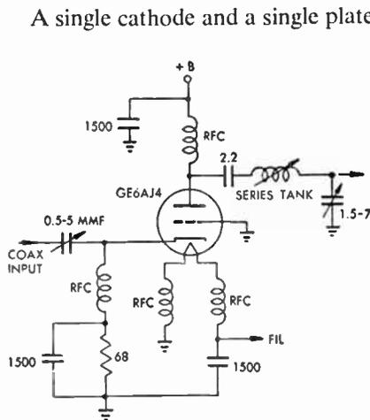
FIG. 389e Grounded-Grid R-F Stage
