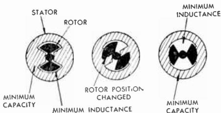
FIG. 383 Butterfly-Tuned Circuit
