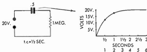
FIG. 345 Time Constant and Capacitor Charge
