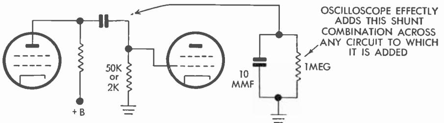
FIG. 293 Loading Effect of Scope
