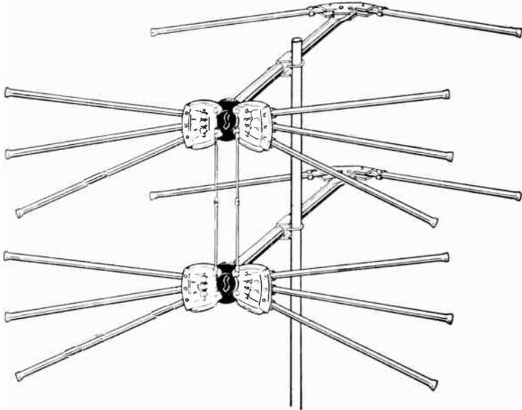
FIG. 254 Snyder Stacked Conicals
