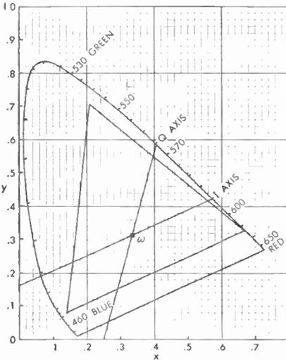
FIG. 20 Axes of  $I$  and  $Q$  Signals
