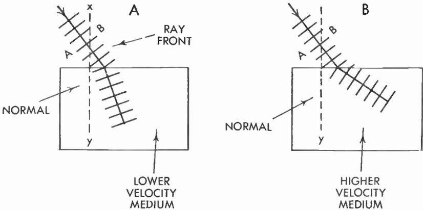
FIG. 218 Refraction of Rays Traveling between Two Media
