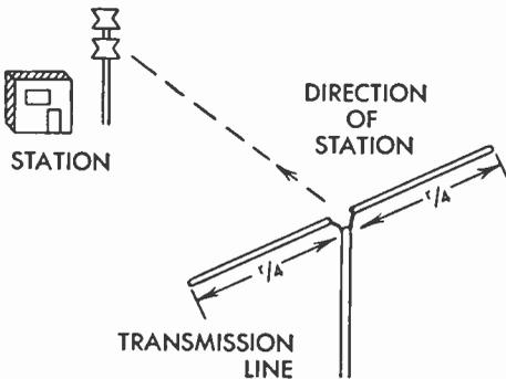
FIG. 233 Dipole Antenna Properly Oriented for Reception
