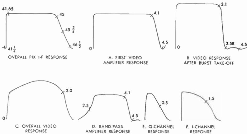
FIG. 44 Alignment Response Curves
