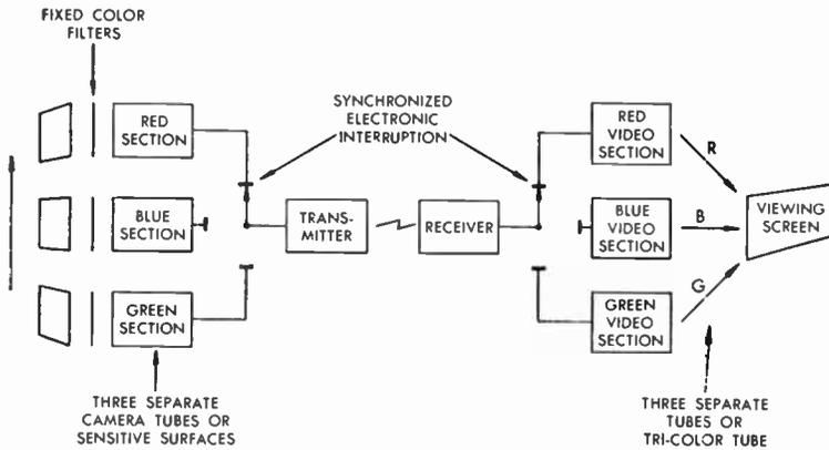
FIG. 11 Field Sequential Scanning with Electronic Interruption
