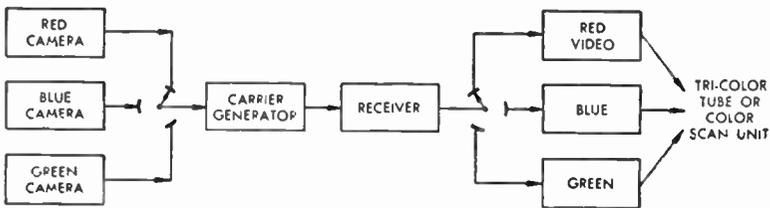
FIG. 6 Basic Methods of Color Transmission
