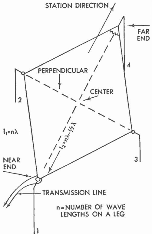
Fig. 264 Rhombic Construction
