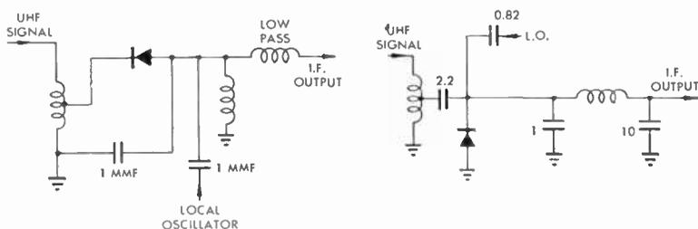
FIG. 389b Crystal Mixer Circuits
