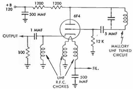
FIG. 409 UHF Test Oscillator
