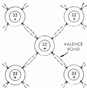
FIG. 418 Partial Arrangement of Germanium Atoms
