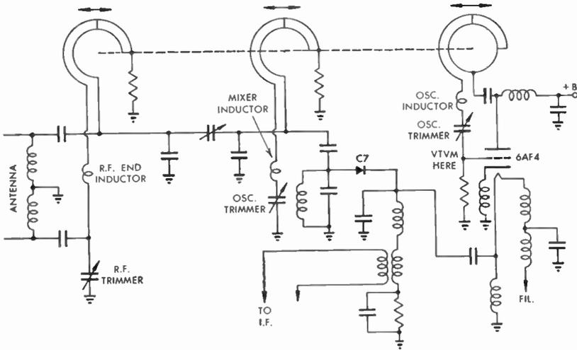
FIG. 413 Alignment of Sutco UHF Section
