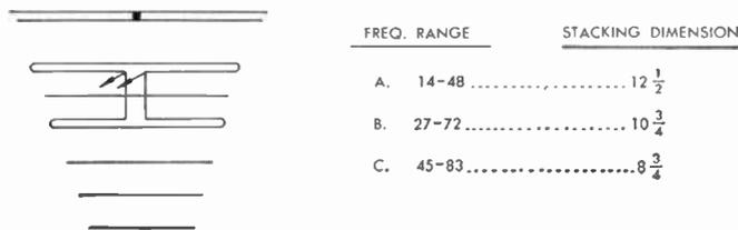
FIG. 362 Snyder UHF Yagi
