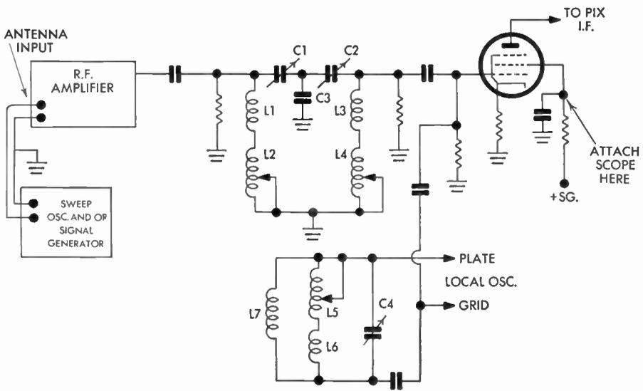
FIG. 313 Inductuner Alignment
