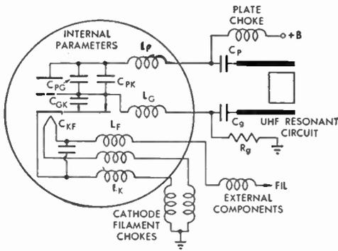
FIG. 389c Local Oscillator Stage
