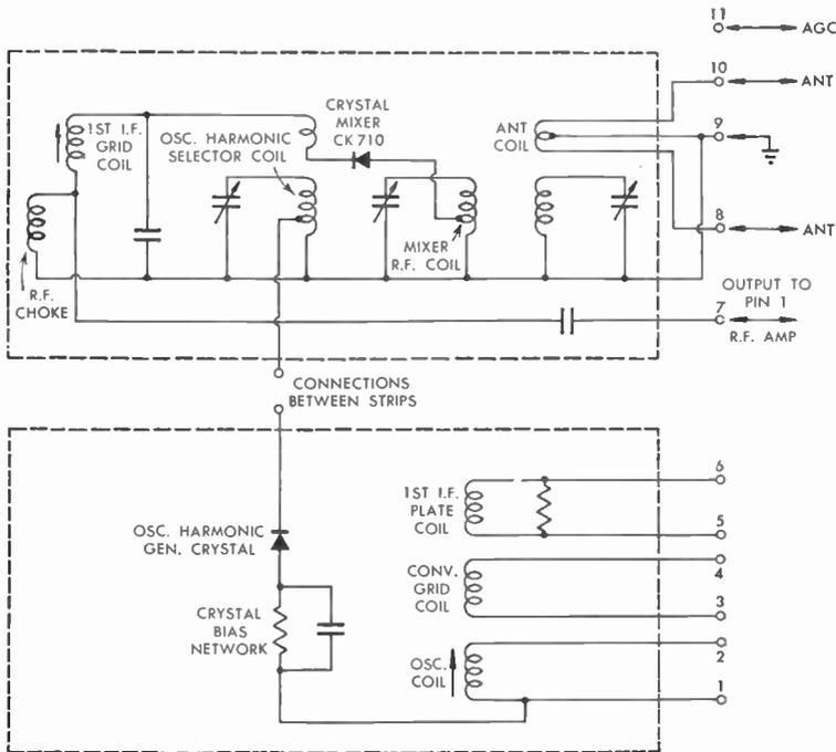
FIG. 373 Schematic of Standard Coil Plug-In Strip
