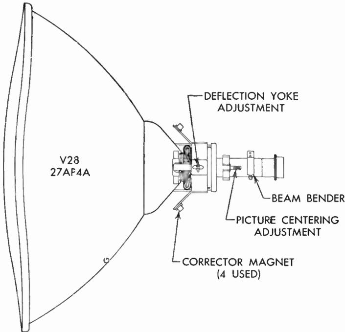
FIG. 277 Zenith Picture-Tube Mount
