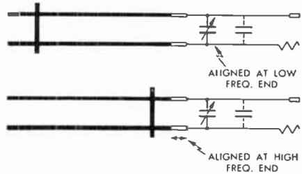
FIG. 380 Tuned Lines as Resonant Circuits
