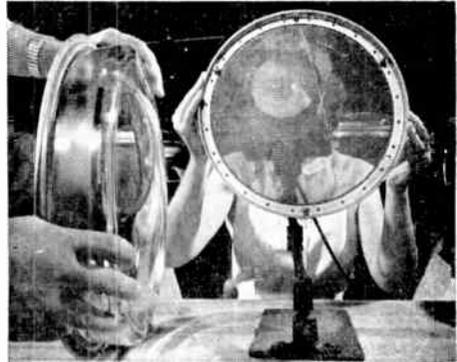
FIG. 35 Shadow Mask of Tricolor Tube
