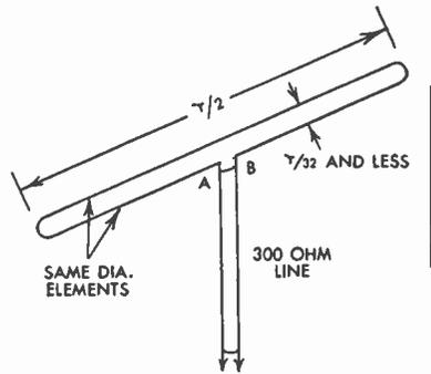
FIG. 239 Folded Dipole Antenna
