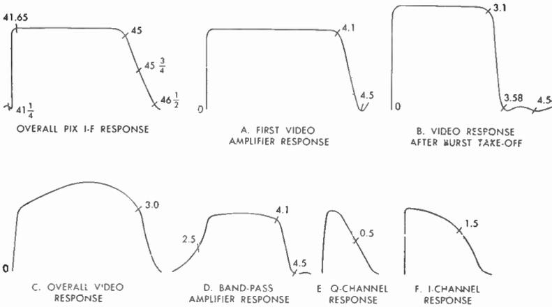
Fig. 44 Alignment Response Curves (Repeated)
