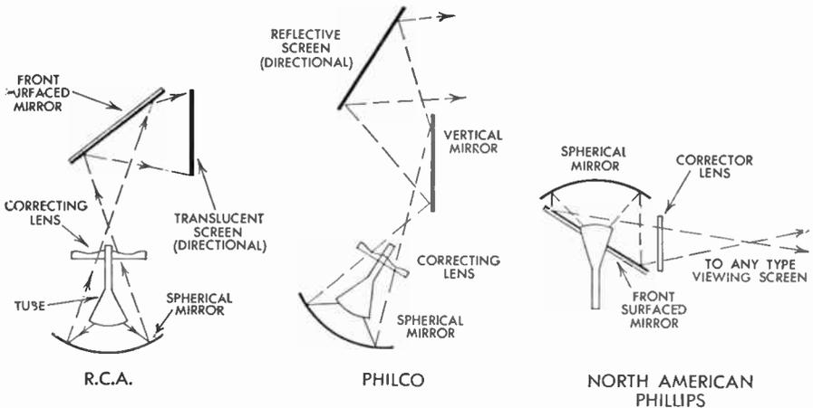
FIG. 224 Modified Schmidt Projection Systems for Television
