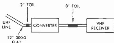
FIG. 415 Peaking of UHF Signal
