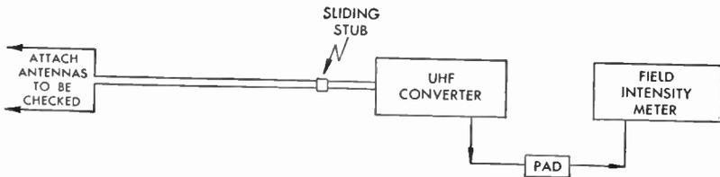
FIG. 411 Antenna-Performance Checks
