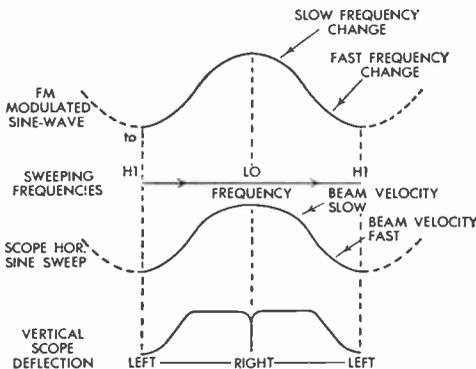
FIG. 298 Timing of Sweep Frequencies and Scope Sweep
