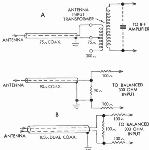
FIG. 292 Matching Coaxial Lines to Receiver Input
