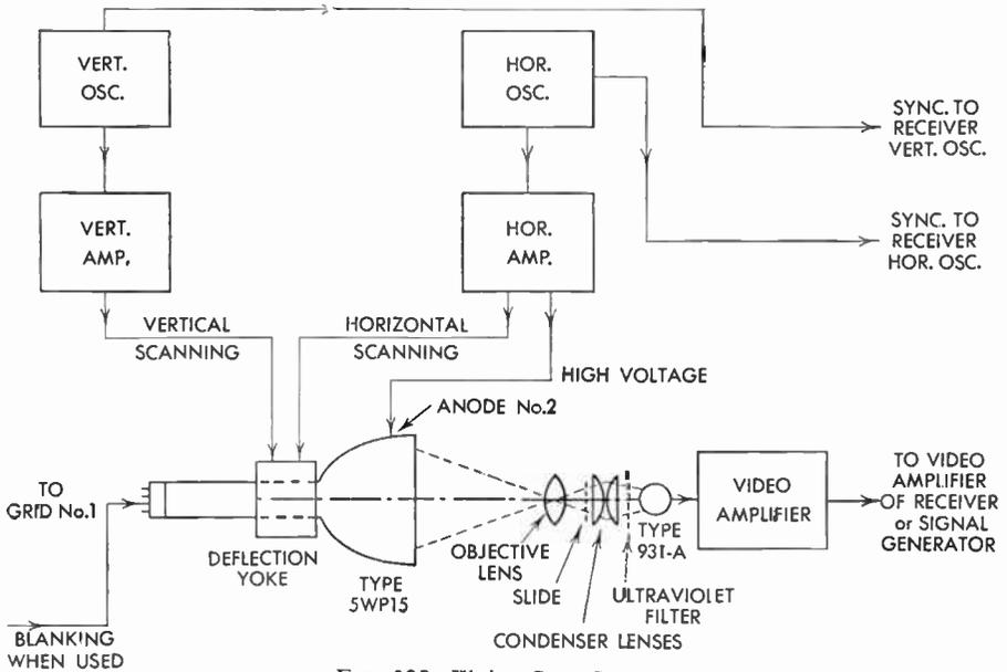
FIG. 322 Flying Spot Scanner
