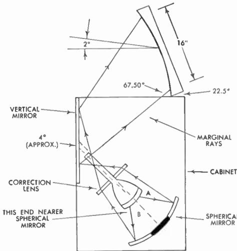
FIG. 227 Mechanical Layout Philco Projection System
