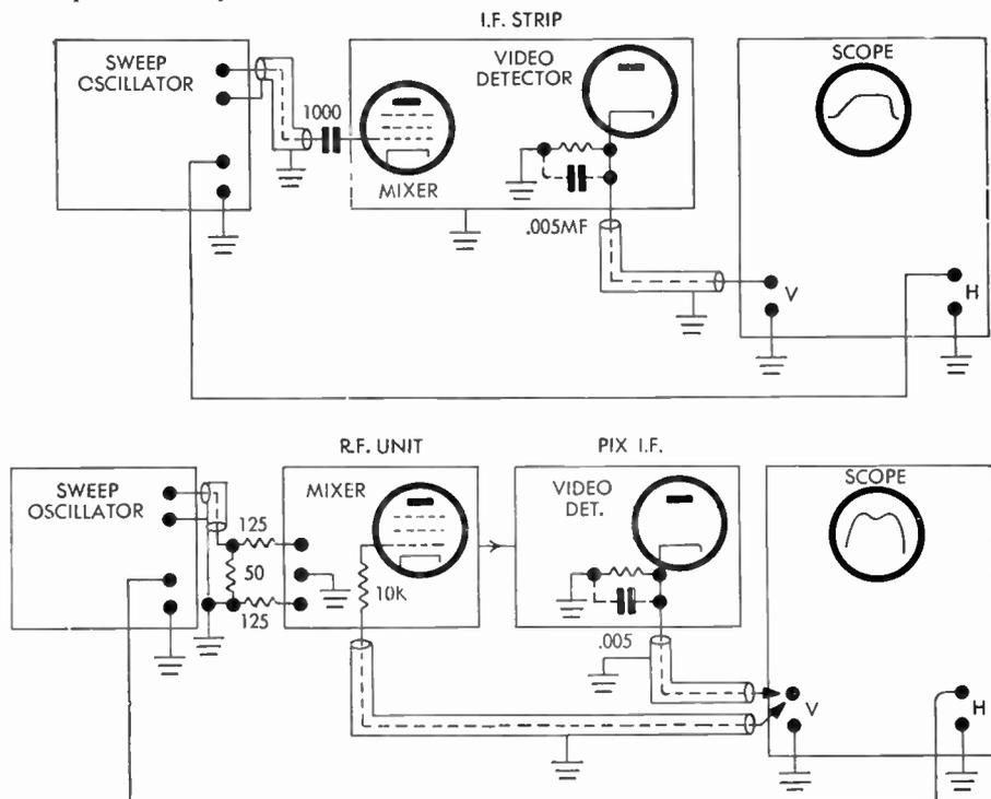
FIG. 306 Sweep Oscillator Interconnections for TV R-F and I-F Alignment
