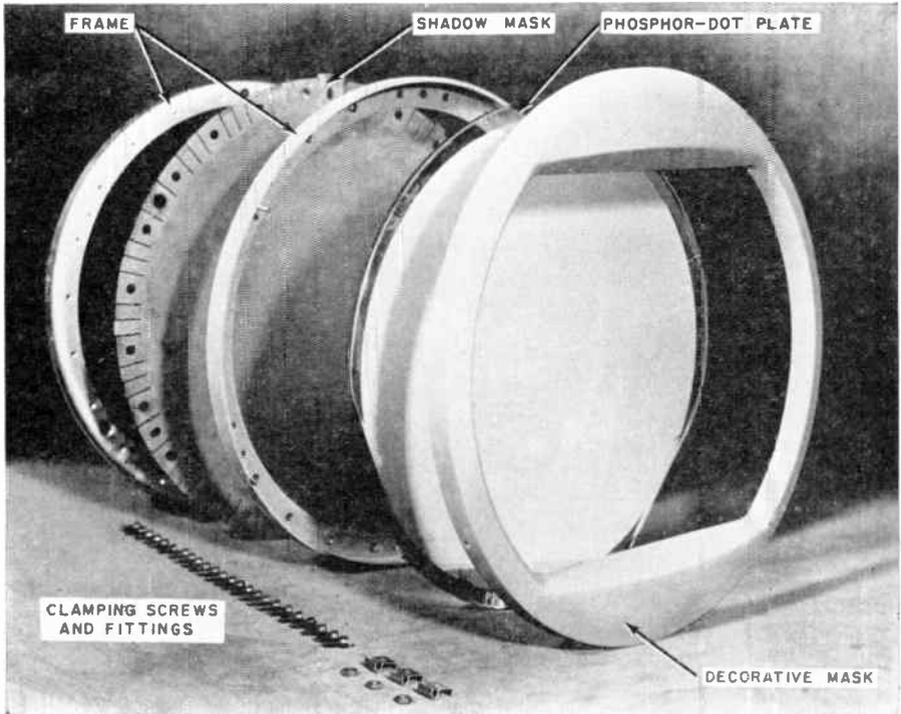
FIG. 36 RCA Tricolor Tube Viewing Screen Assembly
