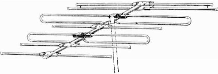
FIG. 258 Snyder Wideband Yagi
