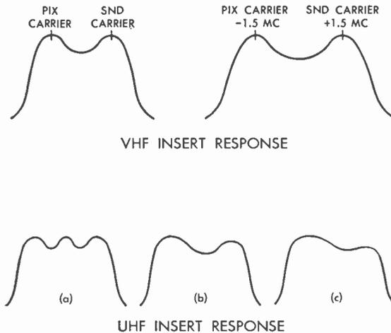
FIG. 326 Tuner Response Curves
