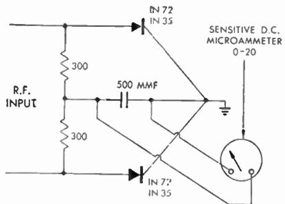
Fig. 408 Balanced Crystal Detector
