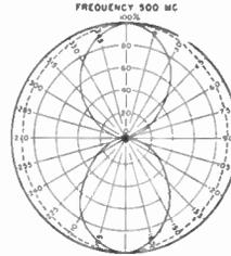
The triangular dipole has a bi-directional pattern and a rising gain with frequency. It provides an optimum match over the UHF band and represents a simple, small, and effective antenna for UHF strong signal areas.
