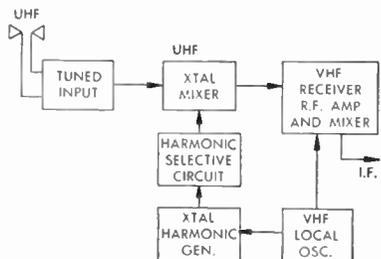
Fig. 372 Block Diagram Plan of UHF Plug-In Strip
