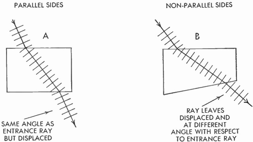
FIG. 219 Rays Leaving Parallel and Nonparallel Exit Sides of Different Media
