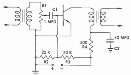
FIG. 423 Transistor Audio Amplifier
