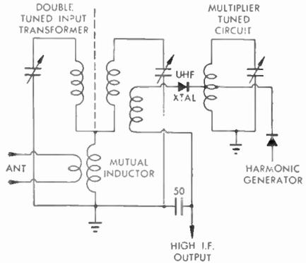
FIG. 374 UHF Section of Zenith Strip
