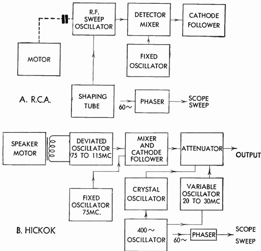
FIG. 299 Mechanical Sweep Oscillators
