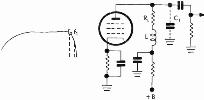
FIG. 332 Video Amplifier, Shunt Peaking
