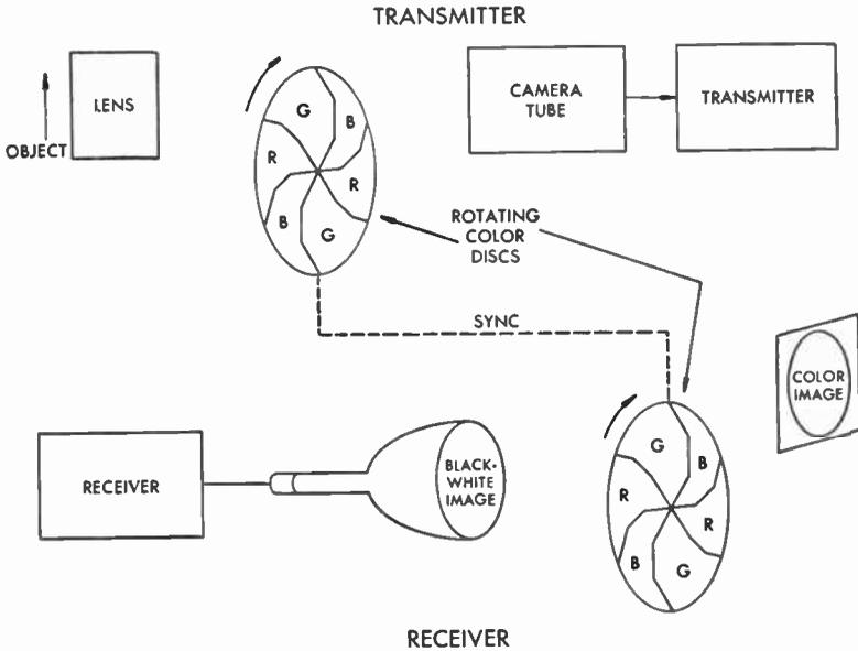
FIG. 10 Field Sequential Color System
