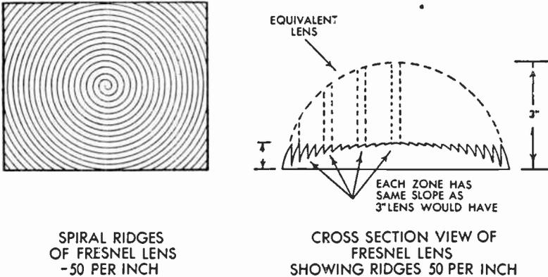
FIG. 232 Fresnel Lens System
