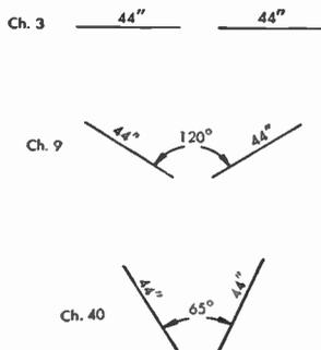
FIG. 363 Antenna Element Tilt Angle
