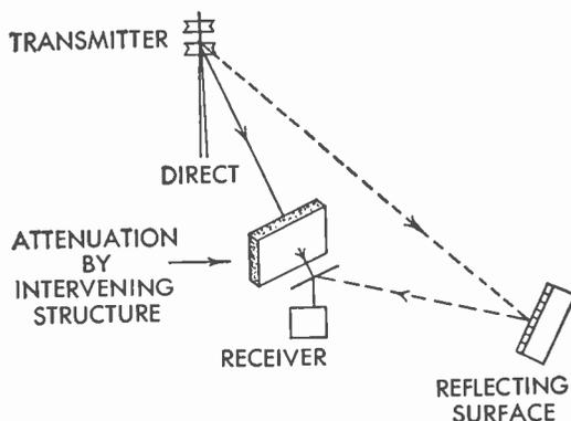
FIG. 288 Attenuation of Direct Signal by Intervening Structure
