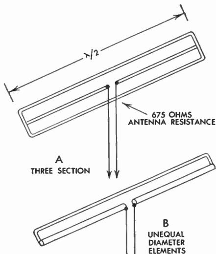
FIG. 240 Special Folded Dipoles
