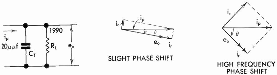
FIG. 336 High-Frequency Phase-Shift Vectors
