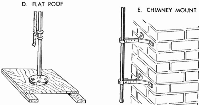
FIG. 287 Supporting Antenna on Roof
