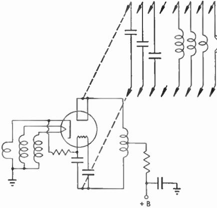
FIG. 406 UHF Local Oscillator Switching
