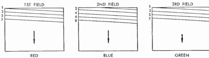
FIG. 7 Field Sequential Color Scanning
