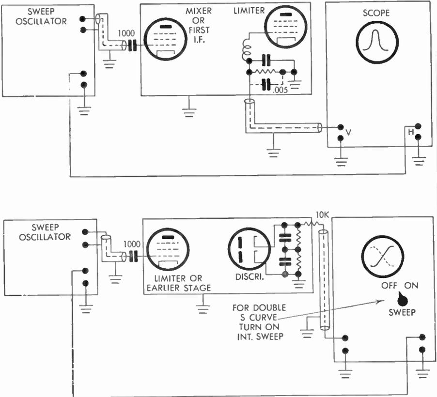
FIG. 307 Sound Channel Alignment with Sweep Oscillator
