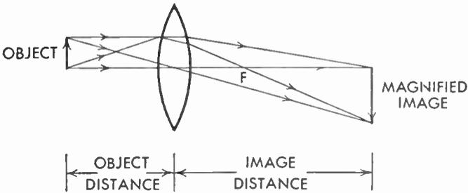
FIG. 221 Object Inversion with a Lens
