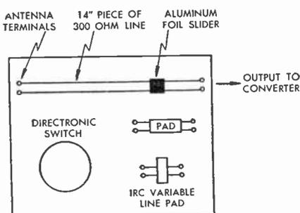
FIG. 412 UHF Test Board
