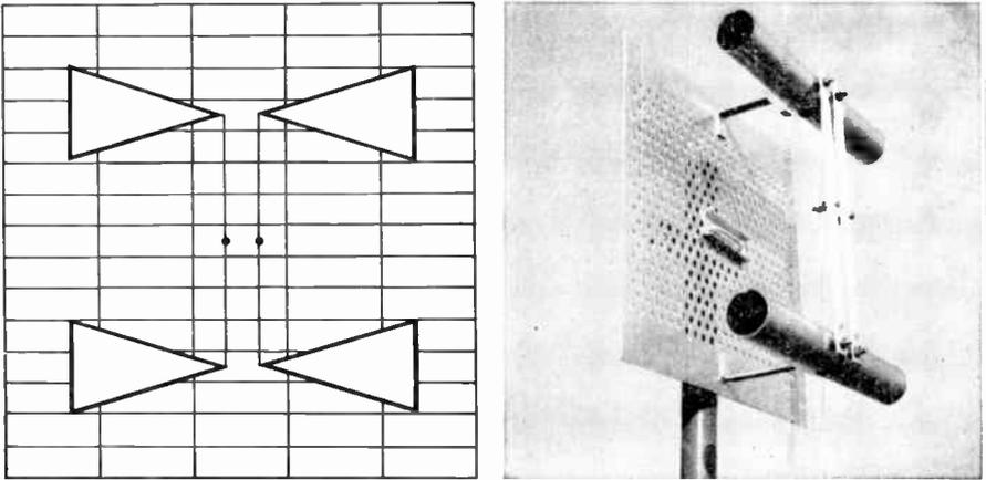
FIG. 360 Stacked UHF Antennas
