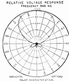
The corner reflector is a more elaborate UHF antenna, but it has a high gain and an excellent response pattern when dimensioned properly. It can be used for UHF fringe reception and, despite its high gain, will also have wide application in stronger signal areas because of its excellent rejection of reflections and interference. It will solve many propagation problems which other types cannot.
