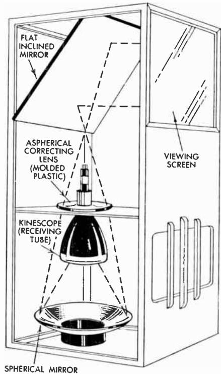
FIG. 230 Arrangement of Components of RCA Projection System
