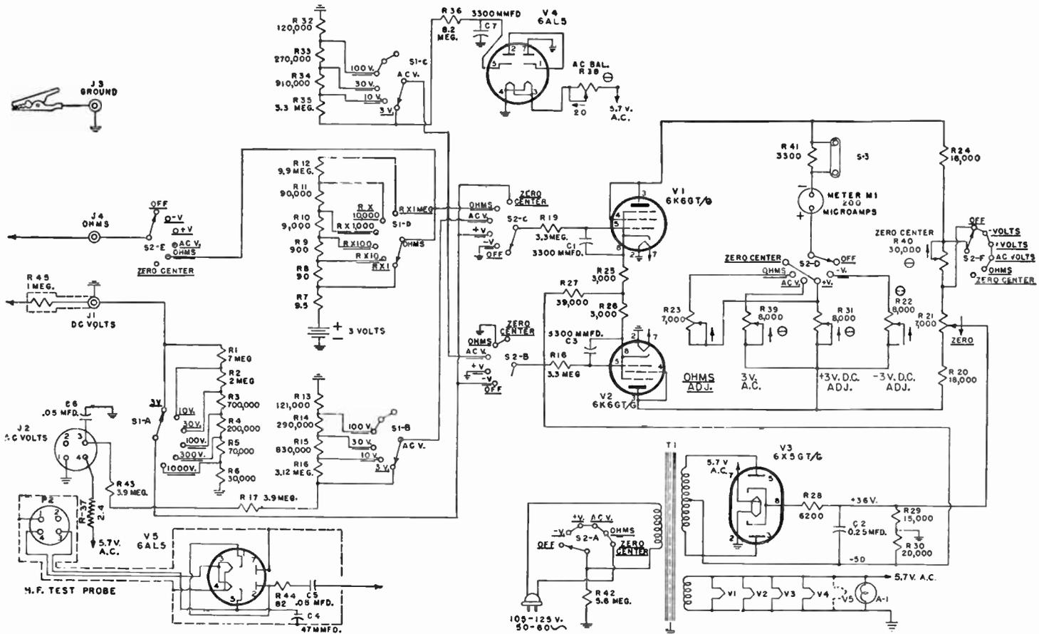
FIG. 296 RCA Vacuum-Tube Voltmeter
