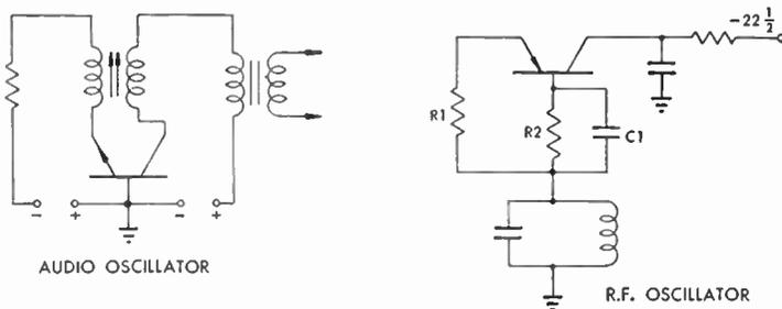
Fig. 425 Transistor Oscillators
