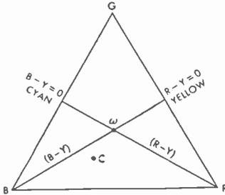
FIG. 28 Position of Axes on Color Triangle
