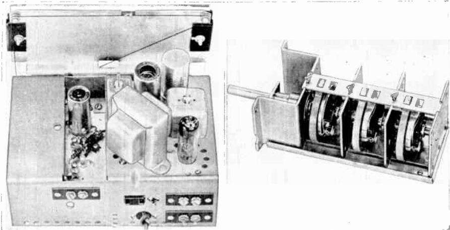
FIG. 392 Mallory UHF Converter and Tuned Lines
