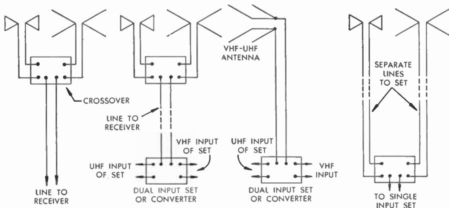
FIG. 369a Applications for VHF-UHF Crossover Networks
