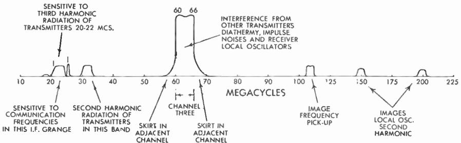
FIG. 290 Sources of Interference with Receiver Set on Channel 3—25 Megacycle-I-F
