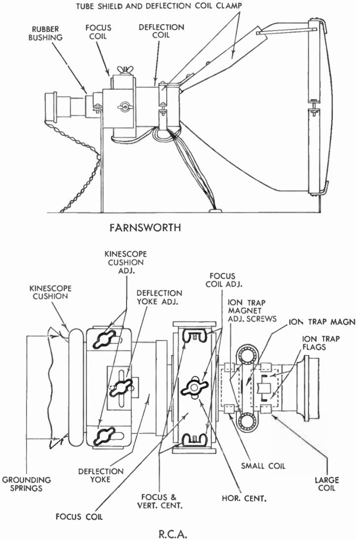
Fig. 273 Typical Picture-Tube Mountings
