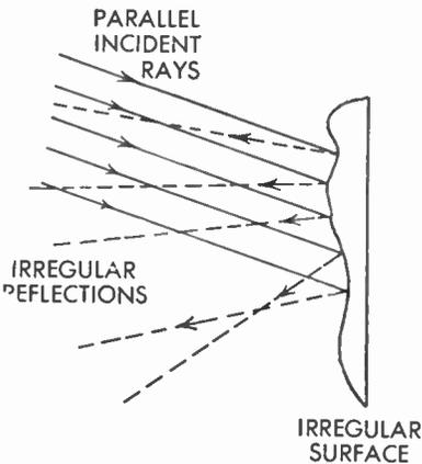
FIG. 215 Reflection from Irregular Surfaces
