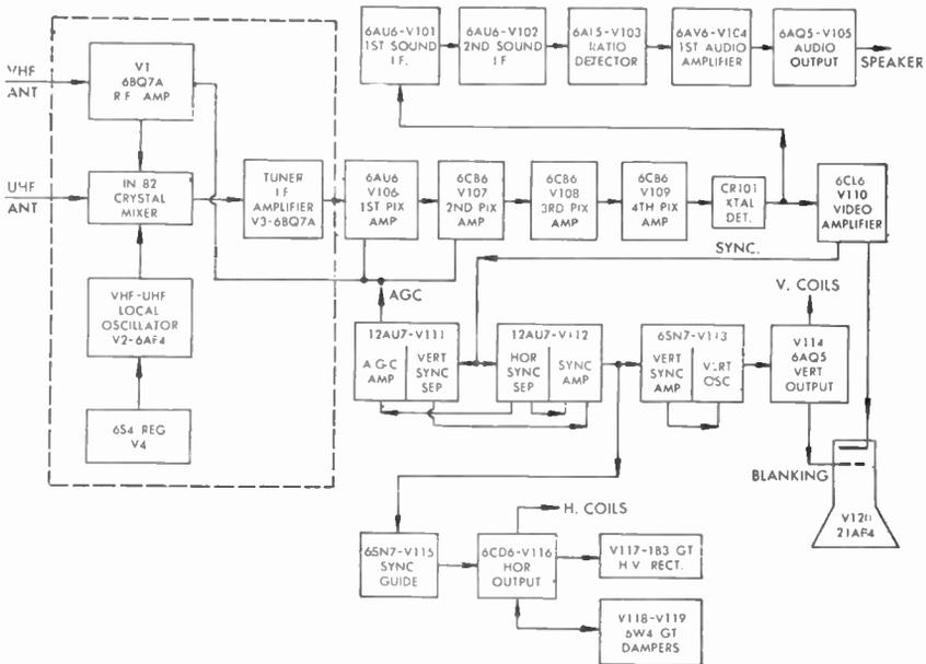
Fig. 210a Functional Block Diagram of Modern Receiver
