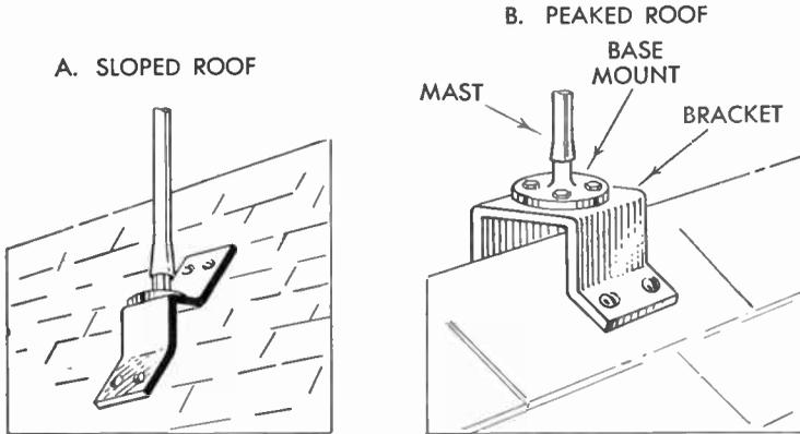
FIG. 285 Roof Mounts
