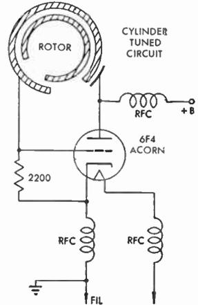
FIG. 387 UHF Oscillator with Cylinder-Tuned Circuit
