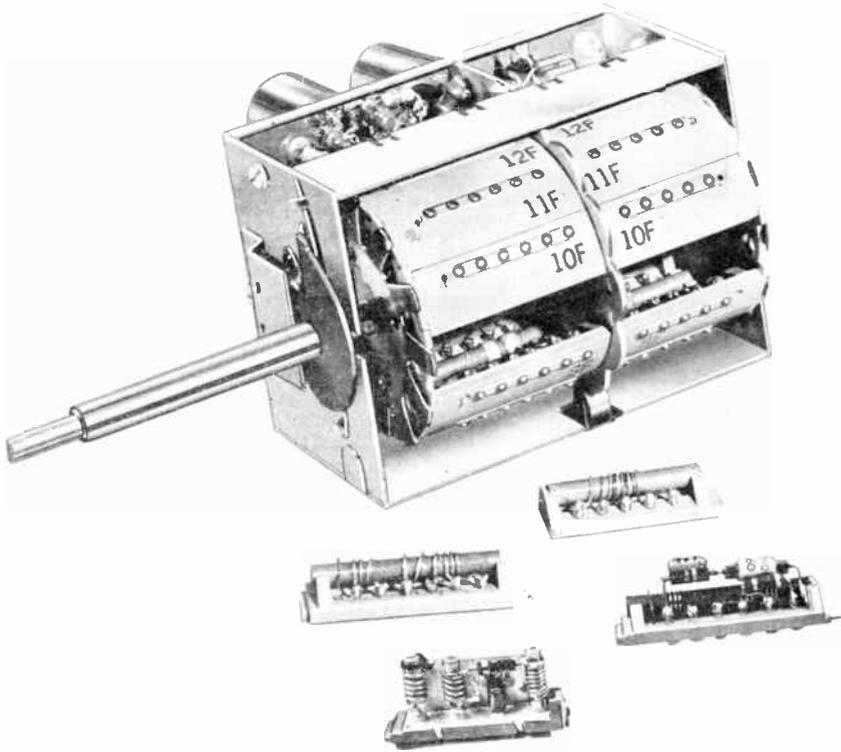
FIG. 370 Standard Coil UHF Strips
