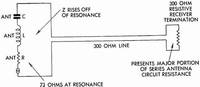
FIG. 235 Equivalent Antenna Circuit—Current Take-Off
