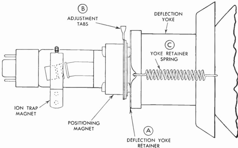
FIG. 278 DuMont Picture-Tube Mount
