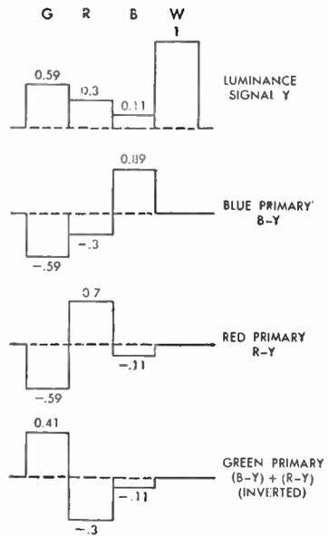
FIG. 23 Signals for Saturated Color Bars—NTSC Constant Luminance
