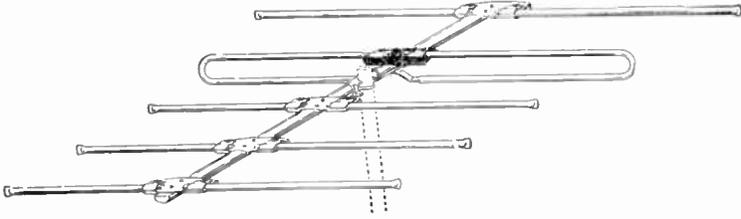
FIG. 257 Single-Channel 5-Element Yagi
