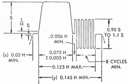
FIG. 16 Color Sync Burst on Backporch of Horizontal Sync Pulse
