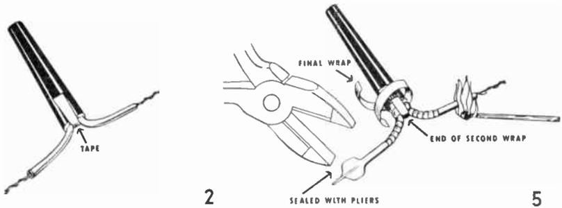
Spread the conductors apart and place two 1" pieces of sealing tape across the crotch as illustrated in step 2. The tape should be applied under tension.
