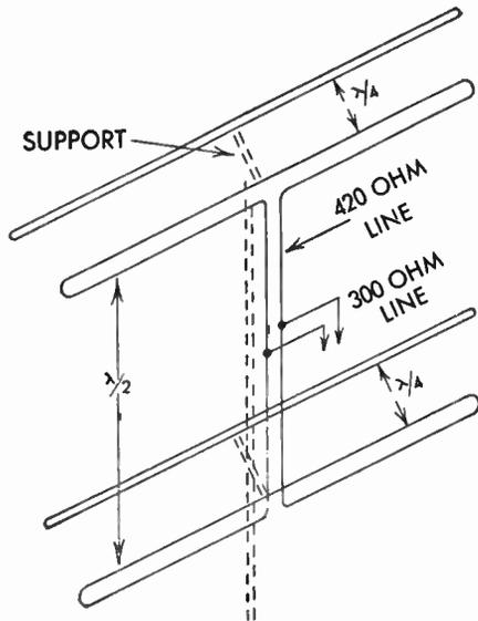
FIG. 246 Stacked Folded Dipoles and Parasitic Reflectors
