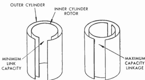
FIG. 386 Cylinder-Tuned Circuit
