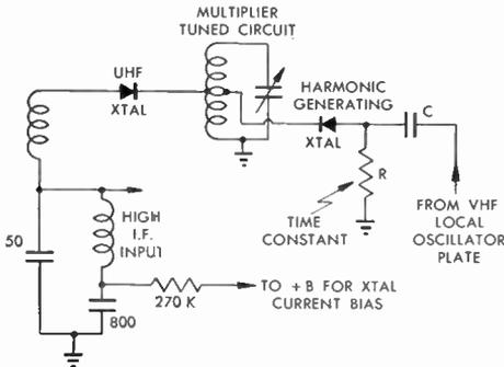
FIG. 376 Harmonic Generating Section
