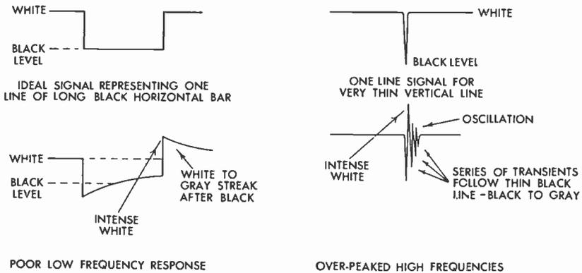
FIG. 270 Frequency Response and Its Effect on Portions of Picture Signal
