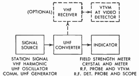
FIG. 407 UHF Test Equipment Plan
