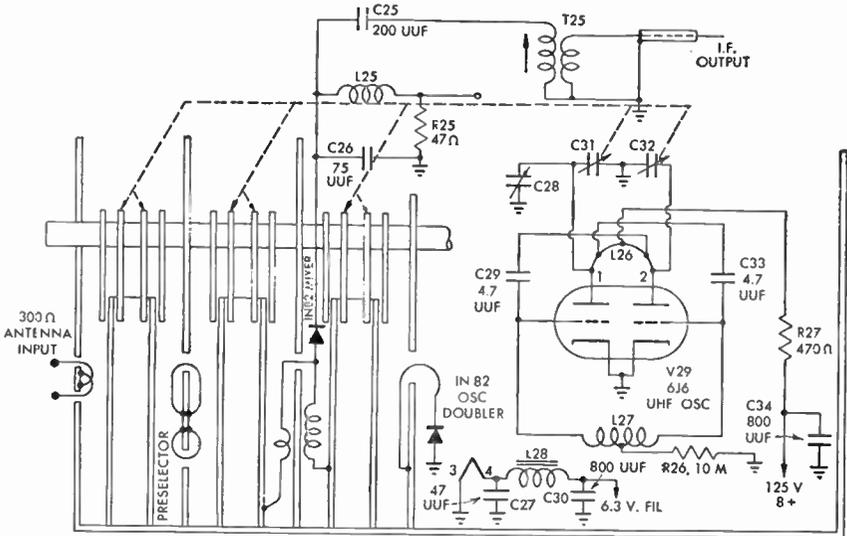
FIG. 397 General Instrument Converter
