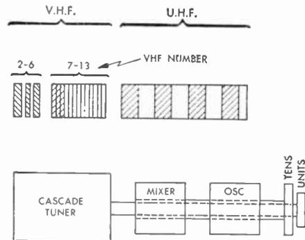
FIG. 405 Channel Selection Plan
