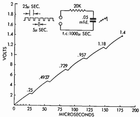
FIG. 351 Voltage across Integrating Capacitor
