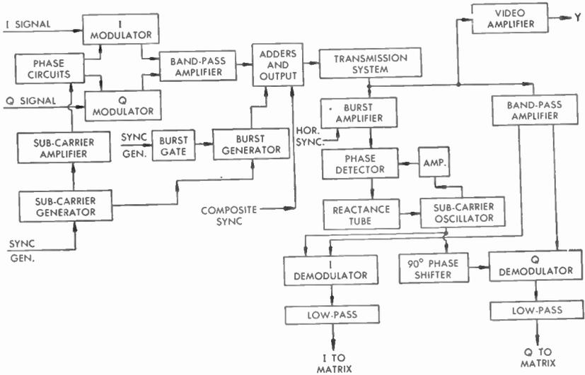
FIG. 26 Functional Block Plan of Chrominance Modulation System
