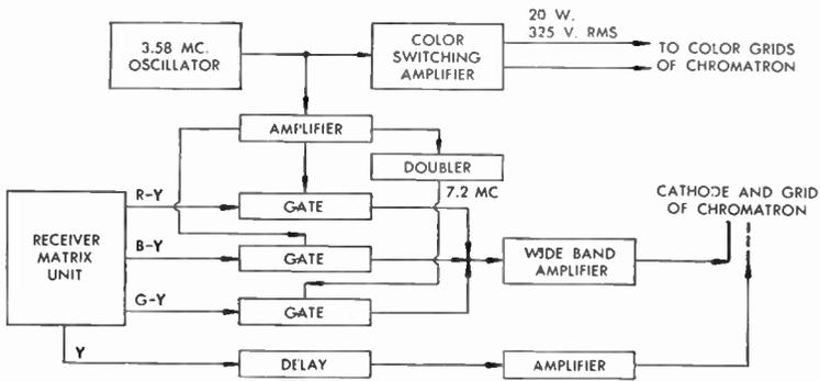
FIG. 46 Decoding NTSC Signal for Chromatron
