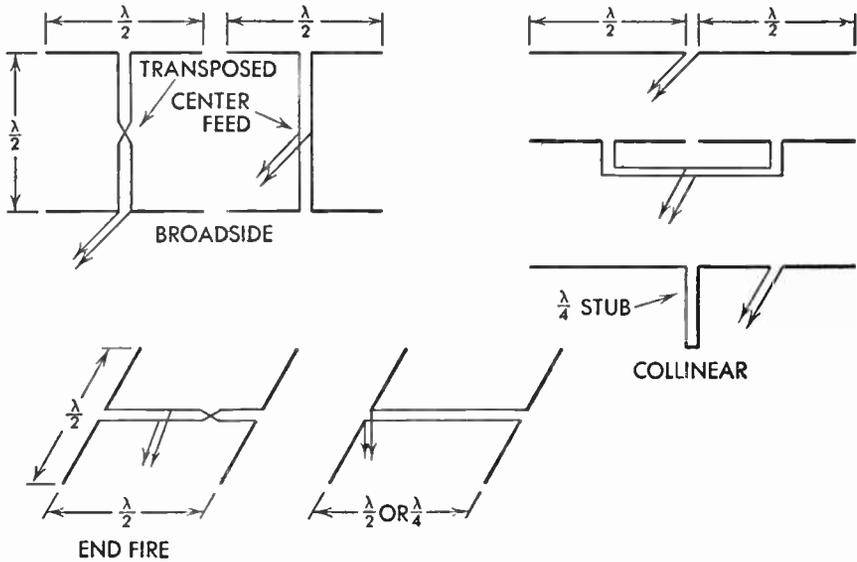
FIG. 248 Types of Two-Element Phased Antennas \*
