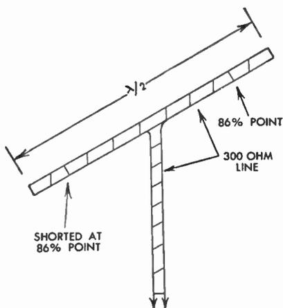
FIG. 241 Twin-Wire Folded Dipole
