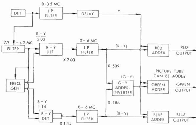
FIG. 45 Narrow Band Decoder
