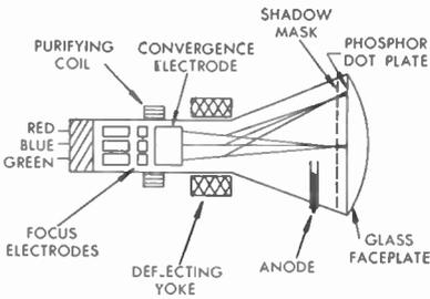
FIG. 33 Components of Color Tube
