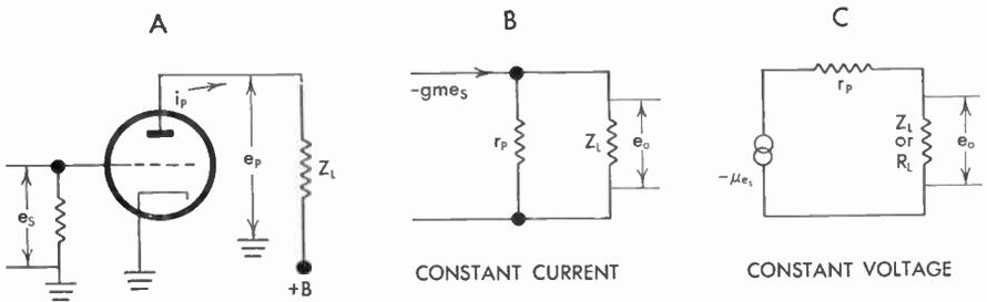
FIG. 328 Basic Vacuum Tube and Equivalents
