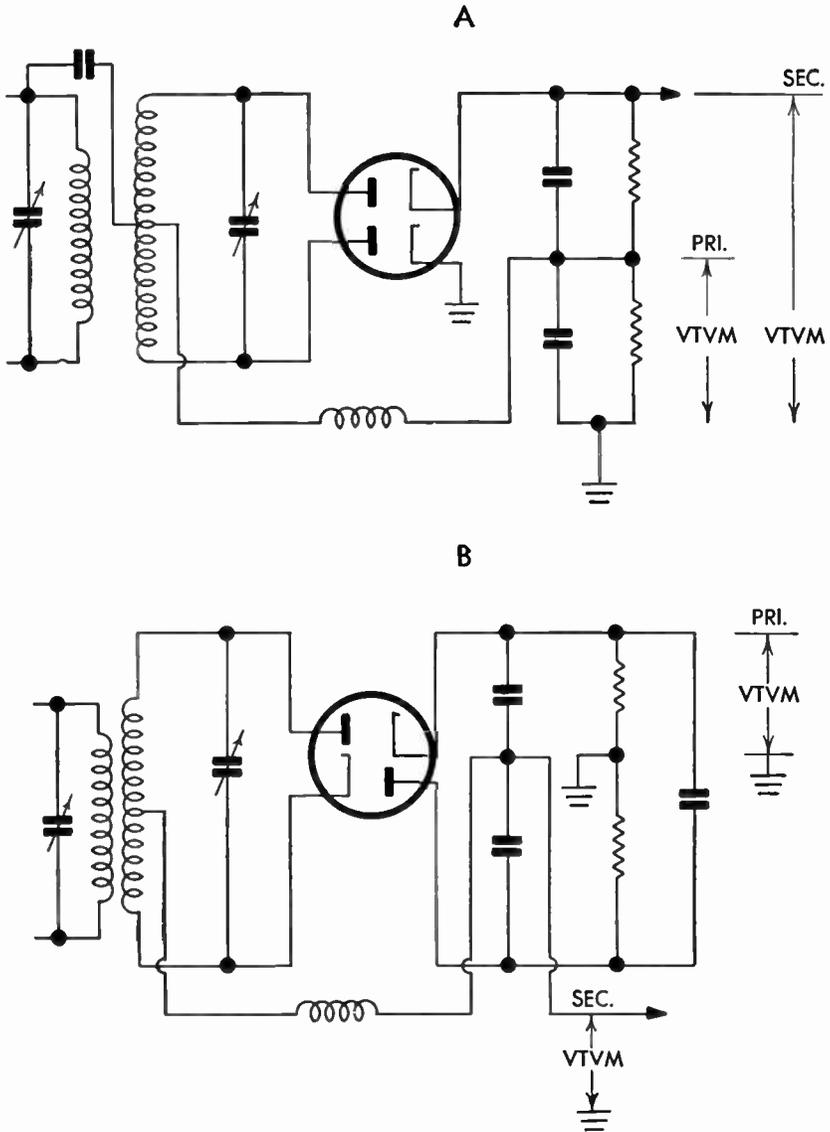
FIG. 309 Meter Alignment of Discriminator and Ratio Detector
