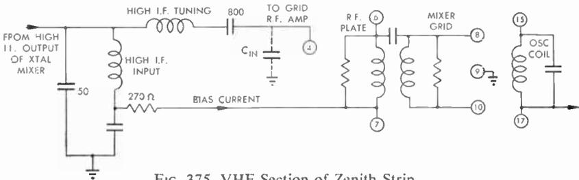
FIG. 375 VHF Section of Zenith Strip
