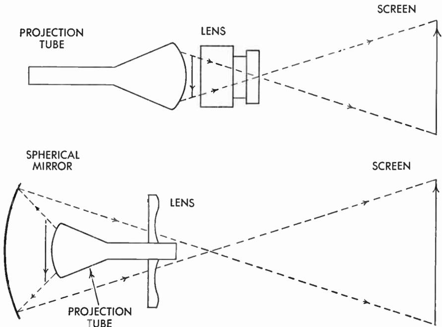
FIG. 211 Direct and Reflective Projection Systems
