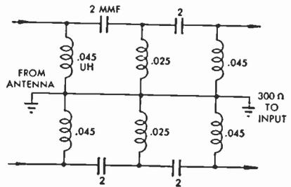
FIG. 389a High-Pass Filter to Block VHF Interference
