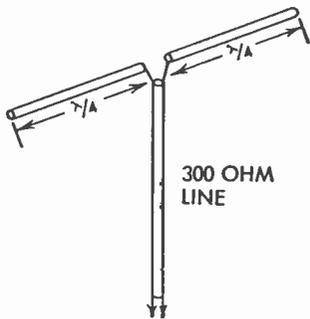
FIG. 236 Dipole Antenna—Mismatched
