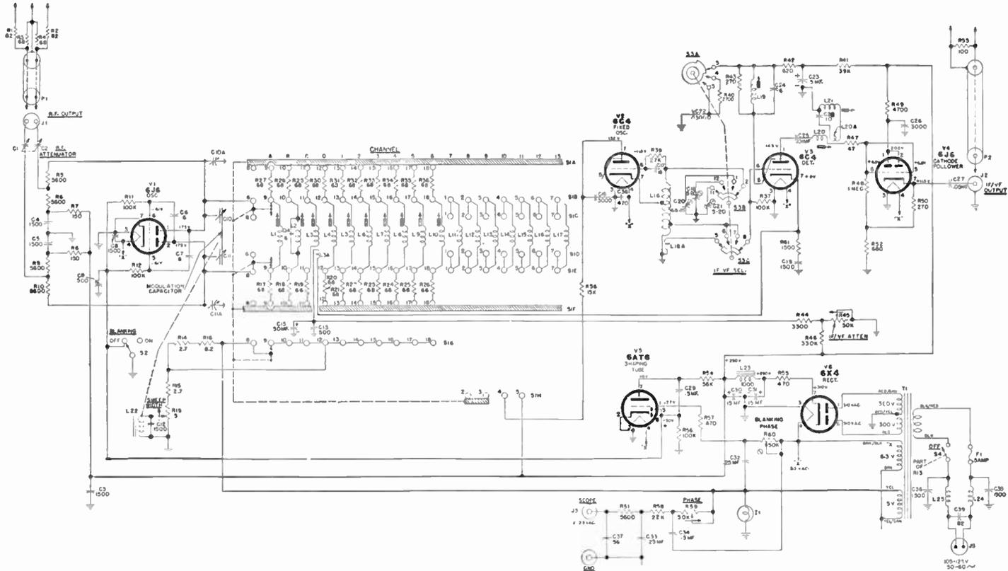
FIG. 303 RCA Sweep Oscillator
