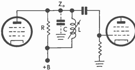
FIG. 356 Wideband Amplifier Output Circuit
