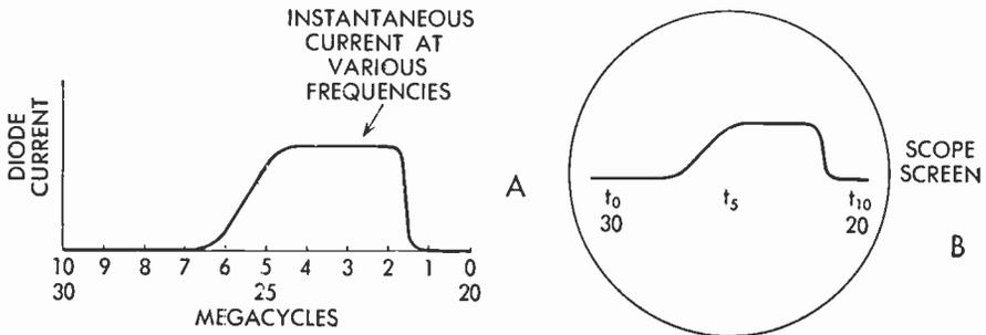
FIG. 297 Diode Current and Response Curve on Scope
