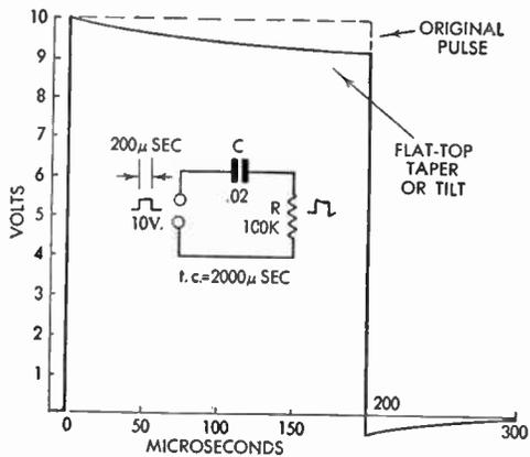
FIG. 352 Conveying a Pulse through  $RC$  Coupling Network
