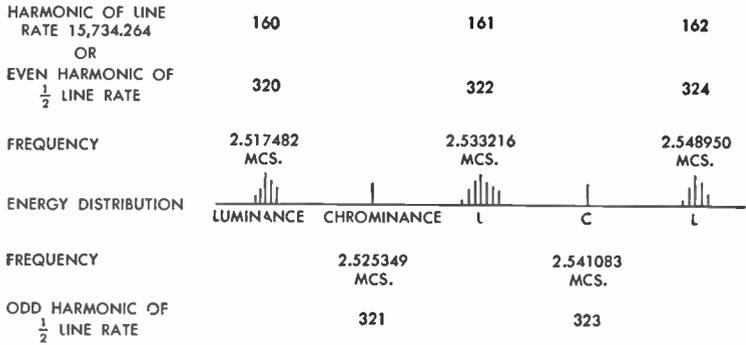
FIG. 12 Energy Distribution over Small Segment of Video Spectrum
