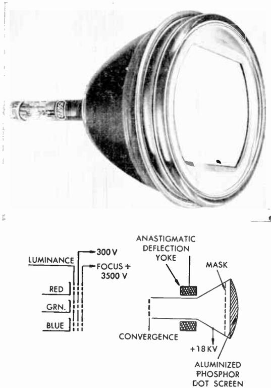
FIG. 17 General Plan of Tricolor Tube
