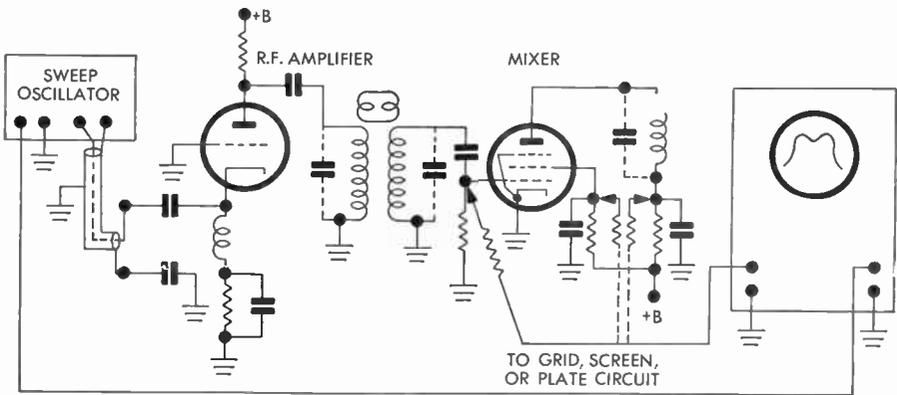
FIG. 312 R-F Amplifier and Mixer Alignment
