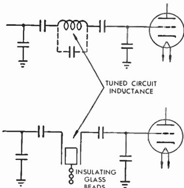
FIG. 388 Reactance Section as Tuned Element
