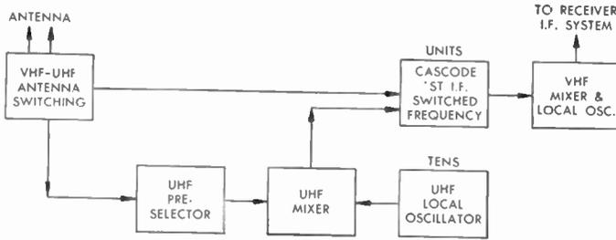
FIG. 404 Block Plan of VHF-UHF Tuner
