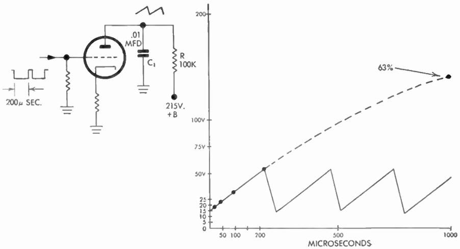
FIG. 353 Generation of a Sawtooth
