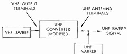
Fig. 414b Indirect UHF Sweep Generator
