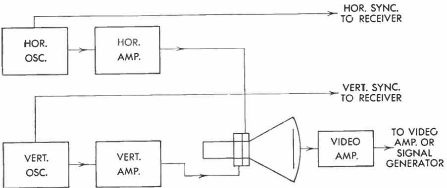
FIG. 323 Monoscope Video Signal Generator
