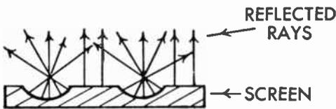
FIG. 229 Vertical Grooves Disperse Light Horizontally
