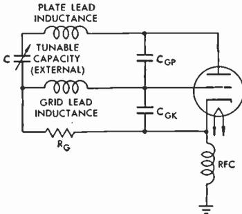
FIG. 389 Series-Tuned Oscillator
