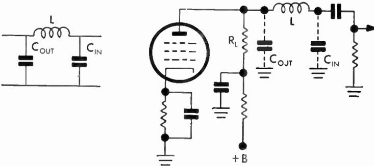
FIG. 333 Video Amplifier, Series Peaking
