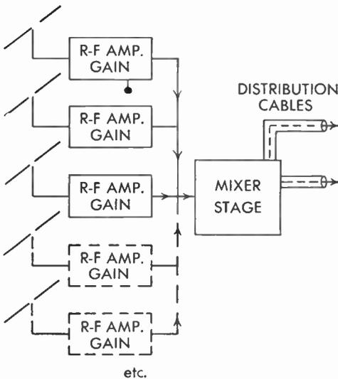
FIG. 267 Multiple-Outlet System. Separate Antennas
