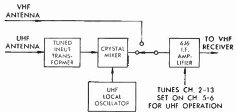
FIG. 395 Sutco VHF-Booster UHF-Converter Plan
