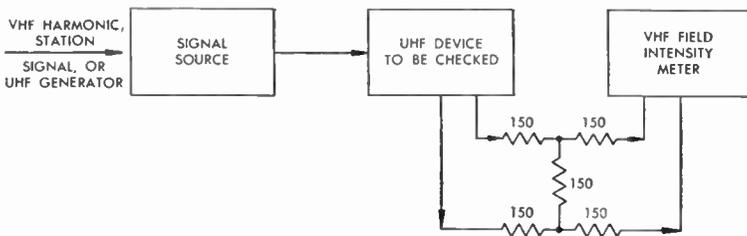
Fig. 407a VHF Field-Intensity Meter as UHF Peak Alignment Indicator
