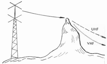
FIG. 358 VHF-UHF Coverage at Rear of Hill
