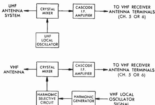
FIG. 377 Basic UHF Converter Methods
