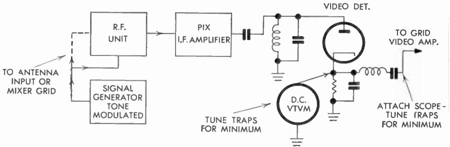
FIG. 314 Wavetrapping Alignment
