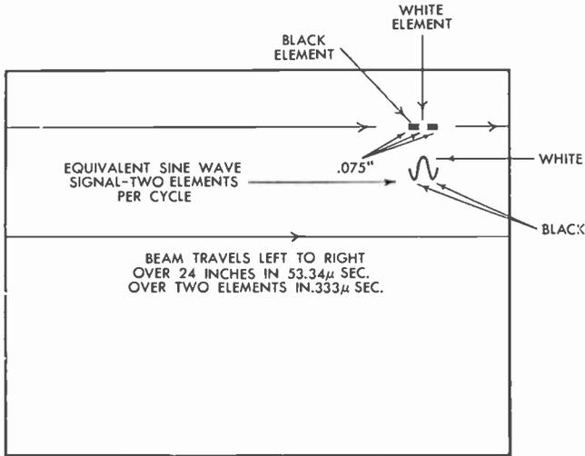
FIG. 272 Scanning of Three Equivalent Elements of a Line of Picture
