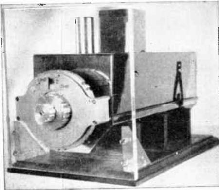
FIG. 403 Standard Coil 82-Channel Dial System
