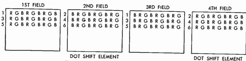
FIG. 9 Dot Sequential Color Scanning
