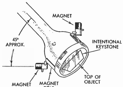
FIG. 228 Position of Keystone Magnets and Keystone Pattern
