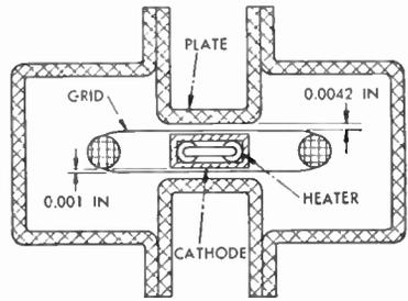
FIG. 389d UHF Tube Construction, RCA 6AF4
