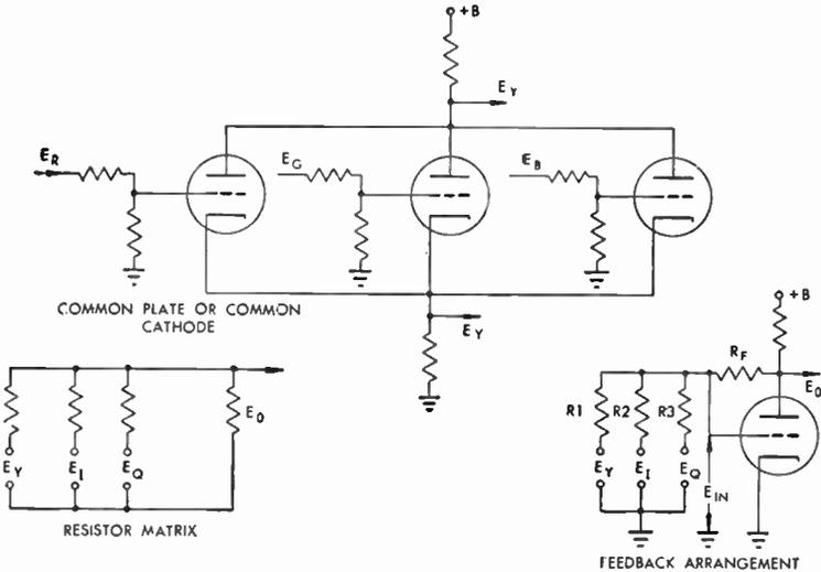
FIG. 24 Typical Matrix Circuits
