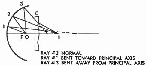
FIG. 226 Correction of Spherical Aberration by Corrector Lens at Center of Curvature
