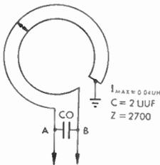
FIG. 382 Tuned Lines in Form of Arc
