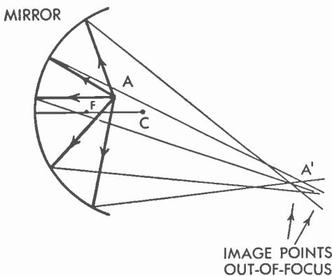
FIG. 217 Spherical Aberration
