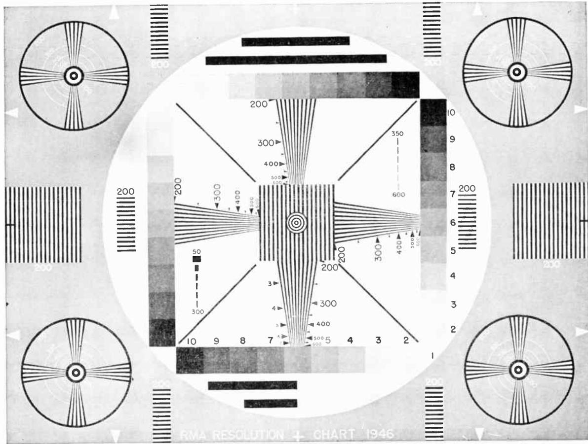
Fig. 269 RETMA Standard Test Chart
