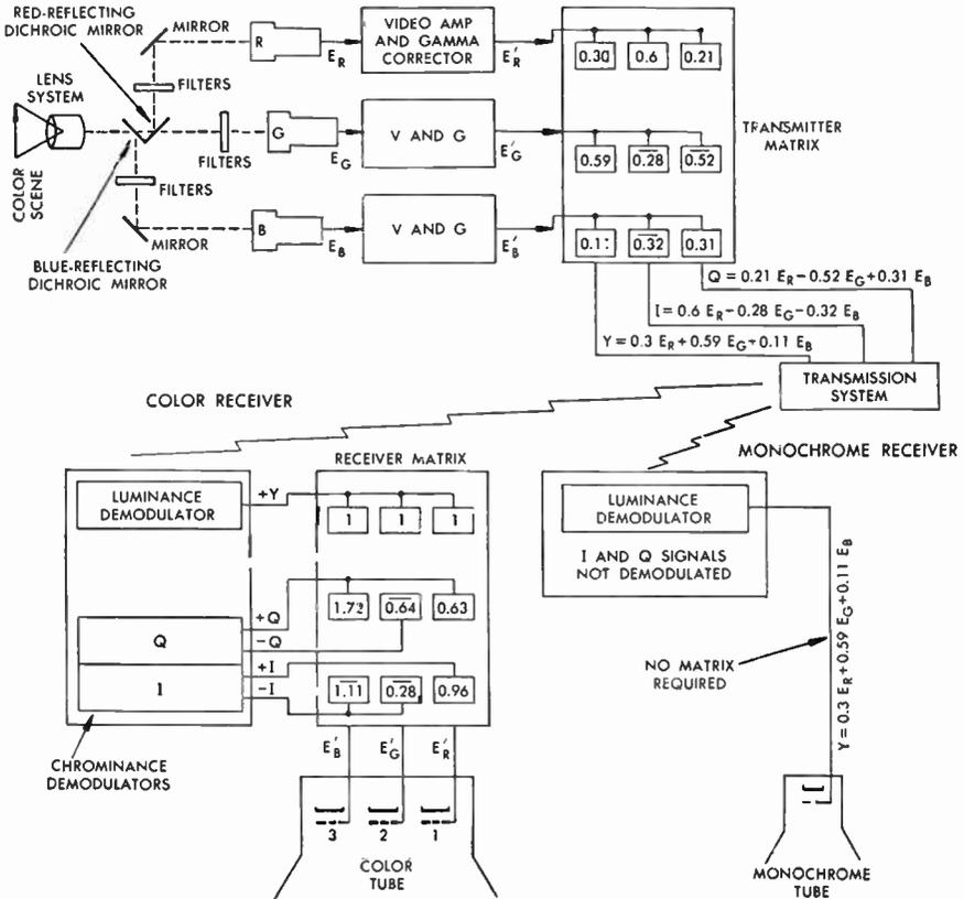
FIG. 19 Formation of NTSC Signals Showing Matrix Constants
