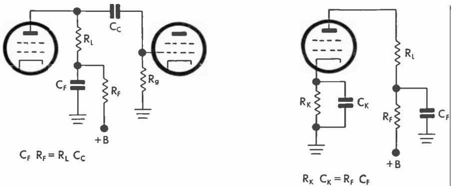
FIG. 330 Low-Frequency Compensation
