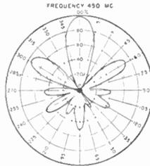
The stacked V is a longer-element and higher-gain antenna for UHF reception. It is inexpensive to construct and permits longer-range reception. It does have a multiple-lobe pattern and cannot be used in areas with reflection problems or severe interference.
