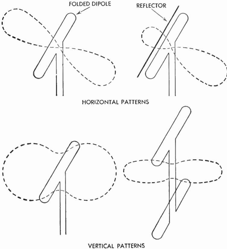
FIG. 247 Horizontal and Vertical Plane Directivity \*
