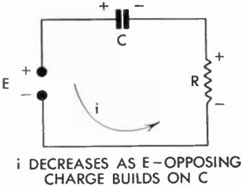
FIG. 342 Resistor-Capacitor Combination
