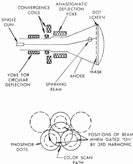
FIG. 43 Single-Gun Display for Color-Dot Screen
