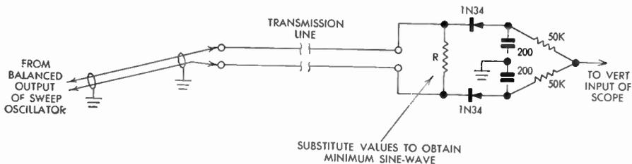
FIG. 320 Check of Transmission Line Surge Impedance
