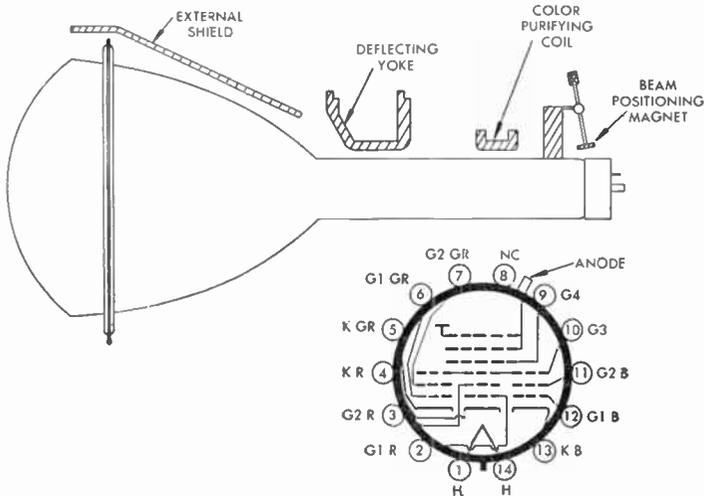
FIG. 39 Components and Basing of Colortron
