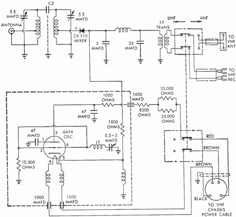
FIG. 398 RCA Single-Channel UHF Converter
