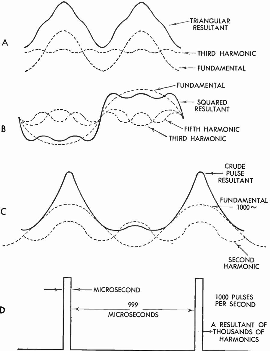
FIG. 348A Components of Complex Waves
