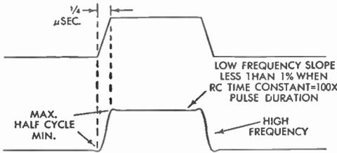
FIG. 349 Frequency Components of Pulse
