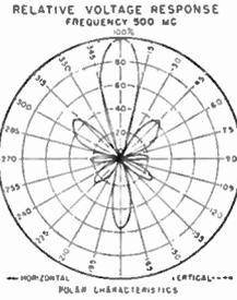
The rhombic antenna is a practical type for UHF reception because proper rhombic length at these frequencies comes down to some 50 inches. It has a high gain and a sharp directional pattern and must be oriented carefully. Fringe UHF reception is possible with this type. Although some minor lobes exist, reasonably good rejection of reflections and interference is provided.
