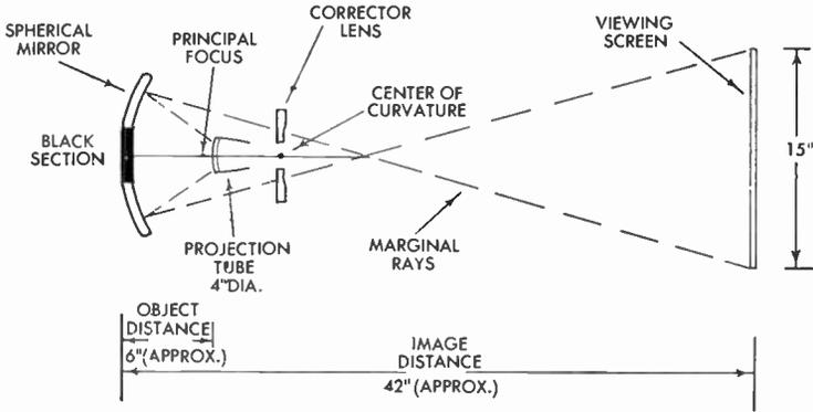
FIG. 225 Basic Plan of Philco Projection System
