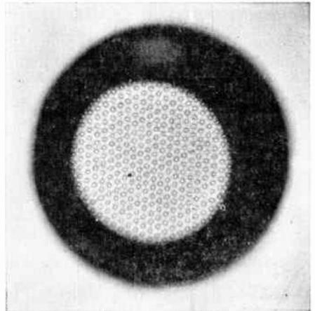
FIG. 34 Magnified Segment of Color-Dot Pattern on Screen
