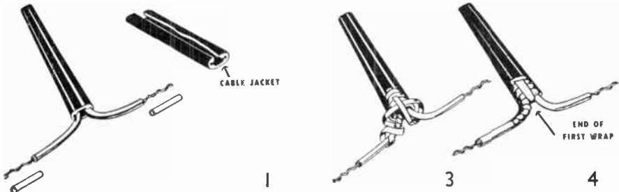
Make a circular cut around, but only partly through the cable jacket 4 inches from the end. Next make a longitudinal cut entirely through the jacket from the initial cut to the end of the cable. The jacket is removed back to the circular cut as shown in step 1.
