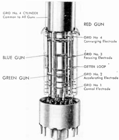
FIG. 37 Electron Gun of Tricolor Tube
