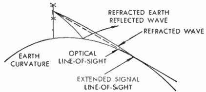
FIG. 357 VHF-UHF Propagation
