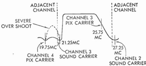
FIG. 316 Response Curve of Stagger-Tuned I-F
