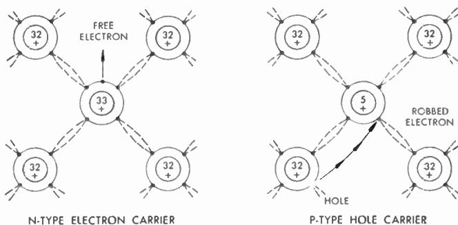
FIG. 419 Electron and Hole-Carriers in Germanium
