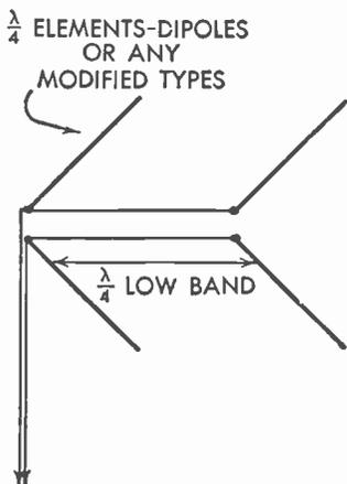
FIG. 256 End-Fire V Antenna
