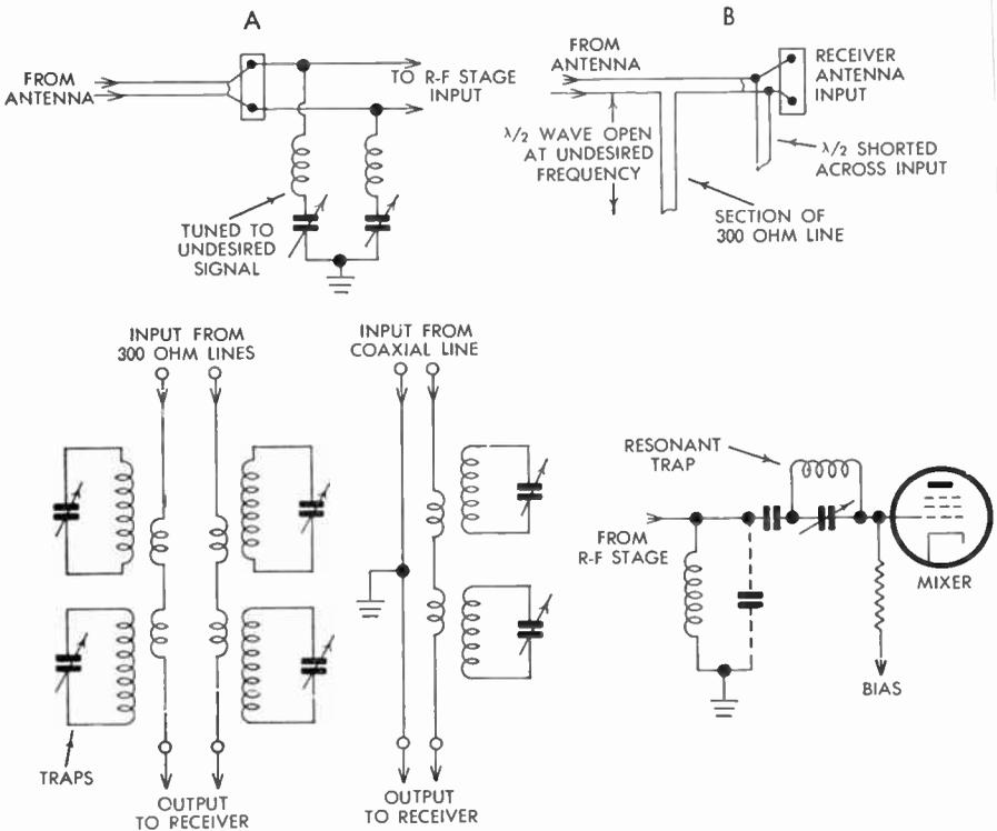
FIG. 291 Input Traps to Remove Spurious Signals
