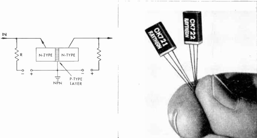
FIG. 421 Junction Transistors, Raytheon CK721 and CK722
