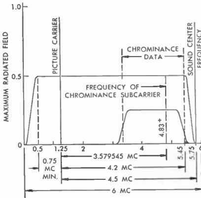
FIG. 15 Idealized Amplitude Characteristic
