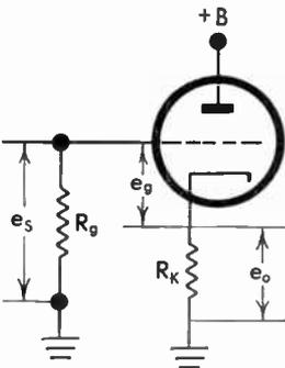
FIG. 341 Reduction in Input Capacity
