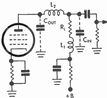
FIG. 334 Series-Shunt Peaking
