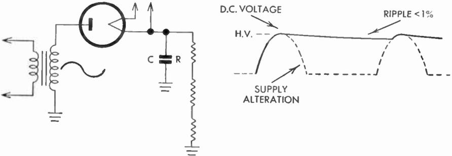
FIG. 348 High-Voltage RC Filtering
