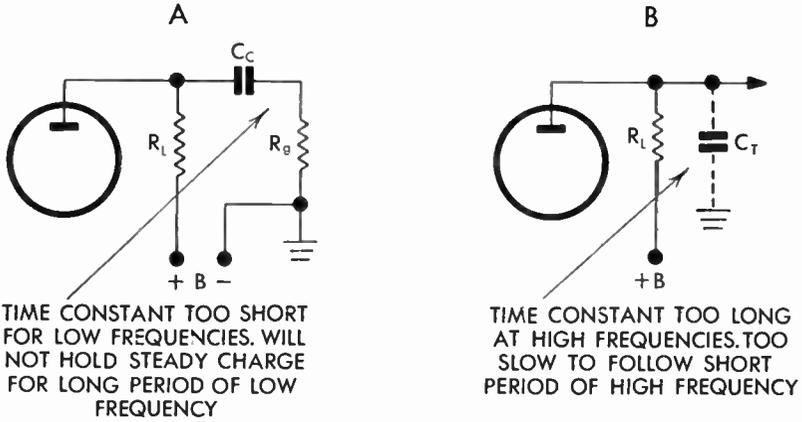
FIG. 346 Time Constant and Sine-Wave Period
