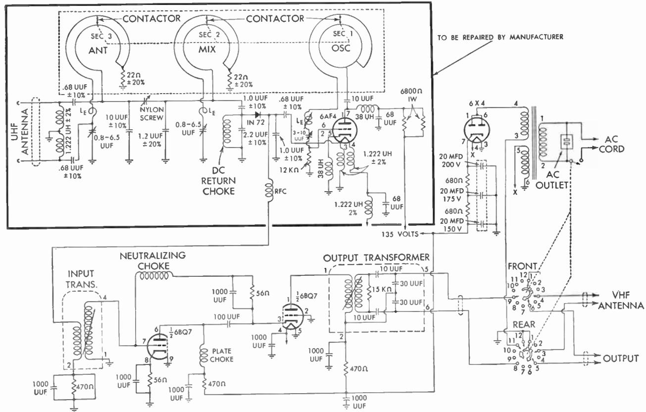
Fig. 391 Schematic, Mallory UHF Converter
