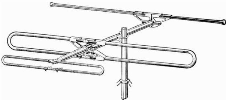
FIG. 255 In-Line Type Antenna \*
