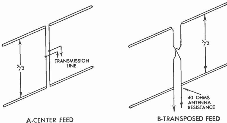
FIG. 245 Stacked Dipoles and Feed Methods
