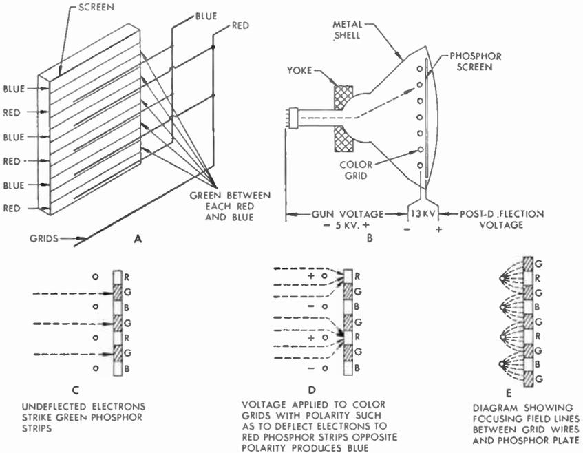
FIG. 41 Plan of Chromatron
