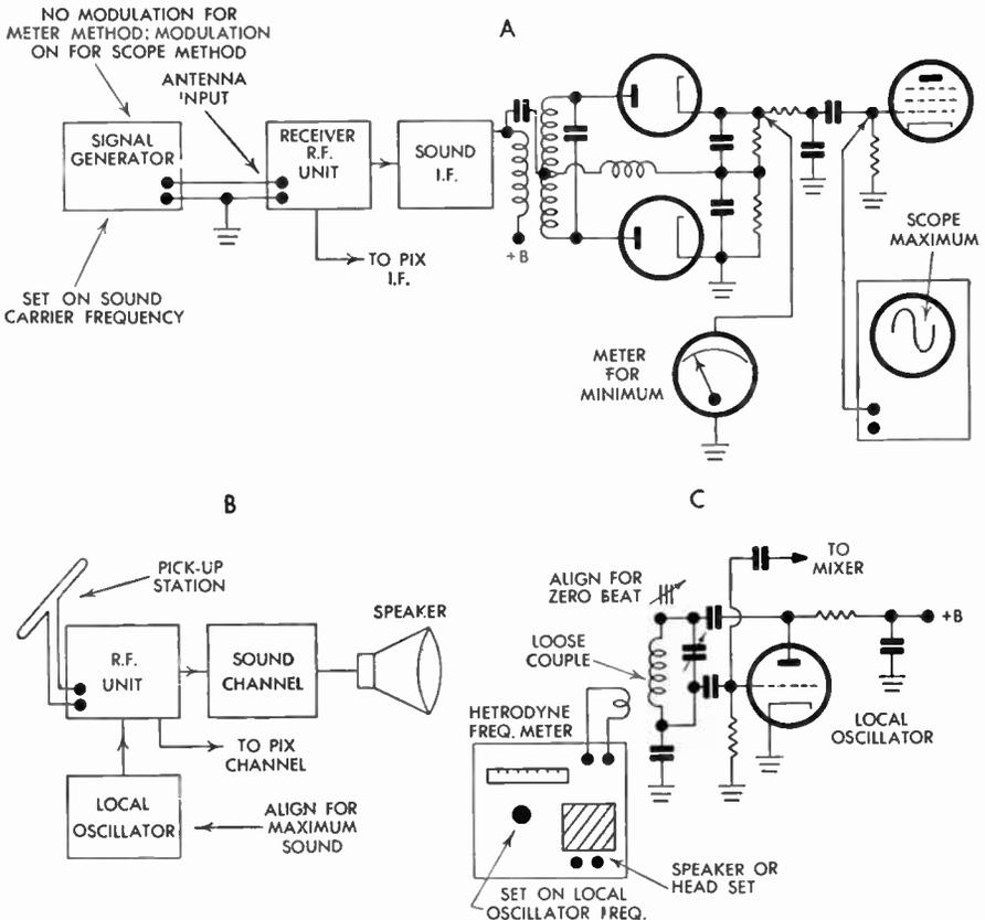
FIG. 311 Local Oscillator Alignment
