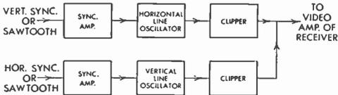
FIG. 321 Block Diagram of Crosshatch Generator
