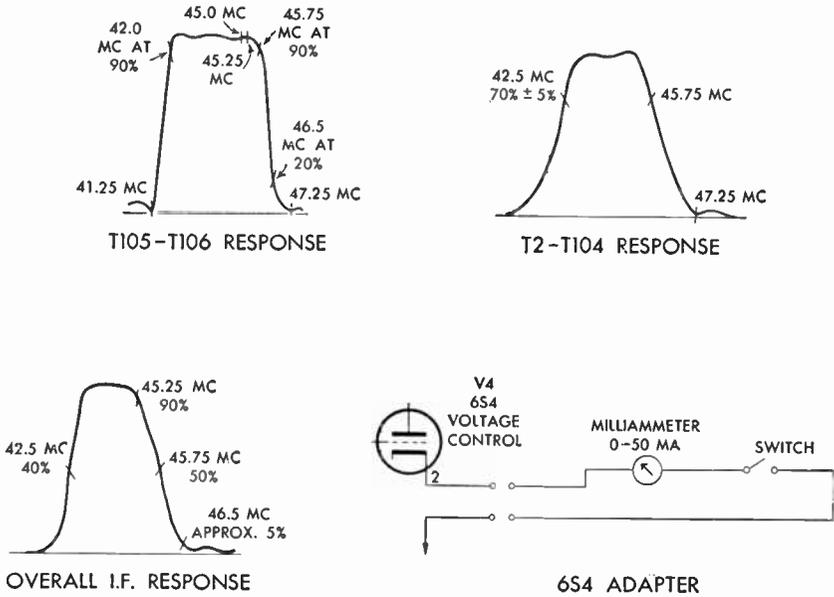
FIG. 325 Alignment Response Curves
