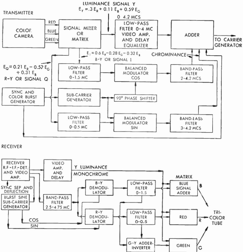
FIG. 14 Functional Block Plan of NTSC Color System
