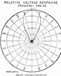
The Yagi is also an excellent UHF antenna but is restricted to operation on a limited number of adjacent channels. It has a high gain and a good directional pattern. Its rather narrow-band sensitivity means it has good noise and interference rejection (rejects image frequencies and many types of beat interference).
