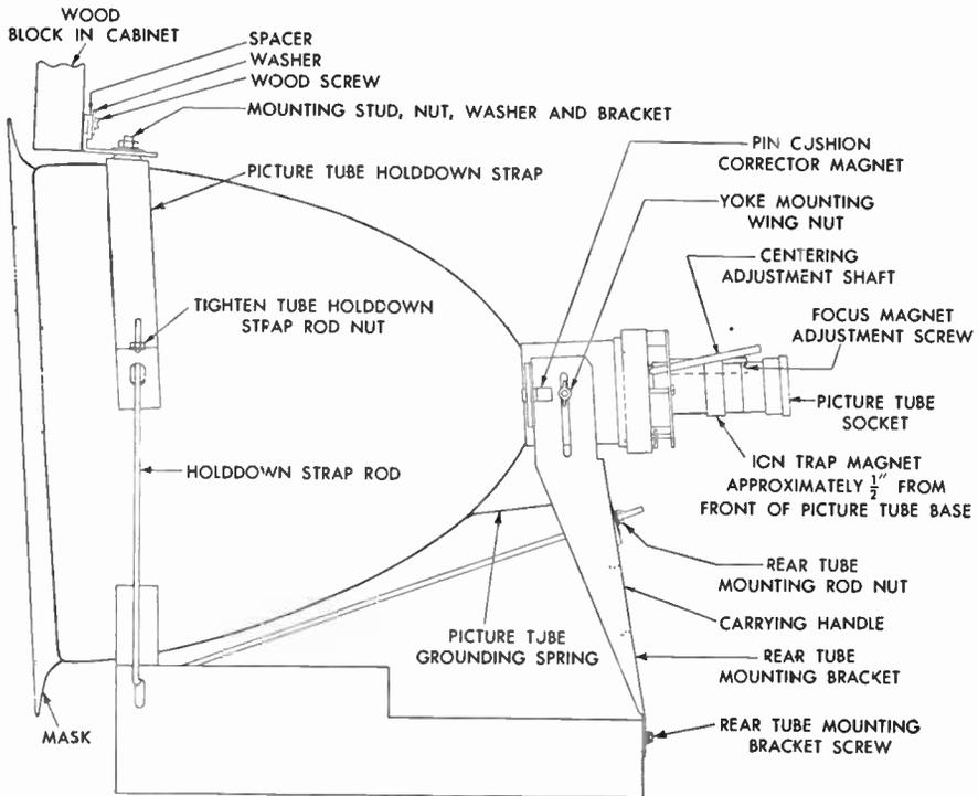
FIG. 276 Sylvania Picture-Tube Mount
