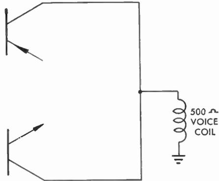
FIG. 424a Transformerless Output
