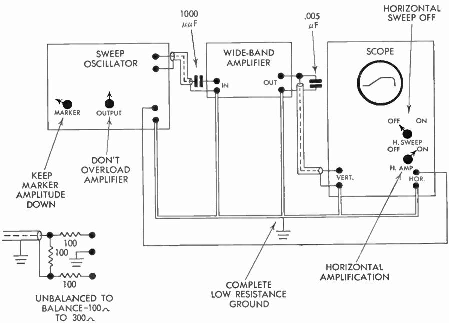
FIG. 305 Interconnection of Units for Sweep Oscillator Alignment
