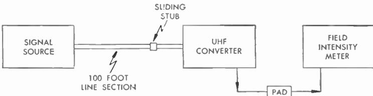
Fig. 410 Transmission-Line Check
