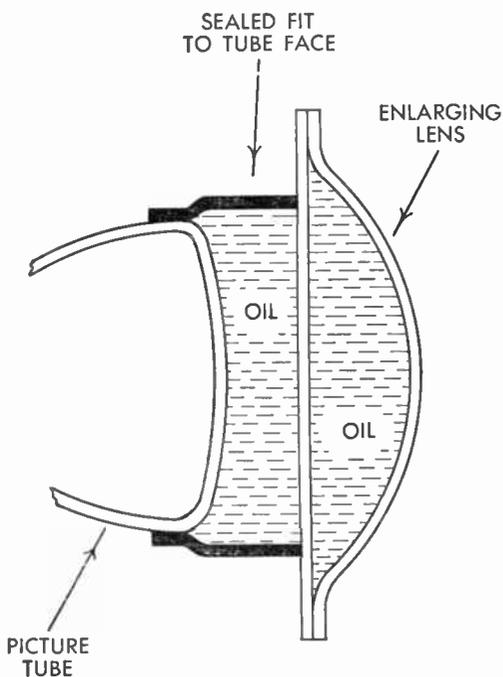
FIG. 210d Lens of Liquid Lens Corporation
