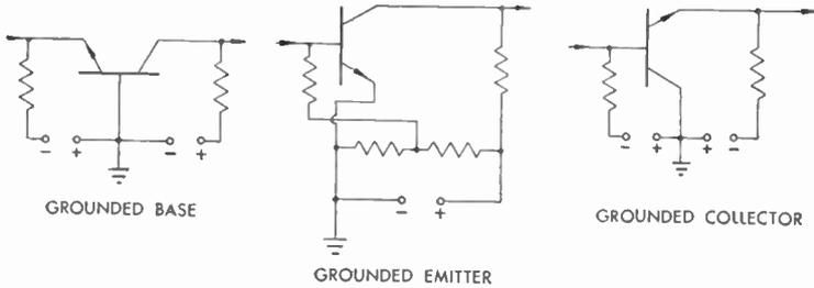
FIG. 422 Basic Transistor Circuits
