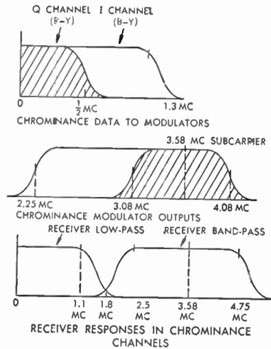
Fig. 25 Bandwidths in the Chrominance Channels
