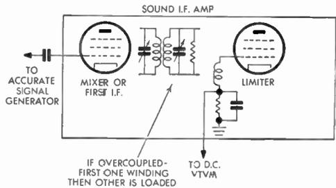
FIG. 308 Meter Alignment of Sound I-F Stages
