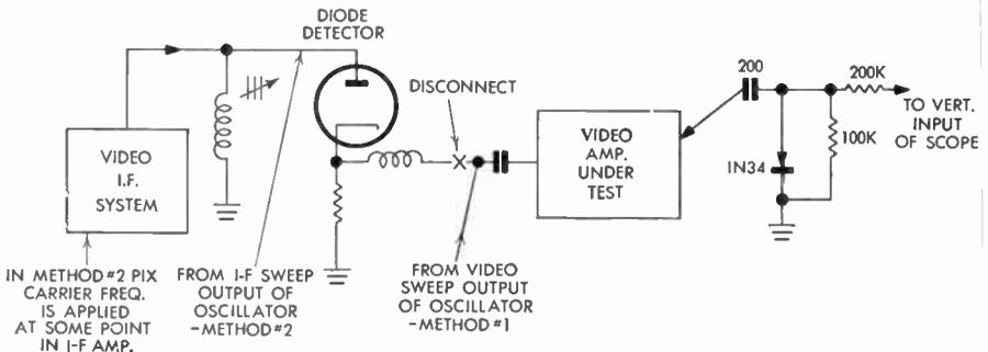
FIG. 319 Video Amplifier Response Using a Video Sweep
