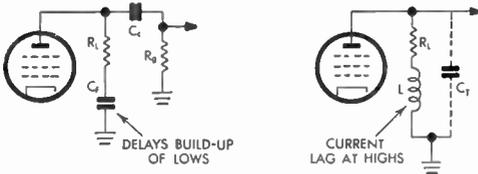
FIG. 337 Phase Correction with Frequency-Compensating Systems
