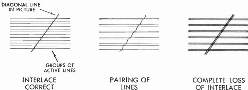
FIG. 271 Effects of Interlace on Diagonal Line
