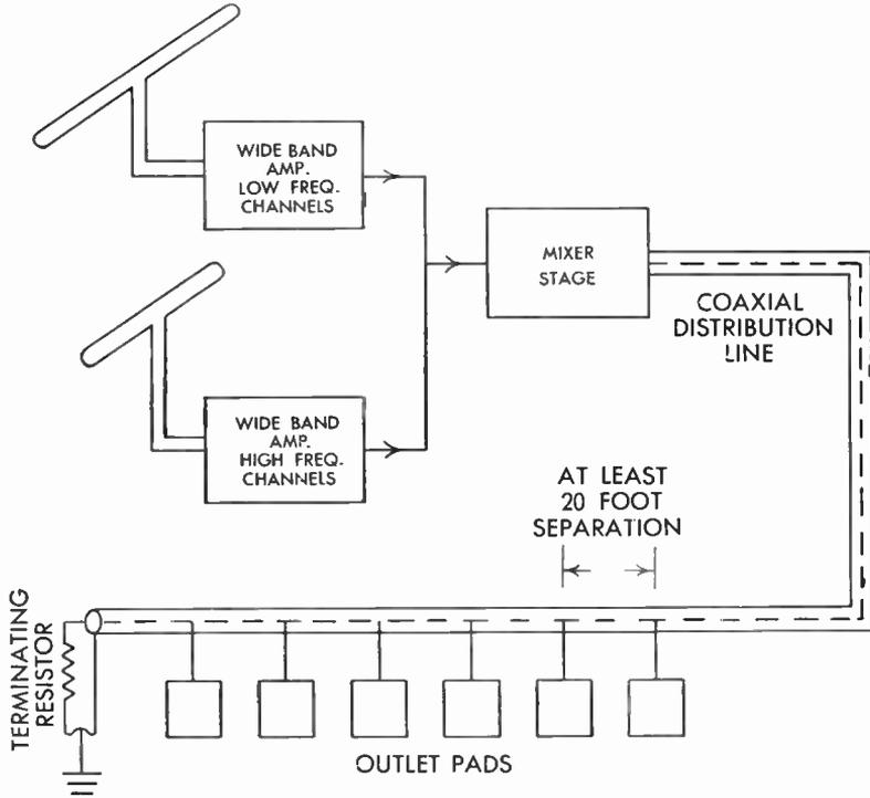
FIG. 268 Receiver Feeding With Outlet System
