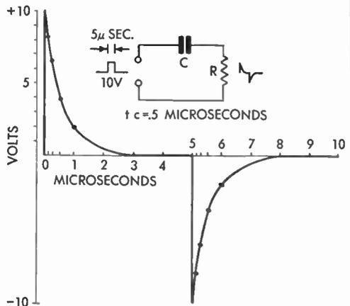
FIG. 350 Voltage across Differentiating Resistor
