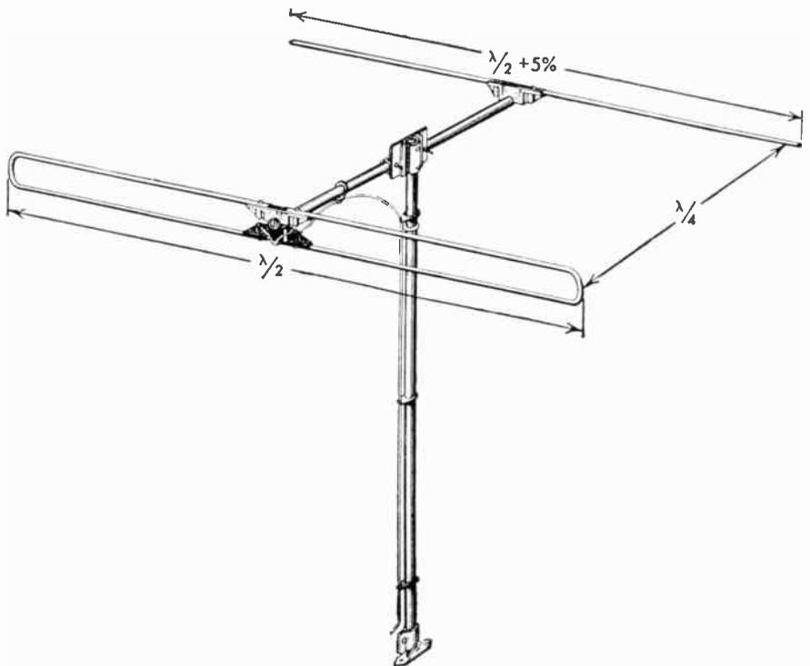
FIG. 250 Ward Folded Dipole and Reflector (Courtesy of The Ward Products Corporation) \*
