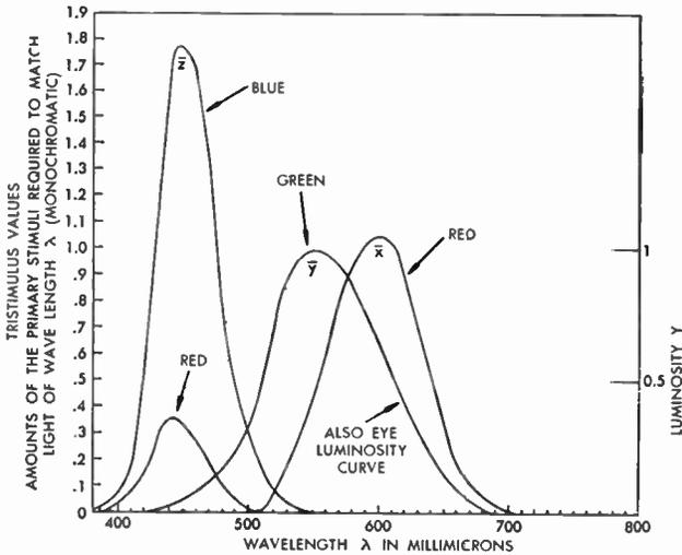
FIG. 2 Standard CIE Color-Mixture Curves
