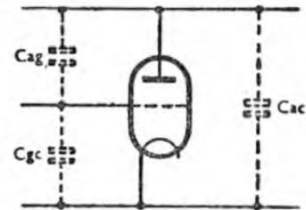
*Miller effect.* (Fig. 105.) The electrodes in a valve have capacitance, which may be expressed as the capacitance between any two electrodes and is called *inter-electrode* capacitance. The effective value of this inter-electrode capacitance is increased because the voltages are amplified on certain electrodes.
