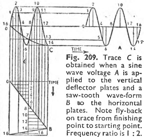
**Fig. 209.** Trace C is obtained when a sine wave voltage A is applied to the vertical deflector plates and a saw-tooth wave-form B to the horizontal plates. Note fly-back on trace from finishing point to starting point. Frequency ratio is 1 : 2.
