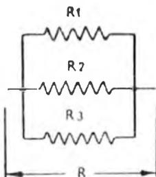
Fig. 4. (Right) Three resistors in parallel.
