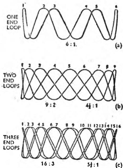
**Fig. 216.** (Left) Figure obtained with phase-splitting circuit. **Fig. 217.** (Right) Frequency ratio determination by examination of peaks and end loops. These are 'flat' patterns obtained when not using phase-splitting circuit.
