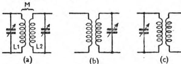
**Fig. 48.** Three forms of tuned high-frequency transformer.
