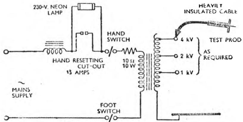
Fig. 87. Circuit for a high-voltage flash tester.
