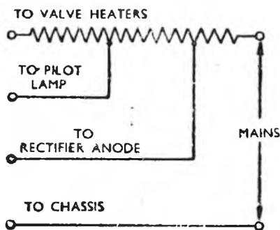
**Fig. 94.** Sometimes line cord resistors are tapped.
