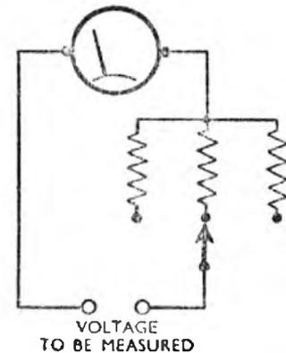
Fig. 194. Three multiplier resistances arranged with a switch to give a triple-range voltmeter.
