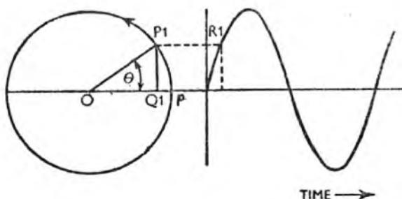
**Fig. 18.** Derivation of a sine curve.
