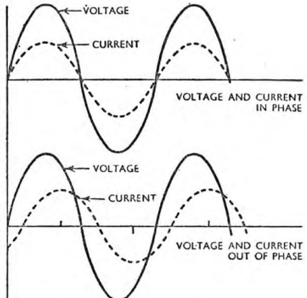
**Fig. 21.** Curves representing voltage and current in phase and out of phase.
