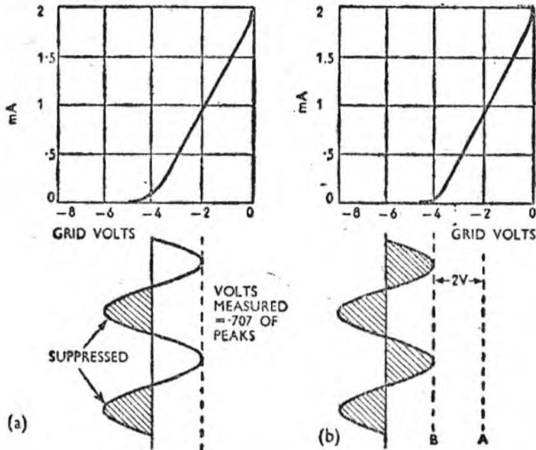
**Fig. 227.** Left (a) Anode-bend valve voltmeter indicates, by the change in anode current, the effective value of the applied AC volts. (b) Peak valve voltmeter indicates (by a voltmeter across the bias supply) the volts necessary to shift the peaks from position A to position B.
