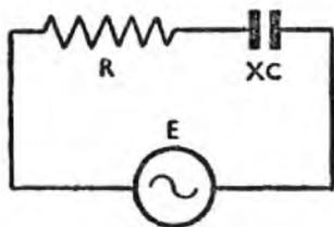
Fig. 24. Resistance and capacitance in series.
