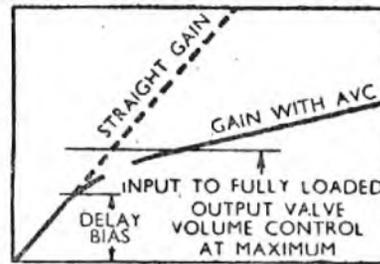
from sharp bends and the possibility of rectification and cross modulation is, therefore, reduced. The main advantage, however, is that the gain of the valve can be controlled by alteration to the grid bias. With a large signal input and a large bias, the mutual conductance is low. With small input and small bias, the gain is high. The valve is an essential part of automatic volume-control circuits.
