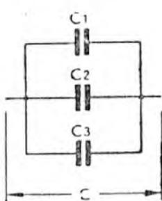
Fig. 9 (Left). Three capacitors in parallel.
