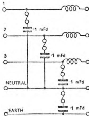
Fig. 169. Filter components for a four-wire mains system.
