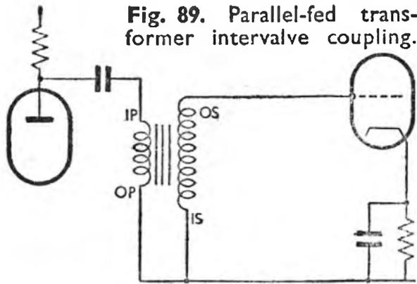
**Fig. 89.** Parallel-fed transformer intervalve coupling.
