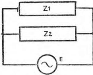
Fig. 43. Alternating voltage applied to impedances in parallel.
