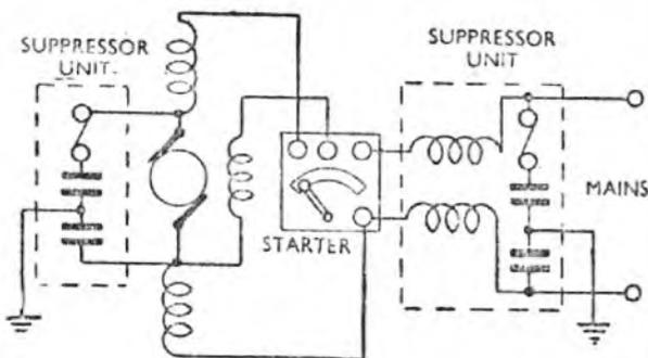
Fig. 168. Suppression applied to motor and starter.
