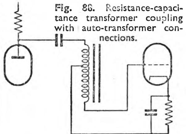
Fig. 88. Resistance-capacitance transformer coupling with auto-transformer connections.
