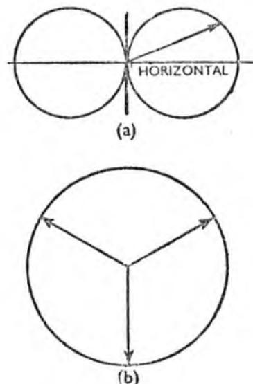
Fig. 236. Directivity curves of vertical dipole in free space. (a) Vertical directivity curve; length of the arrow indicates the intensity of radiation in that direction. (b) Horizontal directivity curve; the dipole radiates equally well in all horizontal directions.
