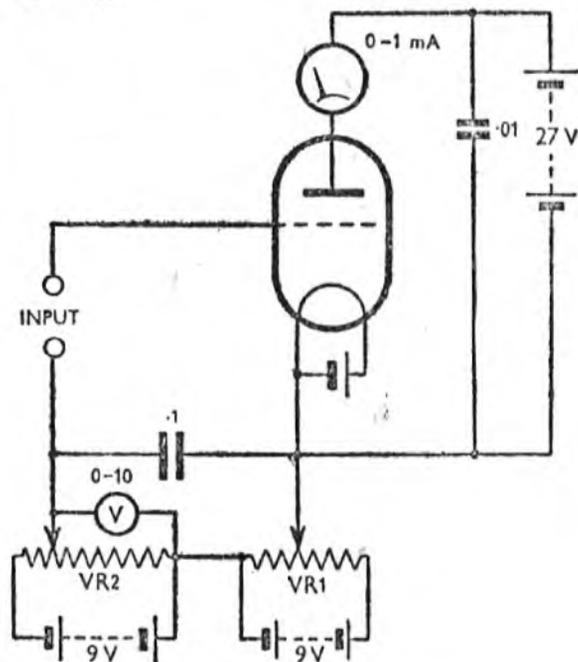
**Fig. 228.** Peak valve voltmeter of the slide-back type. The bias voltmeter  $V$  should be accurate but need not be exceptionally sensitive; 500 or 1,000 ohms-per-volt being suitable.
