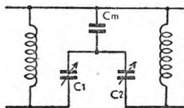
**Fig. 50.** Band-pass circuit with common capacitance  $C_m$  for transference of signal.
