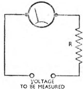
Fig. 193. Multiplier resistance  $R$  limits the current to the maximum that meter can carry.
