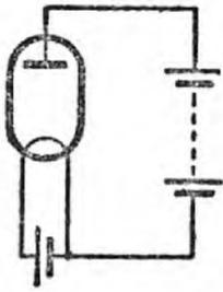
Fig. 98. Diode valve with filament and anode batteries.
