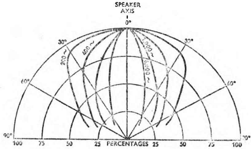
Fig. 189. Polar curves of typical projector loudspeaker.
