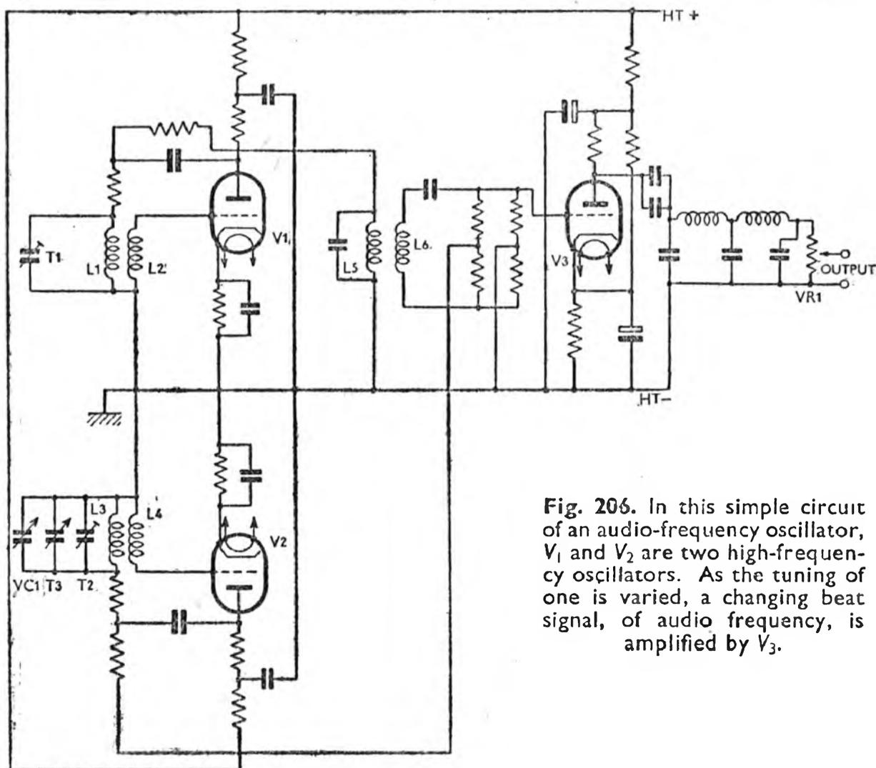
**Fig. 206.** In this simple circuit of an audio-frequency oscillator,  $V_1$  and  $V_2$  are two high-frequency oscillators. As the tuning of one is varied, a changing beat signal, of audio frequency, is amplified by  $V_3$ .
