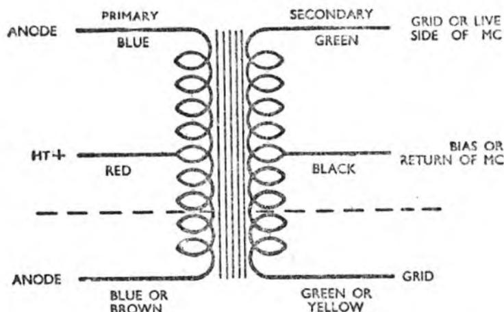
Fig. 166. Colour coding for output and intervalve transformers.
