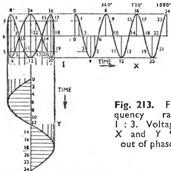
**Fig. 213.** Frequency ratio 1 : 3. Voltages X and Y 90° out of phase.
