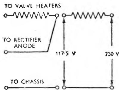
**Fig. 93.** An extra line cord is needed when U.S. midget sets are used on mains of over 117.5 volts.
